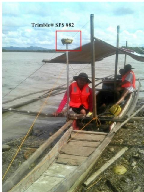
Figure 50. Bathymetric survey set-up using OHMEX™ single beam echo sounder and a mounted with Trimble® SPS 882
