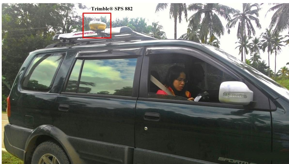
Figure 48. Validation points acquisition survey setup: A Trimble® SPS 882, mounted on top of the vehicle
