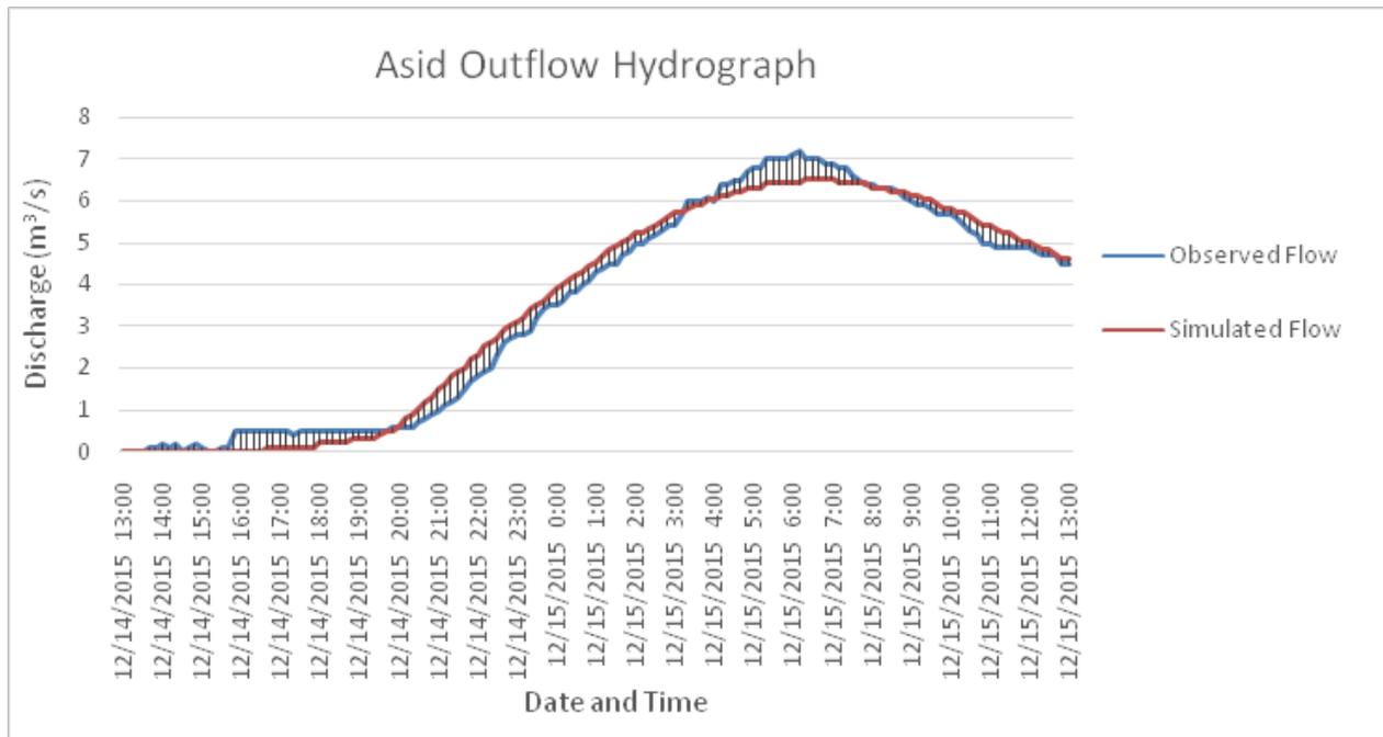
Figure 64. Outflow hydrograph of Asid River Basin produced by the HEC-HMS model compared with observed outflow
