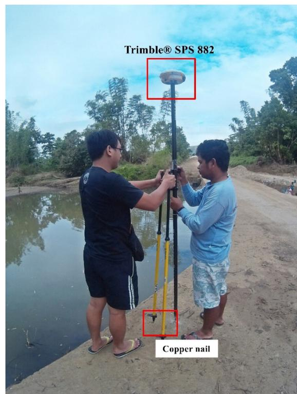
Figure 41. Trimble® SPS 882 setup at UP-ALA, an established control point located at Alas Bridge in Brgy. Alas, Mandaon, Masbate
