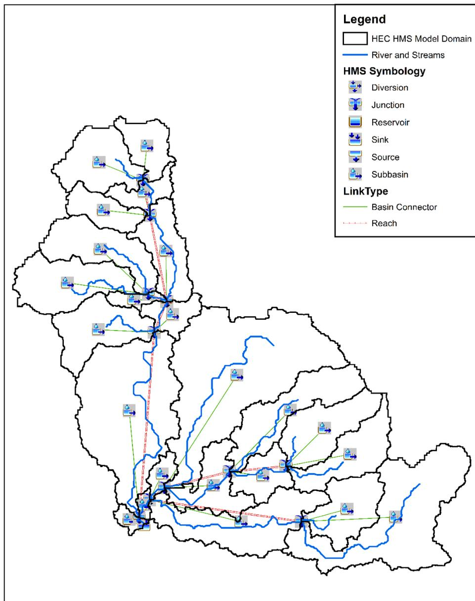
Figure 62. The Asid River Basin model generated in HEC-HMS
