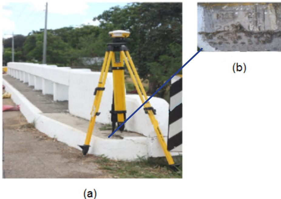
Figure 3. a) GPS set-up over MST-28 as recovered in Mambog Bridge, Barangay Bat-ongan, municipality of Mandaon, Masbate. b) NAMRIA reference point MST-28 as recovered by the field team.
