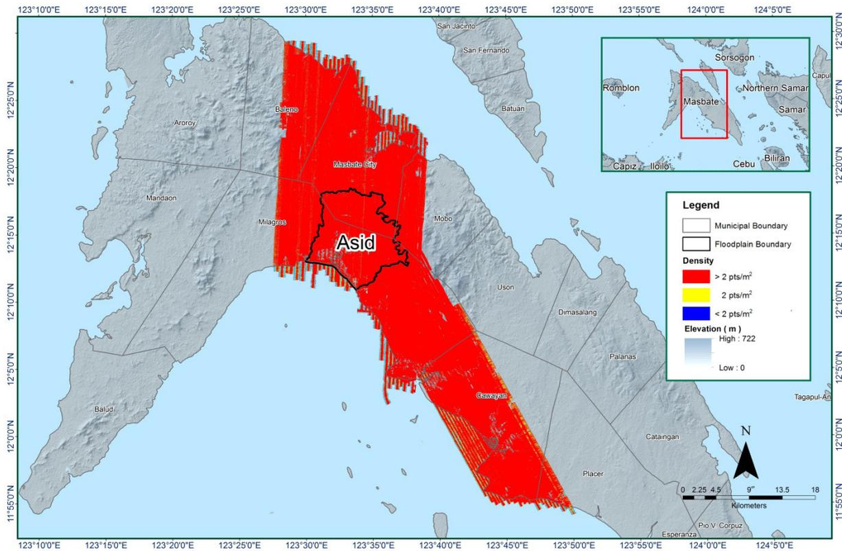
Figure 20. Density map of merged LiDAR data for Asid Floodplain.
