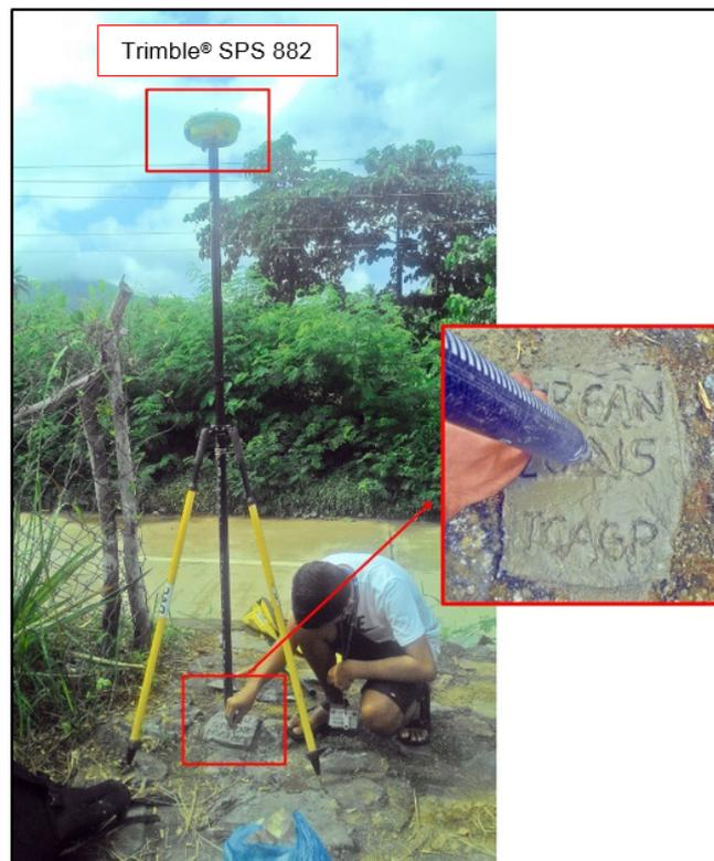
Figure 43. GNSS receiver setup, Trimble® SPS 882, at UP-GAN, an established control point located on the top of a riprap near Gangao Bridge, along Central Nautical Highway, Brgy. Gangao, Baleno, Masbate
