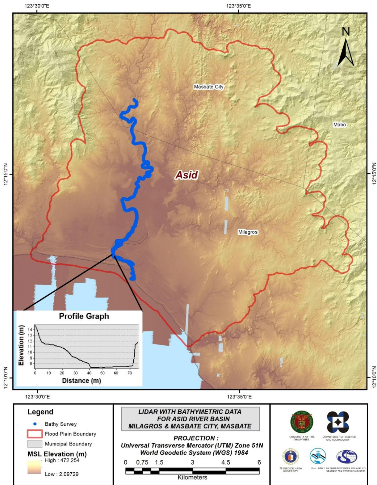
Figure 33. Map of Asid Flood Plain with bathymetric survey points shown in blue.
