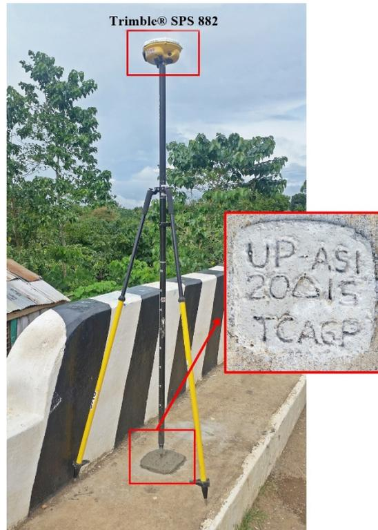
Figure 42. GNSS receiver setup, Trimble® SPS 882, at UP-ASI, an established control point located at Asid Bridge, along Central Nautical Highway, Brgy. Asid, Masbate City
