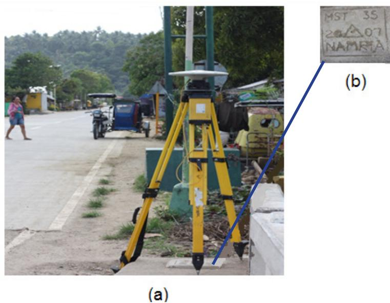
Figure 7. a) GPS set-up over MST-35 as recovered in Marcella Bridge in Brgy. Cagay, City of Masbate, Province of Masbate b) NAMRIA reference point MST-35 as recovered by the field team.
