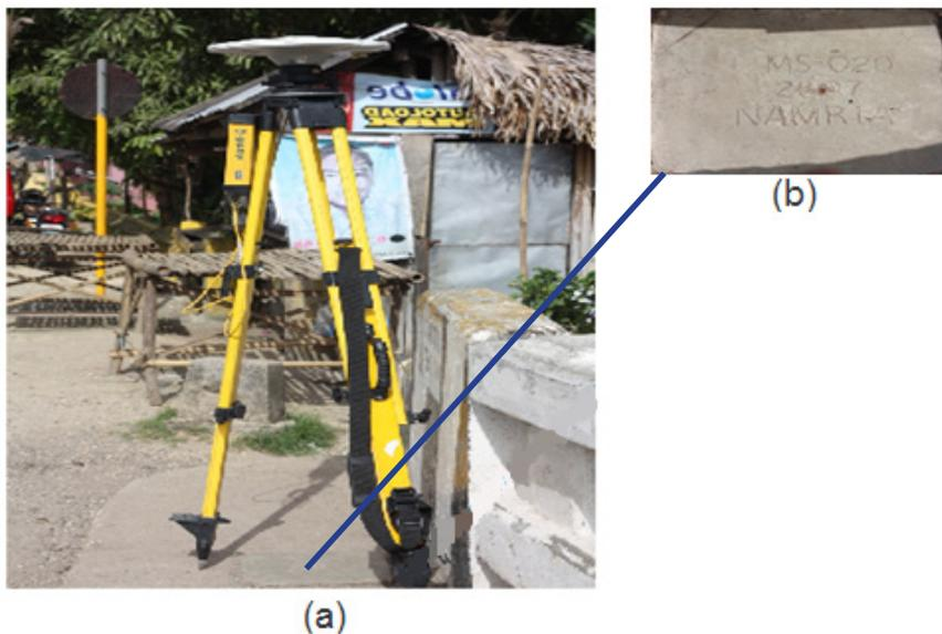
Figure 11. a) GPS set-up over MS-20 as recovered in Manaswang Bridge in Brgy. Marcella, Municipality of Uson, Masbate b) NAMRIA reference point MS-20 as recovered by the field team.
