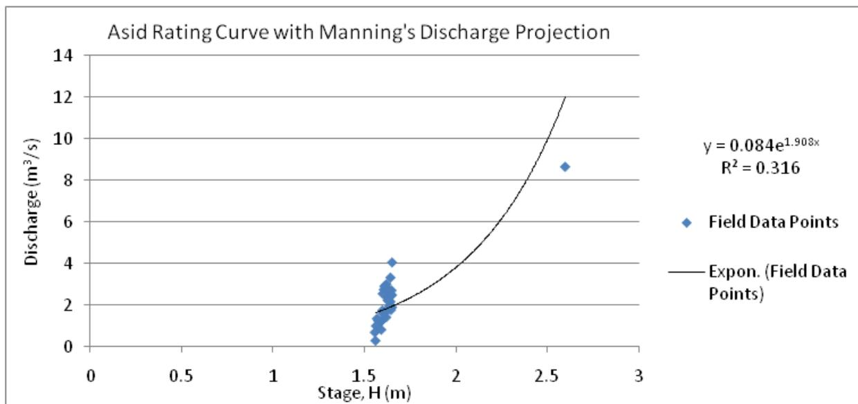
Figure 57. Rating Curve at Asid Bridge, Masbate City
