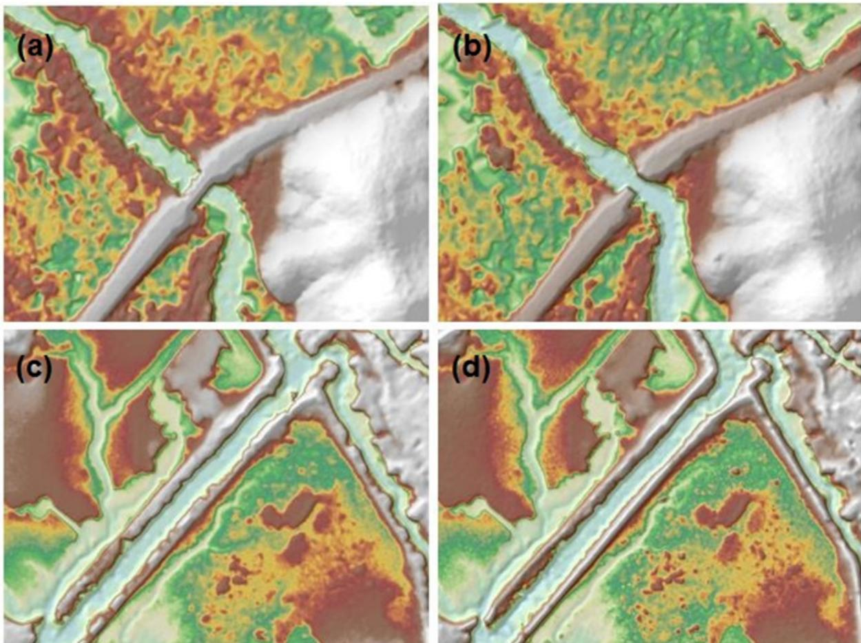
Figure 28. Portions in the DTM of Asid Floodplain – a bridge before (a) and after (b) manual editing; and an embankment before (c) and after (d) data retrieval
