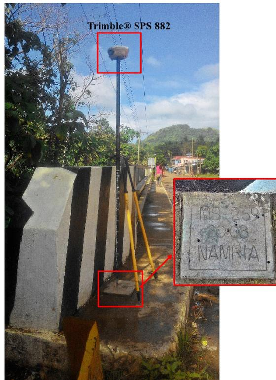
Figure 38. GNSS base set up, Trimble® SPS 852 at MS-269 benchmark located at Lanang Bridge, along Central Nautical Highway in Brgy. Luy-A, Aroroy, Masbate
