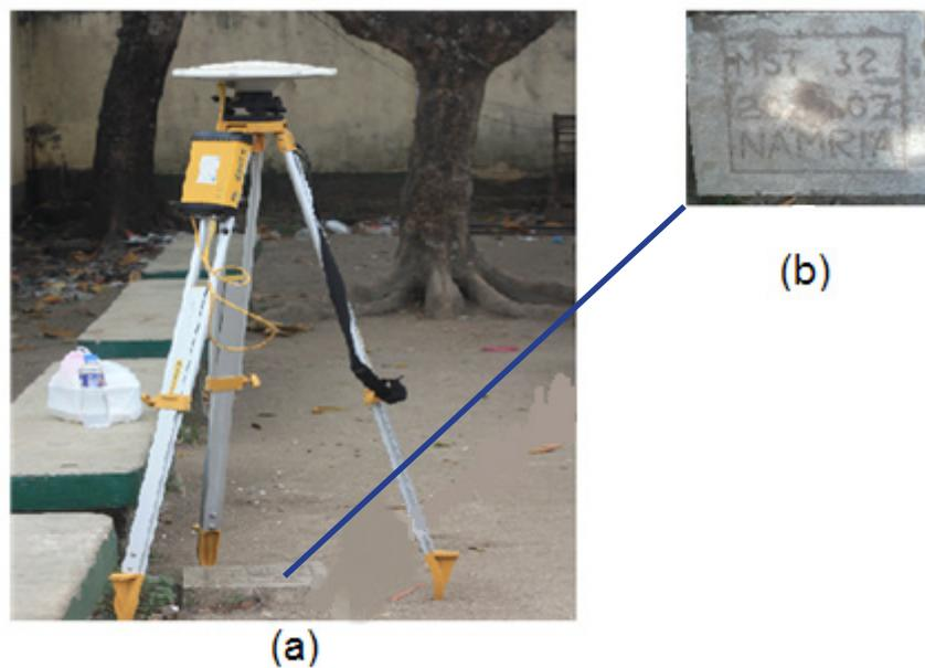
Figure 5. a) GPS set-up over MST-32 as recovered inside the compound of Milagros Municipal Hall, Masbate. b) NAMRIA reference point MST-32 as recovered by the field team.
