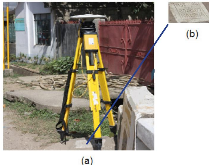
Figure 8. a) GPS set-up over MST-40 as recovered in Buenavista Bridge in Brgy. Buenavista, Municipality of Uson, Masbate. b) NAMRIA reference point MST-40 as recovered by the field team.
