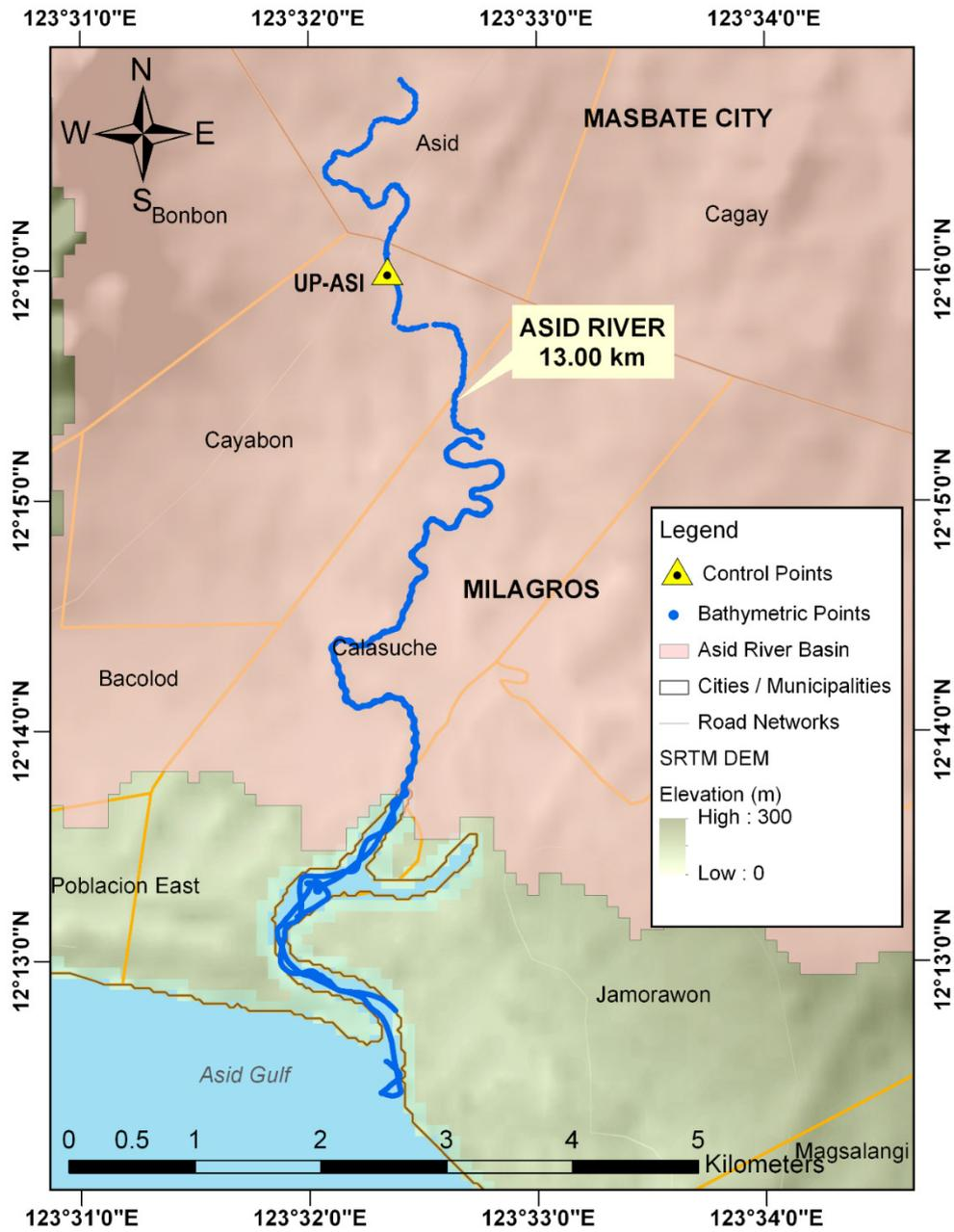
Figure 52. Bathymetric survey along Asid River
