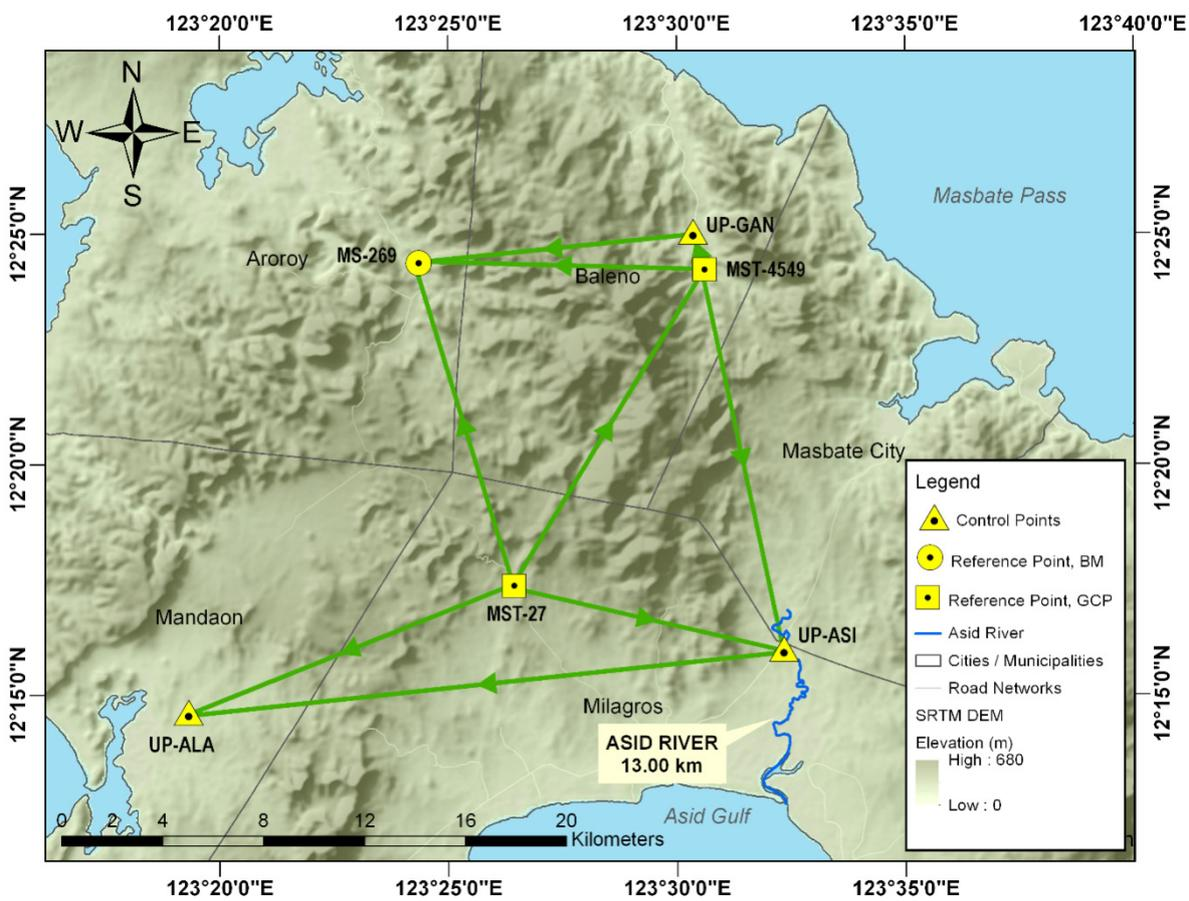
Figure 37. GNSS Network of Asid River field survey
