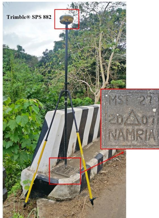
Figure 39. GNSS receiver set up, Trimble® SPS 882 at MST-27, a second order GCP located at Mabuaya Bridge along Central Nautical Highway in Brgy. Matiporon, Milagros, Masbate
