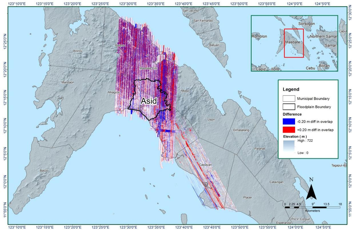
Figure 21. Elevation difference map between flight lines for Asid Floodplain.
