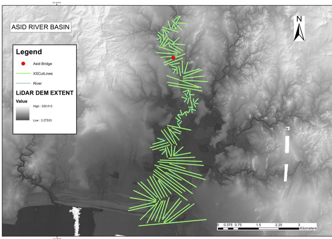
Figure 63. River cross-section of Asid River generated through Arcmap HEC GeorAS tool
