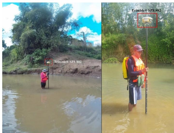
Figure 51. Manual bathymetry in Asid River
