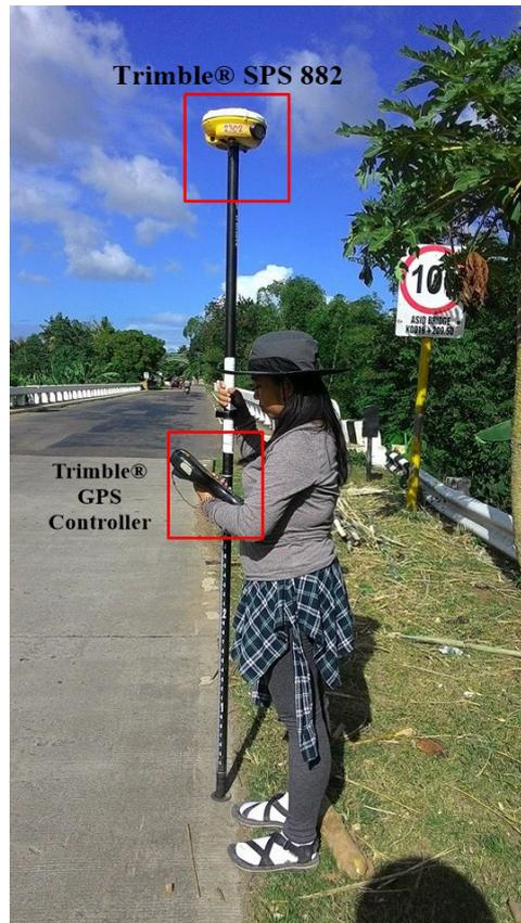
Figure 44.As-built survey using Trimble® SPS 882
