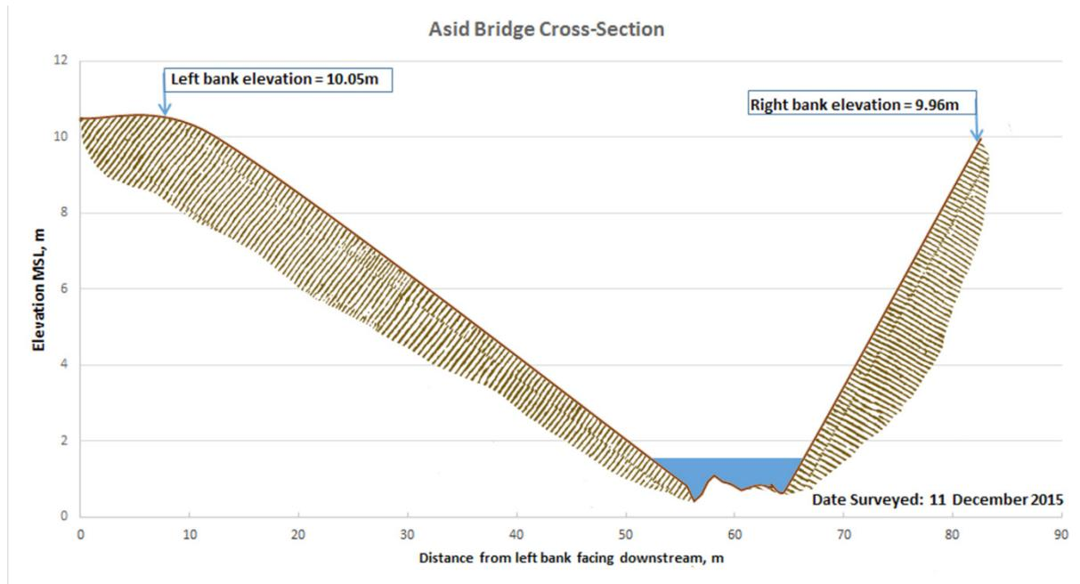
Figure 56. Cross-Section Plot of Asid Bridge
