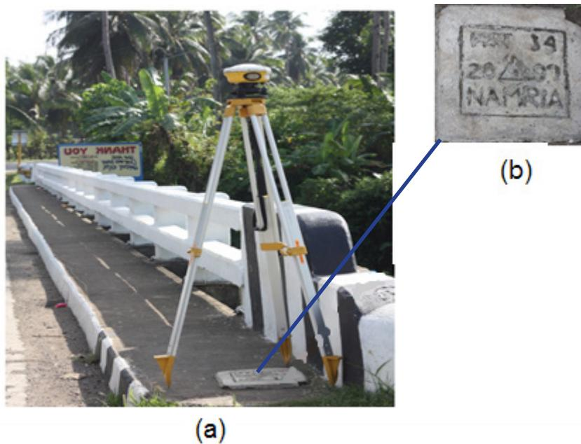
Figure 6. a) GPS set-up over MST-34 as recovered in Sagawsawan Bridge, Brgy. Umabay Exterior, municipality of Mobo, Masbate b) NAMRIA reference point MST-34 as recovered by the field team.
