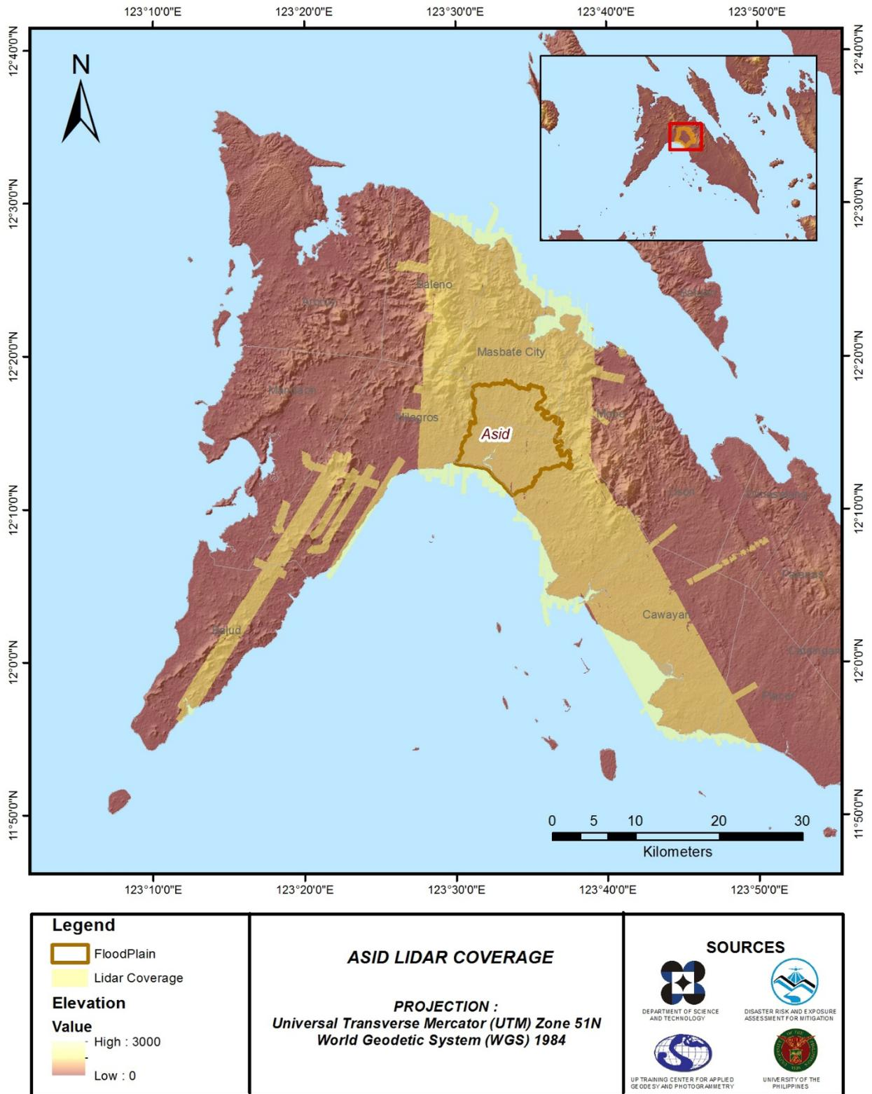
Figure 13. Actual LiDAR survey coverage for Asid floodplain.
