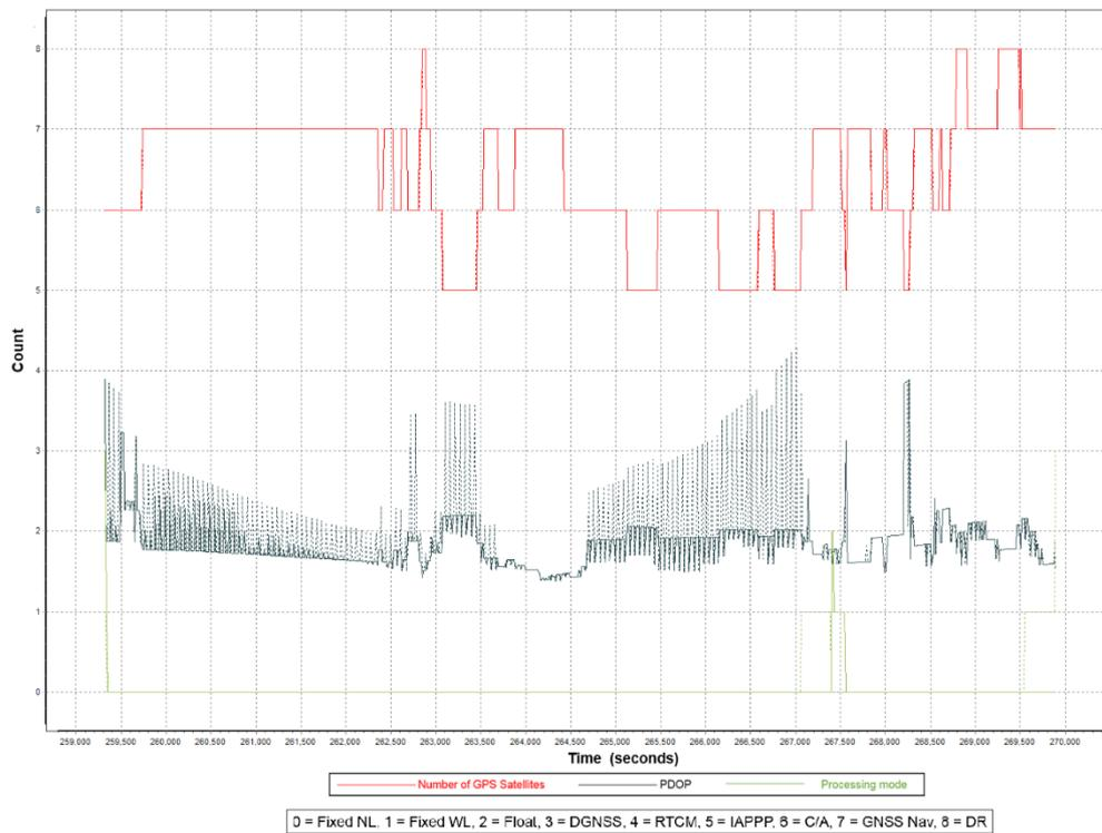
Figure 16. Solution Status Parameters of Asid Flight 1295P.
