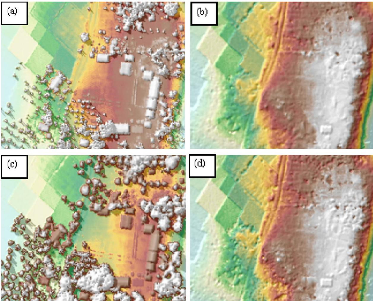
Figure 25. The Production of last return DSM (a) and DTM (b), first return DSM (c) and secondary DTM (d) in some portion of Asid floodplain.
