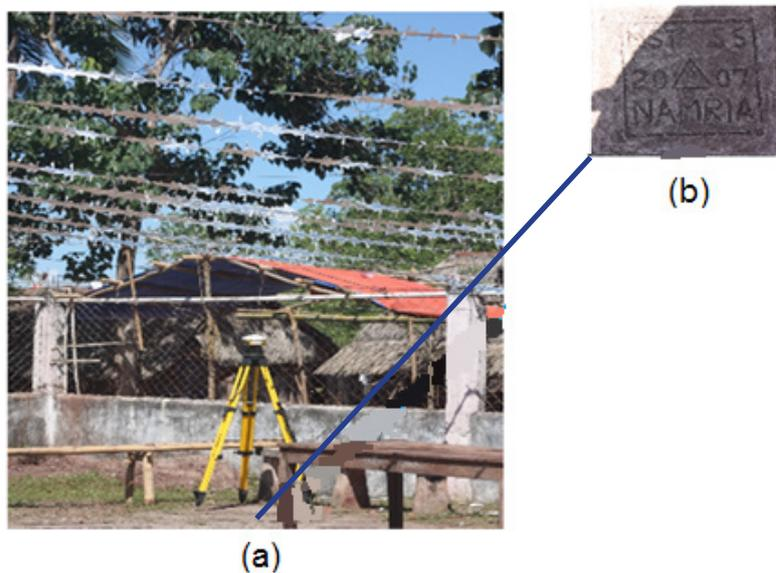
Figure 10. a) GPS set-up over MST-55 as recovered inside the compound of Casamongan Brgy. Hall, Municipality of Balud, Masbate. b) NAMRIA reference point MST-55 as recovered by the field team.
