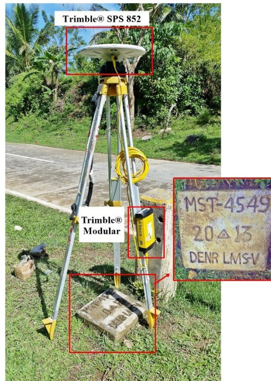
Figure 40. Trimble® SPS 852 base setup at MST-4945, a DENR-established control point located at the approach of Cancahorao Bridge along Central Nautical Highway in Brgy. Gangao, Baleno, Masbate
