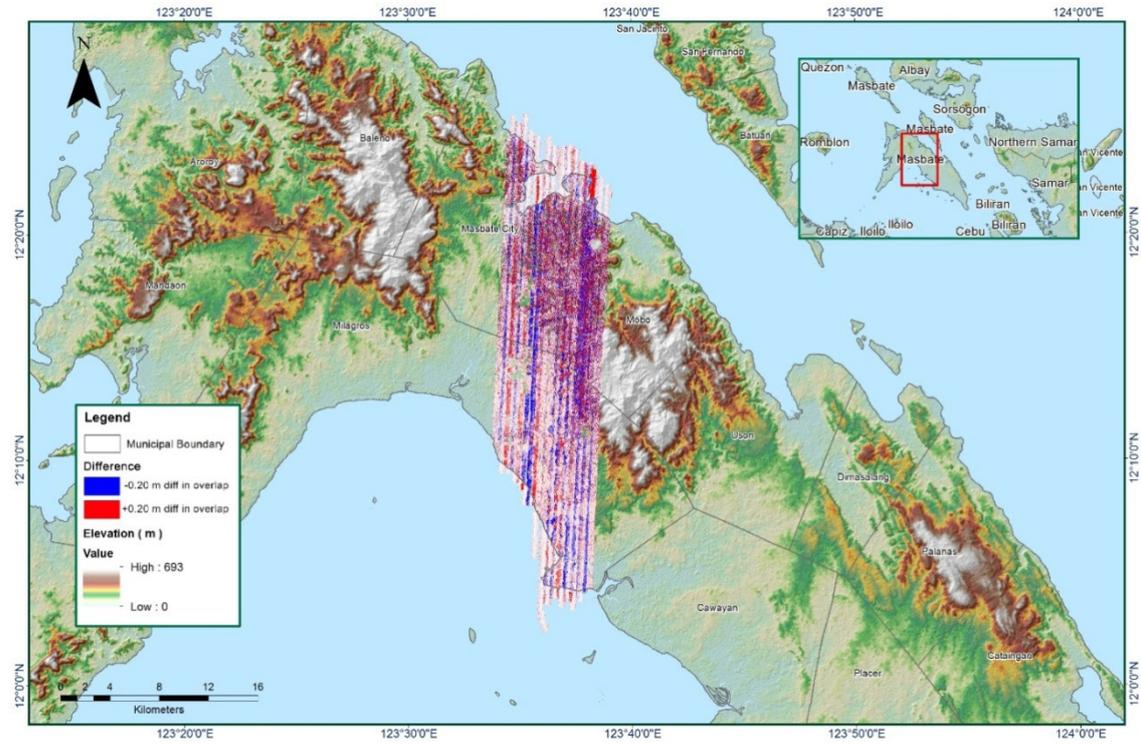
Figure A-8.21 Elevation difference between flight lines
