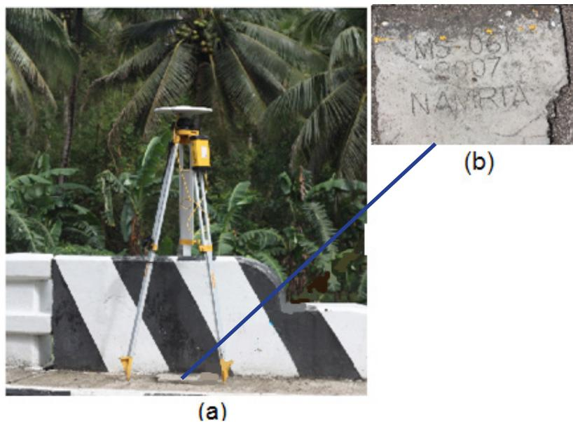
Figure 12. a) GPS set-up over MS-61 as recovered in Nabangig Bridge, Brgy. Nabangig, Municipality of Palanas, Masbate b) NAMRIA reference point MS-61 as recovered by the field team.
