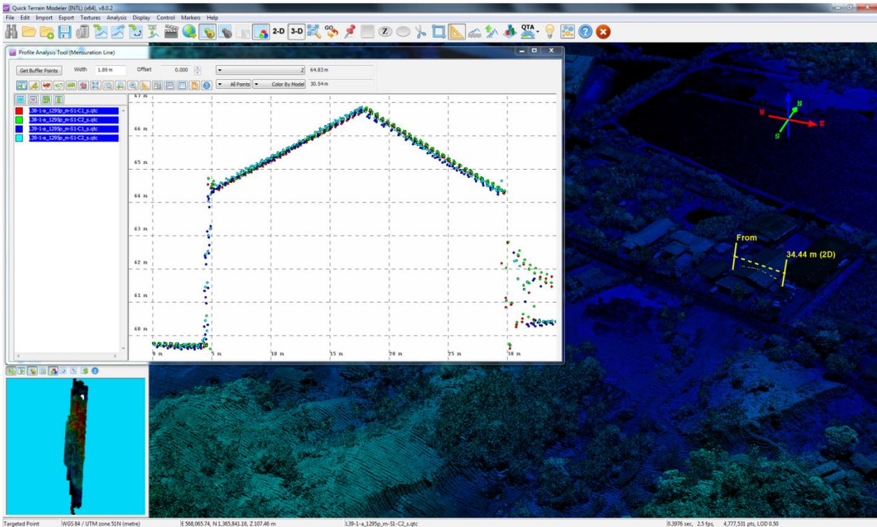
Figure 22. Quality checking for Asid flight 1295P using the Profile Tool of QT Modeler.
