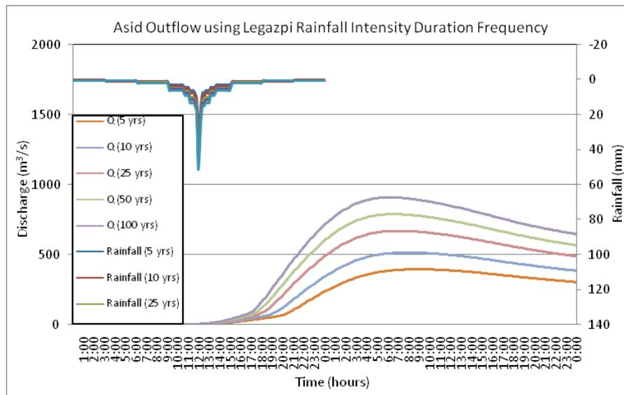
Figure 65. The outflow hydrograph at Asid Basin, generated using the simulated rain events for 24-hour period for Legazpi station
