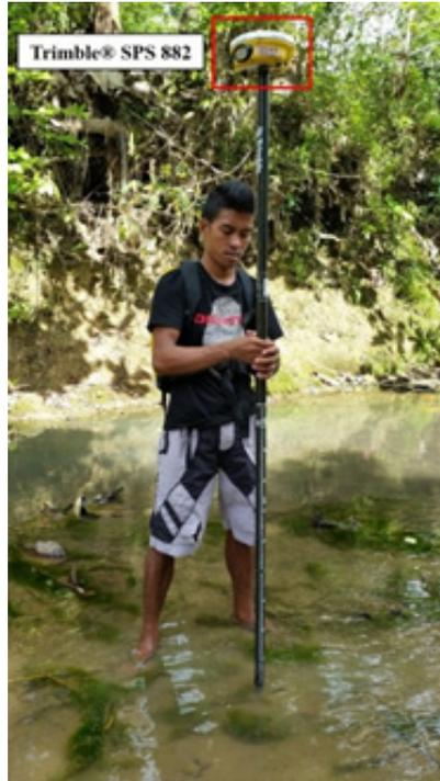
Figure 49. Setup of Trimble® SPS 882 receiver on a range pole for the manual bathymetric survey in Baleno River
