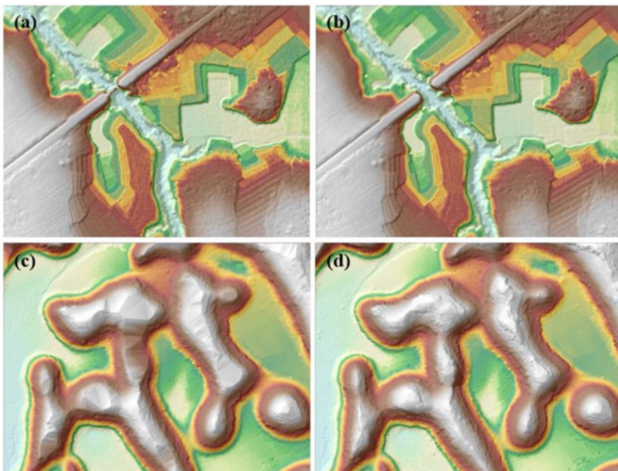
Figure 23. Portions in the DTM of Baleno floodplain – a bridge before (a) and after (b) manual editing; a misclassified hill before (c) and after (d) data retrieval.
