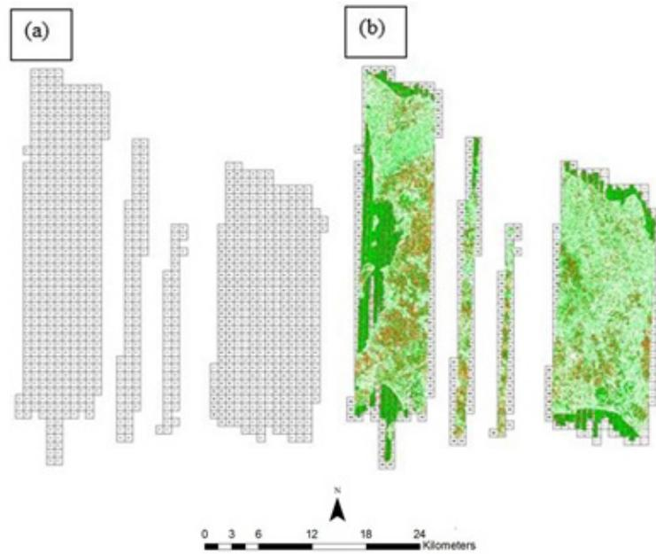
Figure 18. Tiles for Baleno floodplain (a) and classification results (b) in TerraScan.
