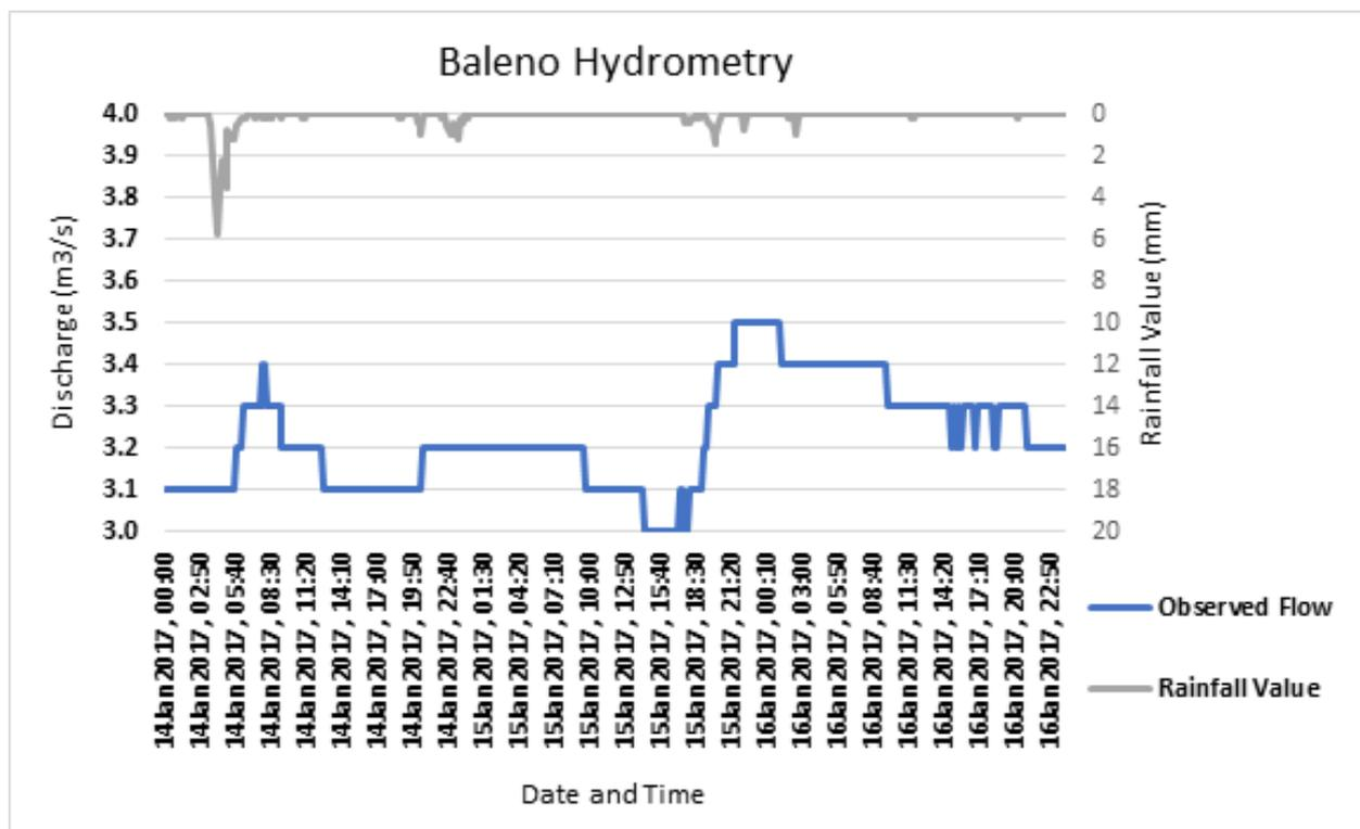
Figure 57. Rainfall and outflow data of the Baleno River Basin, which was used for modeling
