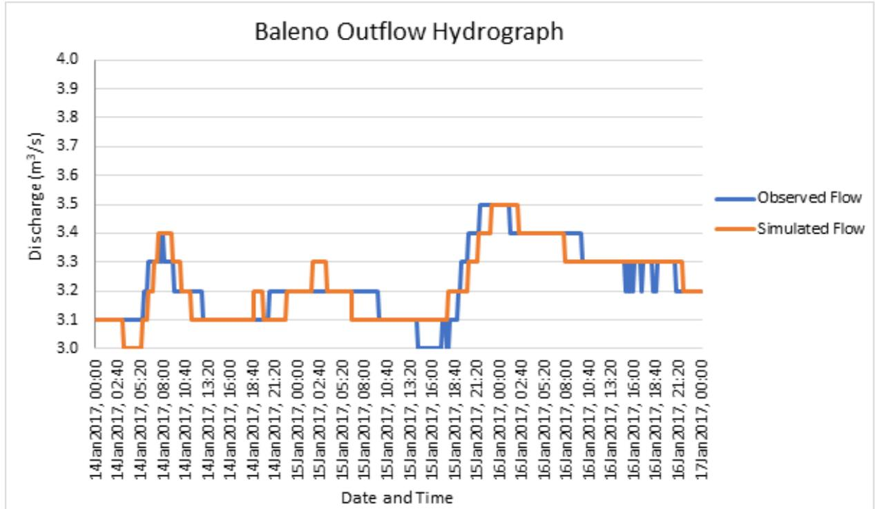
Figure 67. Outflow hydrograph of Baleno River Basin produced by the HEC-HMS model compared with observed outflow
