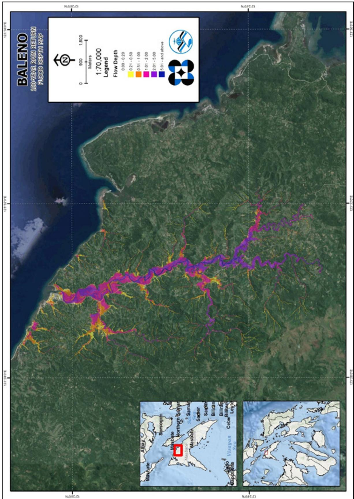
Figure 71. 100-year flow depth map for the Baleno flood plain overlaid on Google Earth imagery
