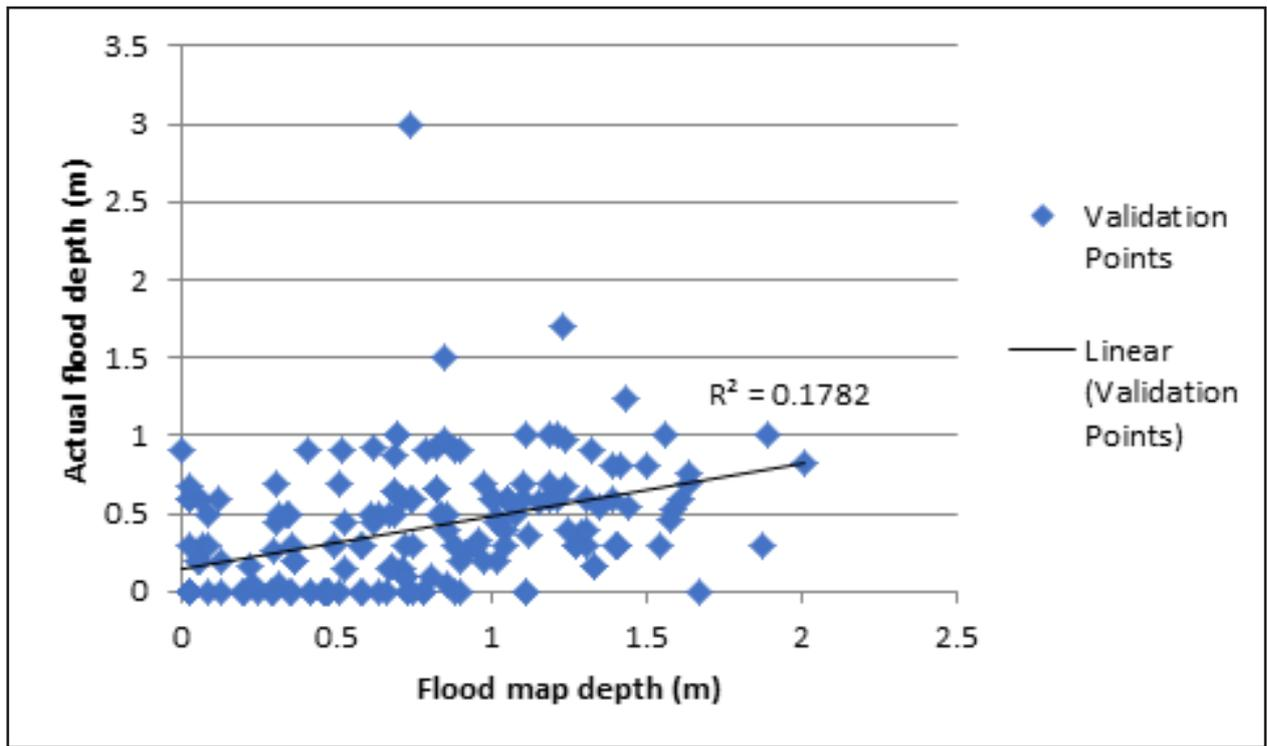
Figure 83. Flood map depth vs. Actual flood depth
