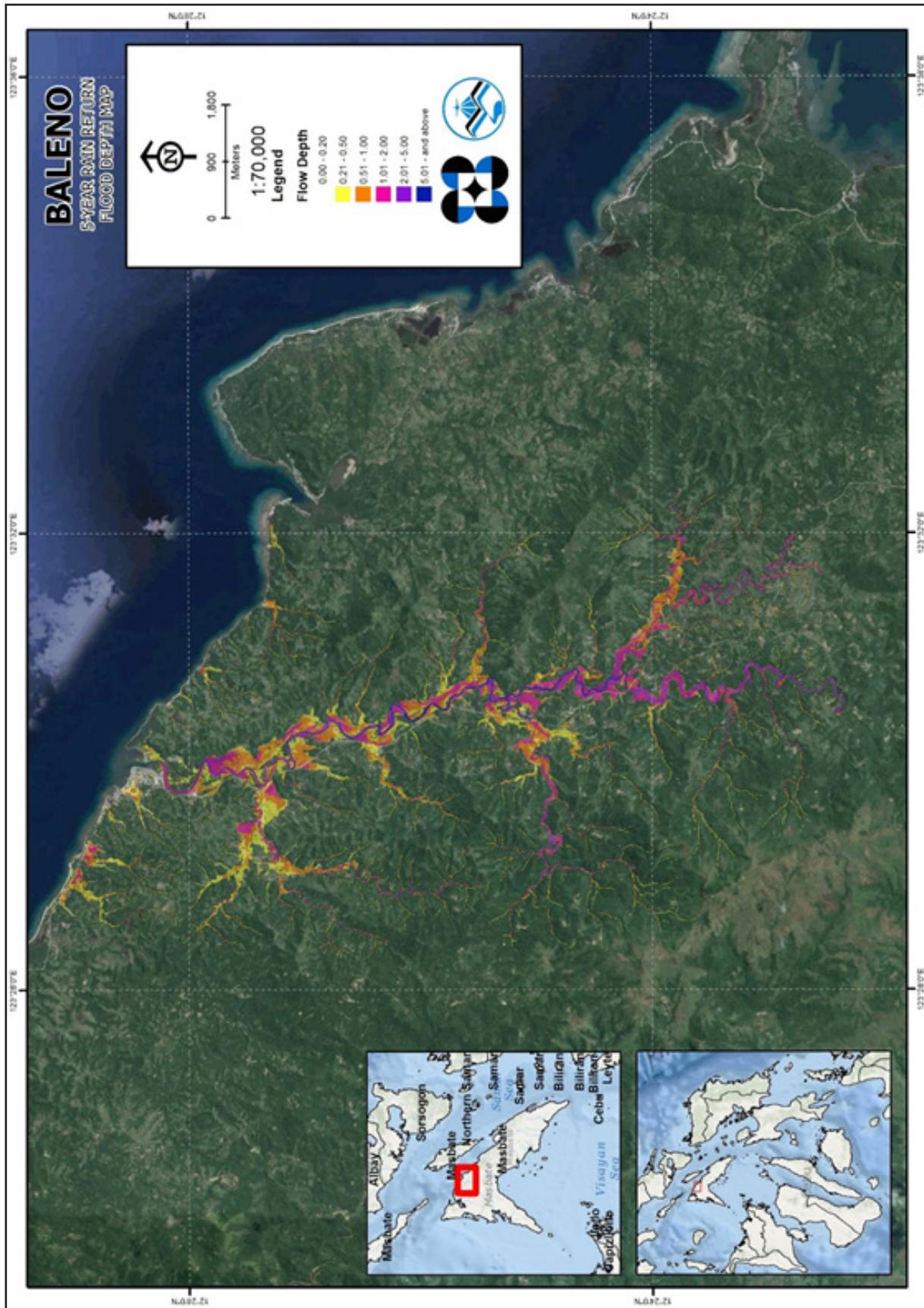
Figure 75. 5-year flow depth map for the Baleno flood plain overlaid on Google Earth imagery
