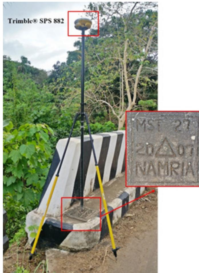
Figure 33. GNSS receiver set up, Trimble® SPS 852 at MST-27, located at Mabuaya Bridge along Central Nautical Highway in Brgy. Matiporon, Milagros, Masbate
