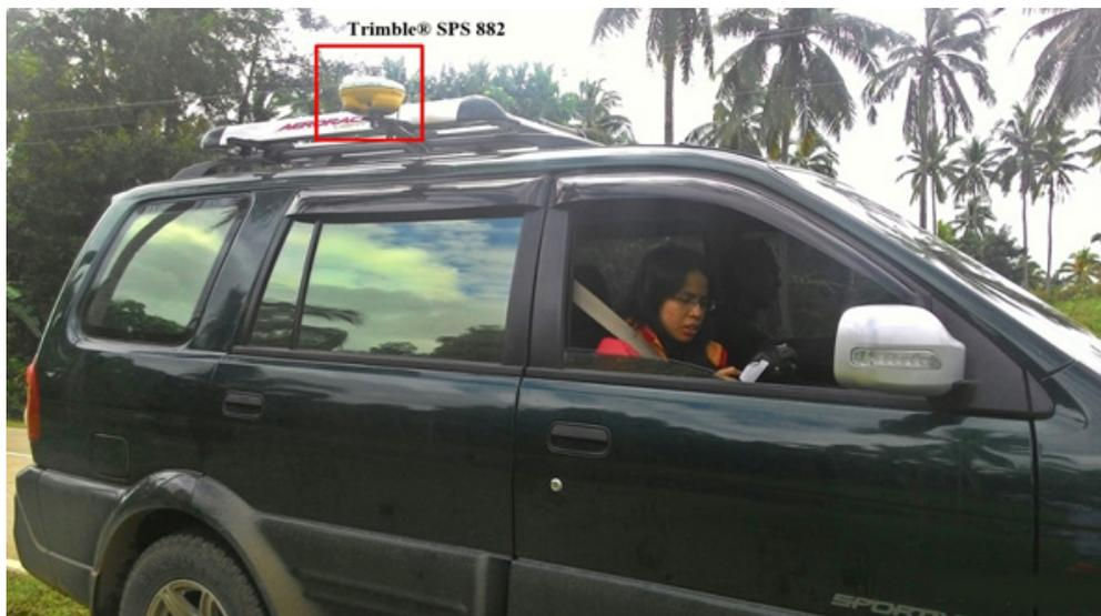
Figure 47. Validation points acquisition survey setup: A Trimble® SPS 882, mounted on top of the vehicle
