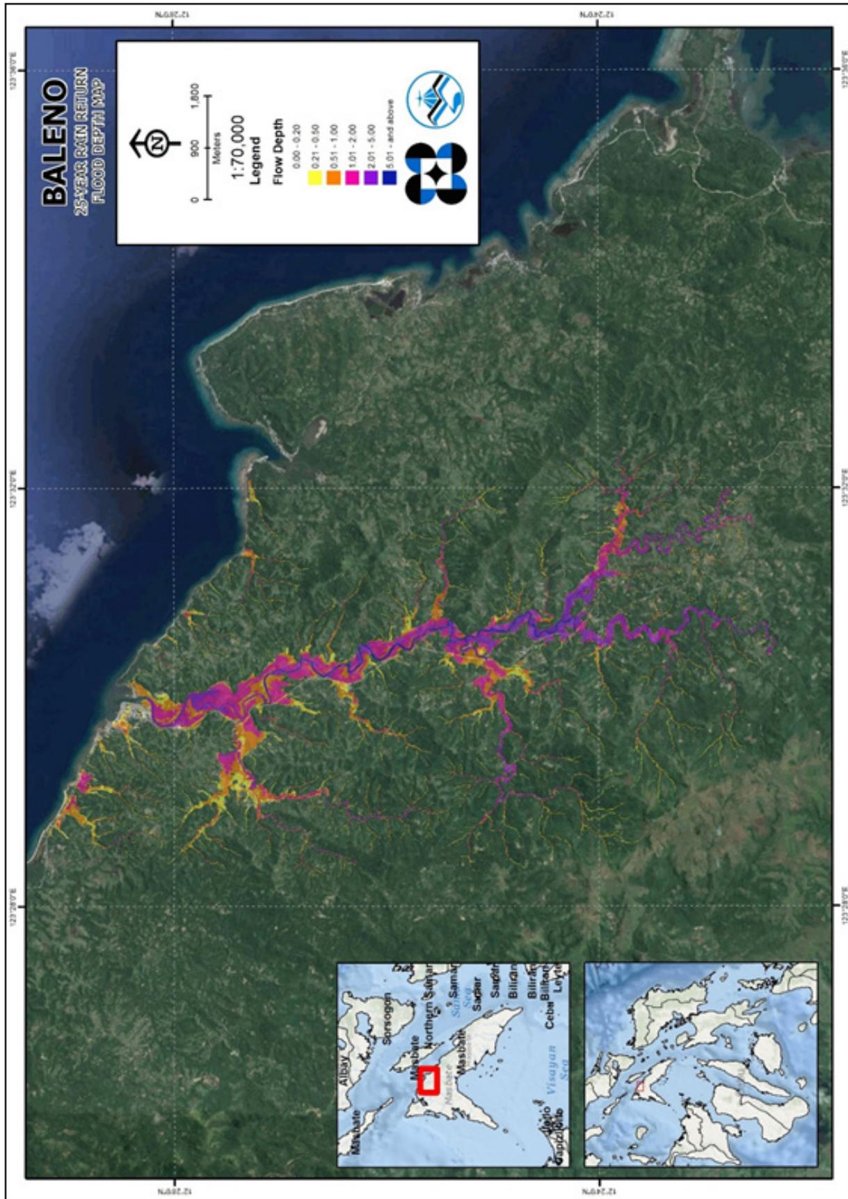
Figure 73. 25-year flow depth map for the Baleno flood plain overlaid on Google Earth imagery
