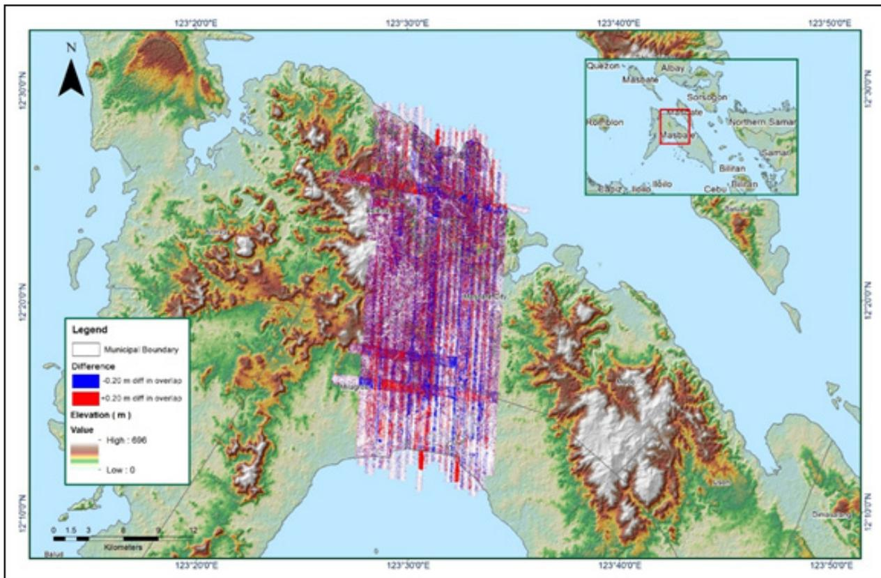
Figure A-8.7. Elevation difference between flight lines
