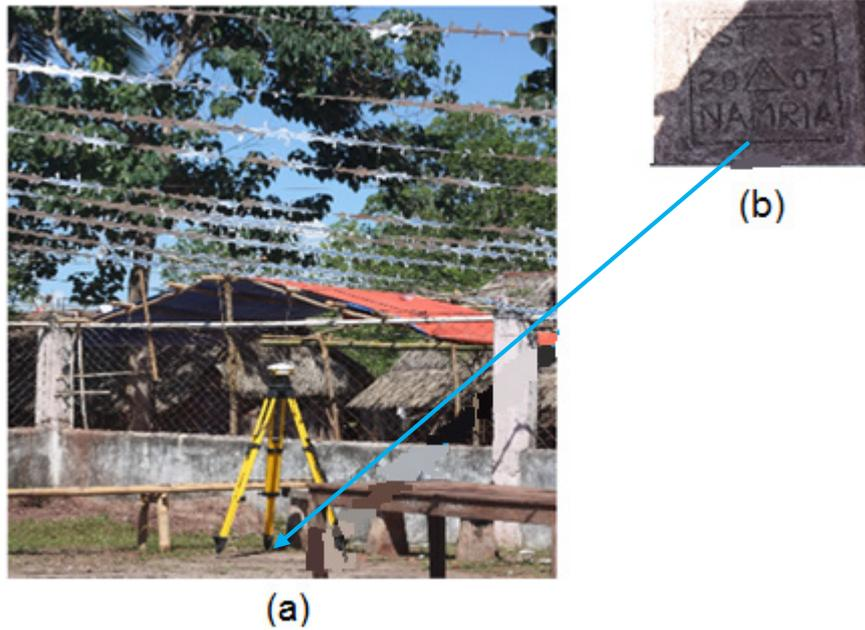
Figure 6. GPS set-up over MST-55 inside the compound of Casamongan Brgy. Hall, municipality of Balud, Masbate (a) and NAMRIA reference point MST-55 (b) as recovered by the field team.
