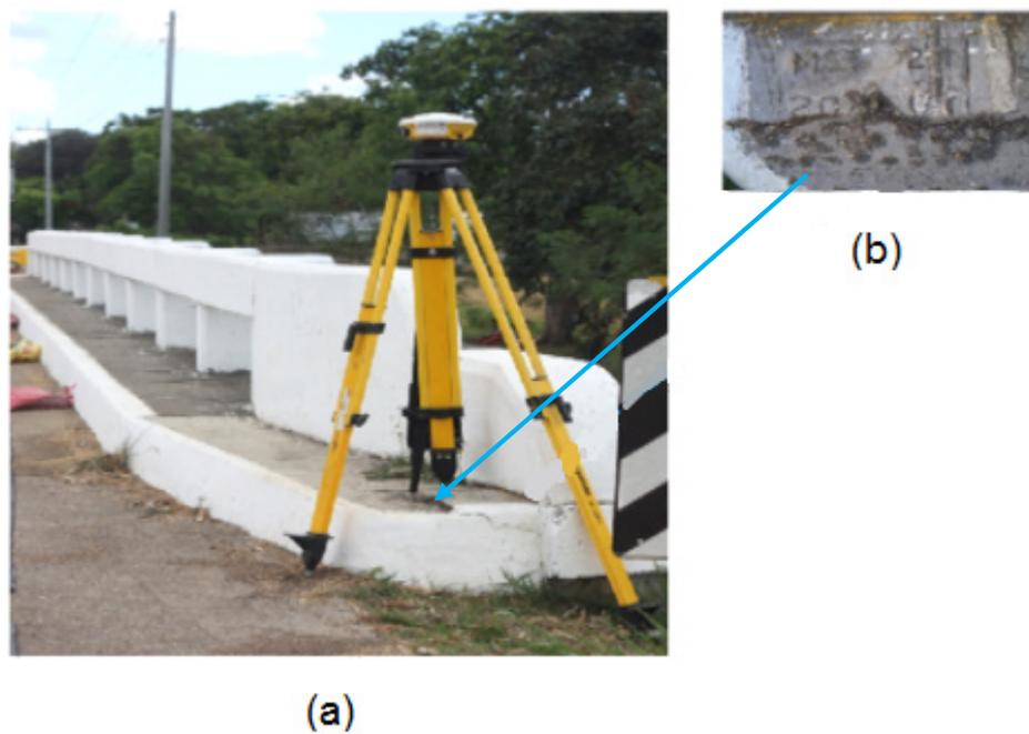
Figure 3. GPS set-up over MST-28 in Mambog Bridge, Barangay Bat-ongan, municipality of Mandaon, Masbate (a) and NAMRIA reference point MST-28 (b) as recovered by the field team.
