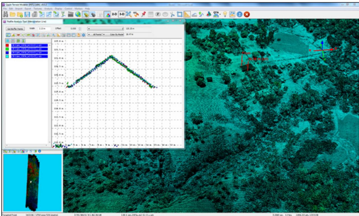
Figure 17. Quality checking for a Baleno flight I307P using the Profile Tool of QT Modeler.
