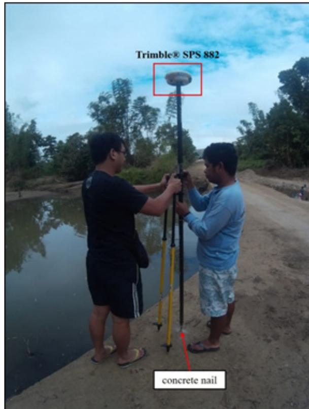
Figure 36. Trimble® SPS 882 setup at UP-ALA, located at Alas Bridge in Brgy. Alas, Mandaon, Masbate
