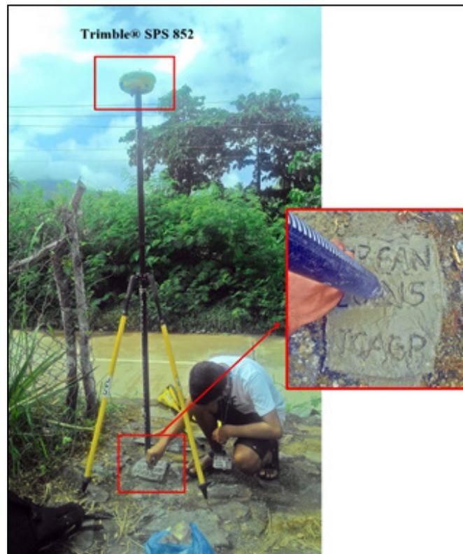
Figure 38. GNSS receiver setup, Trimble® SPS 852, at UP-GAN, located on the top of a riprap near Gangao Bridge, along Central Nautical Highway, Brgy. Gangao, Baleno, Masbate
