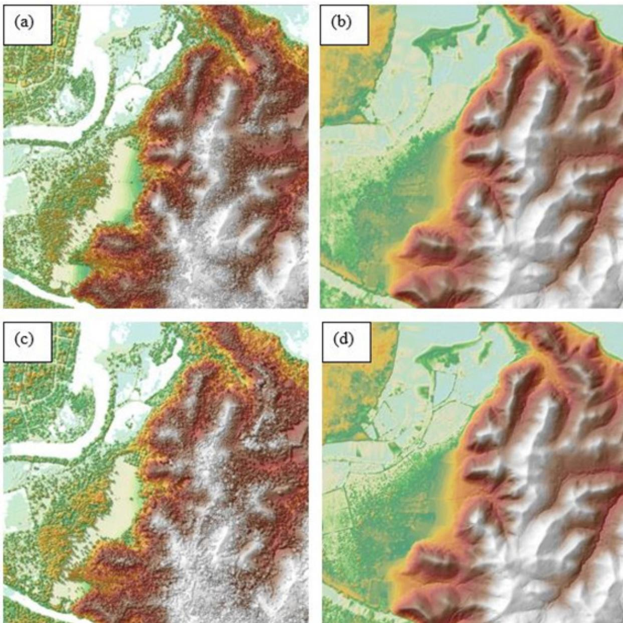
Figure 20. The production of last return DSM (a) and DTM (b), first return DSM (c) and secondary DTM (d) in some portion of Baleno floodplain.
