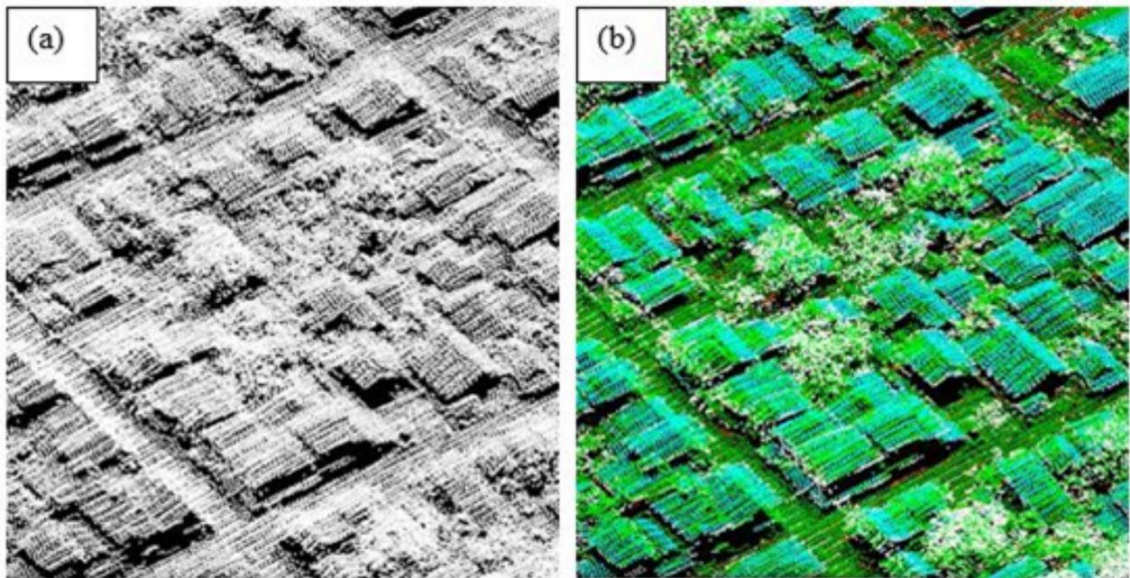
Figure 19. Point cloud before (a) and after (b) classification.
