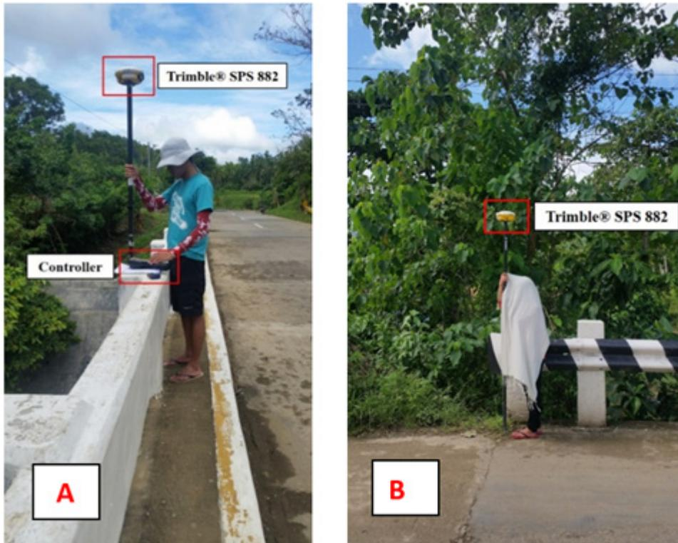
Figure 39. Setup during the Bridge As-built measurement in A) Cancahorao and B) Gangao Bridge
