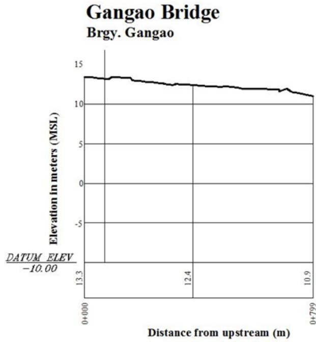
Figure 53. Segment 2 of 2 of Baleno centerline riverbed profile
