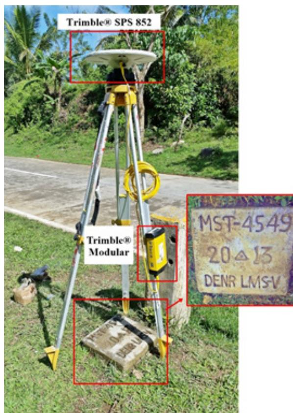
Figure 35. Trimble® SPS 882 base setup at MST-4945, a DENR-established control point located at the approach of Cancahorao Bridge along Central Nautical Highway in Brgy. Gangao, Baleno, Masbate
