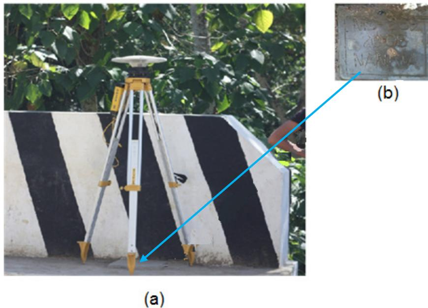
Figure 7. GPS set-up over MS-269 in Luy-a Bridge in Aroroy, Masbate (a) and NAMRIA benchmark MS-269 (b) as recovered by the field team.
