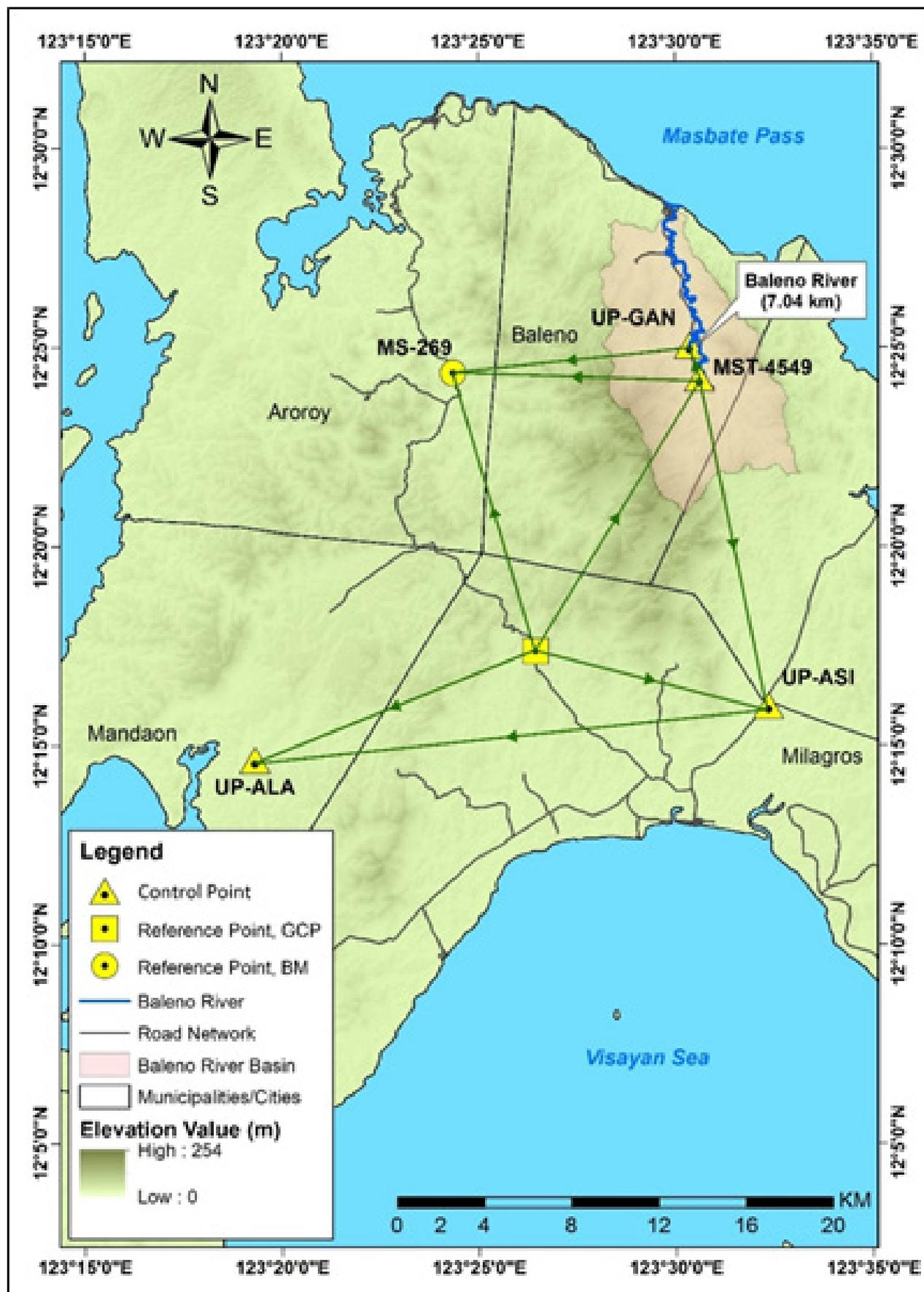
Figure 32. GNSS Network occupied in Baleno River Basin field survey
