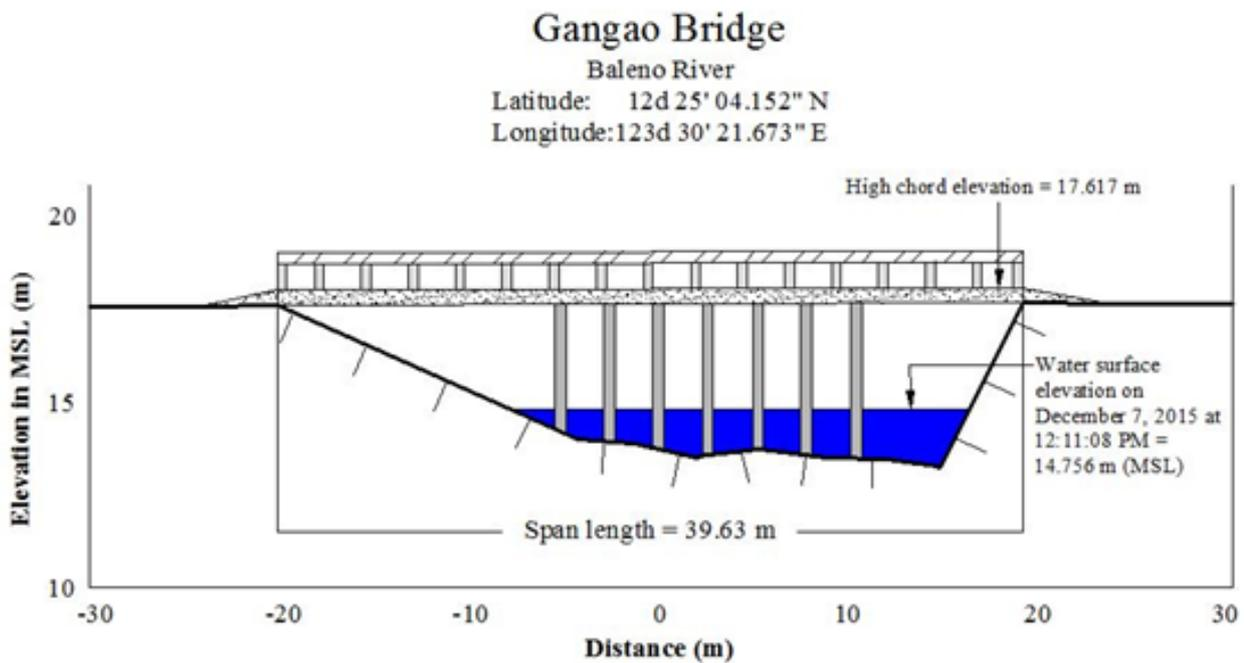
Figure 43. Bridge as-built and cross-sectional diagram of Baleno River at Gangao Bridge, Brgy. Gangao, Municipality of Baleno, Masbate
