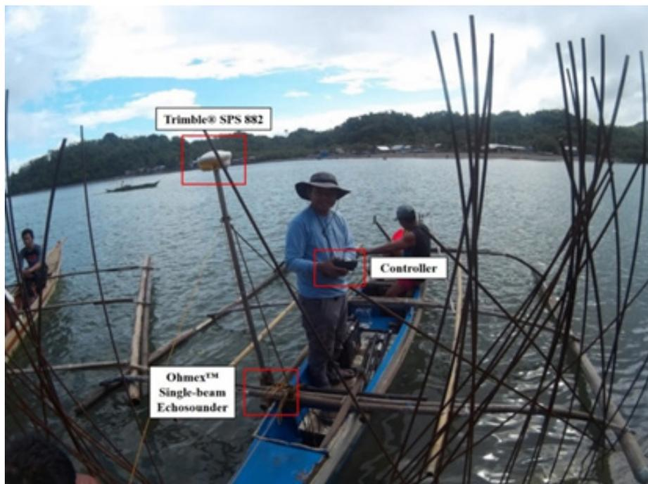
Figure 50. Setup of Trimble® SPS 882 receiver and Ohmex™ single-beam echosounder in a boat for the bathymetric survey in Baleno River
