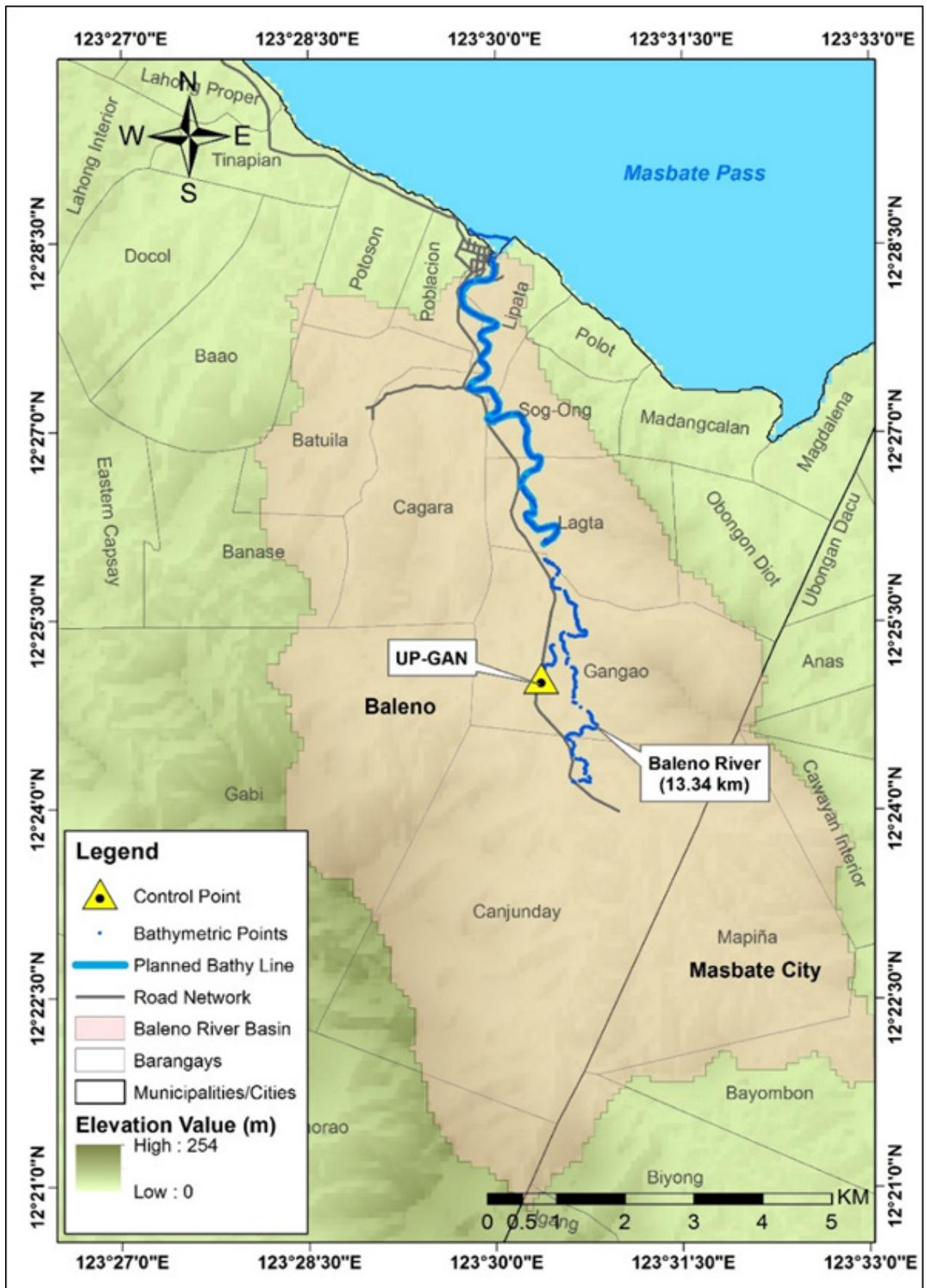
Figure 51. Acquired bathymetric points for Baleno River
