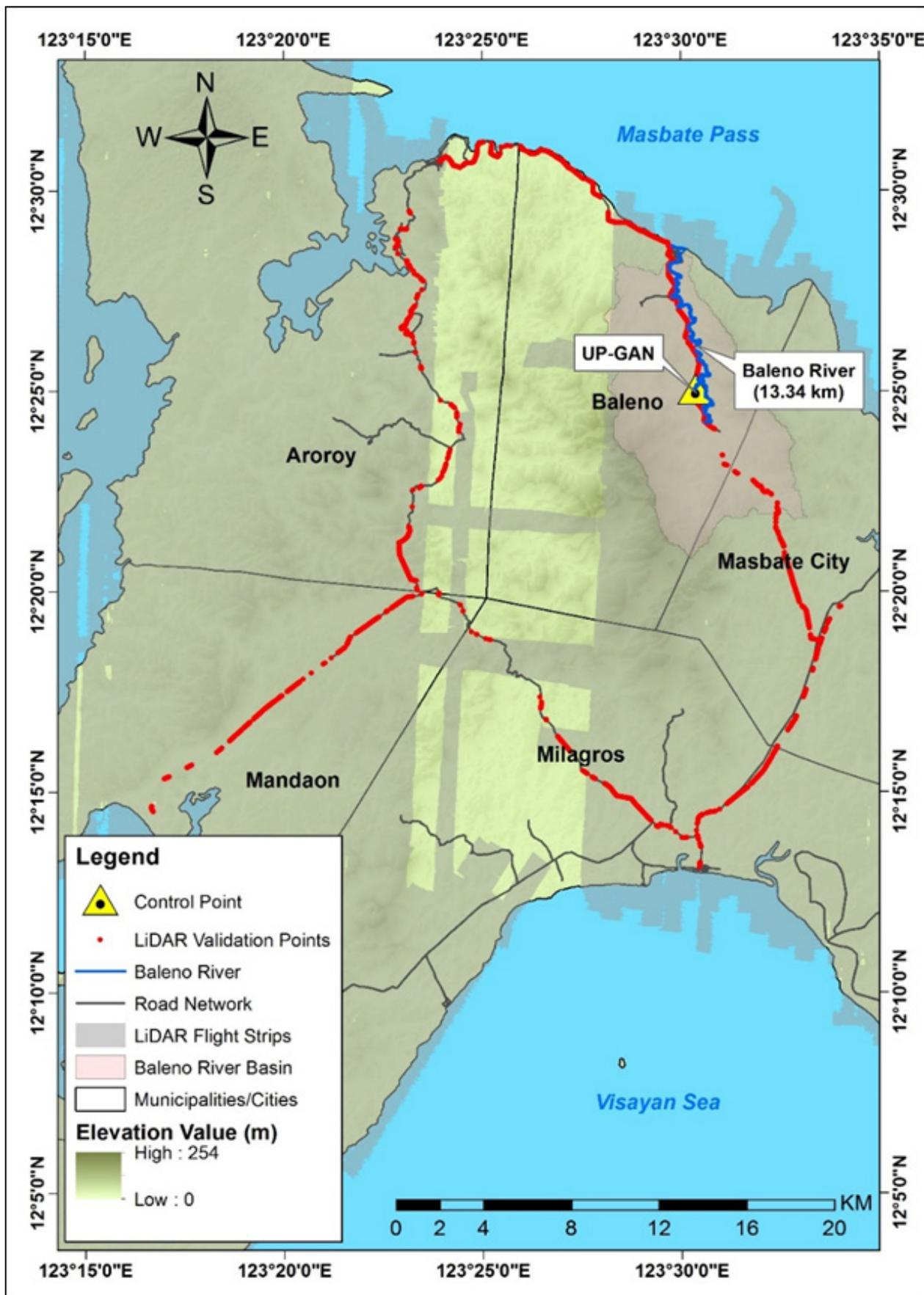
Figure 48. Points gathered during the LiDAR Ground Validation Survey for Baleno River Basin
