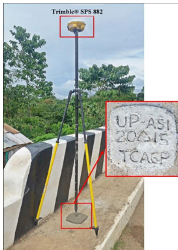
Figure 37. GNSS receiver setup, Trimble® SPS 882, at UP-ASI, at Asid Bridge, along Central Nautical Highway, Brgy. Asid, Masbate City
