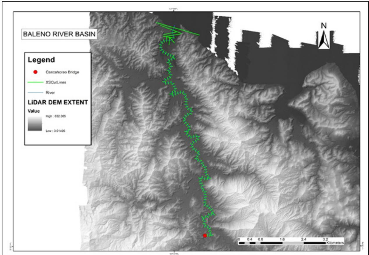
Figure 65. River cross-section of Baleno River generated through Arcmap HEC GeoRAS tool
