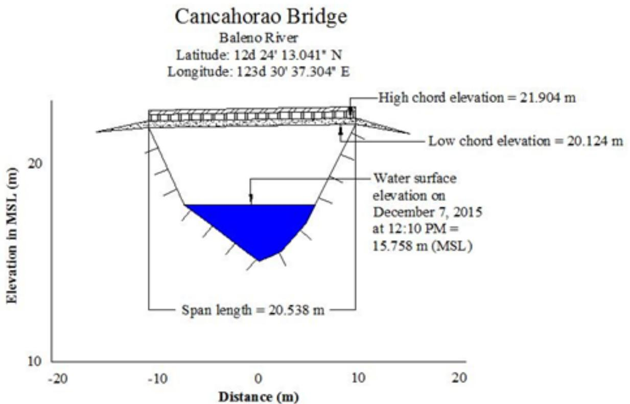
Figure 41. Cancahorao Bridge cross-section diagram
