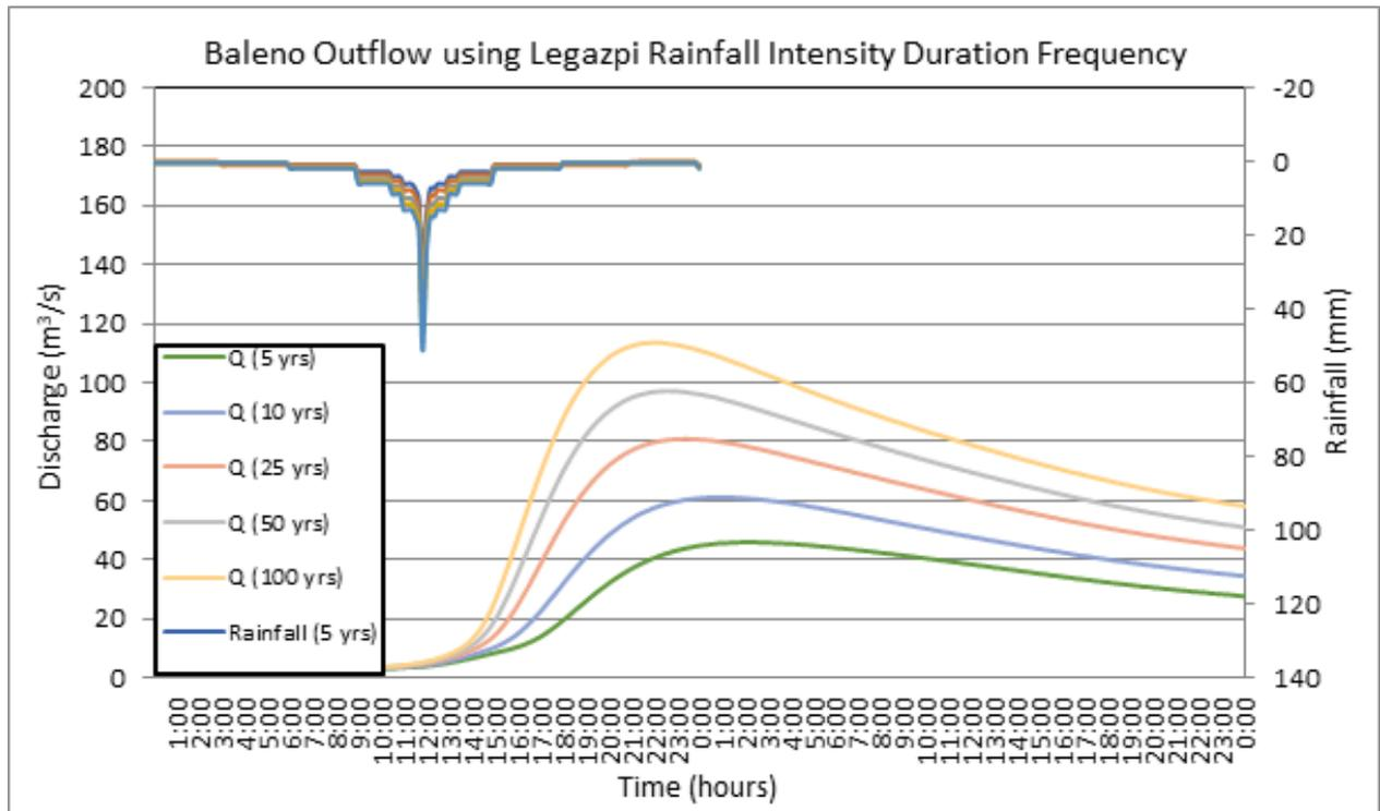
Figure 68. The outflow hydrograph at the Baleno River Basin, generated using the simulated events for 24-hour period for Legazpi station
