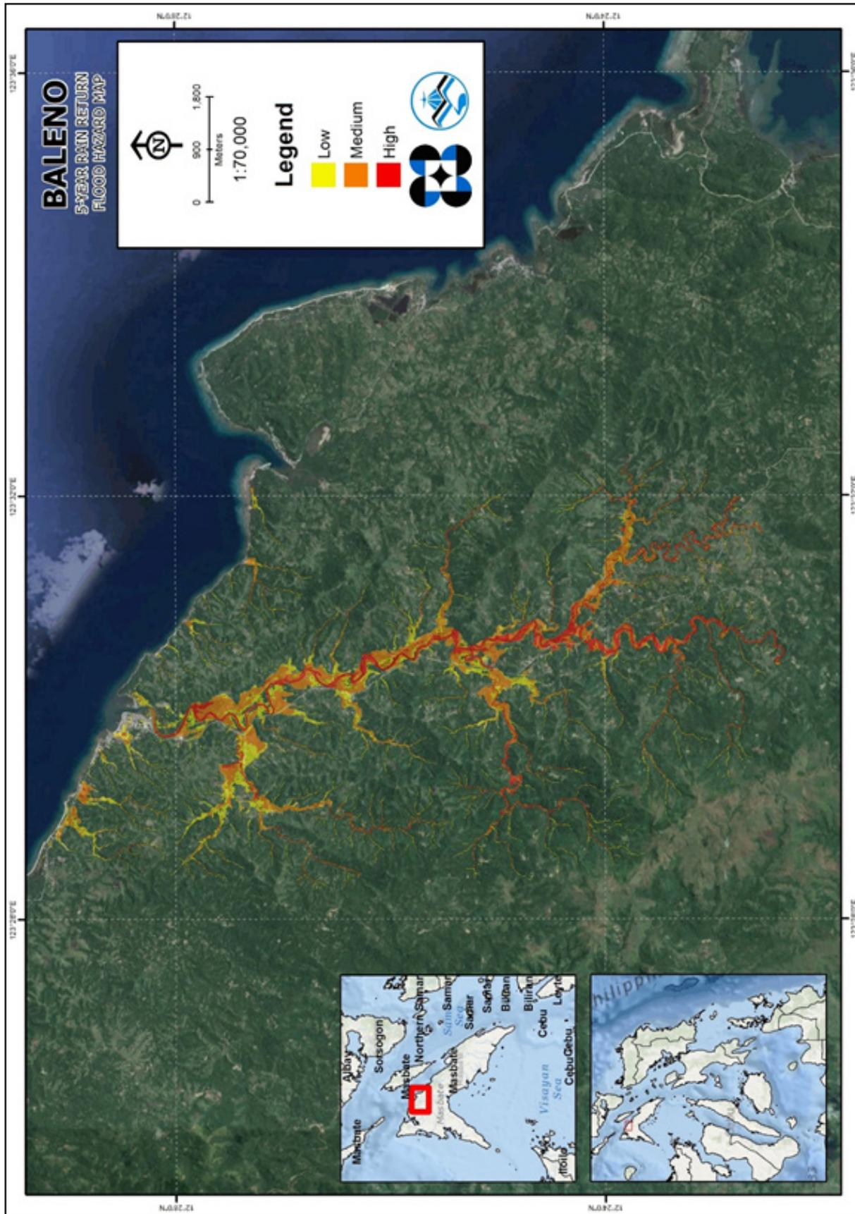
Figure 74. 5-year flood hazard map for the Baleno flood plain overlaid on Google Earth imagery
