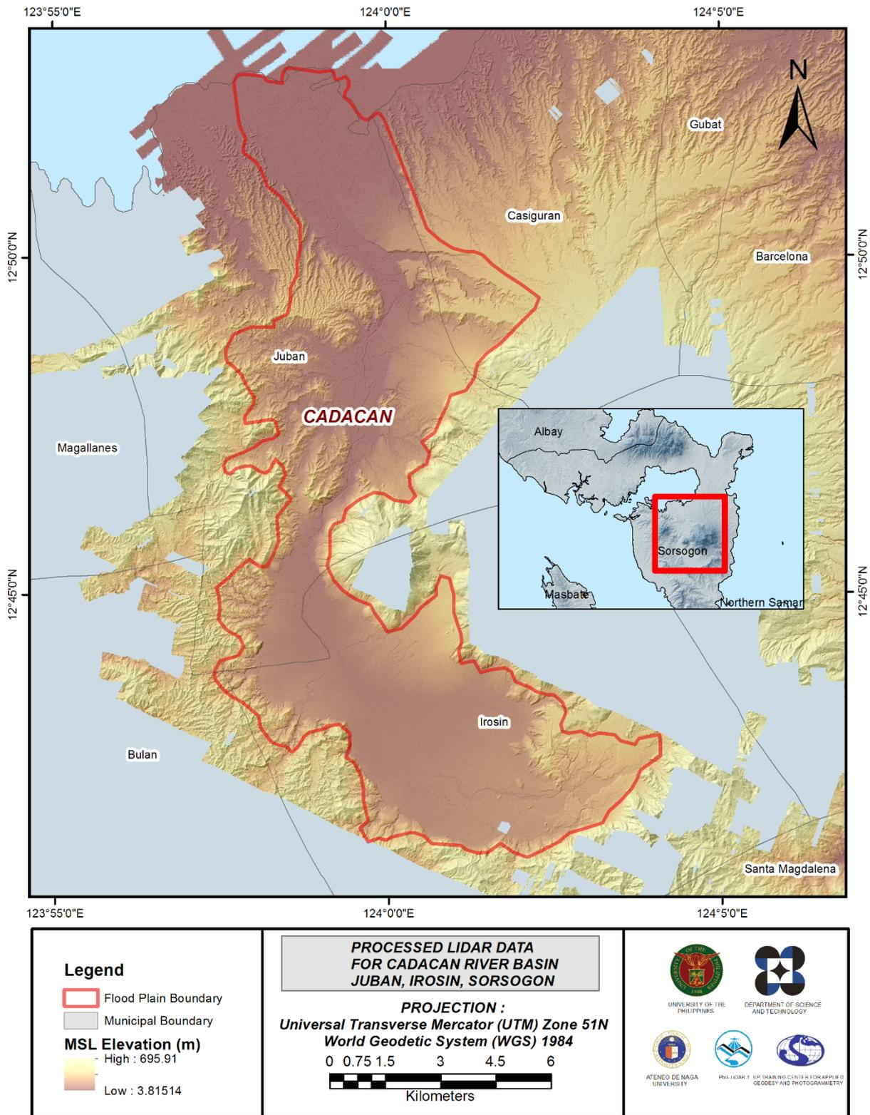
Figure 24. Map of Processed LiDAR Data for Cadacan Flood Plain.
