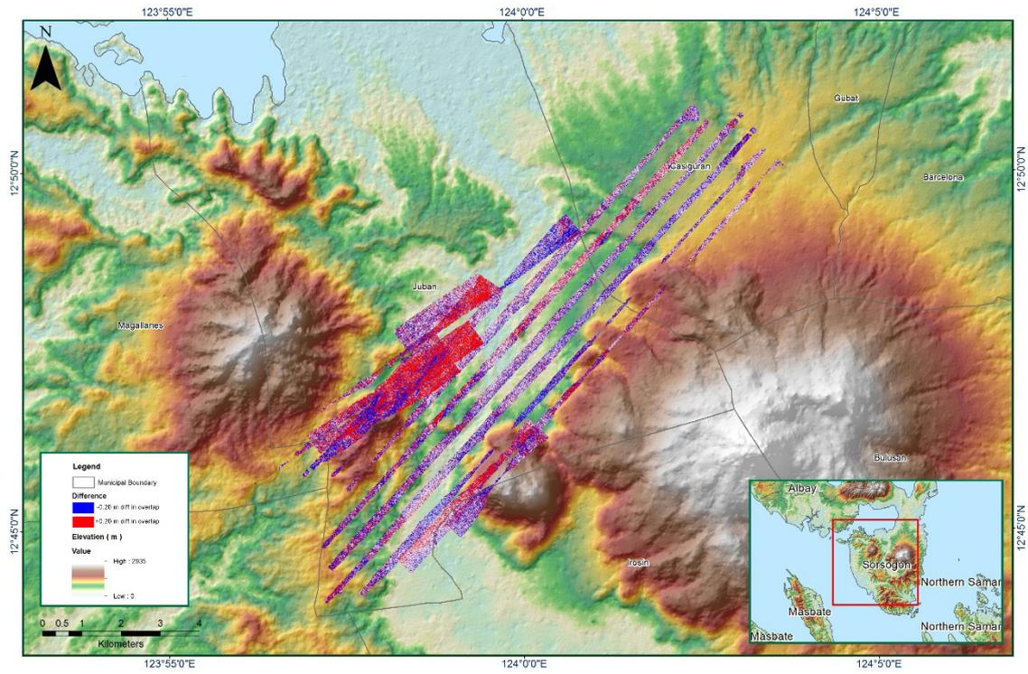
Figure 1.17.7. Elevation difference between flight lines
