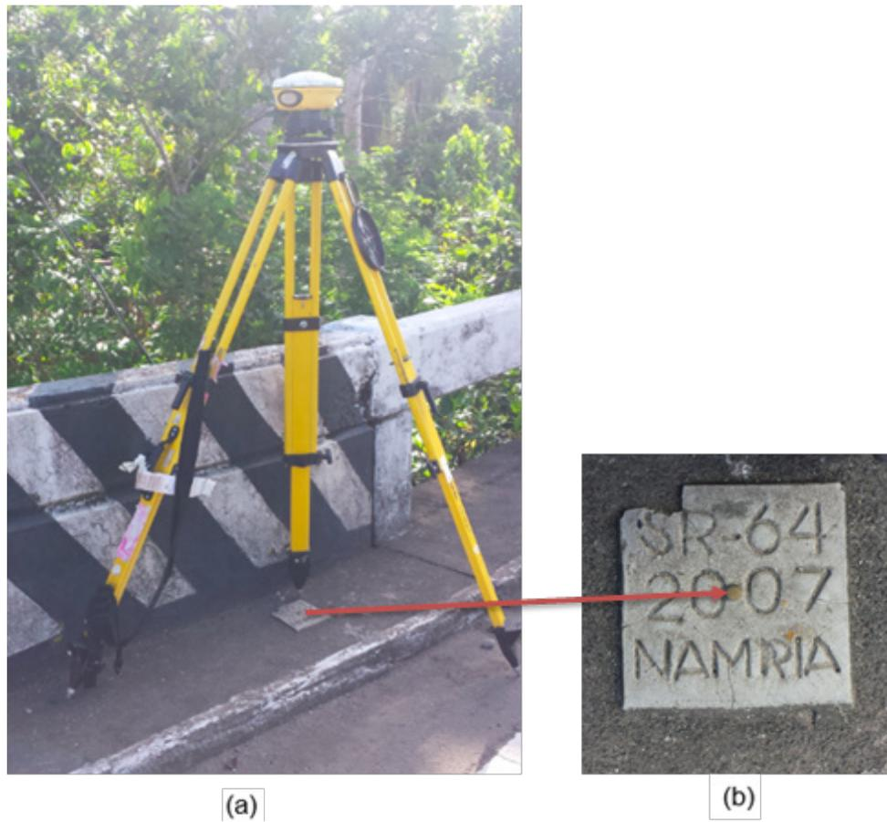
Figure 5. GPS set-up over SR-64 along National Highway No. 1 at km 645+80 in Barrio caluscus, Irosin, Sorsogon Province (a) and NAMRIA reference point SR-64 (b) as recovered by the field team.
