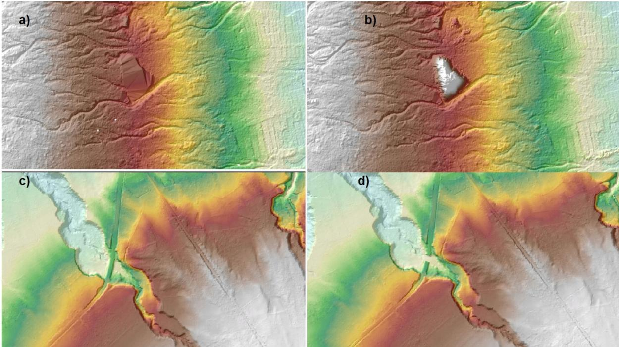
Figure 23. Portions in the DTM of Cadacan floodplain – a hilltop before (a) and after (b) data retrieval; a bridge before (c) and after (d) manual editing
