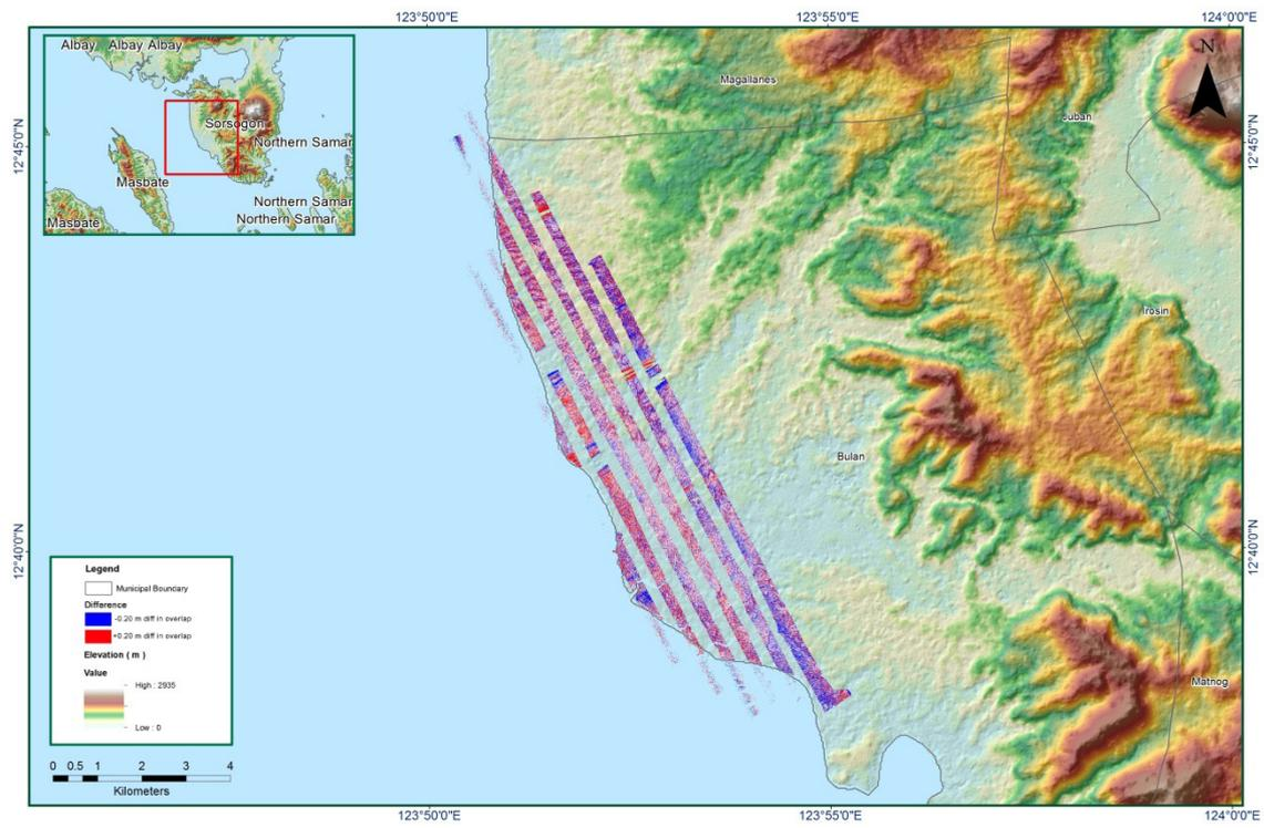
Figure 1.14.7. Elevation difference between flight lines
