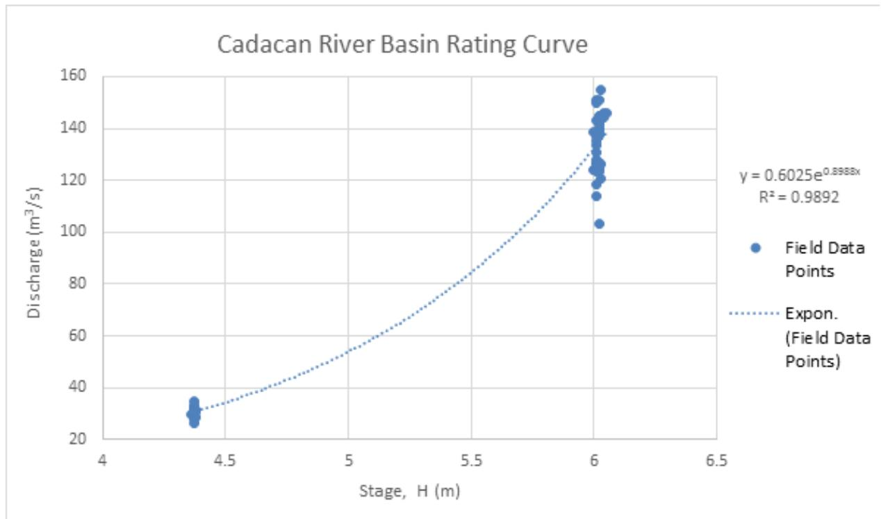
Figure 52. The rating curve of Taboc Bridge in Cadacan, Sorsogon
