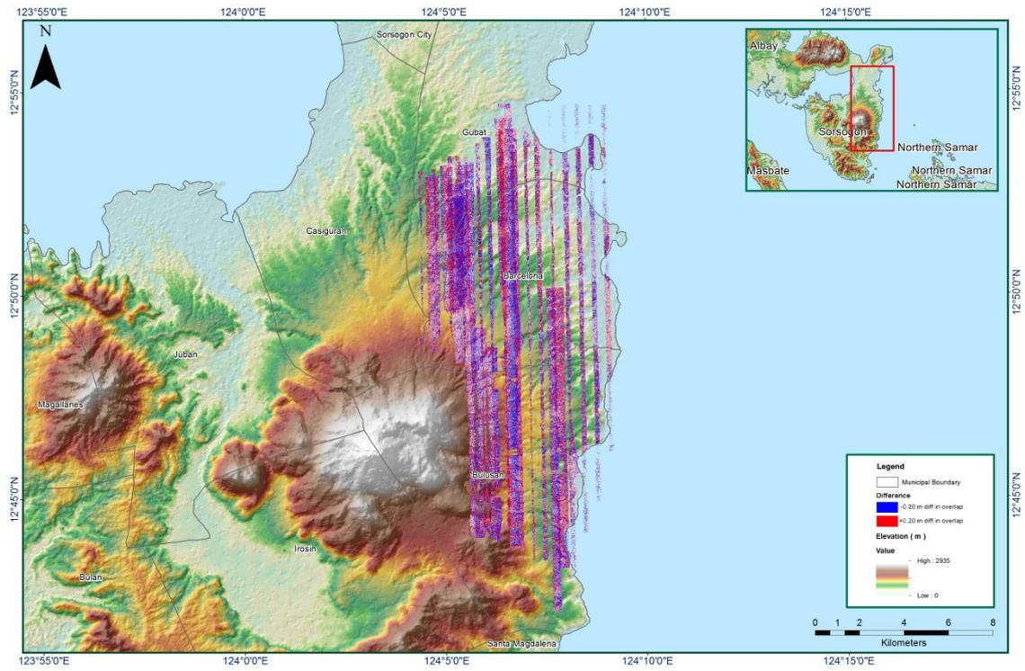
Figure 1.11.7. Elevation difference between flight lines
