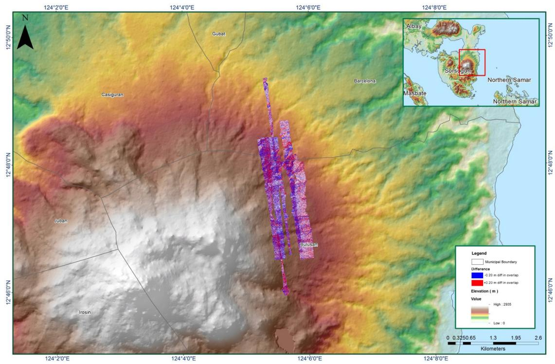
Figure 1.9.7. Elevation difference between flight lines
