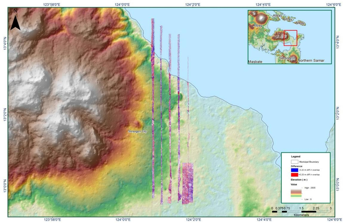
Figure 1.4.7. Elevation difference between flight lines
