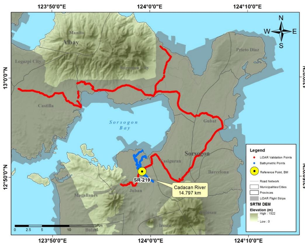
Figure 44. Validation point acquisition survey of Cadacan River Basin
