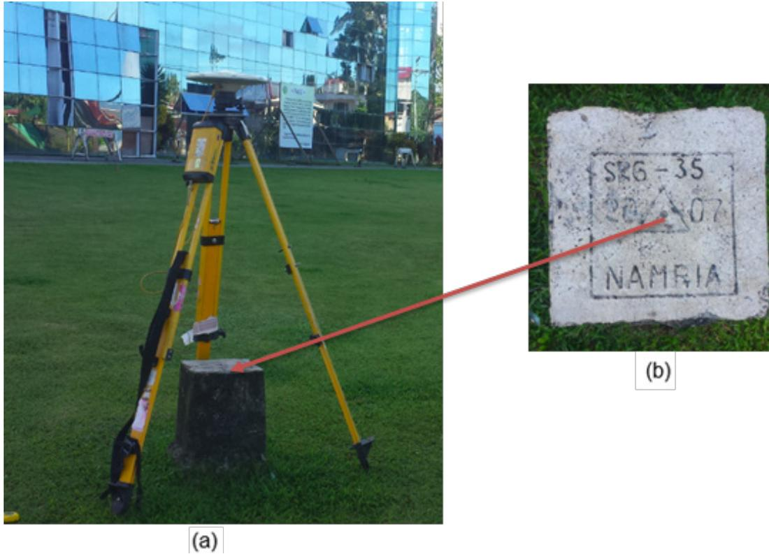
Figure 3. GPS set-up over SRG-35 as recovered in front of Casiguran Municipal Hall from the concrete fence and 13 meters from the flagpole (a) and NAMRIA reference point SRG-35 (b) as recovered by the field team.
