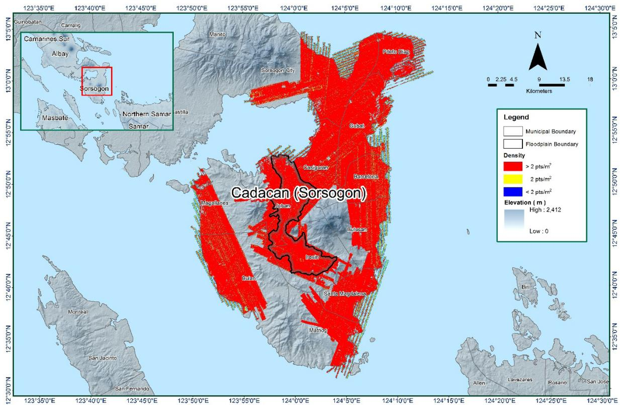
Figure 15. Pulse density map of merged LiDAR data for Cadacan floodplain.
