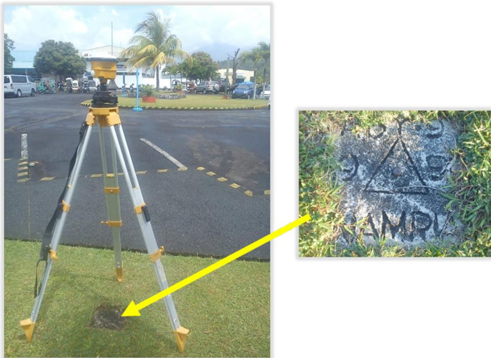
Figure 4. GPS set-up over ABY-9 inside Legaspi Airport Compound 52.0 meters SE of Legaspi Airport Flagpole, 35 meters NE of Legaspi Airport Welcome Post 3.30 meters NW of Lamp (a) and NAMRIA reference point ABY-9 (b) as recovered by the field team.
