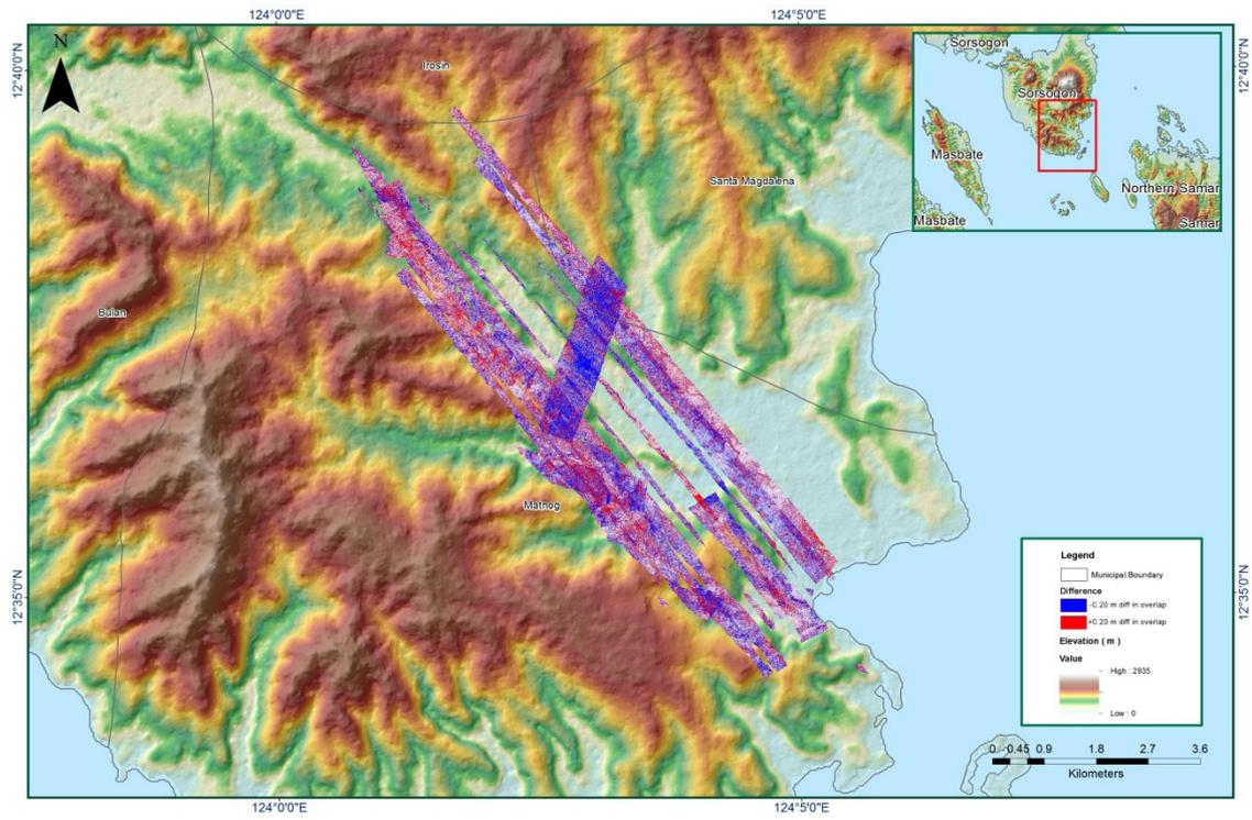
Figure 1.7.7. Elevation difference between flight lines
