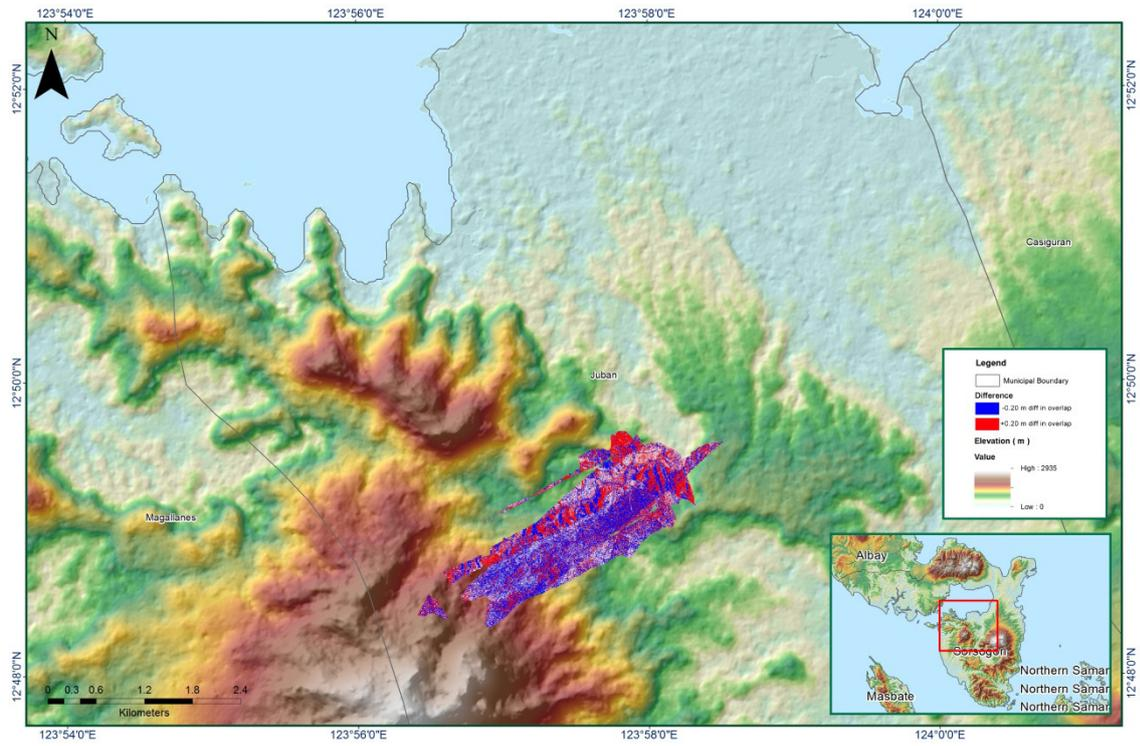
Figure 1.2.7. Elevation difference between flight lines
