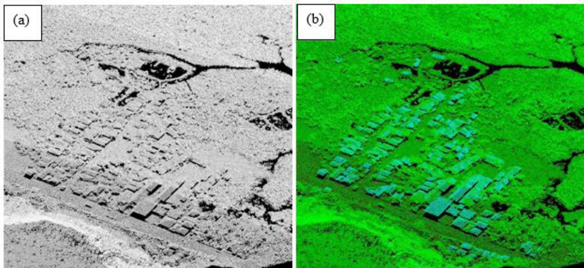
Figure 19. Point cloud before (a) and after (b) classification.
