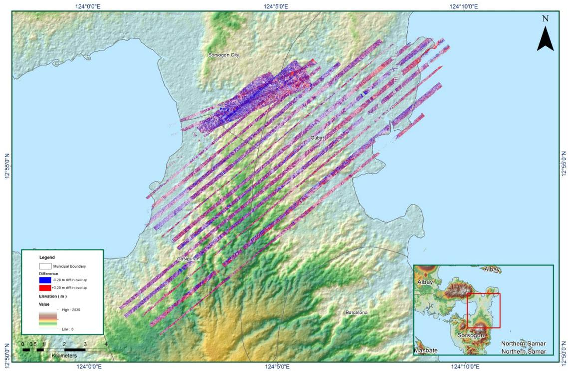
Figure 1.12.7. Elevation difference between flight lines
