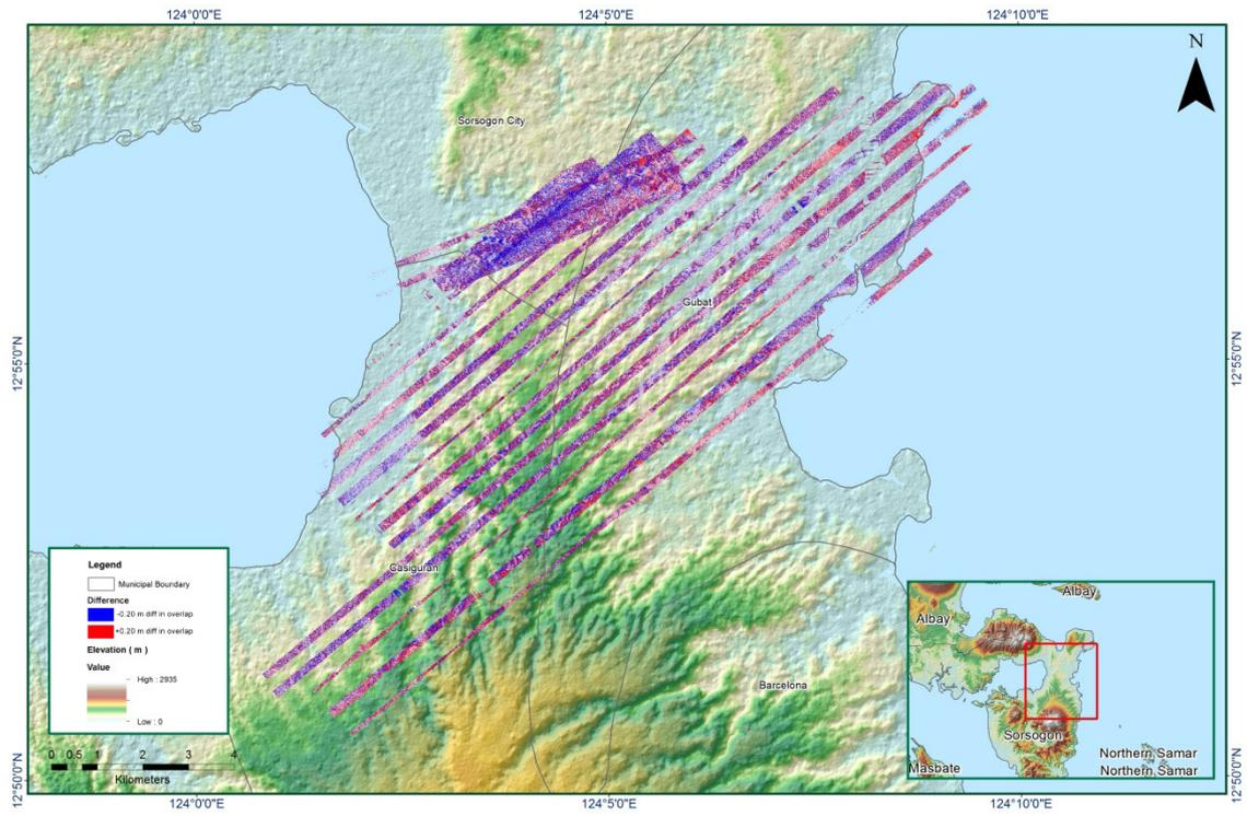
Figure 1.13.7. Elevation difference between flight lines
