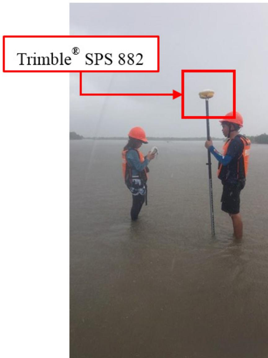
Figure 46. Manual Bathymetric survey using in Cadacan River
