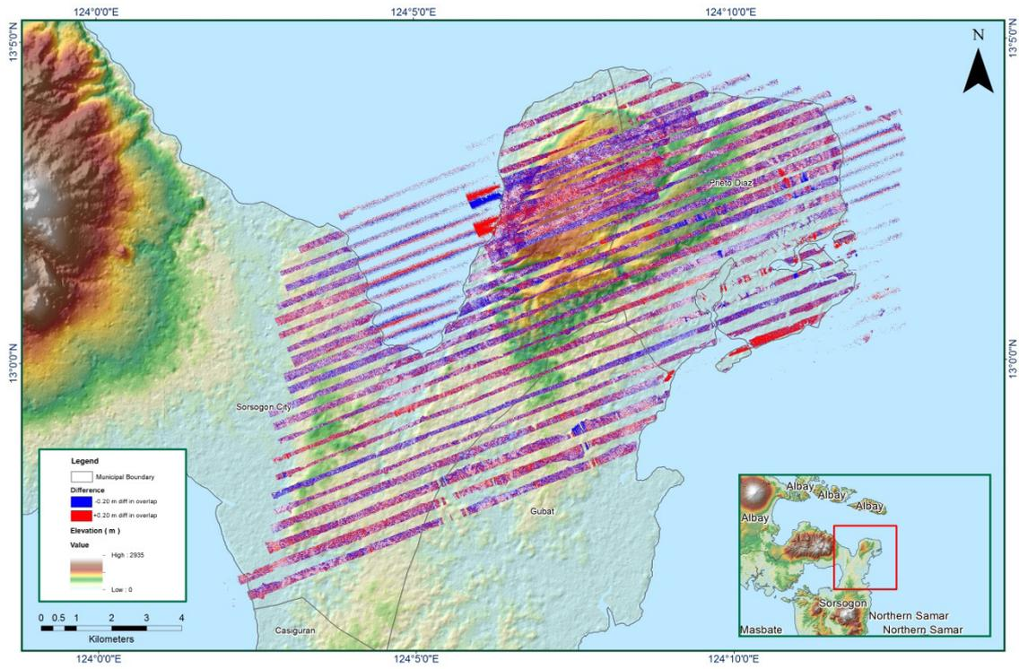
Figure 1.10.7. Elevation difference between flight lines
