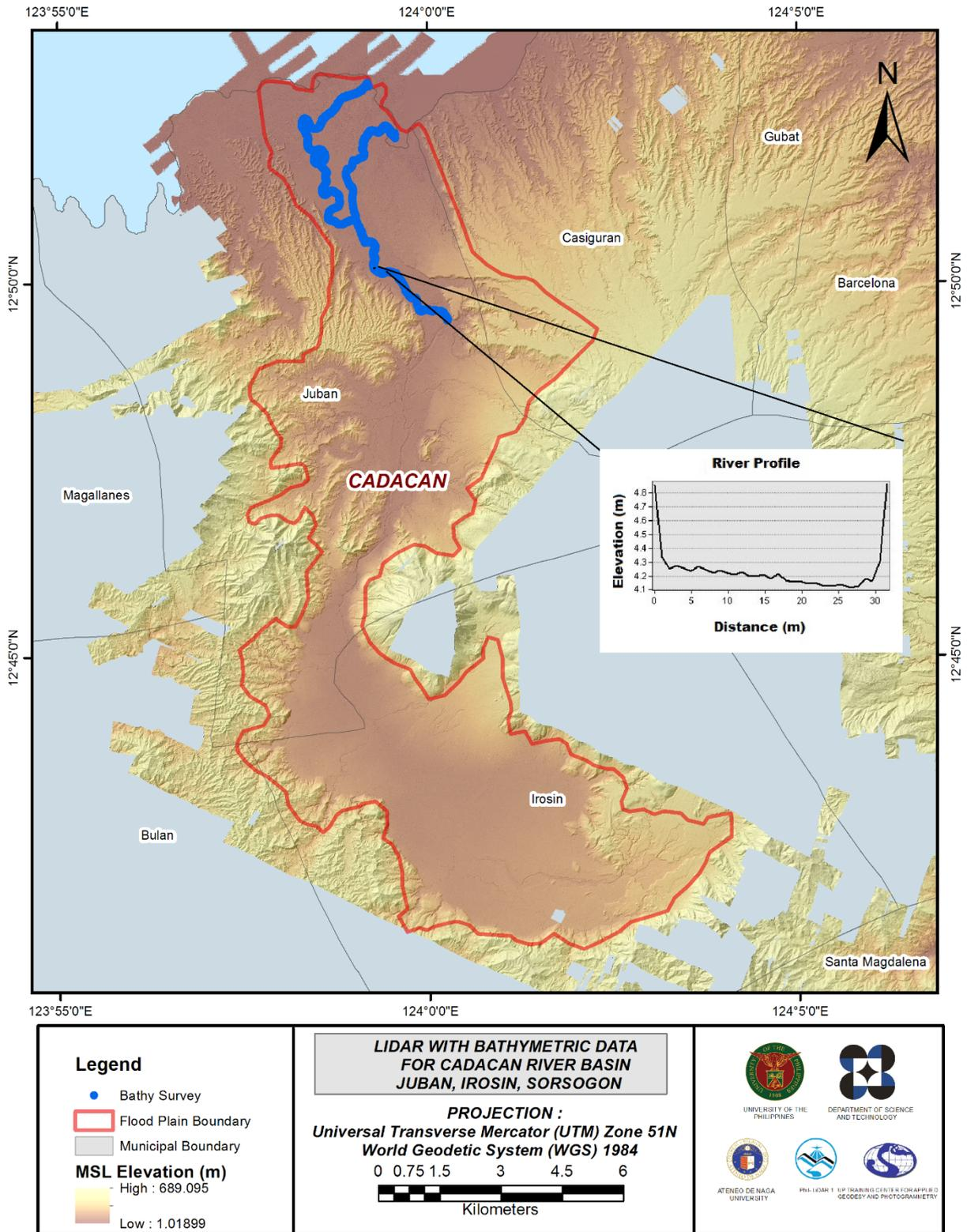
Figure 28. Map of Cadacan Flood Plain with bathymetric survey points shown in blue.
