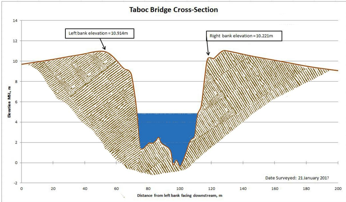
Figure 51. The cross-section plot of Taboc Bridge
