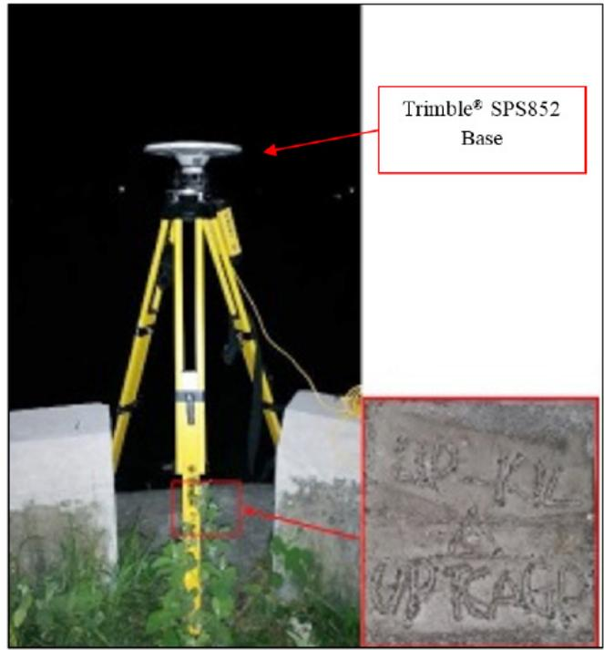
Figure 36. GNSS base, Trimble® SPS852 base set-up at UP-KIL in Kilicao Bridge in Daraga, Albay
