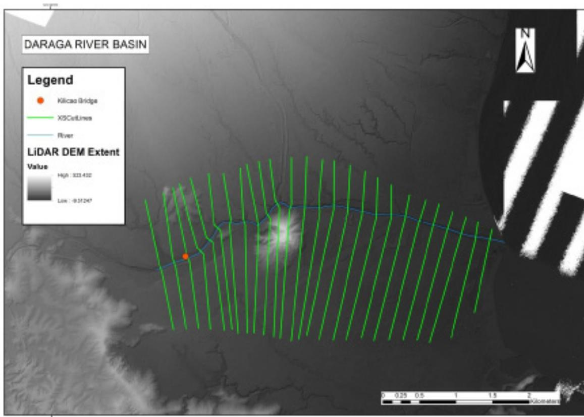
Figure 58. River cross-section of Daraga River generated through Arcmap HEC GeoRAS tool
