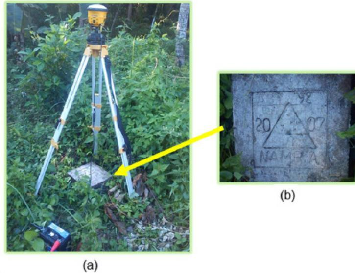
Figure 3. a) GPS set-up over ABY-92 beside the baseline of the basketball court at about 19 m from the barangay hall, and b) NAMRIA reference point ABY-92 as recovered by the field team.
