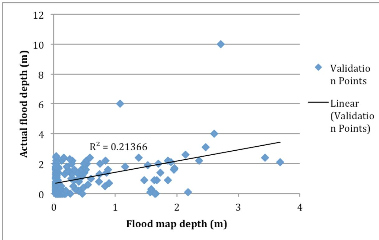
Figure 97. Flood map depth vs. Actual flood depth
