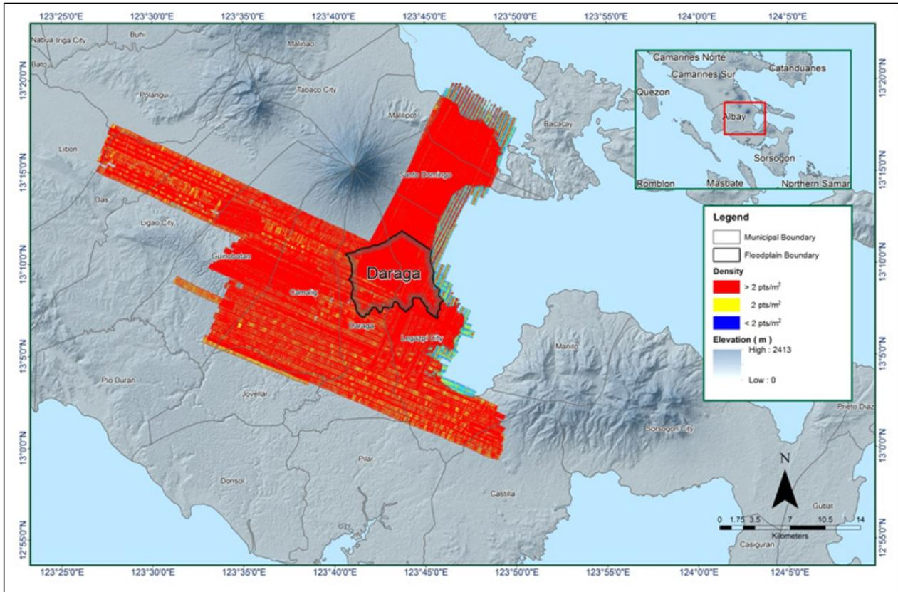
Figure 16. Pulse density map of merged LiDAR data for Daraga Floodplain.
