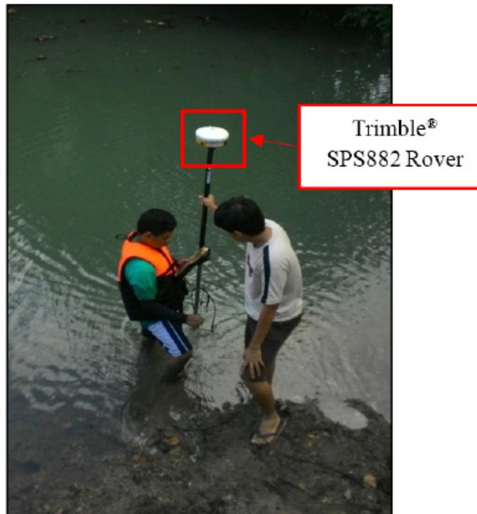
Figure 44. Manual bathymetric survey along Yawa River in Brgy. Binitaya, Daraga, Albay
