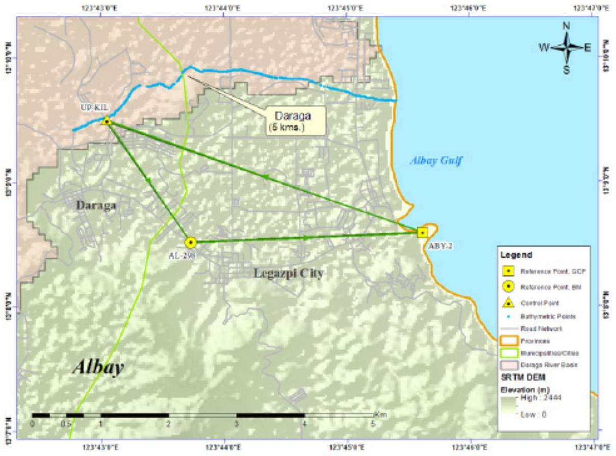
Figure 33. GNSS Network of Daraga River Basin Survey
