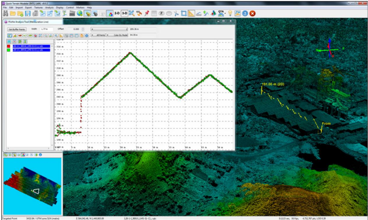
Figure 18. Quality checking for Daraga Flight 3891G using the Profile Tool of QT Modeler.
