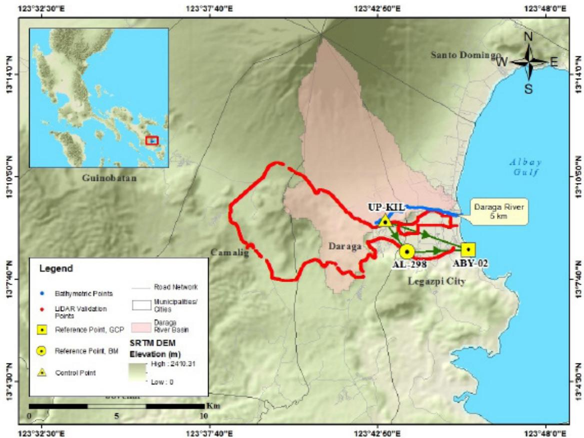
Figure 32. Extent of the bathymetric survey (in blue line) in Daraga River and the LiDAR data validation survey (red).
