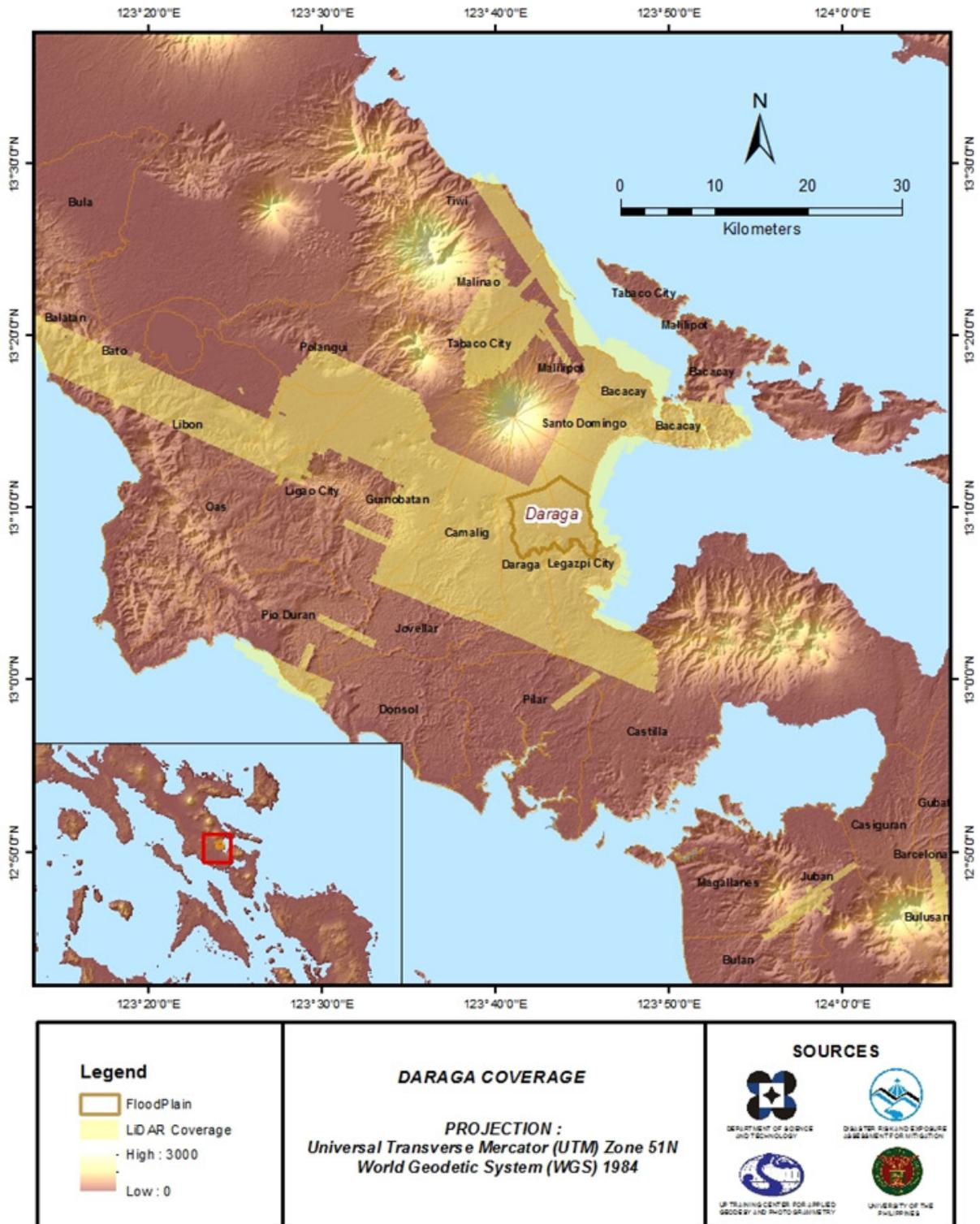
Figure 9. Actual LiDAR survey coverage for Daraga Floodplain.
