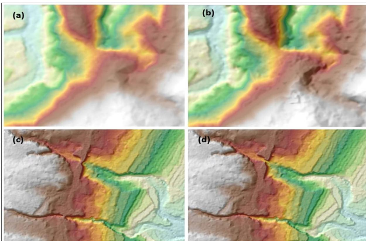
Figure 24. Portions in the DTM of Daraga floodplain –a mountain ridge before (a) and after (b) data retrieval; and a bridge before (c) and after (d) manual editing
