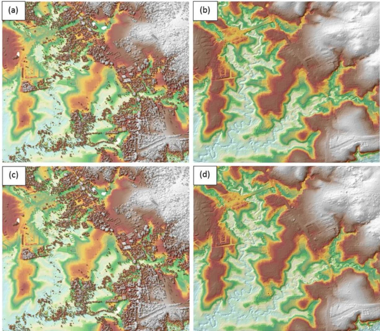
Figure 21. The Production of last return DSM (a) and DTM (b), first return DSM (c), and secondary DTM (d) in some portion of Daraga Floodplain.
