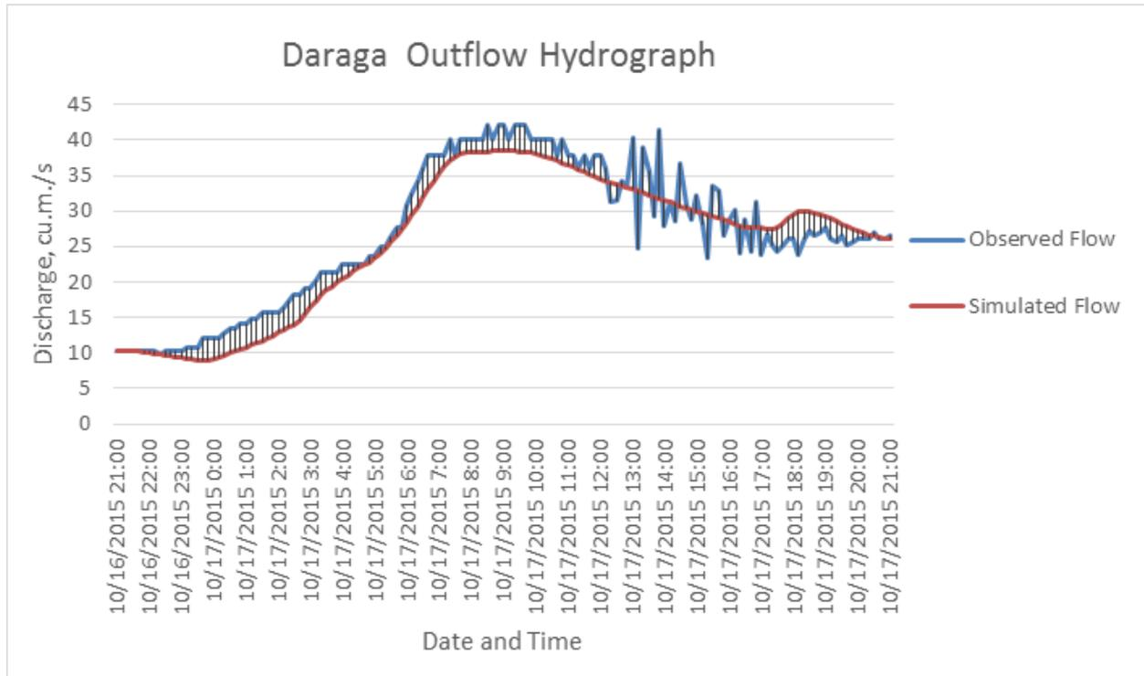
Figure 60. Outflow hydrograph of Daraga produced by the HEC-HMS model compared with observed outflow
