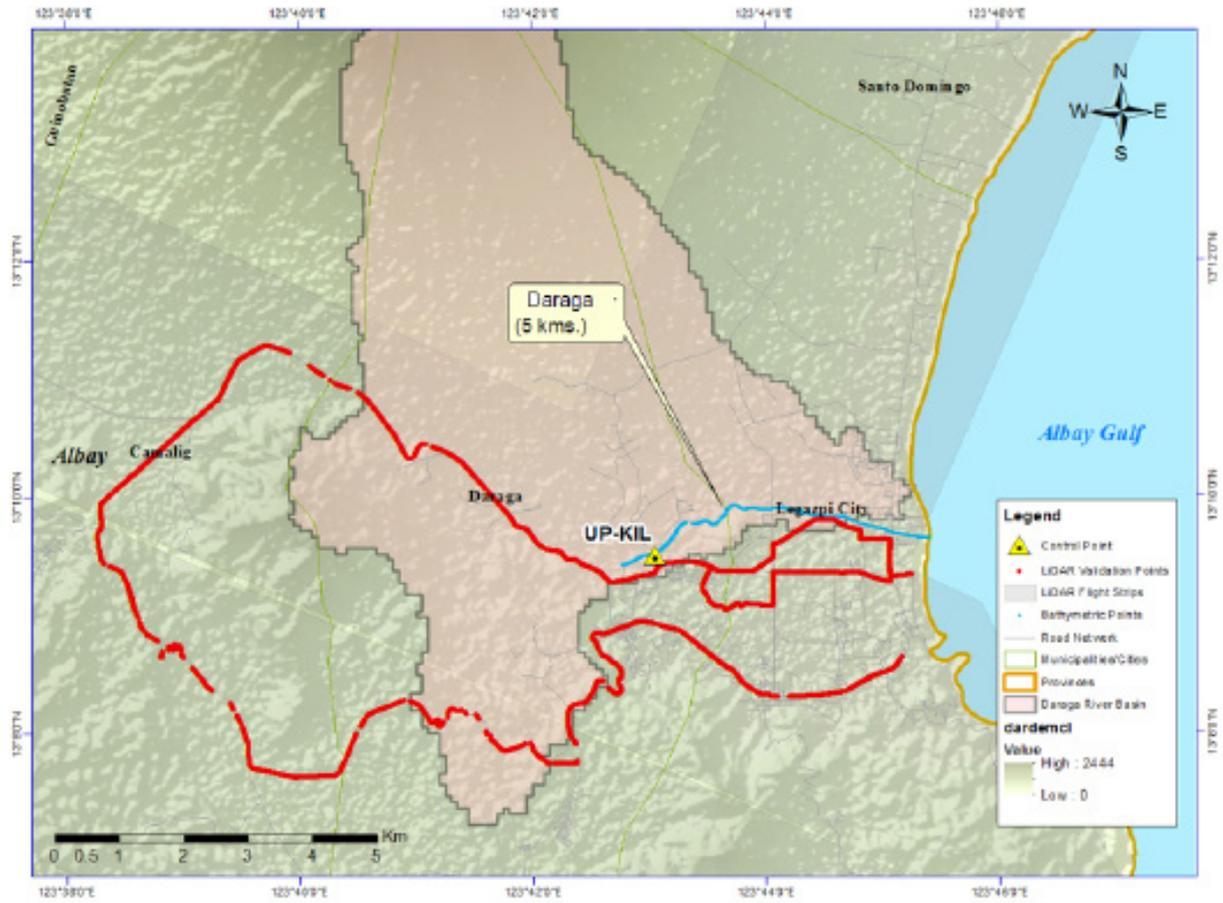
. Figure 43. LiDAR Ground Validation Survey along Daraga River Basin
