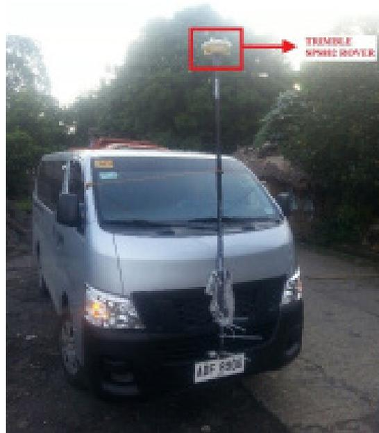
Figure 42. Trimble® SPS 882 set up for the acquisition of LiDAR validation points
