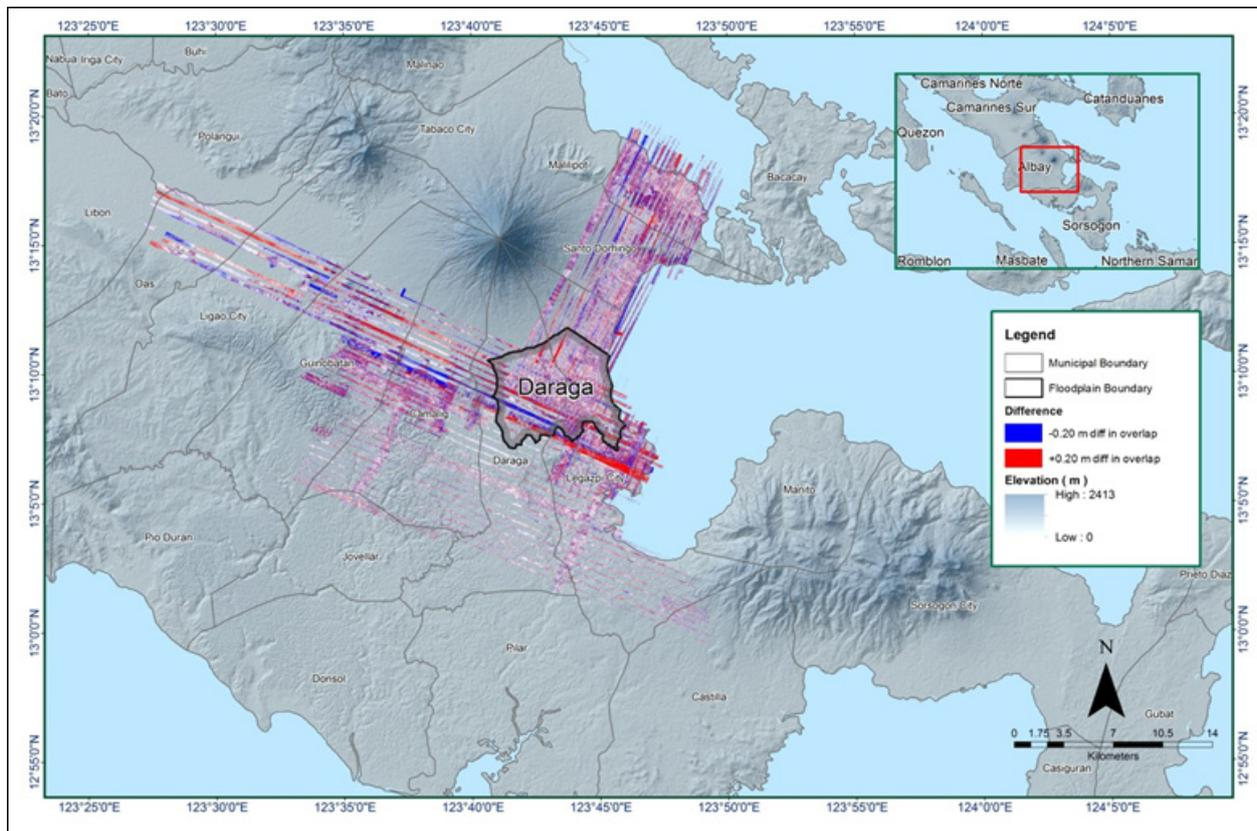
Figure 17. Elevation difference map between flight lines for Daraga Floodplain.
