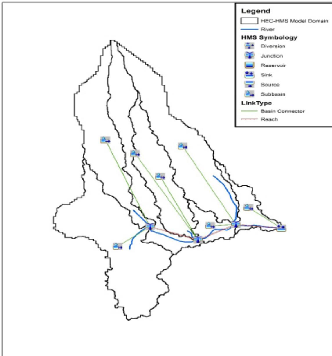
Figure 57. The Daraga River Basin model generated in HEC-HMS
