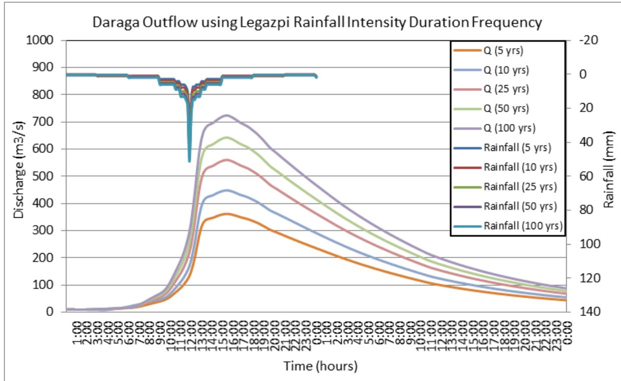
Figure 61. The Outflow hydrograph at the Daraga Station, generated using the simulated rain events for 24-hour period for Legazpi station
