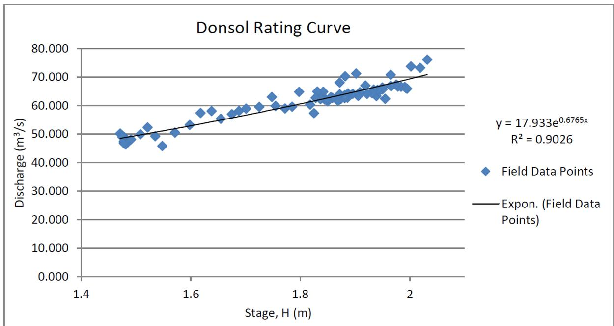
Figure 46. The rating curve of Ilog Bridge in Pilar, Sorsogon
