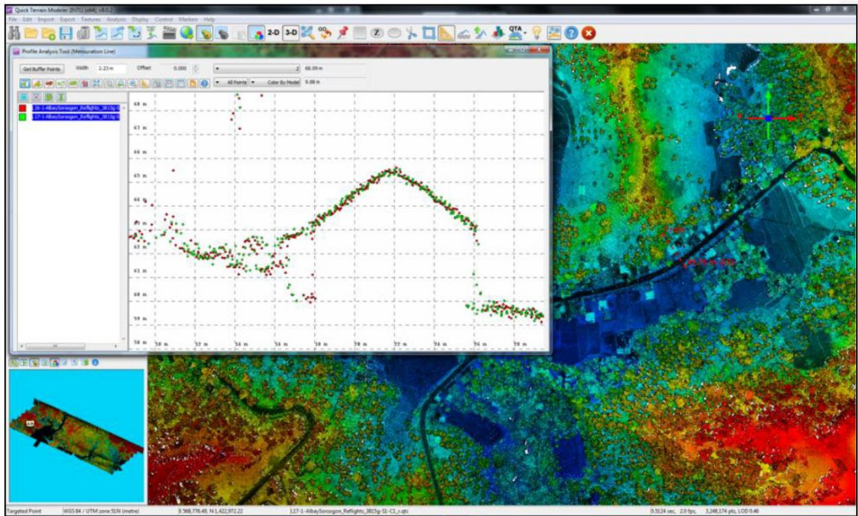
Figure 16. Quality checking for a Donsol flight 3815G using the Profile Tool of QT Modeler
