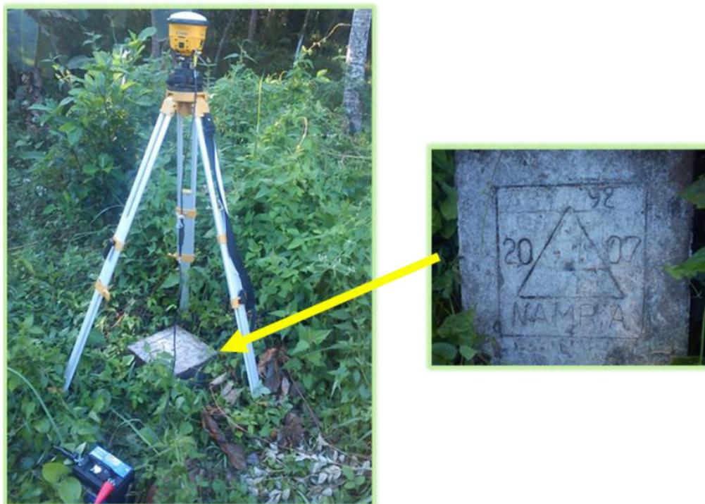
Figure 4. GPS set-up over ABY-92 located beside the baseline of the basketball court, about 19 meters from barangay hall in Brgy. Allang, Ligao City (a) and NAMRIA reference point ABY-92 (b) as recovered by the field team
