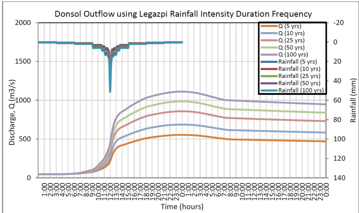
Figure 58. The Outflow hydrograph at the Donsol Station, generated using the simulated rain events for 24-hour period for Tacloban station
