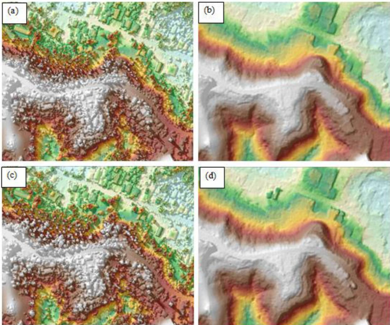
Figure 19. The production of last return DSM (a) and DTM (b), first return DSM (c) and secondary DTM (d) in some portion of Donsol Floodplain
