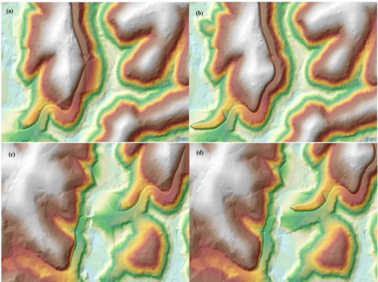
Figure 22. Portions in the DTM of Donsol Floodplain – a mountain ridge and road before (a) and after (b) data retrieval; a bridge before (c) and after (d) manual editing
