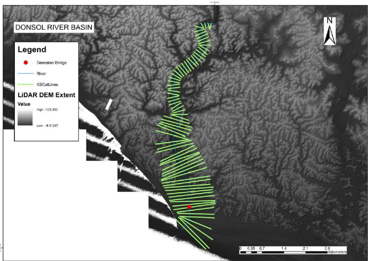
Figure 55. River cross-section of Donsol River generated through Arcmap HEC GeoRAS tool
