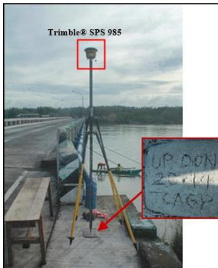
Figure 34. Trimble® SPS 985 at UP-DON at the approach of Dancalan Bridge in Donsol, Sorsogon
