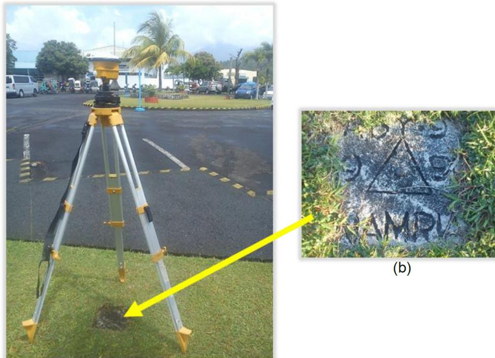
Figure 5. GPS set-up over ABY-9 at Legaspi Airport Compound (a) and NAMRIA reference point ABY-9 (b) as recovered by the field team
