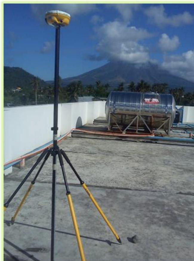
Figure 6. GPS set-up over LPH-01 as established at the rooftop a building at La Piazza Hotel and Convention Center located at Tahao Road, Legazpi, Albay
