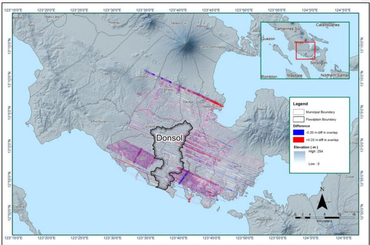
Figure 15. Elevation difference map between flight lines for Donsol Floodplain
