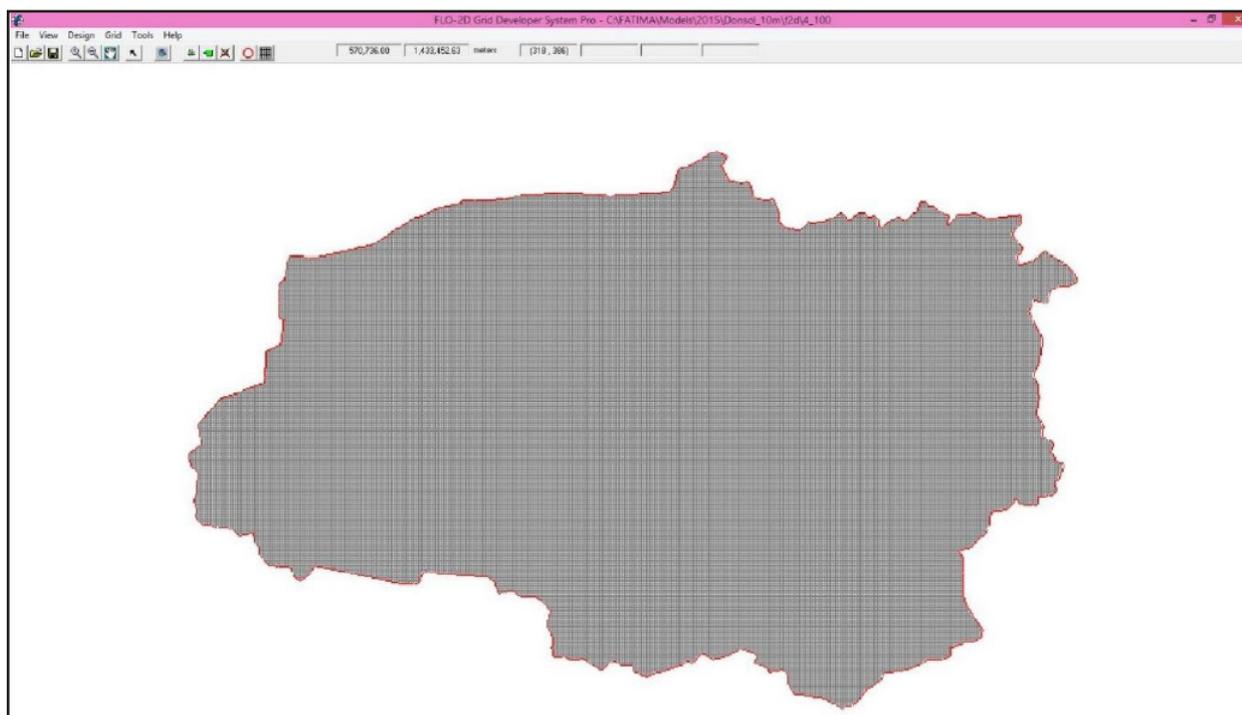
Figure 56. Screenshot of subcatchment with the computational area to be modeled in FLO-2D Grid Developer System Pro (FLO-2D GDS Pro)
