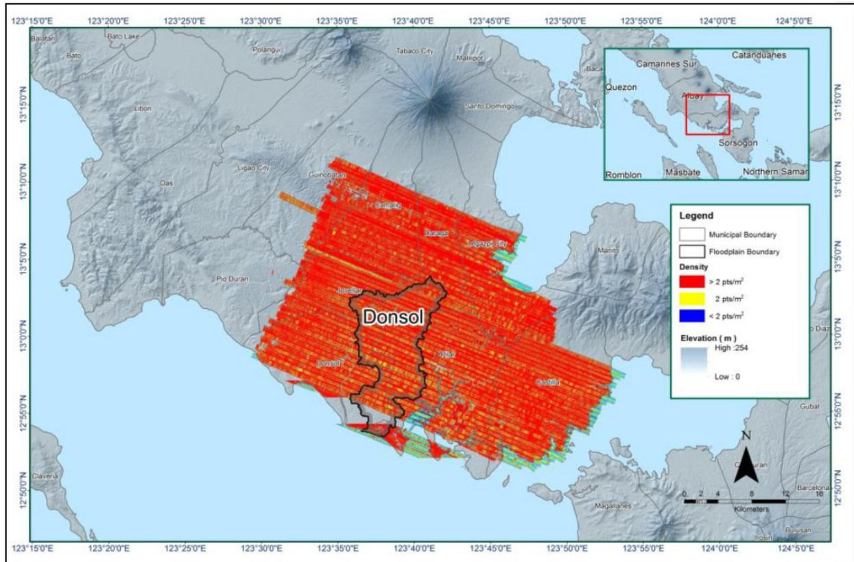
Figure 14. Pulse Density map of merged LiDAR data for Donsol Floodplain
