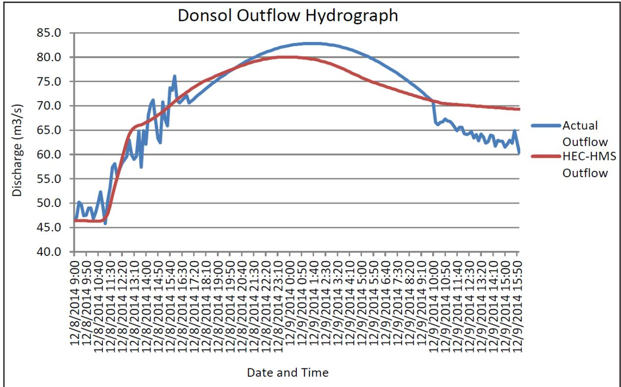
Figure 57. Outflow hydrograph of Donsol River Basin produced by the HEC-HMS model compared with observed outflow
