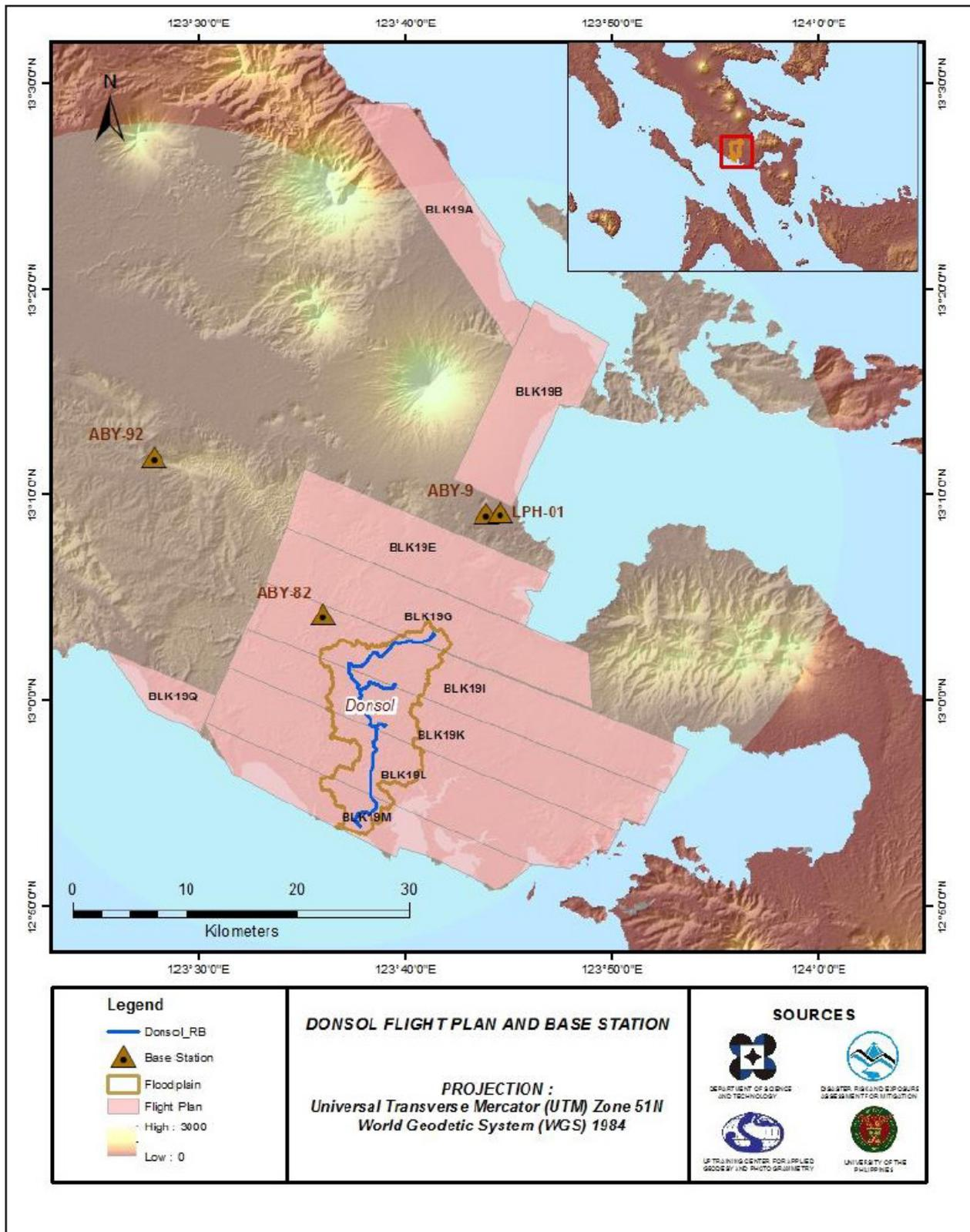
Figure 2. Flight Plan and base stations used for the Donsol Floodplain survey.
