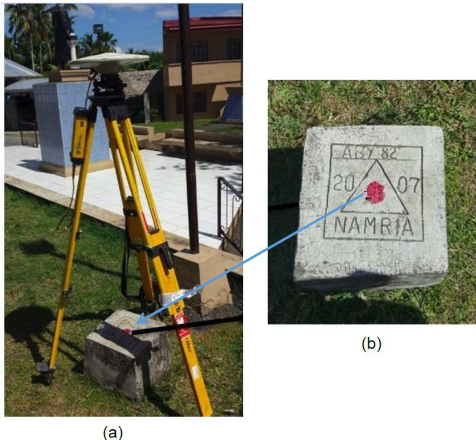
Figure 3. GPS set-up over ABY-82 located at about 12 meters from the right corner of the Rizal monument in front of Jovellar Catholic Church (a) and NAMRIA reference point SMR-53 (b) as recovered by the field team
