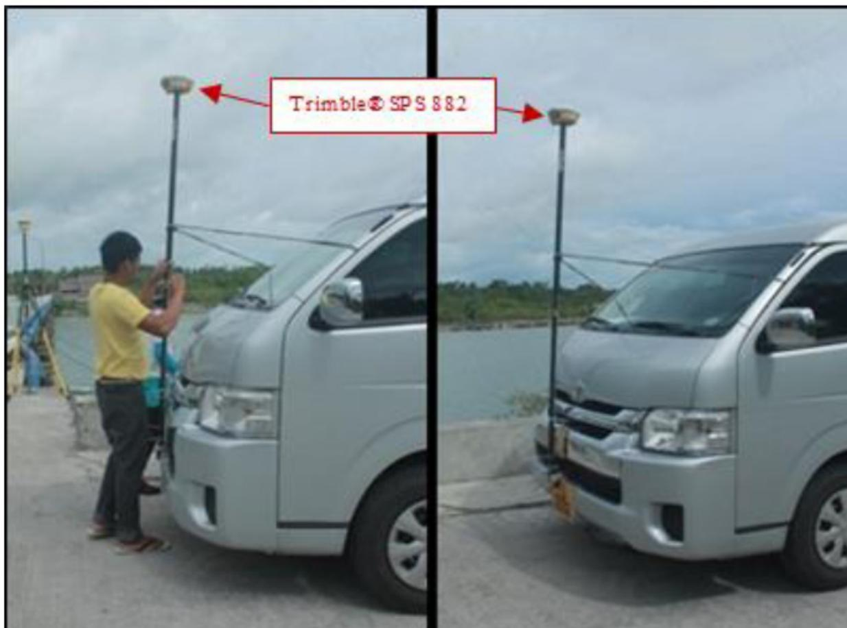
Figure 40. Validation Points Acquisition survey setup
