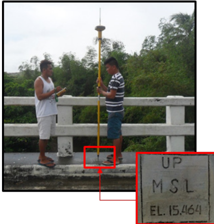
Figure 43. Water surface elevation marking on Baldoza Bridge sidewalk
