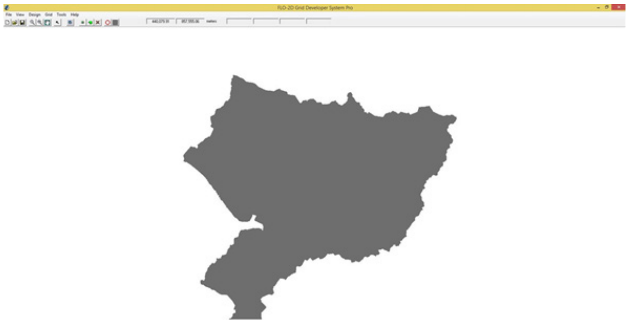
Figure 67. Screenshot of subcatchment with the computational area to be modeled in FLO-2D Grid Developer System Pro (FLO-2D GDS Pro)
