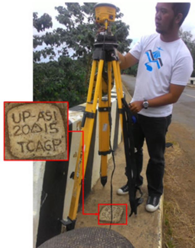
Figure 33. GNSS receiver setup, Trimble® SPS 985, at UP-ASI, located Brgy. Cayabon, Municipality of Milagros, Masbate
