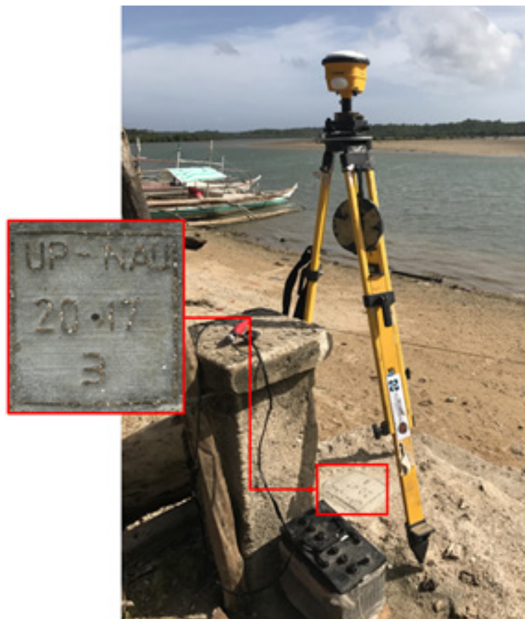
Figure 37. GNSS receiver setup, Trimble® SPS 985, at UP-NAU3, located in Brgy. Taboc, Municipality of Placer, Masbate
