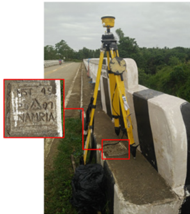
Figure 36. GNSS receiver setup, Trimble® SPS 985, at MST-45, located in Brgy. Villahermosa, Municipality of Cawayan, Masbate
