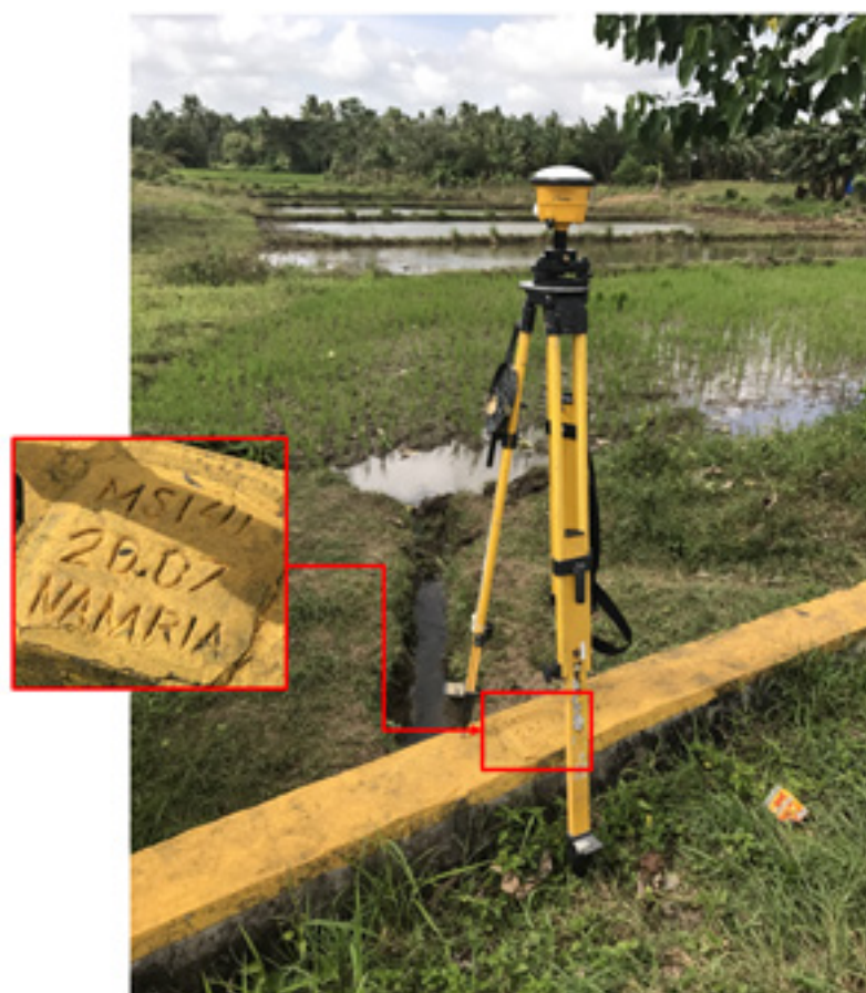
Figure 34. GNSS receiver setup, Trimble® SPS 985, at MS-141, located in Brgy. San Vicente, Municipality of Cawayan, Masbate
