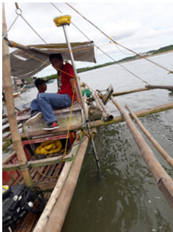
Figure 49. Gathering of random bathymetric points along Guiom River
