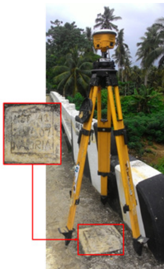
Figure 35. GNSS receiver setup, Trimble® SPS 985, at MST-41, located in Brgy. Gaid, Municipality of Dimasalang, Masbate
