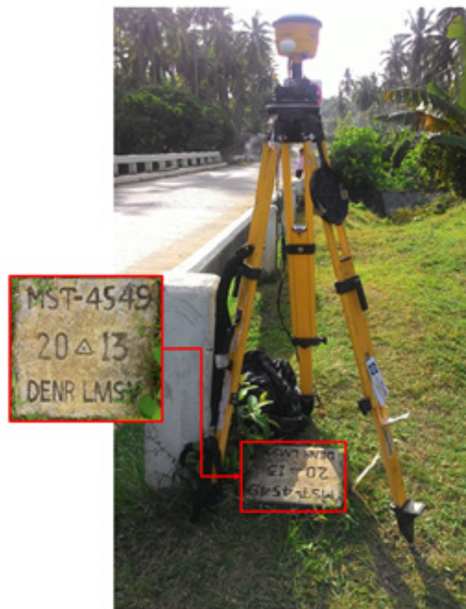
Figure 32. GNSS base set up, Trimble® SPS 985, at MST-4549, located in Brgy. Canjunday, Municipality of Baleno, Masbate
