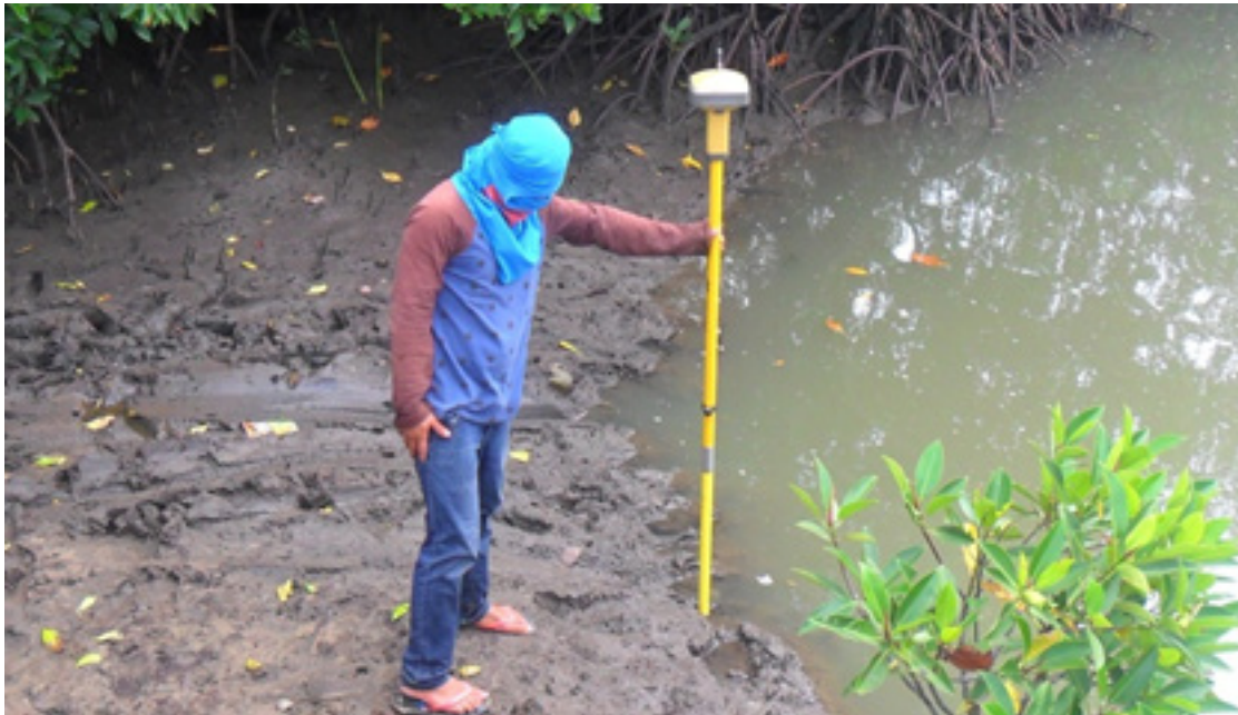
Figure 48. Manual bathymetric survey using a using Topcon™ GR-5 in Guiom River
