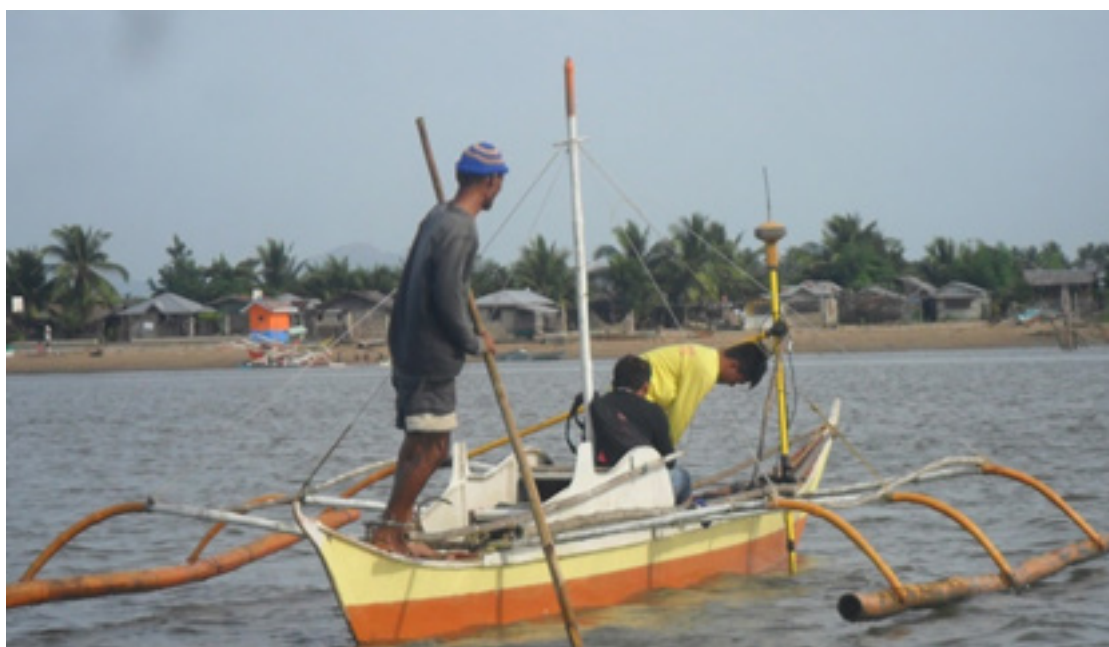
Figure 47. Bathymetric survey using Topcon™ GR-5 in Guiom River
