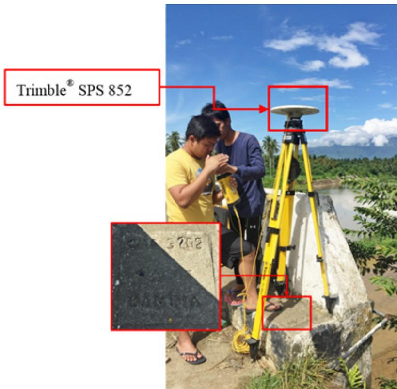
Figure 31. GNSS receiver setup, Trimble® SPS 852, at CMS-3202, located at the approach of Lagonoy Bridge in Brgy. Ginorangan, Municipality of Lagonoy, Camarines Sur
