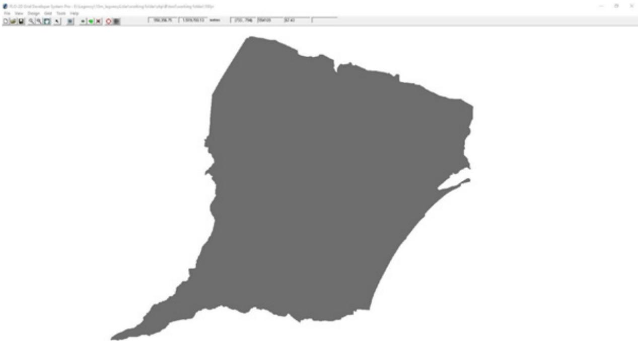
Figure 56. A screenshot of the river subcatchment with the computational area to be modeled in FLO-2D Grid Developer System Pro (FLO-2D GDS Pro)
