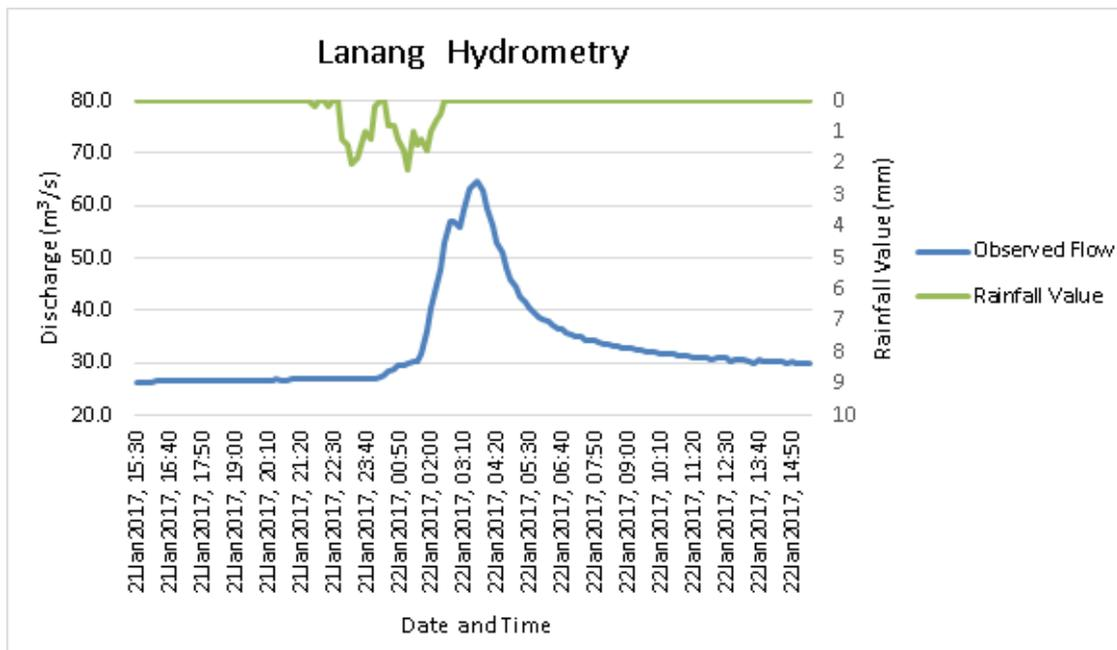
Figure 50. Rainfall and outflow data of the Lanang River Basin, which was used for modeling
