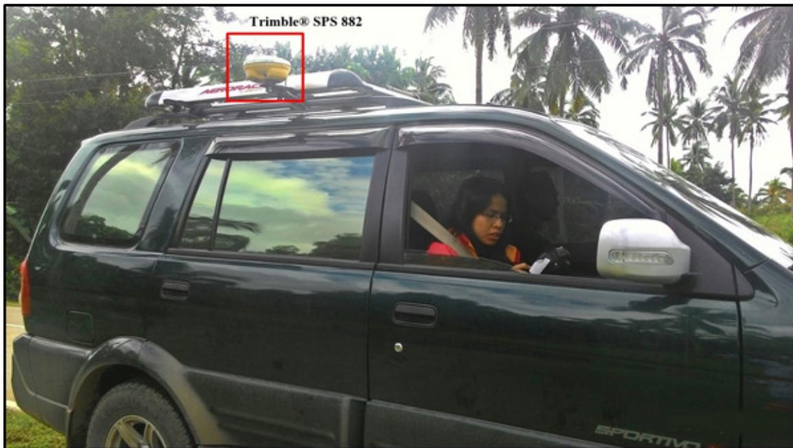
Figure 42. The validation points acquisition survey set-up using a GNSS receiver mounted on top of the vehicle along Lanang River Basin.
