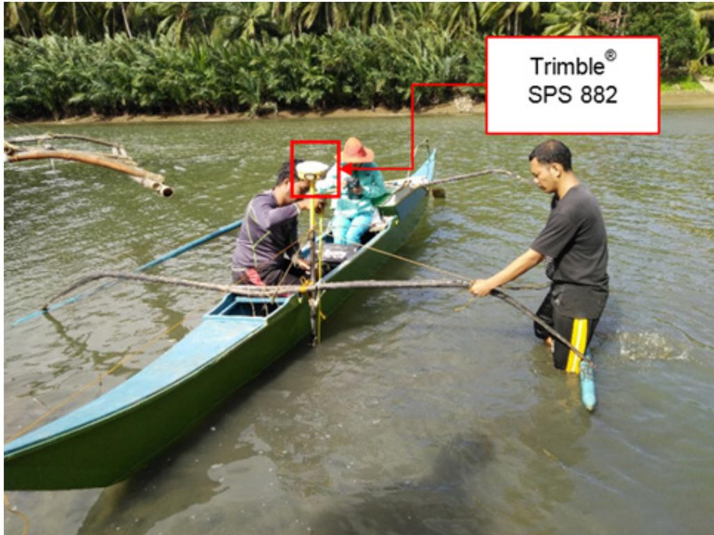
Figure 44. Bathymetric survey using a Trimble® SPS 882 in GNSS PPK in Lanang River
