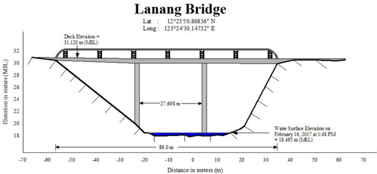
Figure 39. Lanang bridge cross-section survey drawn to scale
