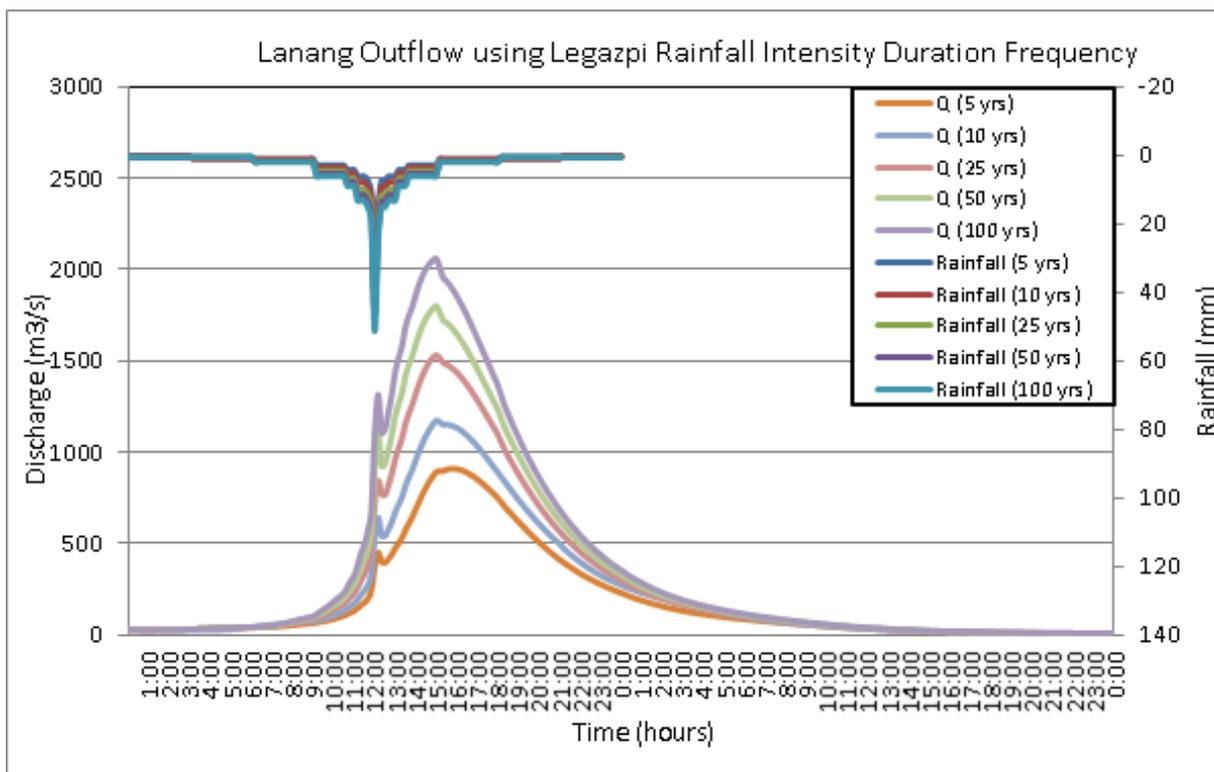
Figure 61. Outflow hydrograph at Lanang station generated using Legazpi RIDF simulated in HEC-HMS
