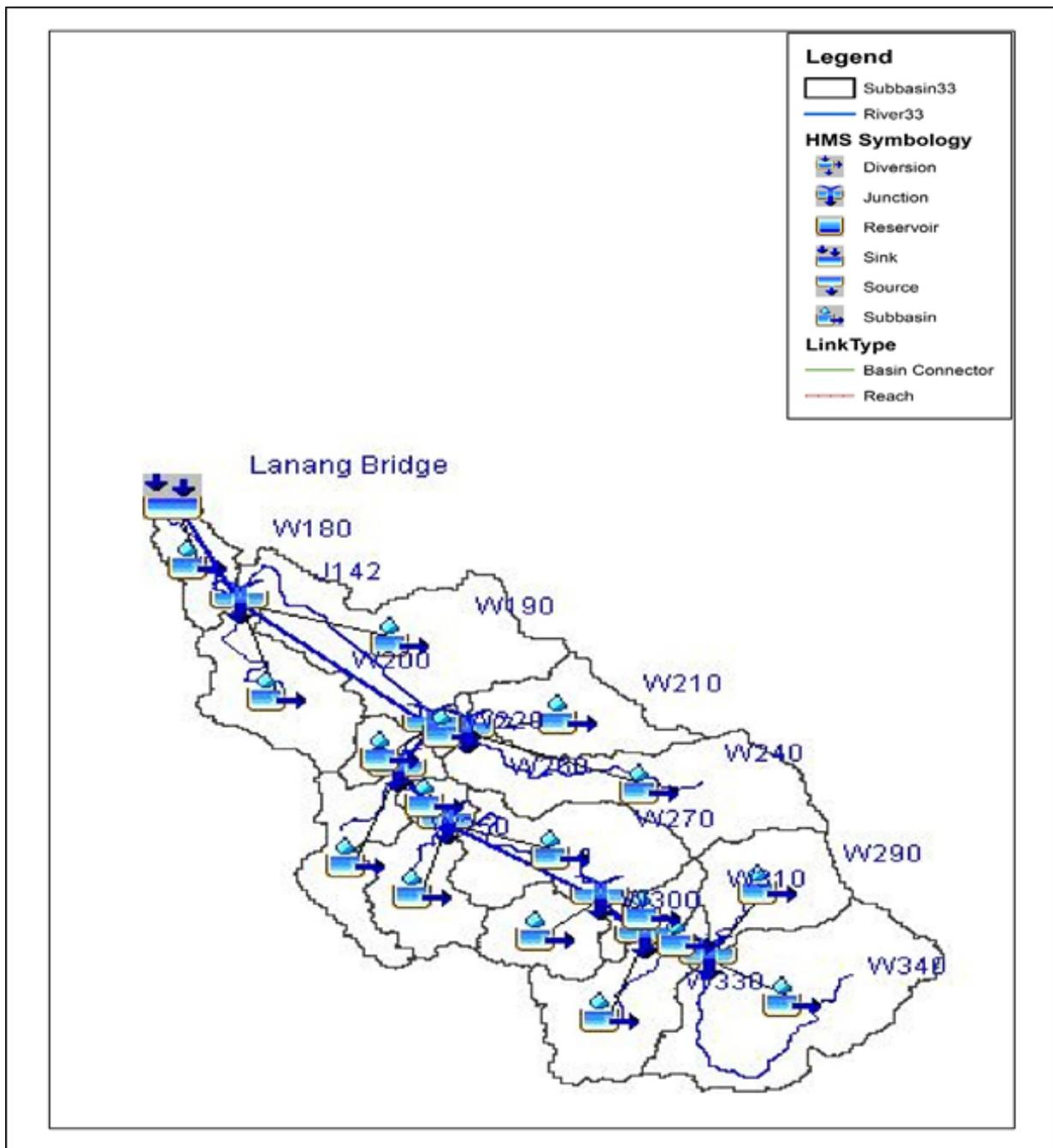
Figure 57. The Lanang Hydrologic Model generated in HEC-HMS
