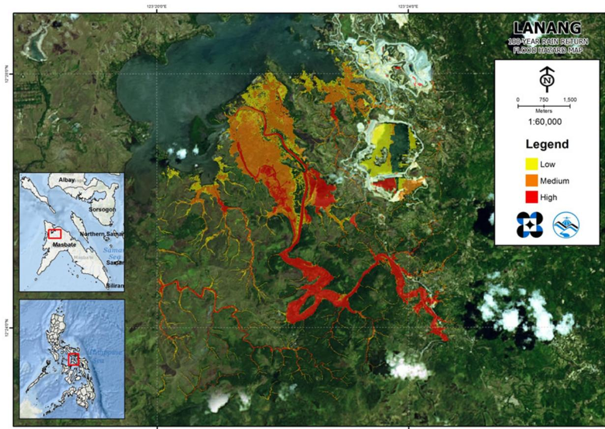
Figure 64. 100-year flood hazard map for the Lanang flood plain overlaid on Google Earth imagery
