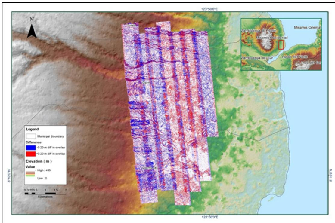
Figure A-8.12. Elevation difference between flight lines
