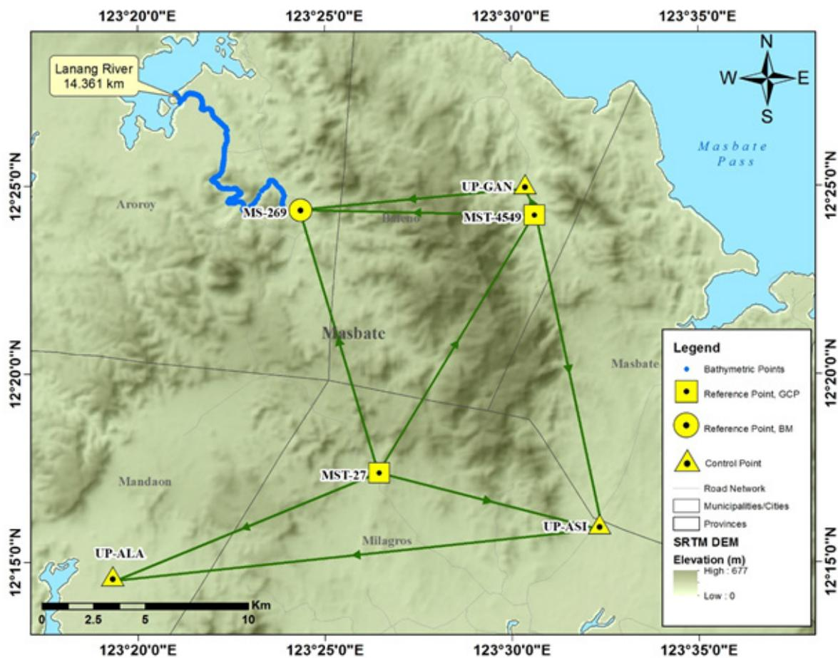
Figure 30. The GNSS Network established in the Lanang River
