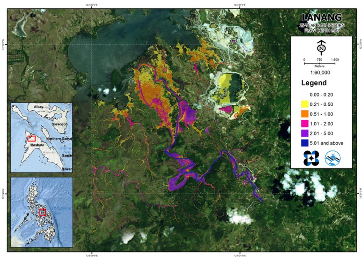
Figure 67. 25-year flow depth map for the Lanang flood plain overlaid on Google Earth imagery.
