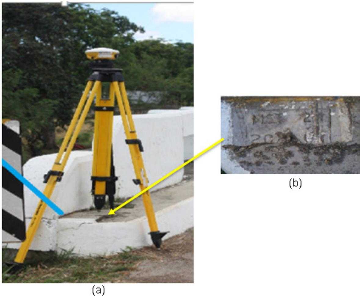
Figure 3. GPS set-up over MST-28 in Mambog Bridge, Barangay Bat-ongan, Municipality of Mandaon, Masbate (a) and NAMRIA reference point MST-28 (b) as recovered by the field team.
