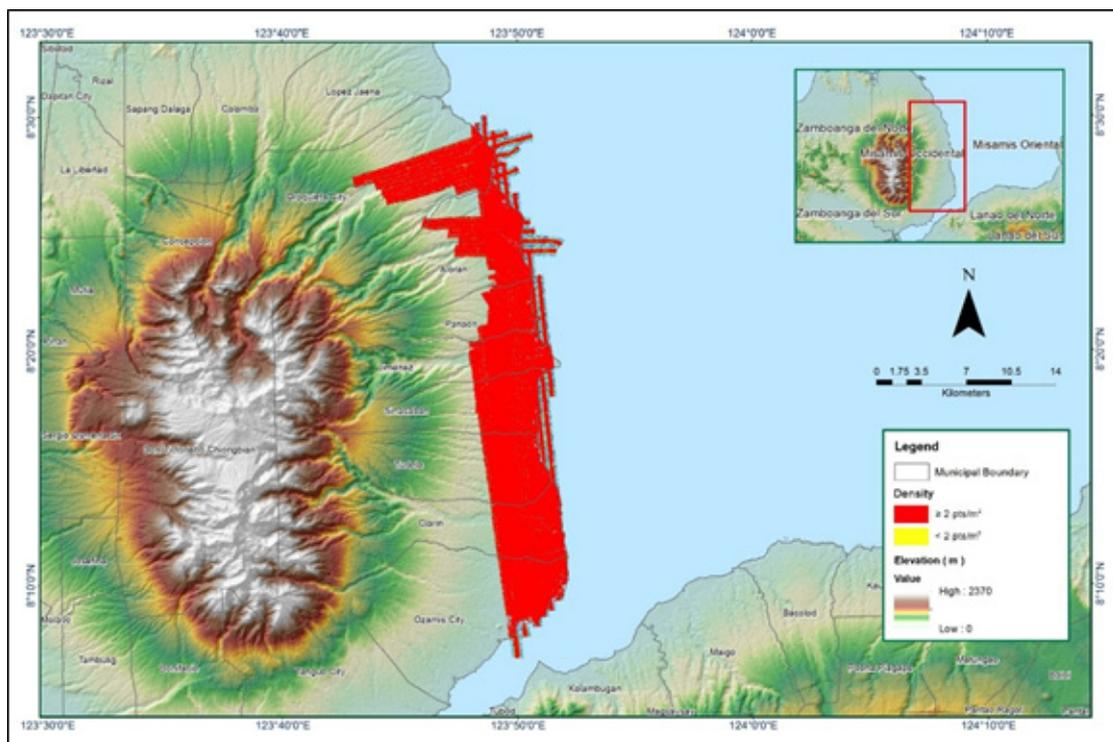
Figure A-8.17. Density map of merged LiDAR data
