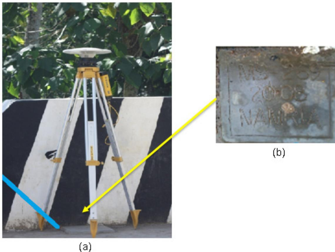
Figure 5. GPS set-up over MS-269 in Luy-a Bridge in Barangay Luy-a, Municipality of Aroroy, Masbate (a) and NAMRIA reference point MS-269 (b) as recovered by the field team.
