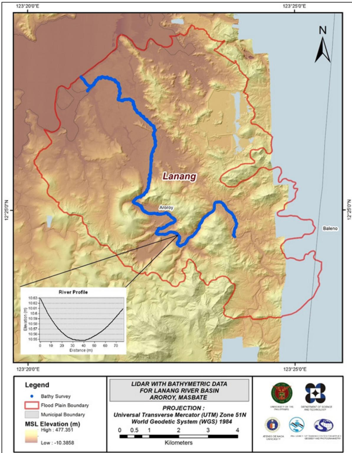
Figure 26. Map of Lanang Floodplain with bathymetric survey points in blue.
