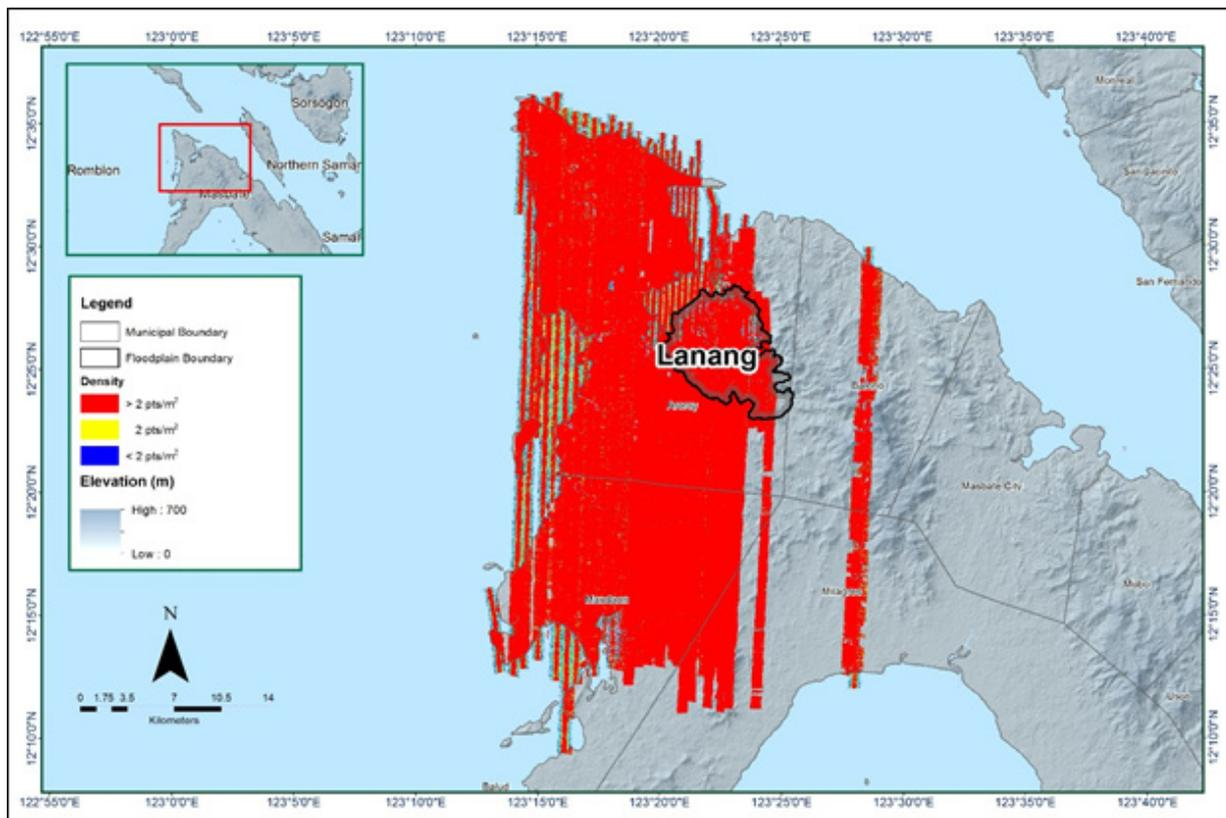
Figure 13. Pulse density map of merged LiDAR data for Lanang floodplain.
