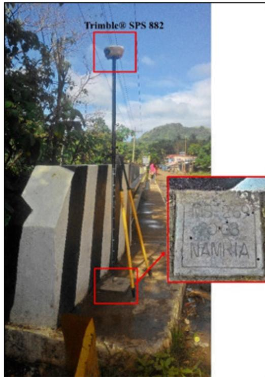
Figure 31. GNSS base set up, Trimble® SPS 882 at MS-269 benchmark located at Lanang Bridge, along Central Nautical Highway in Brgy. Luy-A, Aroroy, Masbate.
