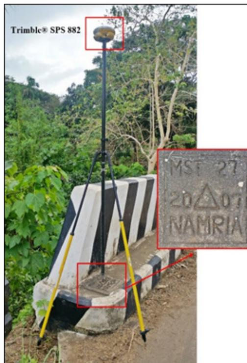
Figure 32. GNSS receiver set up, Trimble® SPS 882 at MST-27, a second order GCP located at Mabuaya Bridge along Central Nautical Highway in Brgy. Matiporon, Milagros, Masbate.
