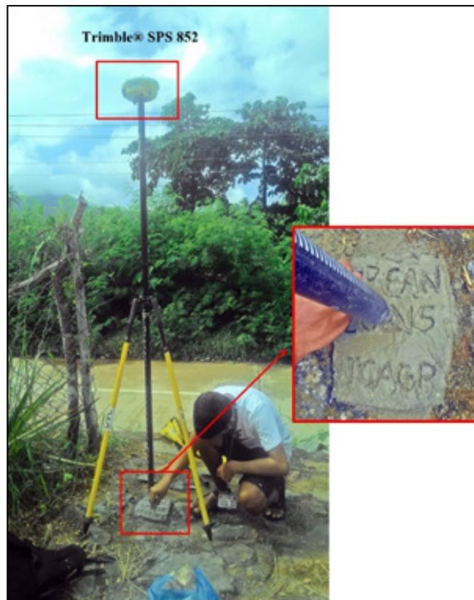
Figure 36. GNSS receiver setup, Trimble® SPS 882, at UP-GAN, an established control point located on the top of a riprap near Gangao Bridge, along Central Nautical Highway, Brgy. Gangao, Baleno, Masbate.
