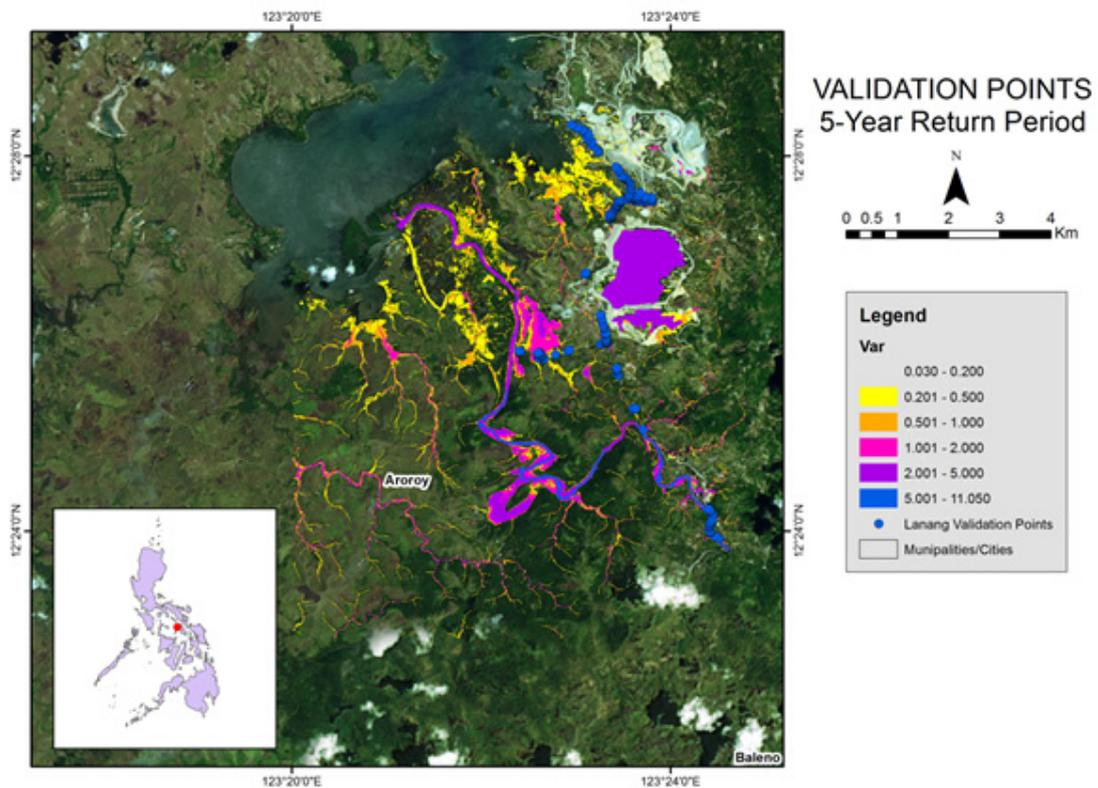
Figure 73. Validation points for the 5-Year Flood Depth Map of the Lanang Floodplain
