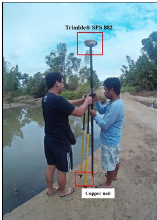
Figure 34. Trimble® SPS 882 setup at UP-ALA, an established control point located at Alas Bridge in Brgy. Alas, Mandaon, Masbate.
