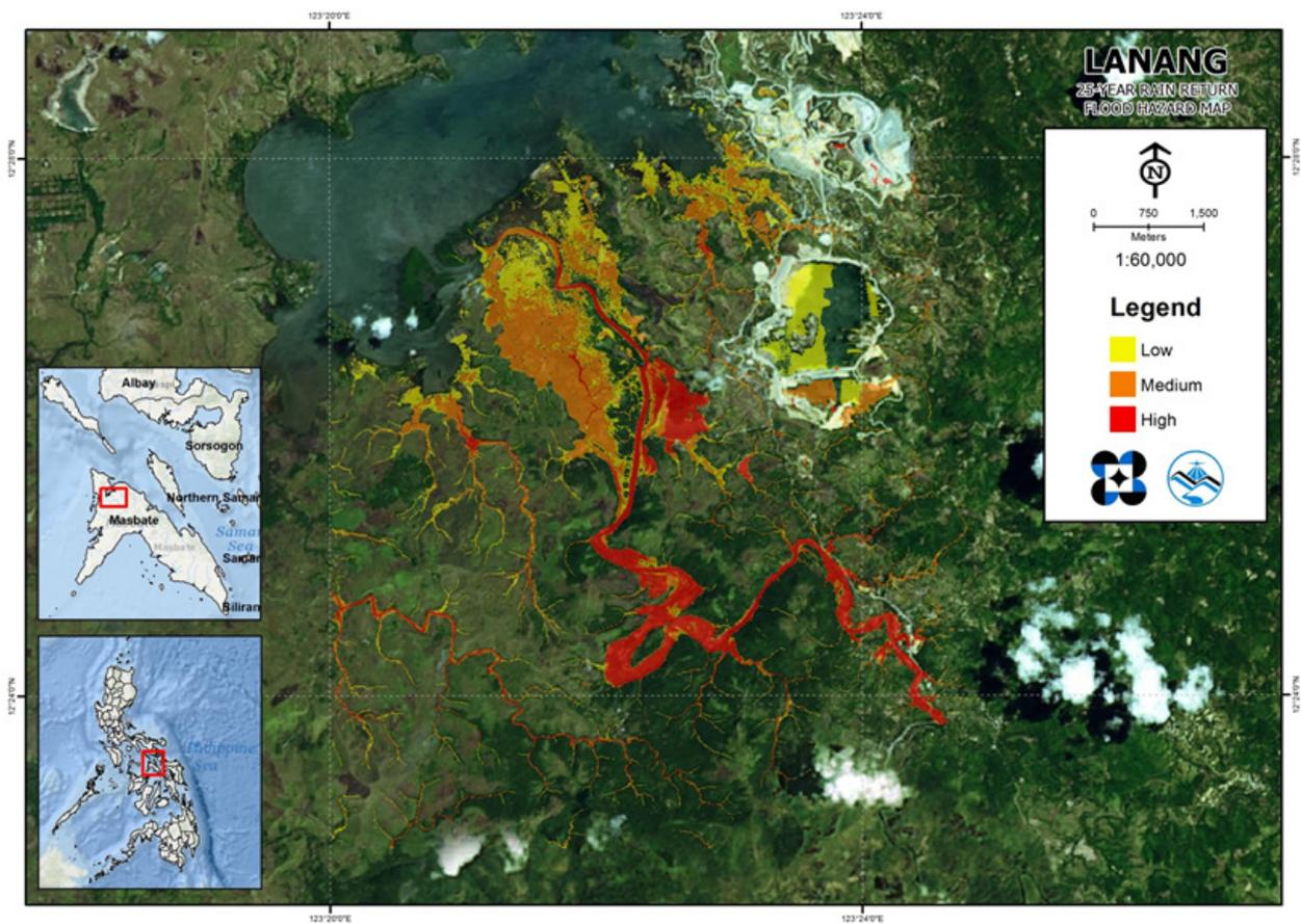
Figure 66. 25-year flood hazard map for the Lanang flood plain overlaid on Google Earth imagery.
