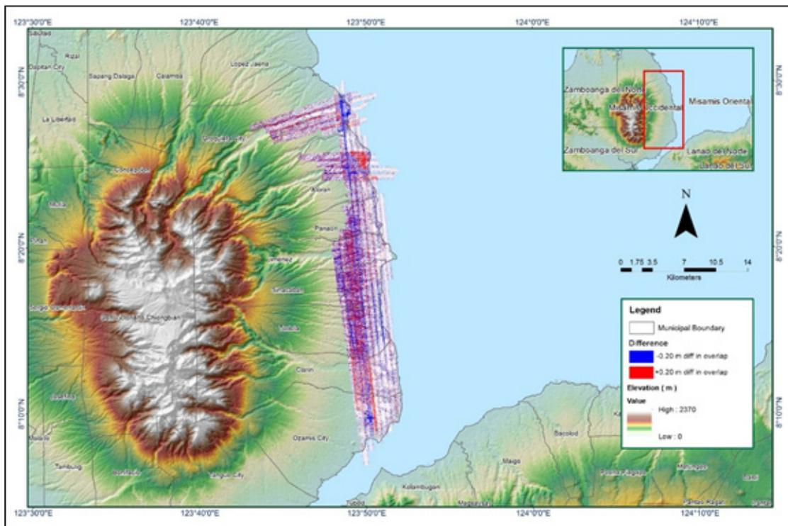
Figure A-8.18 Elevation difference between flight lines
