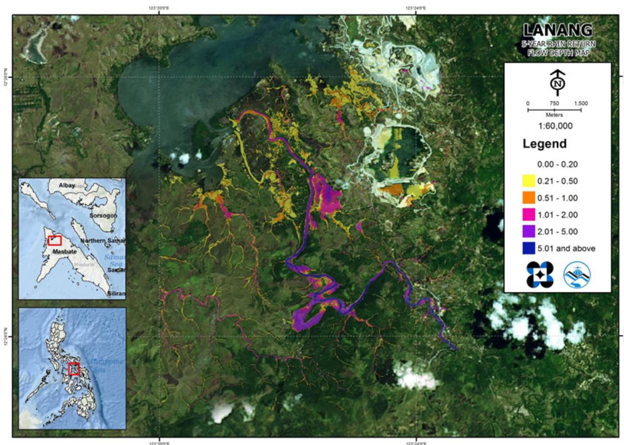
Figure 69. 5-year flow depth map for the Lanang flood plain overlaid on Google Earth imagery .
