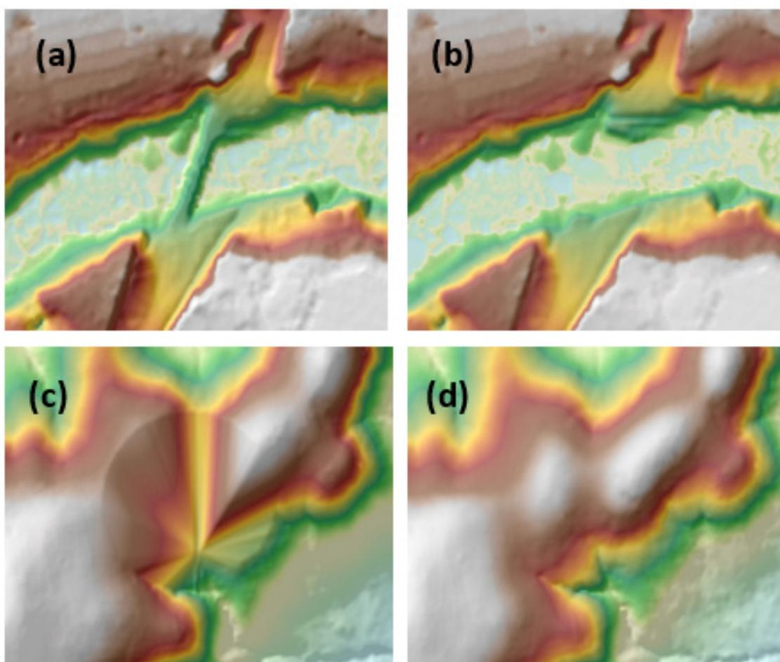
Figure 21. Portions in the DTM of Lanang floodplain – a bridge before (a) and after (b) manual editing; and an elevated area before (c) and after (d) data retrieval.
