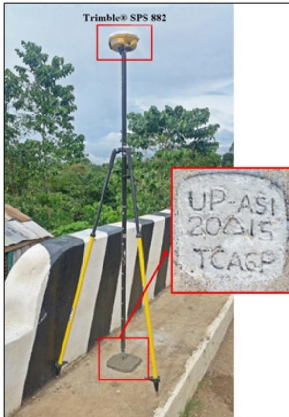
Figure 35. GNSS receiver setup, Trimble® SPS 882, at UP-ASI, an established control point located at Asid Bridge, along Central Nautical Highway, Brgy. Asid, Masbate City.
