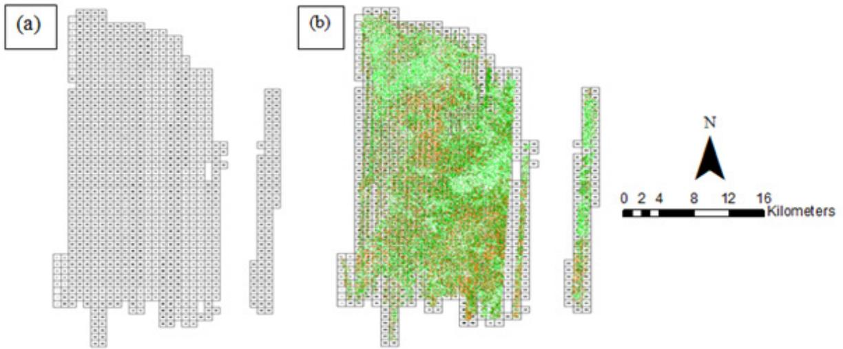
Figure 16. Tiles for Lanang floodplain (a) and classification results (b) in TerraScan.
