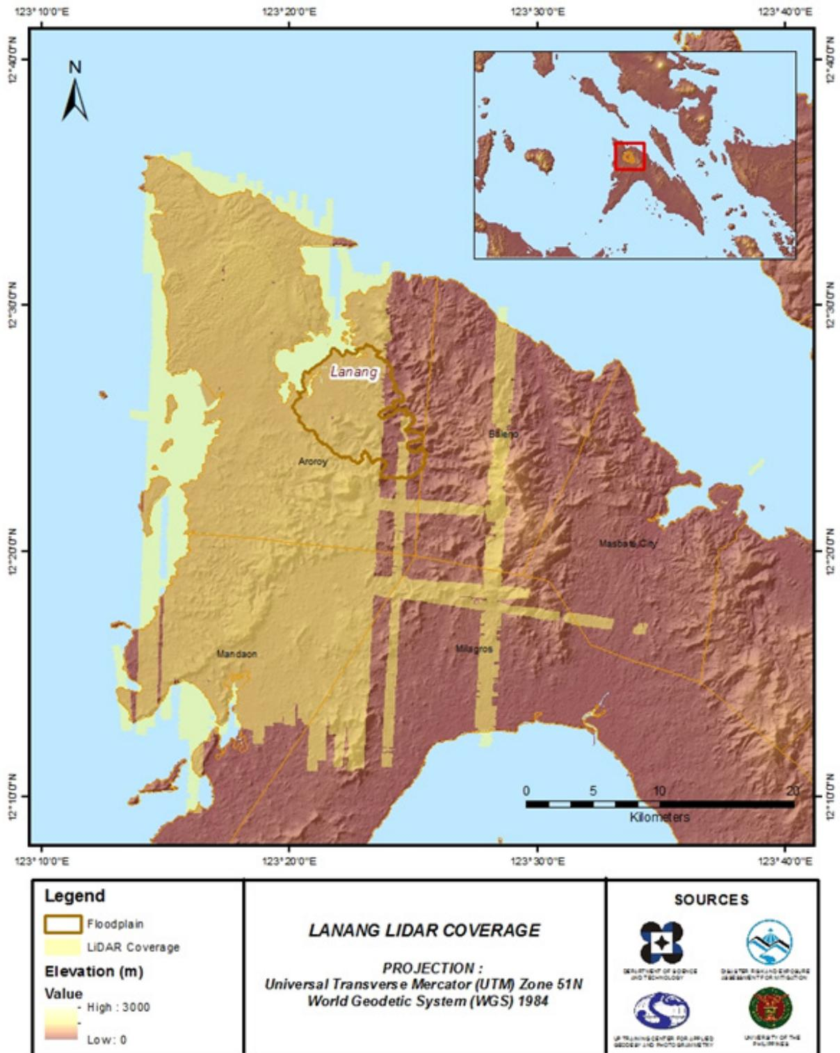
Figure 6. Actual LiDAR data acquisition of the Lanang floodplain.
