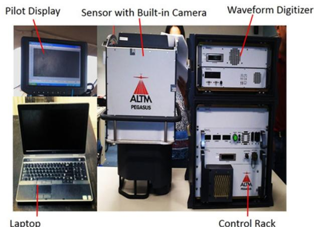
Parameters and Specifications of the OPTECH Sensor
