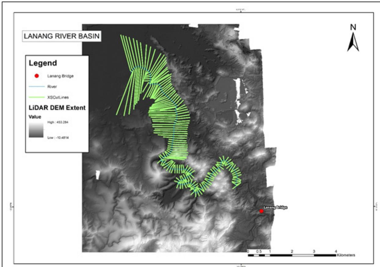
Figure 58. River cross-section of Lanang River through Arcmap HEC GeoRAS tool
