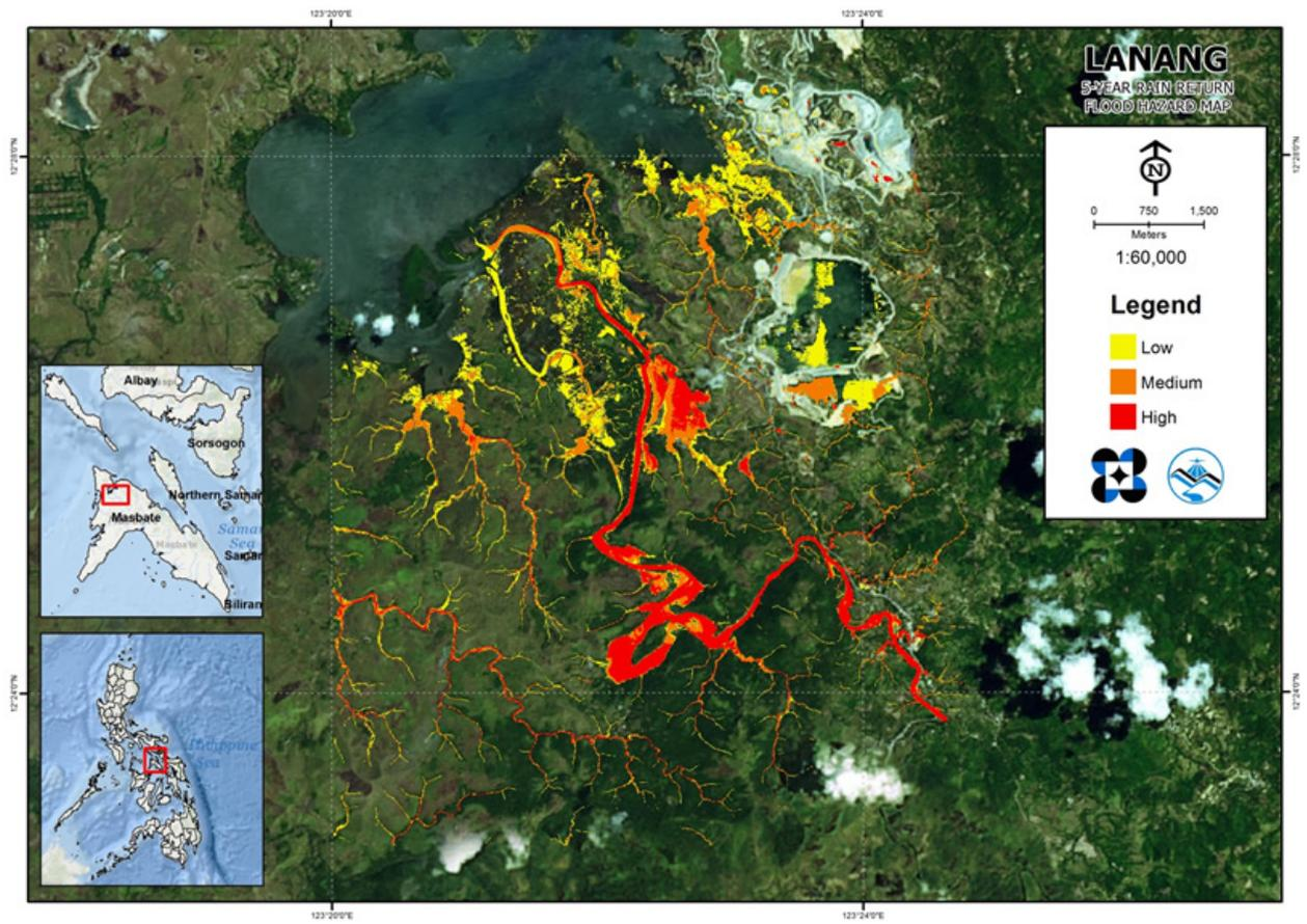
Figure 68. 5-year flood hazard map for the Lanang flood plain overlaid on Google Earth imagery.
