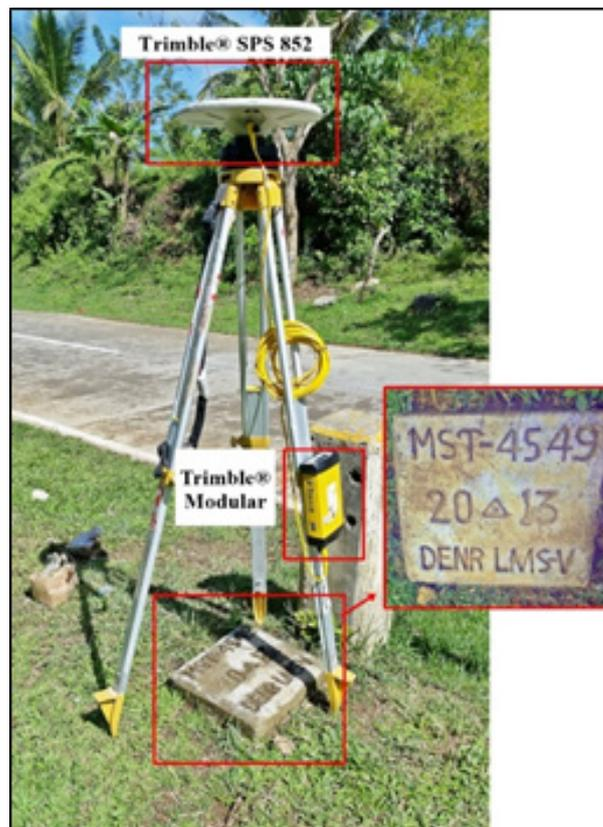
Figure 33. Trimble® SPS 852 base setup at MST-4945, a DENR-established control point located at the approach of Cancahorao Bridge along Central Nautical Highway in Brgy. Gangao, Baleno, Masbate.
