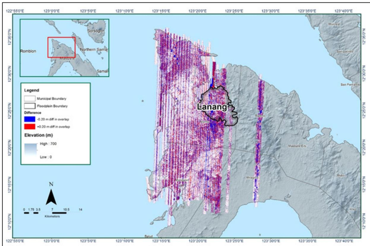
Figure 14. Elevation difference map between flight lines for Lanang floodplain.
