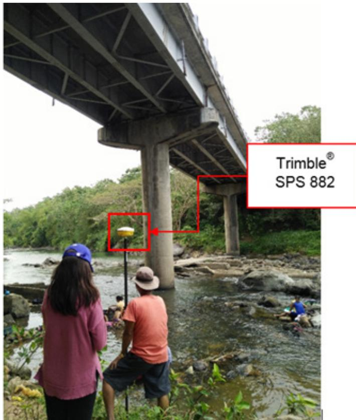
Figure 37. Cross-section survey on the downstream side of Lanang Bridge
