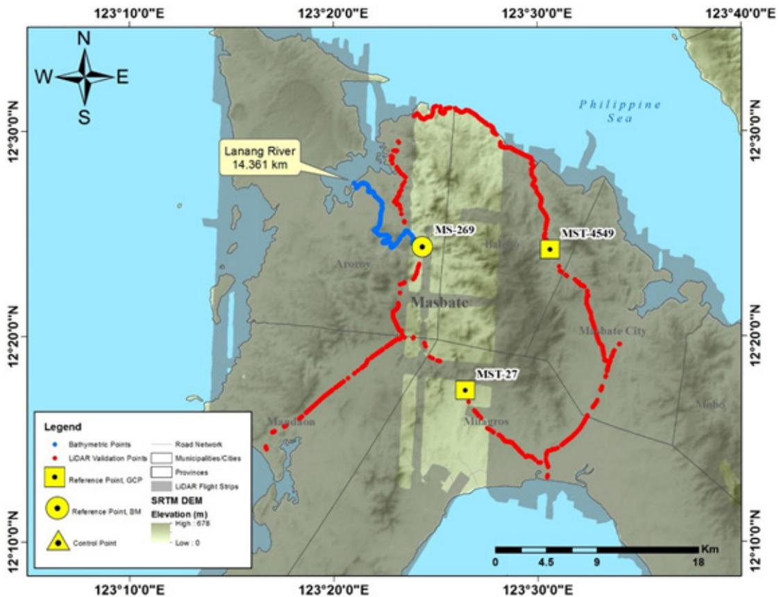
Figure 43. Extent of the LiDAR ground validation survey of the Lanang River basin
