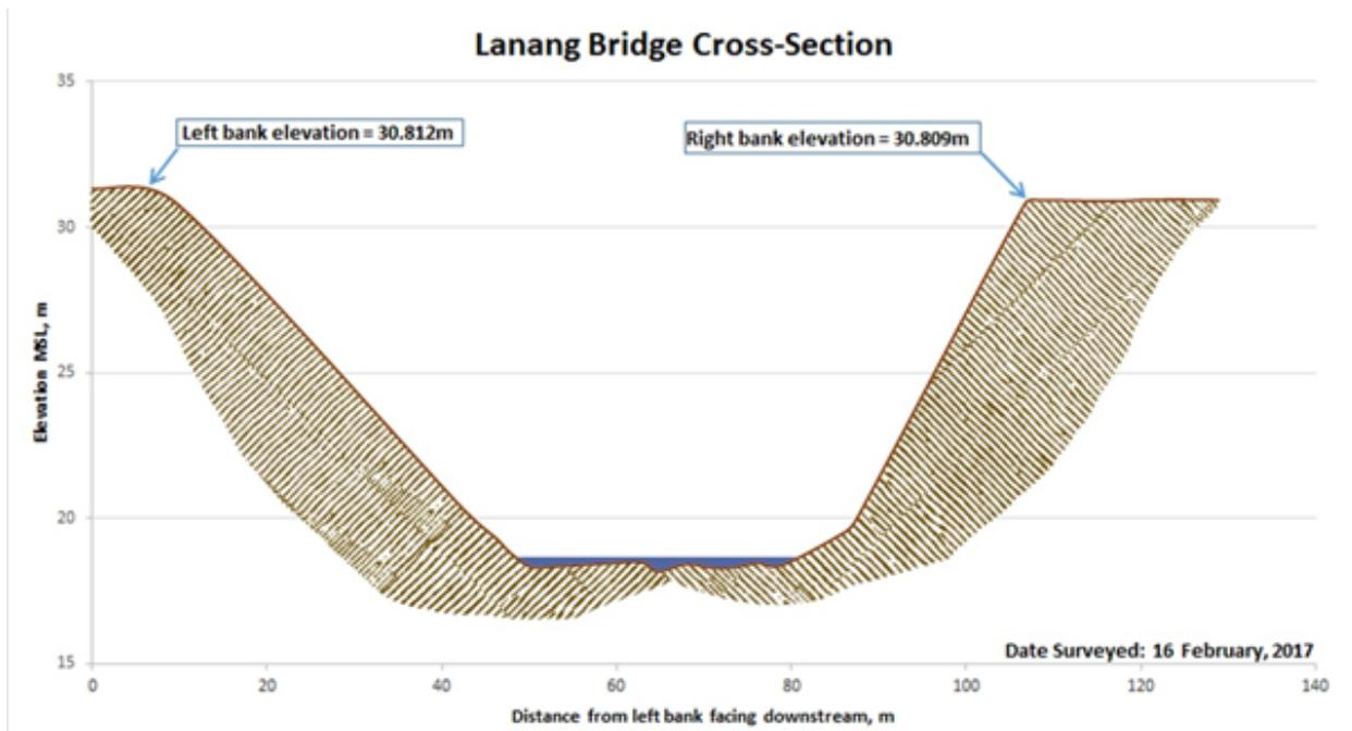
Figure 48. Cross-Section Plot of Lanang Bridge
