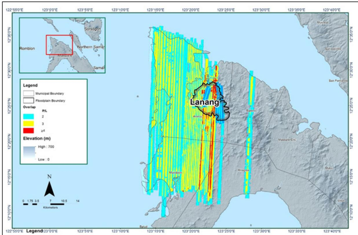
Figure 12. Image of data overlap for Lanang floodplain.
