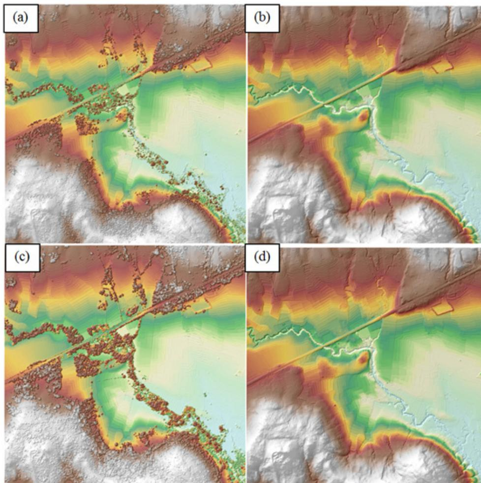
Figure 18. The production of last return DSM (a) and DTM (b), first return DSM (c) and secondary DTM (d) in some portion of Lanang floodplain.
