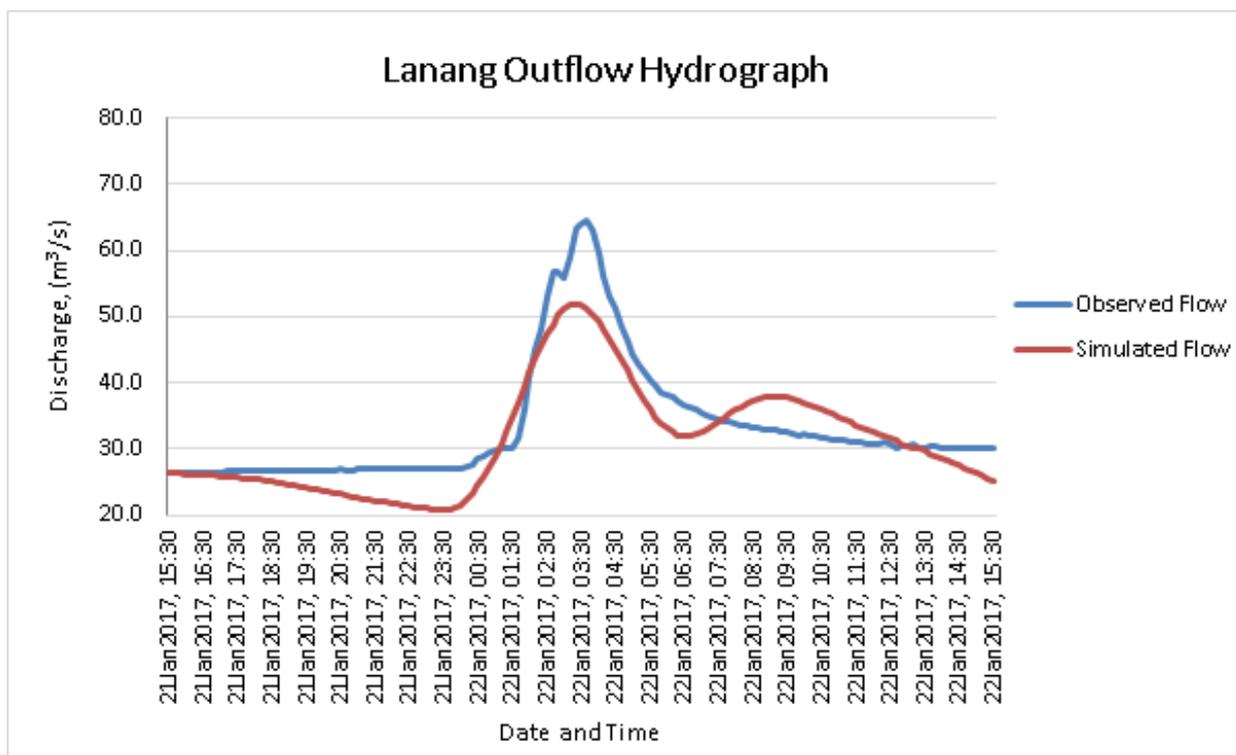
Figure 60. Outflow hydrograph of Lanang River Basin produced by the HEC-HMS model compared with observed outflow.
