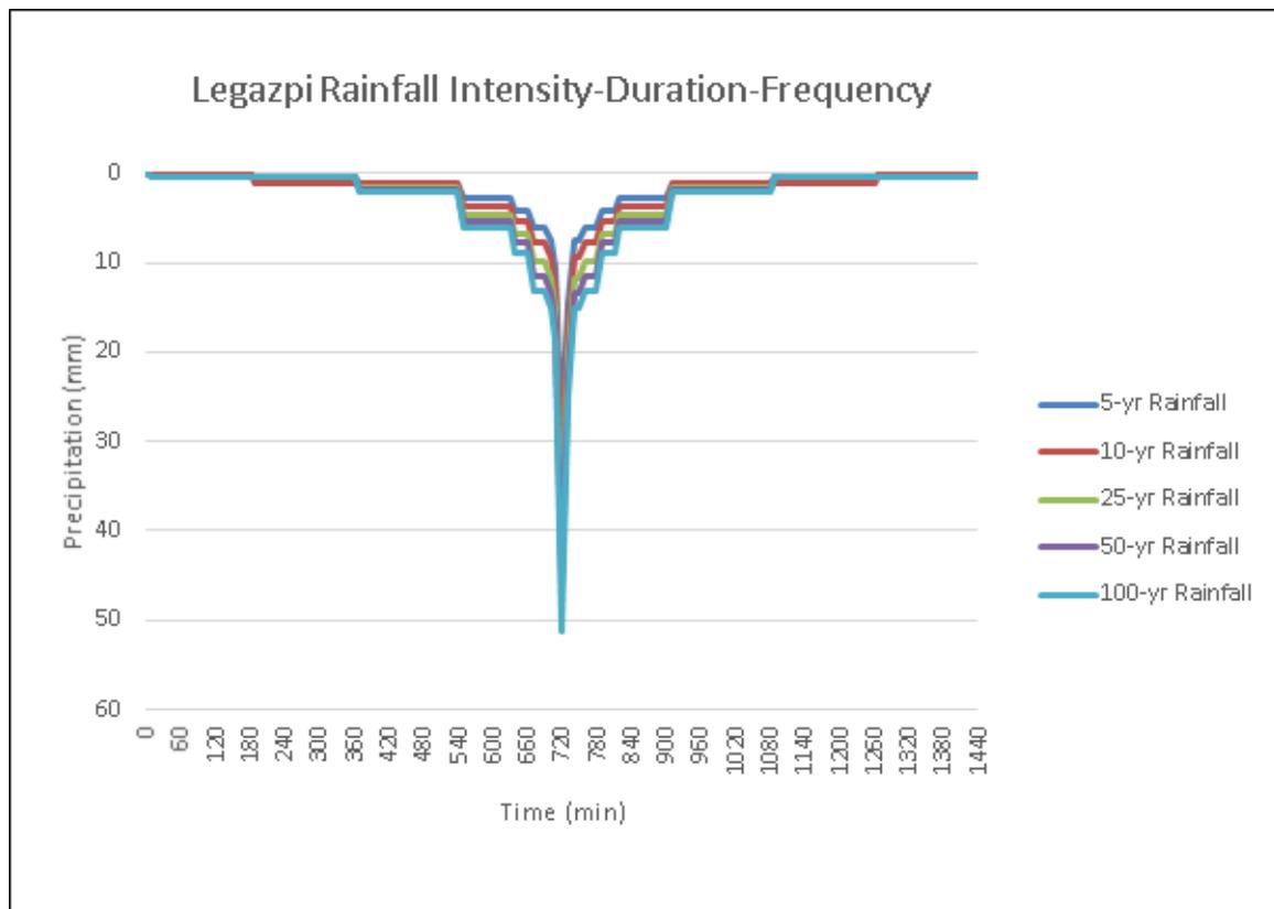
Figure 52. Synthetic storm generated for a 24-hour period rainfall for various return periods
