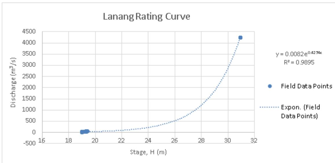
Figure 49. Rating Curve at Lanang Bridge, Masbate City.
