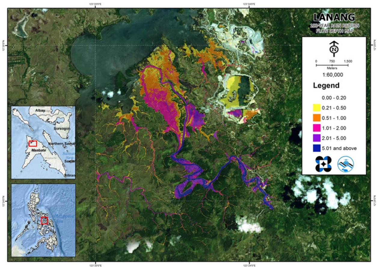
Figure 65. 100-year flow depth map for the Lanang flood plain overlaid on Google Earth imagery.
