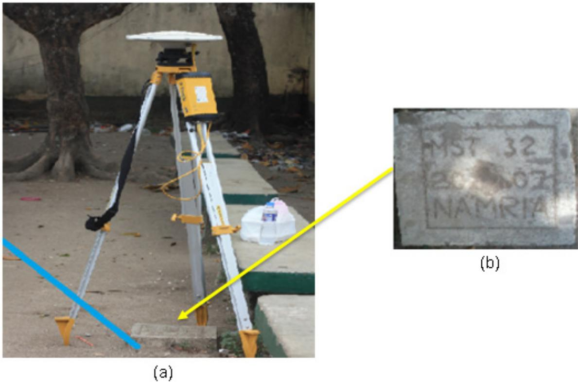
Figure 4. GPS set-up over MST-32 in Sagawsawan Bridge, Barangay Umabay Exterior, Municipality of Mobo, Masbate (a) and NAMRIA reference point MST-32 (b) as recovered by the field team.
