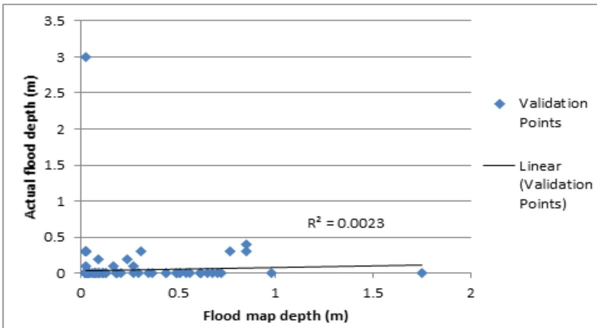
Figure 74. Flood depth map vs. Actual flood depth.
