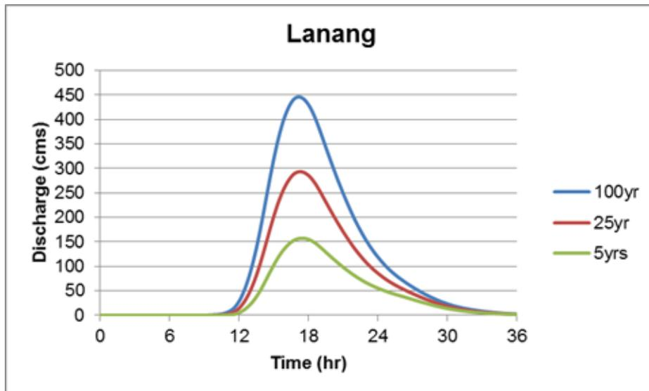
Figure 62. Lanang river generated discharge using 5-, 25-, and 100-year Legazpi rainfall intensity-duration-frequency (RIDF) in HEC-HMS.
