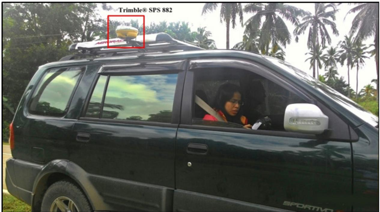
Figure 44 Validation points acquisition survey set-up: A Trimble® SPS 882, mounted on top of the vehicle
