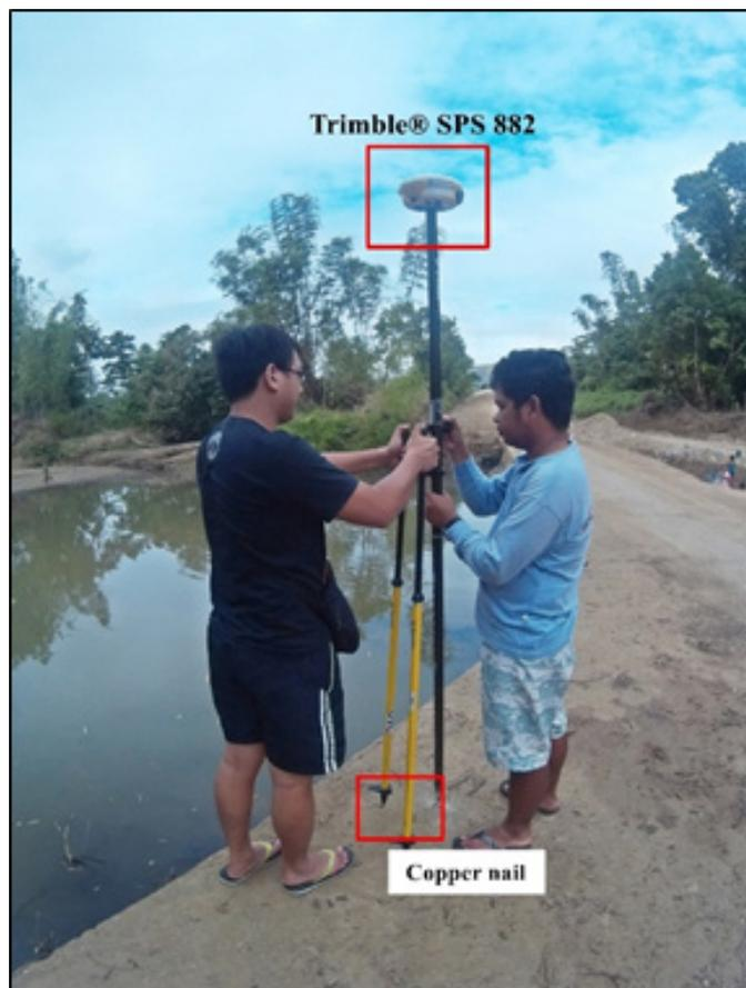
Figure 37 Trimble®SPS 882 set-up at UP-ALA, located at Alas Bridge in Brgy. Alas, Mandaon, Masbate
