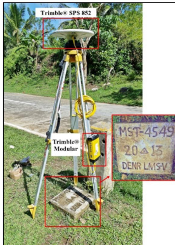
Figure 36 Trimble® SPS 852 base set-up at MST-4945, a DENR-established control point located at the approach of Cancahorao Bridge along Central Nautical Highway in Brgy. Gangao, Baleno, Masbate
