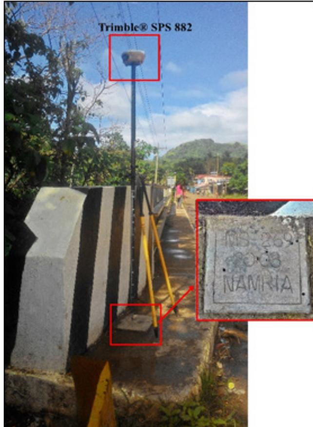
Figure 34 GNSS base set-up, Trimble® SPS 852at MS-269, located at Lanang Bridge, along Central Nautical Highway in Brgy. Luy-A, Aroroy, Masbate
