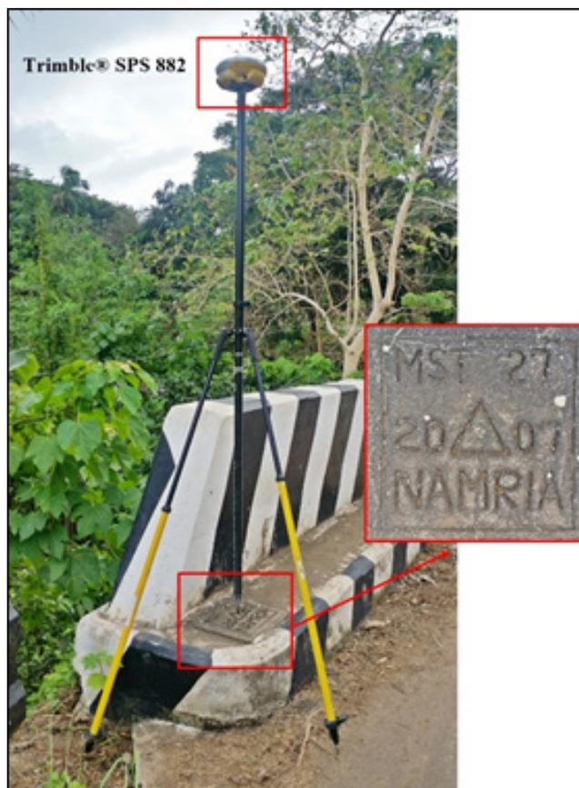
Figure 36. GNSS receiver, Trimble® SPS 882, at SE-85, located at the approach of the Llorente Bridge in Barangay II, Municipality of Llorente, Eastern Samar
