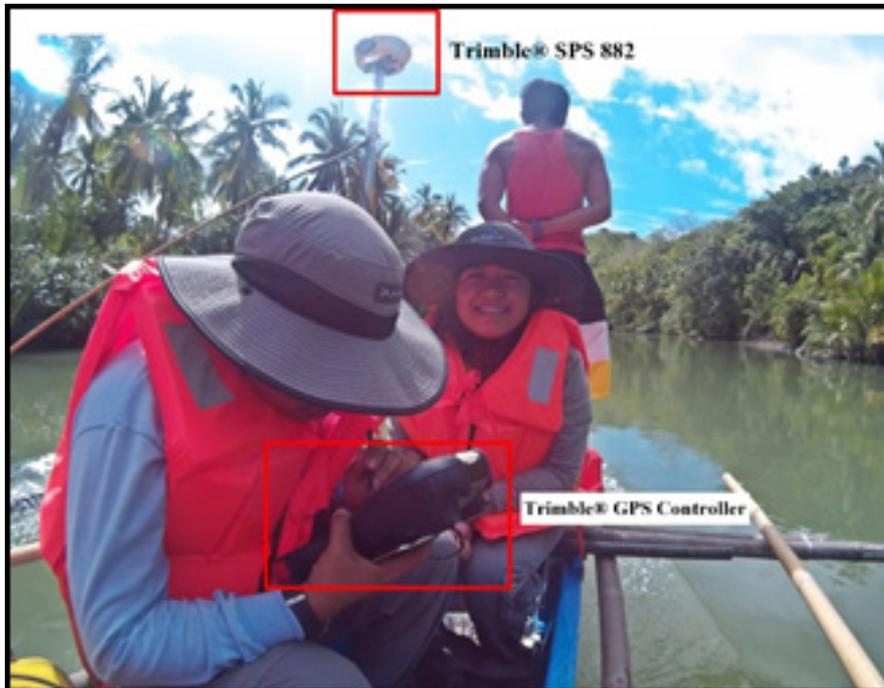
Figure 46 Bathymetric survey set-up using OHMEX™ single beam echo sounder and amounted with a Trimble® SPS 882
