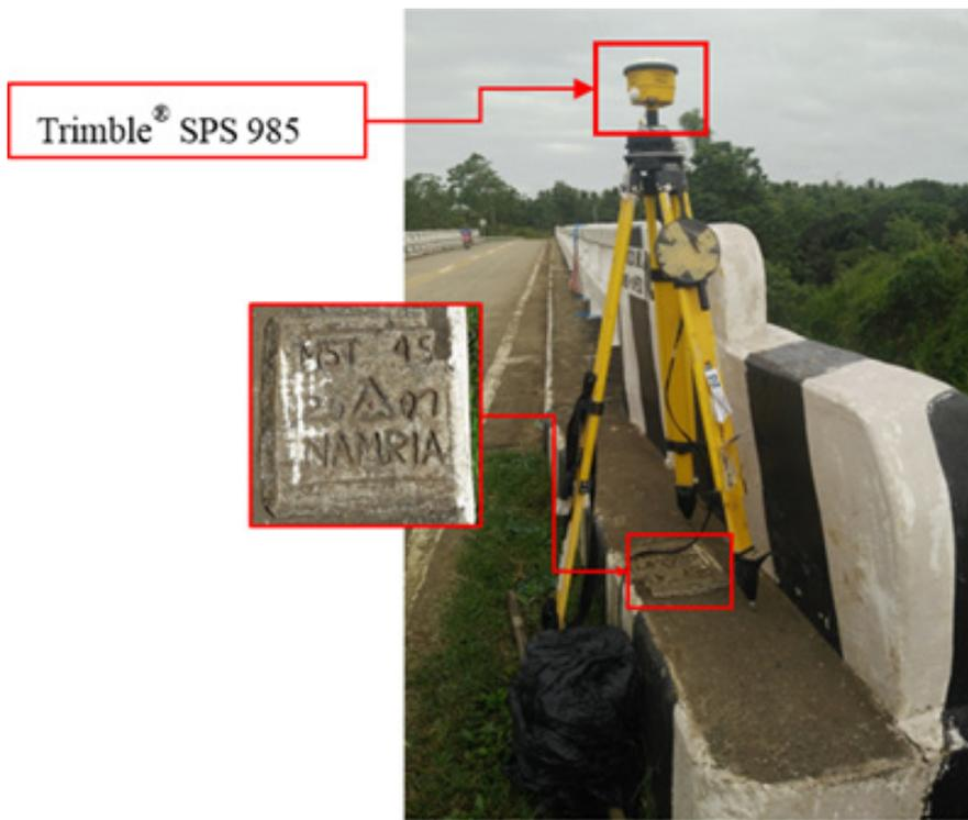
Figure 36. GNSS receiver setup, Trimble® SPS 985, at MST-45, located in Brgy. Villahermosa, Municipality of Cawayan, Masbate.
