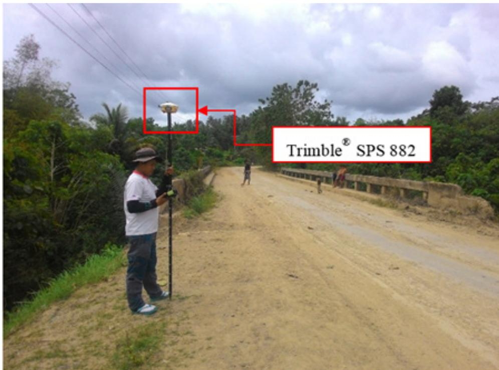
Figure 41. The Bridge As-Built Survey using PPK Survey Technique.
