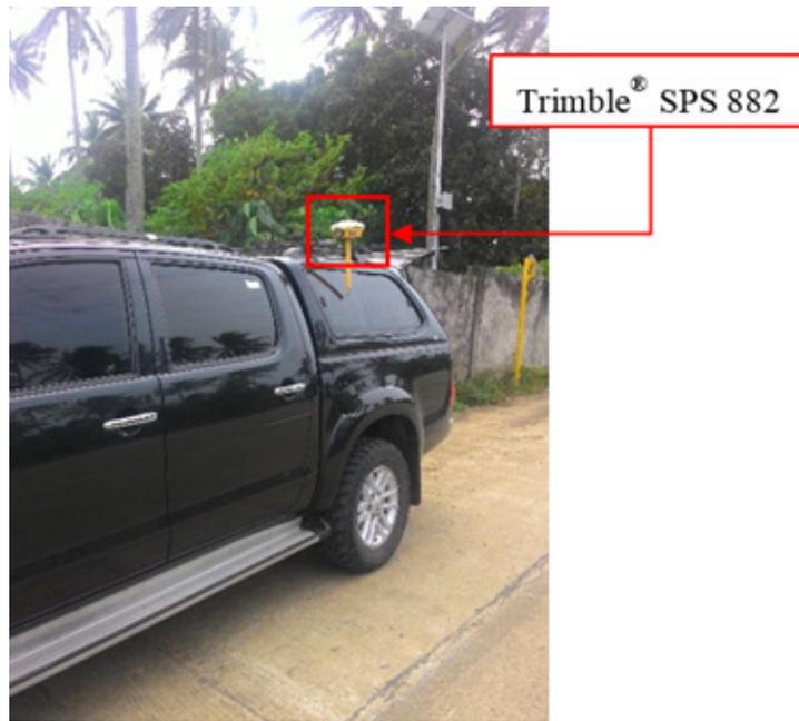
Figure 46. The validation point acquisition survey setup using a GNSS receiver fixed in a van along the Nainday River Basin.
