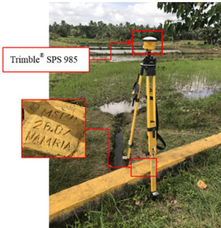
Figure 37. GNSS receiver setup, Trimble® SPS 985, at MS-141, located in Brgy. San Vicente, Municipality of Cawayan, Masbate.
