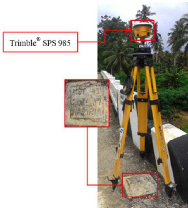
Figure 35. GNSS receiver setup, Trimble® SPS 985, at MST-41, located in Brgy. Gaid, Municipality of Dimasalang, Masbate.
