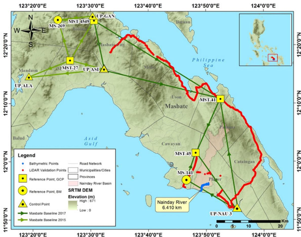
Figure 32. Extent of the bathymetric survey (in blue line) in Nainday River and the LiDAR data validation survey (in red).
