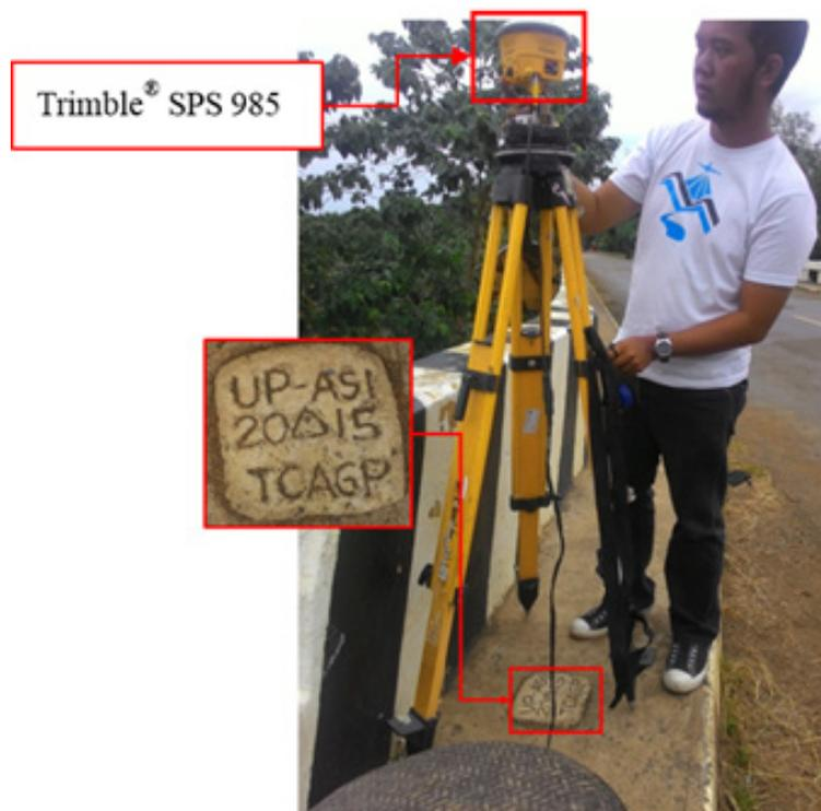
Figure 38. GNSS receiver setup, Trimble® SPS 985, at UP-ASI, located Brgy. Cayabon, Municipality of Milagros, Masbate.
