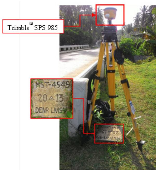
Figure 34. GNSS base set up, Trimble® SPS 985, at MST-4549, located in Brgy. Canjunday, Municipality of Baleno, Masbate.
