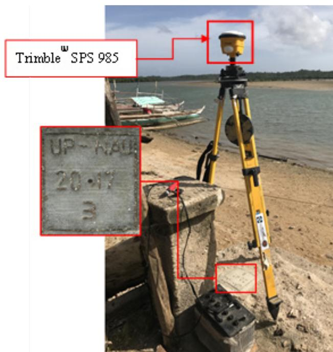
Figure 39. GNSS receiver setup, Trimble® SPS 985, at UP-NAU3, located in Brgy. Taboc, Municipality of Placer, Masbate.
