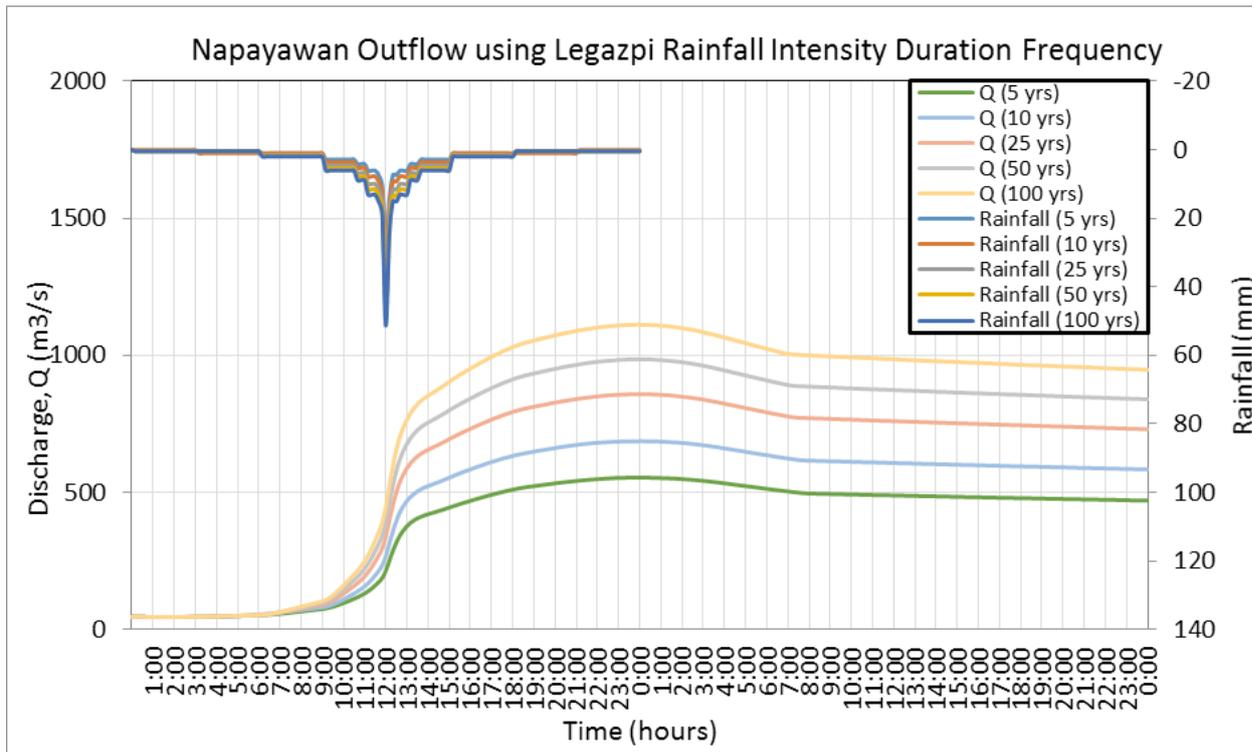
Figure 60. Outflow hydrograph at the Napayawan Basin generated using the simulated rain events for 24-hour period for Legazpi station
