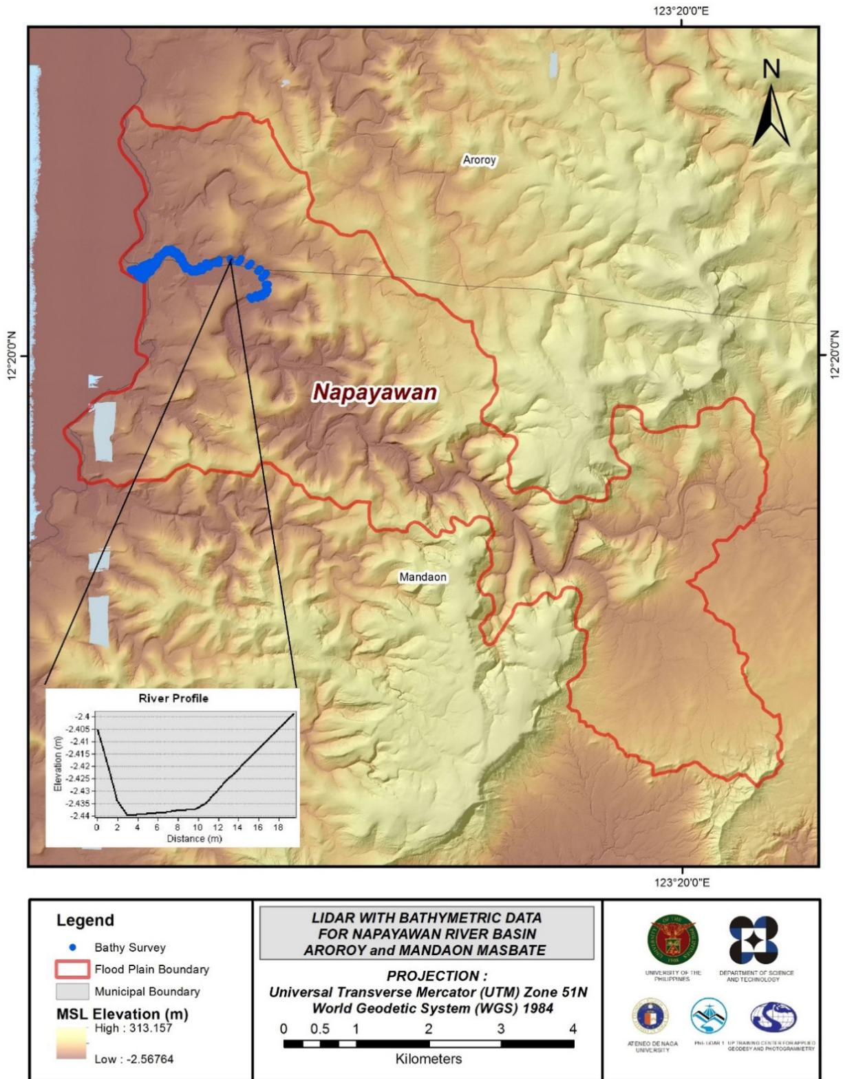
Figure 26. Map of Napayawan Floodplain with bathymetric survey points shown in blue.
