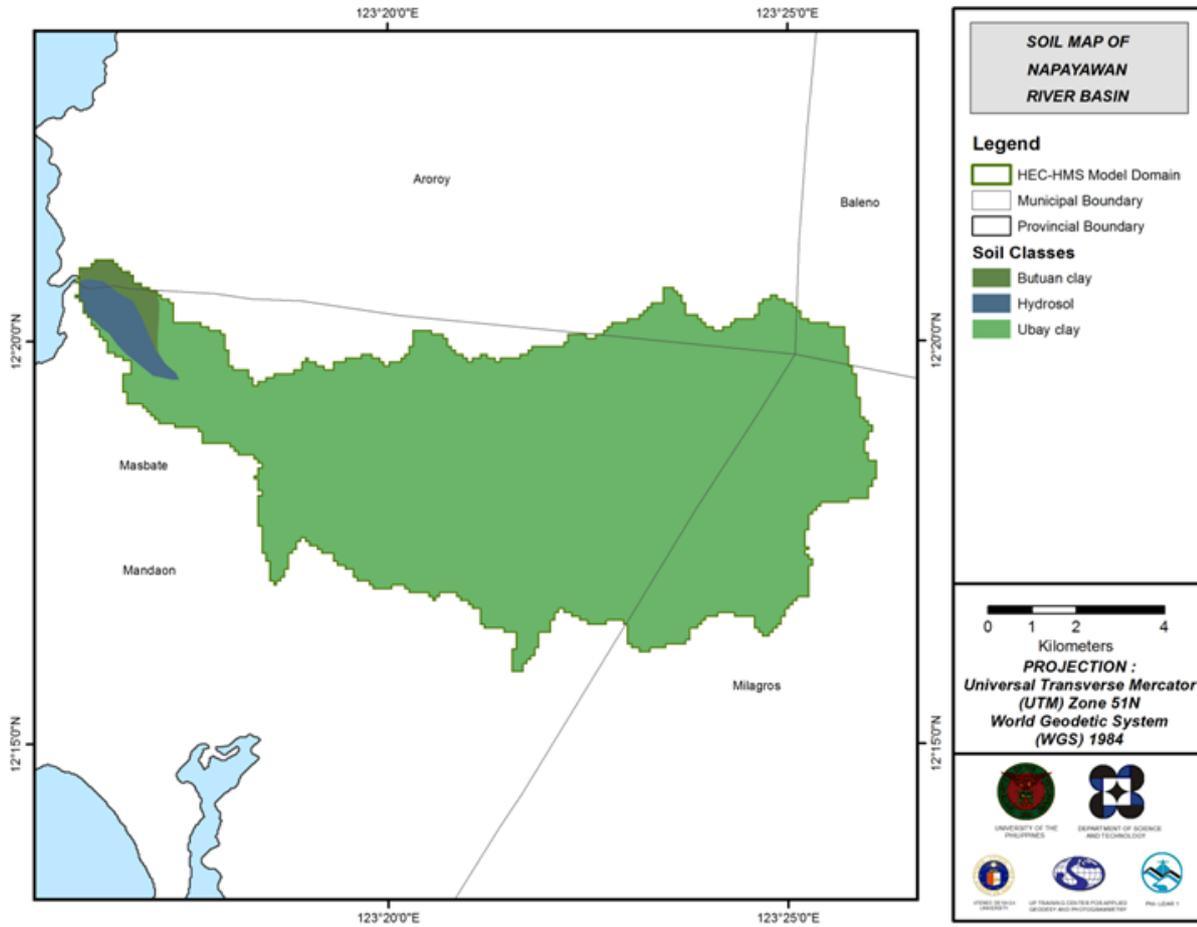
Figure 52. Soil Map of Napayawan River Basin used for the estimation of the CN parameter.
