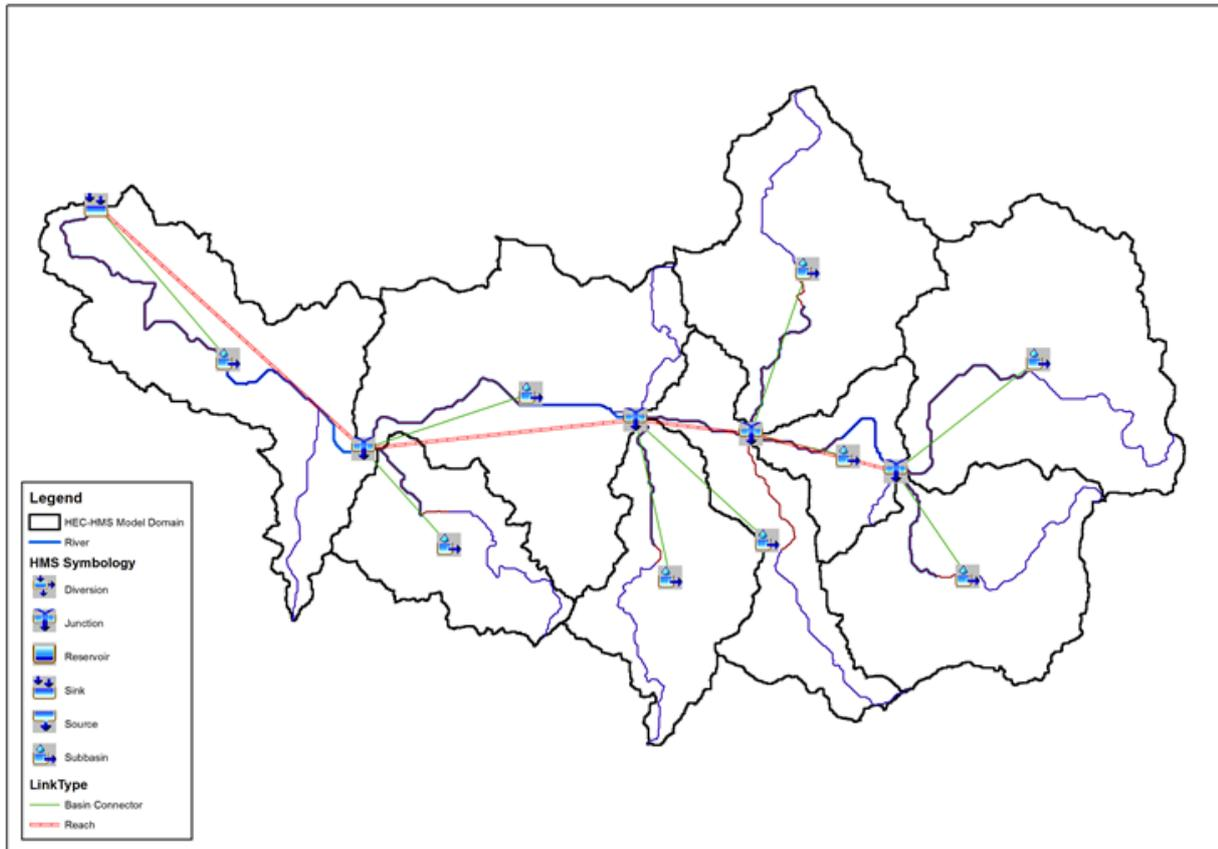
Figure 56. Napayawan River Basin model generated in HEC-HMS
