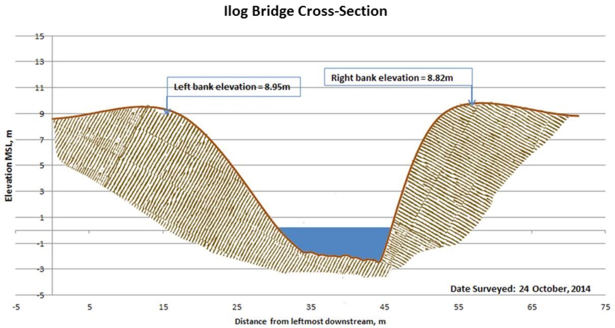
Figure 47. Cross-section plot of Napayawan (also known as Ilog) Bridge
