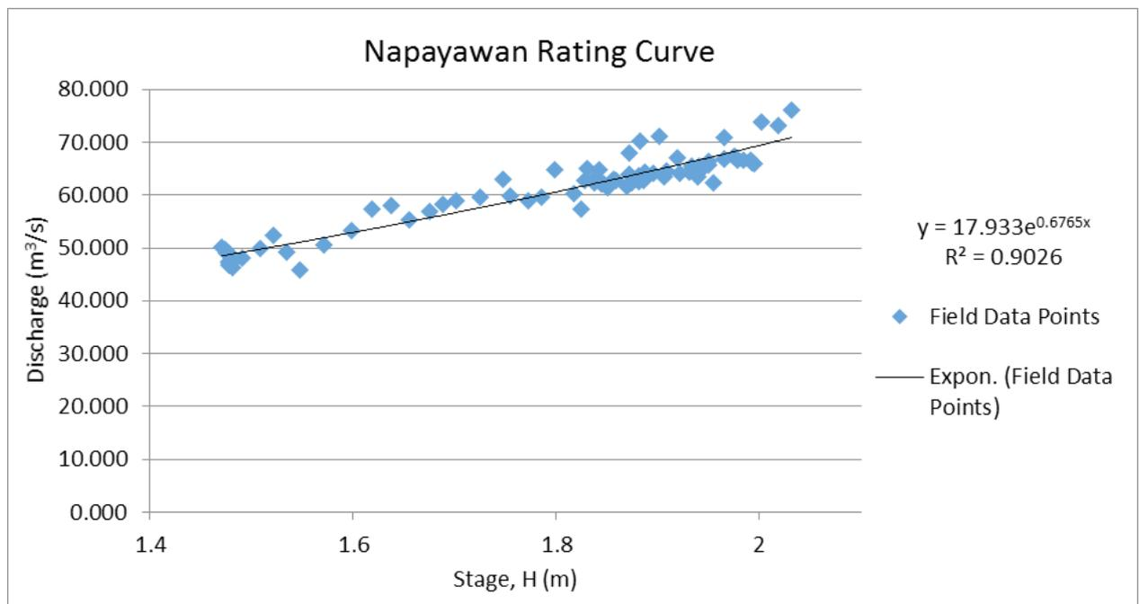
Figure 48. Rating curve of Napayawan (also known as Ilog) Bridge in Pilar, Sorsogon
