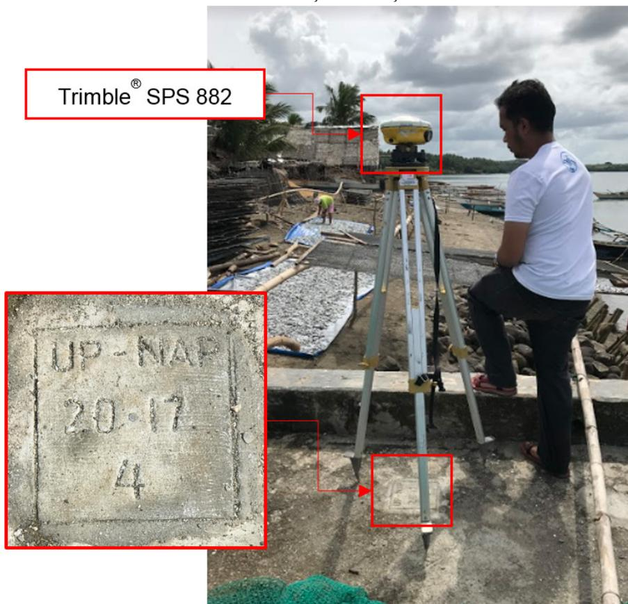
Figure 33. GNSS receiver set up, Trimble® SPS 985, at UP-NAP-4, located at the port in Brgy. Bugtong, Mandaon, Masbate
