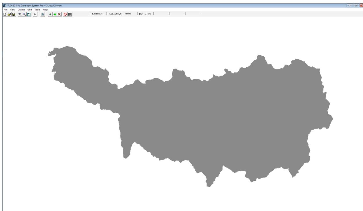
Figure 58. Screenshot of the river sub-catchment with the computational area to be modeled in FLO-2D Grid Developer System Pro (FLO-2D GDS Pro)
