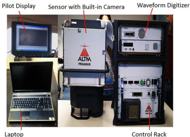
Figure A-1.1. Parameters and Specification of the Pegasus Sensor
