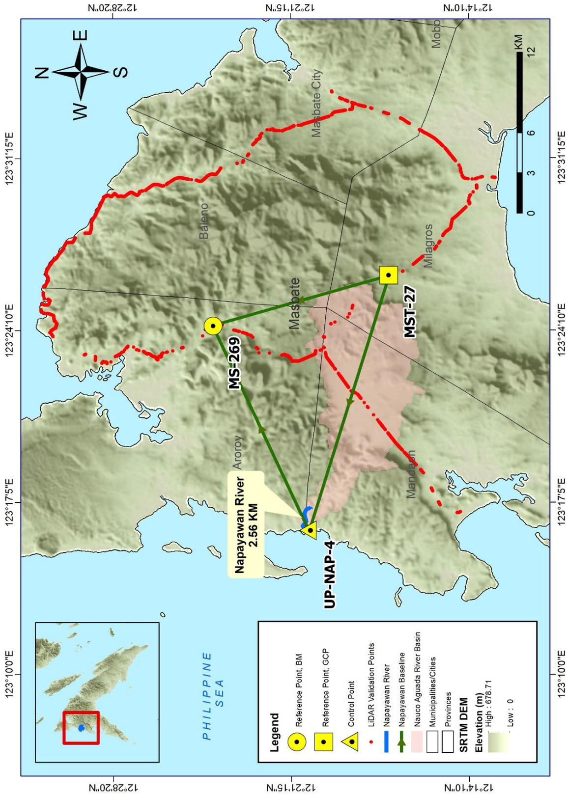
Figure 29. Extent of the bathymetric survey (in blue line) in Napayawan River and the LIDAR data validation survey (in red).
