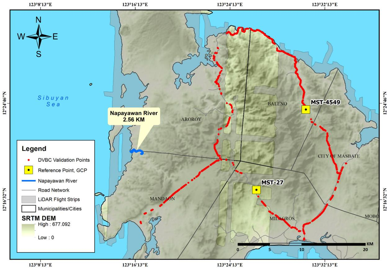
Figure 39. Validation point acquisition survey of Napayawan River basin
