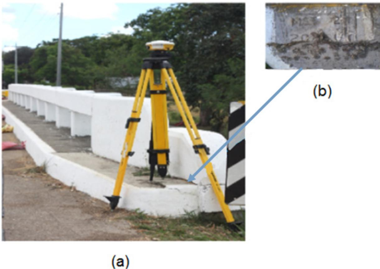
Figure 3. GPS set-up over MST-28 in Mambog Bridge, Barangay Bat-ongan, municipality of Napayawan, Masbate (a) and NAMRIA reference point MST-28 (b) as recovered by the field team.
