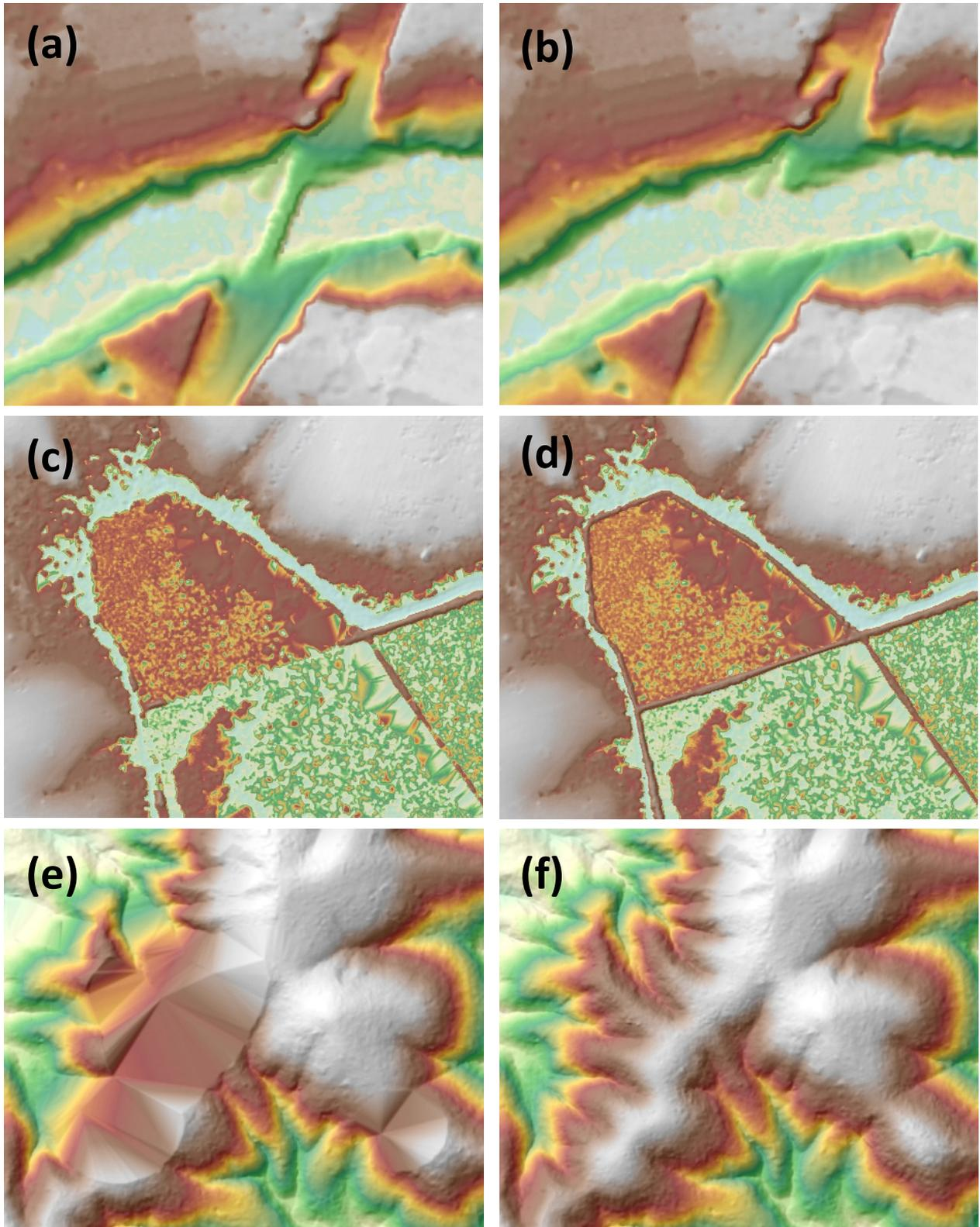
Figure 21. Portions in the DTM of Napayawan floodplain – a bridge before (a) and after (b) manual editing; a paddy field before (c) and after (d) data retrieval; and a highland before (e) and after (f) data retrieval.
