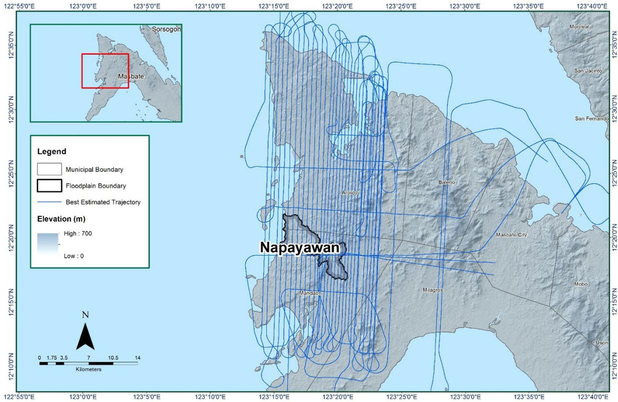
Figure 10. Best estimated trajectory of the LiDAR missions conducted over the Napayawan Floodplain.
