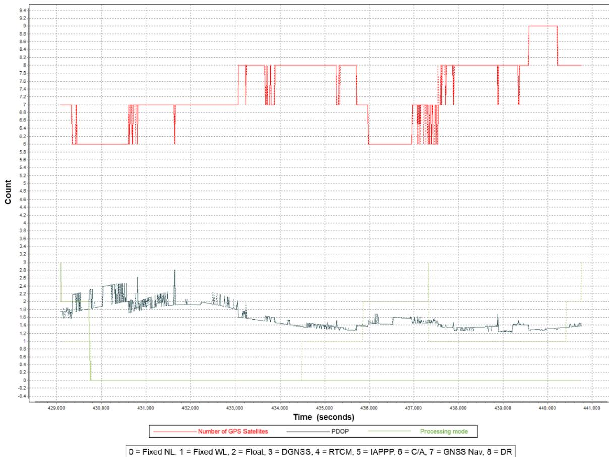
Figure 9. Solution Status Parameters of Napayawan Flight 1303P.
