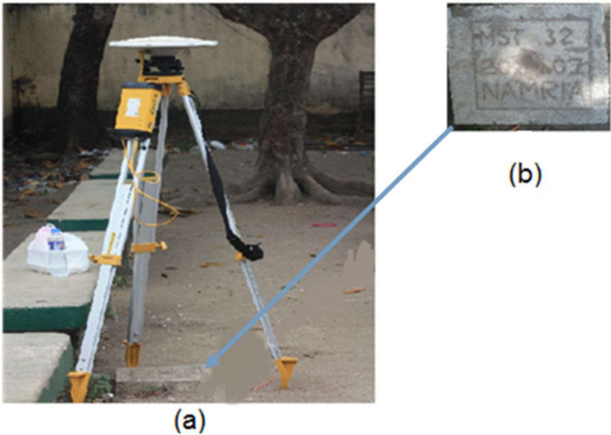
Figure 4. GPS set-up over MST-32 inside the compound of the Milagros Municipal Hall, Masbate (a) and NAMRIA reference point MST-32 (b) as recovered by the field team.
