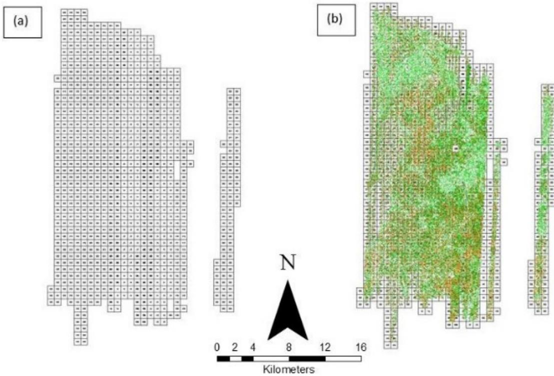
Figure 16. Tiles for Napayawan Floodplain (a) and classification results (b) in TerraScan.
