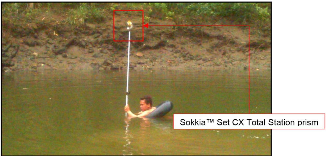
Figure 41. Manual bathymetric survey of HONS along Napayawan River
