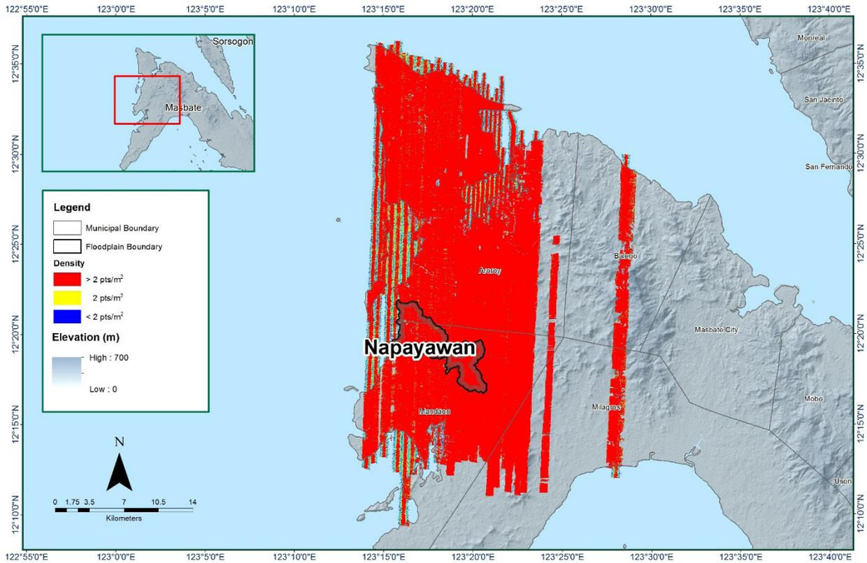
Figure 13. Pulse density map of merged LiDAR data for Napayawan Floodplain.
