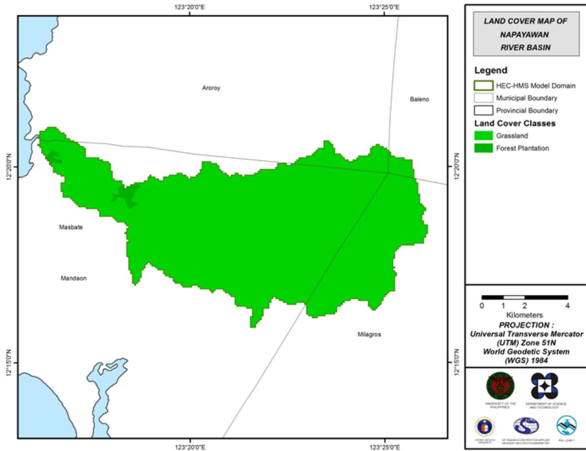
Figure 53. Land Cover Map of Napayawan River Basin used for the estimation of the Curve Number (CN) and the watershed lag parameters of the rainfall-runoff model.
