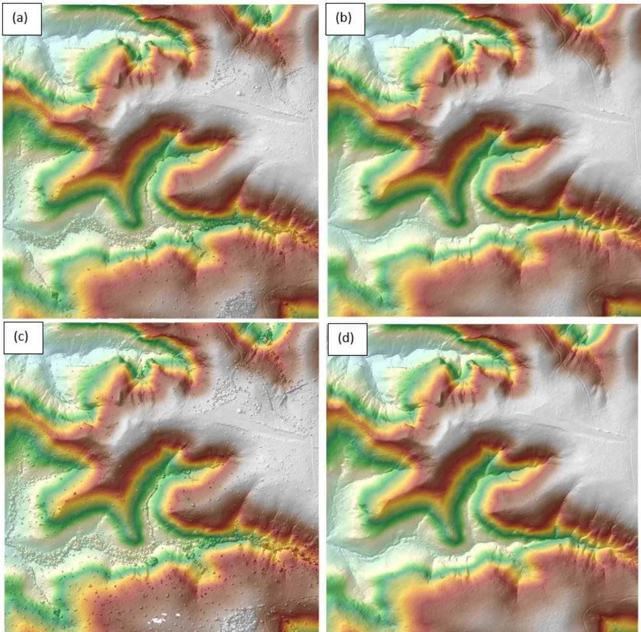
Figure 18. The production of last return DSM (a) and DTM (b), first return DSM (c) and secondary DTM (d) in some portion of Napayawan Floodplain.
