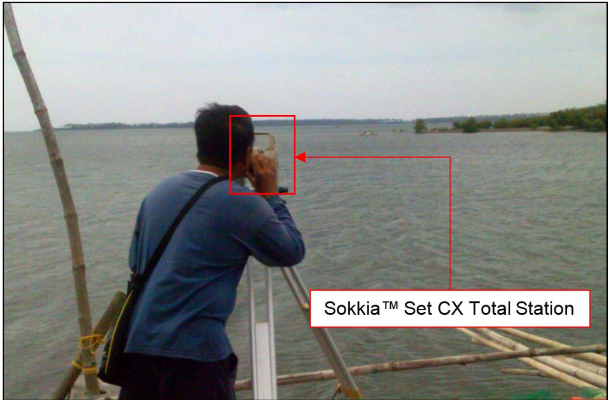
Figure 34. Cross-section survey at the mouth of Napayawan River
