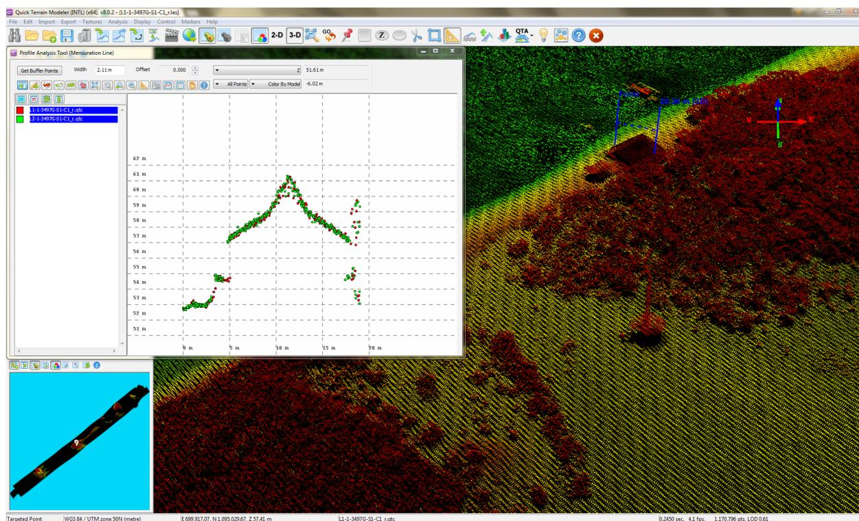
Figure 15. Quality checking for Napayawan Flight 1303P using the Profile Tool of QT Modeler.
