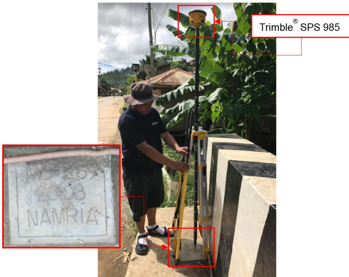
Figure 32. GNSS receiver set up, Trimble® SPS 985, at MS-269, located at the approach of Luy-A bridge in Brgy. Luy-A, Aroroy, Masbate
