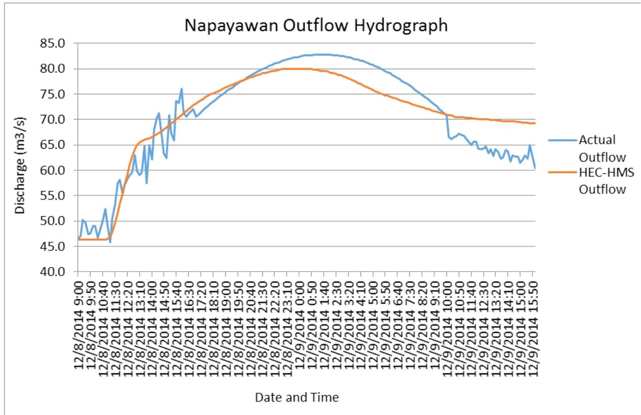
Figure 59. Outflow hydrograph of Napayawan produced by the HEC-HMS model compared with observed outflow
