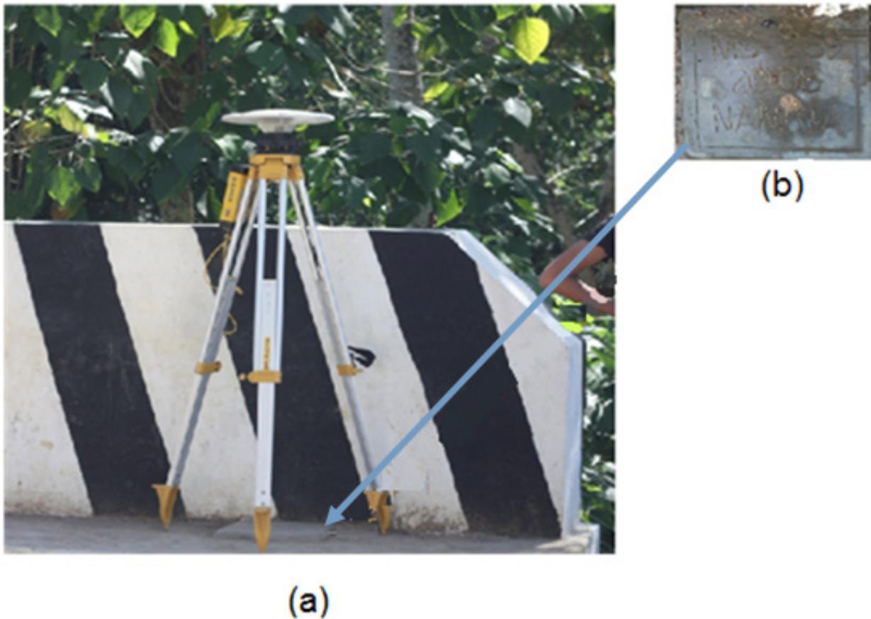
Figure 5. GPS set-up over MS-269 in Luy-a Bridge in Aroroy, Masbate (a) and NAMRIA benchmark MS-269 (b) as recovered by the field team.
