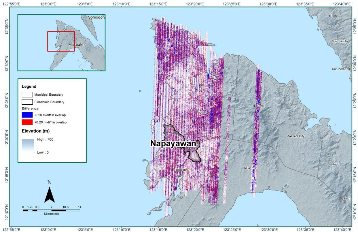
Figure 14. Elevation Difference Map between flight lines for Napayawan Floodplain Survey.
