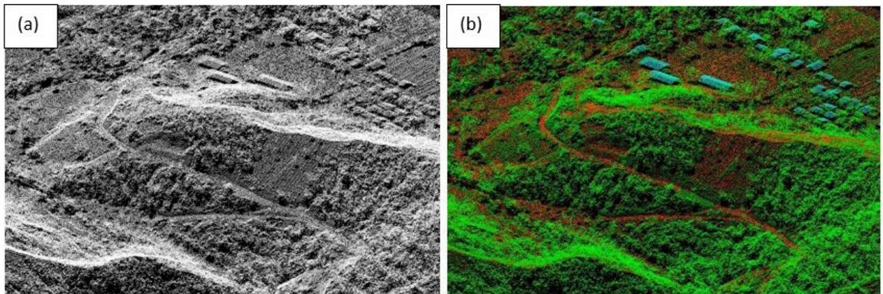
Figure 17. Point cloud before (a) and after (b) classification
