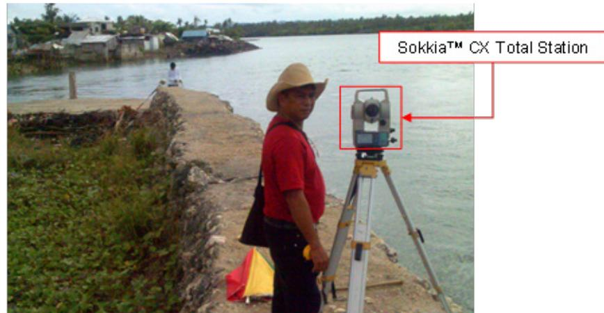
Figure 44. Set-up of the manual bathymetric survey of H.O. Noveloso Surveying along Nauco Aguada River
