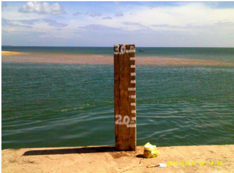
Figure 40. Water level markings along Nauco Aguada River.
