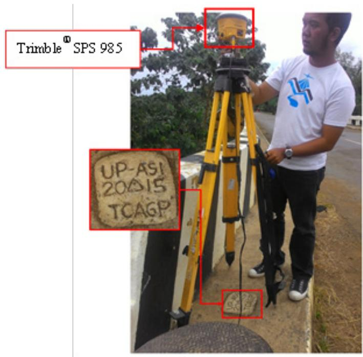
Figure 32. GNSS receiver setup, Trimble® SPS 985, at UP-ASI, located Brgy. Cayabon, Municipality of Milagros, Masbate.
