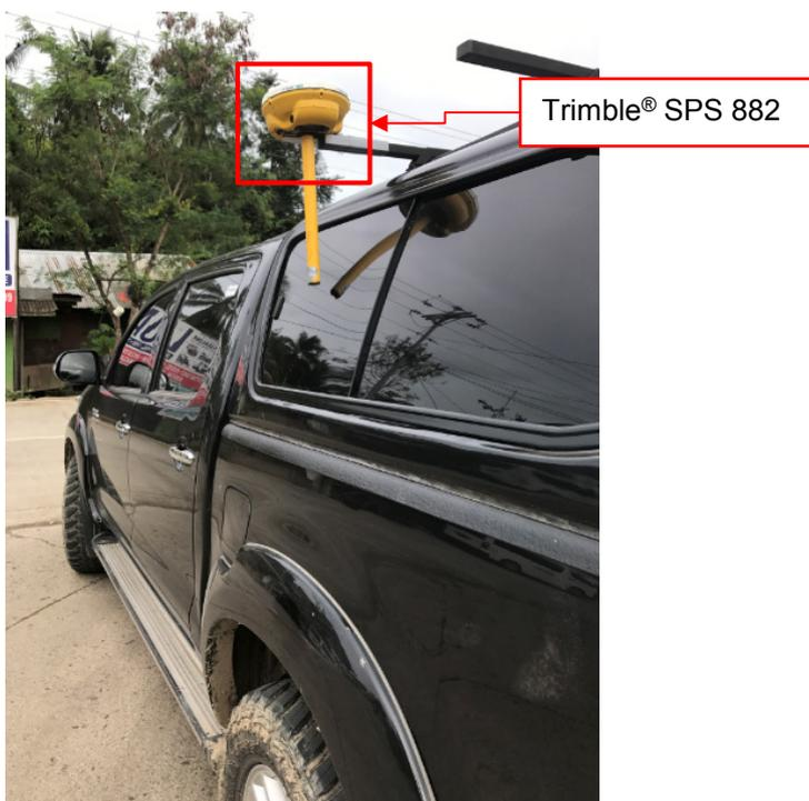
Figure 41. The validation point acquisition survey setup using a GNSS receiver fixed in a van along the Nauco Aguada River Basin.
