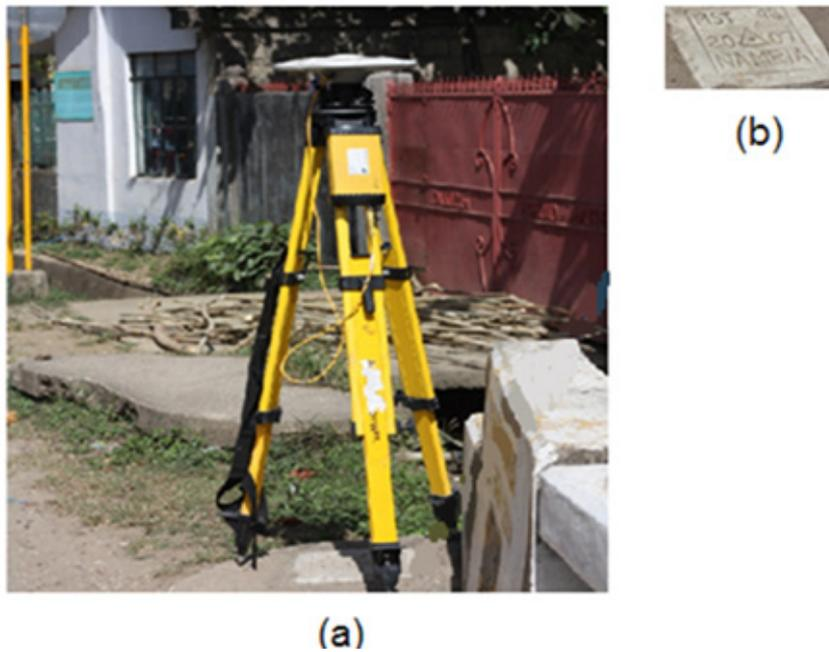
Figure 3. GPS set-up over MST-40 (a) as recovered in Buenavista Bridge in Brgy. Buenavista, municipality of Uson, Masbate; and NAMRIA reference point MST-40 (b) as recovered by the field team.
