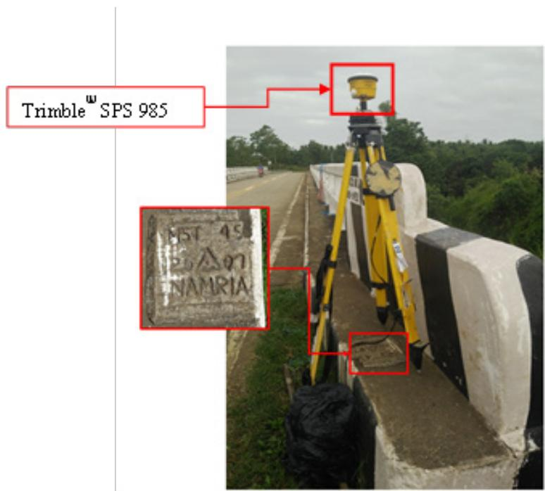
Figure 35. GNSS receiver setup, Trimble® SPS 985, at MST-45, located in Brgy. Villahermosa, Municipality of Cawayan, Masbate.
