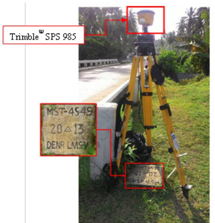
Figure 31. GNSS base set up, Trimble® SPS 985, at MST-4549, located in Brgy. Canjunday, Municipality of Baleno, Masbate.
