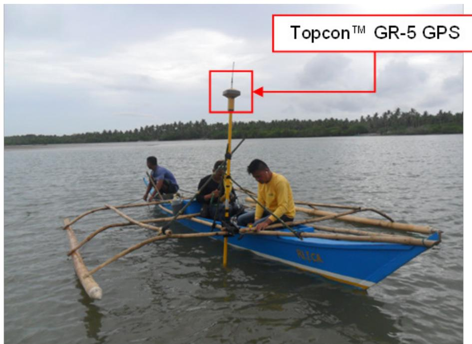
Figure 43. Set-up of the bathymetric survey in Nauco Aguada River conducted by H.O. Noveloso Surveying.
