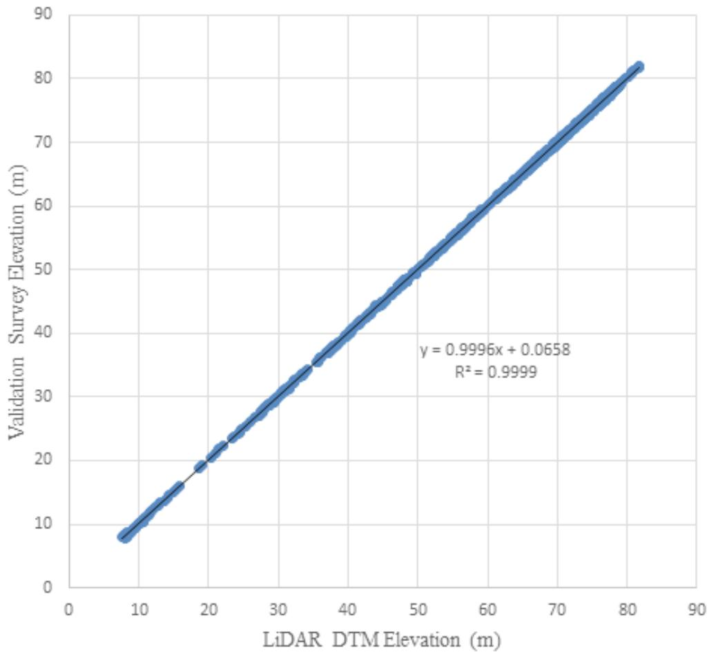
Figure 26. Correlation plot between validation survey points and LiDAR data
