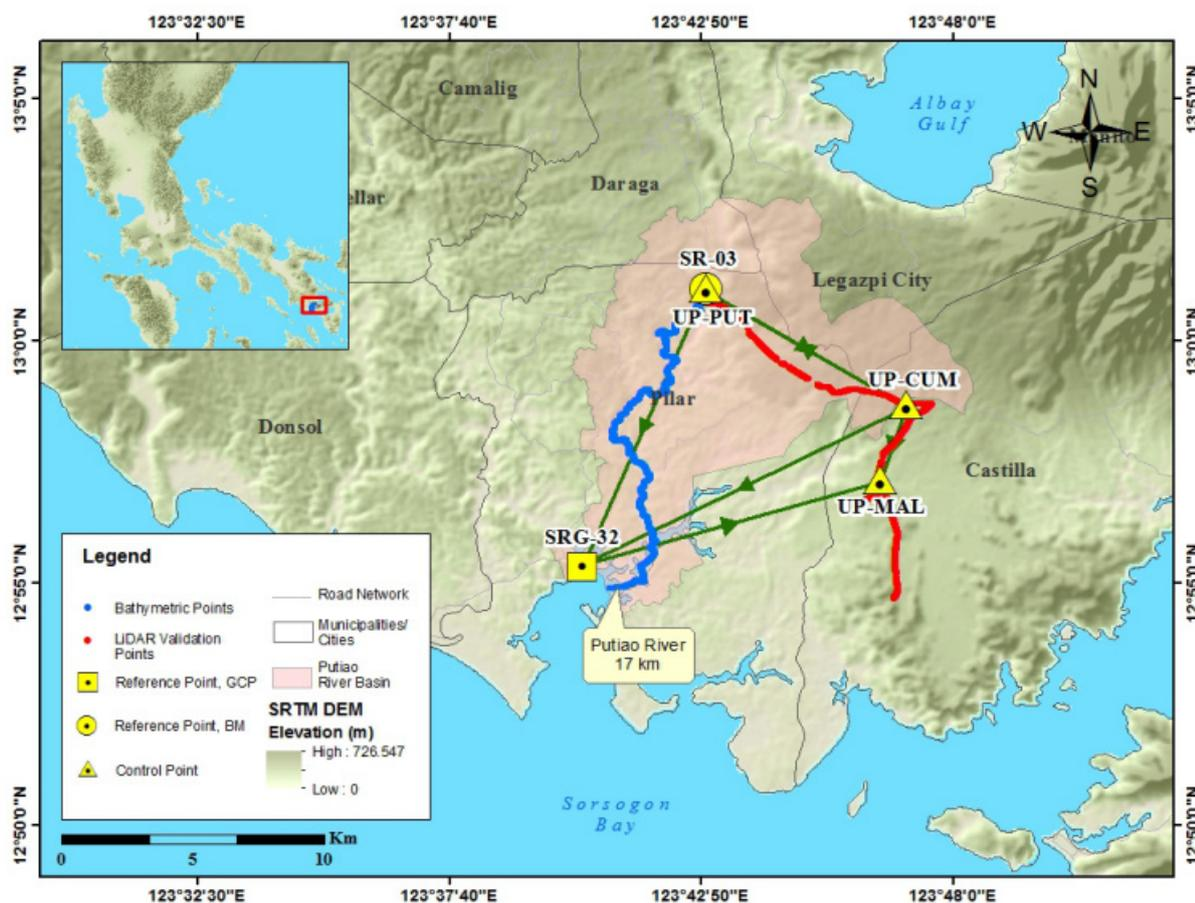
Figure 30. Extent of the bathymetric survey (in blue line) in Putiao River Survey and the LiDAR data validation survey (in red)
