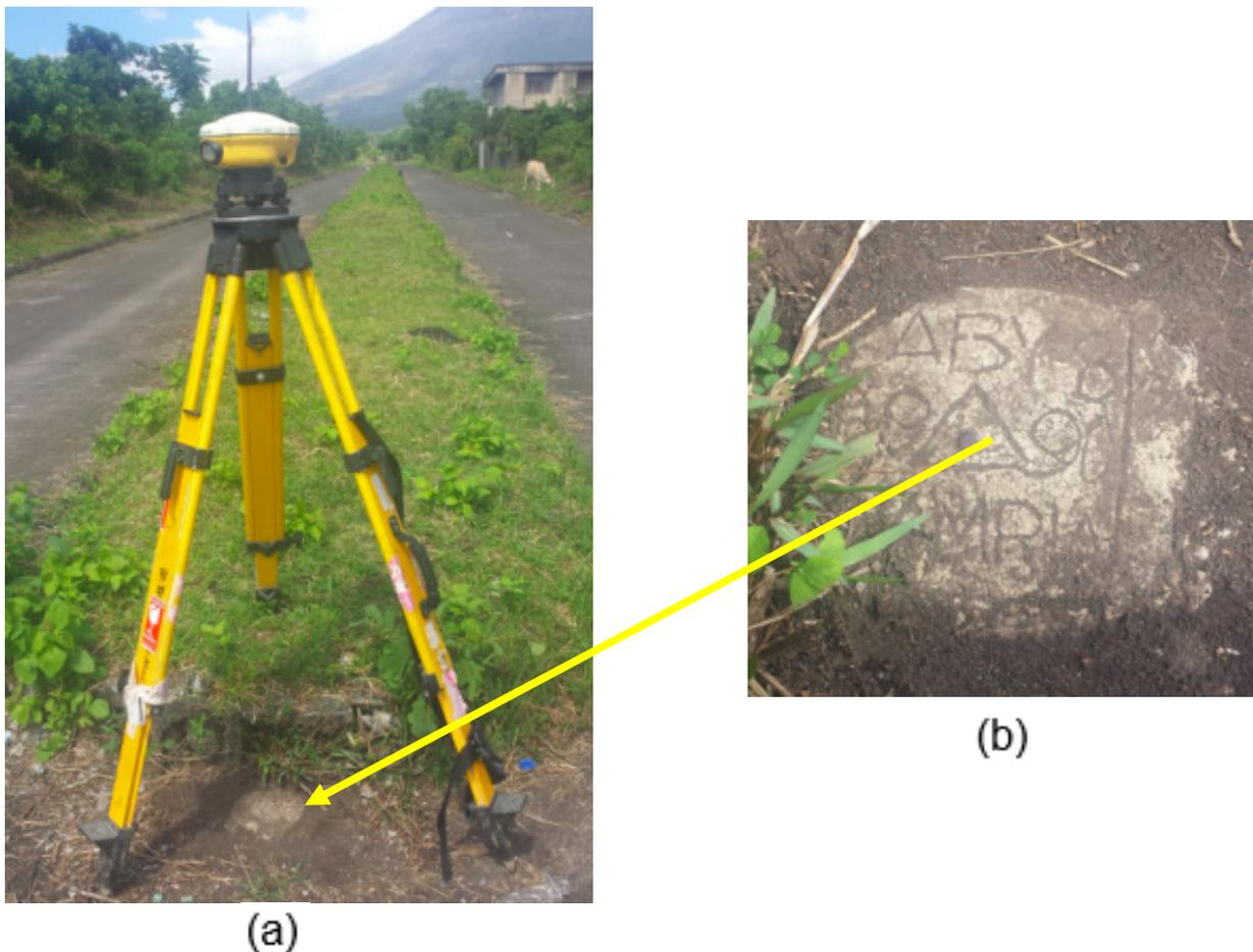
Figure 5. GPS set-up over ABY-8 at the center of the island of Mayon Riviera Subdivision. Highest prominent mark is the electric timber post 9.50 meters SE of the station (a) and NAMRIA reference point ABY-8 (b) as recovered by the field team.
