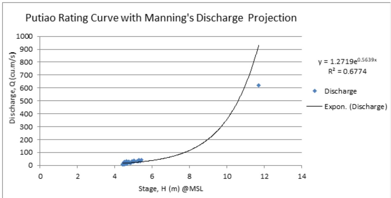
Figure 49. The rating curve of Putiao Bridge in Pilar, Sorsogon
