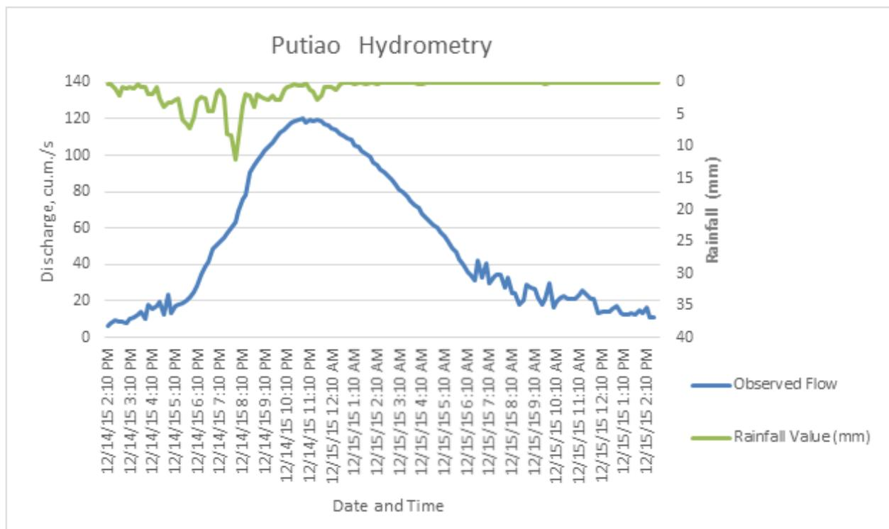
Figure 50. Rainfall and outflow data of the Putiao River Basin, which was used for modeling
