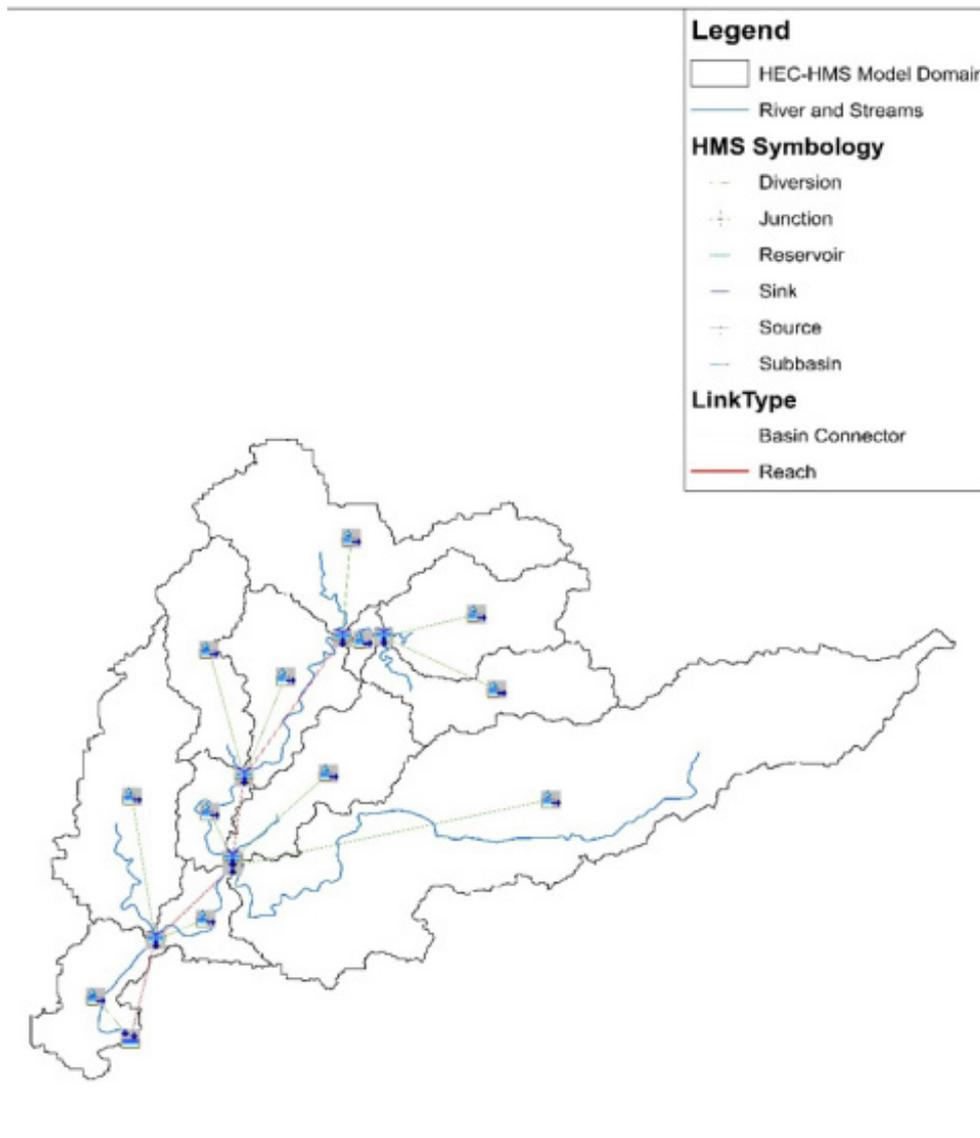
Figure 57. The Putiao river basin model generated using HEC-HMS
