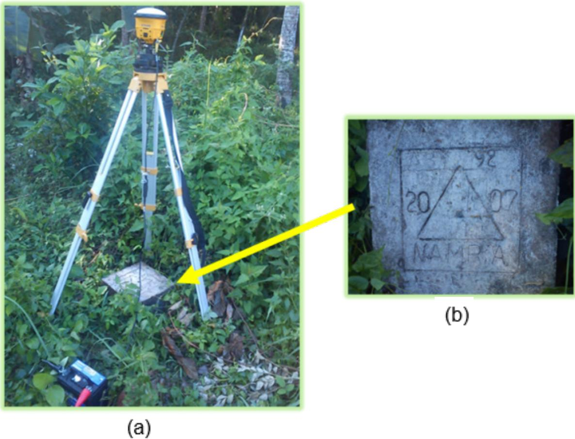
Figure 4. GPS set-up over ABY-92 beside the baseline of the basketball court at about 19 meters from the barangay hall (a) and NAMRIA reference point ABY-92 (b) as recovered by the field team.
