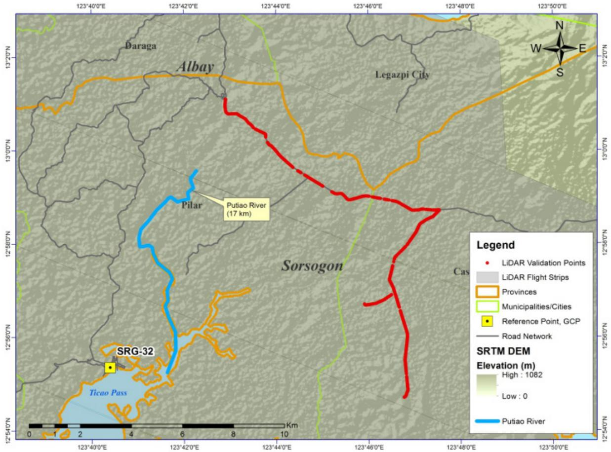
Figure 43. Extent of the LiDAR ground validation survey along Putiao River Basin
