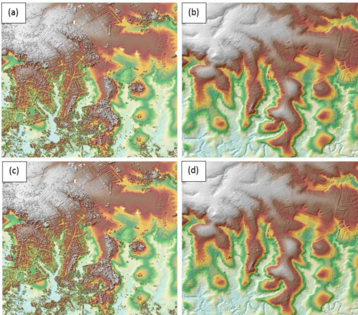
Figure 21. The production of last return DSM (a) and DTM (b), first return DSM (c) and secondary DTM (d) in some portion of Putiao floodplain.
