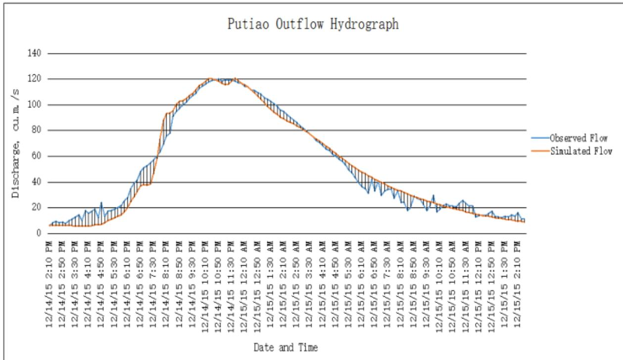
Figure 60. Outflow Hydrograph produced by the HEC-HMS model compared with observed outflow
