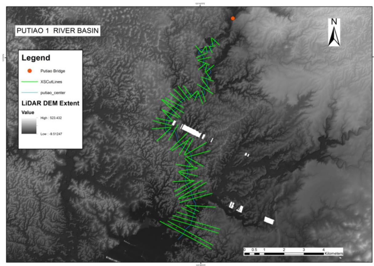
Figure 58. River cross-section of Putiao River generated through ArcMap HEC GeoRAS tool
