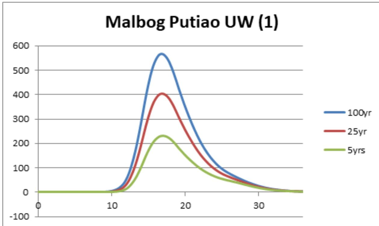
Figure 62. Putiao river (1) generated discharge using 5-, 25-, and 100-year Legazpi City rainfall intensity-duration-frequency (RIDF) in HEC-HMS
