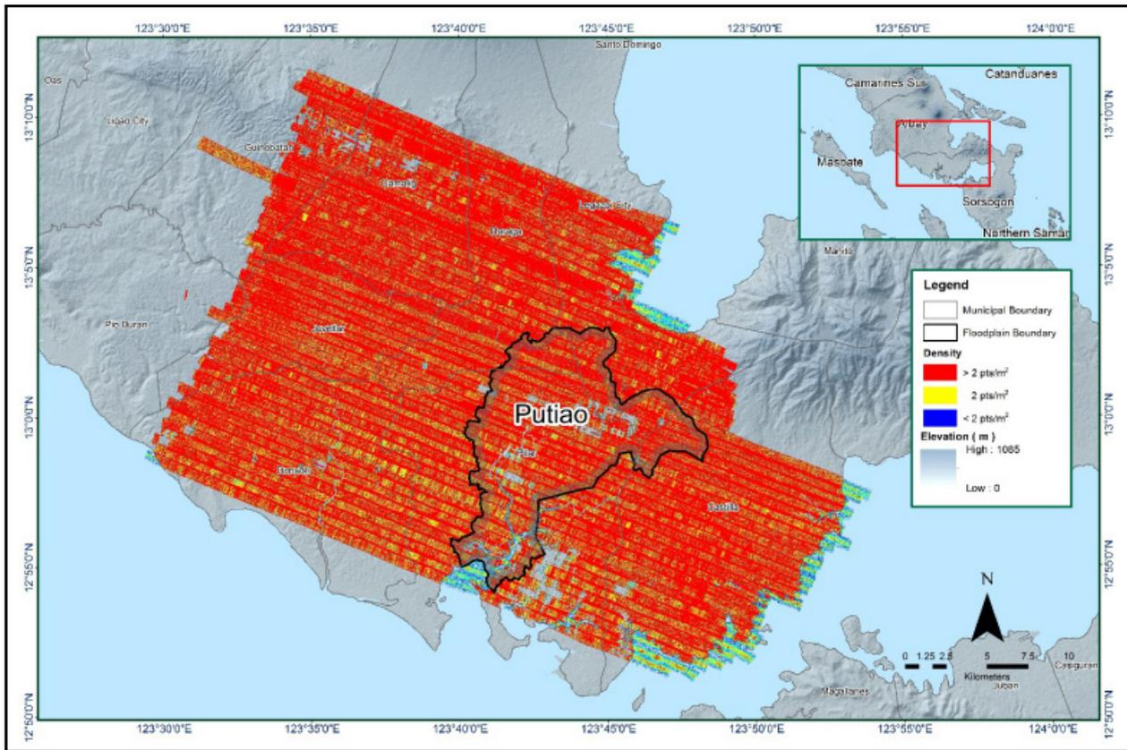
Figure 16. Pulse density map of merged LiDAR data for Putiao floodplain
