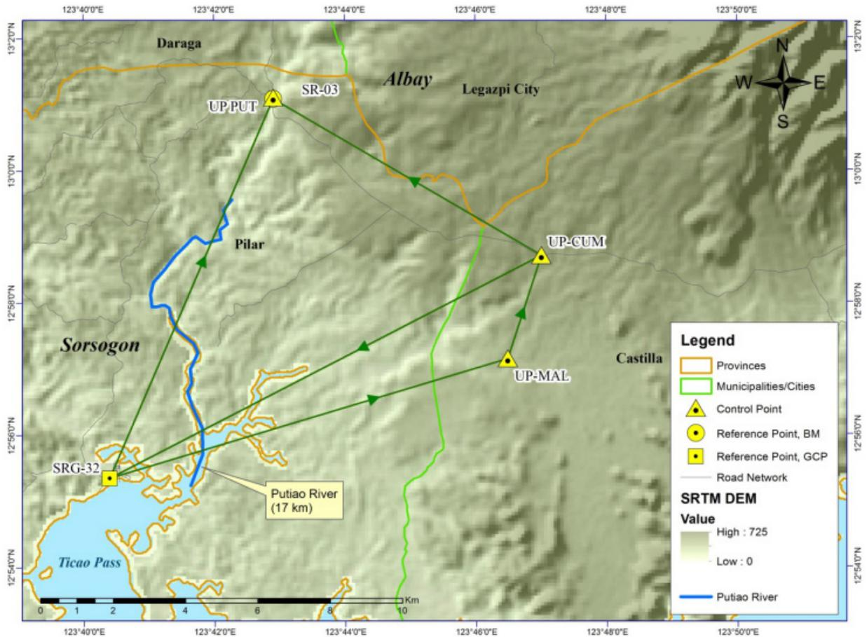
Figure 31. GNSS Network established for Putiao River Basin survey
