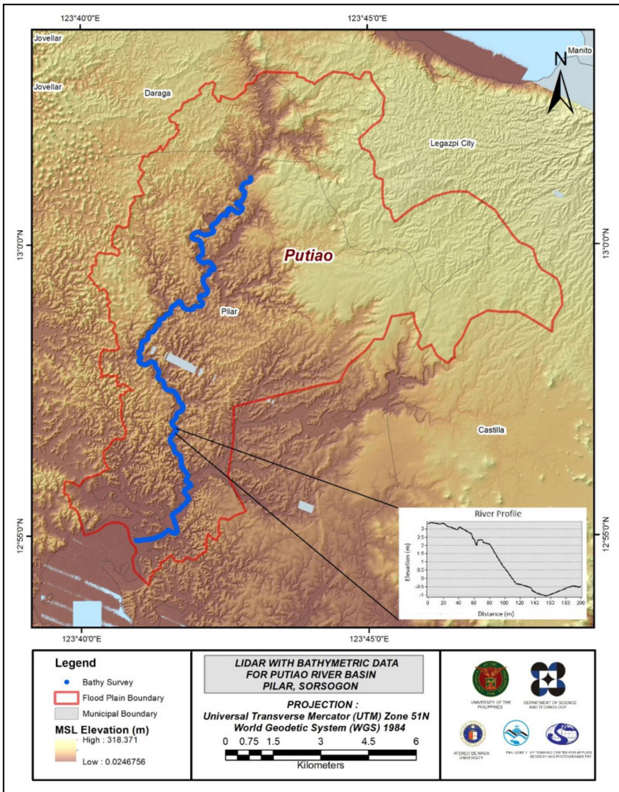
Figure 27. Map of Putiao Floodplain with bathymetric survey points shown in blue.
