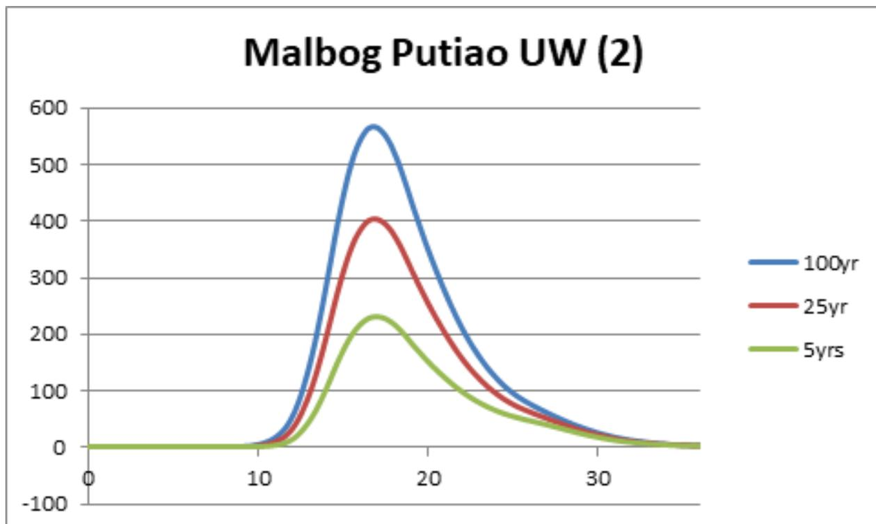
Figure 63. Putiao river (2) generated discharge using 5-, 25-, and 100-year Legazpi City rainfall intensity-duration-frequency (RIDF) in HEC-HMS
