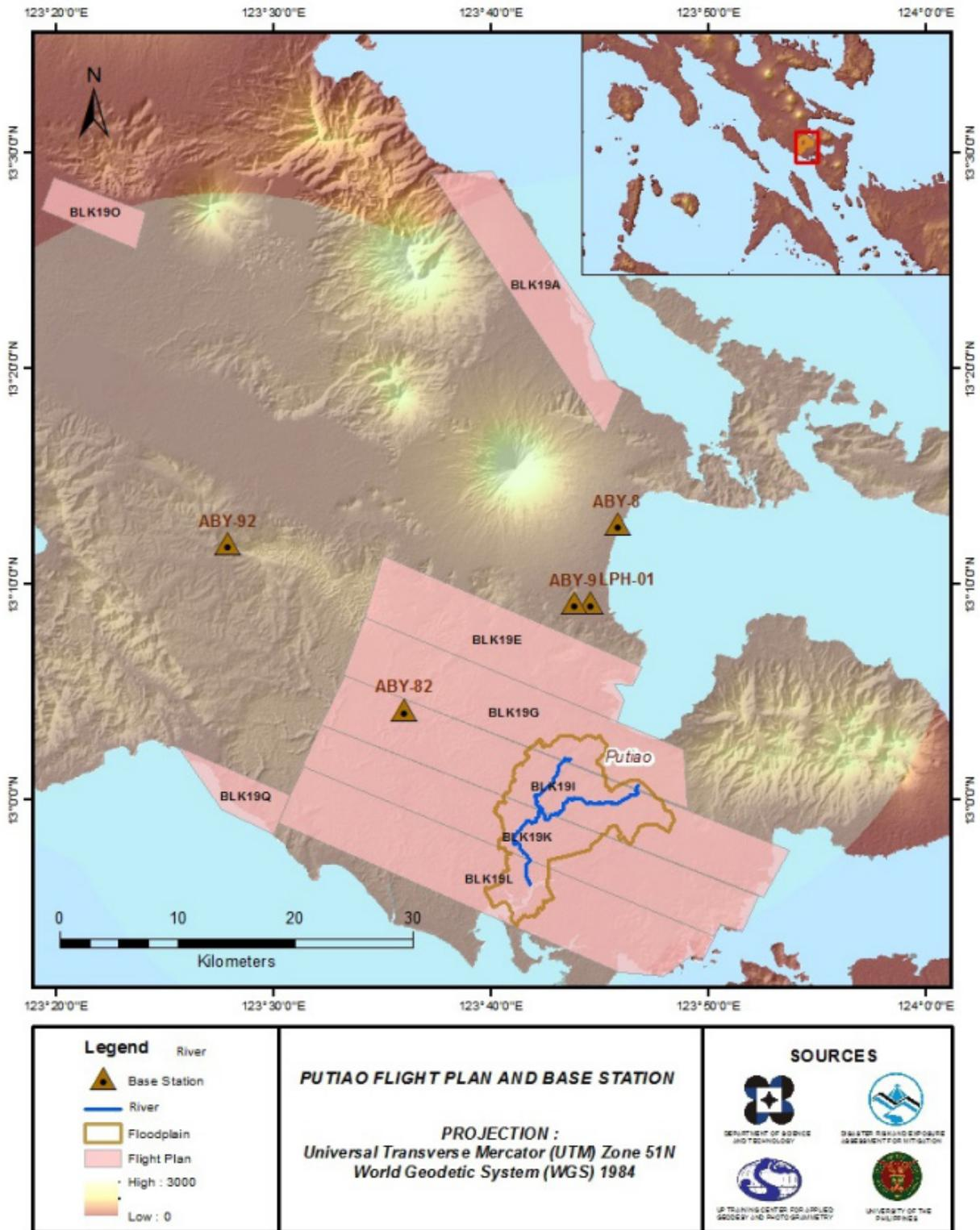
Figure 3. Flight Plan and base stations used for the Putiao Floodplain survey.
