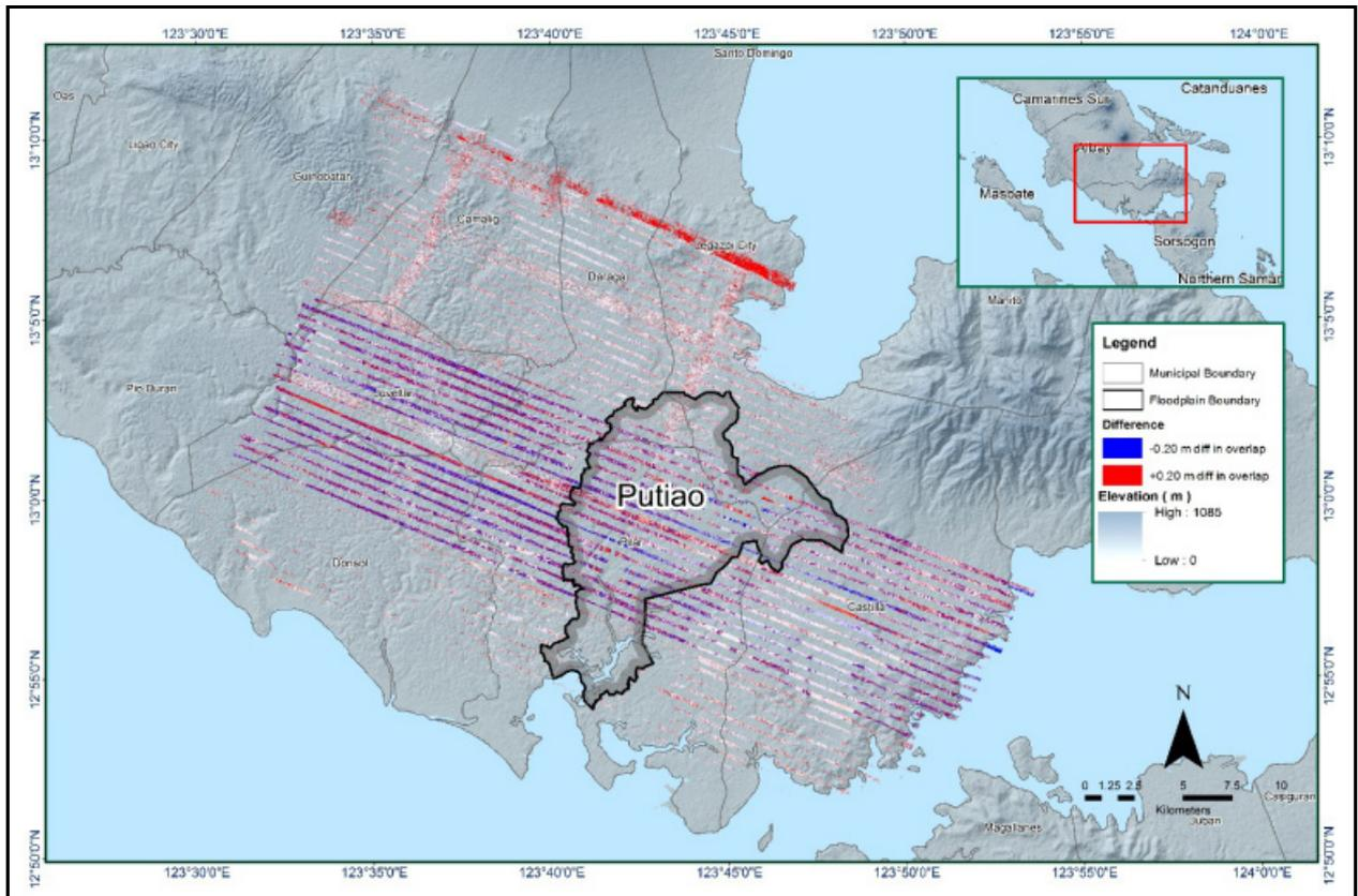
Figure 17. Elevation difference map between flight lines for Putiao Floodplain survey.
