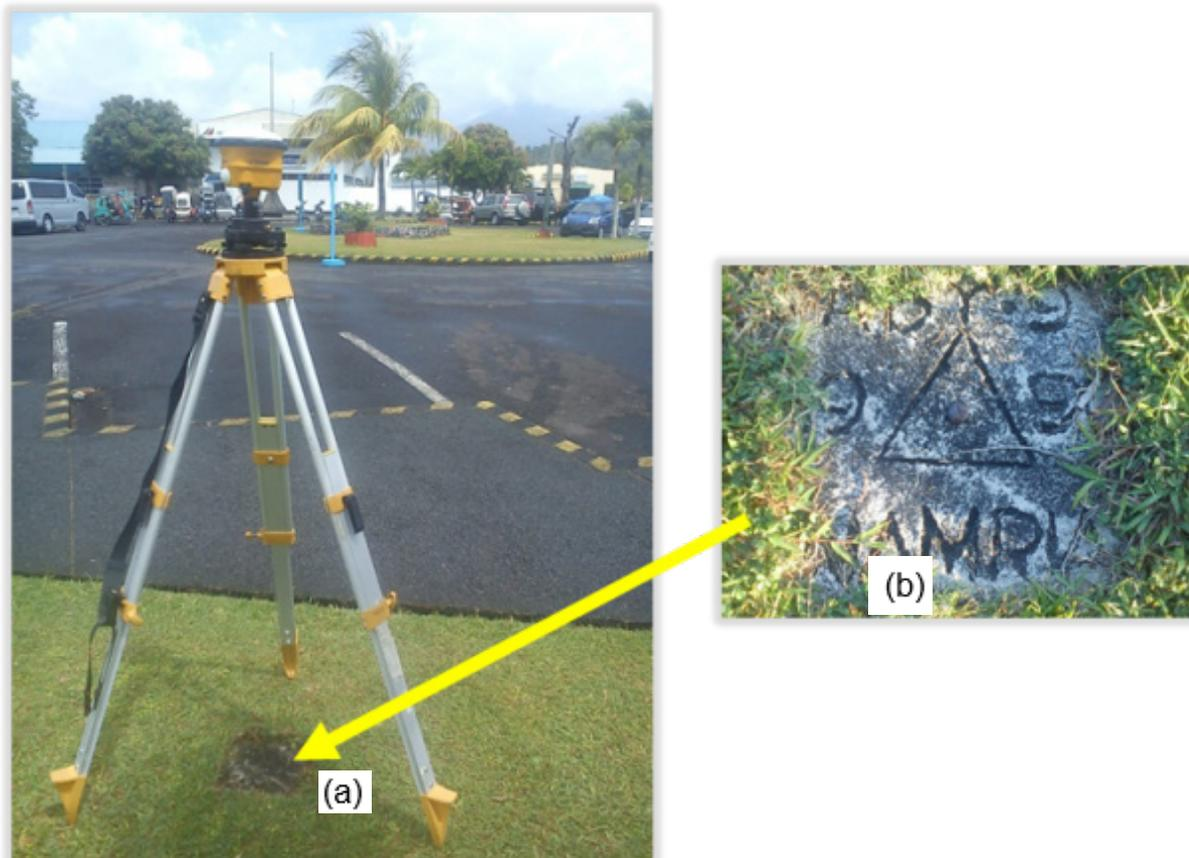
Figure 7. GPS set-up over ABY-9 inside Legaspi Airport Compound 52.0 meters SE of Legaspi Airport Flagpole, 35 meters NE of Legaspi Airport Welcome Post 3.30 meters NW of Lamp (a) and NAMRIA reference point ABY-9 (b) as recovered by the field team
