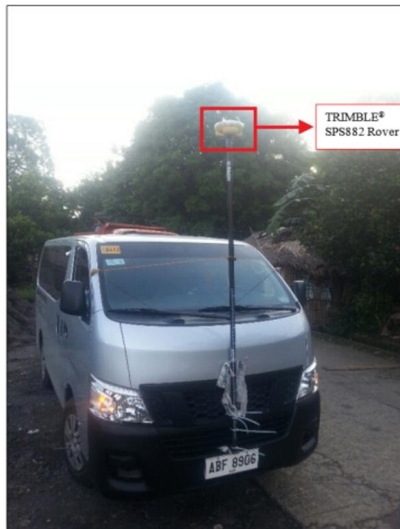
Figure 42. Trimble® SPS 882 set up for the acquisition of LiDAR validation points
