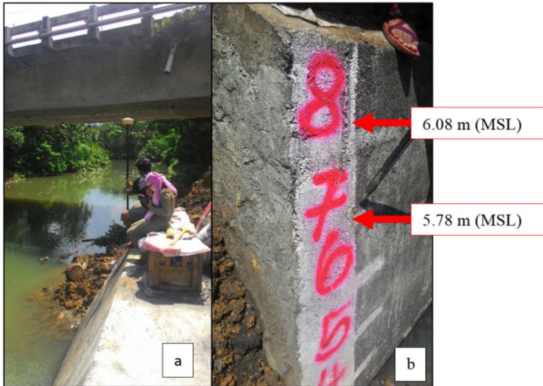
Figure 41. (a) Getting the MSL elevations of the existing markings on the dike (b) The existing markings with their corresponding MSL elevations
