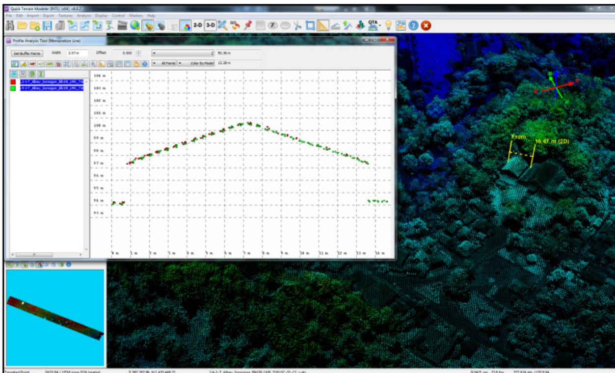
Figure 18. Quality checking for a Putiao flight 7161G using the Profile Tool of QT Modeler.
