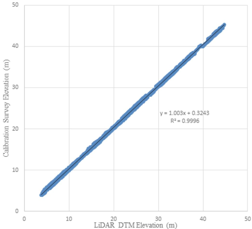
Figure 25. Correlation plot between calibration survey points and LiDAR data.
