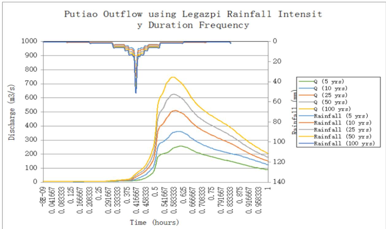
Figure 61. The outflow hydrograph at the Putiao Basin, generated using the simulated events for 24-hour period for Legazpi station
