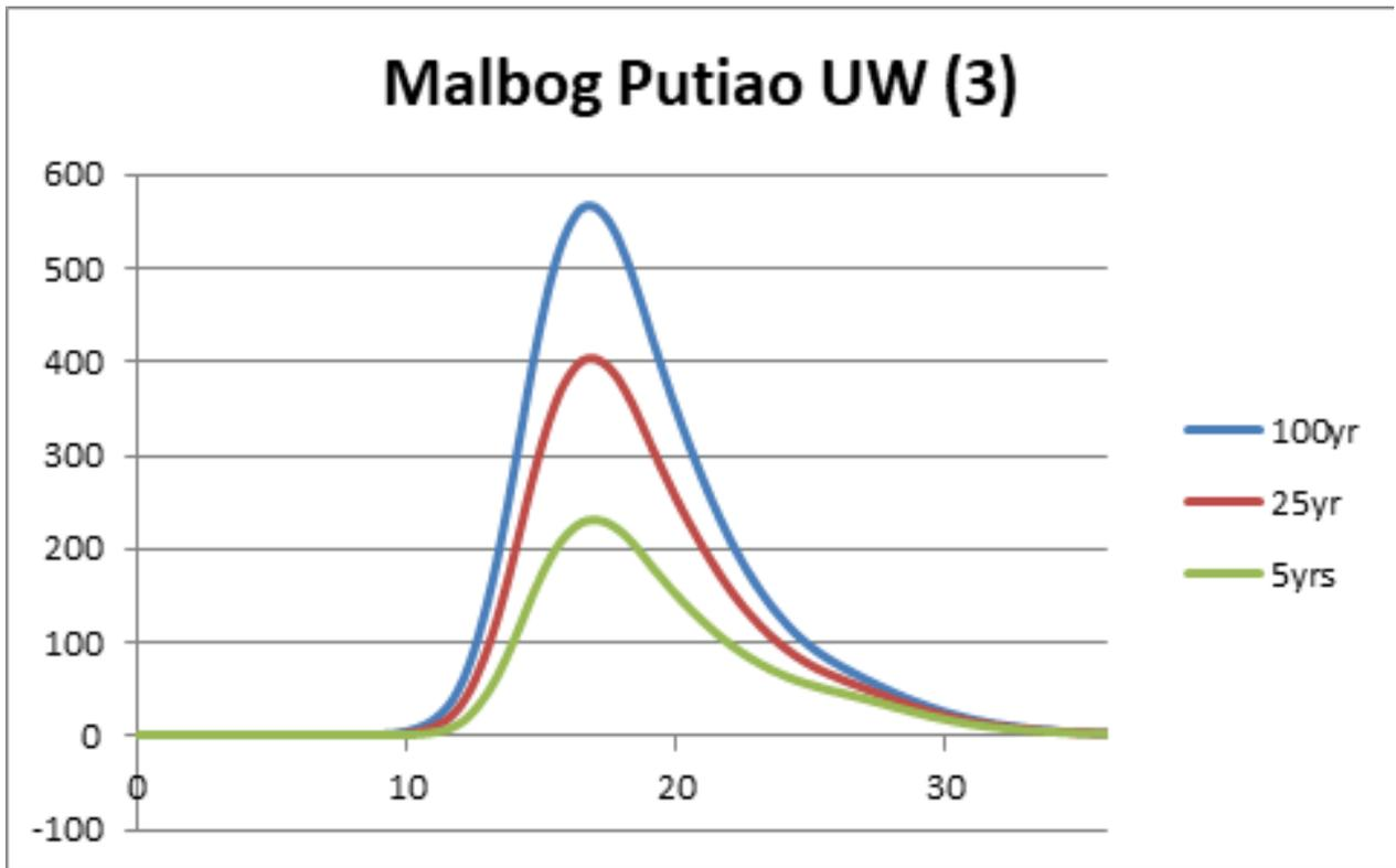
Figure 64. Putiao river (3) generated discharge using 5-, 25-, and 100-year Legazpi City rainfall intensity-duration-frequency (RIDF) in HEC-HMS
