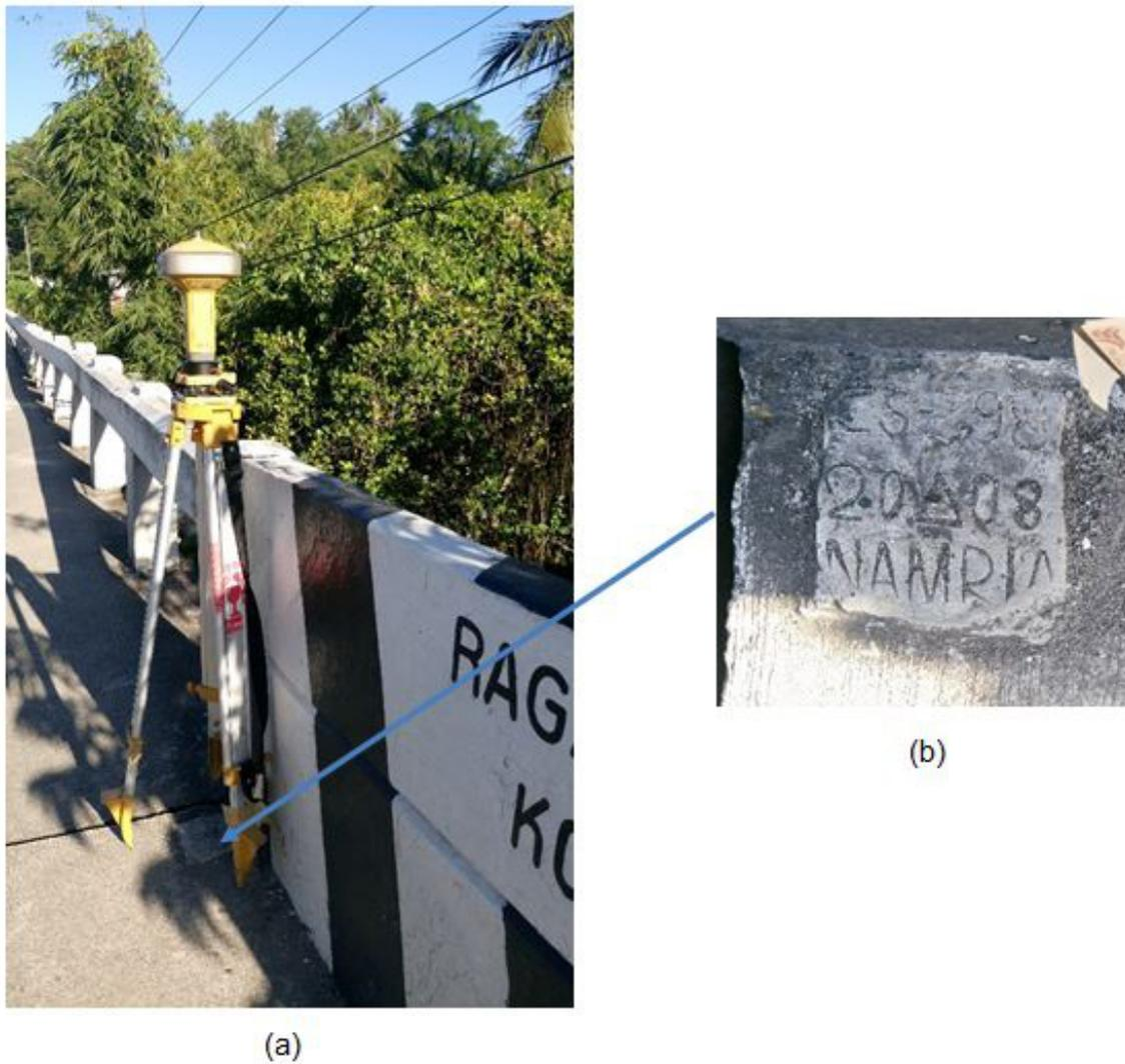
Figure 4. GPS set-up over CS-98 (a) and NAMRIA reference point CS-98 (b) as recovered by the field team.
