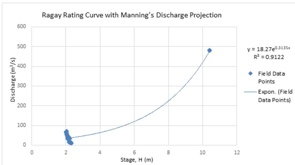
Figure 46. Rating curve of Ragay Bridge in Ragay, Camarines Sur
