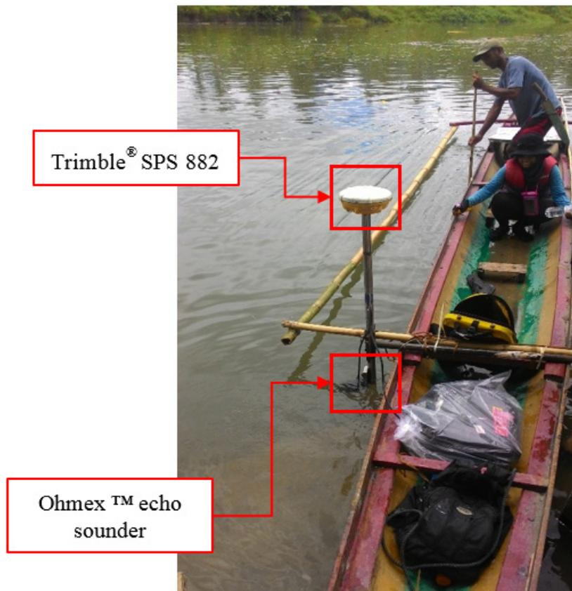
Figure 40. Bathymetric survey using Ohmex™ single beam echo sounder in Ragay River
