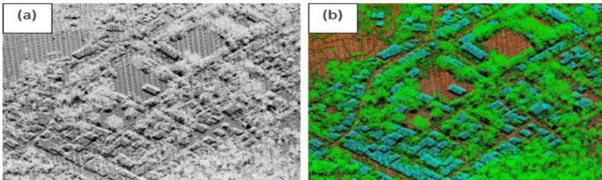
Figure 16. Point cloud before (a) and after (b) classification
