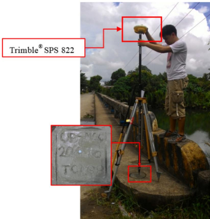
Figure 33. GNSS receiver setup, Trimble® SPS 822, at UP-MOC, located at the approach of Mocong Bridge in Brgy. Mocong, Municipality of Basud, Camarines Norte.
