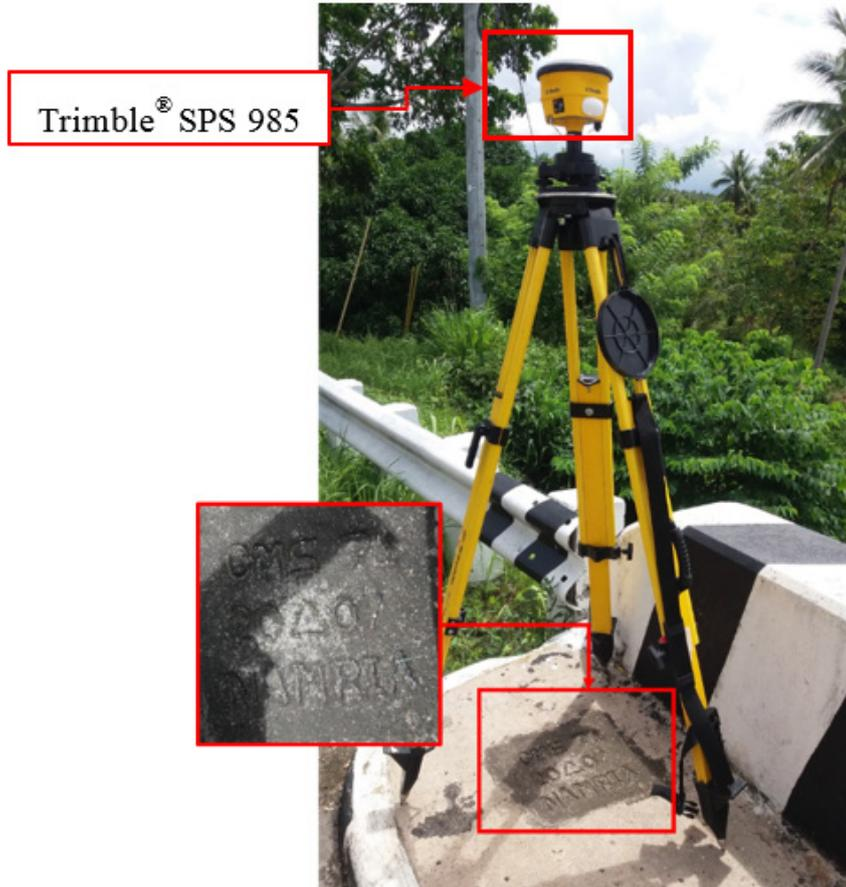
Figure 30. GNSS base set up, Trimble® SPS 985, at CMS-71, situated at the approach of Kilbay Bridge in Brgy. Cabasag, Municipality of Del Gallego, Camarines Sur.
