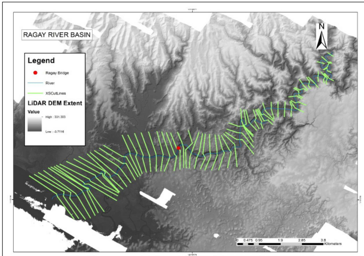
Figure 55. River cross-section of the Ragay River through the ArcMap HEC GeoRAS tool.
