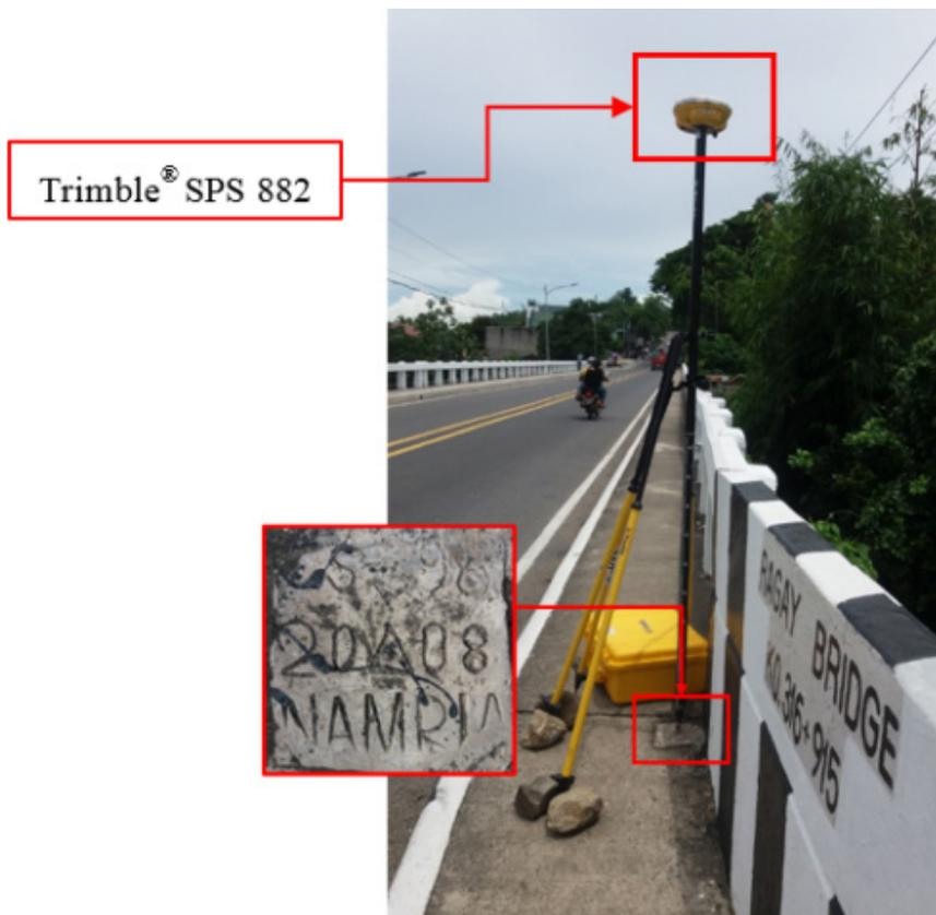
Figure 31. GNSS receiver setup, Trimble® SPS 882, at CS-398, located at the approach of Ragay Bridge in Brgy. Pangitayan, Municipality of Ragay, Camarines Sur.
