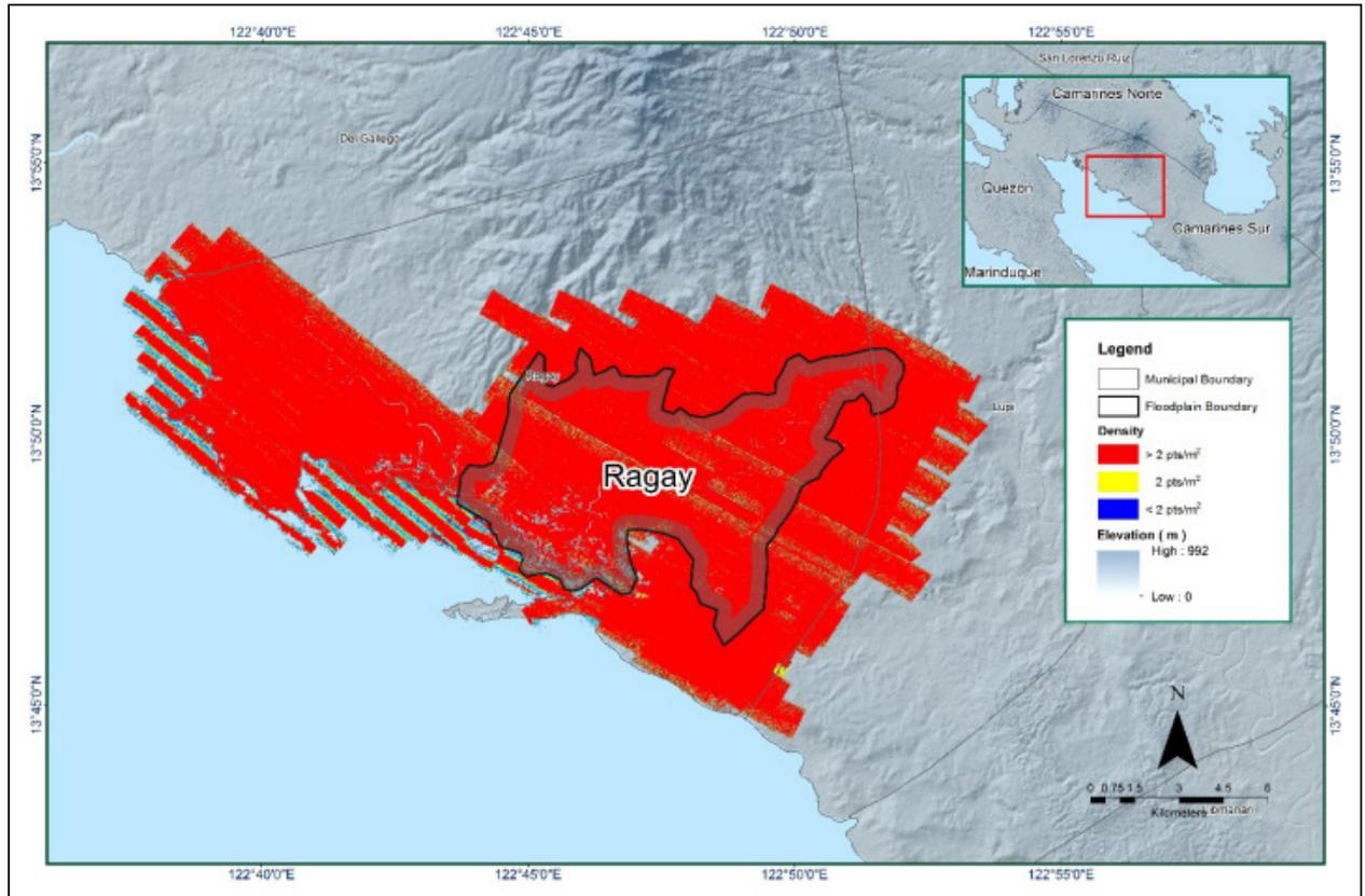
Figure 12. Pulse density map of merged LiDAR data for Ragay Floodplain.
