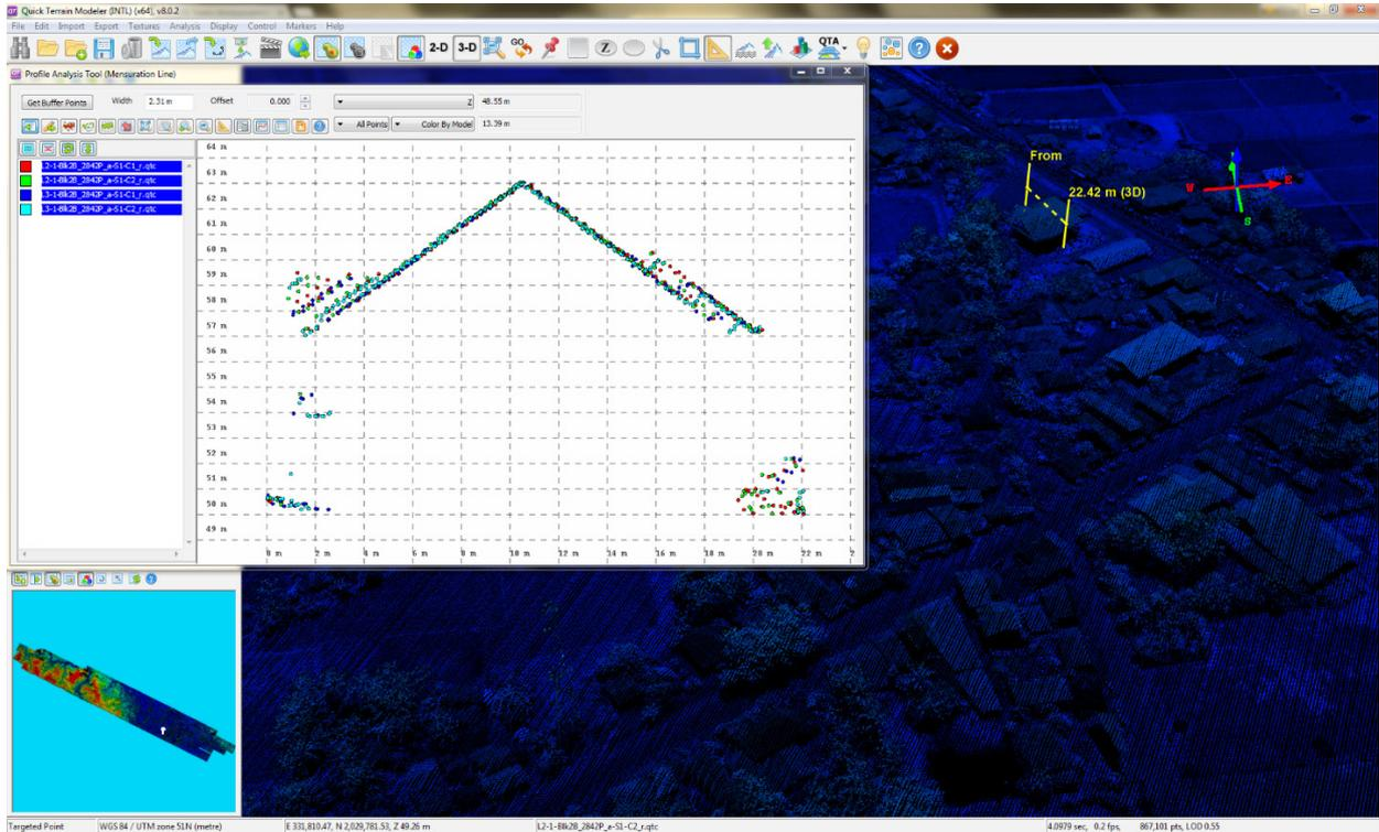
Figure 14. Quality checking for a Ragay flight 2842P using the Profile Tool of QT Modeler.
