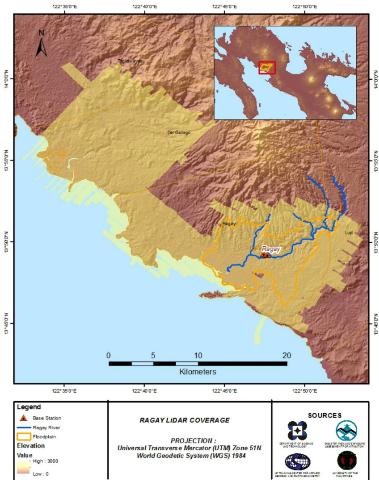
Figure 5. Actual LiDAR survey coverage of the Ragay Floodplain.
