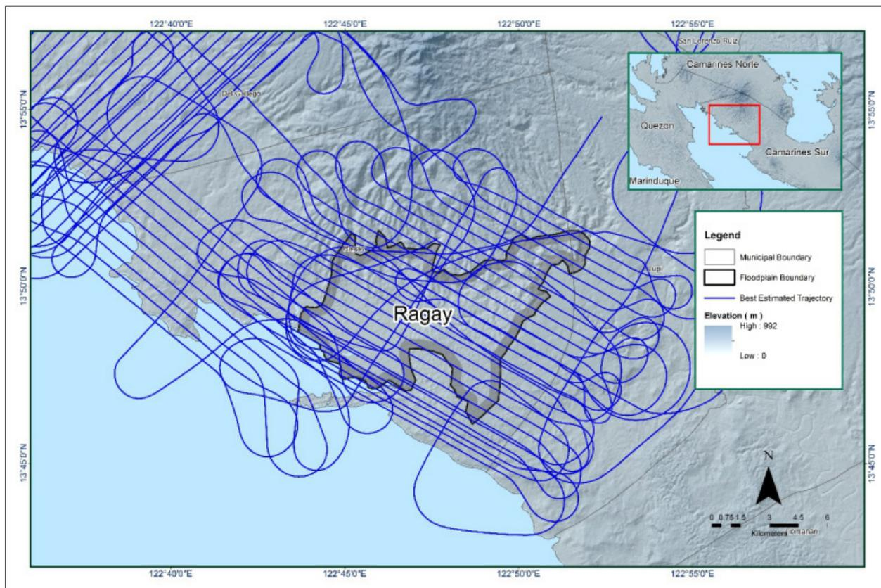
Figure 9. Best Estimated Trajectory of the LiDAR missions conducted over the Ragay Floodplain.
