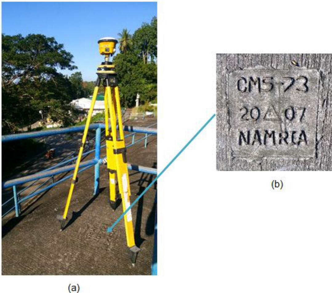
Figure 3. GPS set-up over CMS-73 (a) and NAMRIA reference point CMS-73 (b) as recovered by the field team.
