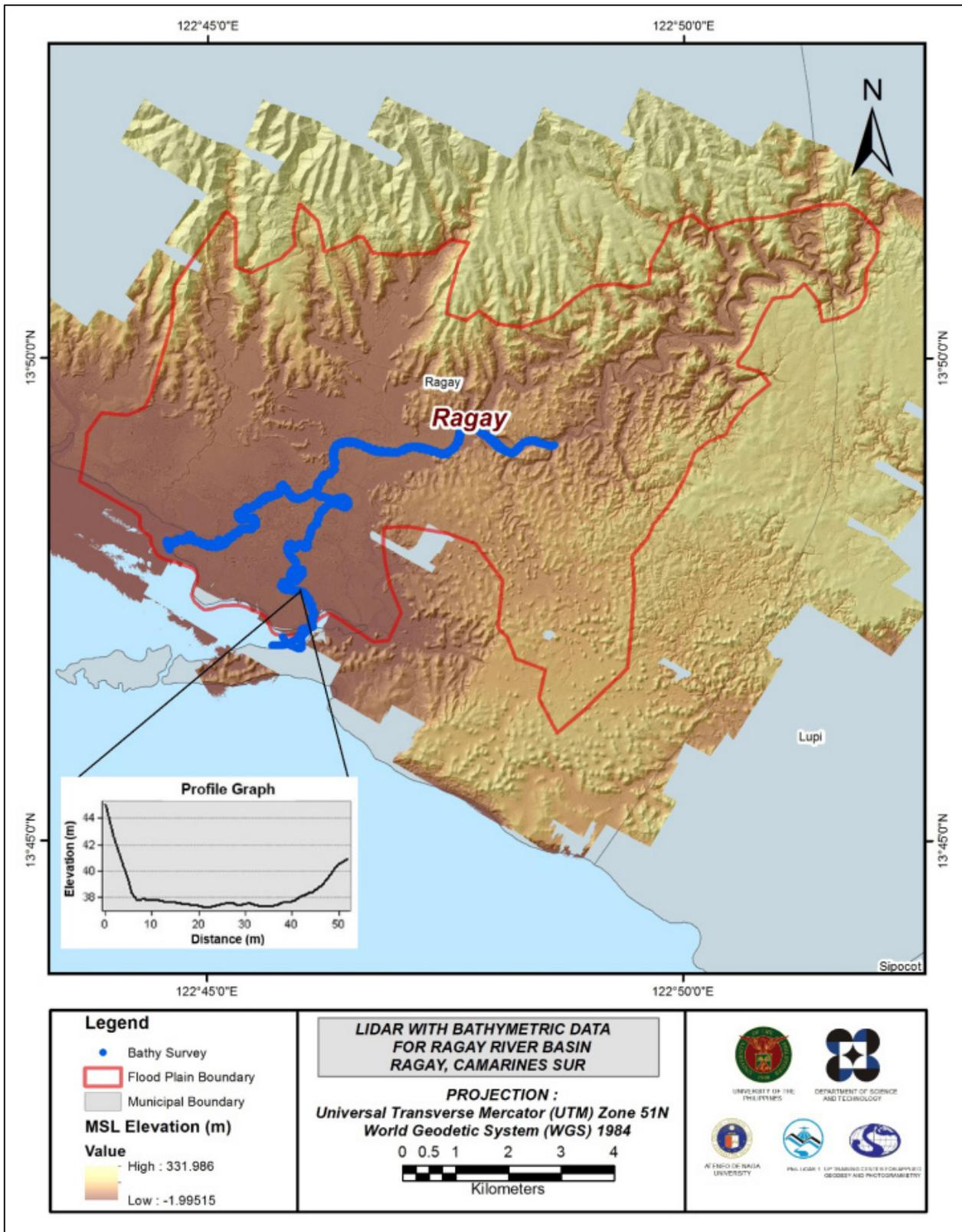
Figure 25. Map of Ragay Floodplain with bathymetric survey points shown in blue.
