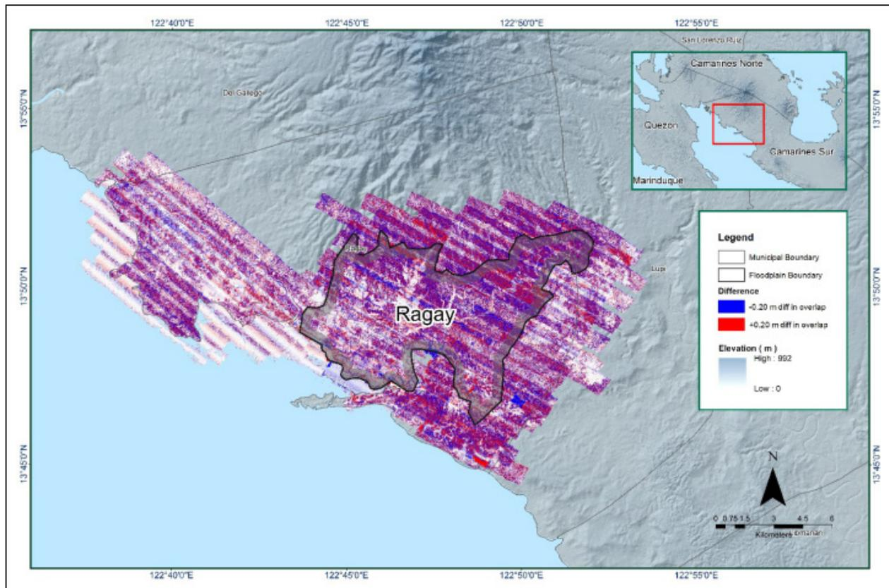
Figure 13. Elevation Difference Map between flight lines for Ragay Floodplain Survey.
