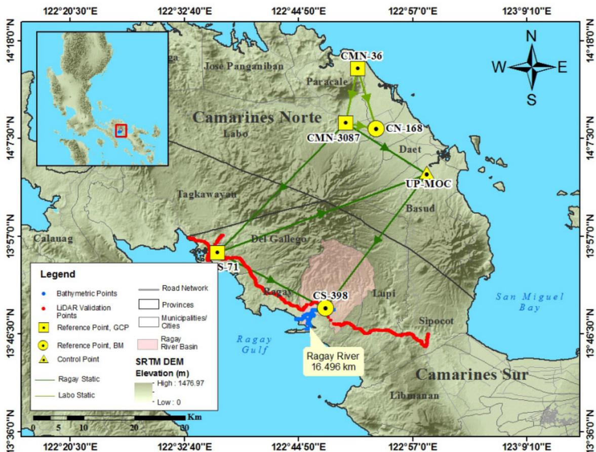
Figure 28. Extent of the bathymetric survey (in blue line) in Ragay River and the LiDAR data validation survey (in red).
