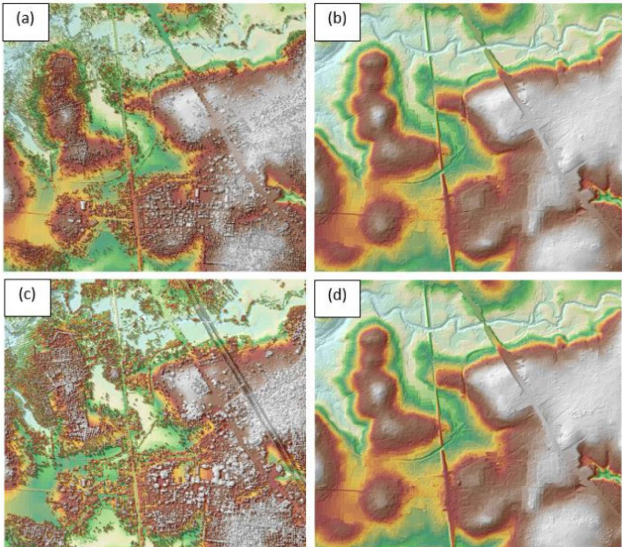
Figure 17. The production of last return DSM (a) and DTM (b), first return DSM (c) and secondary DTM (d) in some portion of Ragay floodplain.
