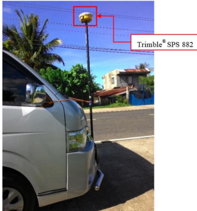
Figure 38. Validation points acquisition survey set up along Ragay River Basin
