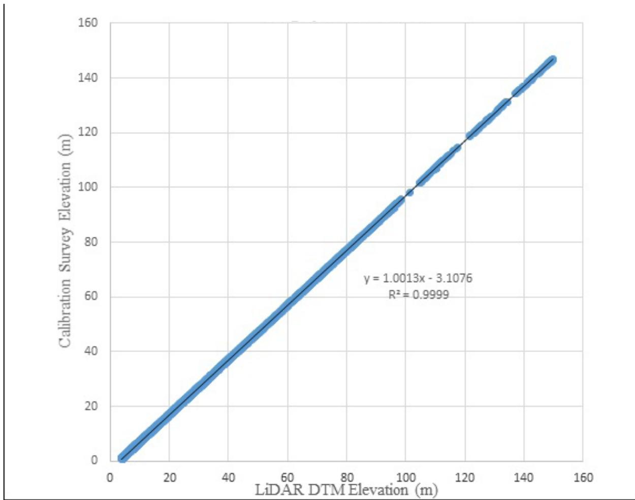
Figure 23. Correlation plot between calibration survey points and LiDAR data.
