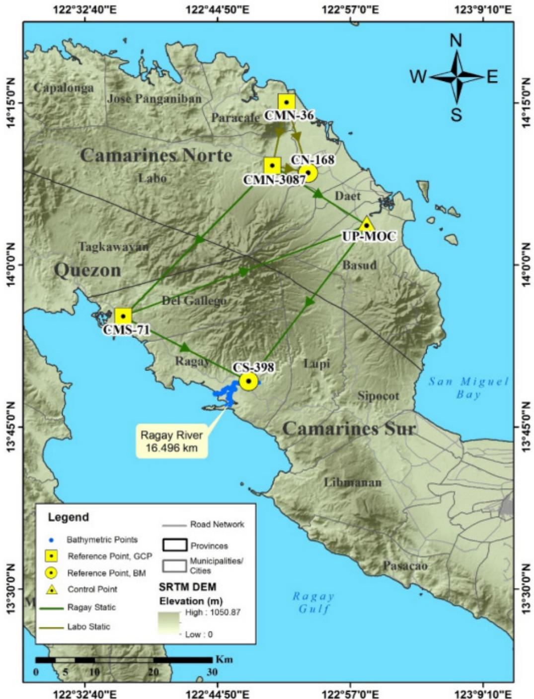
Figure 29. The GNSS Network established in the Ragay River Survey.
