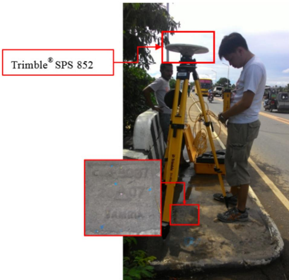
Figure 32. GNSS receiver setup, Trimble® SPS 852, at CMN-3087, located at the approach of Labo Bridge in Brgy. Bakiad, Municipality of Labo, Camarines Norte.
