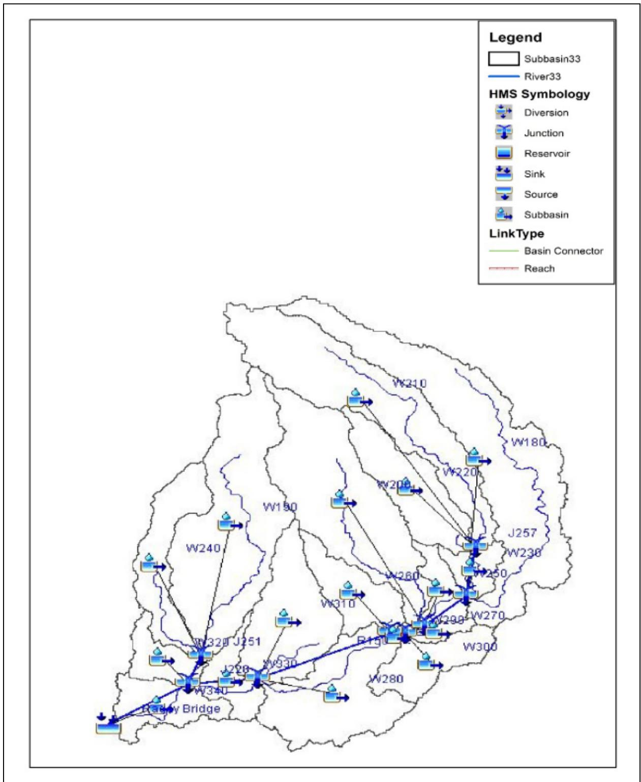
Figure 54. Ragay River Basin model generated in HEC-HMS
