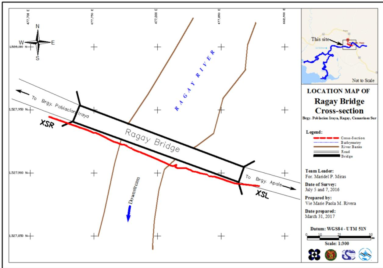
Figure 35. Location map of the Ragay bridge cross-section survey
