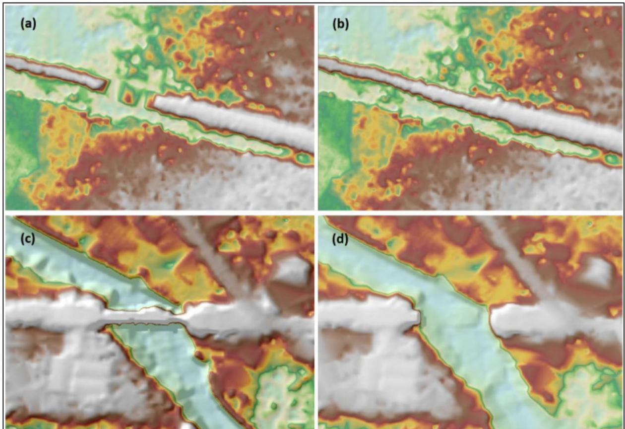
Figure 20. Portions in the DTM of the Ragay Floodplain – a road before (a) and after (b) data retrieval; and a bridge before (c) and after (d) manual editing.
