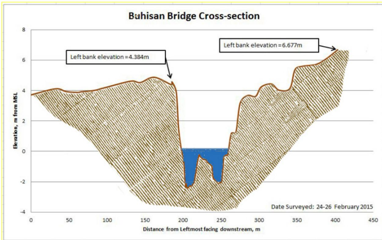
Figure 45. Cross-section plot of Ragay Bridge (also known as Buhisan Bridge)
