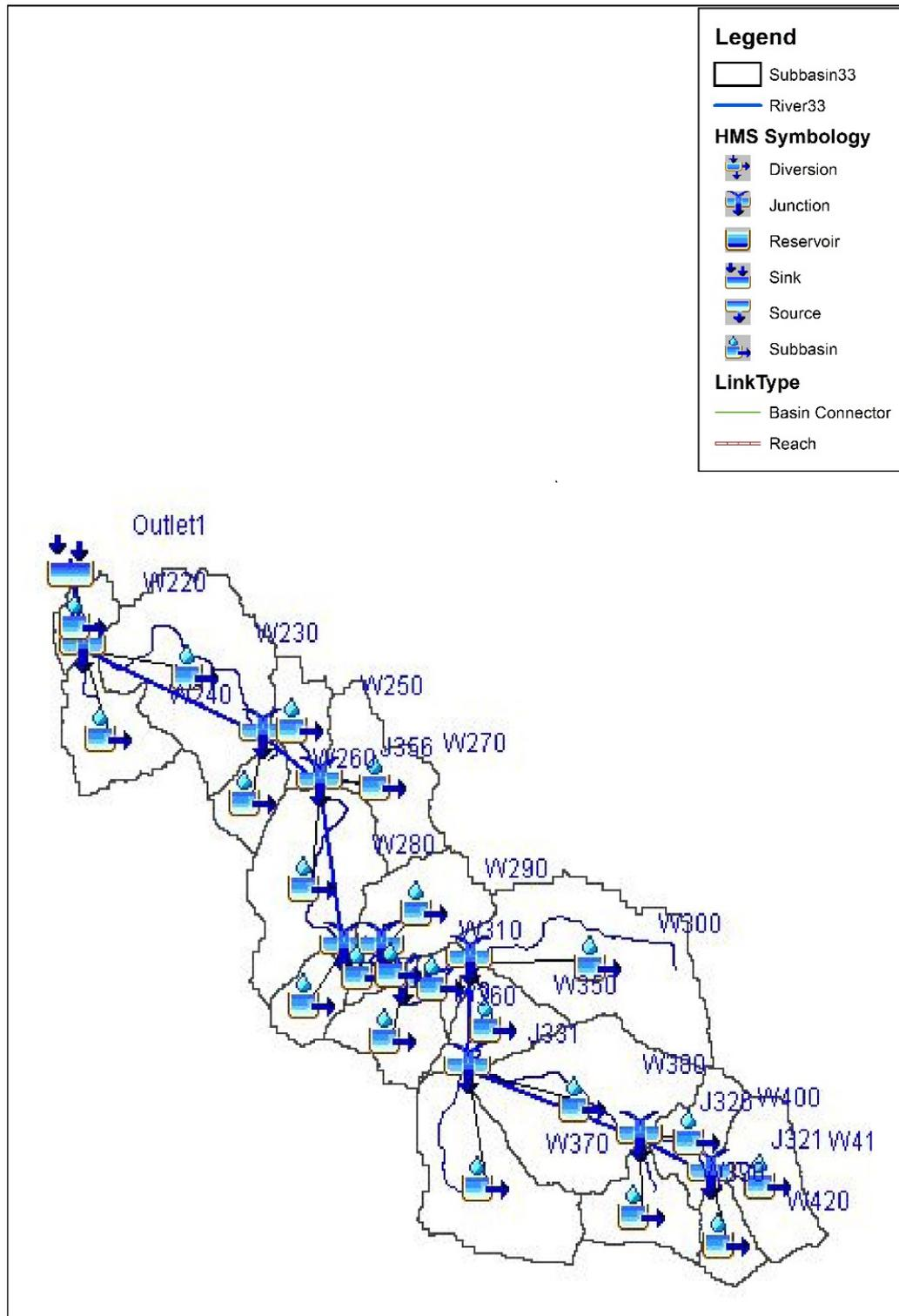
Figure 51. Tambang River Basin model generated in HEC-HMS
