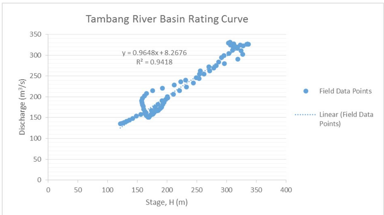
Figure 43. Rating curve of Brgy. Bocogan in Lagonoy, Camarines Sur
