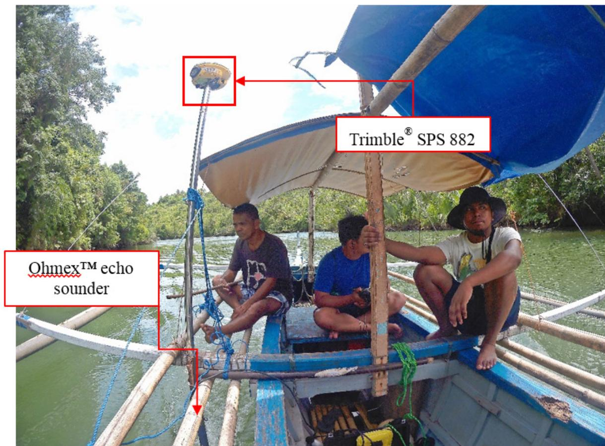
Figure 38. Bathymetric survey using Ohmex™ single beam echo sounder in Tambang River
