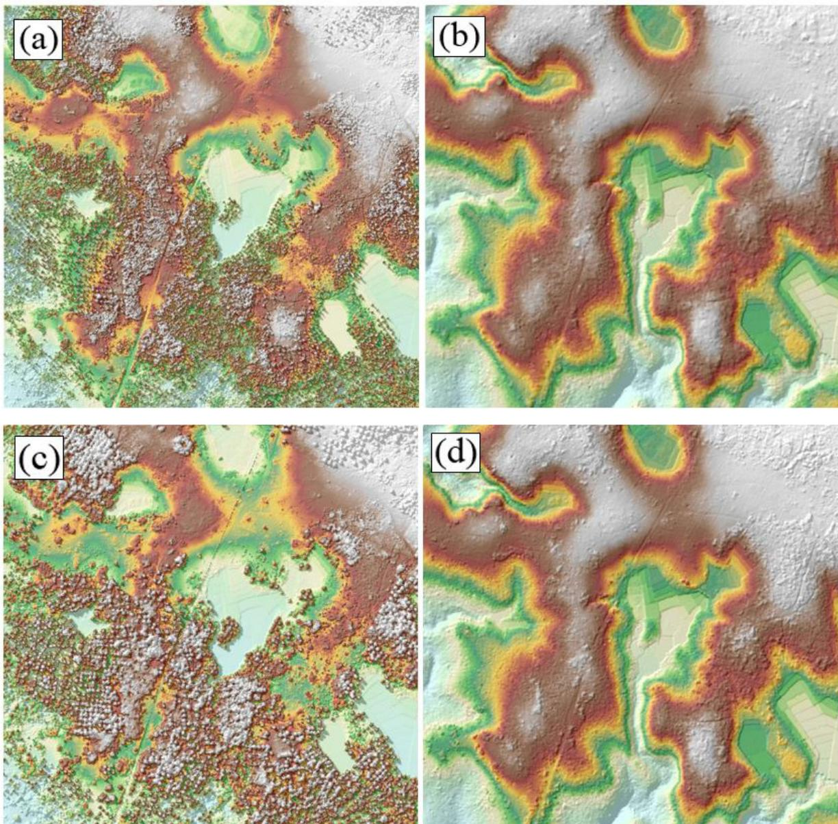
Figure 18. The production of last return DSM (a) and DTM (b), first return DSM (c) and secondary DTM (d) in some portion of Tambang Floodplain.
