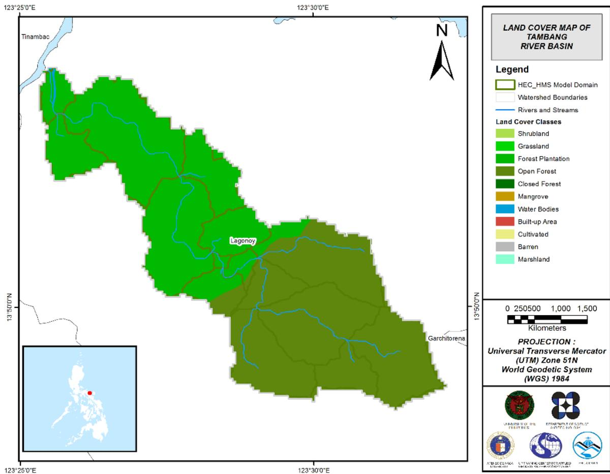
Figure 48. Land Cover Map of Tambang River Basin used for the estimation of the Curve Number (CN) and the watershed lag parameters of the rainfall-runoff model.
