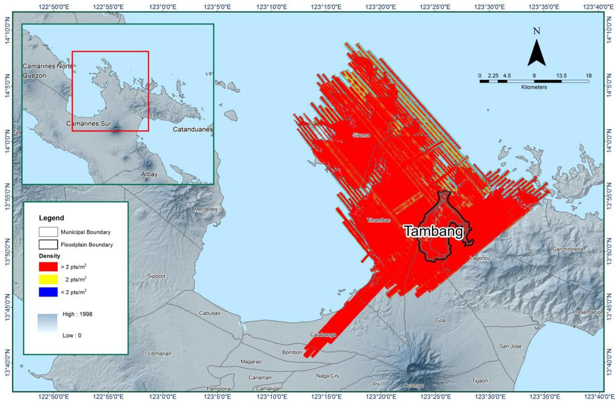
Figure 13. Pulse density map of merged LiDAR data for Tambang Floodplain.
