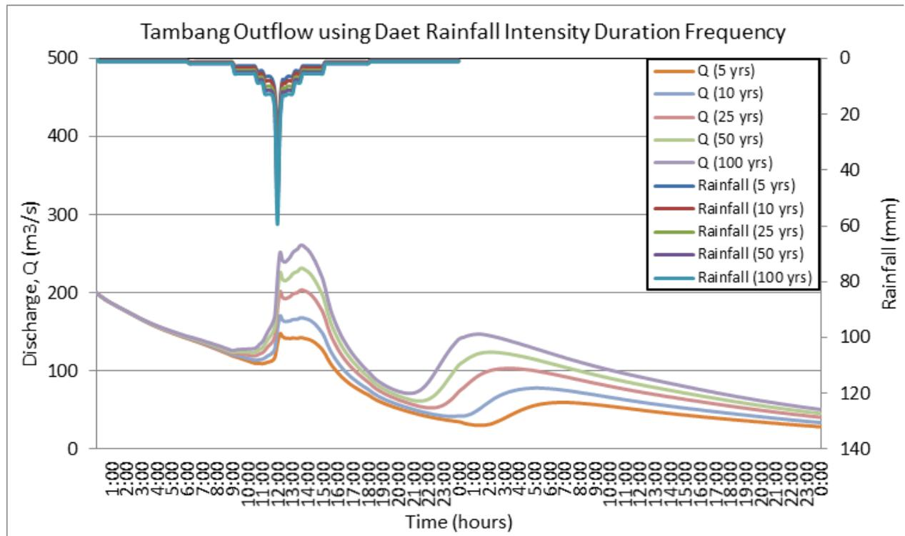
Figure 55. Outflow hydrograph at the Tambang Basin generated using the simulated rain events for 24-hour period for Daet station
