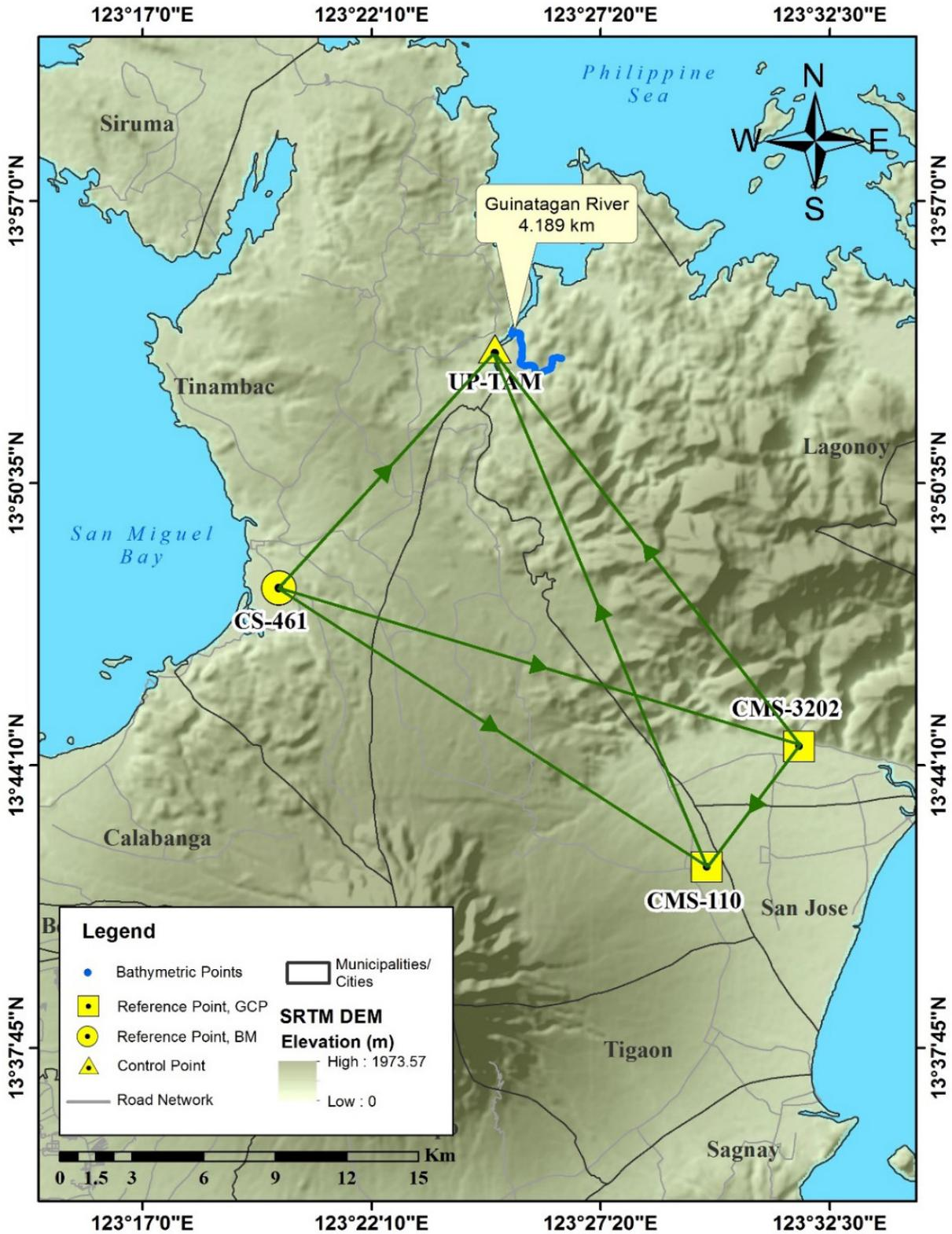
Figure 28. The GNSS Network established in the Tambang River Survey.
