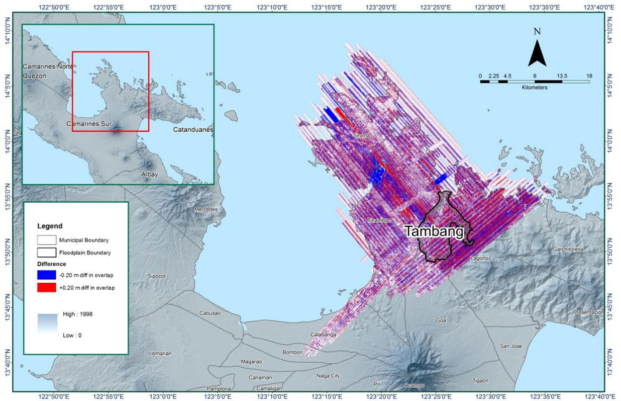
Figure 14. Elevation Difference Map between flight lines for Tambang Floodplain Survey.
