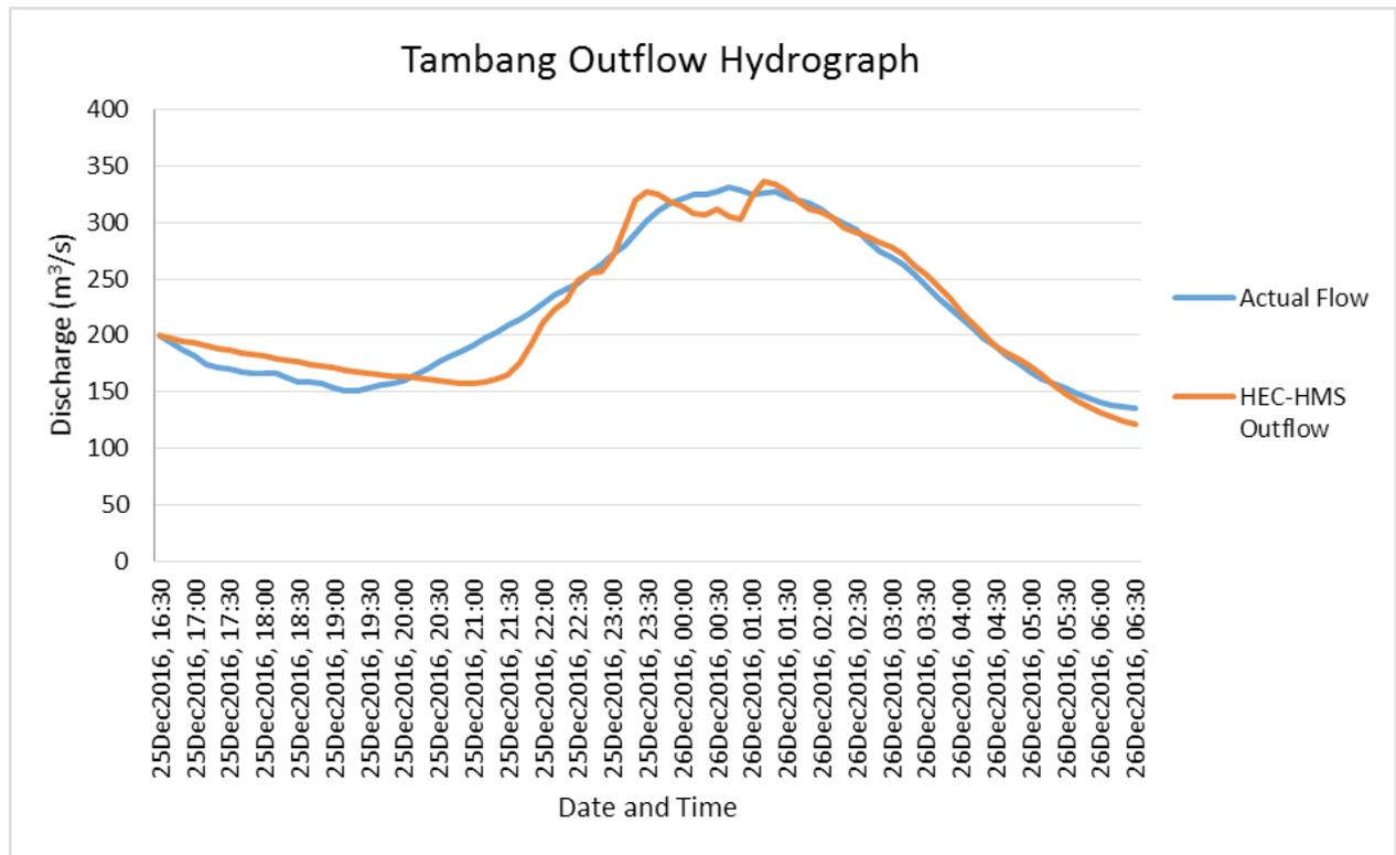
Figure 54. Outflow hydrograph of Tambang produced by the HEC-HMS model compared with observed outflow
