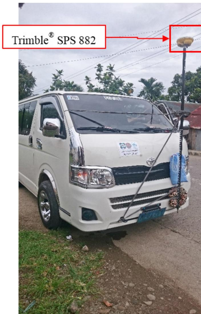
Figure 36. Validation points acquisition survey set up along Tambang River Basin
