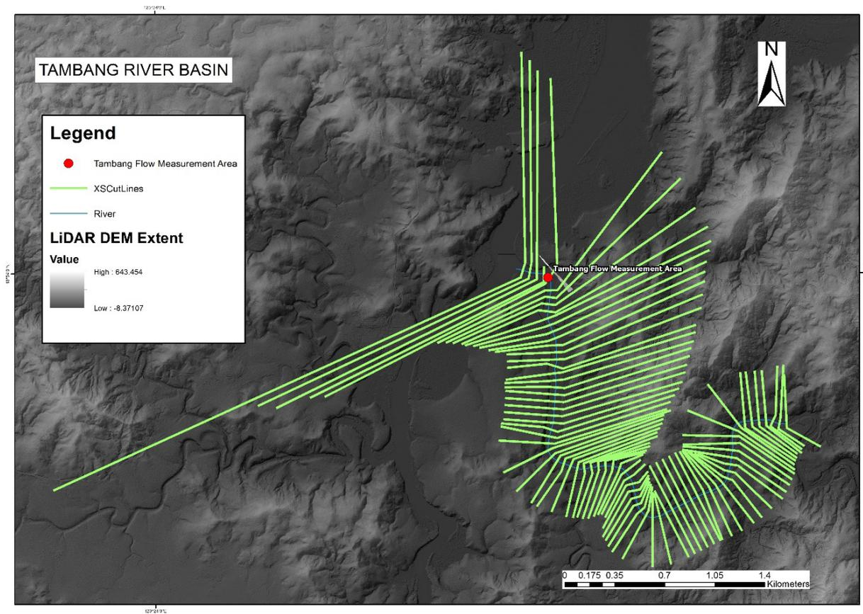
Figure 52. River cross-section of Tambang River generated through Arcmap HEC GeoRAS tool
