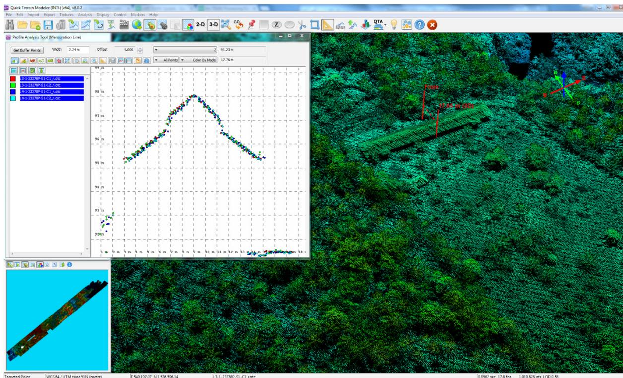
Figure 15. Quality checking for Tambang Flight 23278P using the Profile Tool of QT Modeler.
