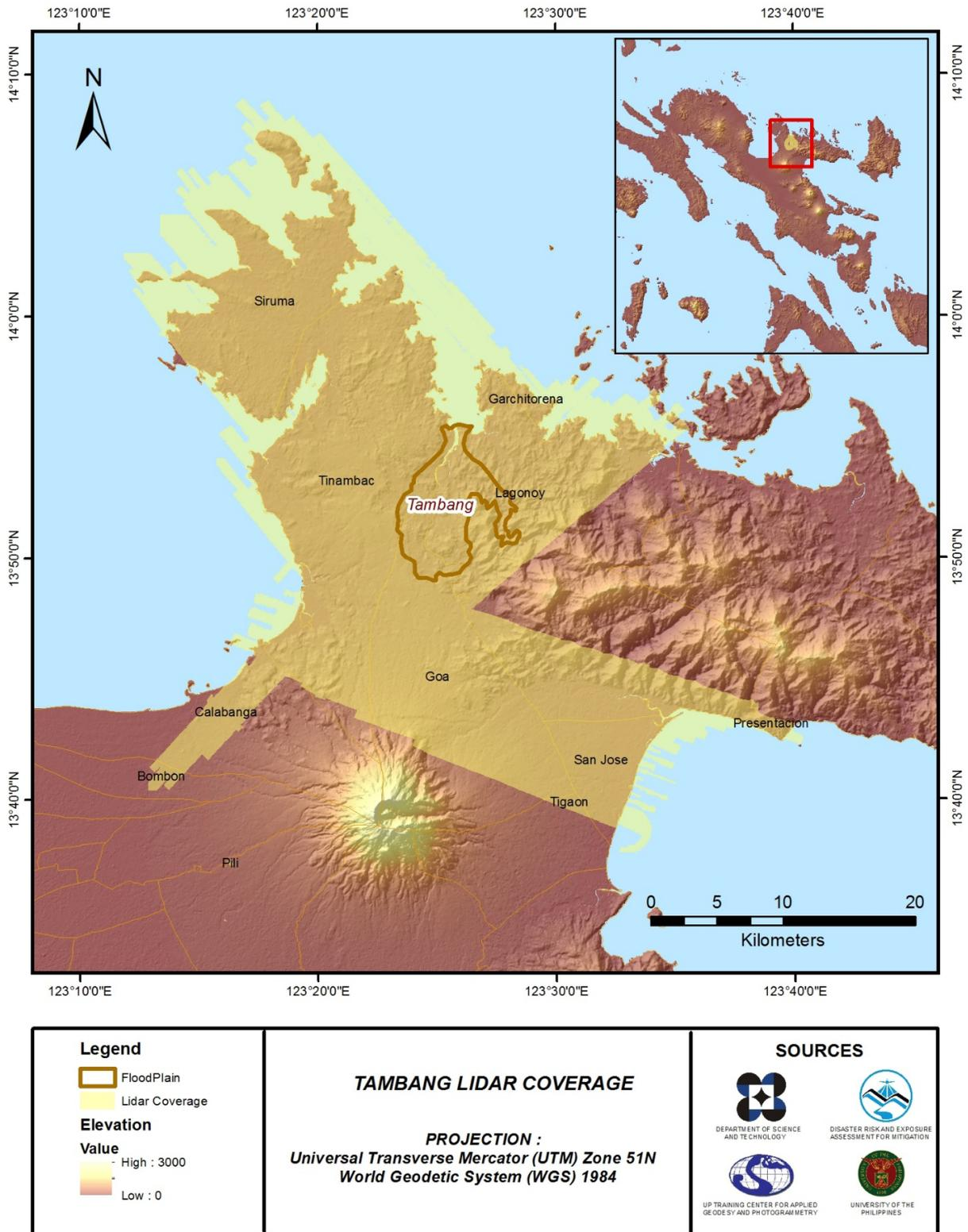
Figure 6. Actual LiDAR survey coverage of the Tambang Floodplain.
