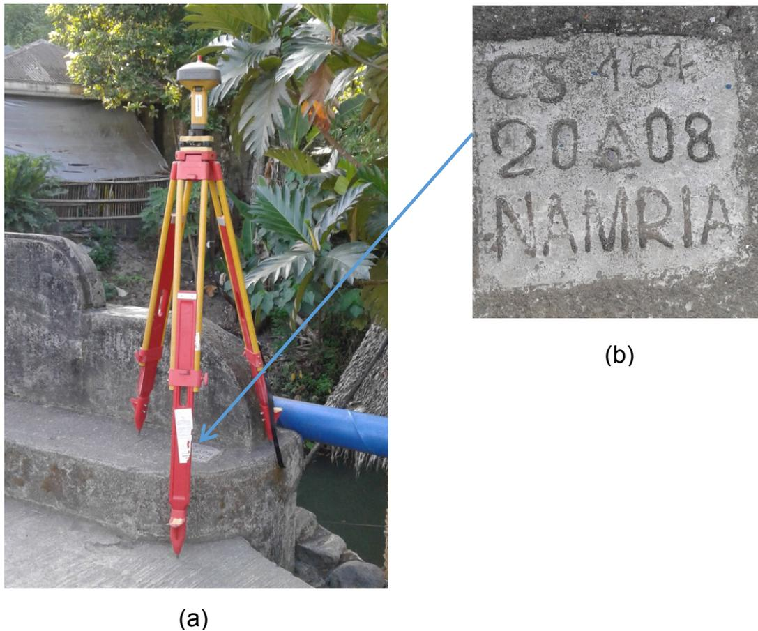
Figure 5. GPS set-up (a) over CS-464 located in the Municipality of Mananao, Province of Camarines Sur, and NAMRIA benchmark CS-464 (b) as recovered by the field team.
