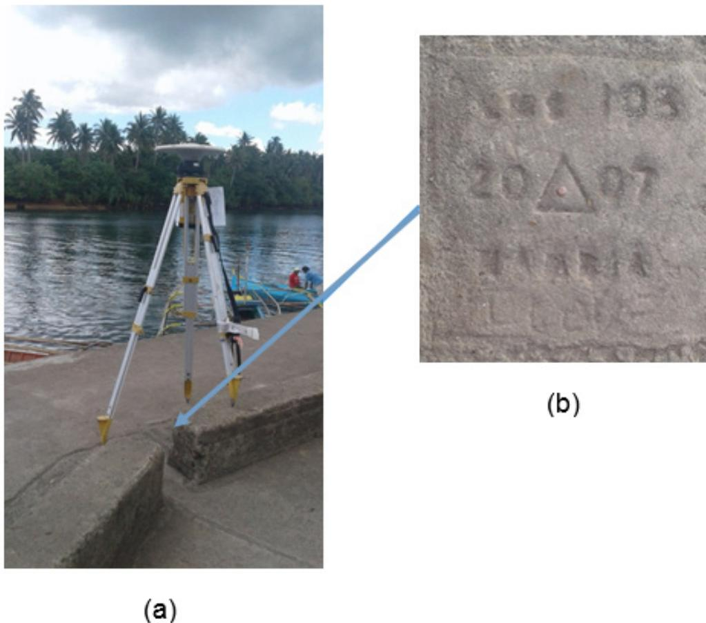
Figure 3. GPS set-up (a) over CMS-103 located at Tamban port area on top of the seawall, and NAMRIA reference point CMS-103 (b) as recovered by the field team.
