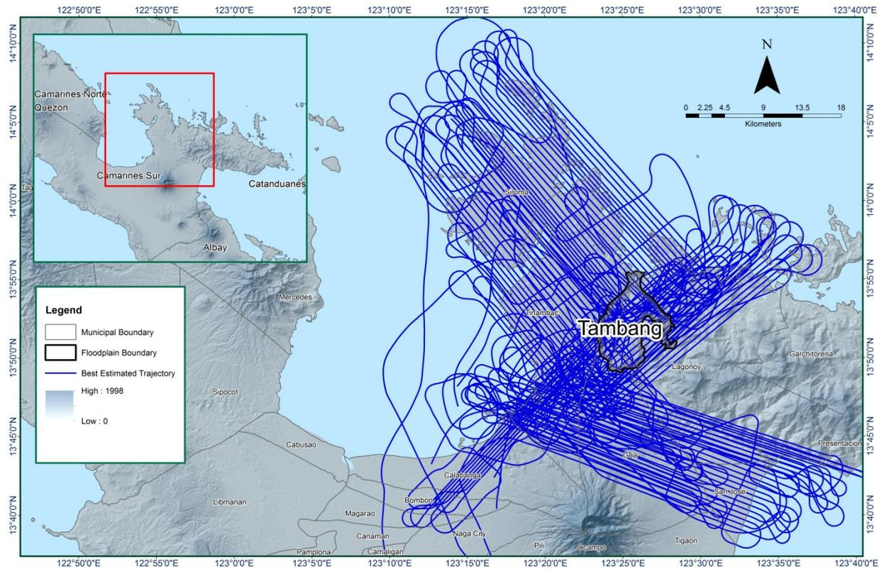
Figure 10. Best Estimated Trajectory of the LiDAR missions conducted over the Tambang Floodplain.
