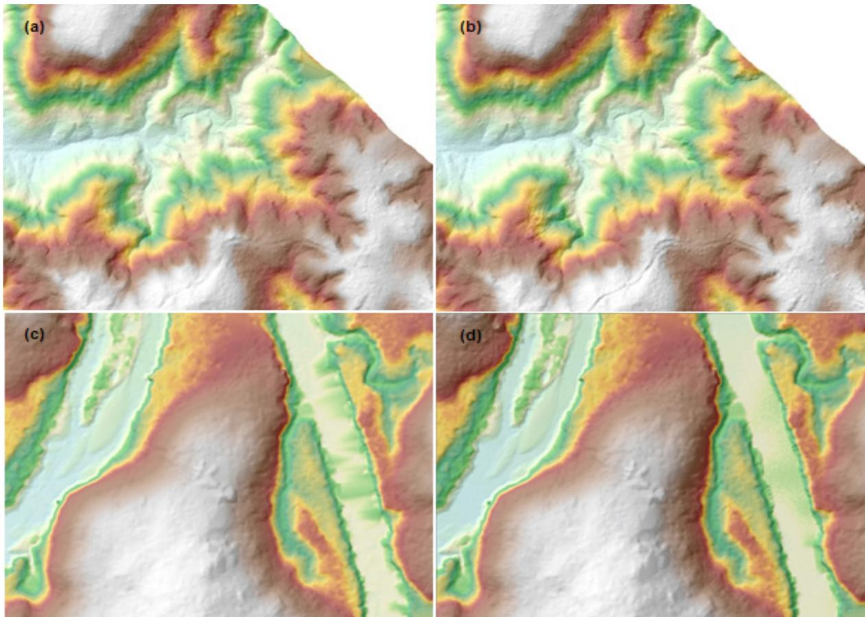
Figure 19. Portions in the DTM of Tambang Floodplain –a mountain ridge before (a) and after (b) data retrieval; a triangulated riverbank before (c) and after (d) manual editing
