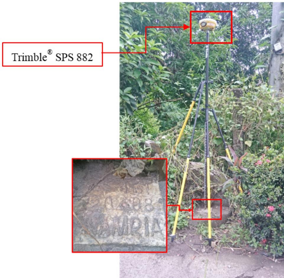
Figure 30. GNSS receiver setup, Trimble® SPS 882, at CS-461, located at the approach of a bridge in Brgy. Balaobalite, Municipality of Tinambac, Camarines Sur
