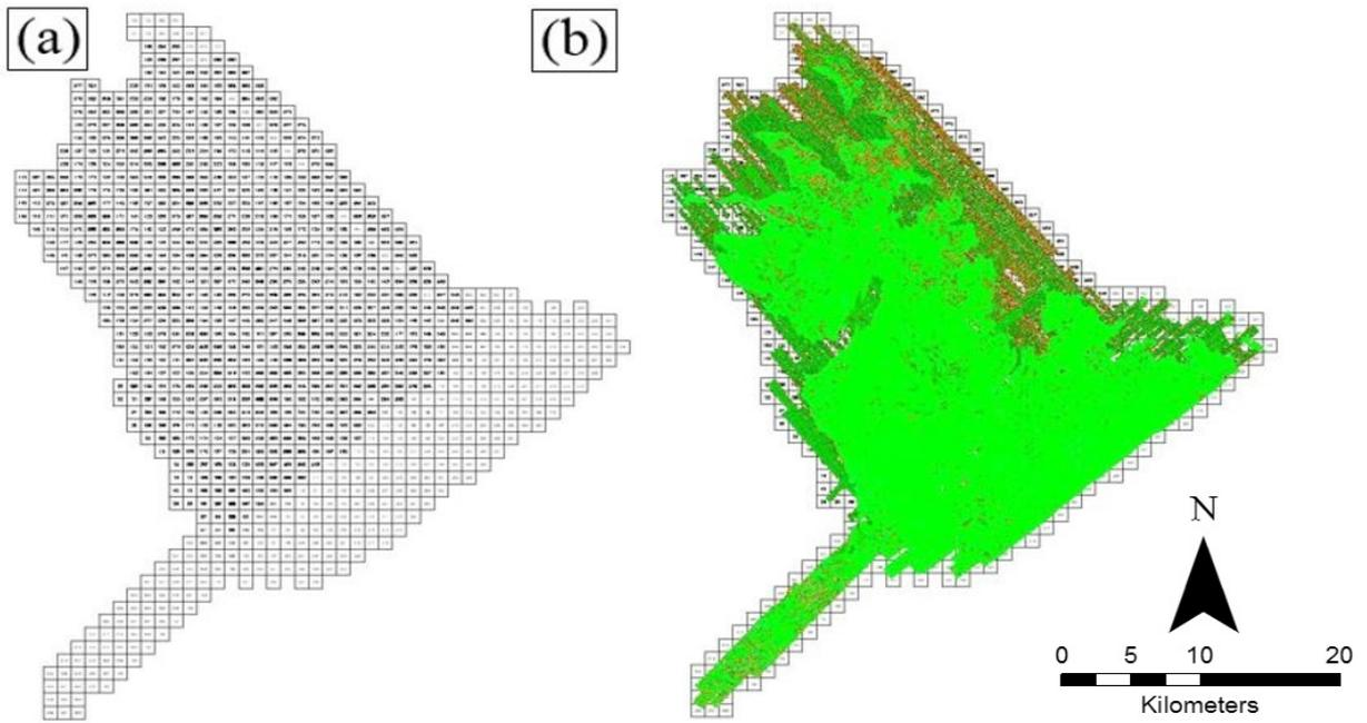
Figure 16. Tiles for Tambang Floodplain (a) and classification results (b) in TerraScan.
