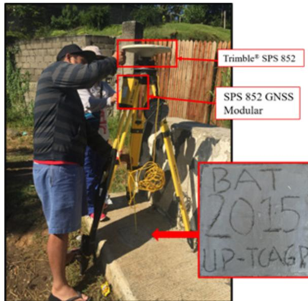
Figure 31. GNSS receiver, Trimble® SPS 852 setup at control point BAT, at Batu Bridge in Brgy. Batu, Municipality of Siay, Zamboanga Sibugay along the PAN-Philippine National Highway
