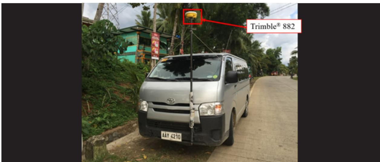
Figure 37. Trimble® SPS882 set-up for validation points acquisition survey for Maligaya River
