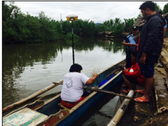
*Figure 39. Bathymetric Survey with echosounder in Batu River*
