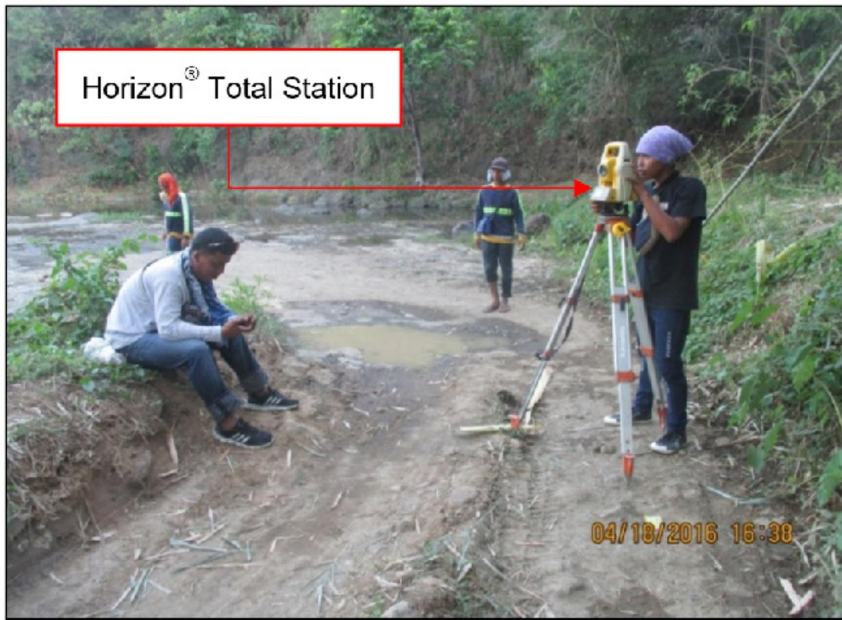
Figure 43. Manual bathymetric survey of ABSD at Buluan River using Horizon® Total Station
