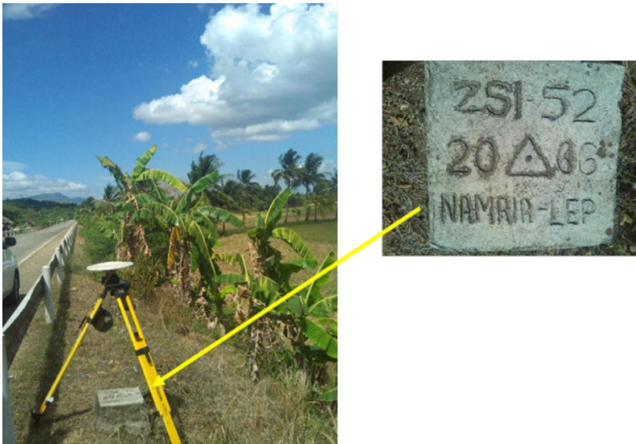
Figure 6. GPS set-up over ZSI-52 at Barangay Tupilac, Zamboanga Sibugay (a) and NAMRIA reference point ZSI-52 (b) as recovered by the field team.
