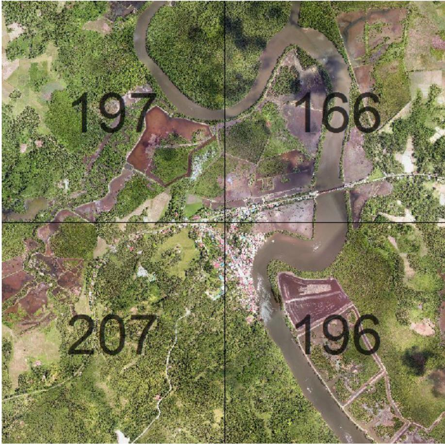
Figure 21. Sample orthophotograph tiles for Buluan Floodplain.
