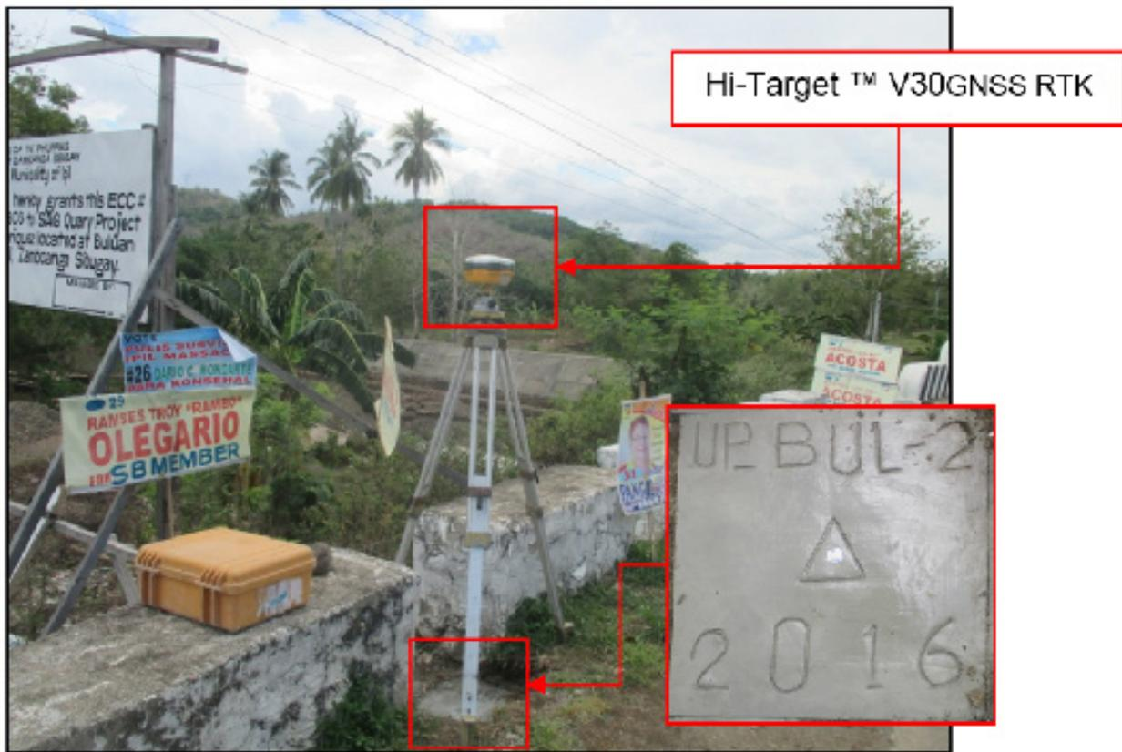
Figure 34. GNSS receiver set up, Hi-Target™ V30, at UP\_BUL-2, located on the side of the National Road near the bridge in Brgy. Bulu-An, Ipil, Province of Zamboanga Sibugay.
