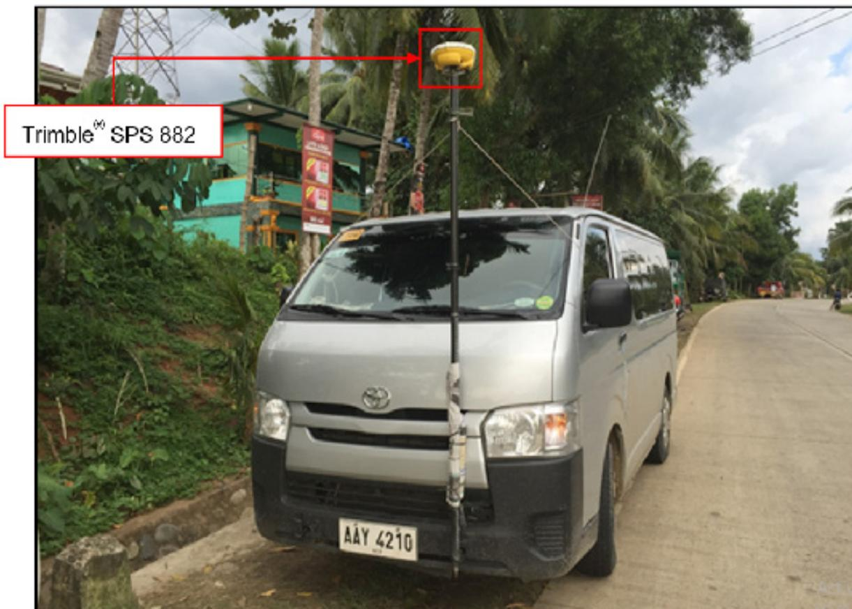
Figure 41. Validation points acquisition survey set-up for Tupilac River
