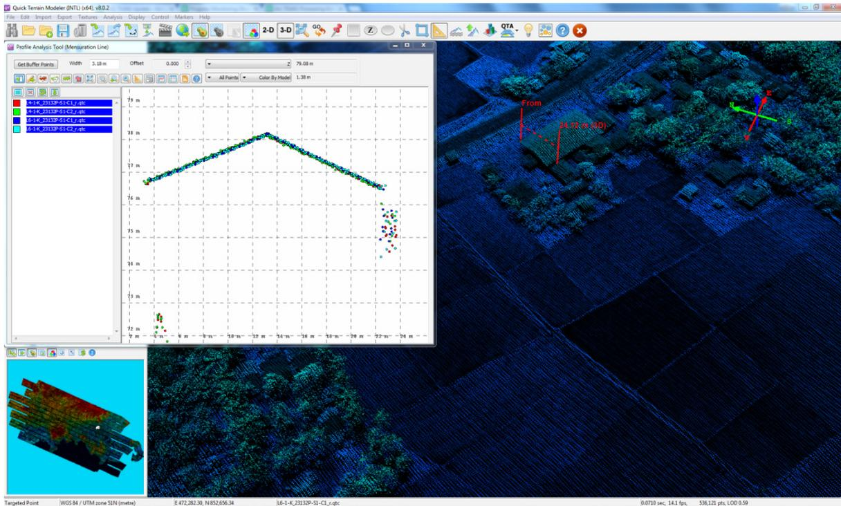
Figure 17. Quality checking for a Kabasalan flight 23132P using the Profile Tool of QT Modeler
