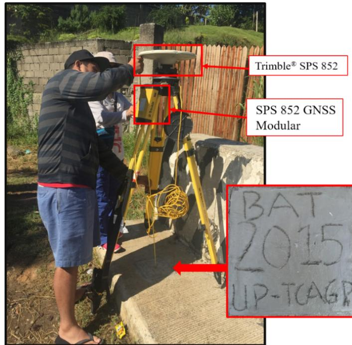
Figure 33. GNSS receiver, Trimble® SPS 852 set-up at control point BAT, at Batu Bridge in Brgy. Batu, Municipality of Siay, Zamboanga Sibugay along the PAN-Philippine National Highway
