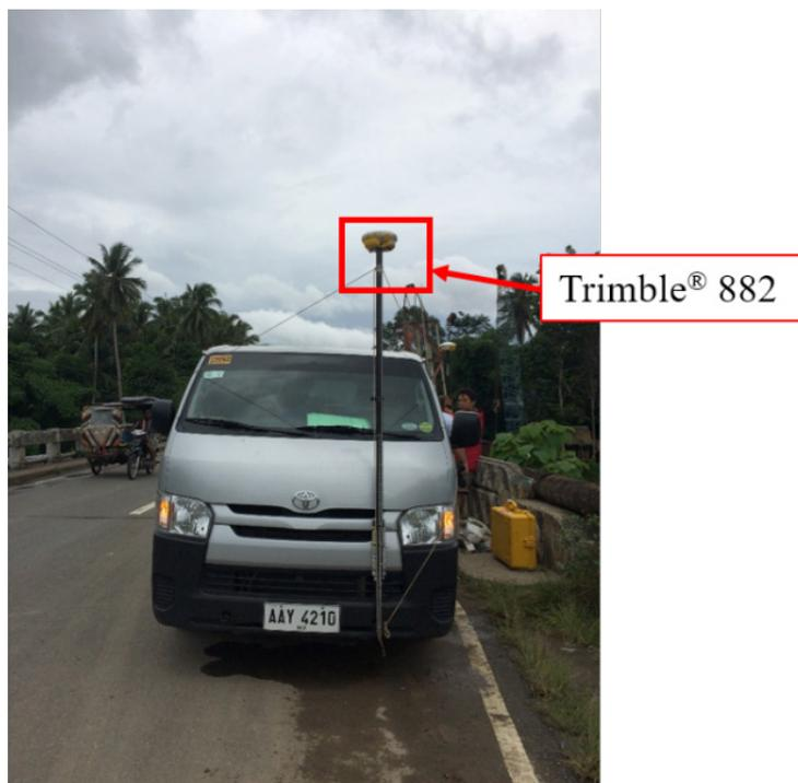
Figure 39. Trimble SPS882 set-up on a vehicle for validation points acquisition along the major roads near Kabasalan River
