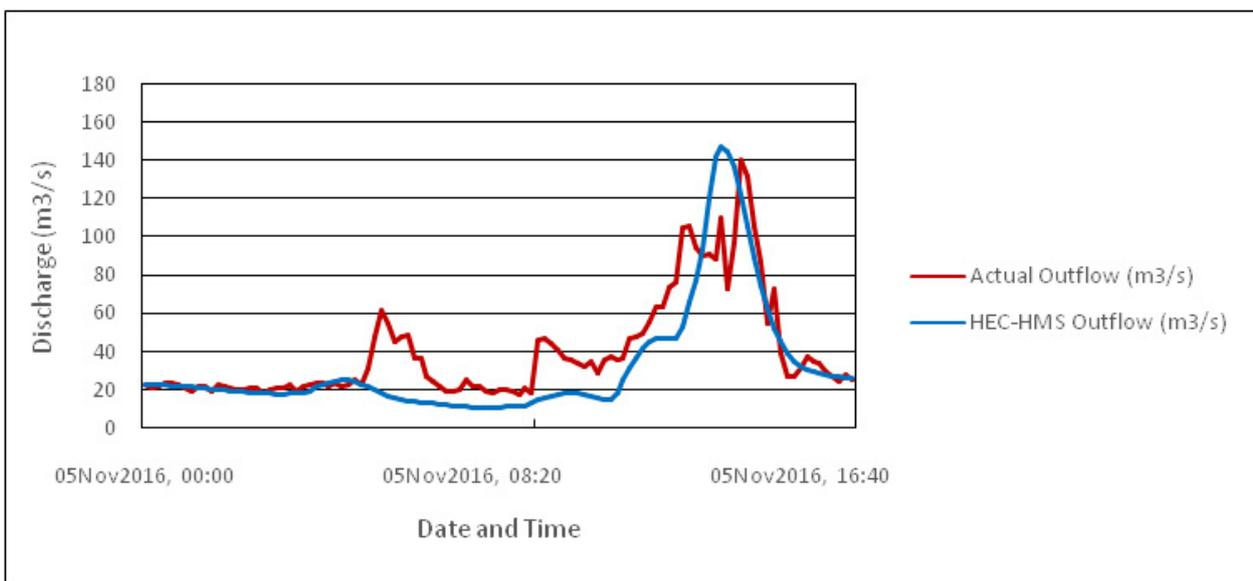
Figure 59. Outflow hydrograph of Kabasalan produced by the HEC-HMS model compared with observed outflow
