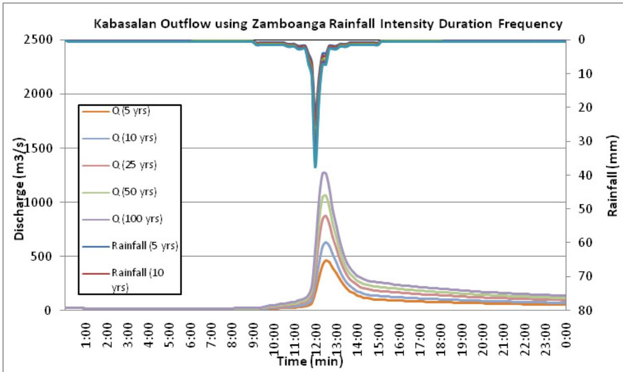
Figure 60. Outflow hydrograph at Tulay ng Pangulo Station generated using Zamboanga City RIDF simulated in HEC-HMS
