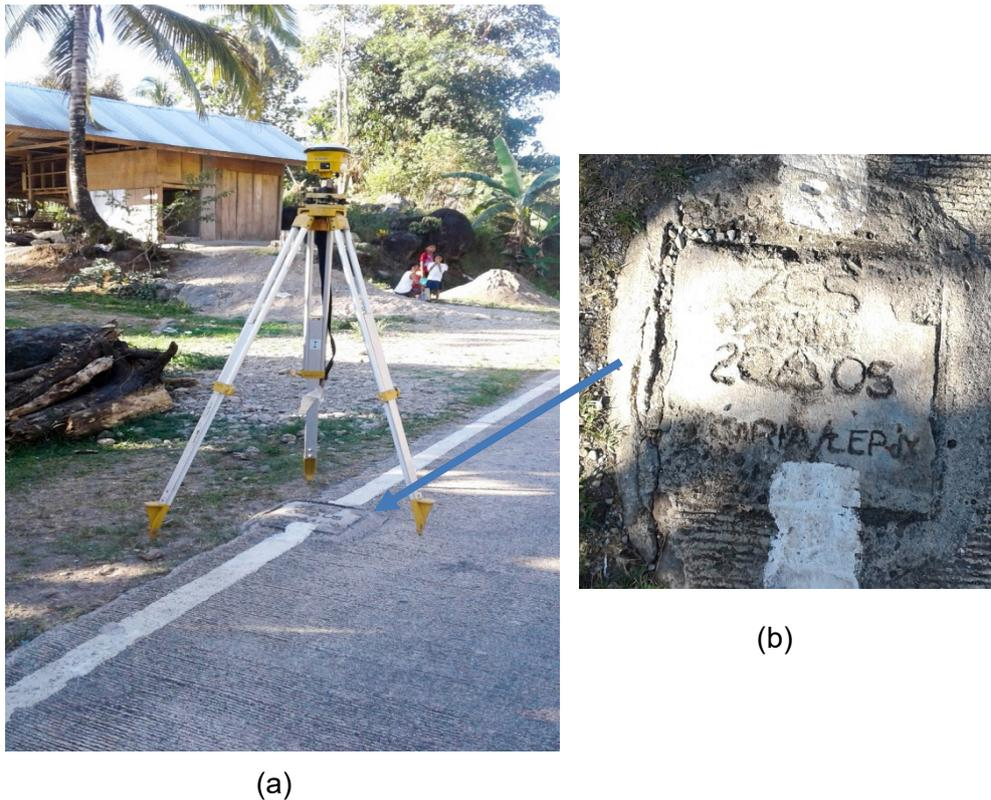
Figure 6. GPS set-up over ZGS-58 at Brgy. Sicade, Municipality of Kumalarang, Zamboanga del Sur (a) and NAMRIA reference point ZGS-58 (b) as recovered by the field team
