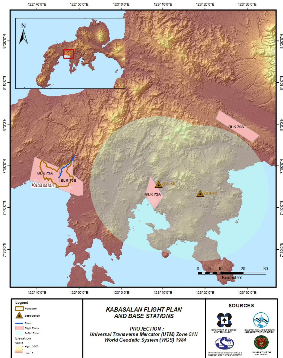
Figure 5. Flight plan and base stations used for Kabasalan Floodplain
