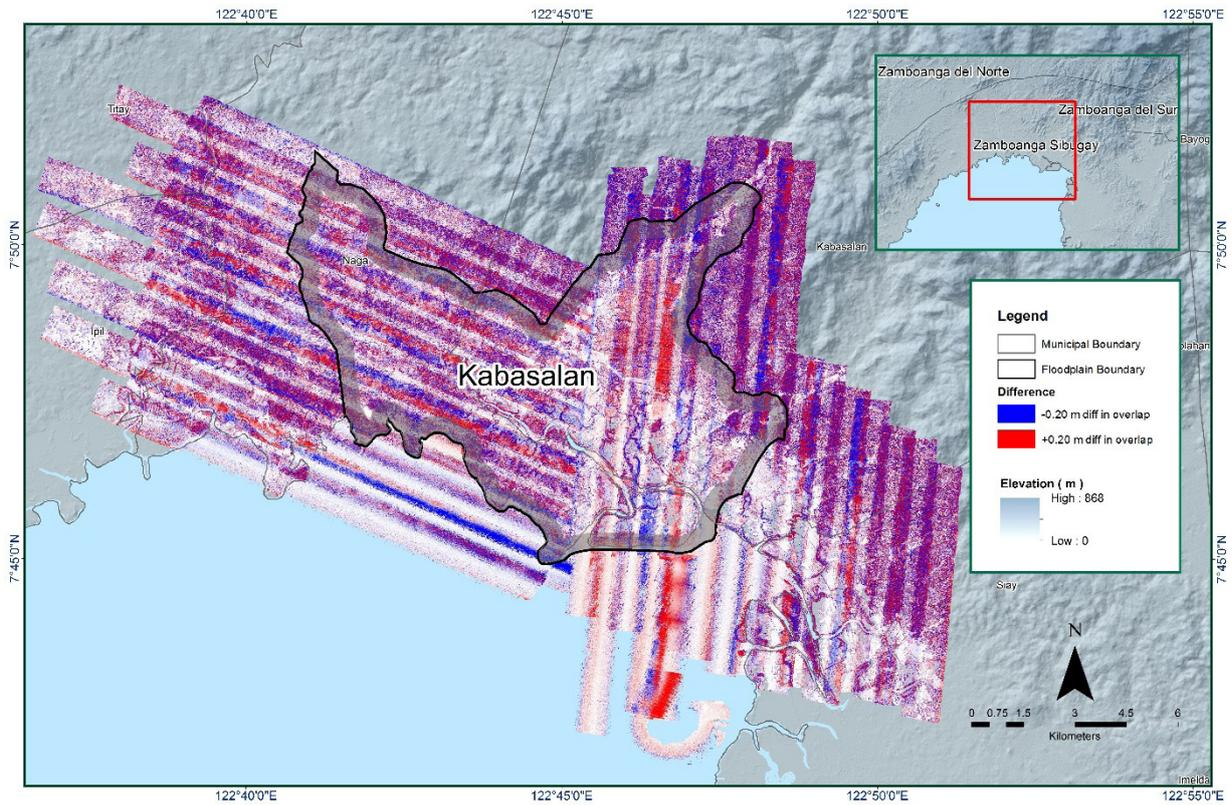
Figure 16. Elevation difference between flight lines for Kabasalan Floodplain
