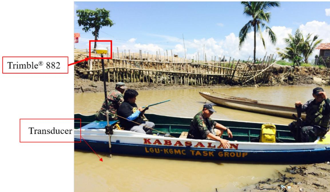
Figure 41. Bathymetric survey instrument set-up on a borrowed boat from Kabasalan local government accompanied by the Philippine Army personnel
