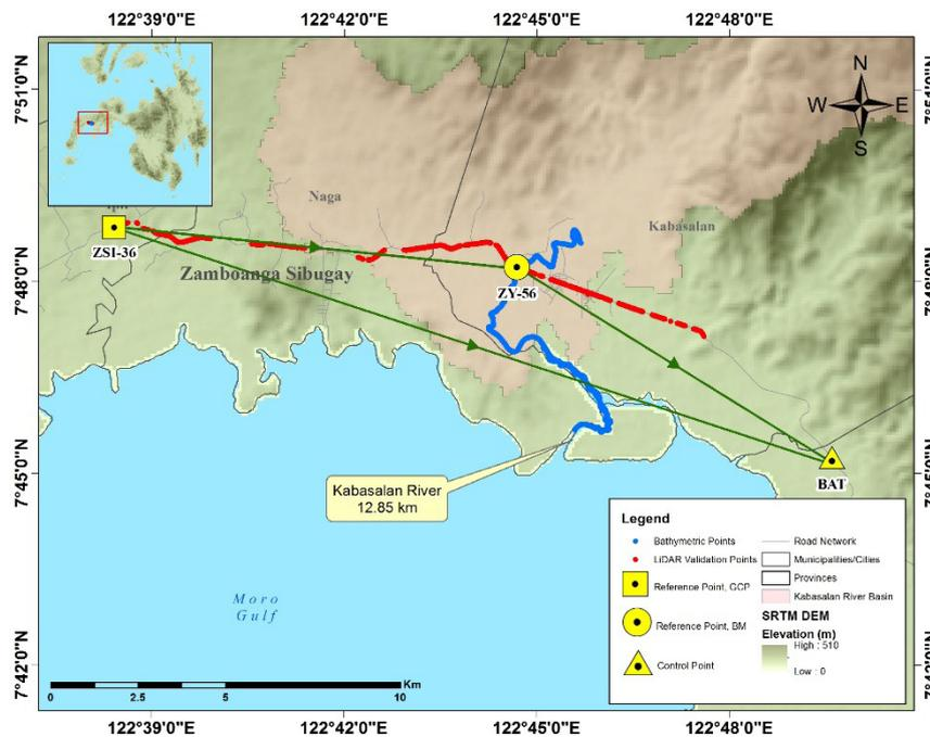
Figure 29. Extent of the bathymetric survey (in blue line) in Kabasalan River and the LiDAR data validation survey (in red)
