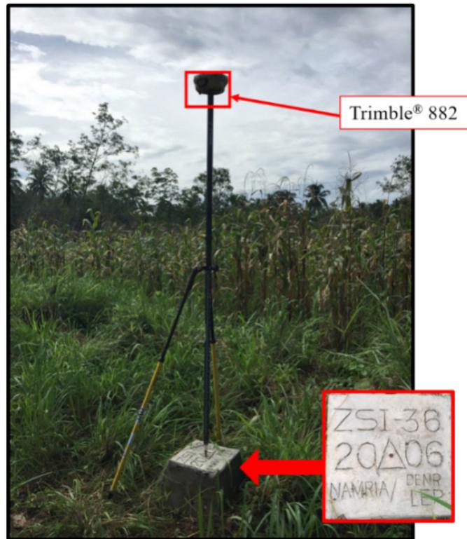
Figure 31. GNSS receiver, Trimble® SPS 882 set-up at reference point ZSI-36, in front of Iglesia Ni Cristo church along the National Highway, Brgy. Bacalan, Municipality of Ipil, Zamboanga Sibugay
