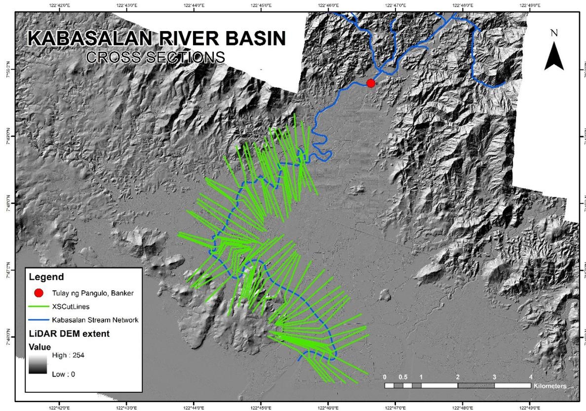
Figure 55. River cross-section of Kabasalan River generated through Arcmap HEC GeoRAS tool
