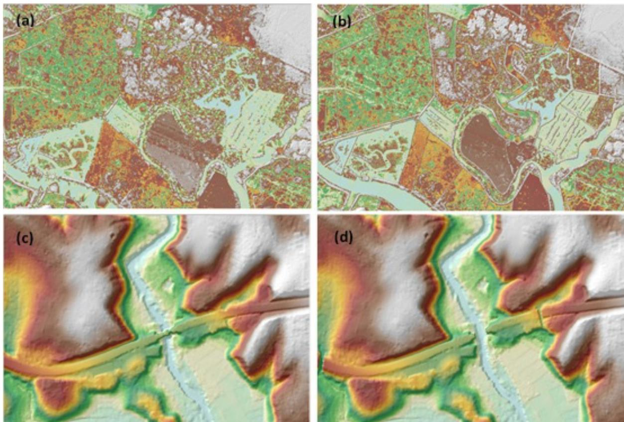
Figure 21. Portions in the DTM of Kabasalan Floodplain—a paddy field before (a) and after (b) data retrieval; a bridge before (c) and after (d) manual editing
