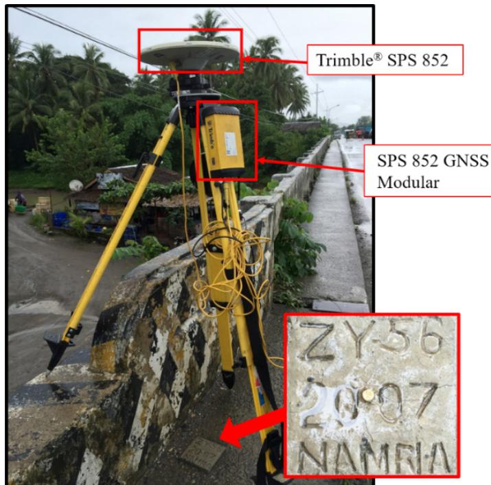
Figure 32. GNSS receiver, Trimble® SPS 852 set-up at benchmark ZY-56, along the Pagadian-Zamboanga National Road at the end of Kabasalan Bridge, Brgy. Sininan, Municipality of Kabasalan, Zamboanga Sibugay
