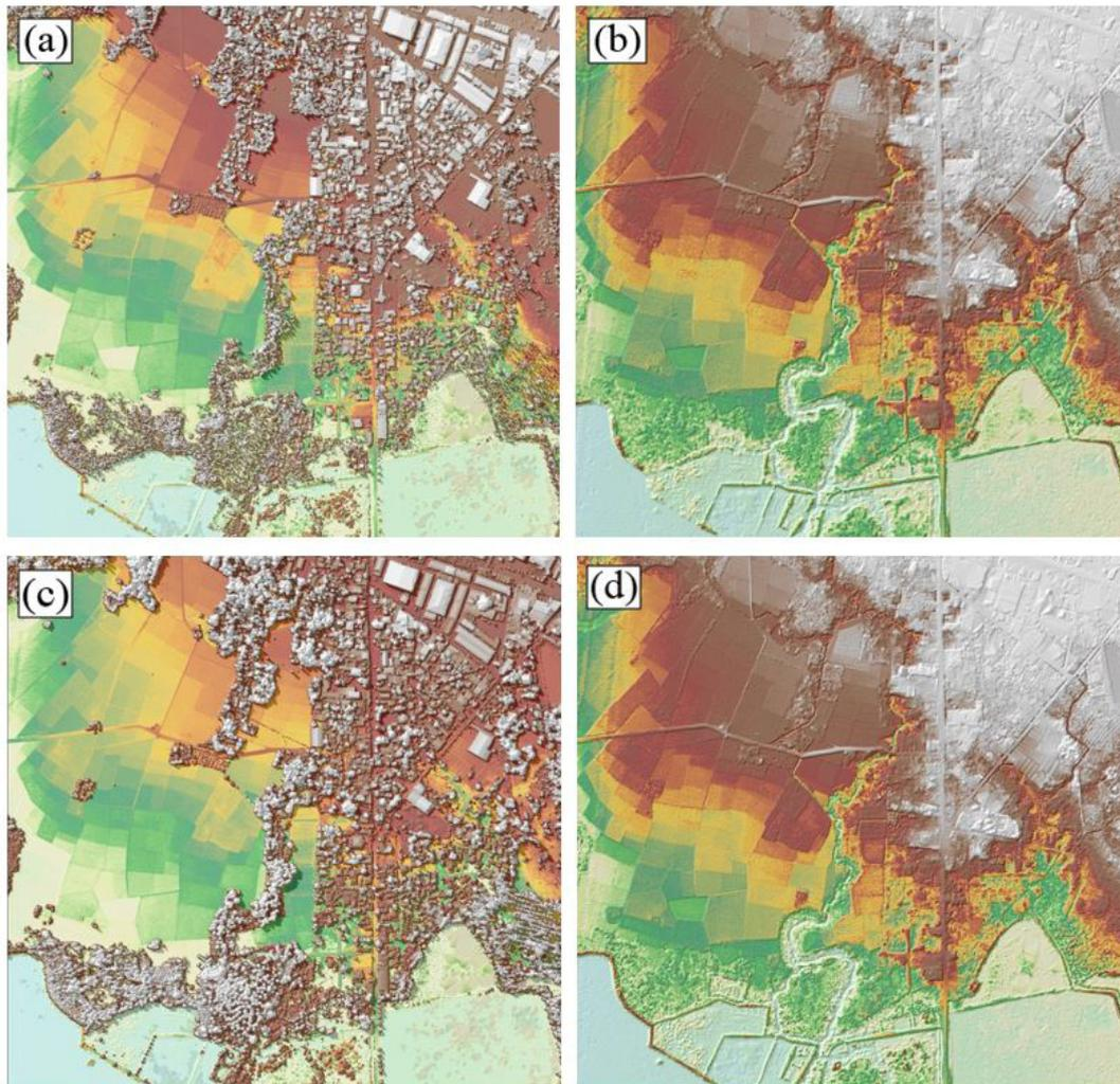
Figure 20. The production of last return DSM (a) and DTM (b), first return DSM (c) and secondary DTM (d) in some portion of Kabasalan Floodplain
