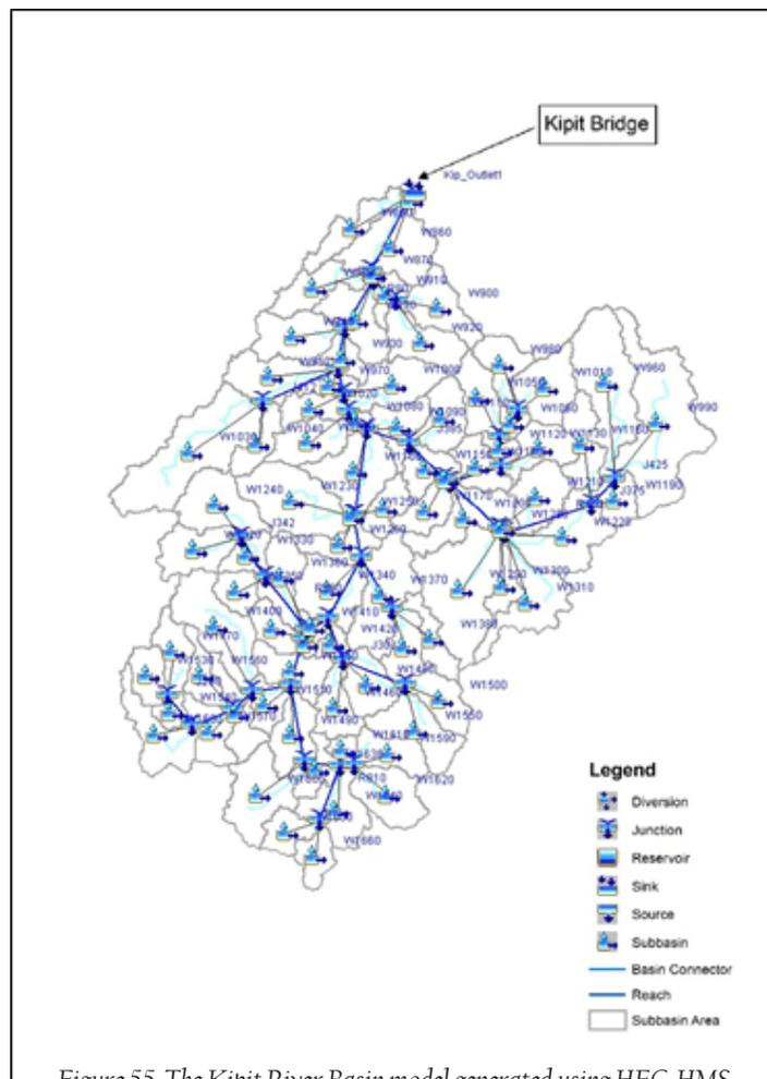
Figure 55. The Kipit River Basin model generated using HEC-HMS
