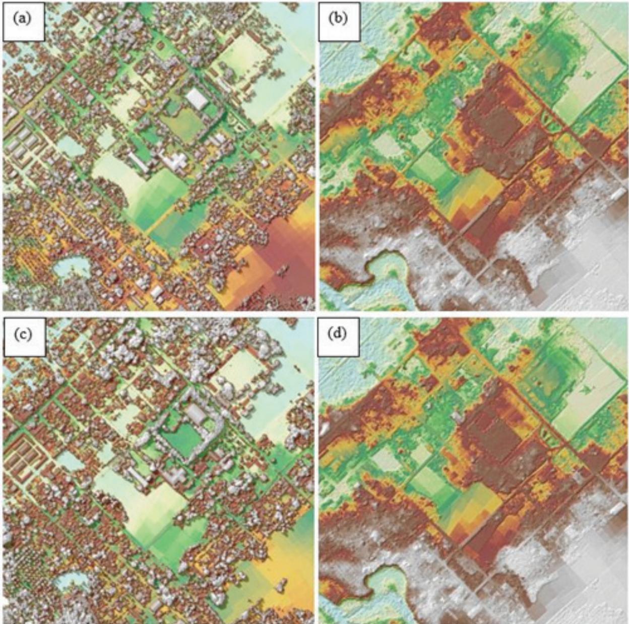
Figure 18. The Production of last return DSM (a) and DTM (b), first return DSM (c) and secondary DTM (d) in some portion of Kipit Floodplain
