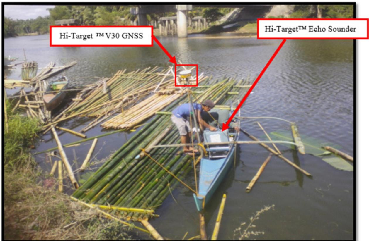
Figure 41. Bathymetric survey of ABSD at Kipit River using Hi-Target™ Echo Sounder (upstream)
