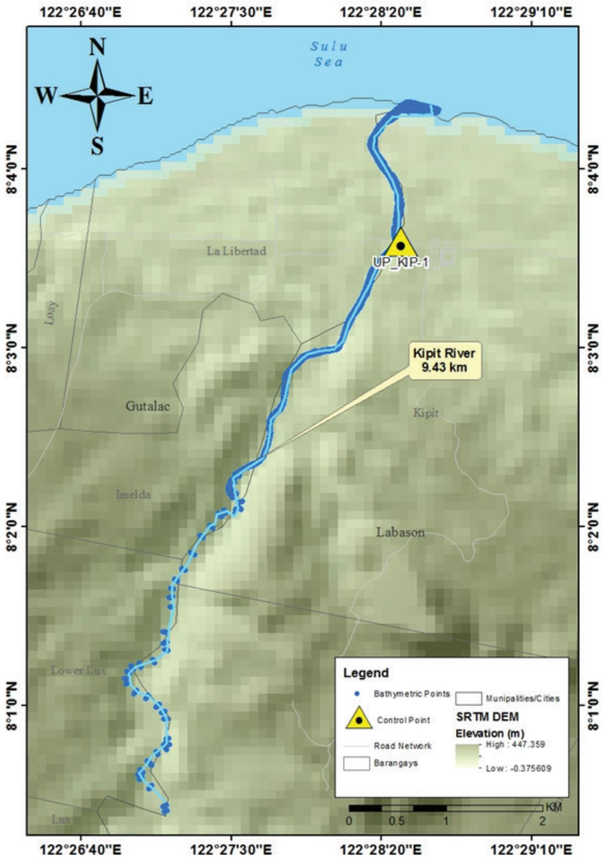
Figure 43. Bathymetric survey of Kipit River
