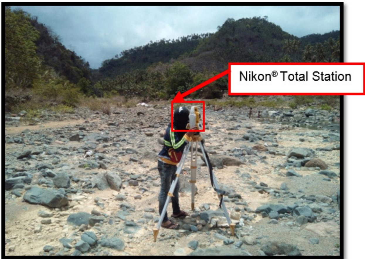
Figure 42. Cross-section survey at Kipit River using Nikon® Total Station
