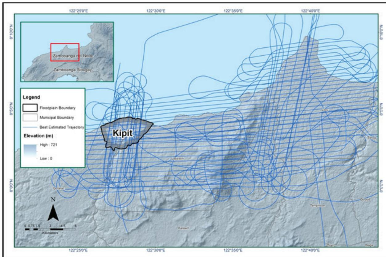
Figure 10. Best estimated trajectory of the LiDAR missions conducted over the Kipit Floodplain
