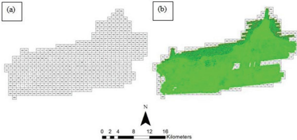
Figure 16. Tiles for Kipit Floodplain (a) and classification results (b) in TerraScan
