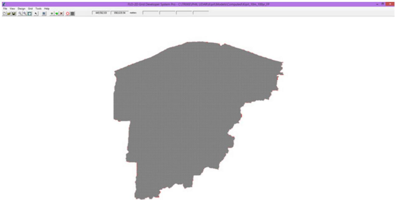
Figure 57. Screenshot of subcatchment with the computational area to be modeled in FLO-2D GDS Pro
