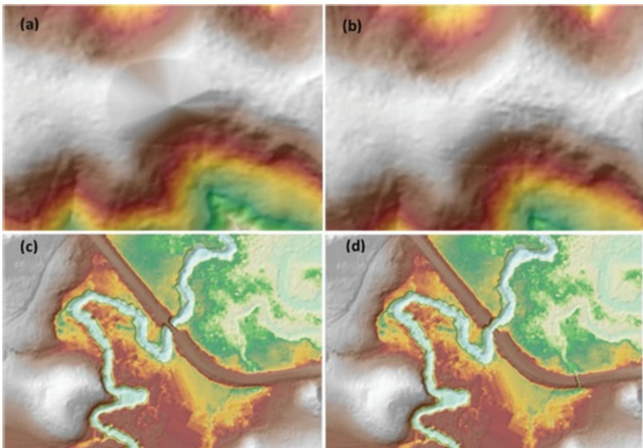
Figure 19. Portions in the DTM of Kipit Floodplain—a cut portion of the mountain before (a) and after (b) data retrieval; a bridge before (c) and after (d) manual editing
