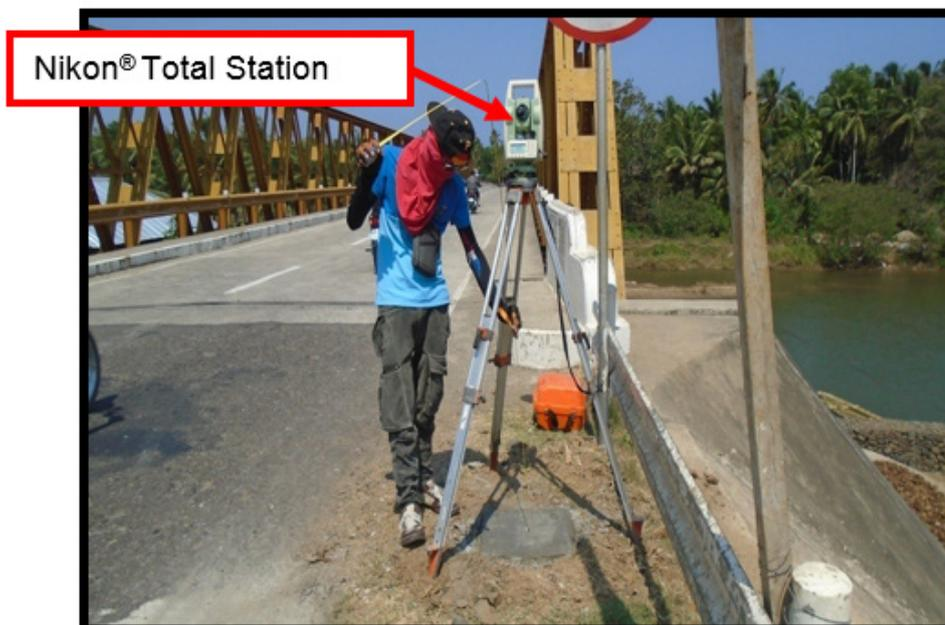
Figure 34. As-built survey of Kipit Bridge
