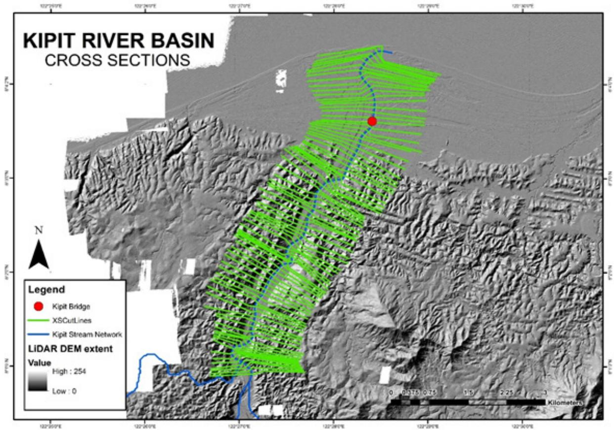
Figure 56. River cross-section of Kipit River generated through Arcmap HEC GeoRAS tool
