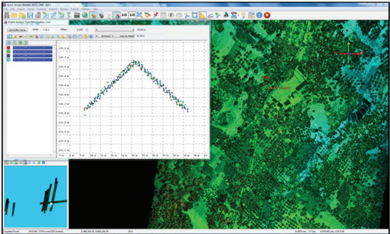
Figure 15. Quality checking for a Kipit flight 2189P using the Profile Tool of QTM Modeler
