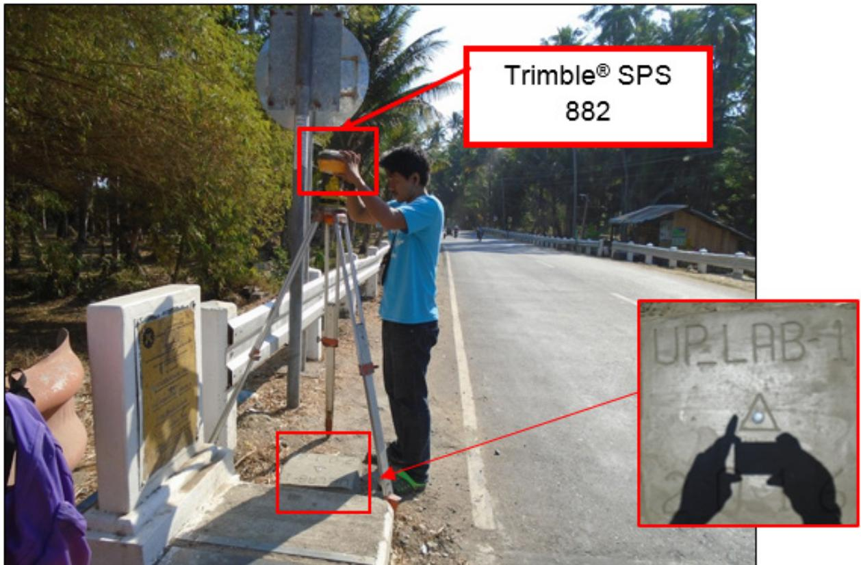
Figure 30. GNSS base set up, Trimble® SPS 882, at UP\_LAB-1 at Labason Bridge in Brgy. Antonio, Municipality of Labason, Province of Zamboanga del Norte
