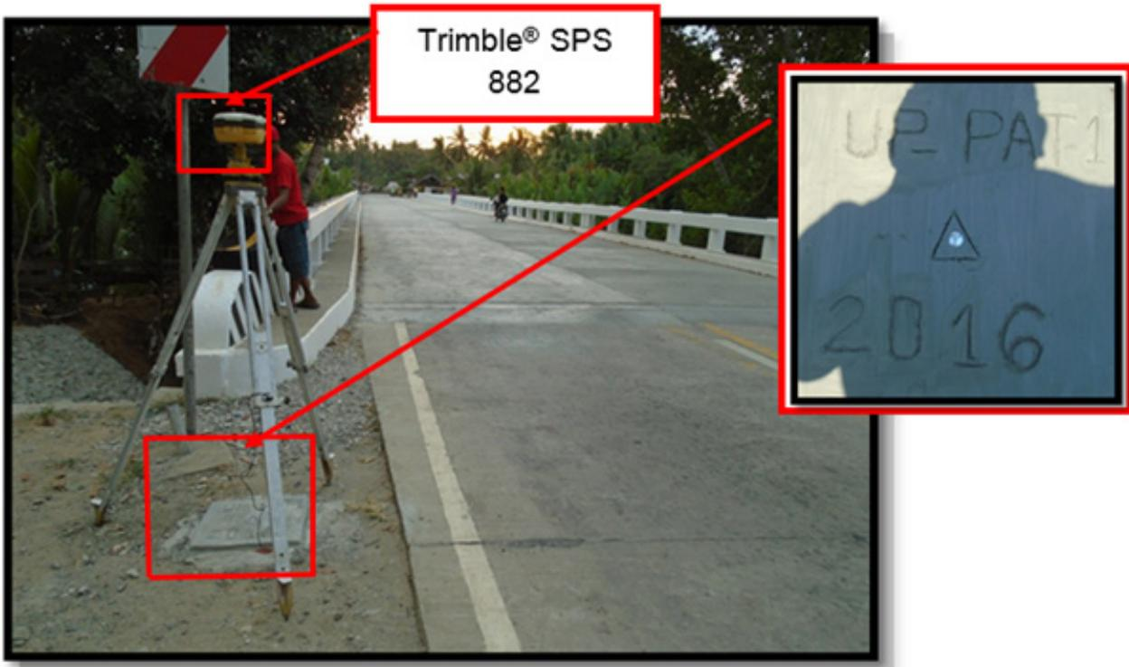
Figure 31. GNSS receiver set up, Trimble® SPS 882, UP\_PAT-1 at the side of Labason-Liloy Road near Patawag Bridge in Brgy. Patawag, Municipality of Labason, Province of Zamboanga del Norte
