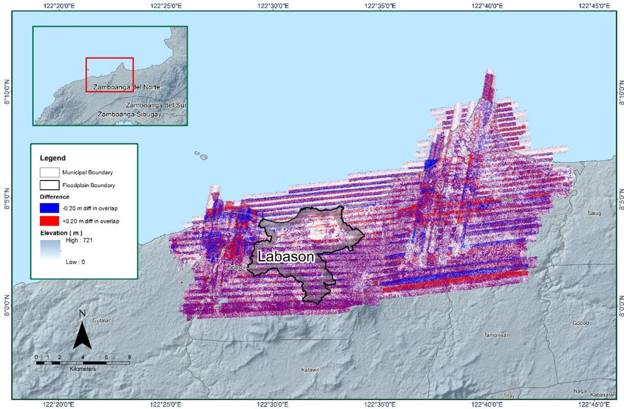
Figure 15. Elevation difference map between flight lines for Labason Floodplain.
