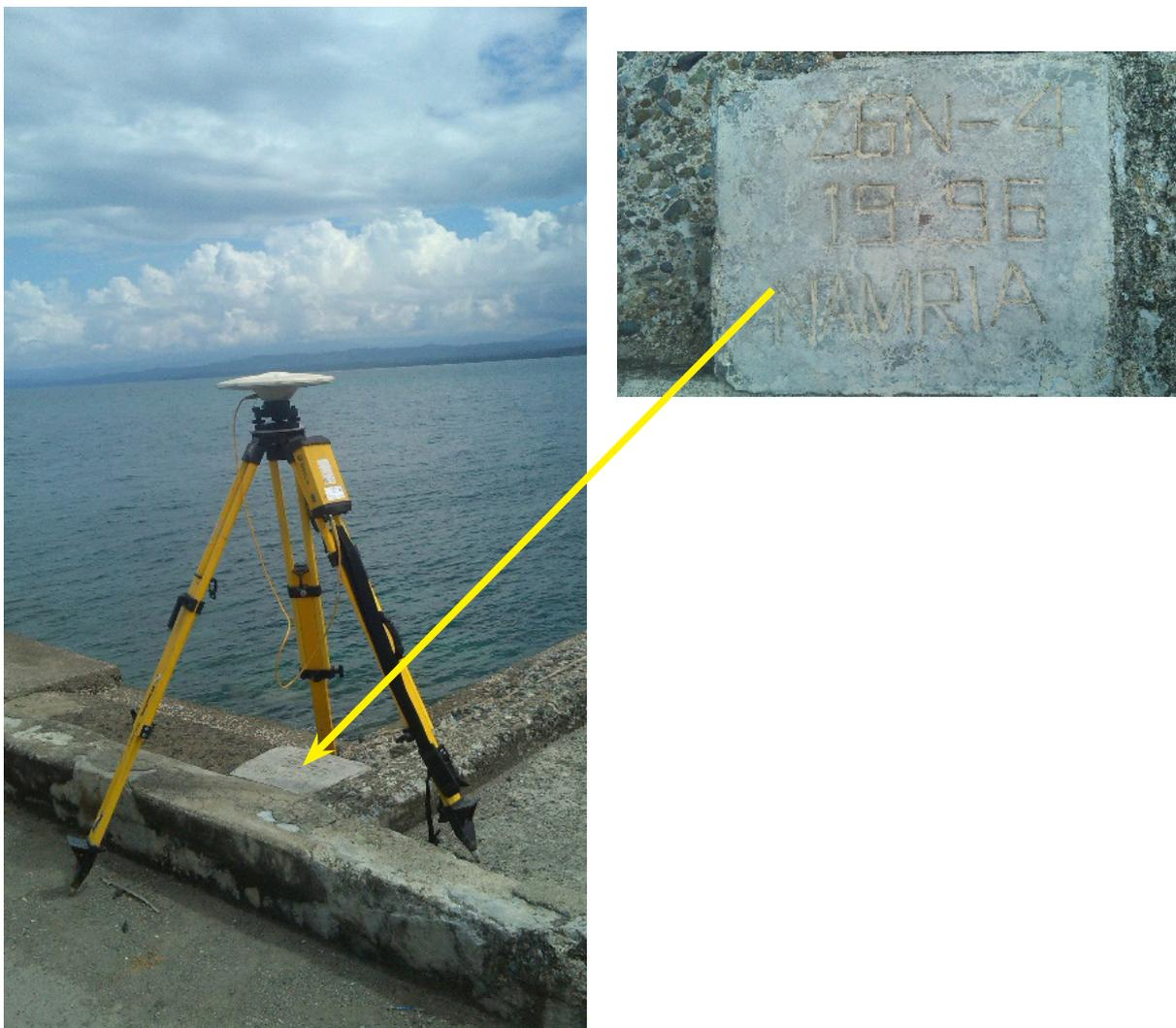
Figure 6. GPS set-up over ZGN-4 at Barangay Lamao, Lilo, Zamboanga del Norte (a) and NAMRIA reference point ZGN-4 (b) as recovered by the field team.
