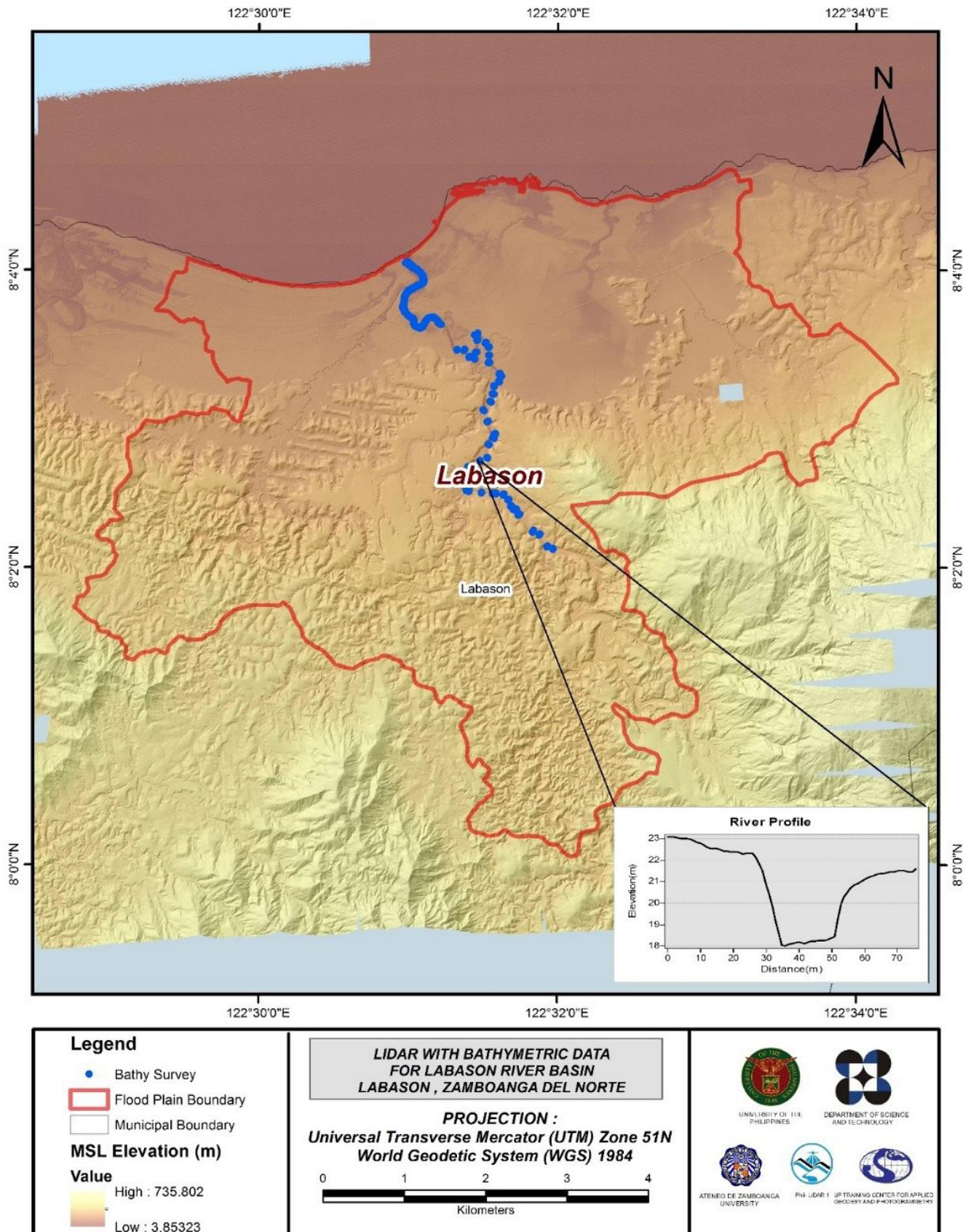
Figure 25. Map of Labason Floodplain with bathymetric survey points shown in blue.
