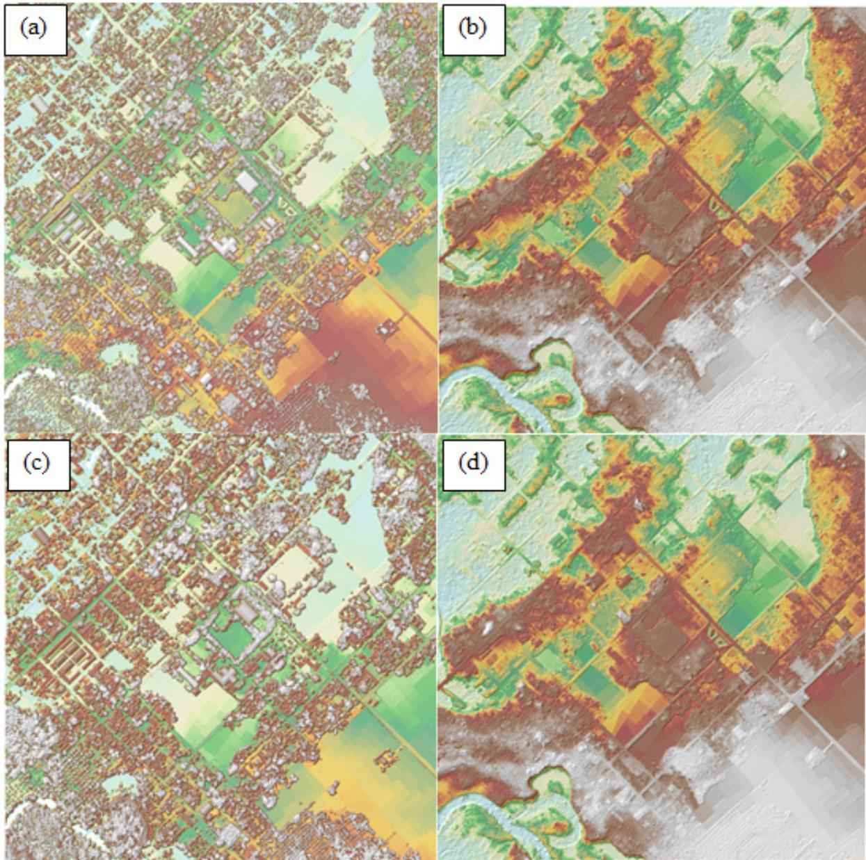
Figure 19. The production of last return DSM (a) and DTM (b), first return DSM (c) and secondary DTM (d) in some portion of Labason Floodplain.
