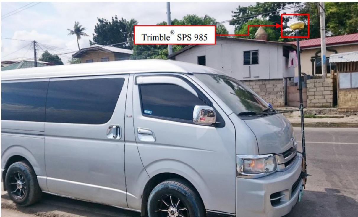
Figure 42. Validation points acquisition survey set-up for Labason River
