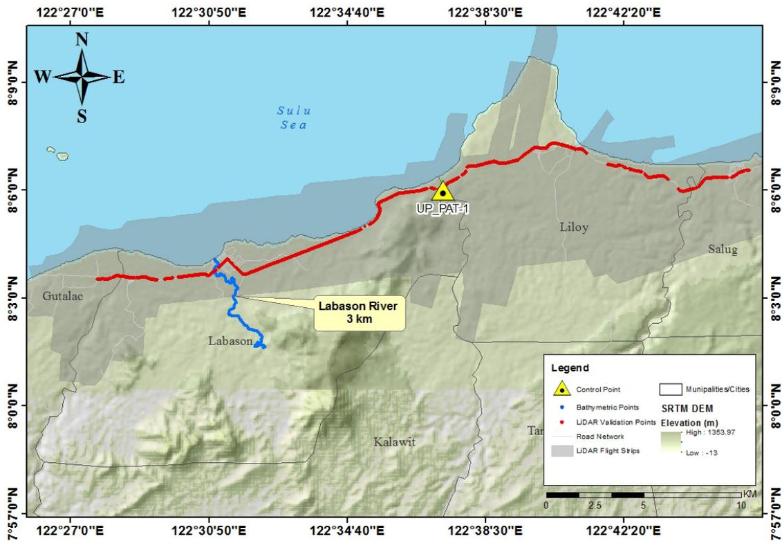
Figure 43. Validation points acquisition covering the Labason River Basin Area
