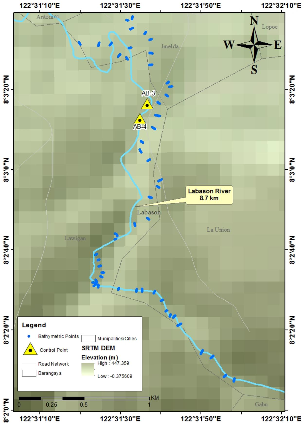
Figure 45. Bathymetric survey of Labason River
