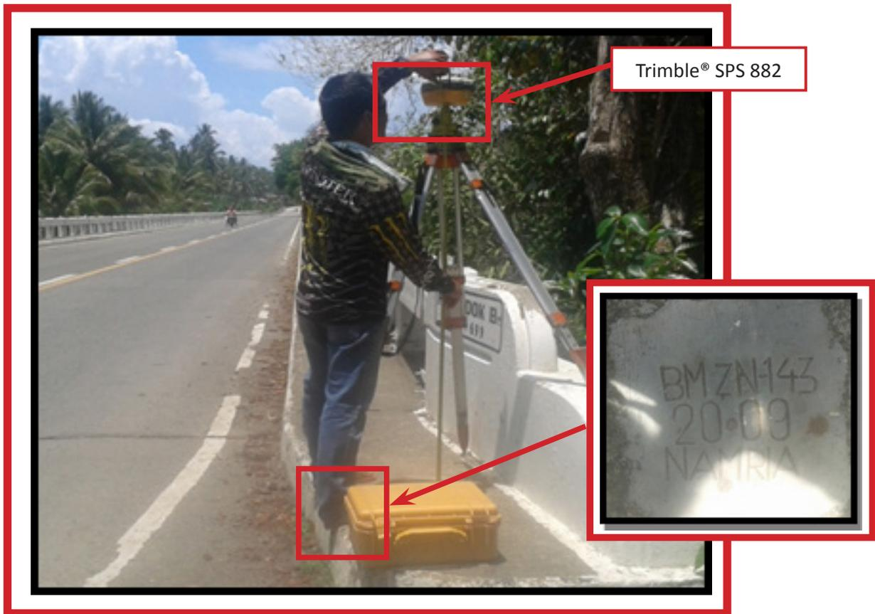
Figure 31. GNSS rover, Trimble® SPS 882, at ZN-143, an established control point, located at the right side walk going to Brgy. Rizon direction of Polandok Bridge in Brgy. Ramon Magsaysay, Salug, Province of Zamboanga del Norte
