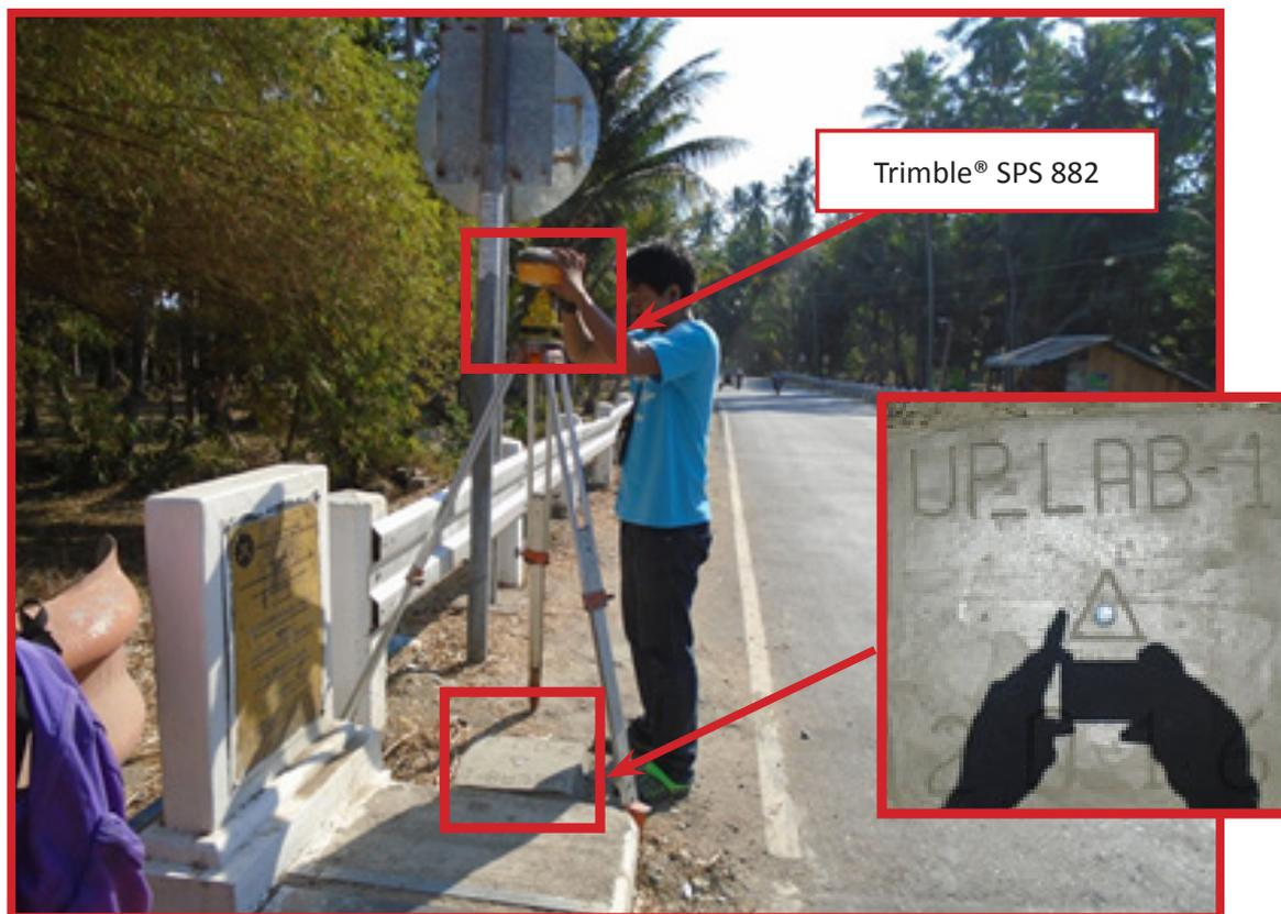
Figure 33. GNSS receiver set up, Trimble® SPS 882, at UP\_LAB-1 at Labason Bridge in Brgy. Antonio, Municipality of Labason, Province of Zamboanga del Norte
