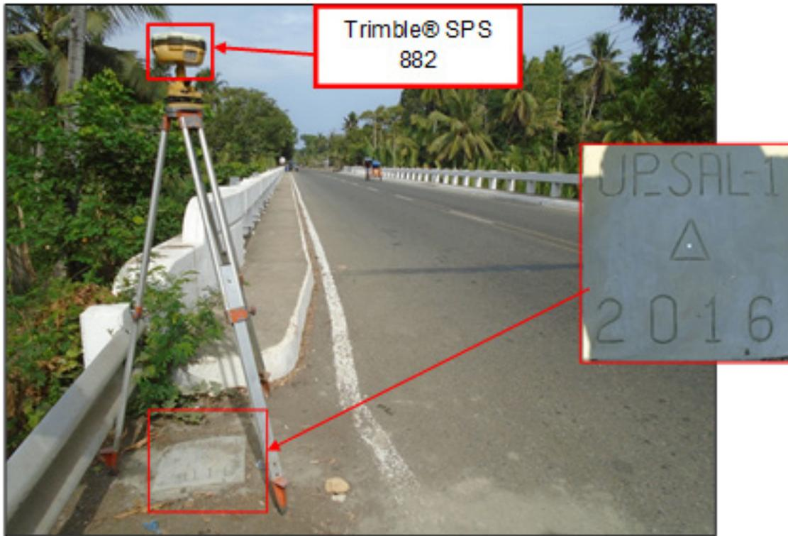
Figure 35. GNSS receiver set up, Trimble® SPS 882, UP\_SAL-1 located at the side of Ipil-Dipolog Highway near Salug Bridge in Brgy. La Libertad, Municipality of Gutalac, Province of Zamboanga del Norte
