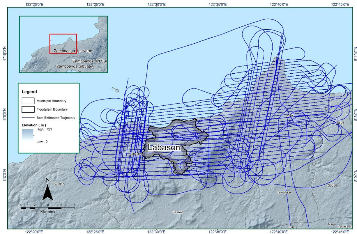
Figure 11. Best Estimated Trajectory of the LiDAR missions conducted over the Labason Floodplain.
