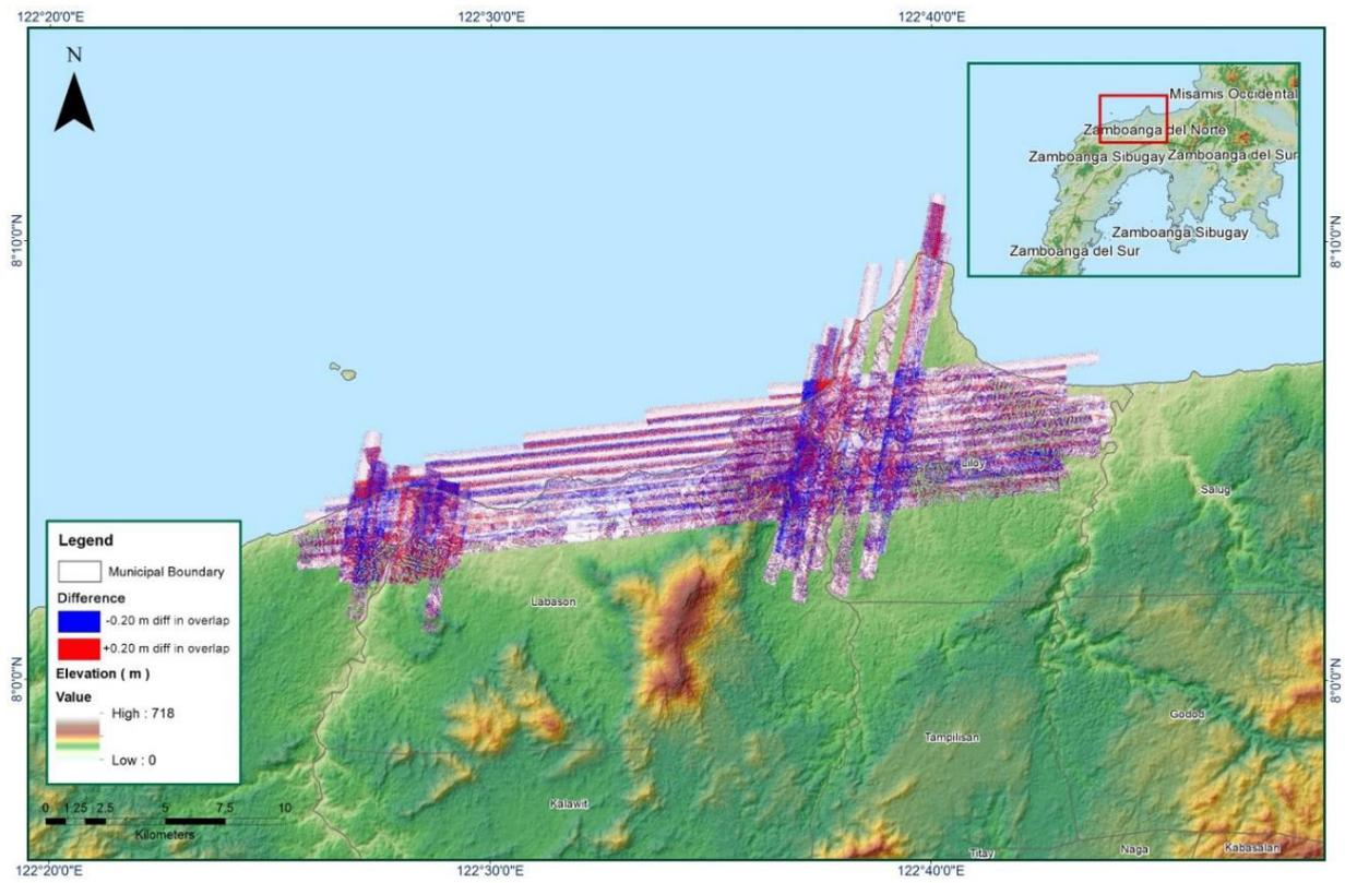
Figure A-8.7. Elevation difference between flight lines
