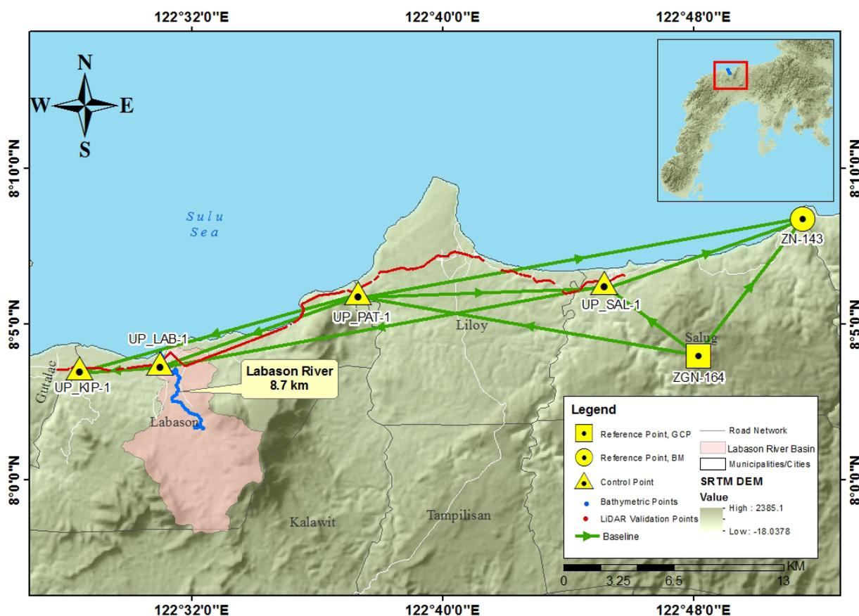
Figure 28. Extent of the bathymetric survey (in blue line) in Labason River and the LiDAR data validation survey (in red)
