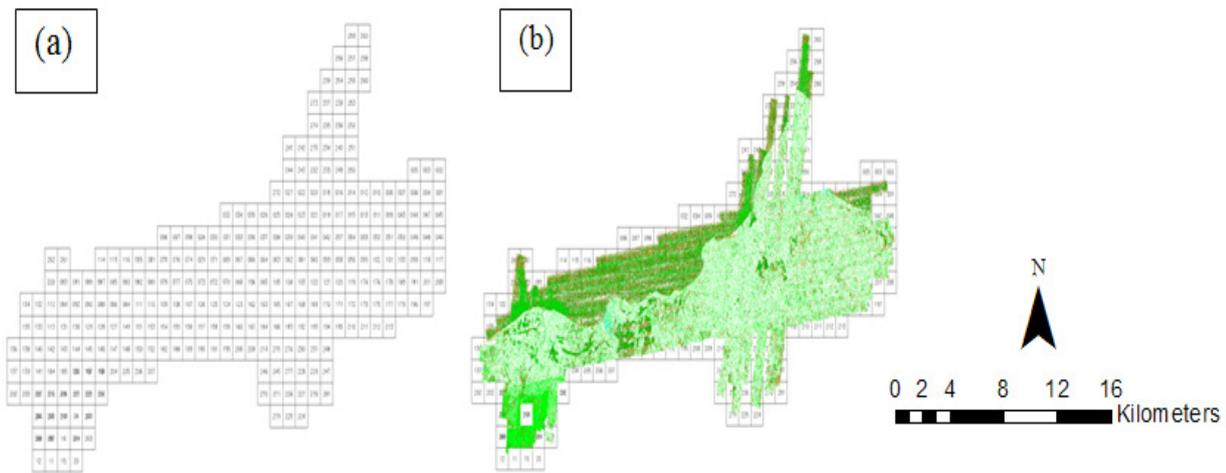
Figure 17. Tiles for Labason Floodplain (a) and classification results (b) in TerraScan.
