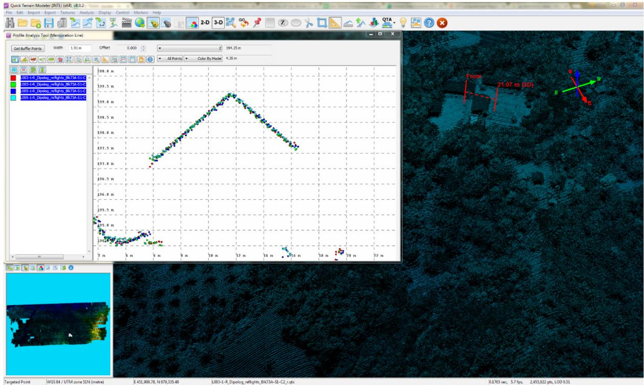
Figure 16. Quality checking for Labason flight 23582P using the Profile Tool of QT Modeler.
