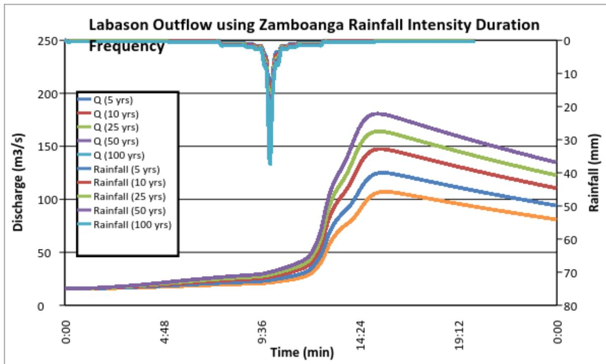
Figure 64. Outflow hydrograph at Brgy. La Union Station generated using Zamboanga City RIDF simulated in HEC-HMS
