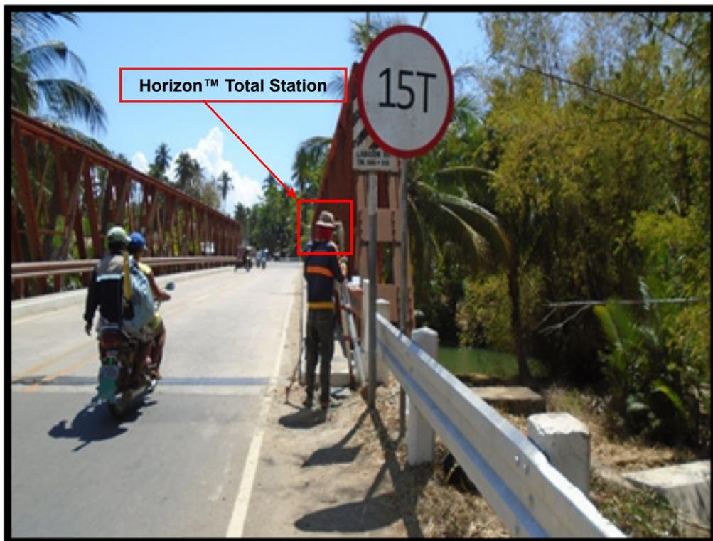
Figure 37. As-built survey of Labason Bridge
