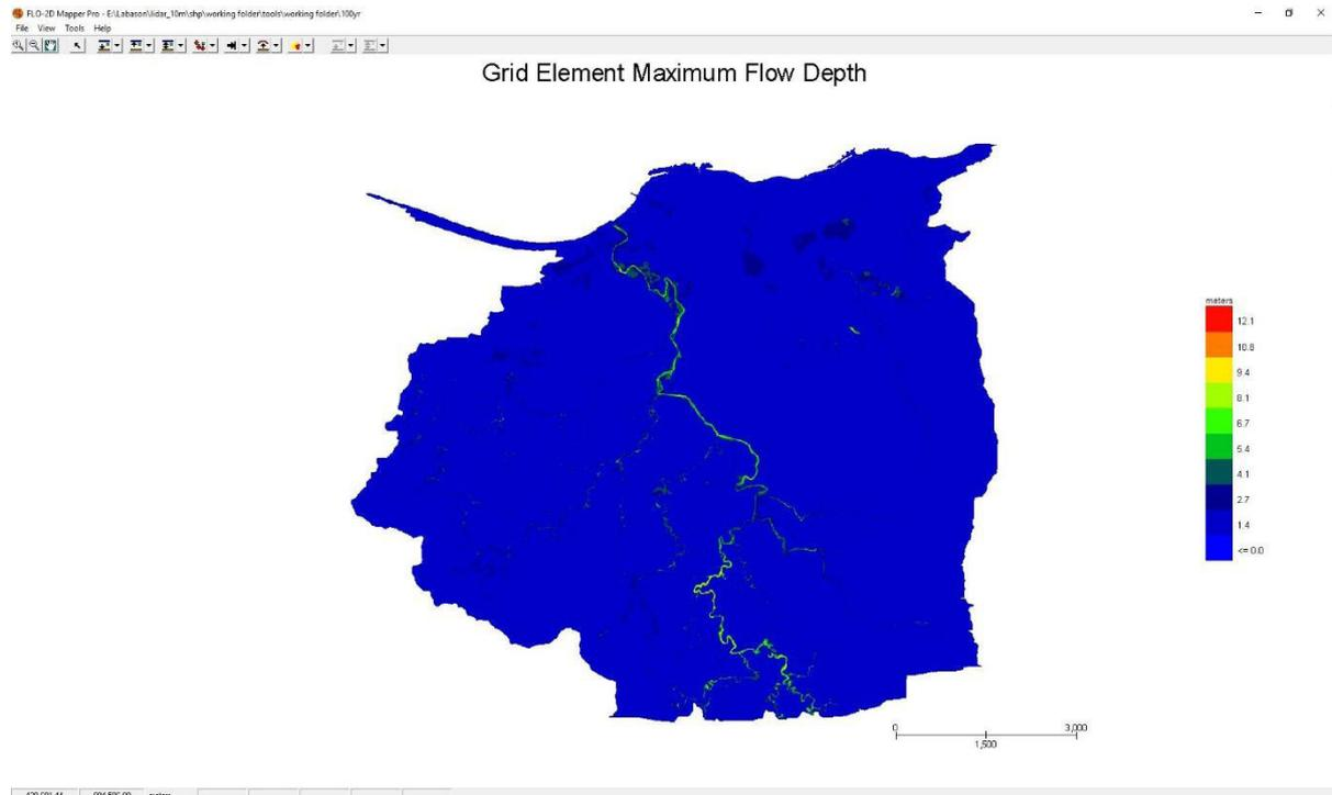
Figure 62. Generated 100-year rain return flow depth map from FLO-2D Mapper
