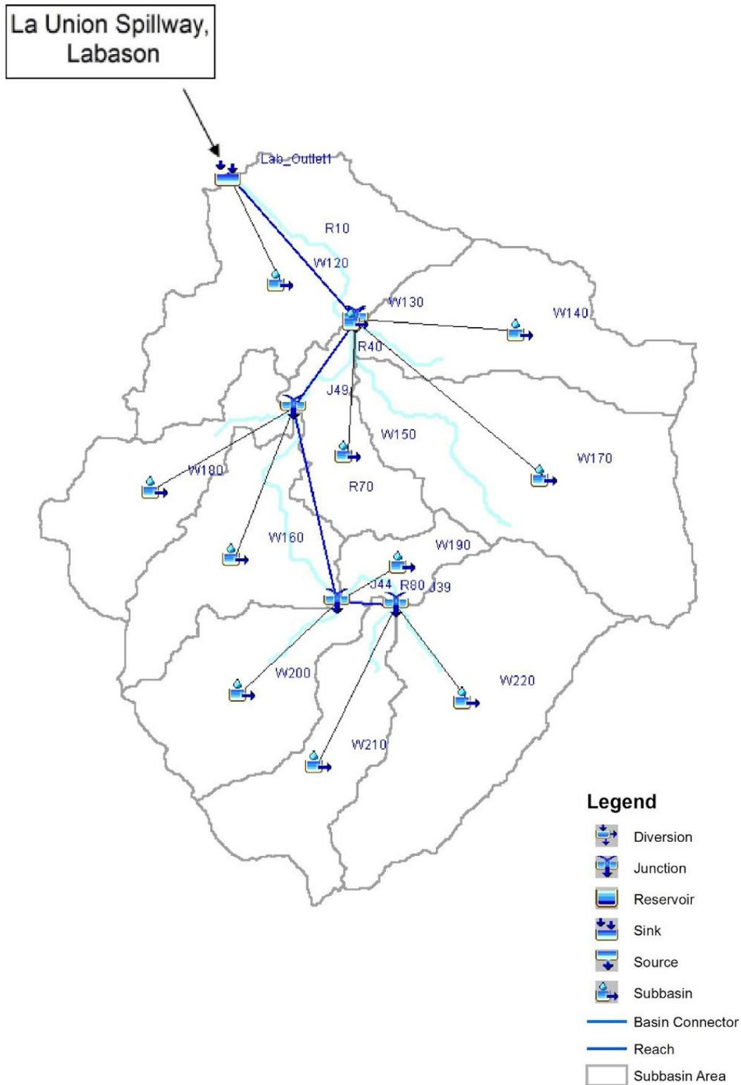
Figure 58. The Labason river basin model generated using HEC-HMS
