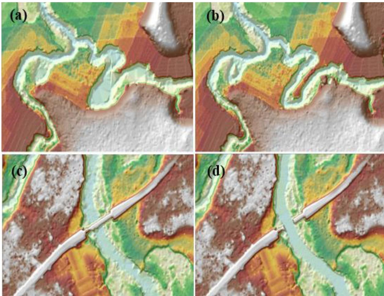
Figure 20. Portions in the DTM of Labason Floodplain – a cut portion of the mountain before (a) and after (b) data retrieval; a bridge before (c) and after (d) manual editing.
