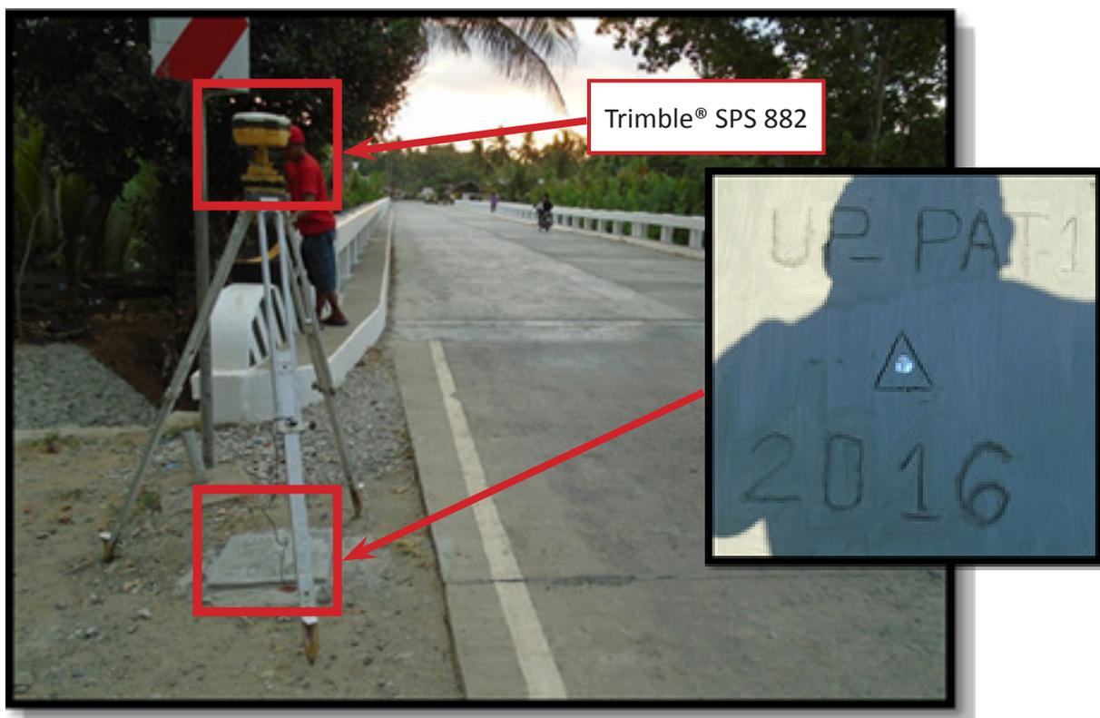
Figure 34. GNSS receiver set up, Trimble® SPS 882, UP\_PAT-1 at the side of Labason-Liloy Road near Patawag Bridge in Brgy. Patawag, Municipality of Labason, Province of Zamboanga del Norte
