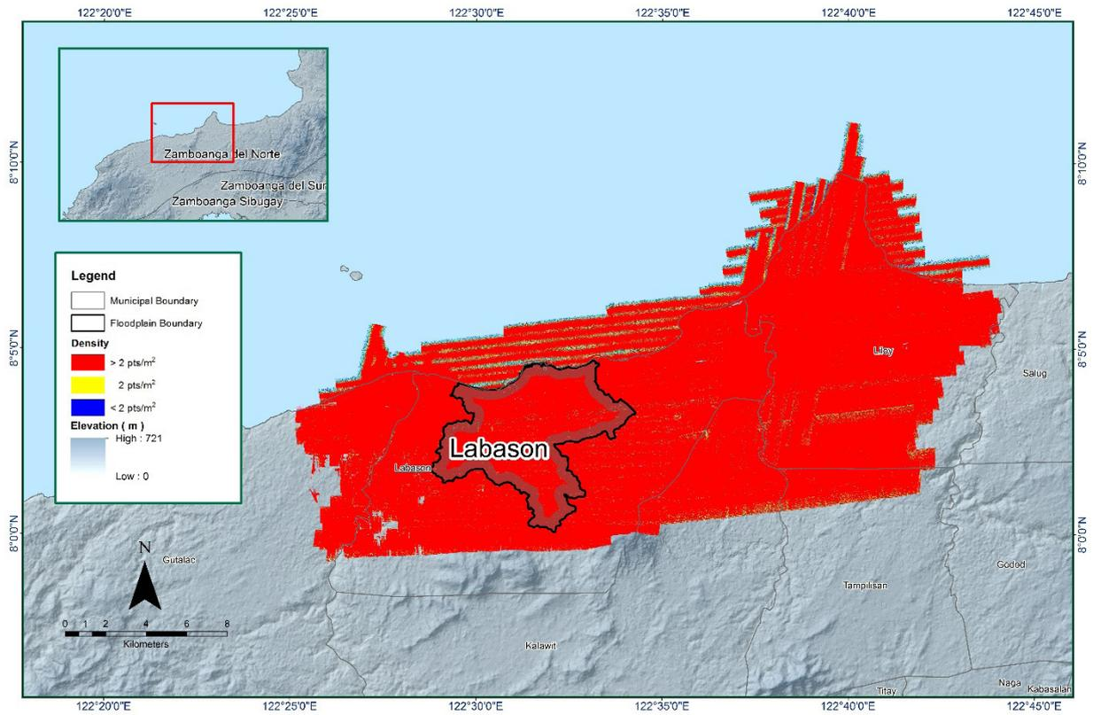
Figure 14. Pulse density map of merged LiDAR data for Labason Floodplain.
