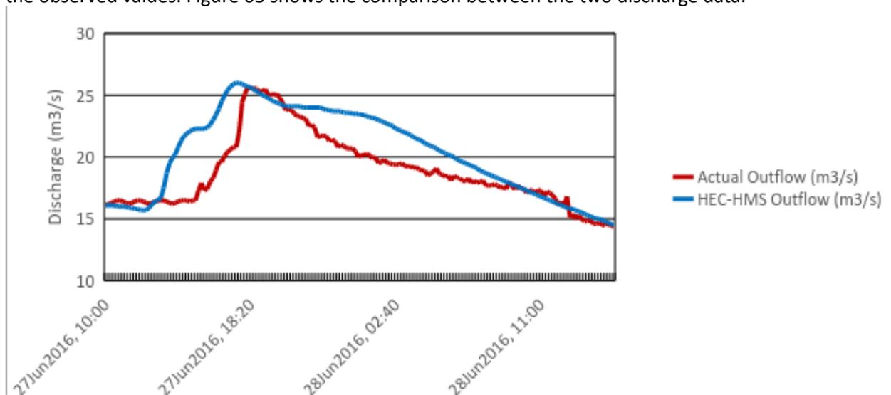
Figure 63. Outflow Hydrograph of Labason produced by the HEC-HMS model compared with observed outflow
