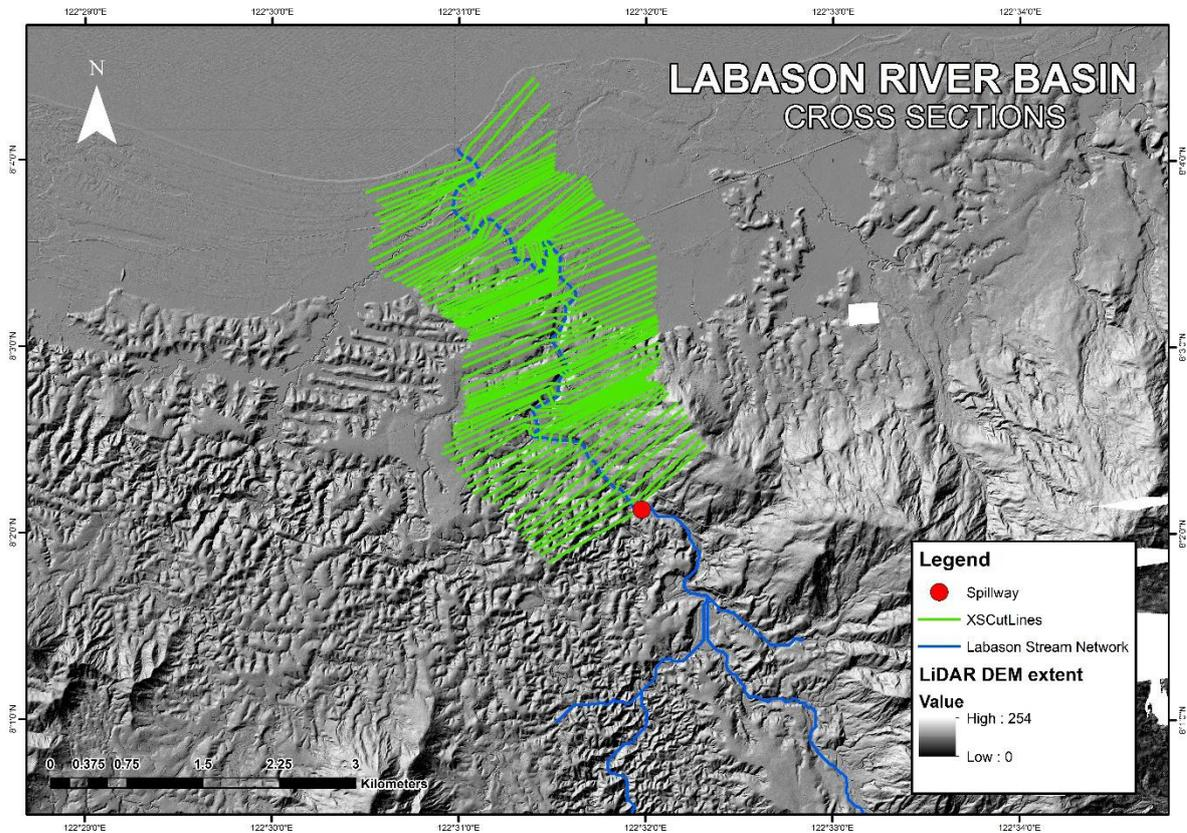
Figure 59. River cross-section of Labason River generated through Arcmap HEC GeoRAS tool
