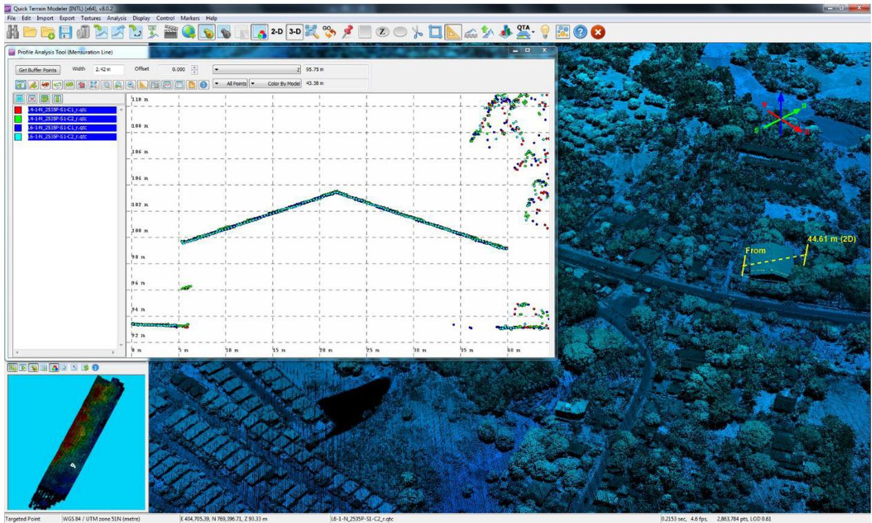
Figure 18. Quality checking for a Mercedes flight 2535P using the Profile Tool of QT Modeler
