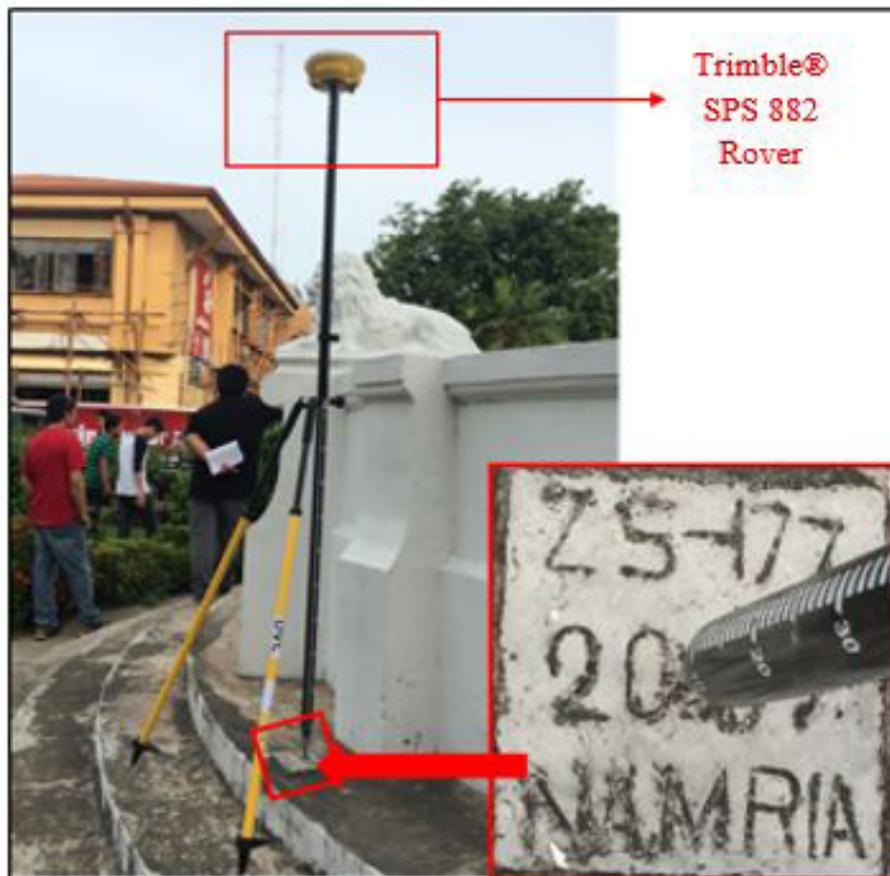
Figure 35. GNSS receiver setup, Trimble® SPS 882 at ZS-177, located in Rizal Park in Brgy. Zone IV, Zamboanga City, Zamboanga Del Sur
