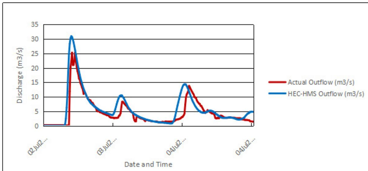
Figure 63. Outflow Hydrograph of Mercedes produced by the HEC-HMS model compared with observed outflow
