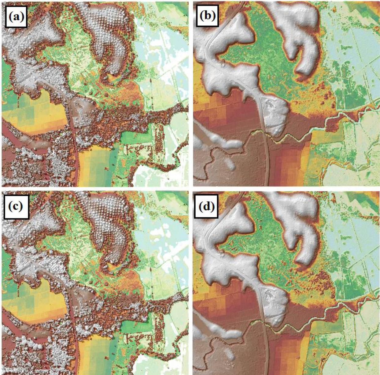
Figure 21. The production of last return DSM (a) and DTM (b), first return DSM (c) and secondary DTM (d) in some portion of Mercedes Floodplain
