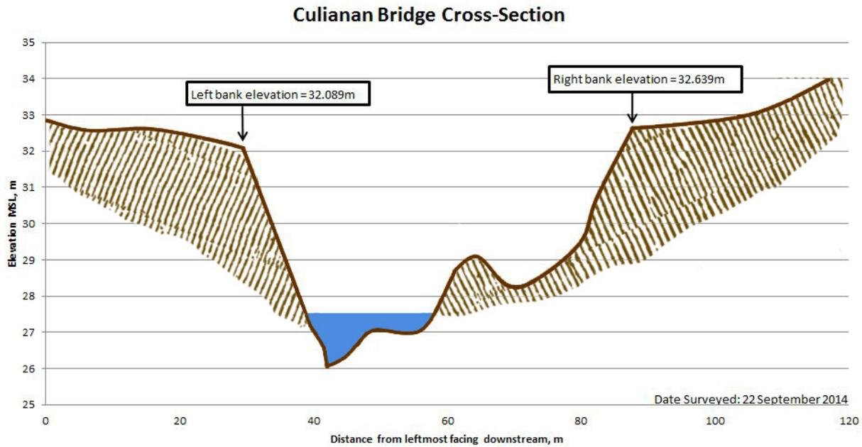
Figure 50. Cross-Section Plot of Culianan Bridge
