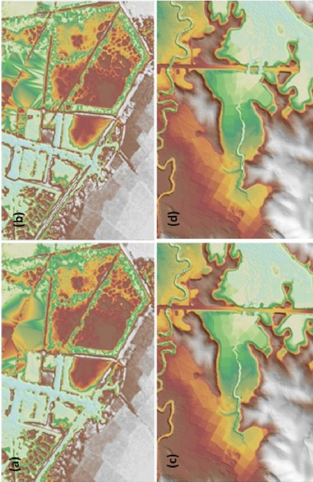
Figure 24. Portions in the DTM of Mercedes Floodplain - a paddy field before (a) and after (b) data retrieval; a bridge before (c) and after (d) manual editing.
