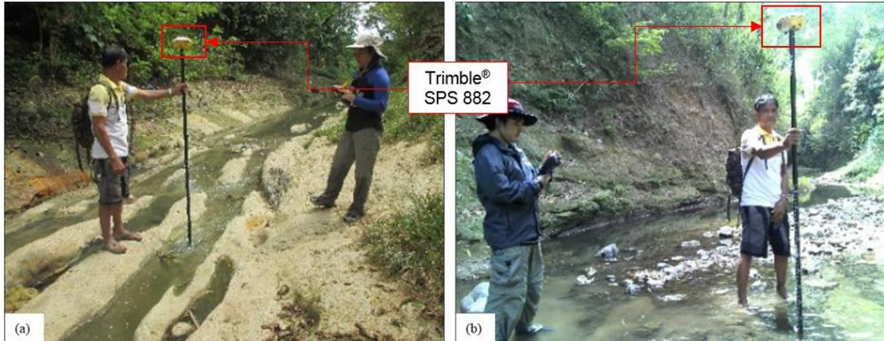
Figure 46. Bathymetric survey in Culianan River: (a) upstream and (b) downstream
