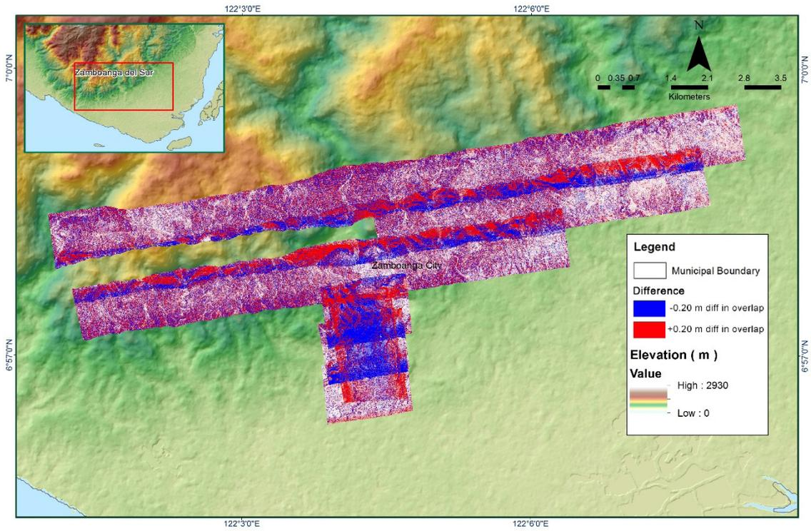
Figure A-8.21 Elevation difference between flight lines
