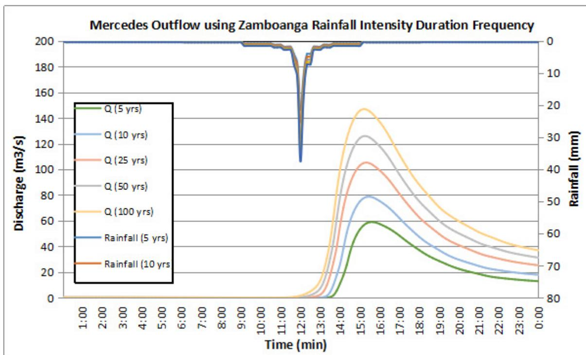
Figure 64. Outflow hydrograph at Mercedes Station generated using Zamboanga City RIDF simulated in HEC-HMS
