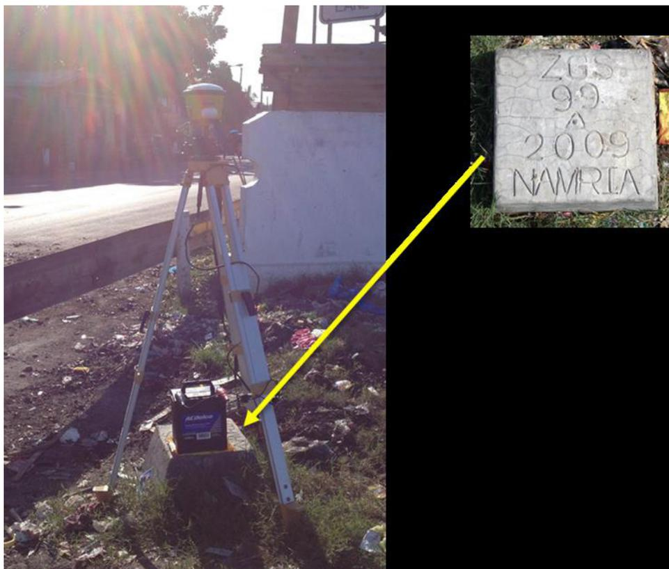
Figure 6. GPS set-up over ZGS-99 beside the seawall in Calarian, Zamboanga City (a) and NAMRIA reference point ZGS-99 (b) as recovered by the field team
