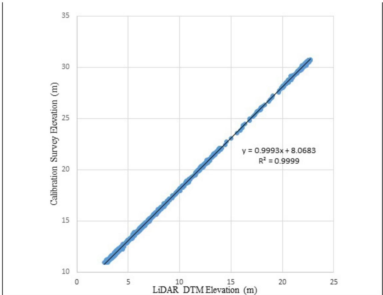
Figure 27. Correlation plot between calibration survey points and LiDAR data
