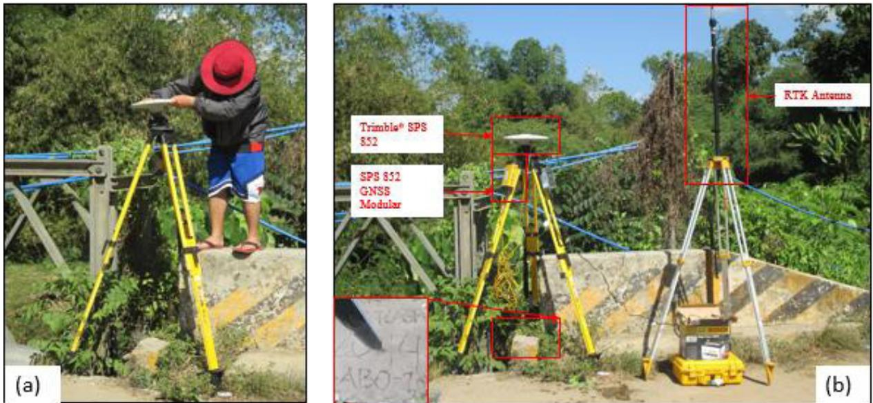
Figure 36. GNSS receiver occupation, Trimble® SPS 852 at ABO-1 located along approach of Abong Bridge, in Brgy. Dulian, Zamboanga City, Zamboanga Del Sur
