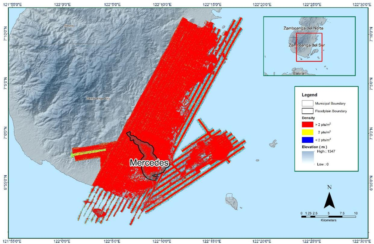
Figure 16. Pulse density map of merged LiDAR data for Mercedes Floodplain
