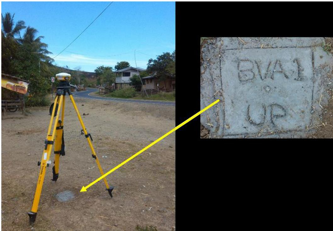
Figure 8. GPS set-up over BVA-1 established in Brgy. Buenavista, Zamboanga City and (a) and Reference point BVA-1 (b) as established by the field team
