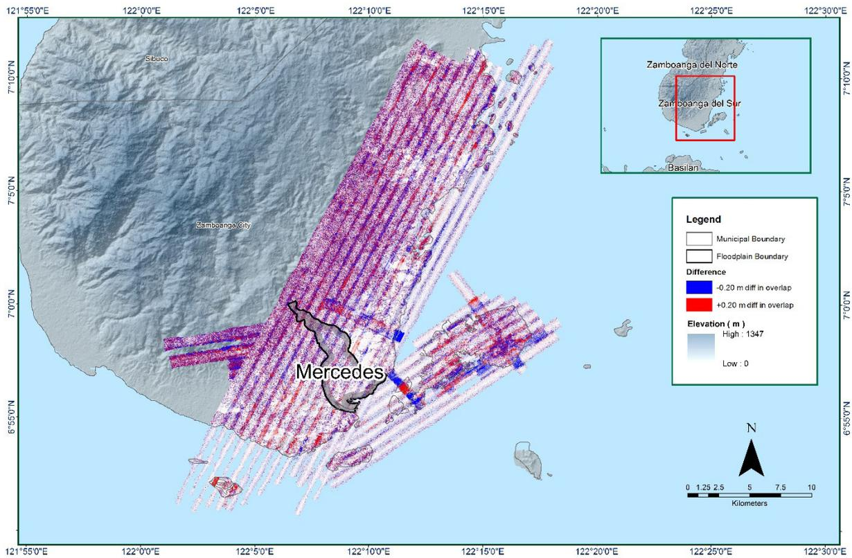
Figure 17. Elevation difference map between flight lines for Mercedes Floodplain
