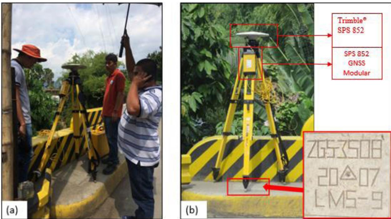
Figure 38. GNSS base receiver setup, Trimble® SPS 852 at ZGS-3508 along Tumaga Bridge in Brgy. Tumaga, Zamboanga City, Zamboanga Del Sur
