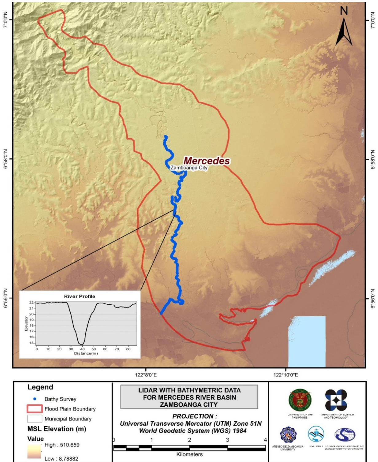
Figure 29. Map of Mercedes Floodplain with bathymetric survey points shown in blue
