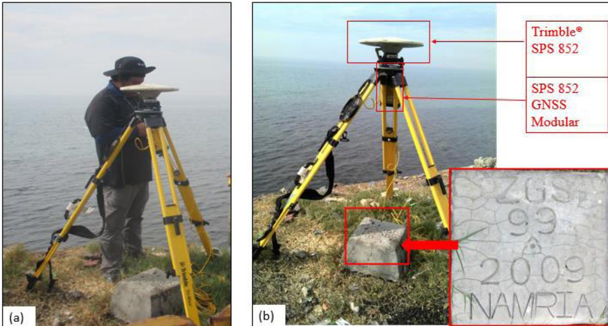
Figure 34. GNSS base receiver setup, Trimble® SPS 852 at ZGS-99 in Brgy. Sinunoc, Zamboanga City, Zamboanga Del Sur
