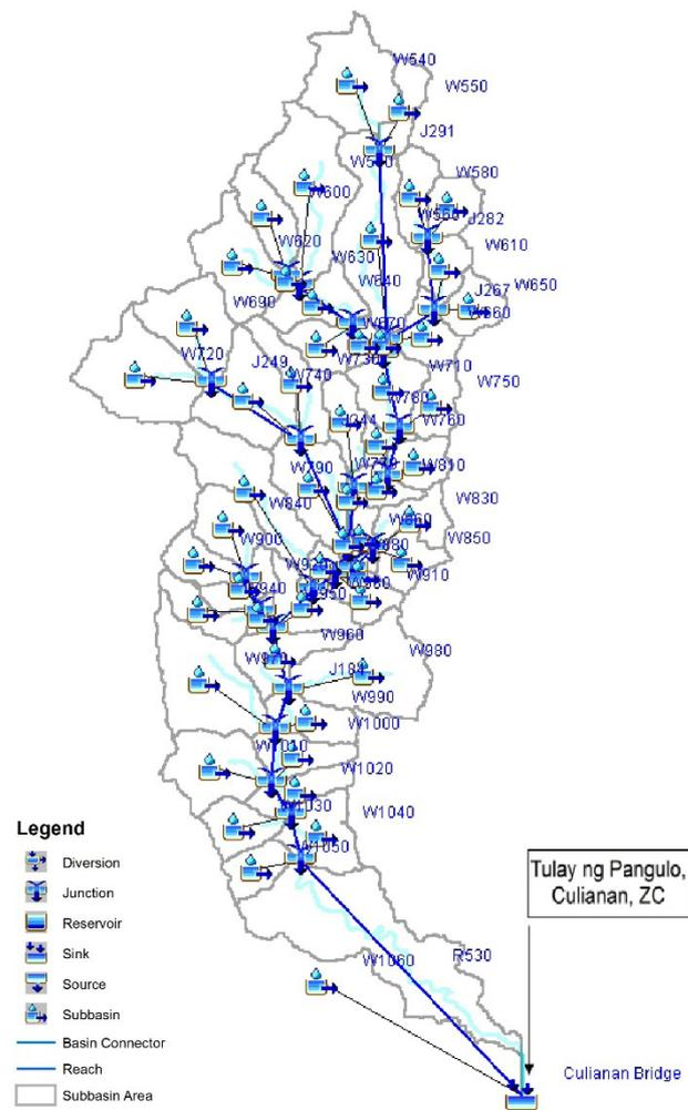
Figure 58. The Mercedes river basin model generated using HEC-HMS
