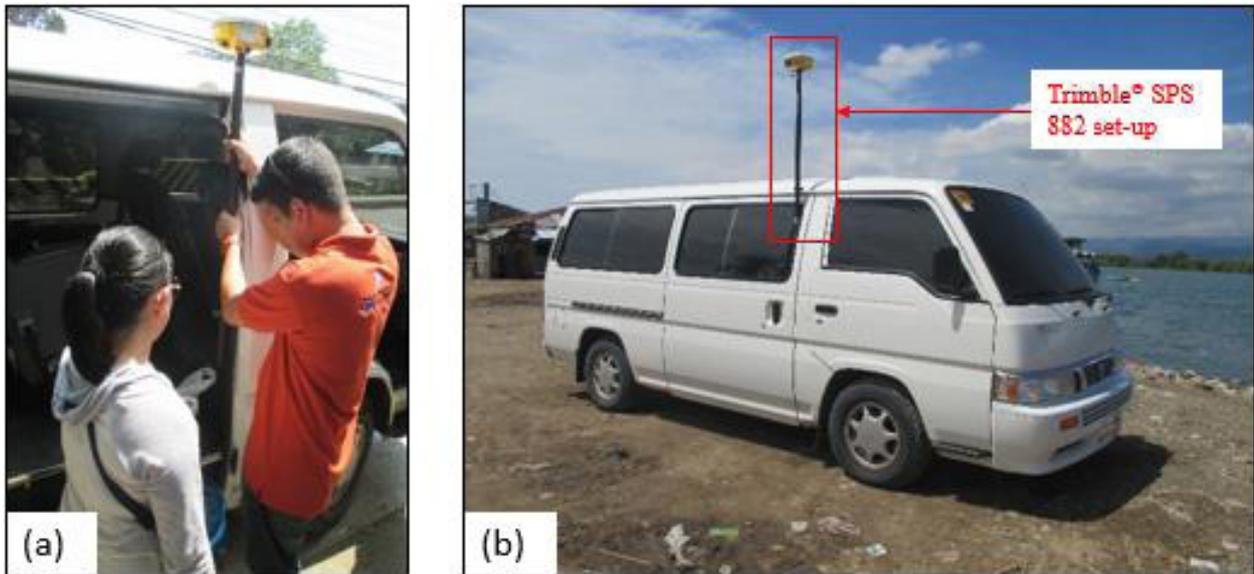
Figure 44. (a) Ground validation set-up by: Trimble® SPS 882 mounted on a pole attached on the side of the vehicle
