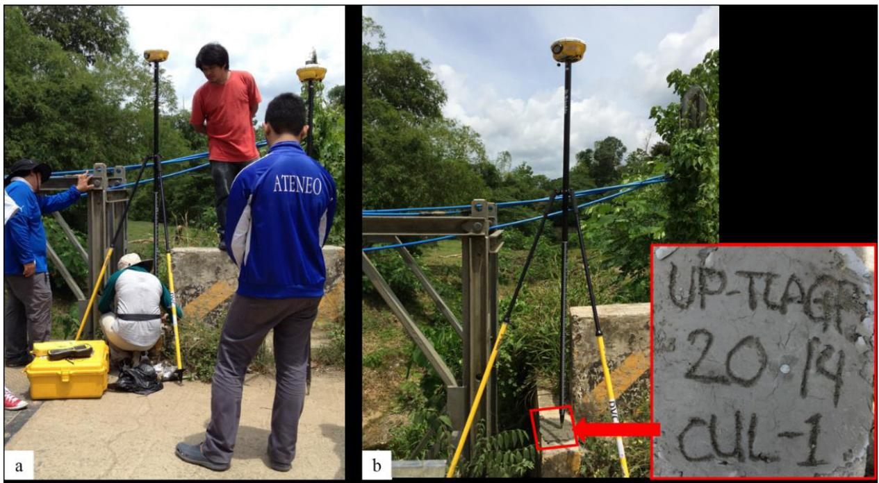
Figure 37. GNSS base receiver setup, Trimble® SPS 882 at CUL-1 along approach of Culianan Bridge in Brgy. Culianan, Zamboanga City, Zamboanga Del Sur
