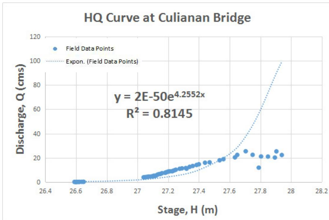
Figure 51. Hydrometry rating curve of Culianan Bridge
