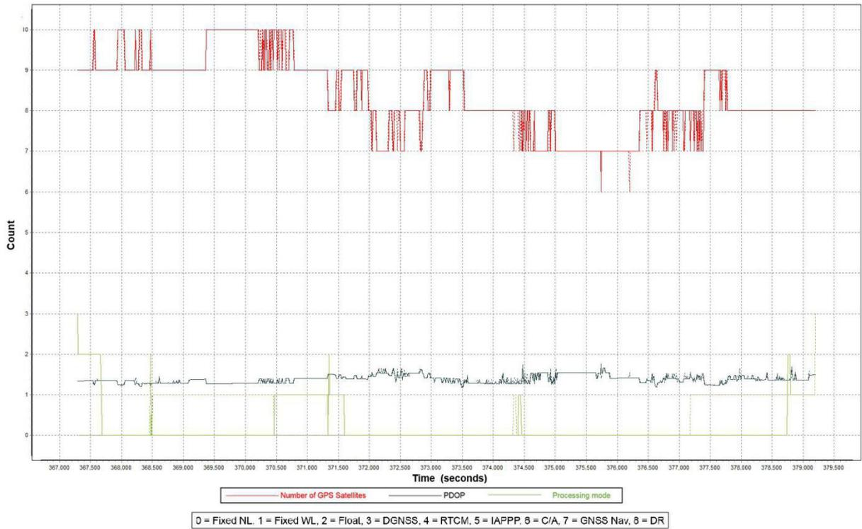
Figure 12. Solution Status Parameters of Mercedes Flight 2535P
