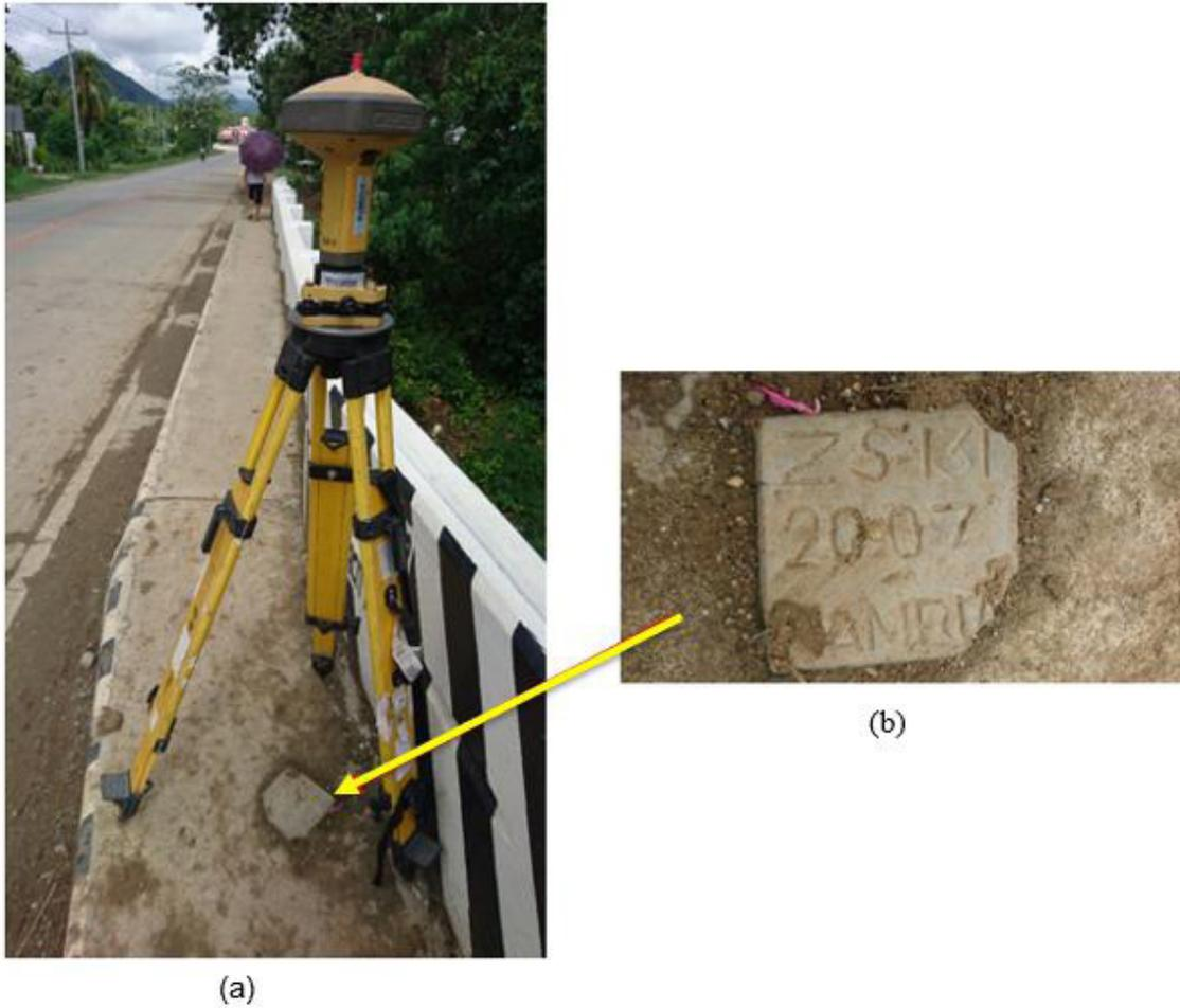
Figure 7. GPS set-up over ZS-131 in Curuan, Zamboanga City (a) and NAMRIA reference point ZS-131 (b) as recovered by the field team
