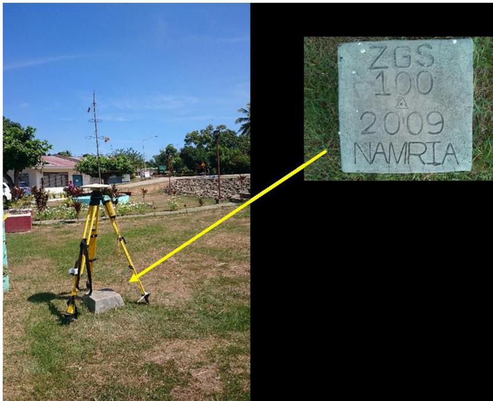
Figure 5. GPS set-up over ZGS-100 in Brgy. Manicahan, Zamboanga del Sur (a) and NAMRIA reference point ZGS-100 (b) as recovered by the field team.
