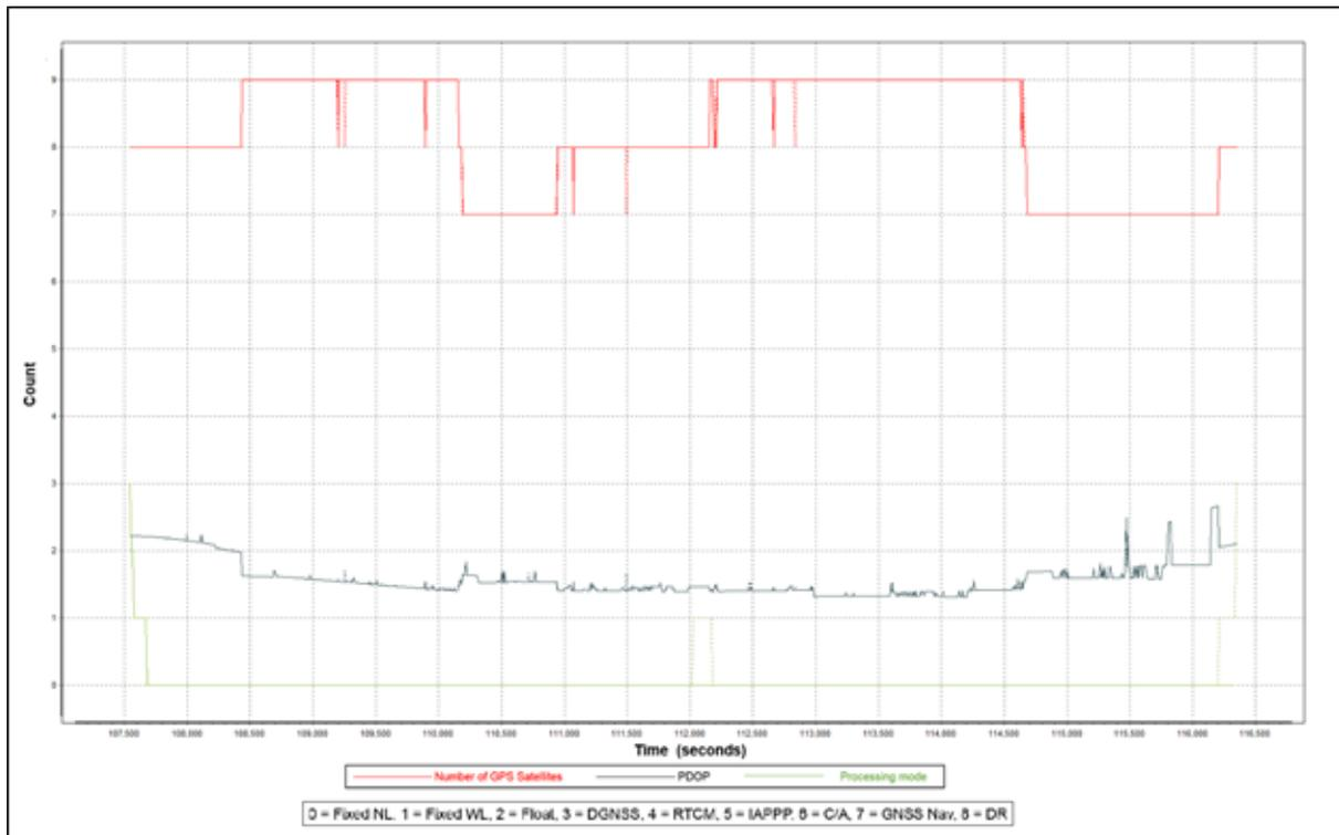
Figure 9. Solution Status Parameters of Patawag Flight 23590P.
