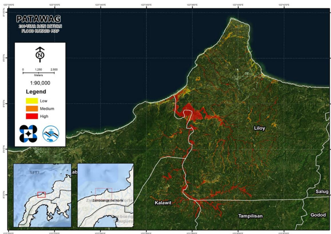
Figure 65. 100-year Flood Hazard Map for Patawag Floodplain
