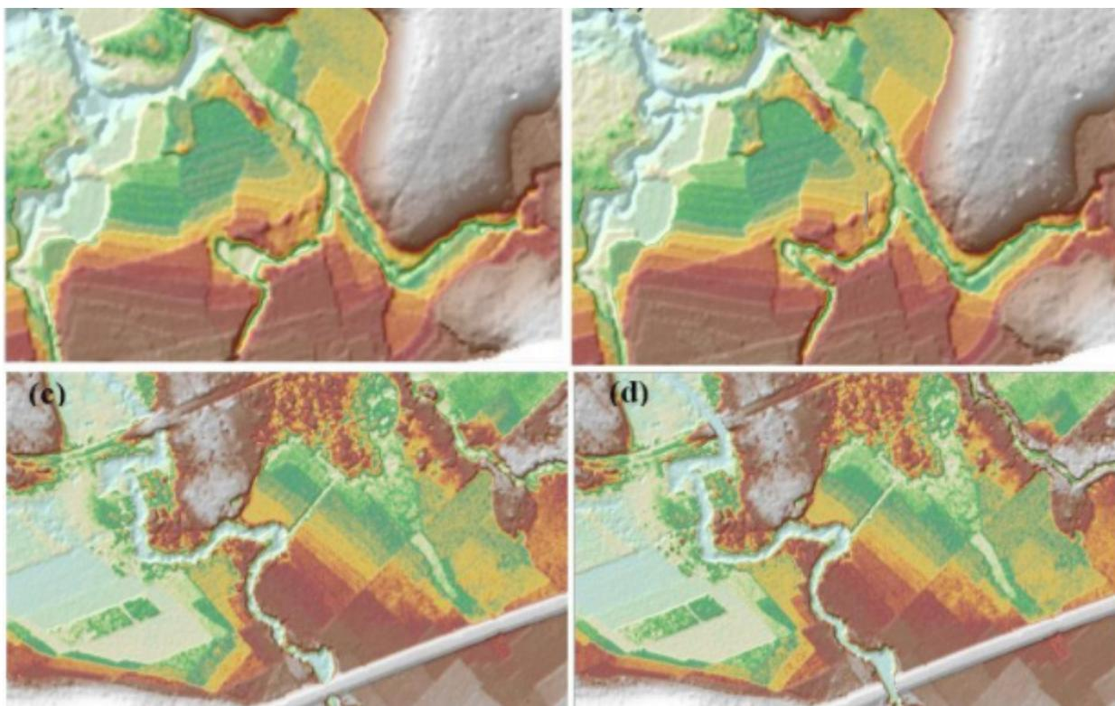
Figure 19. Portions in the DTM of Patawag Floodplain– a cut portion of the mountain before (a) and after (b) data retrieval; a bridge before (c) and after (d) manual editing.
