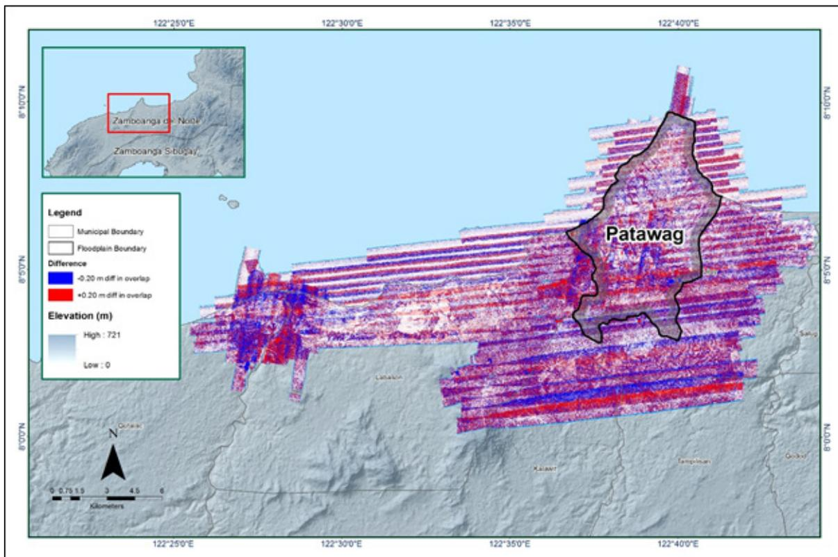
Figure 14. Elevation difference map between flight lines for Patawag floodplain.
