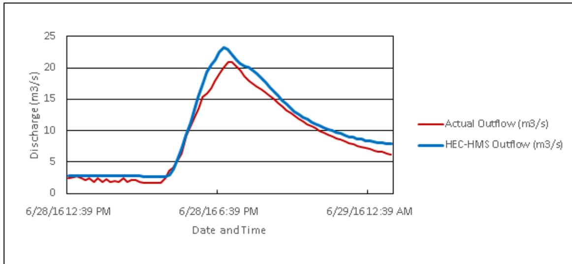
Figure 62. Outflow Hydrograph of Patawag produced by the HEC-HMS model compared with observed outflow
