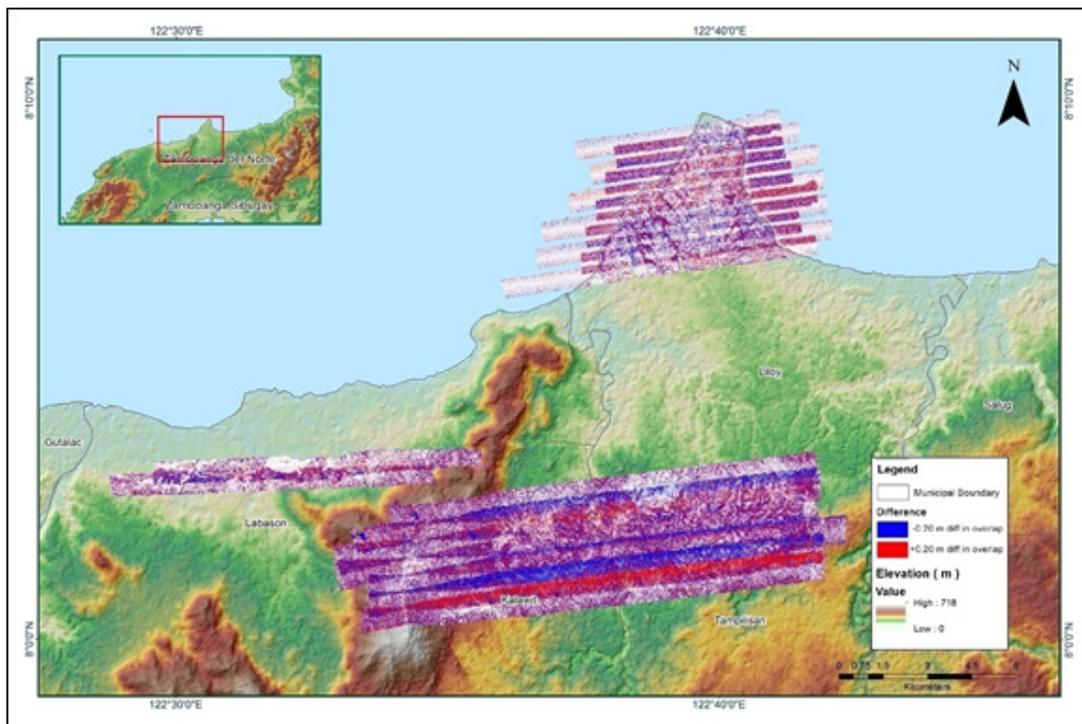
Figure A-8.14. Elevation difference between flight lines
