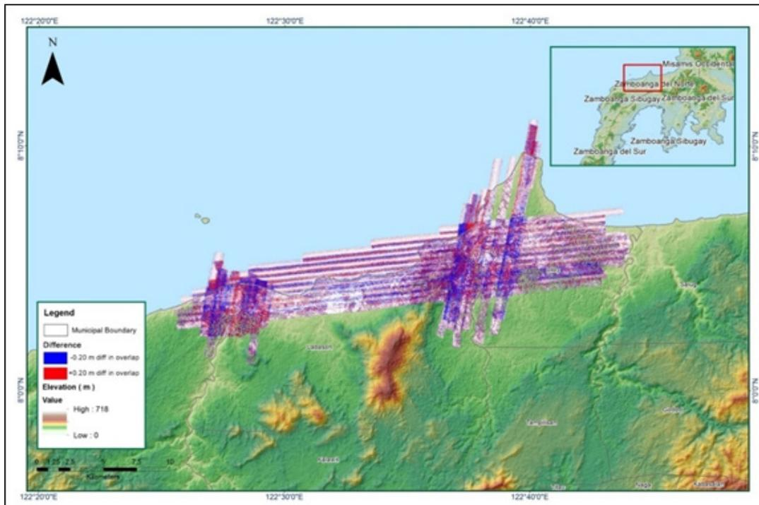
Figure A-8.7. Elevation difference between flight lines
