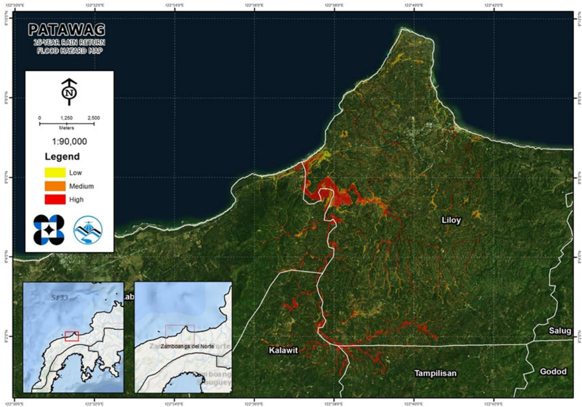
Figure 67. 25-year Flood Hazard Map for Patawag Floodplain
