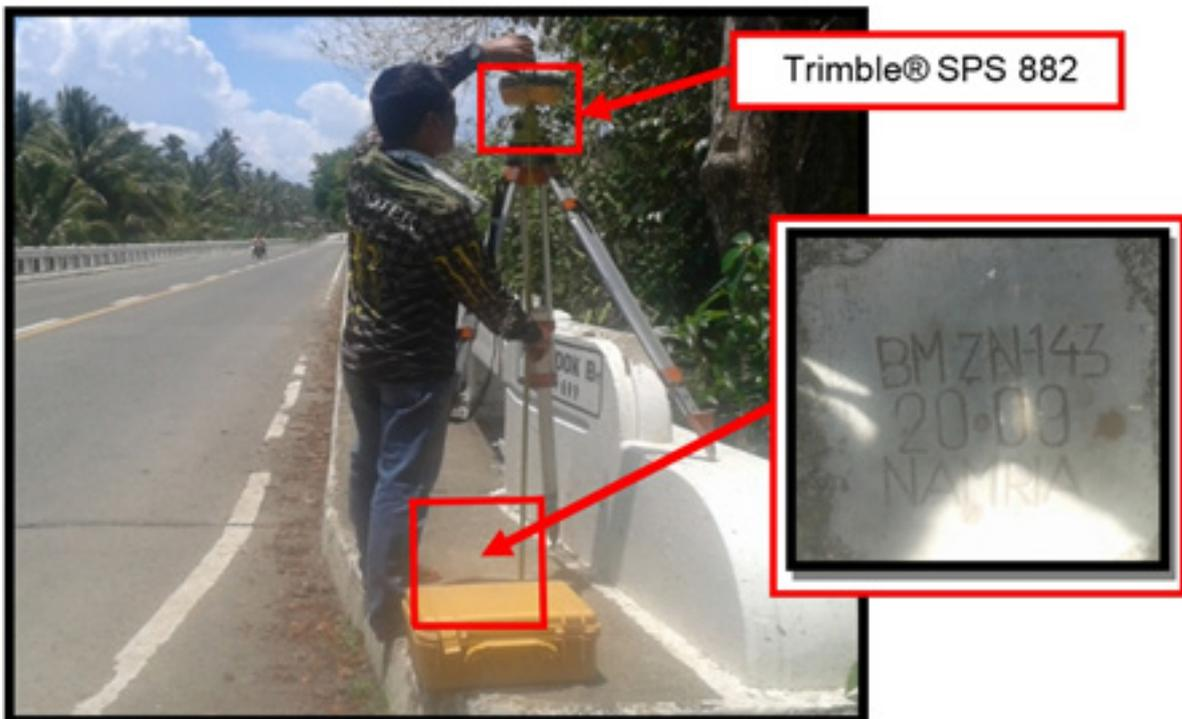
Figure 30. GNSS rover, Trimble® SPS 882, at ZN-143, an established control point, located at the right side walk going to Brgy. Rizon direction of Polandok Bridge in Brgy. Ramon Magsaysay, Salug, Province of Zamboanga del Norte
