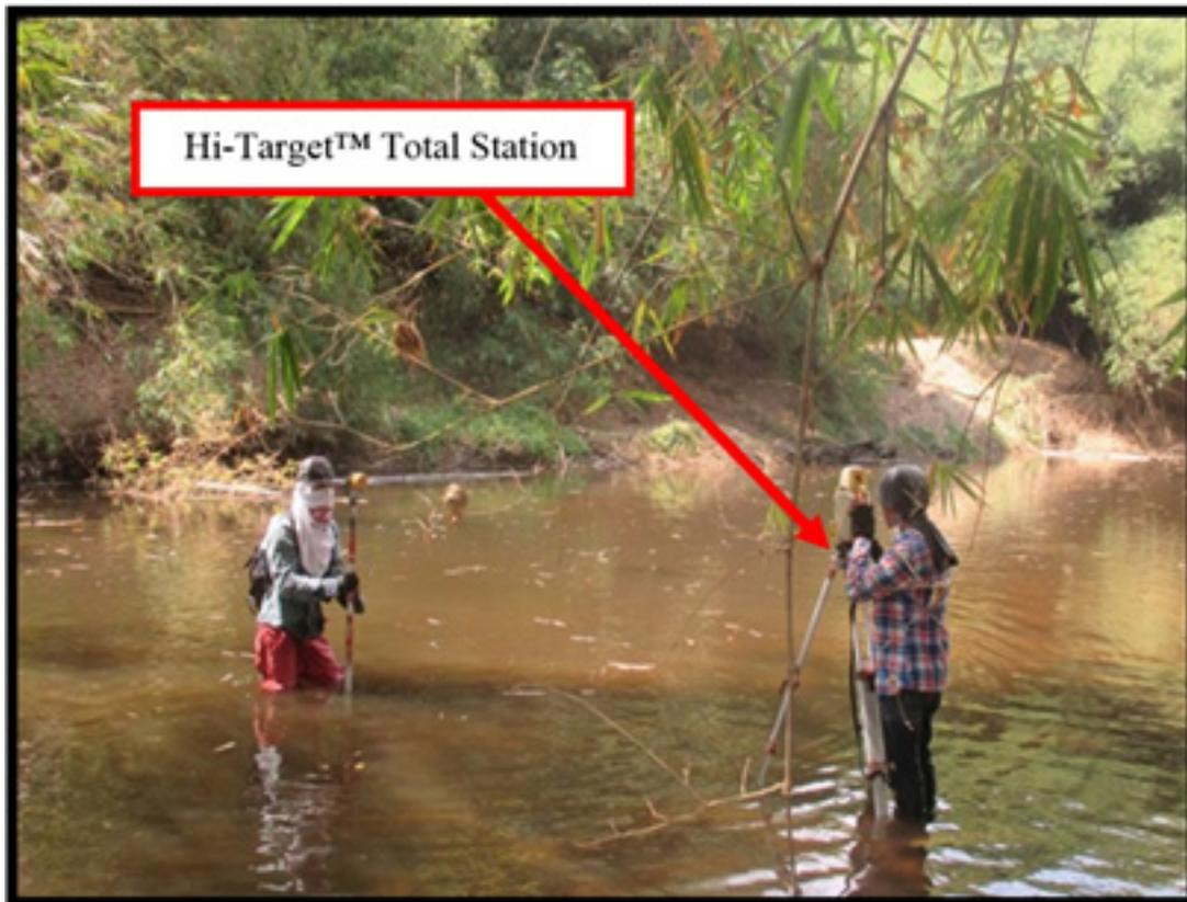
Figure 43. Cross-section survey at Patawag River using Hi-Target™ Total Station
