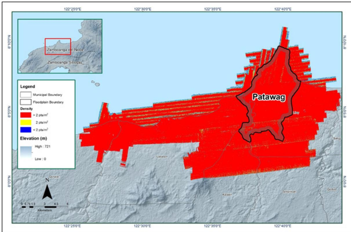
Figure 13. Pulse density map of merged LiDAR data for Patawag floodplain.
