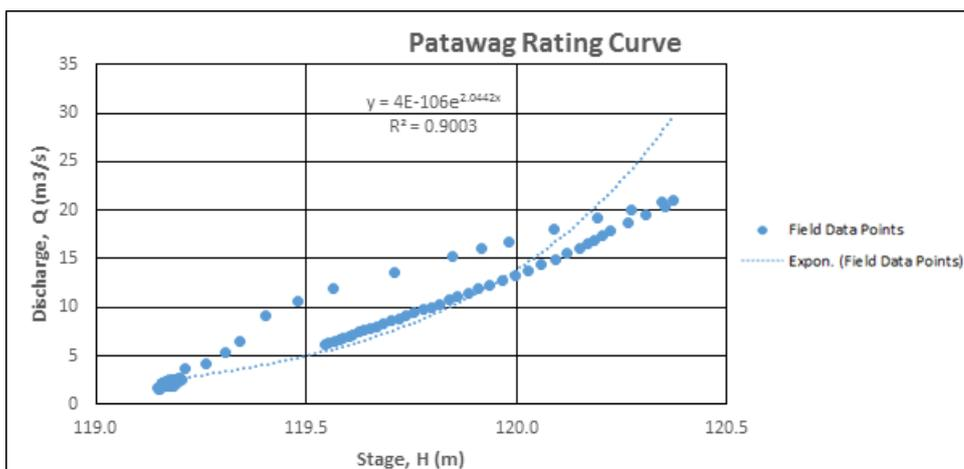
Figure 49. Rating Curve at Spillway, Brgy. El Paraiso, Liloy, Zamboanga del Norte
