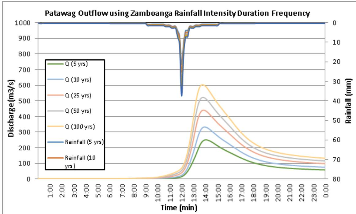
Figure 63. Outflow hydrograph at Patawag Bridge Station generated using Zamboanga City RIDF simulated in HEC-HMS
