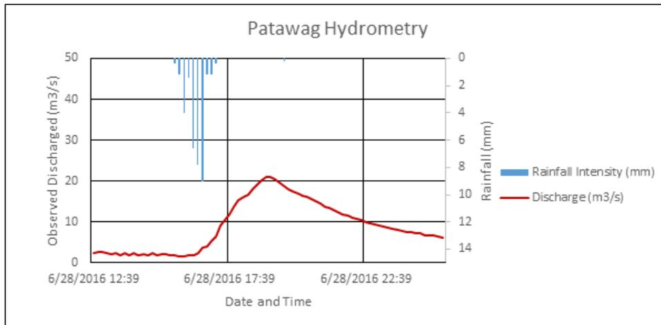
Figure50. Rainfall and outflow data at Spillway, Brgy. El Paraiso used for modeling
