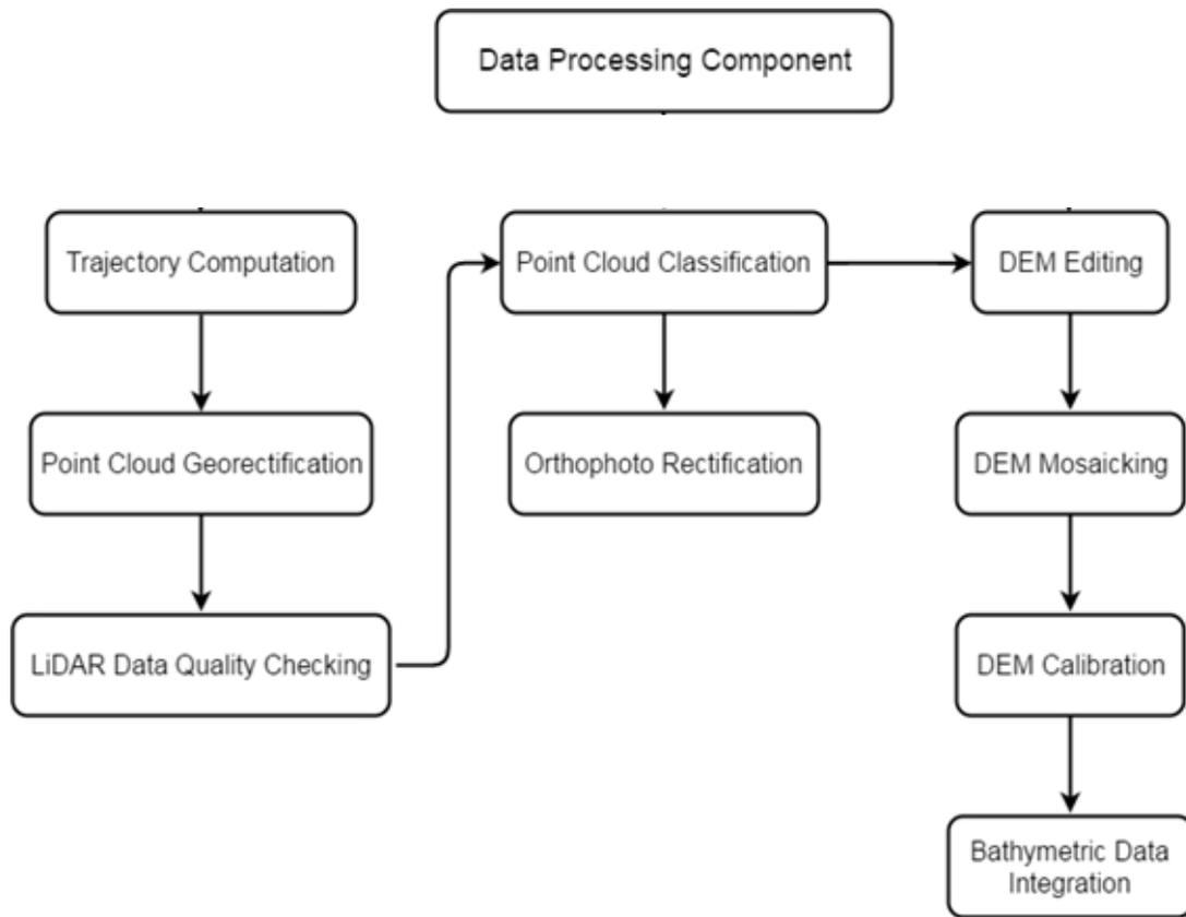
Figure 7. Schematic Diagram for Data Pre-Processing Component
