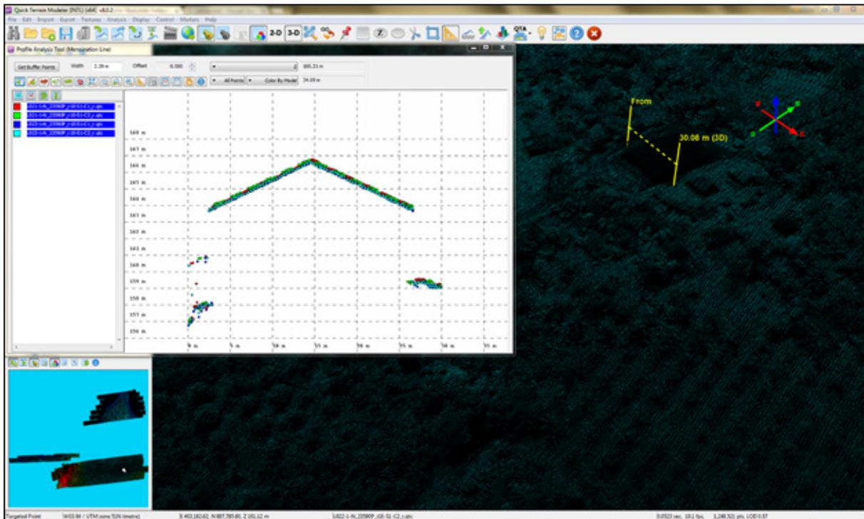
Figure 15. Quality checking for Patowag flight 23590P using the Profile Tool of QT Modeler.
