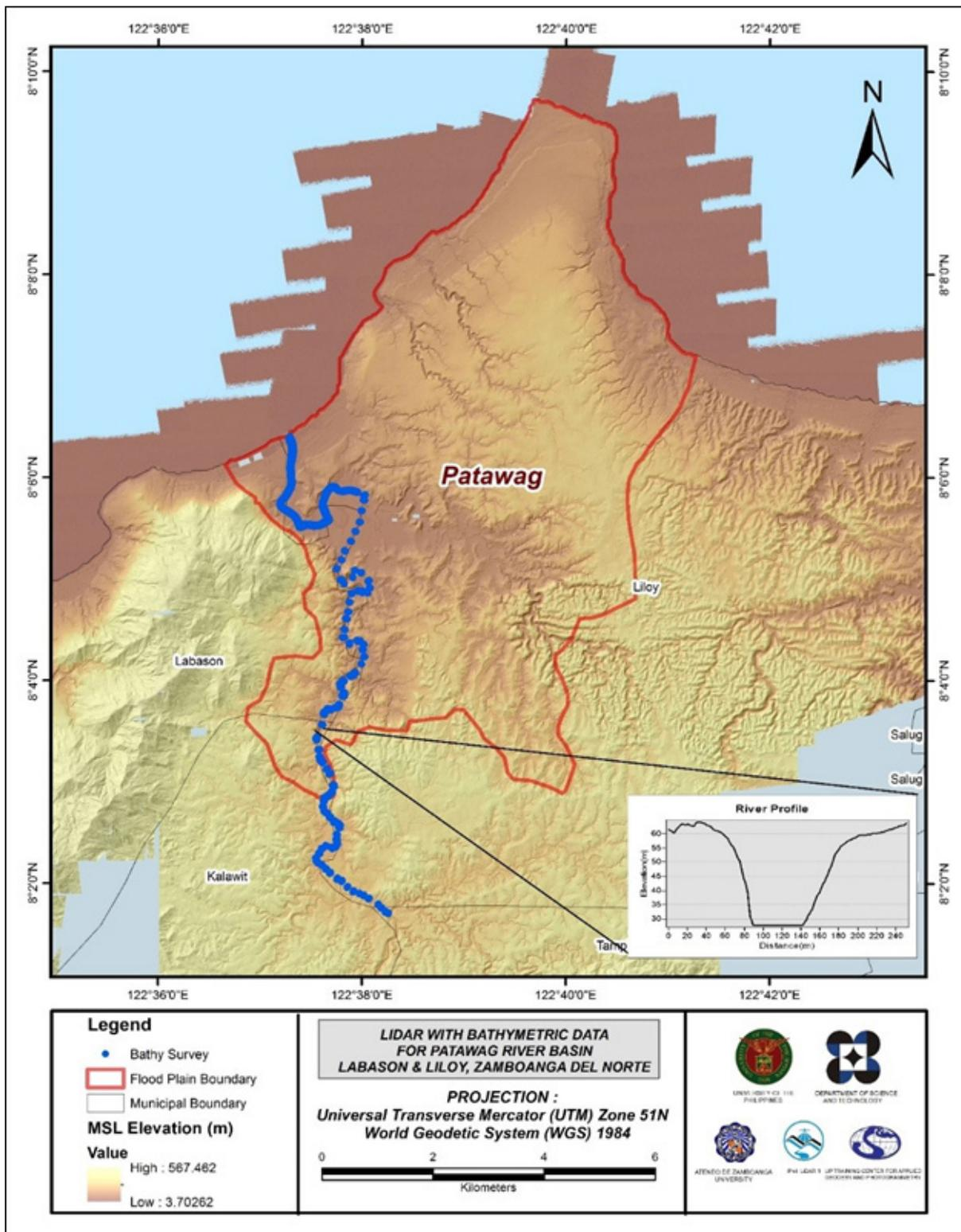
Figure 24. Map of Patawag Floodplain with bathymetric survey points shown in blue.
