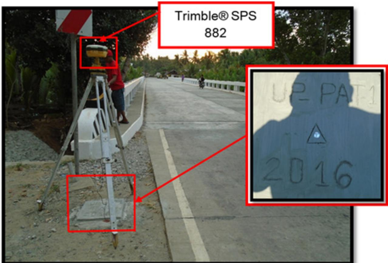
Figure33. GNSS receiver set up, Trimble® SPS 882, UP\_PAT-1 at the side of Labason-Liloy Road near Patawag Bridge in Brgy. Patawag, Municipality of Labason, Province of Zamboanga del Norte
