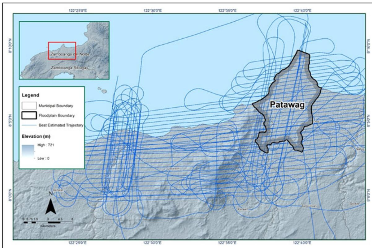
Figure 10. Best estimated trajectory for Patawag Floodplain.Floodplain.
