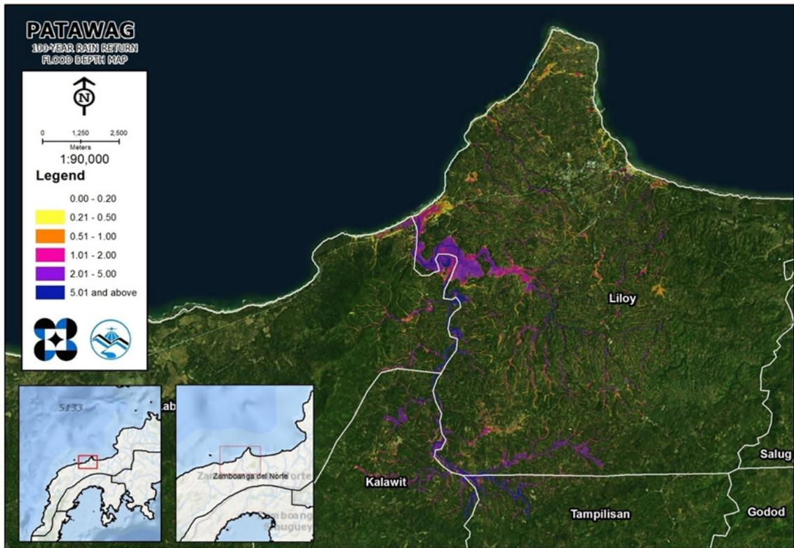
Figure 66. 100-year Flow Depth Map for Patawag Floodplain
