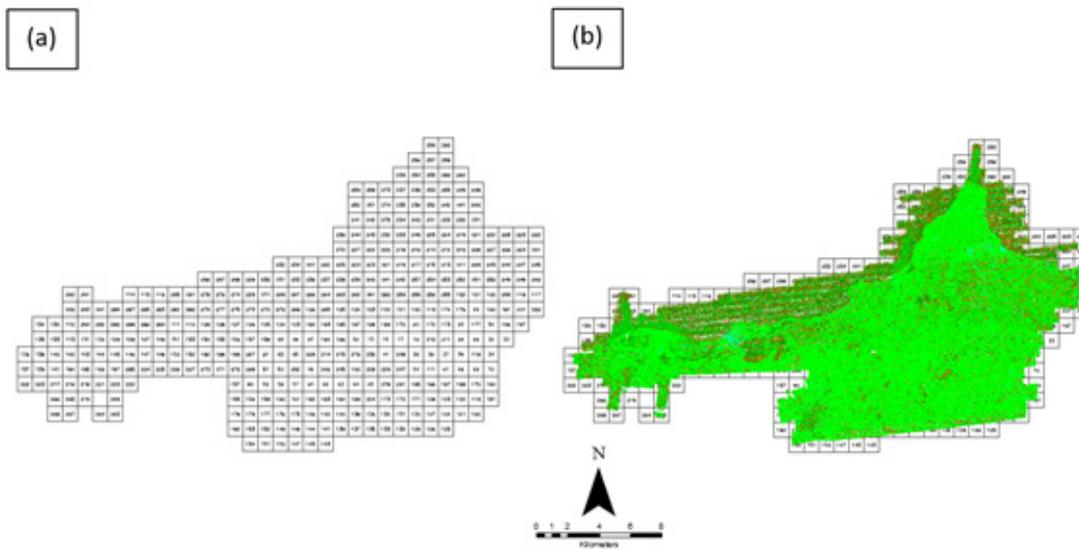
Figure 16. Tiles for Patawag floodplain (a) and classification results (b) in TerraScan.
