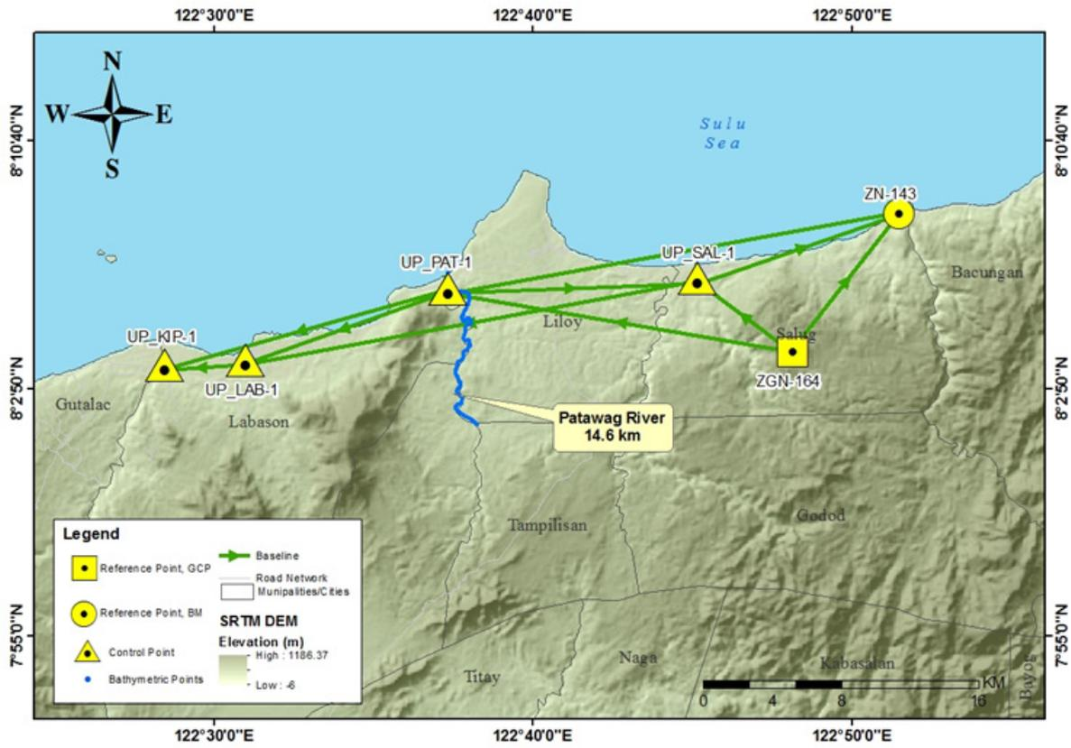
Figure 28. Patawag River Basin Control Survey Extent
