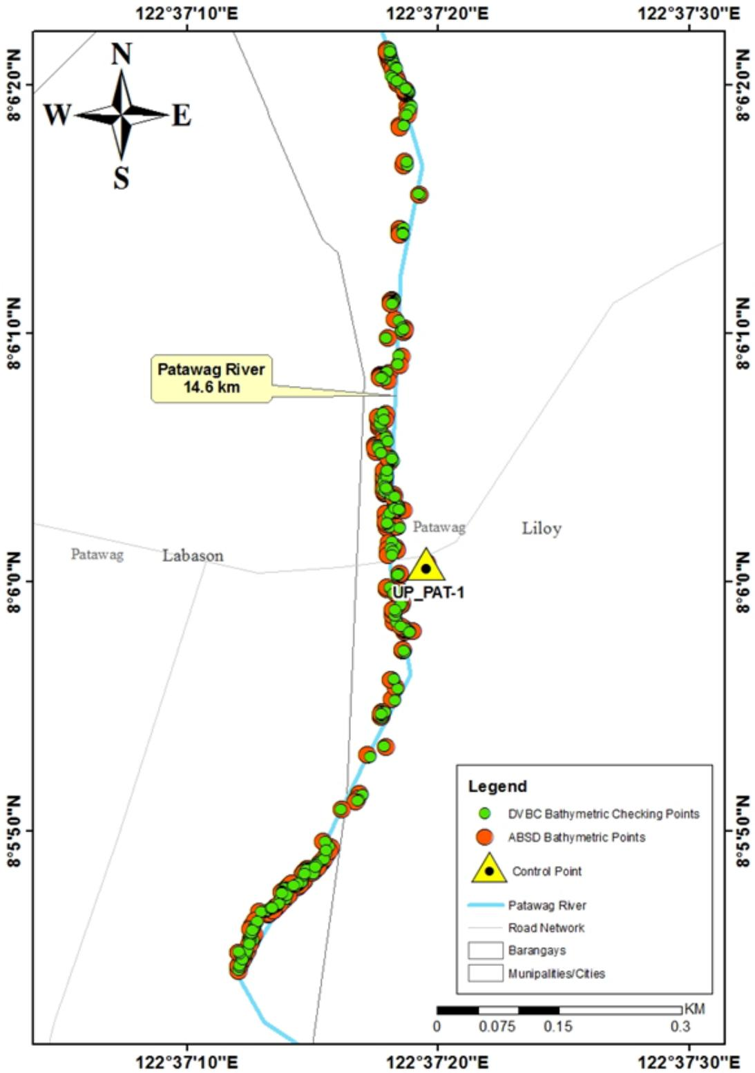
Figure 45. Quality checking points gathered along Patawag River by DVBC
