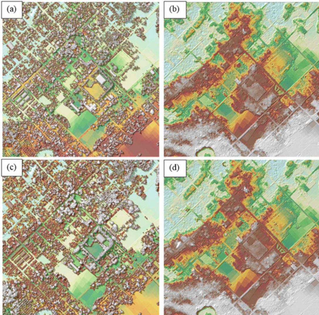
Figure 18. The production of last return DSM (a) and DTM (b), first return DSM (c) and secondary DTM (d) in some portion of Patowag Floodplain.
