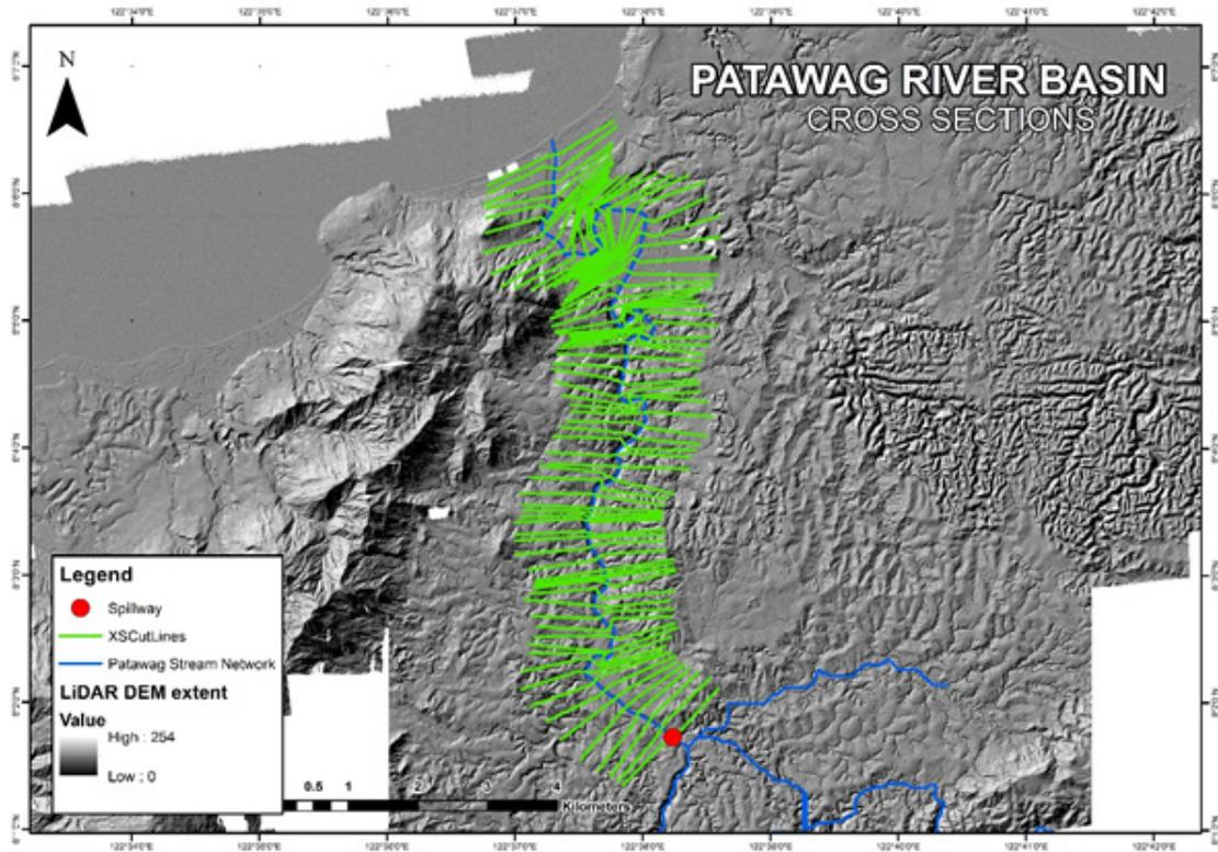
Figure 58. River cross-section of Patawag River generated through Arcmap HEC GeoRAS tool
