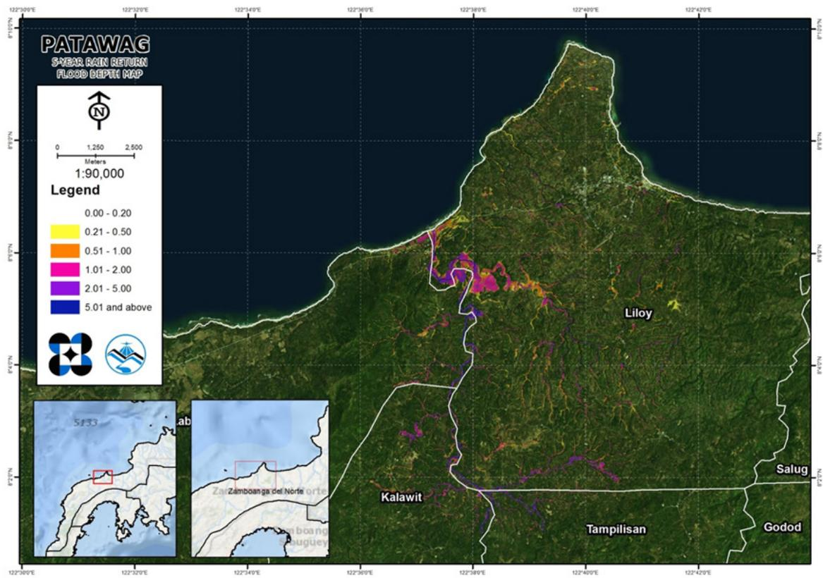
Figure 70. 5-year Flood Depth Map for Patawag Floodplain
