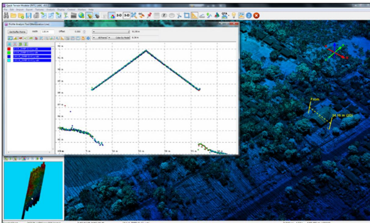
Figure 17. Quality checking for a Sanito flight 2549P using the Profile Tool of QT Modeler.
