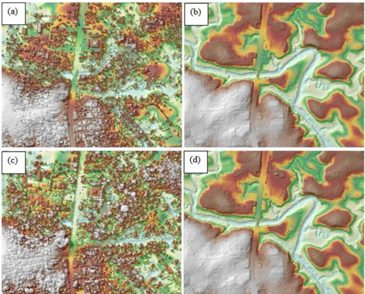
Figure 20. The production of last return DSM (a) and DTM (b), first return DSM (c) and secondary DTM (d) in some portion of Sanito Floodplain.
