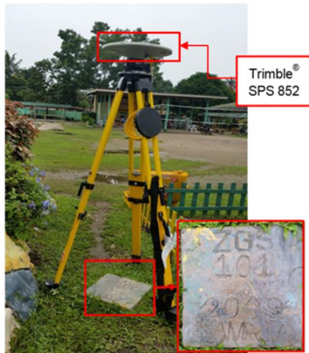
Figure 39. GNSS base set up, Trimble® SPS 852, at ZGS-101, located inside Brgy. Bolong Elementary School, Zamboanga City, Zamboanga Del Sur
