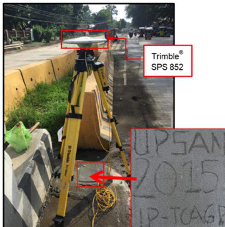
Figure 36. GNSS base set up, Trimble® SPS 882, at UP-SAN, located at the approach of Sanito Bridge in Brgy. Sanito, Municipality of Ipil, Zamboanga Sibugay
