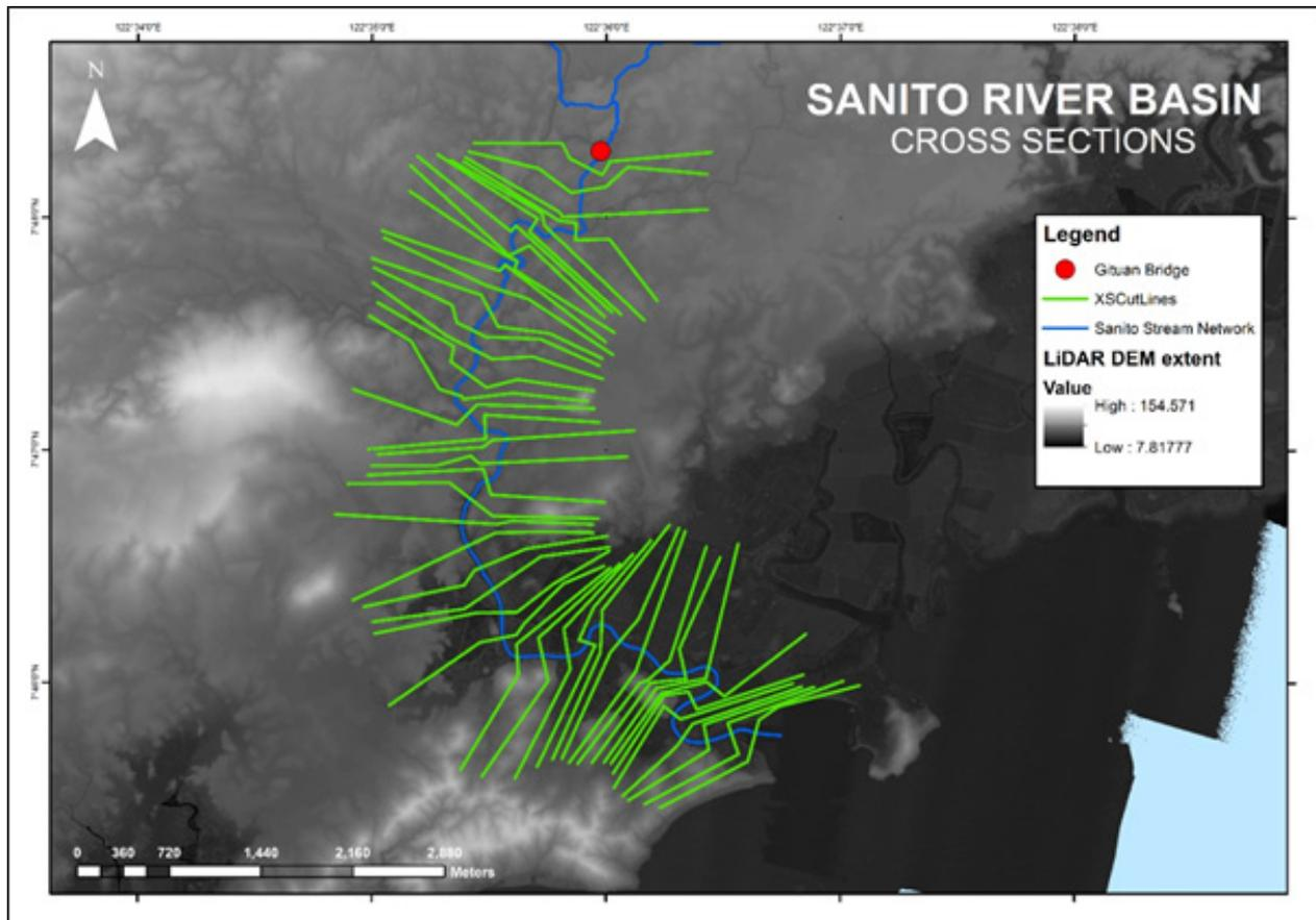
Figure 62. River cross-section of Sanito River generated through Arcmap HEC GeoRAS tool
