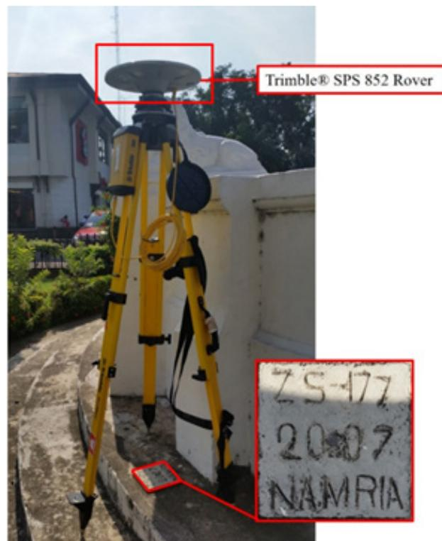
Figure 40. GNSS base set up, Trimble® SPS 852, at ZS-177, located at the stair of Rizal's Park along the Butuan-Zamboanga National Road, Brgy Zone 4, Zamboanga City, Zamboanga Del Sur
