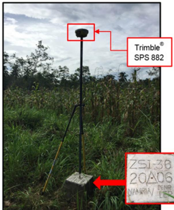
Figure 37. GNSS base set up, Trimble®SPS 882, at ZSI-36, located in front of an Iglesia ni Cristo church along the national highway in Brgy. Bacalan, Municipality of Ipil, Zamboanga Sibugay
