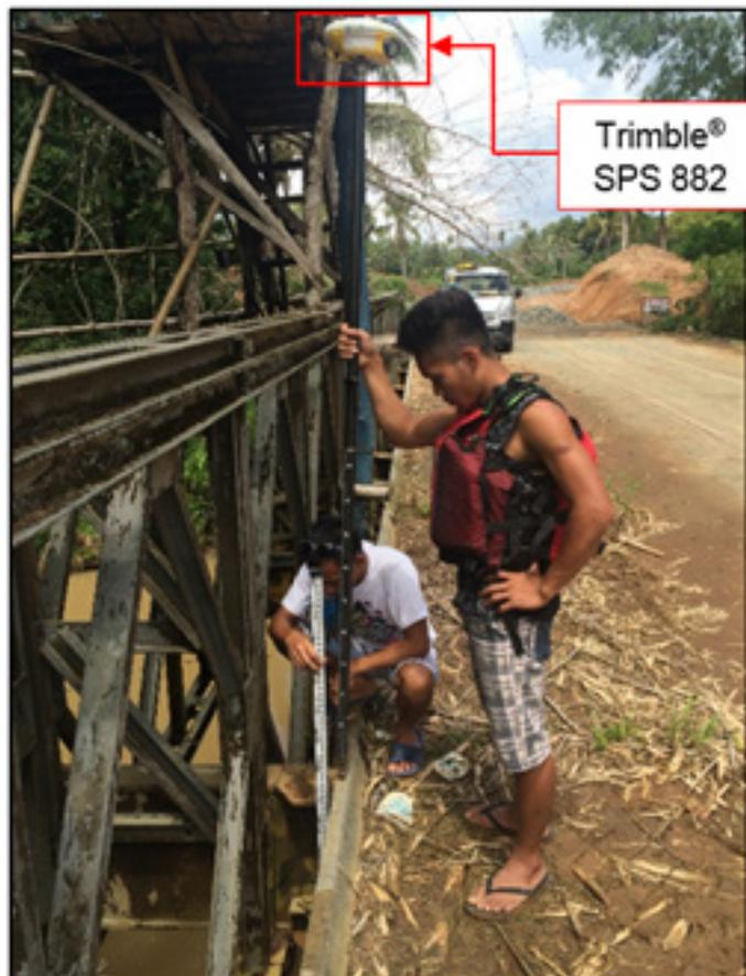
Figure 42. Cross-section and bridge as-built survey for Guituan Bridge, Brgy. Sanito, Ipil Zamboanga Sibugay
