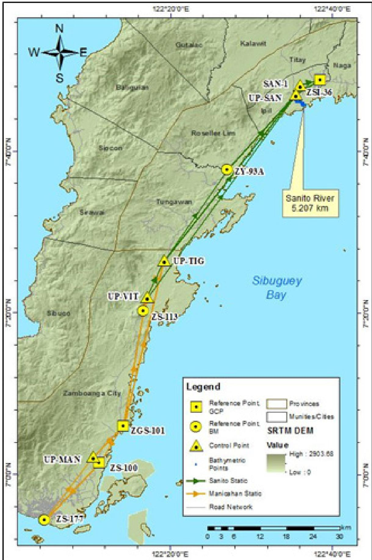
Figure 32. GNSS Network covering Sanito River
