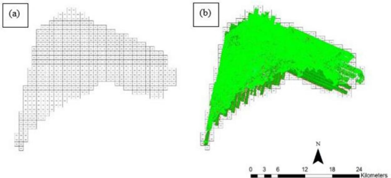
Figure 18. Tiles for Sanito Floodplain (a) and classification results (b) in TerraScan.
