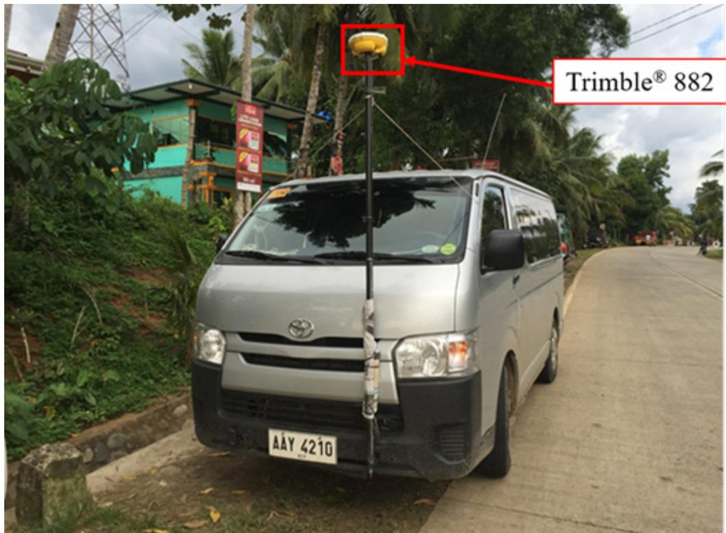
Figure 46. Trimble® SPS882 set-up for validation points acquisition survey for Sanito River
