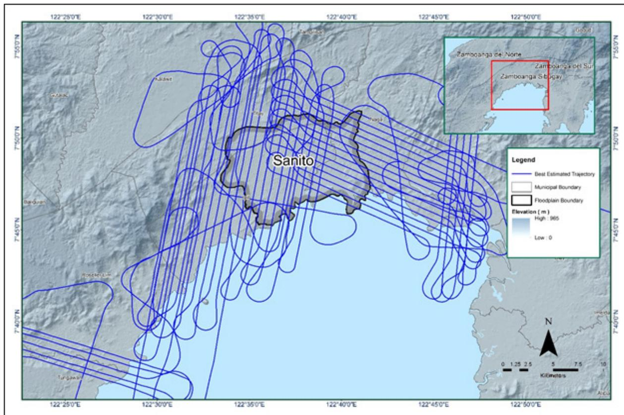
Figure 12. Best estimated trajectory of the LiDAR missions conducted over the Sanito Floodplain.
