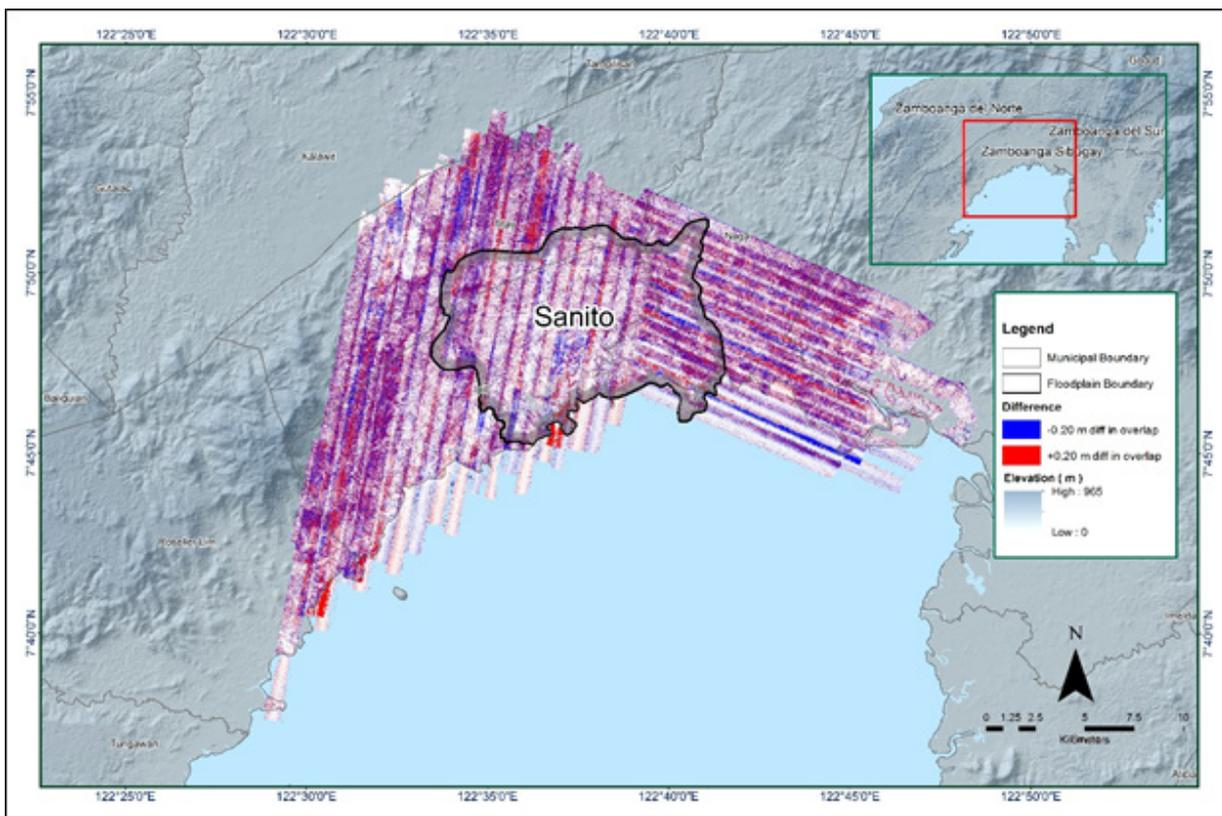
Figure 16. Elevation difference map between flight lines for Sanito Floodplain.
