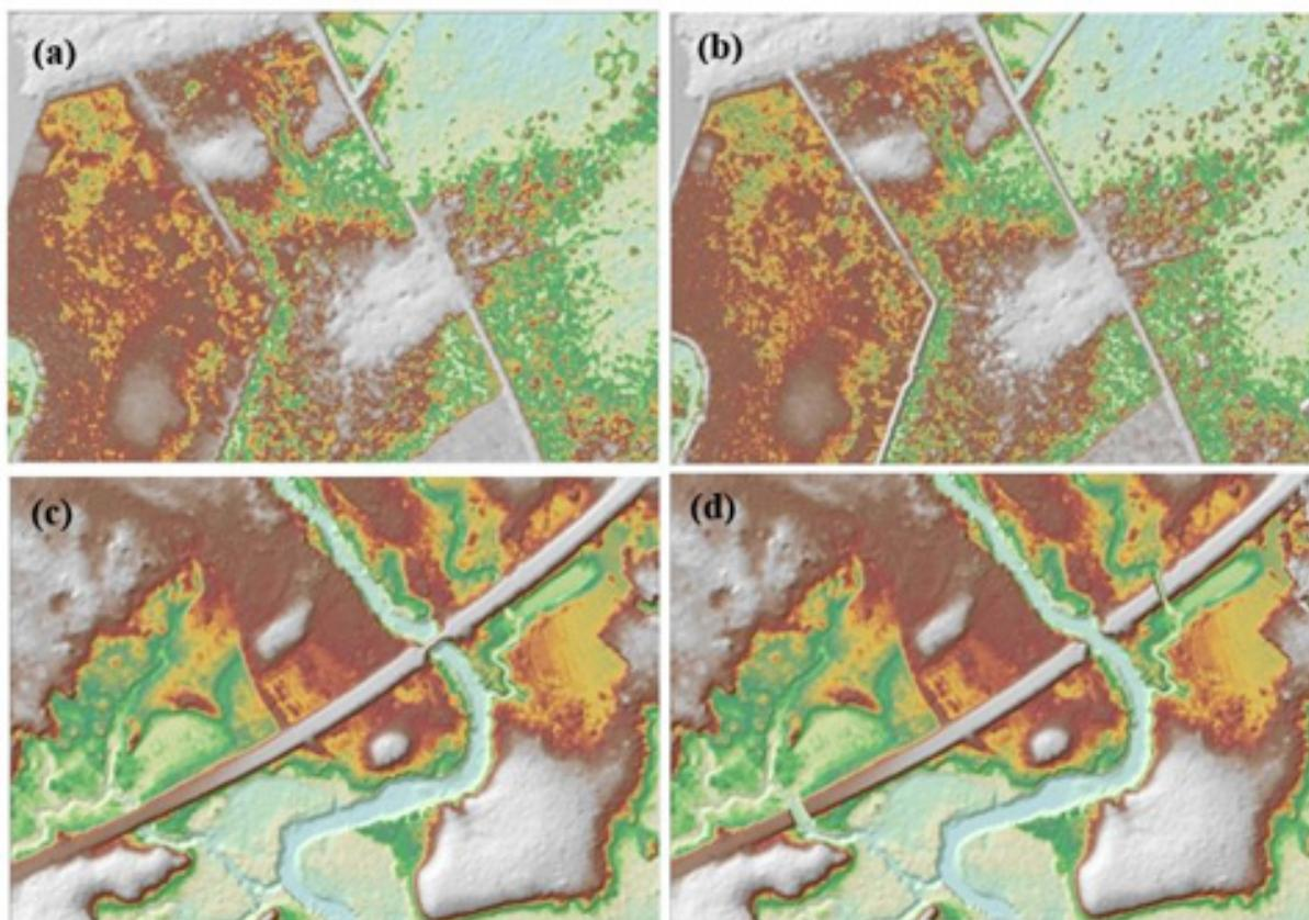
Figure 23. Portions in the DTM of Sanito floodplain – a paddy field before (a) and after (b) data retrieval; a bridge before (c) and after (d) manual editing.
