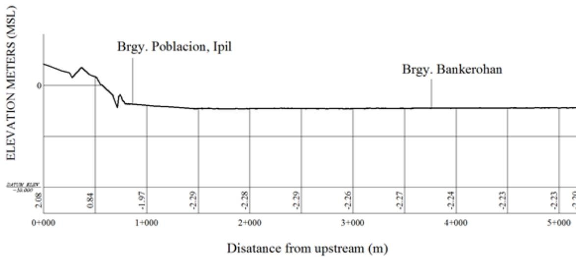
Figure 50. Riverbed Profile of Sanito River
