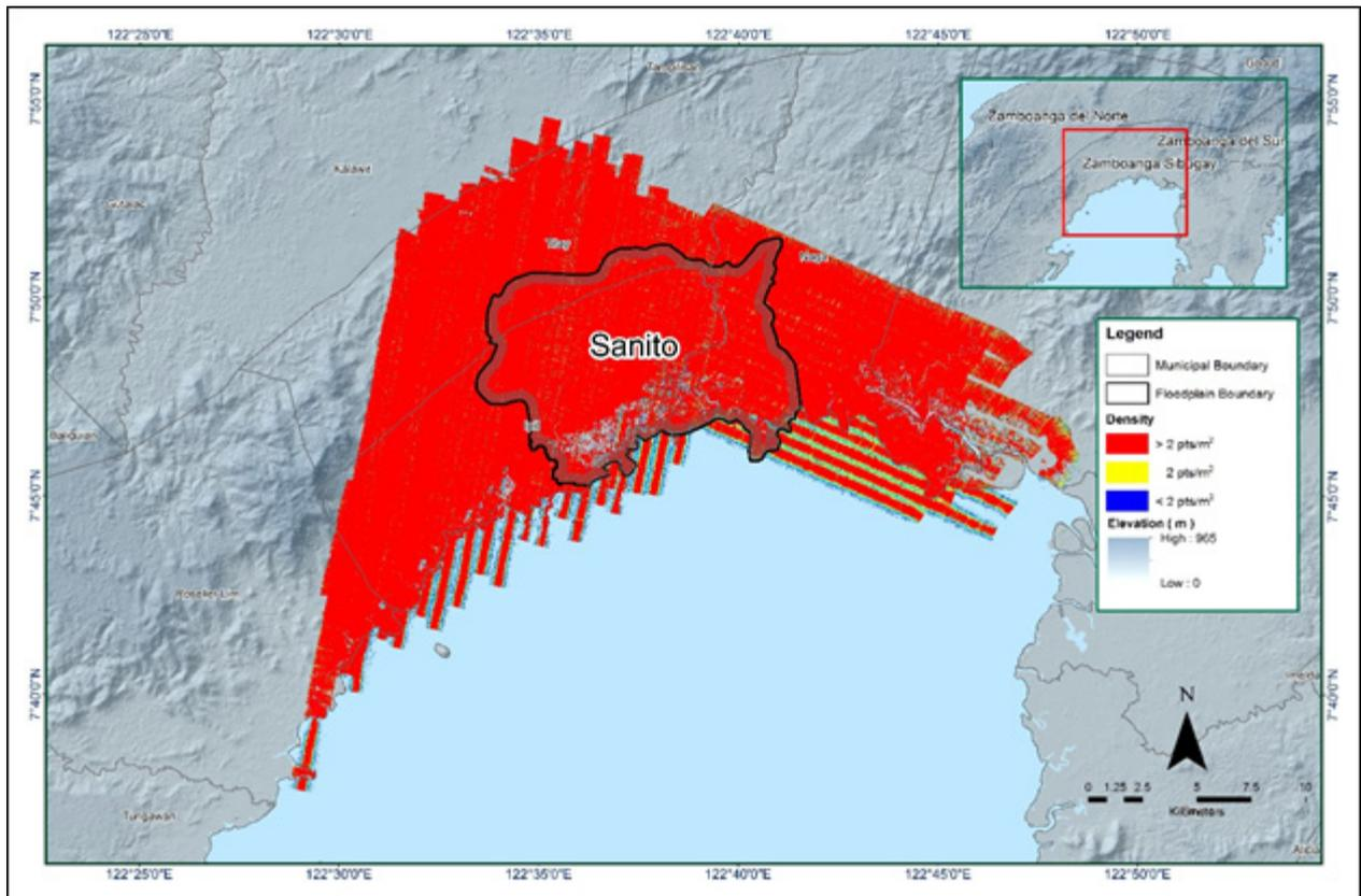
Figure 15. Pulse density map of merged LiDAR data for Sanito Floodplain.
