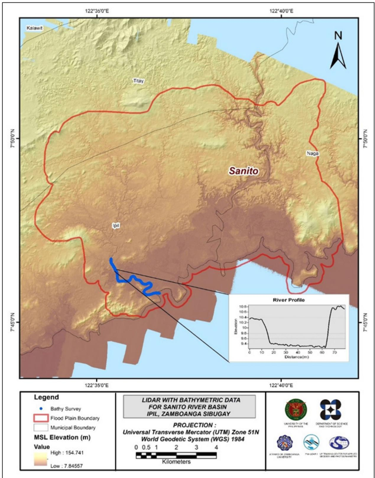
Figure 28. Map of Sanito Floodplain with bathymetric survey points shown in blue.
