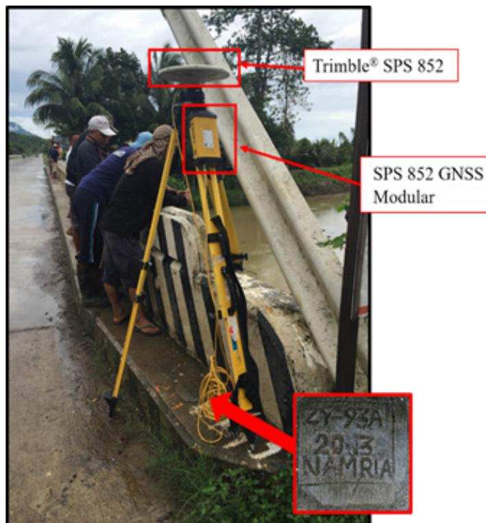
Figure 38. GNSS base set up, Trimble® SPS 852, at ZY-93A, located at the approach of Tupilac Bridge, in Brgy. Tupilac, Municipality of Roseller Lim, Zamboanga Sibugay
