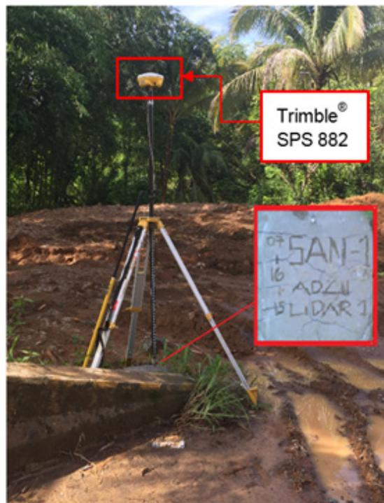
Figure 35. GNSS base set up, Trimble® SPS 882, at SAN-1, located at the approach of an unknown bridge found between Alibutdan and Diversion Rd, in Brgy. Pangi, Municipality of Ipi, Zamboanga Sibugay
