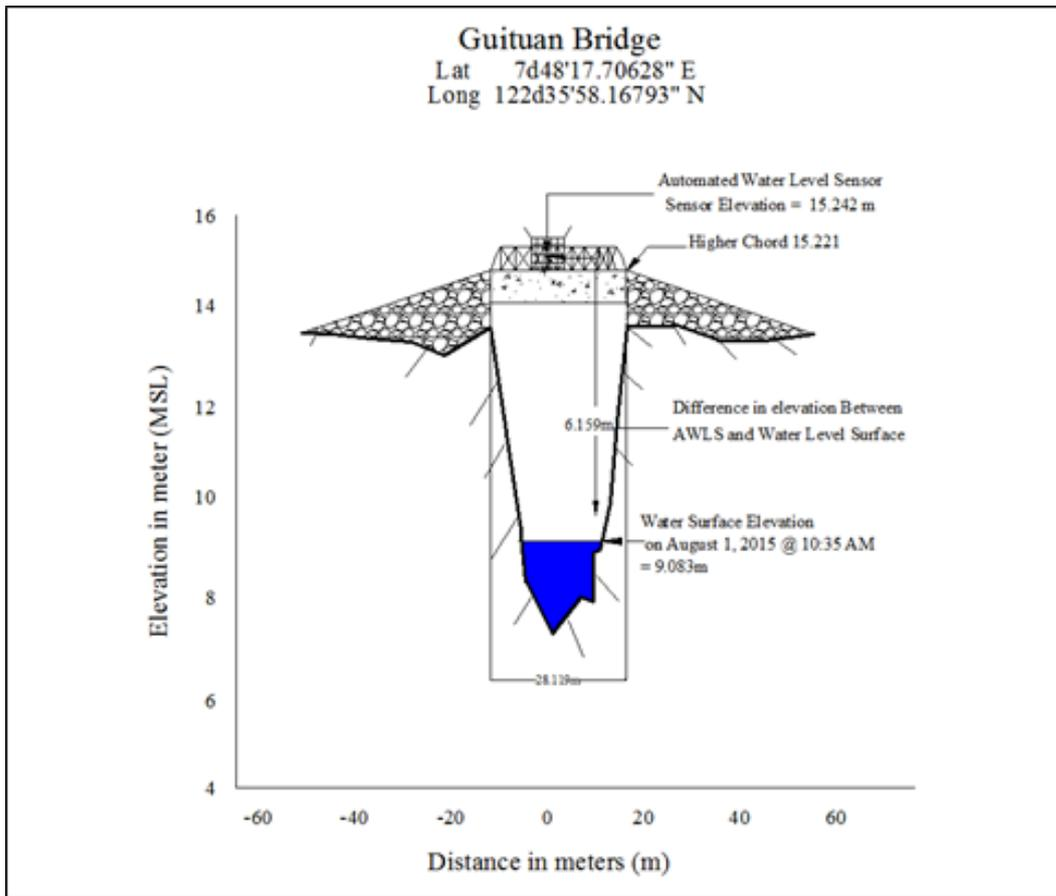
Figure 43. Guituan Bridge cross-sectional diagram
