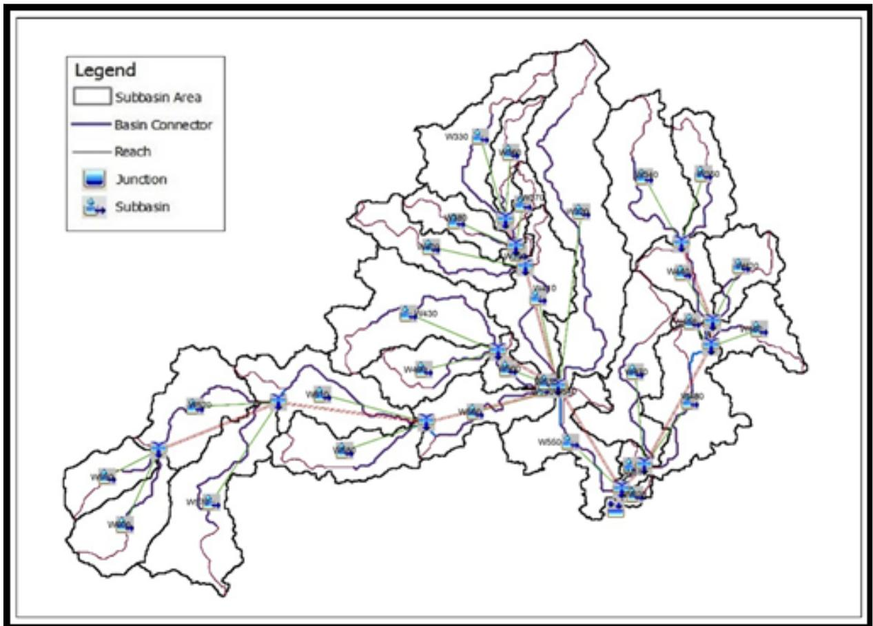
Figure 61. The Sanito river basin model generated using HEC-HMS
