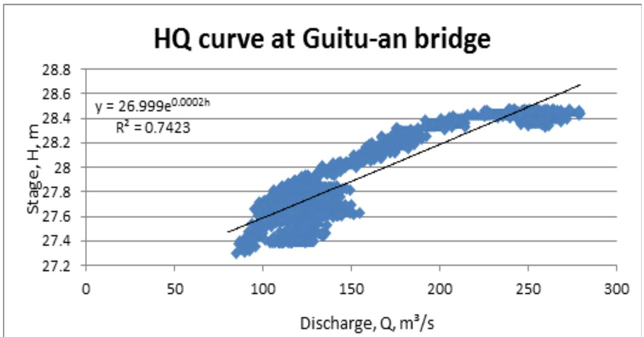
Figure 53. Rating Curve at Guitu-an Bridge, Guitu-an, Ipil, Zamboanga Sibugay
