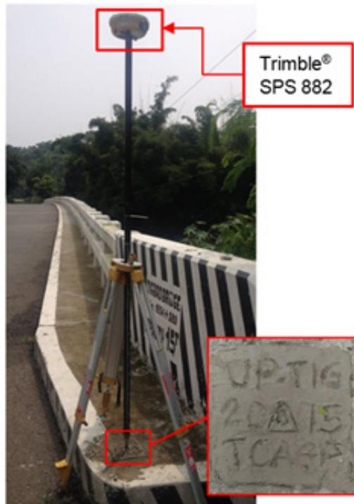
Figure 33. GNSS base set up, Trimble® SPS 882, at UP-TIG, located at the approach of Tigbao Bridge, Brgy. Tictapul, Zamboanga City, Zamboanga Del Sur
