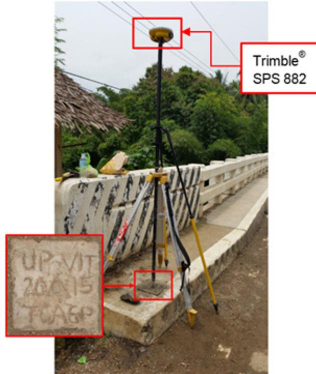
Figure 34. GNSS base set up, Trimble® SPS 882, at UP-VIT, located at the approach of Vitali Bridge in Brgy. Vitali, Zamboanga City, Zamboanga Del Sur
