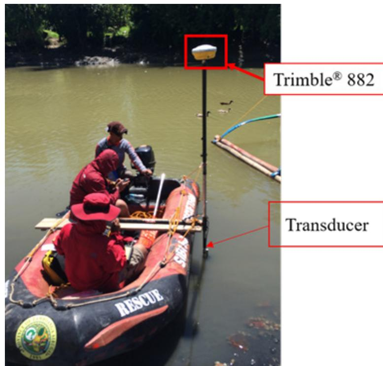
Figure 48. Bathymetric survey in Sanito River
