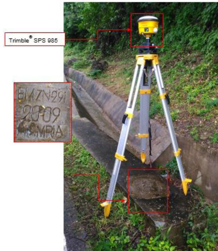
Figure 32. GNSS receiver set up, Trimble® SPS 985, at ZN-291, located in Brgy. Matiag, Siocon, Zamboanga Del Norte
