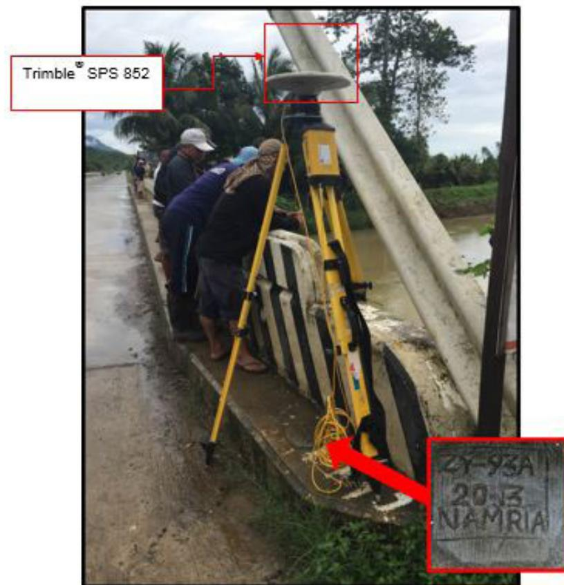
Figure 33. GNSS base set up, Trimble® SPS 852, at ZY-93A, located in Brgy. Tupilac, Roseller Lim, Zamboanga Sibugay
