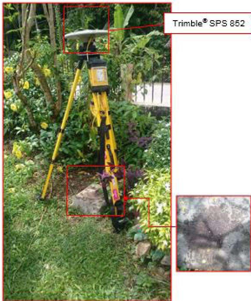
Figure 31. GNSS base set up, Trimble® SPS 852, at ZGN-143, located in Brgy.
