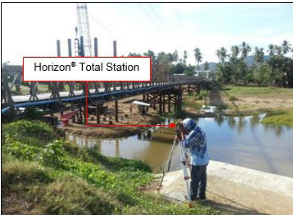
Figure 36. As-built survey of Siocon Bridge
