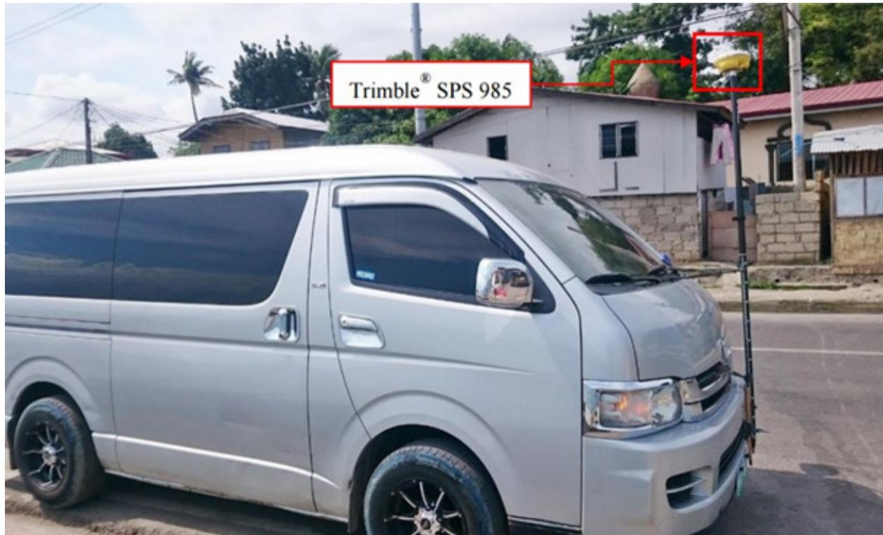
Figure 41. Validation points acquisition survey set-up for Siocon River
