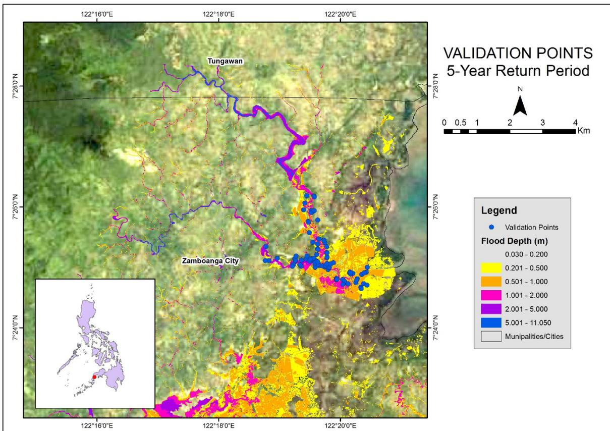
Figure 83. Validation points for 5-year Flood Depth Map of Tigbao Floodplain
