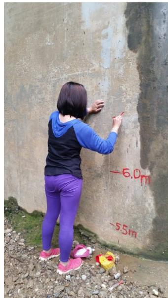
Figure 46. Water-level marking at Tigbao Bridge’s Footing
