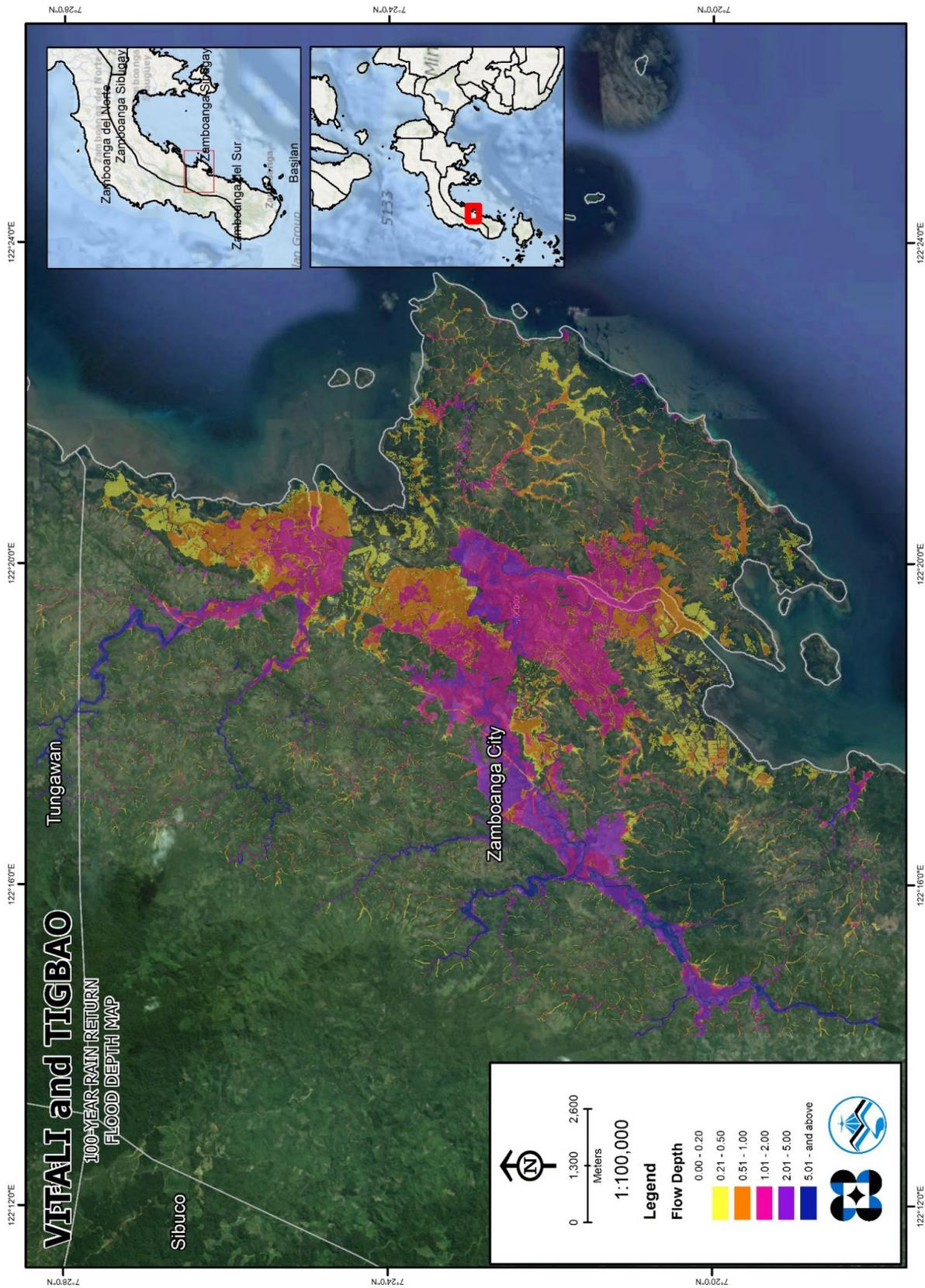
Figure 73. 25-year Flood Hazard Map for Tigbao Floodplain
