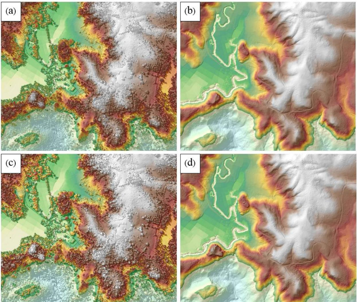
Figure 21. The production of last return DSM (a) and DTM (b), first return DSM (c) and secondary DTM (d) in some portion of Tigbao Floodplain.
