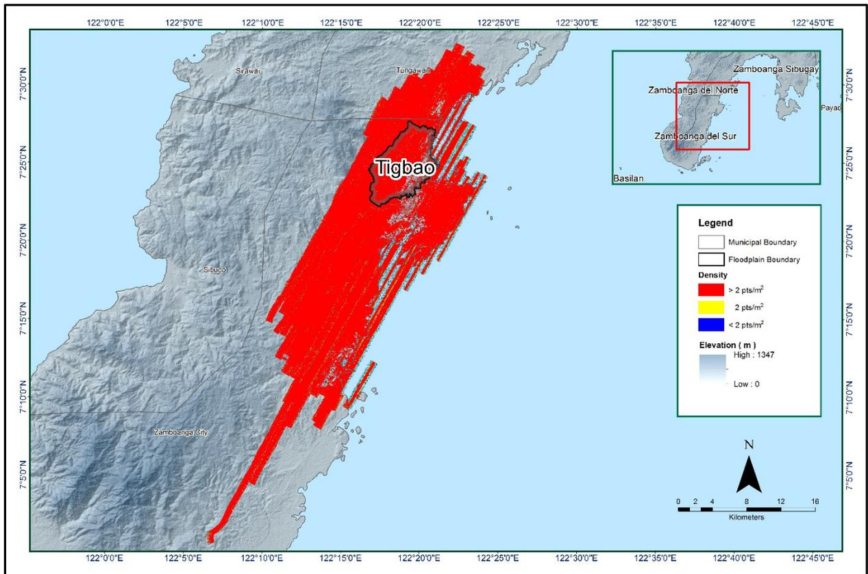
Figure 16. Pulse density map of merged LiDAR data for Tigbao Floodplain.
