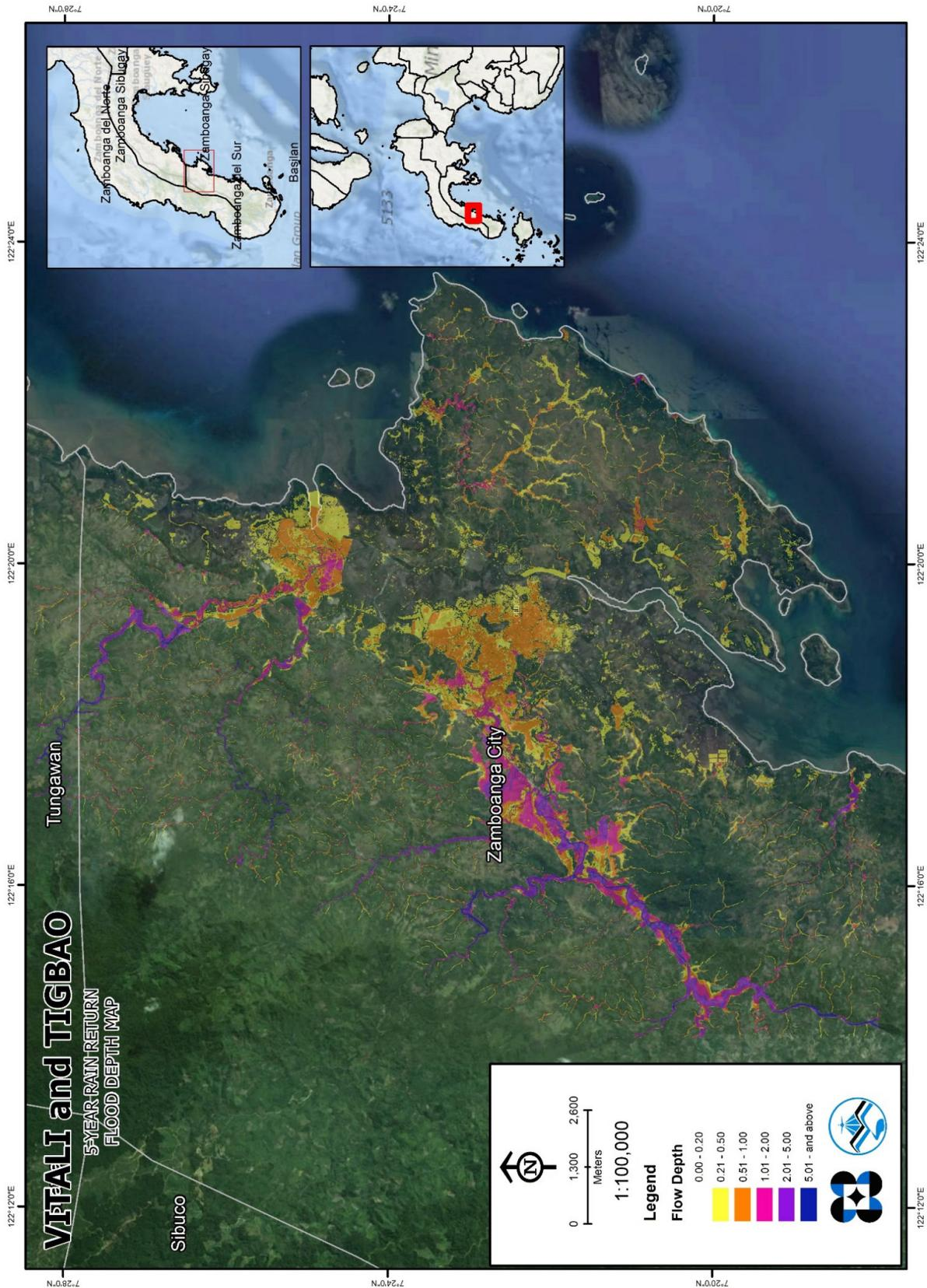
Figure 76. 5-year Flood Depth Map for Tigbao Floodplain
