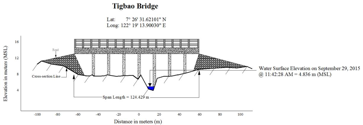
Figure 43. Tigbao River cross-sectional diagram
