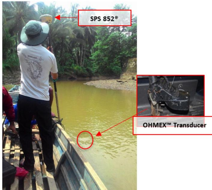
Figure 49. OHMEX™ single beam echo sounder set up on a boat for Tigbao River bathymetric survey
