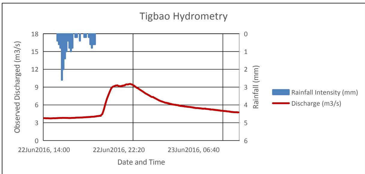
Figure 56. Rainfall and outflow data at Tigbao Bridge used for modeling
