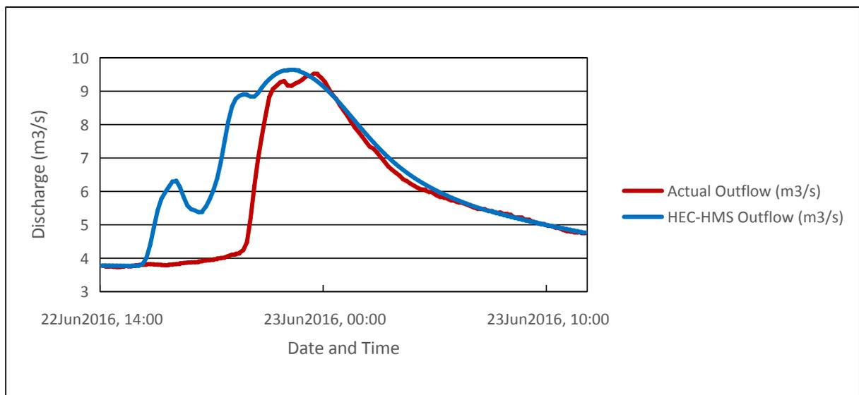
Figure 68. Outflow Hydrograph of Tigbao produced by the HEC-HMS model compared with observed outflow
