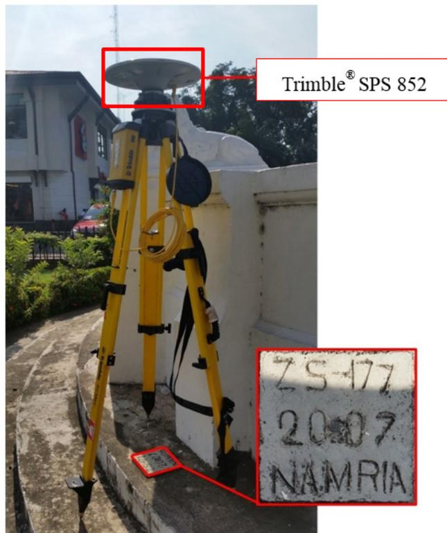
Figure 35. Trimble® SPS 852 set-up at ZS-177 located at the stair of Rizal's Park in Brgy. Poblacion, Zamboanga City
