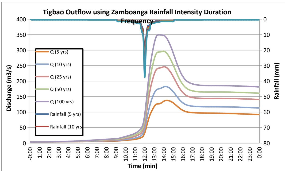
Figure 69. Outflow hydrograph at Guitu-an Bridge Station generated using Zamboanga City RIDF simulated in HEC-HMS
