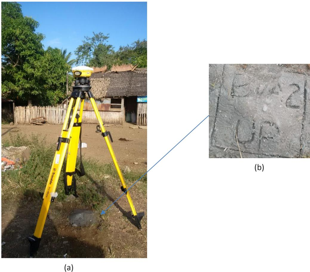
Figure 8. GPS set-up over BVA-2 as established near a waiting shed in Brgy. Buenavista, Zamboanga City (a) and reference point BVA-2 (b) as established by the field team.
