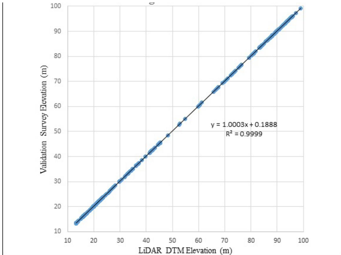
Figure 28. Correlation plot between validation survey points and LiDAR data.
