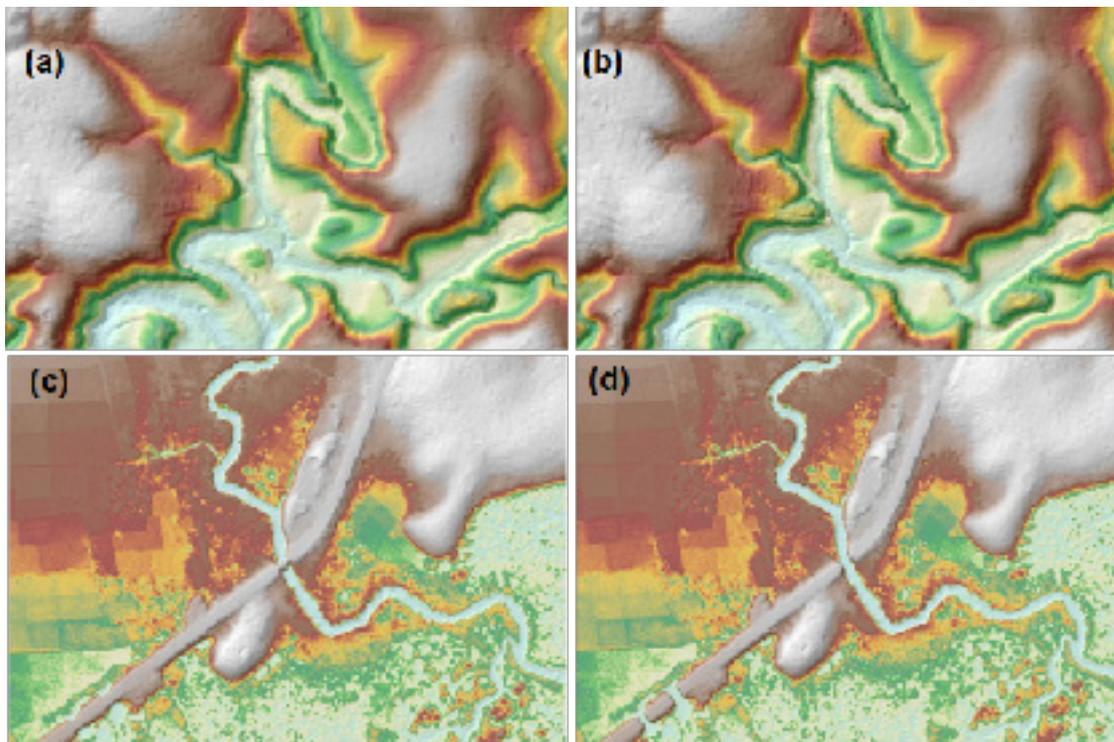
Figure 24. Portions in the DTM of Tigbao Floodplain – a river embankment before (a) and after (b) data retrieval; a road before (c) and after (d) manual editing.
