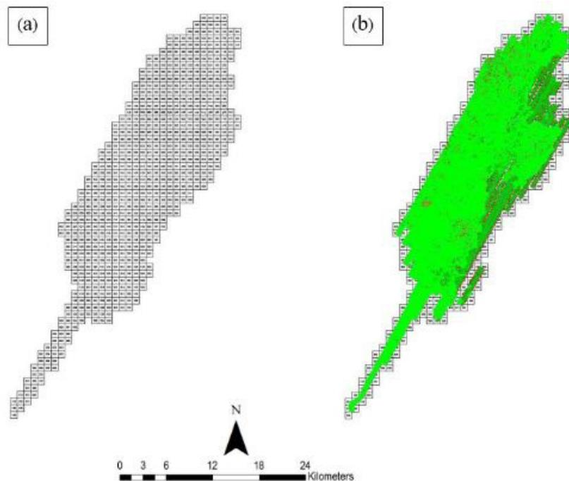
Figure 19. Tiles for Tigbao Floodplain (a) and classification results (b) in TerraScan.
