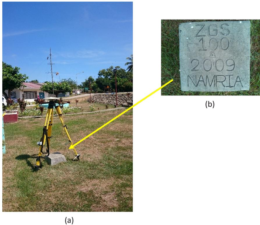
Figure 6. GPS set-up over ZGS-100 in Brgy. Manicahan, Zamboanga City located at the road intersections going to Cagayan de Oro, Butuan City and Iligan City (a) and NAMRIA reference point ZGS-100 (b) as recovered by the field team.
