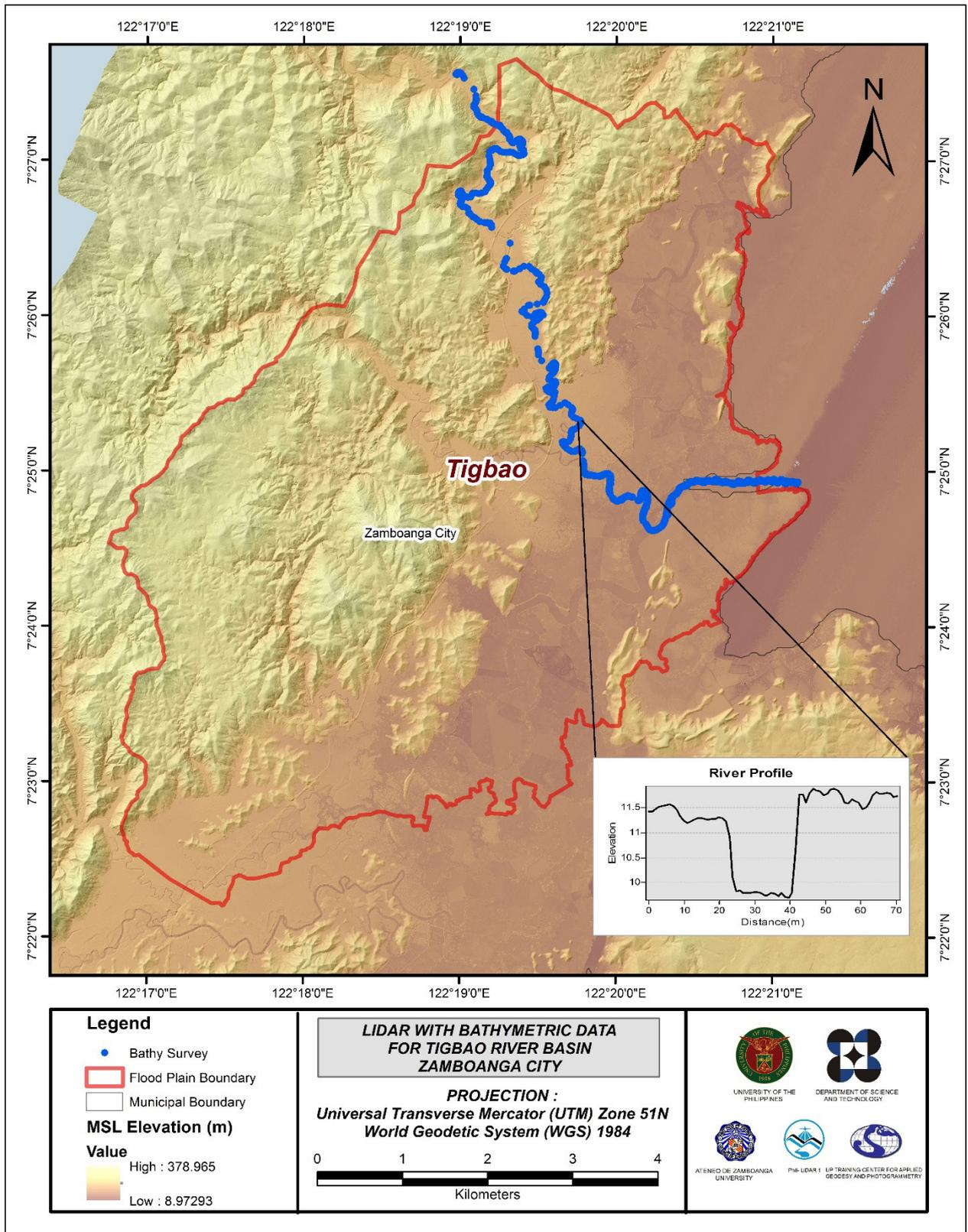
Figure 29. Map of Tigbao Floodplain with bathymetric survey points shown in blue.
