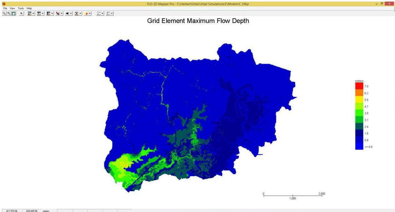
Figure 67. Generated 100-year rain return flow depth map from FLO-2D Mapper
