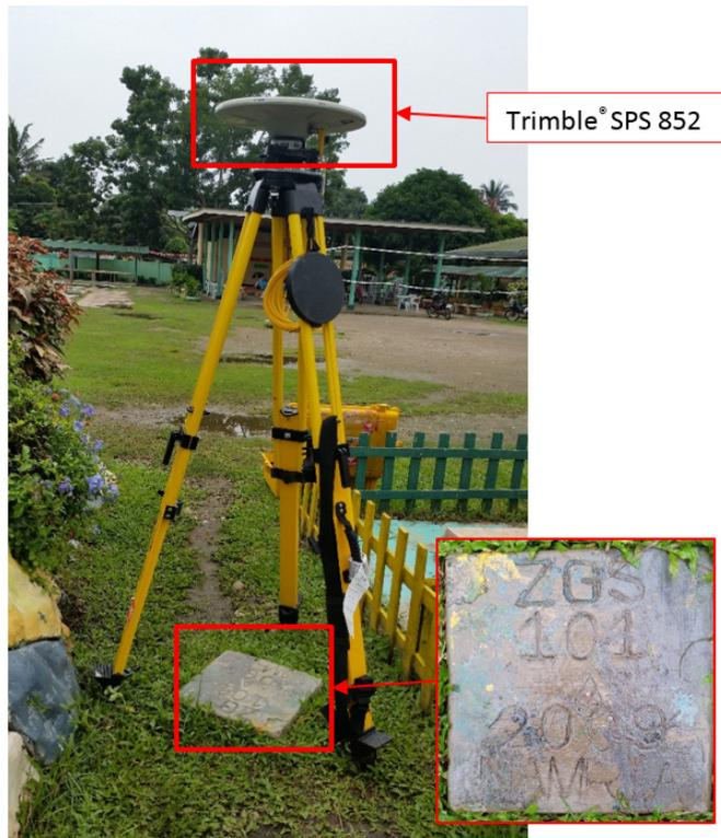
Figure 34. Trimble® SPS 852 set-up at ZGS-101 located at Bolong Elementary School, Brgy. Bolong, Zamboanga City
