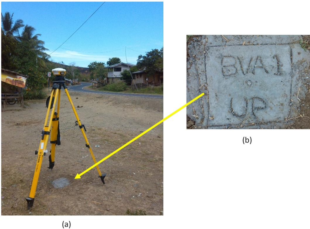
Figure 7. GPS set-up over BVA-1 at Brgy. Buenavista, Zamboanga City (a) and reference point BVA-1 (b) as established by the field team.
