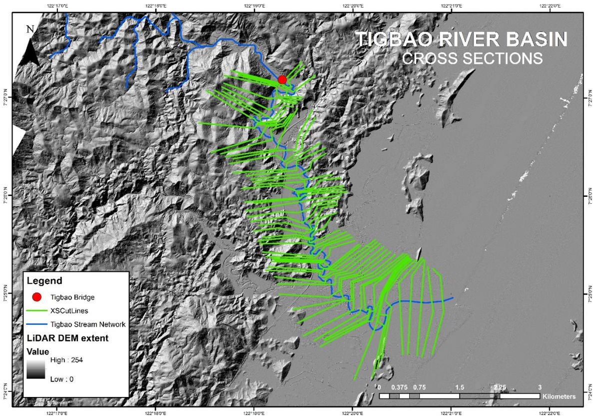
Figure 64. River cross-section of Tigbao River generated through Arcmap HEC GeoRAS tool
