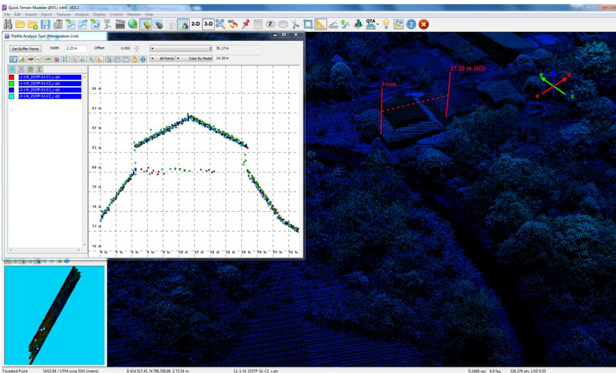
Figure 18. Quality checking for a Tigbao flight 2537P using the Profile Tool of QT Modeler.
