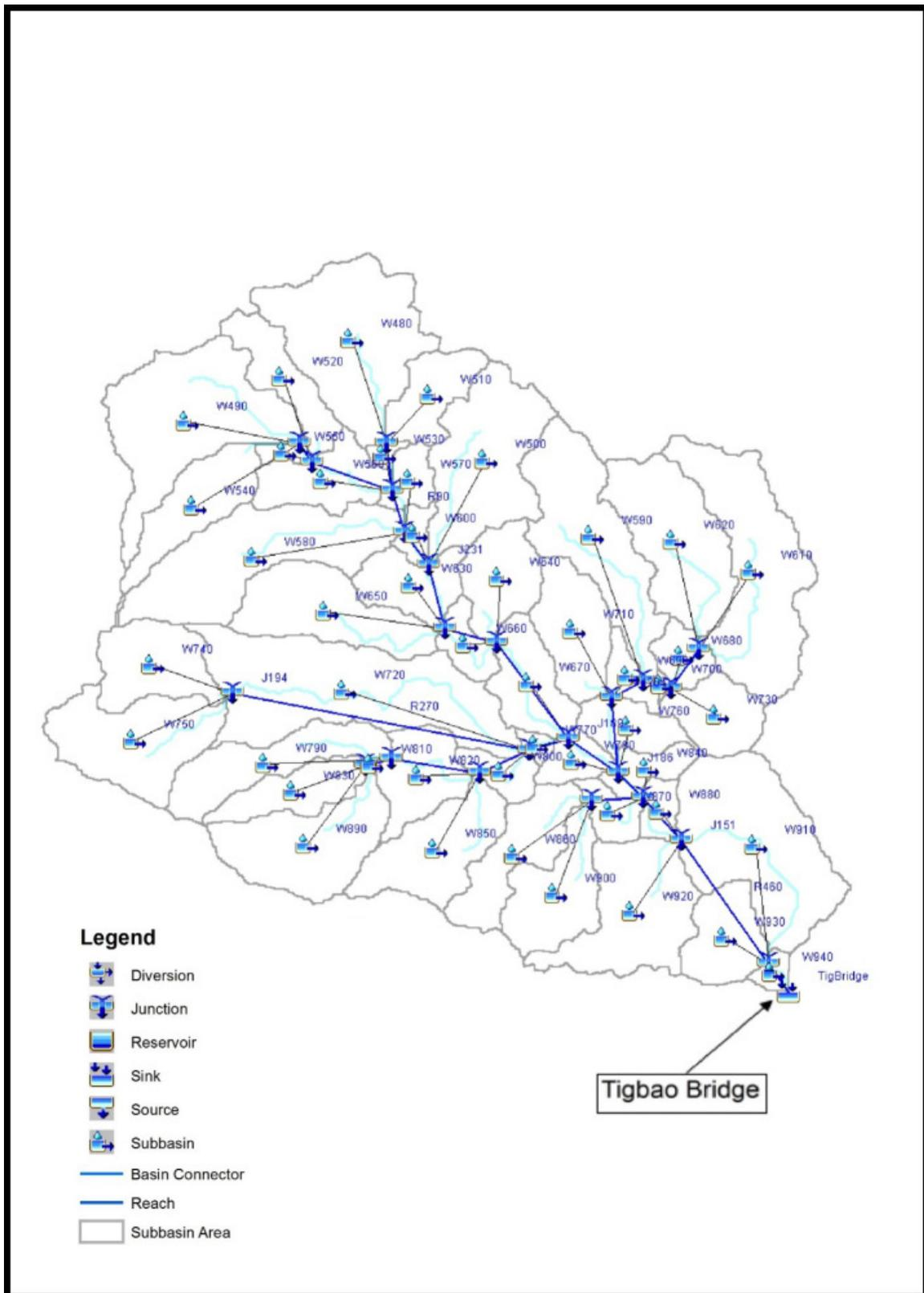
Figure 63. The Tigbao river basin model generated using HEC-HMS
