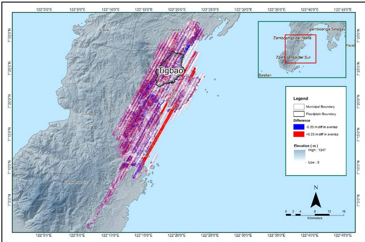
Figure 17. Elevation difference map between flight lines for Tigbao Floodplain.
