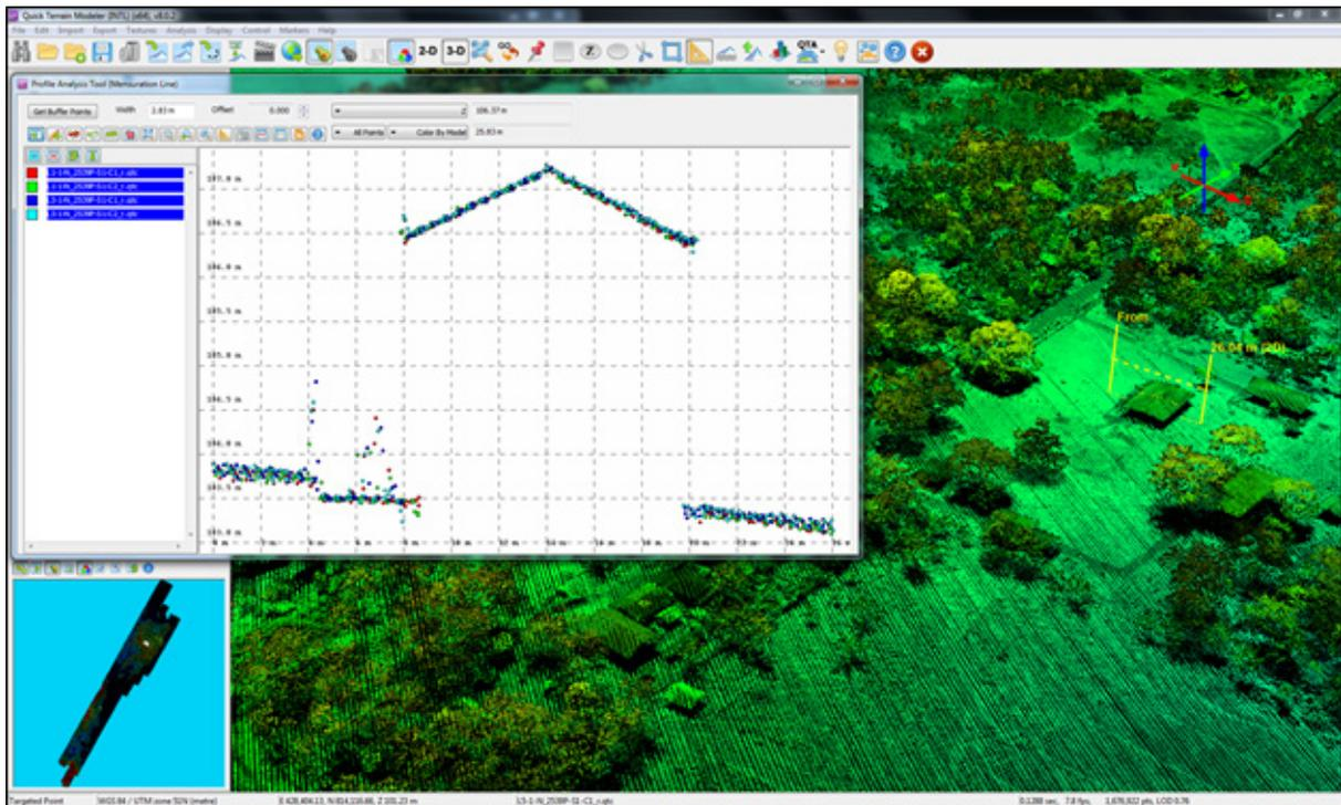
Figure 18. Quality checking for a Vitali flight 2539P using the Profile Tool of QT Modeler.
