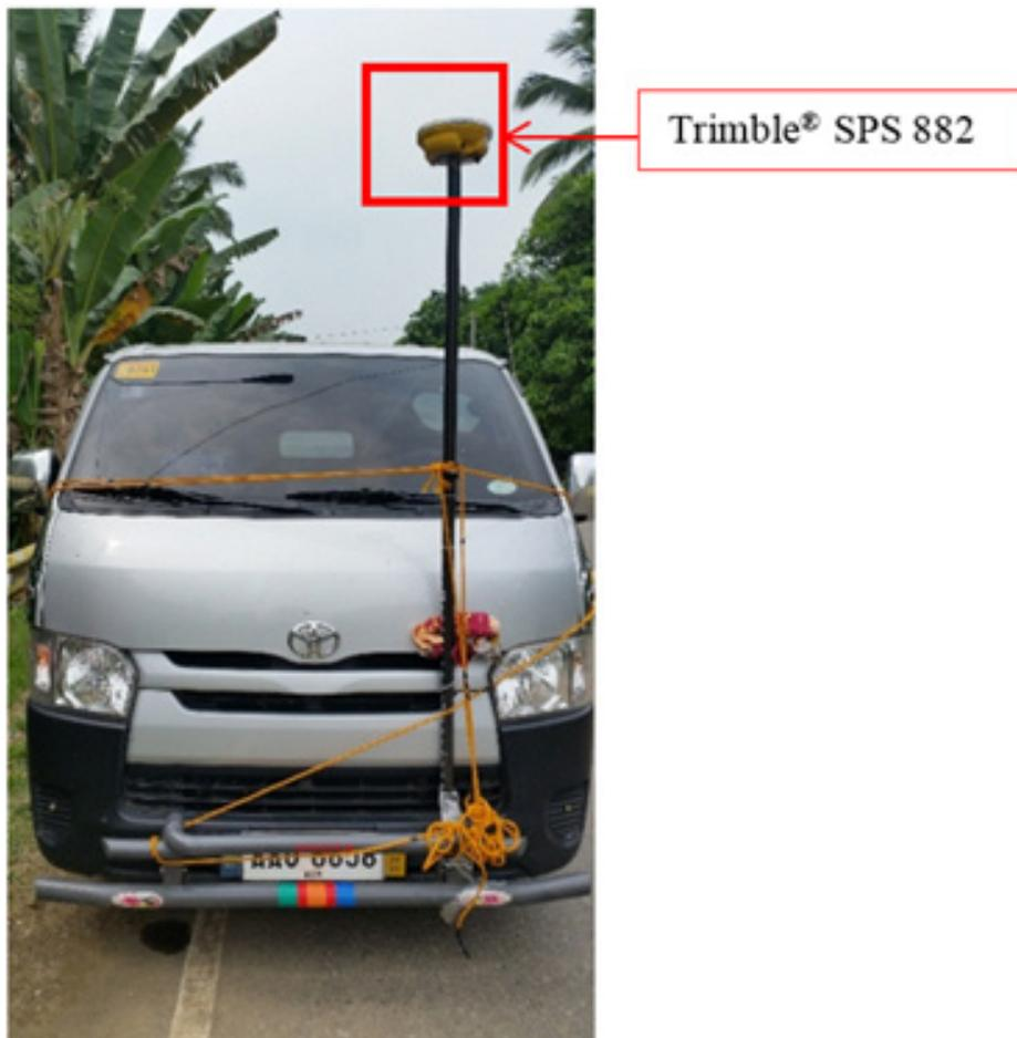
Figure 47. Trimble® SPS 882 set-up for validation points acquisition survey.
