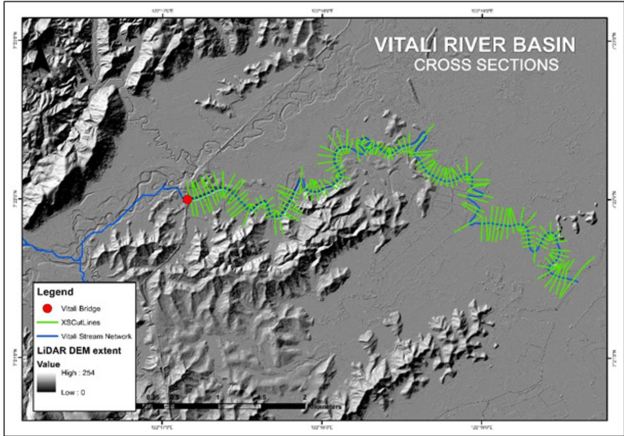
Figure 63. River cross-section of Vitali River generated through Arcmap HEC GeoRAS tool
