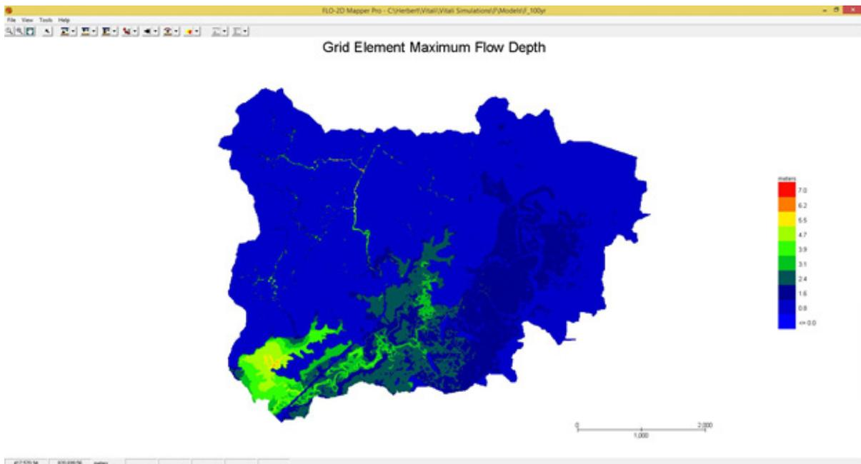
Figure 66. Generated 100-year rain return flow depth map from FLO-2D Mapper.
