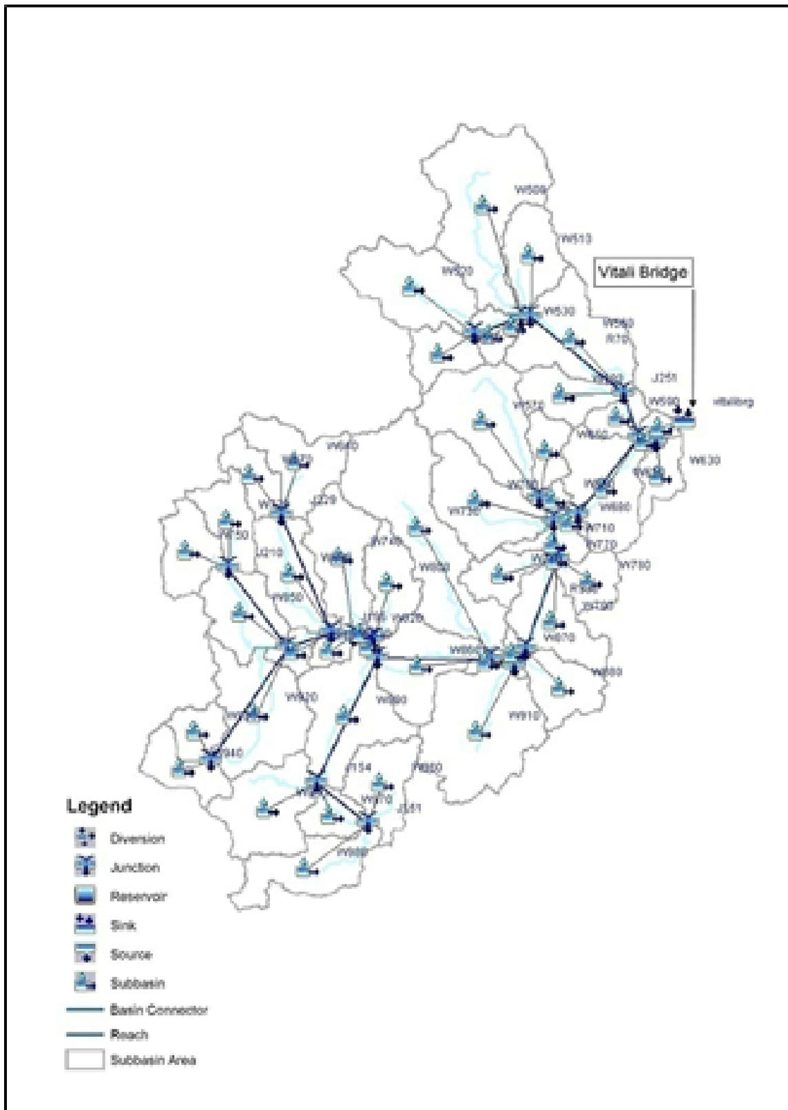
Figure 62. The Vitali river basin model generated using HEC-HMS
