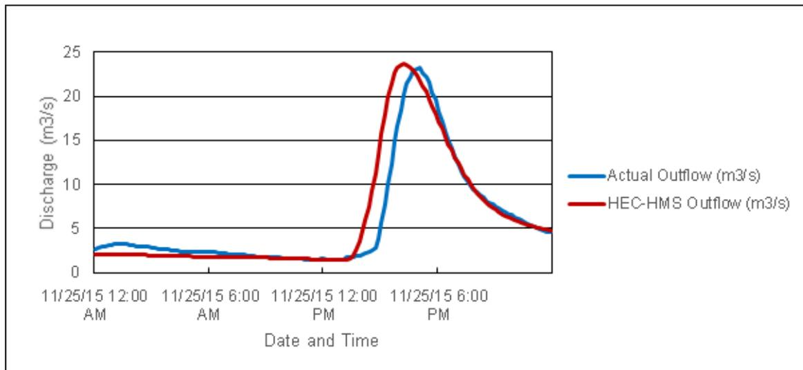
Figure 67. Outflow Hydrograph of Vitali produced by the HEC-HMS model compared with observed outflow.
