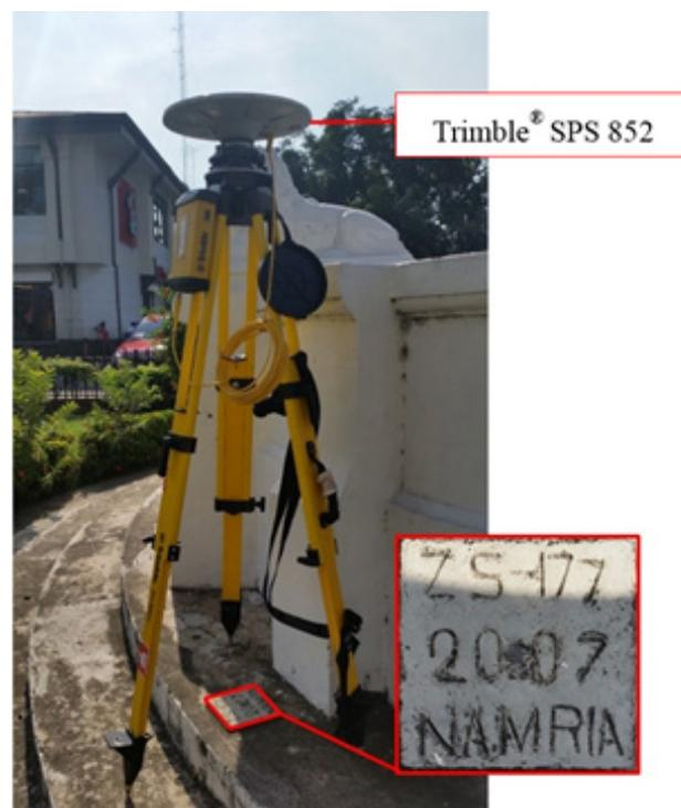
Figure 35. Trimble® SPS 852 set-up at ZS-177 located at the stair of Rizal's Park in Brgy. Poblacion, Zamboanga City
