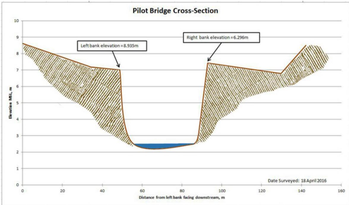
Figure 53. Cross-Section Plot of Vitali Bridge.
