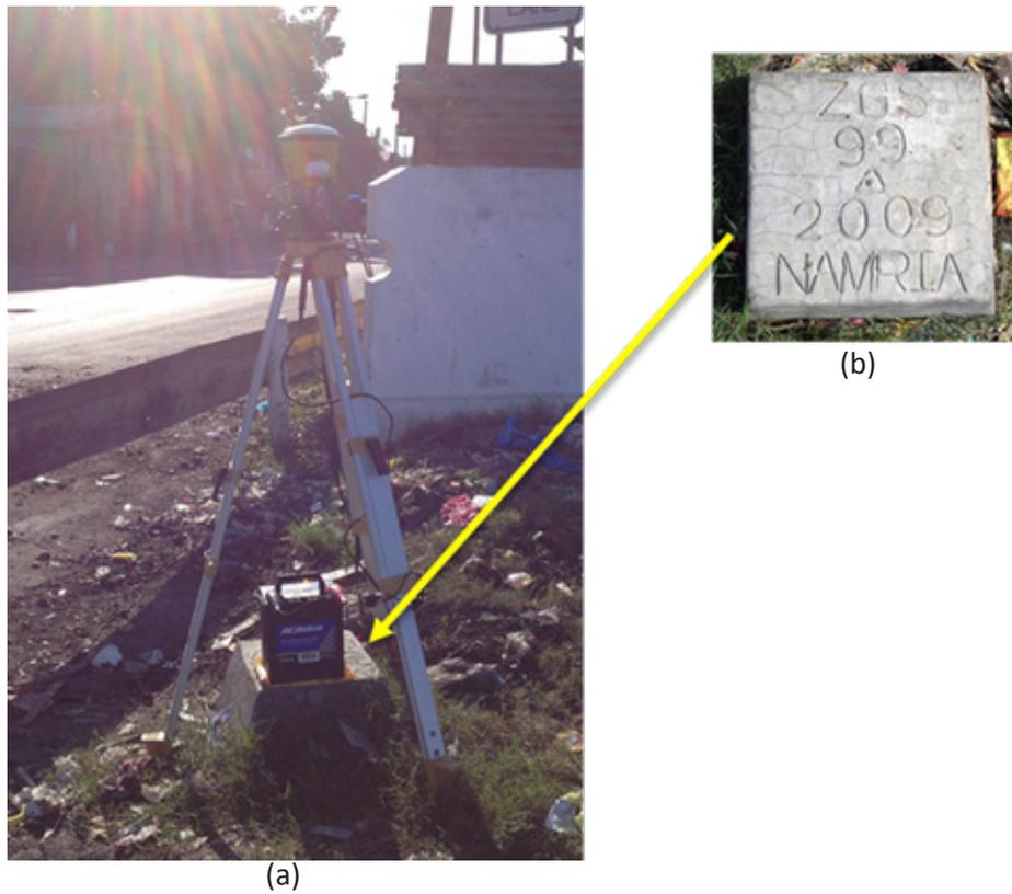
Figure 6. GPS set-up over ZGS-99 beside the seawall in Calarian, Zamboanga City (a) and NAMRIA reference point (b) as recovered by the field team.
