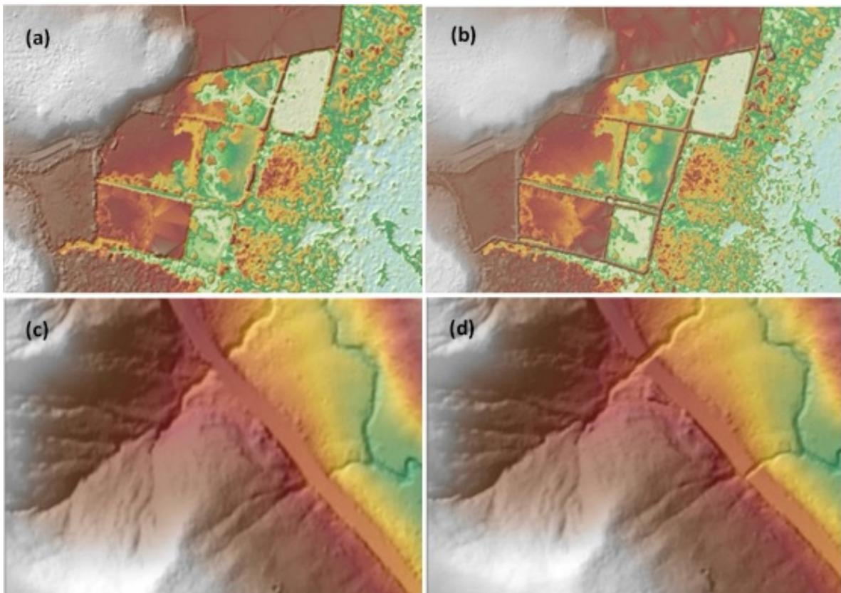
Figure 24. Portions in the DTM of Vitali floodplain – a paddy field before (a) and after (b) data retrieval; a road before (c) and after (d) manual editing.
