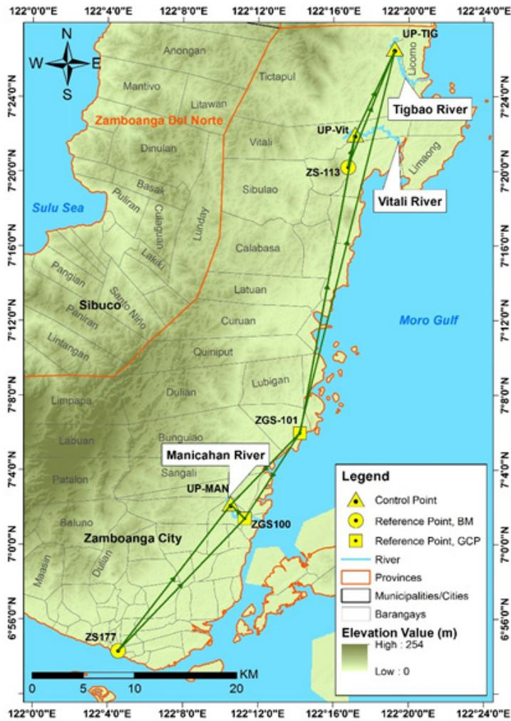
Figure 33. GNSS Network of Zamboanga City Field Survey.
