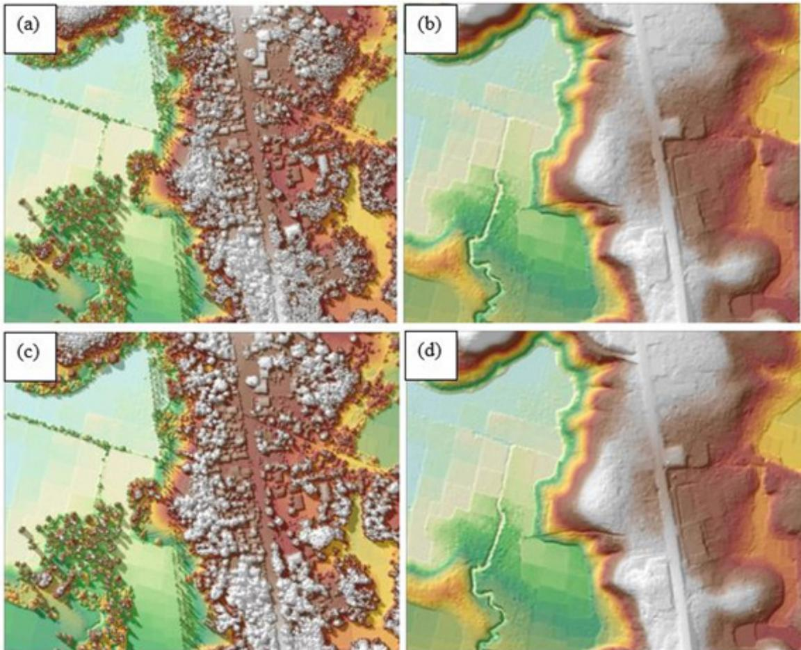
Figure 21. The production of last return DSM (a) and DTM (b), first return DSM (c) and secondary DTM (d) in some portion of Vitali floodplain.
