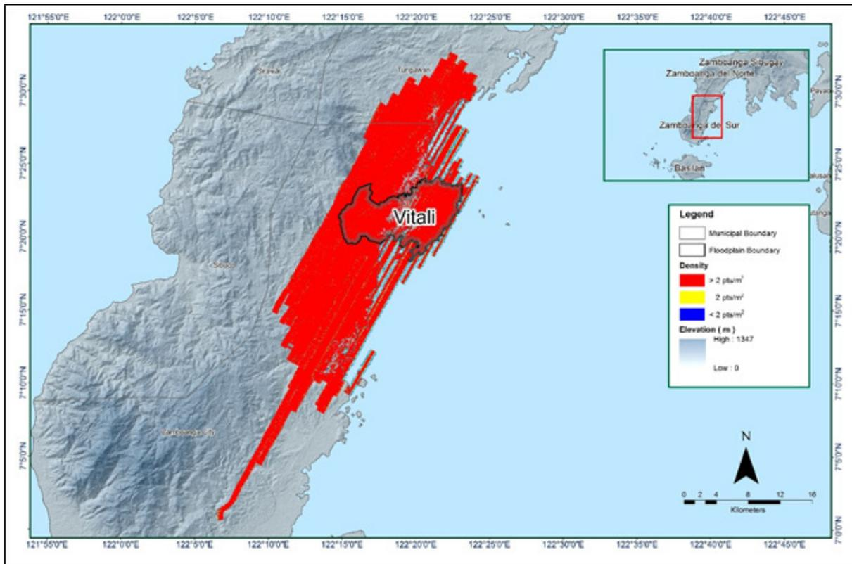
Figure 16. Density map of merged LiDAR data for Vitali floodplain.
