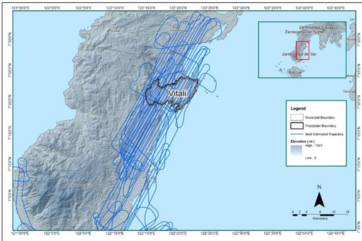
Figure 13. Best estimated trajectory of the LiDAR missions conducted over the Vitali floodplain.
