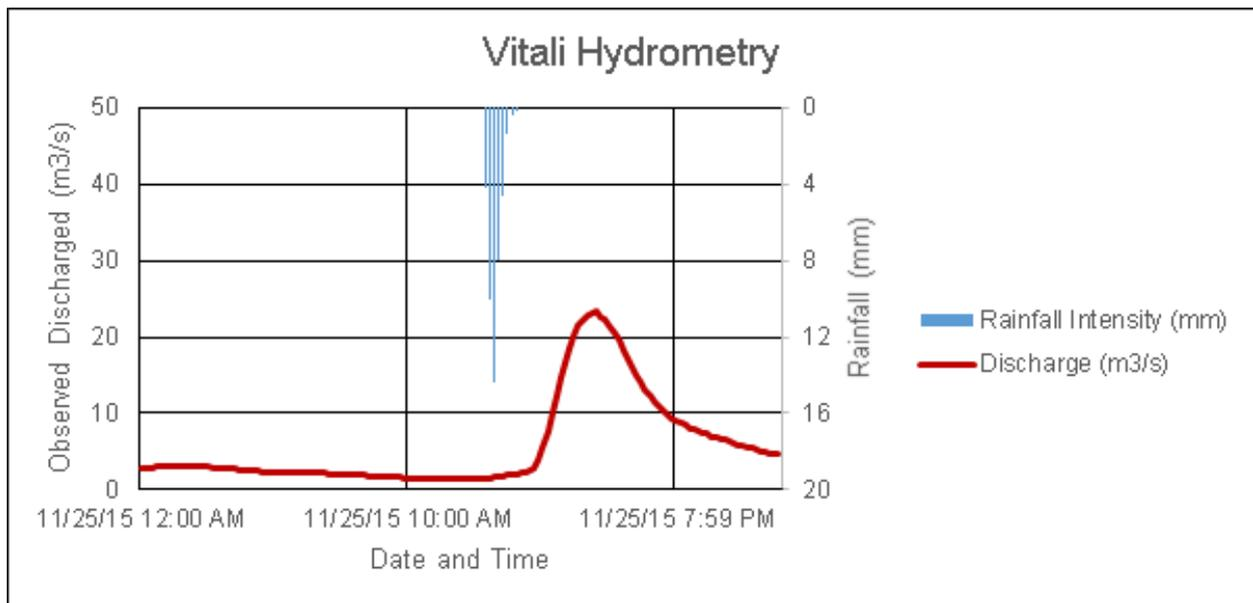
Figure 55. Rainfall and outflow data at Vitali Bridge used for modeling
