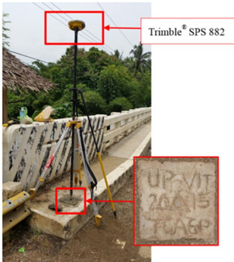
Figure 40. Trimble® SPS 882 set-up at UP-VIT located at the approach of Vitali Bridge in Brgy. Vitali, Zamboanga City.
