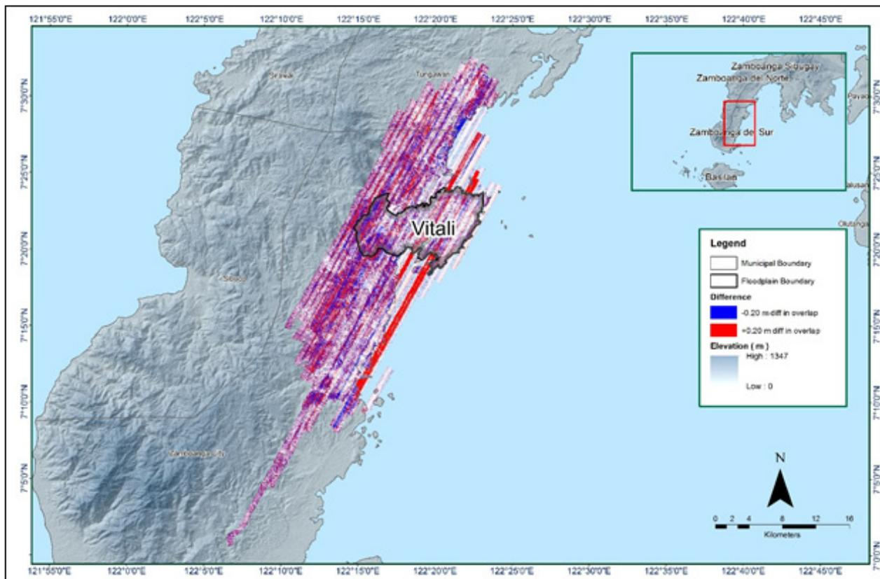
Figure 17. Elevation difference map between flight lines for Vitali floodplain.
