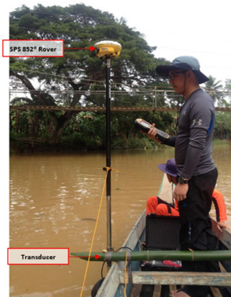
Figure 49. Bathymetry survey for Vitali River.
