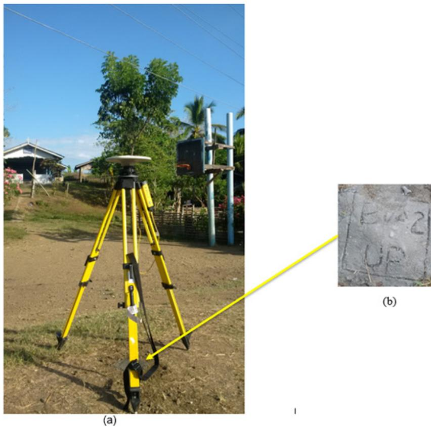
Figure 8. GPS set-up over BVA-2 established in Brgy. Buenavista, Zamboanga City (a) and Reference point BVA-2 (b) as established by the field team.
