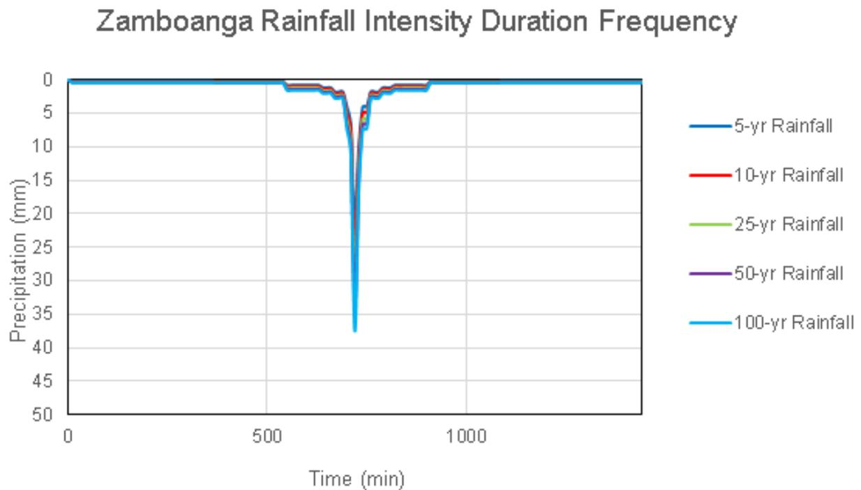
Figure 57. Synthetic storm generated for a 24-hr period rainfall for various return periods
