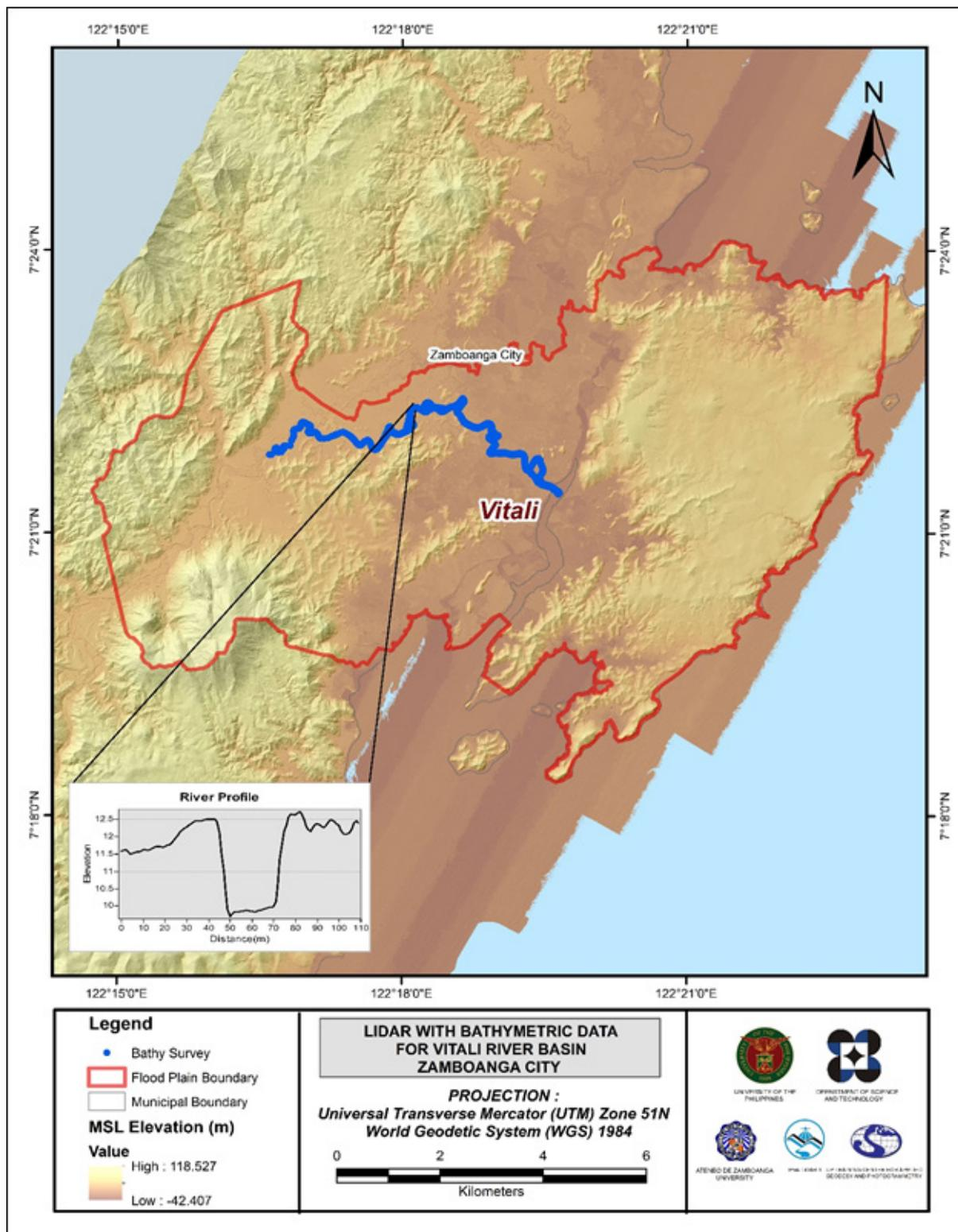
Figure 29. Extend of the bathymetric survey (in blue line) in Vitali River.
