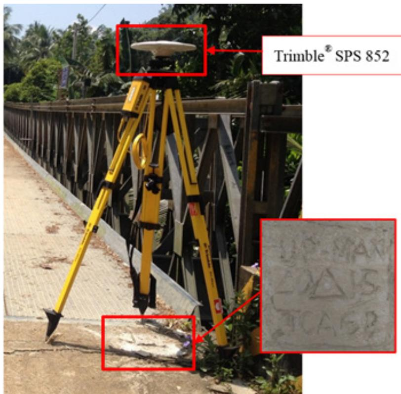
Figure 38. Trimble SPS® 852 set-up at UP-MAN located at the approach of Manicahan Steel Bridge in Brgy. Cacap, Zamboanga City.
