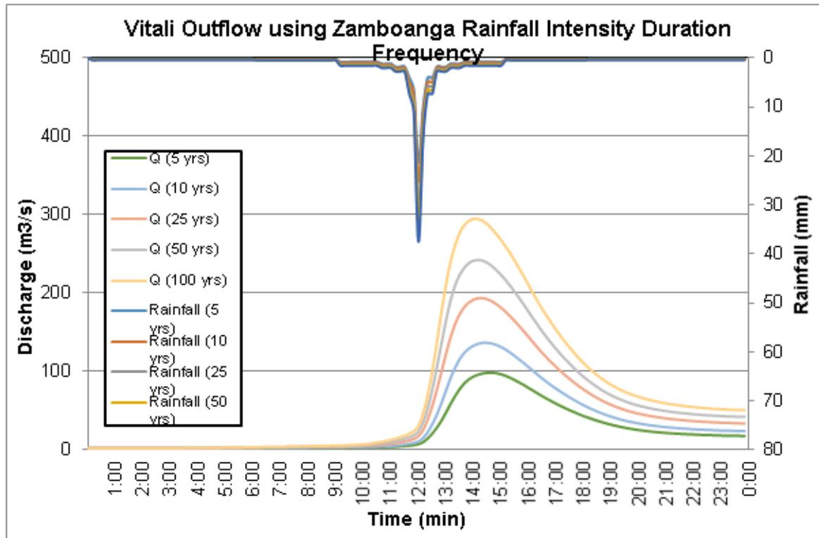
Figure 68. .Outflow hydrograph at Vitali Bridge Station generated using Zamboanga City RIDF simulated in HEC-HMS
