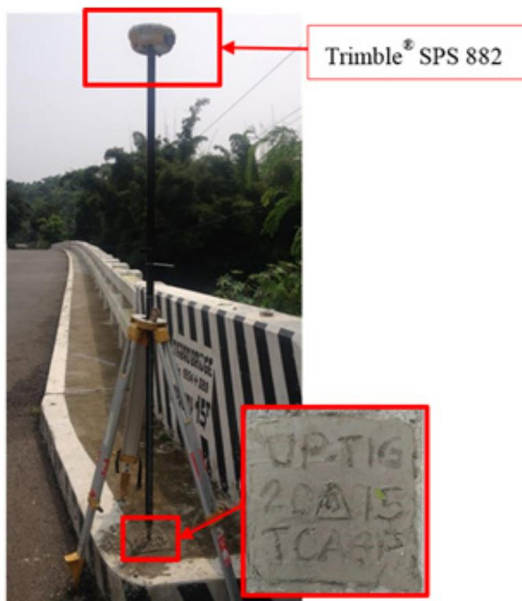
Figure 39. Trimble SPS® 882 set-up at UP-TIG located at the approach of Tigbao Bridge in Brgy. Tictapul, Zamboanga City.
