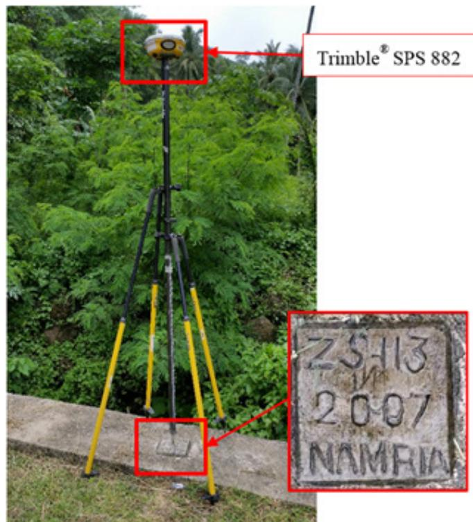
Figure 37. Trimble SPS® 882 set-up at ZS-113 located along Tagasilay-Vitali Road, Brgy. Tigbalabag, Zamboanga City.
