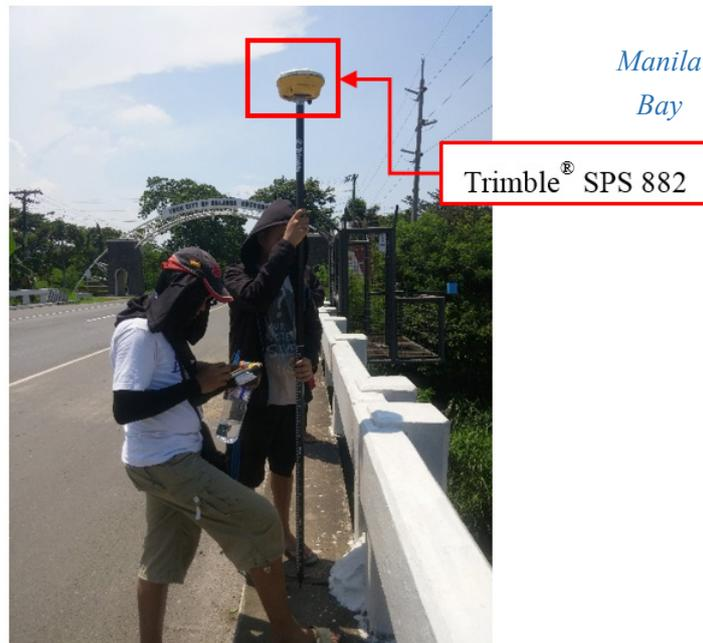
Figure 37. Bridge As-Built Survey using PPK Technique.
