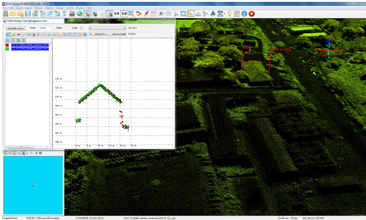
Figure 15. Quality checking for Balanga flight 2656G using the Profile Tool of QT Modeler.
