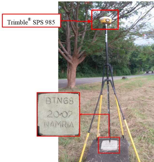
Figure 32. GNSS base set up, Trimble® SPS 882, at BTN-68, located just outside the Bataan Nuclear Power Plant along National High Way, Brgy. Nagbalayong, Municipality of Morong, Bataan
