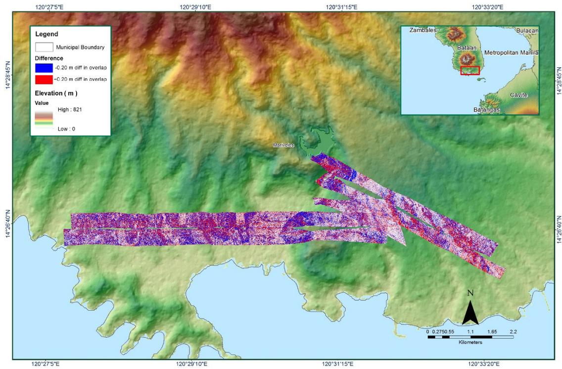
Figure 1.7.7 Elevation difference between flight lines
