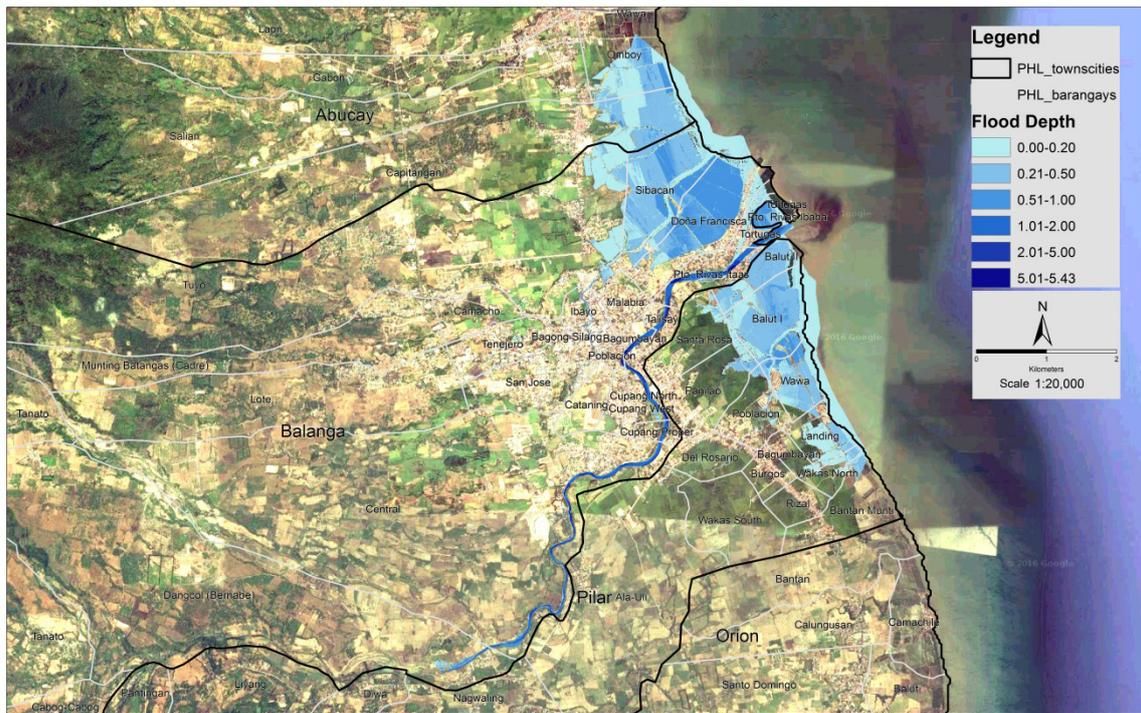
Figure 62. Sample output of Balanga RAS Model
