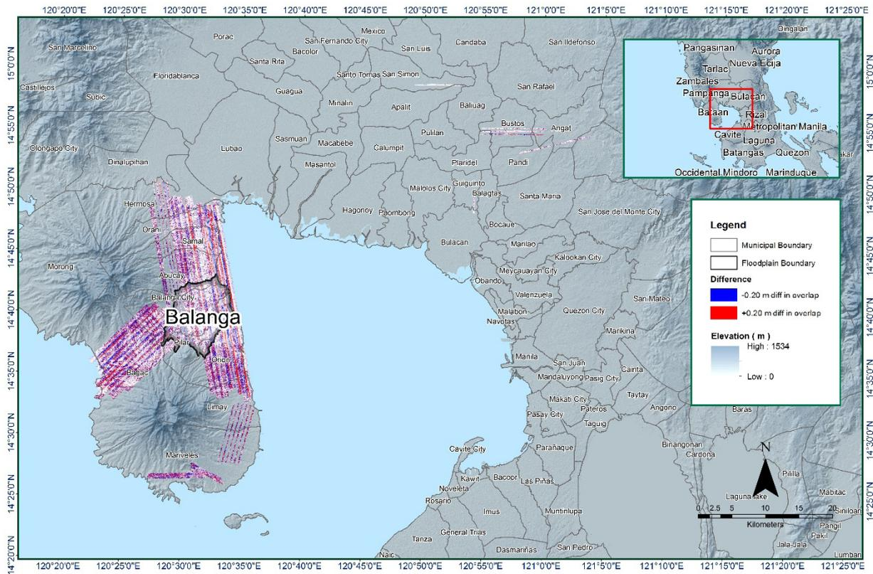
Figure 14. Elevation difference map between flight lines for Balanga floodplain.
