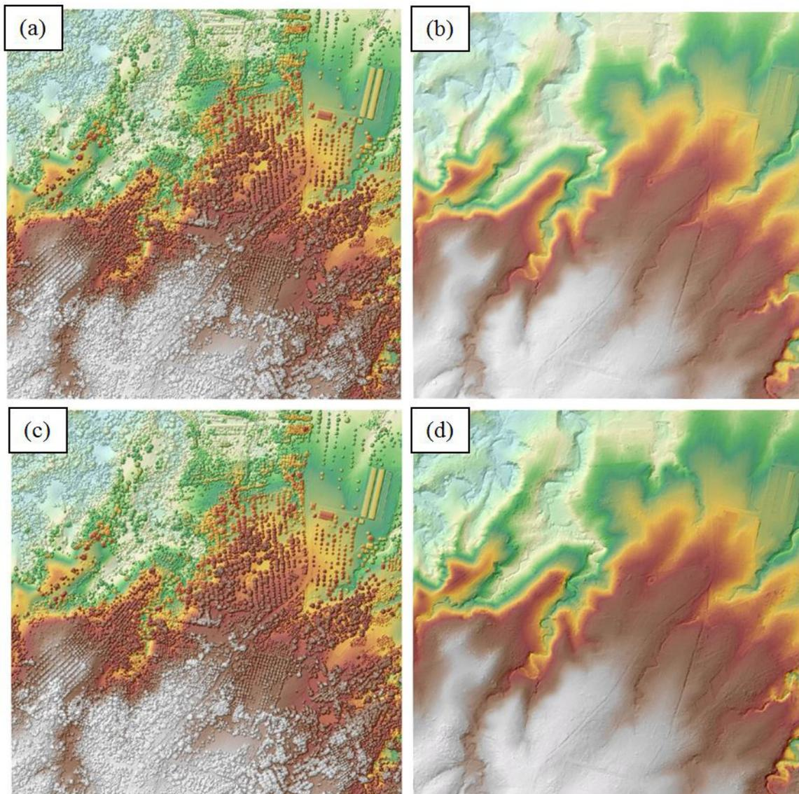
Figure 18. The production of last return DSM (a) and DTM (b), first return DSM (c) and secondary DTM (d) in some portion of Balanga floodplain.
