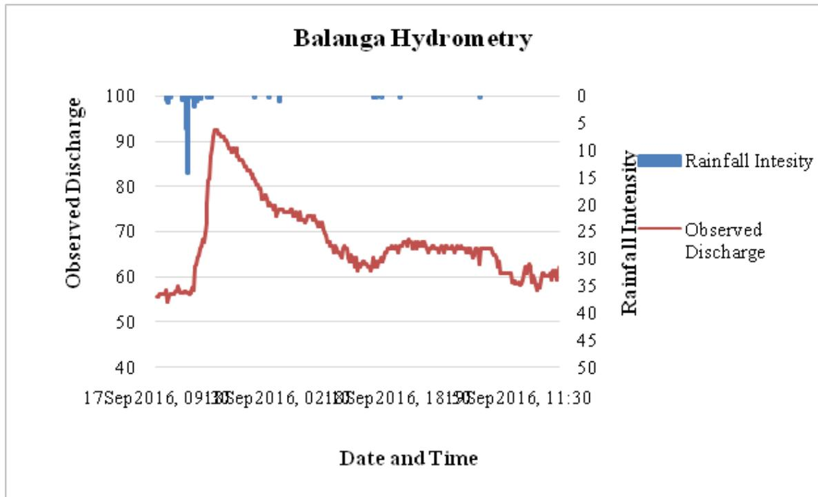
Figure 50. Rainfall and outflow data at Balanga used for modeling
