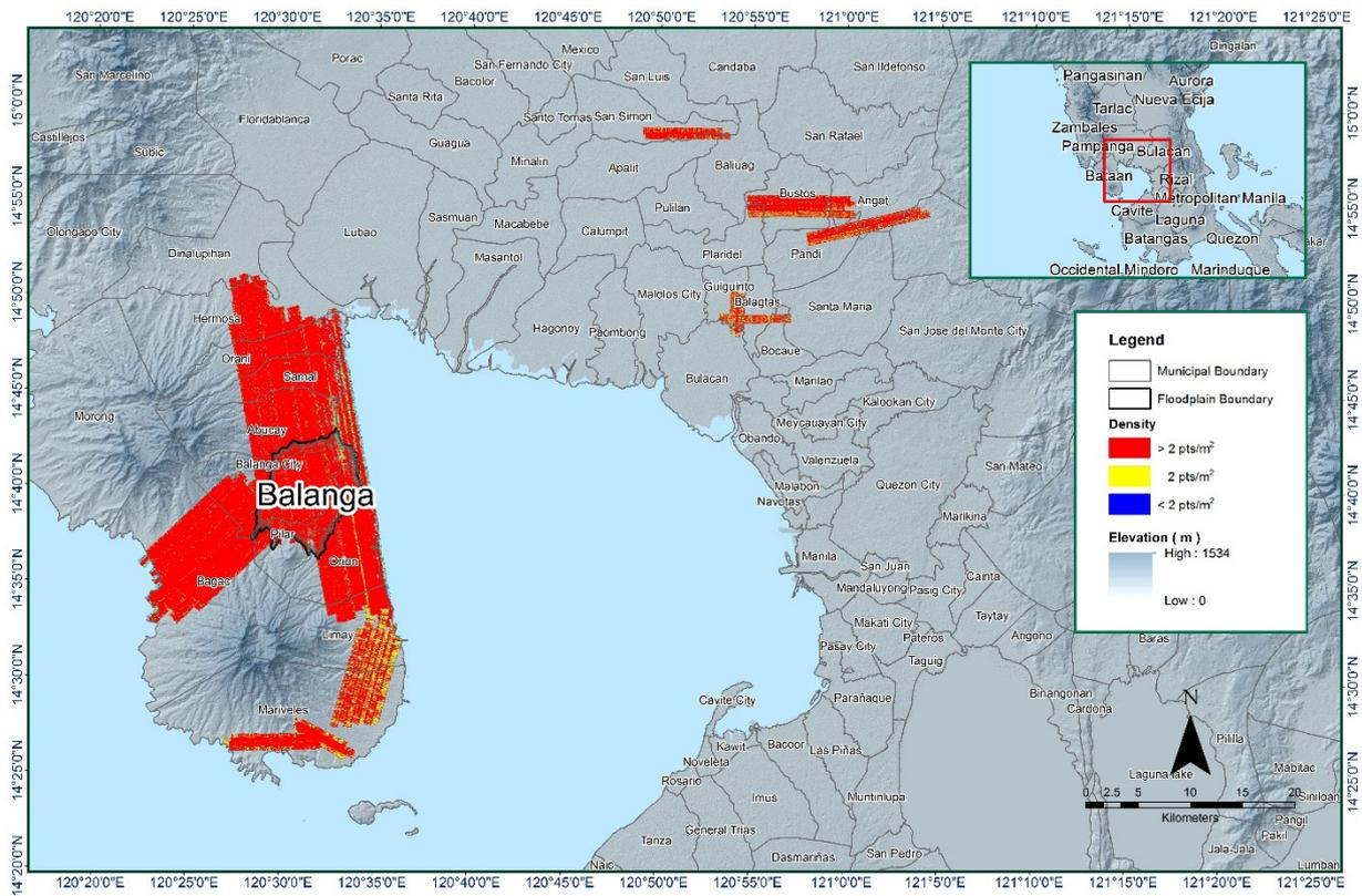
Figure 13. Pulse density map of merged LiDAR data for Balanga floodplain.
