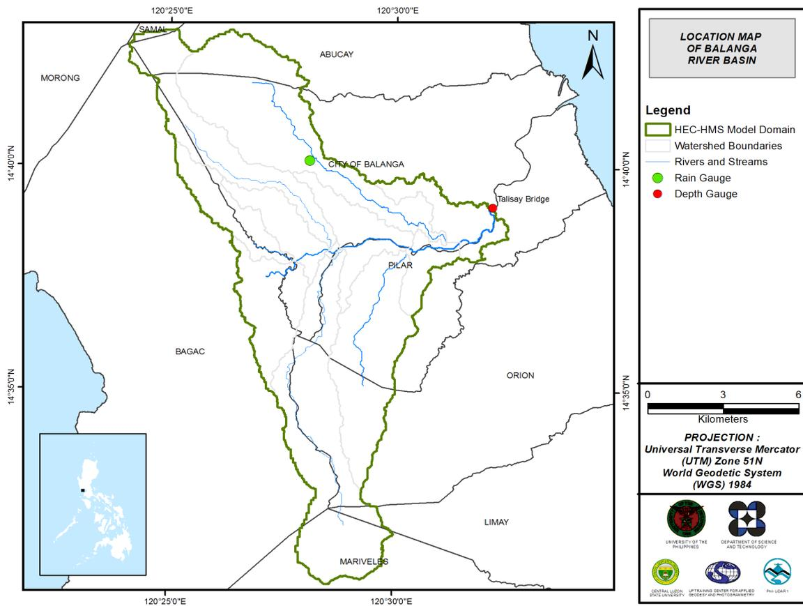
Figure 47. The location map of Balanga HEC-HMS model used for calibration.
