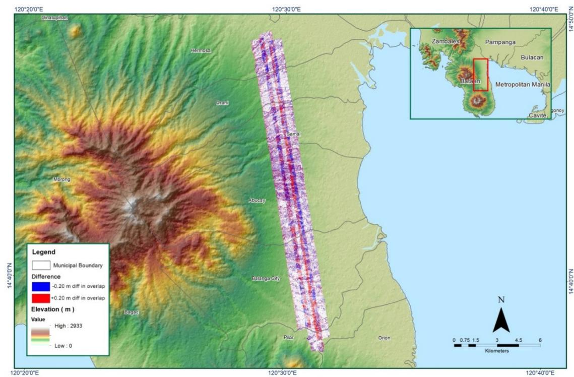
Figure 1.1.7. Elevation difference between flight lines
