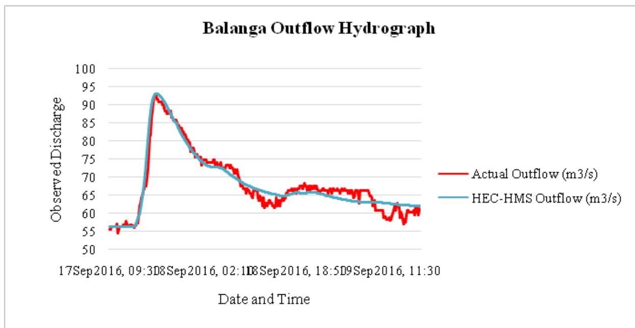
Figure 60. Outflow Hydrograph of Balanga produced by the HEC-HMS model compared with observed outflow
