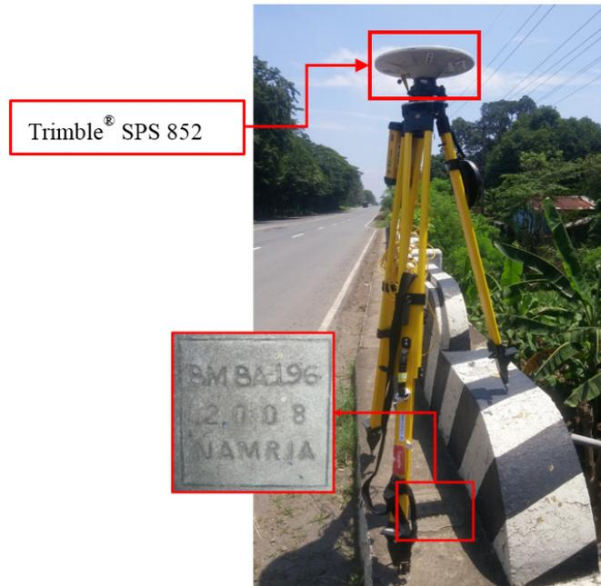
Figure 34. GNSS receiver setup, Trimble® SPS 852, at BA-196, located at the approach of Capitangan Bridge in Brgy. Capitangan, Municipality of Abucay, Bataan
