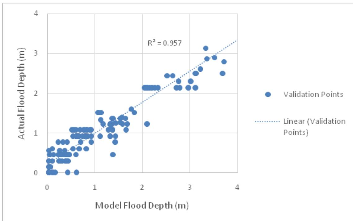
Figure 82. Model flood depth vs actual flood depth
