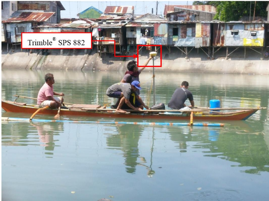
Figure 44. Bathymetric survey using Ohmex™ single beam echo sounder in Talisay River
