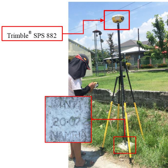
Figure 33. GNSS receiver setup, Trimble® SPS 882, at BTN-71, located at the middle of basketball court, Barangay Day Care Center and Barangay Chapel in Brgy. Apollo, Municipality of Orani, Bataan
