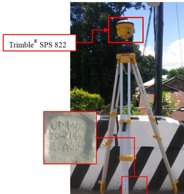
Figure 35. GNSS receiver setup, Trimble® SPS 985, at UP-MOR, located at the approach of Morong Bridge in Brgy. Poblacion, Municipality of Morong, Bataan
