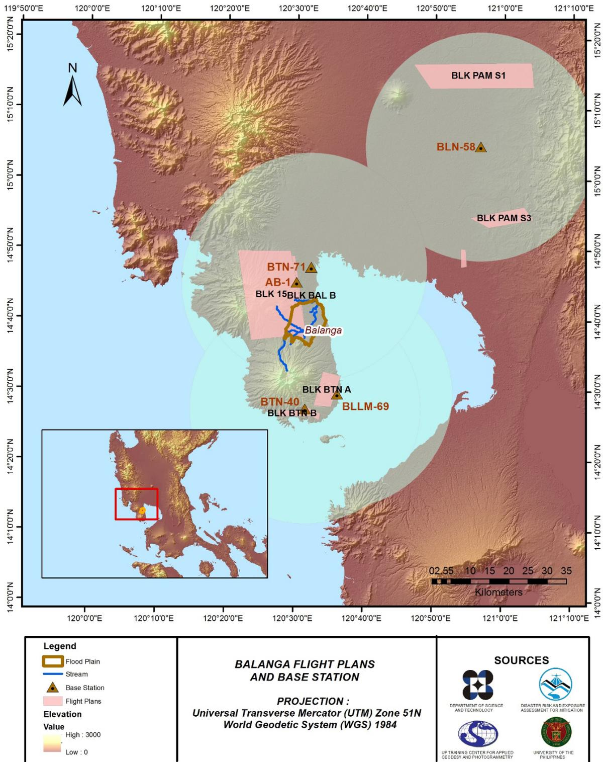
Figure 3. Flight plans and base stations used for Balanga floodplain using Gemini Sensor
