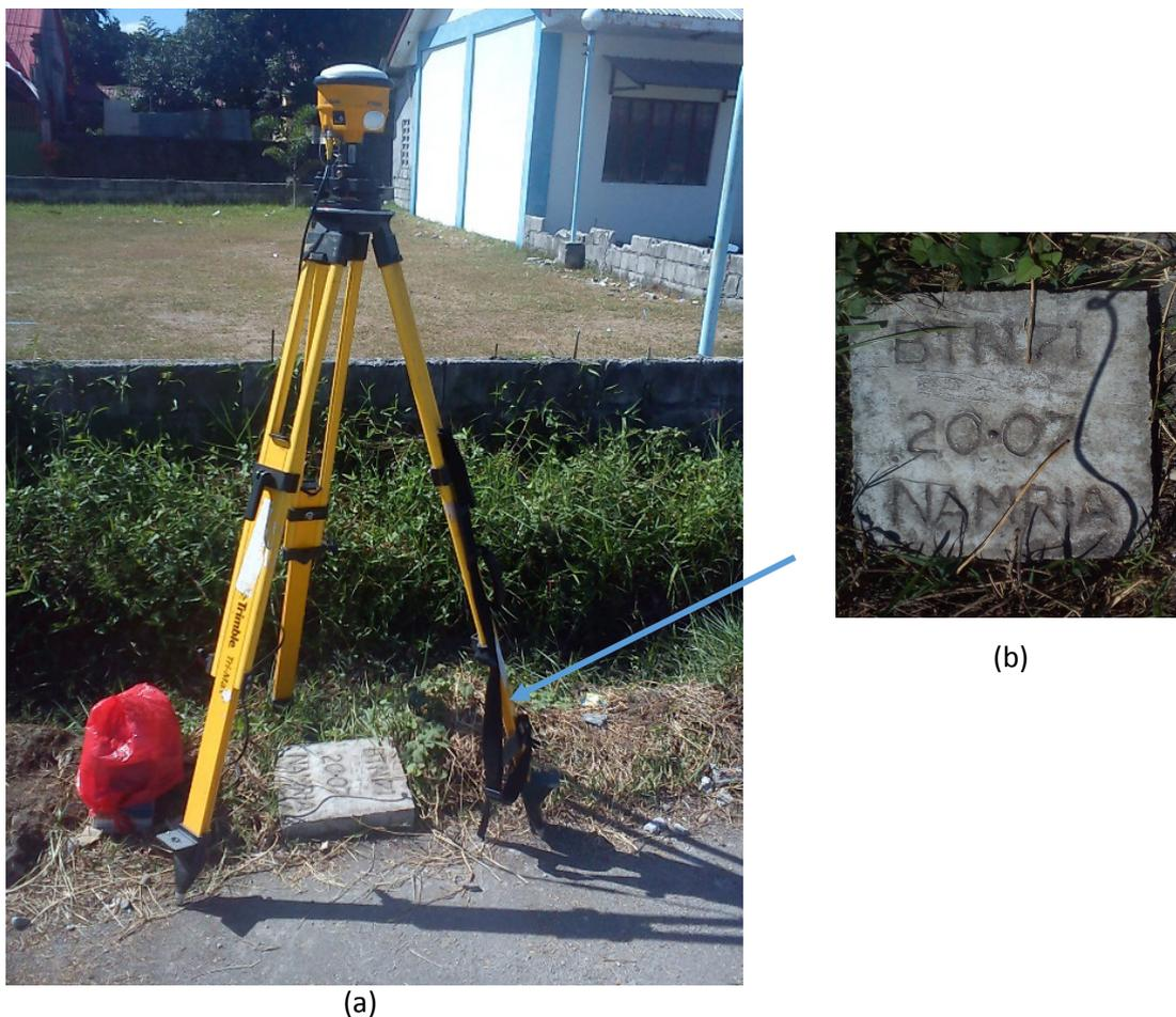
Figure 4. GPS set-up over BTN-71 located in Brgy. Maria Fe, Orani, 30 meters southwest of the Day Care Center, 20 meters southeast of the basketball court and 15 meters of the chapel (a) and NAMRIA reference point BTN-71 (b) as recovered by the field team.
