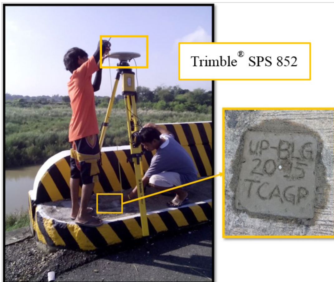
Figure 36. GNSS base receiver setup, Trimble® SPS 852 at UP-BLG at Baloling Bridge in Brgy. Poblacion Municipality of Mapandan, Pangasinan
