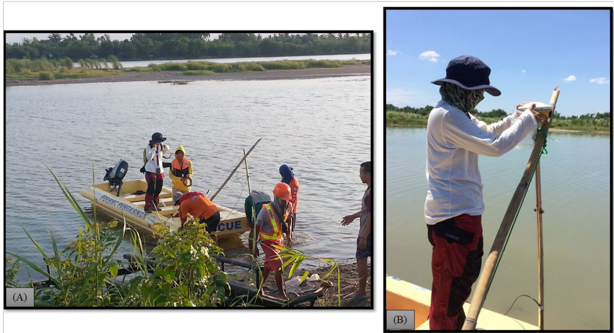
Figure 46. (A) Preparation for the bathymetric survey in Patalan River with assistance from the PDDRMO Pangasinan, and (B) set-up of the GNSS Trimble® SPS 882 attached to the rescue boat
