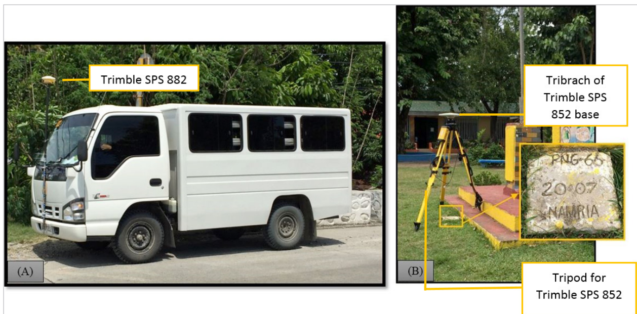
Figure 44. (A) Setup of Trimble® SPS 882 attached to a vehicle and (B) Setting up of GNSS base station at PNG-66
