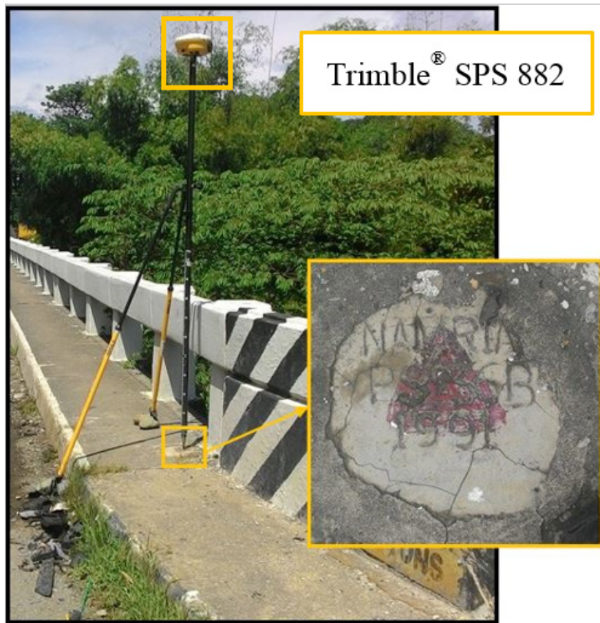
Figure 34. GNSS receiver setup, Trimble® SPS 882 at PS-36B at Villamil Bridge in Brgy. Catablan, Urdaneta City, Pangasinan
