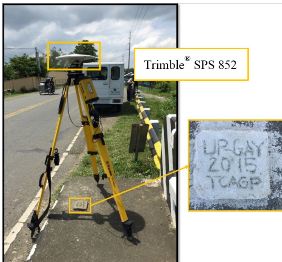
Figure 37. GNSS base receiver setup, Trimble® SPS 852 at UP-GAY at Gayaga Bridge in Brgy. Amandiego, Alaminos City, Pangasinan
