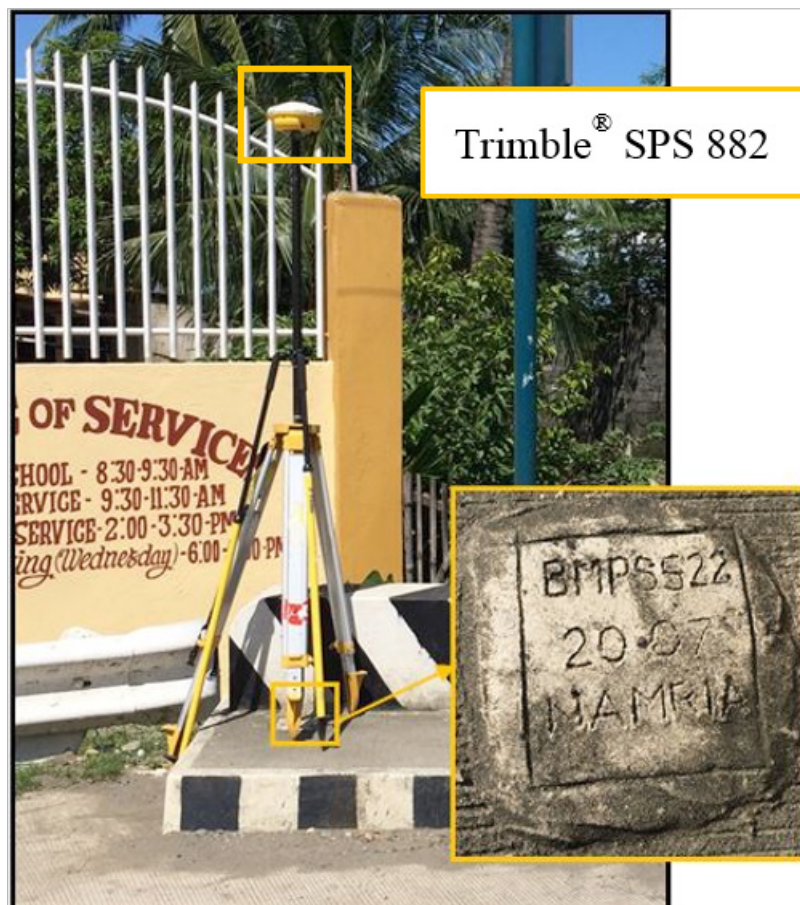
Figure 35. GNSS receiver occupation, Trimble® SPS 882 at PS-522 at Quartel Bridge in Brgy. Poblacion, Municipality of Sual, Pangasinan
