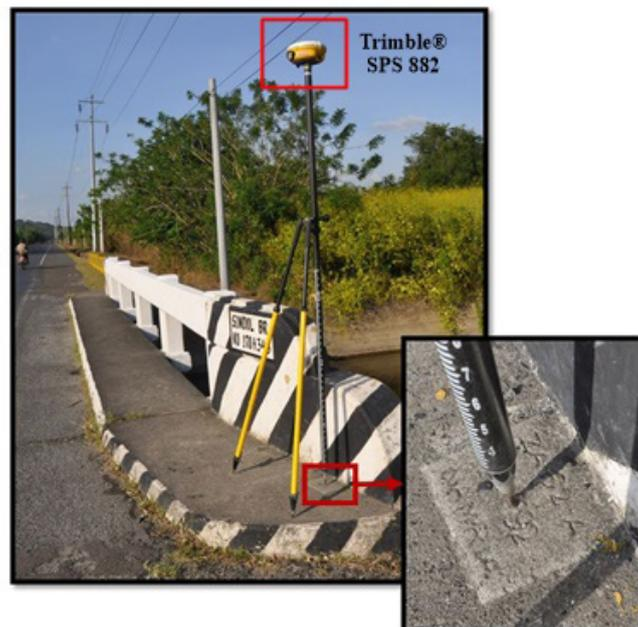
Figure 34. Trimble® SPS 882 occupying ZA-62A located at the approach of Sindol Bridge, Brgy. Sindol, Municipality of San Felipe, Zambales
