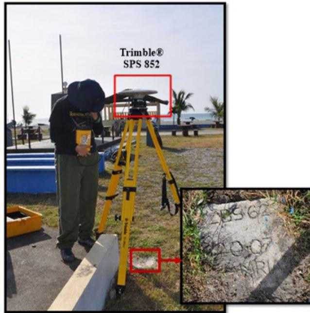
Figure 33. GNSS Base receiver, Trimble® SPS 852 set-up at ZBS-62, located inside Barangay Executive Park in Brgy. La Paz, Municipality of San Narciso, Zambales
