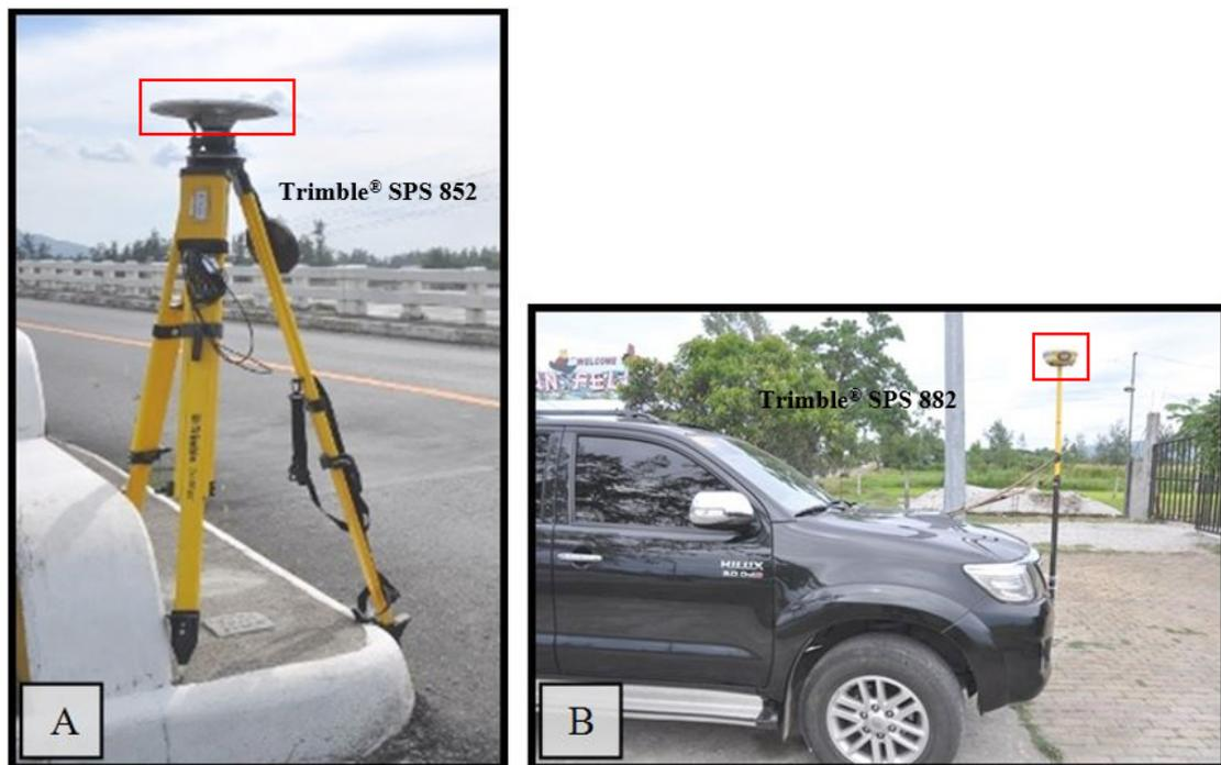
Figure 41. A) The occupied GNSS base station, UP-MAC, in Municipality of San Narciso with Trimble® SPS 852 and (B) the set-up of Trimble® SPS 882 in a vehicle for ground validation acquisition
