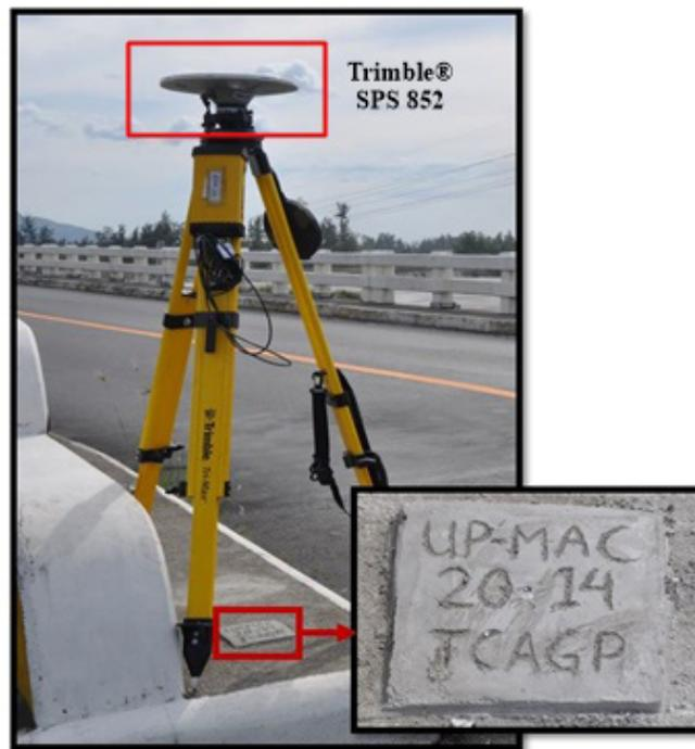
Figure 35. GNSS base receiver, Trimble® SPS 852 set-up at UP-MAC at the approach of Maculcol Bridge, in Brgy. Alusiss, Municipality of San Narciso, Zambales
