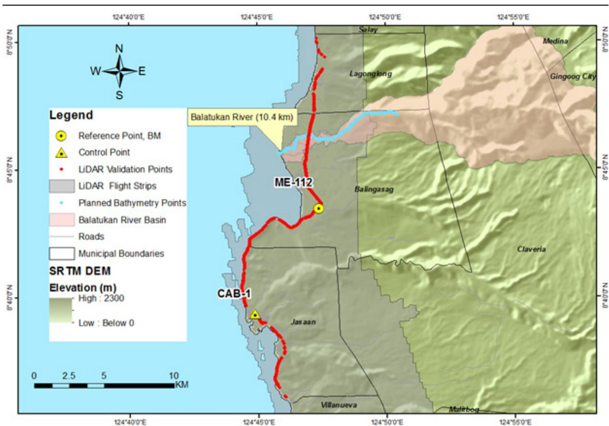
Figure 43. Validation points acquisition survey for Balatukan River.
