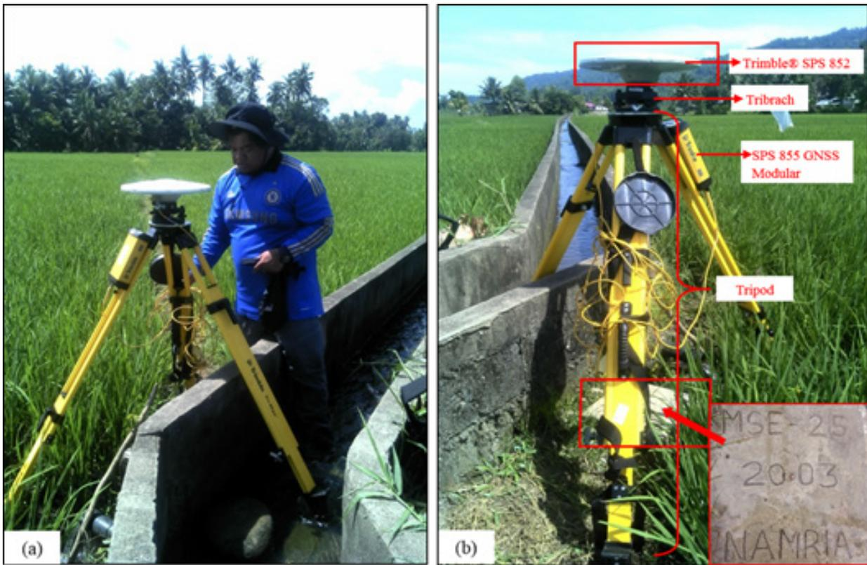
Figure 33. GNSS base receiver set-up, Trimble® SPS 852 at MSE-25 in Brgy. Poblacion 1, Municipality of Villanueva, Misamis Oriental.
