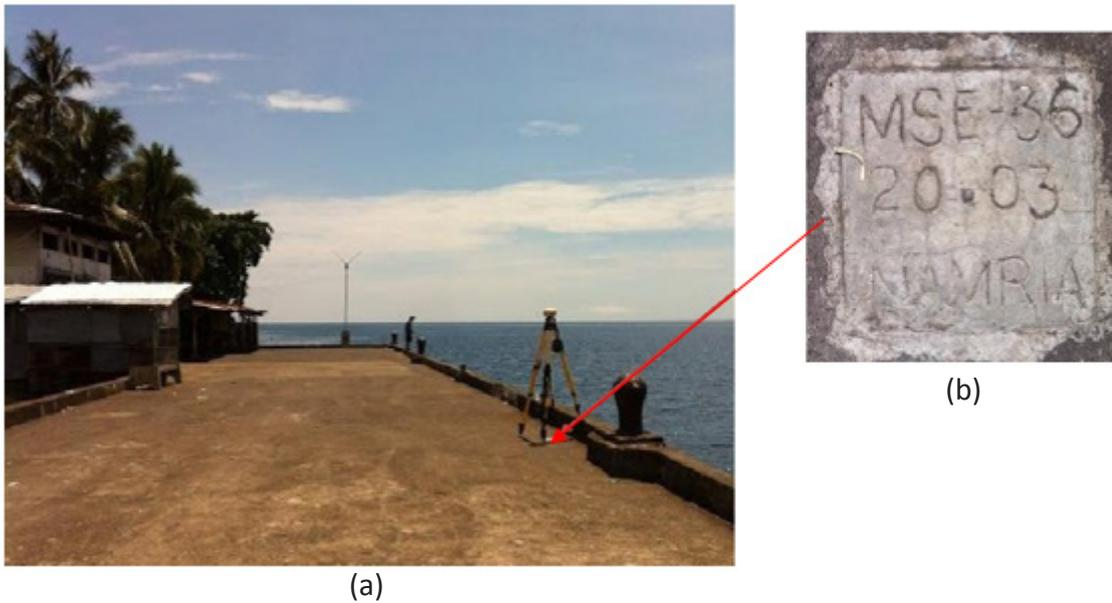
Figure 6. GPS set-up over MSE-36 within Medina municipal port (a) and NAMRIA reference point MSE-32 (b) as recovered by the field team.
