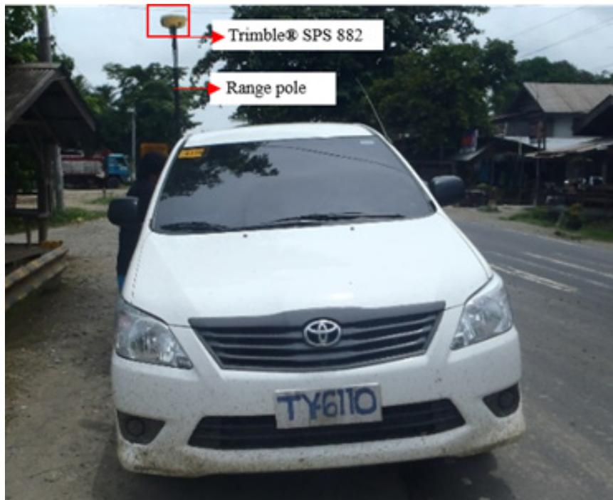
Figure 42. Validation points acquisition survey using Trimble® SPS 882.
