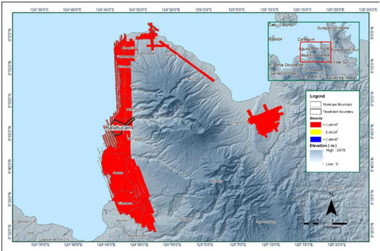
Figure 15. Pulse density map of merged LiDAR data for Balatucan Floodplain.
