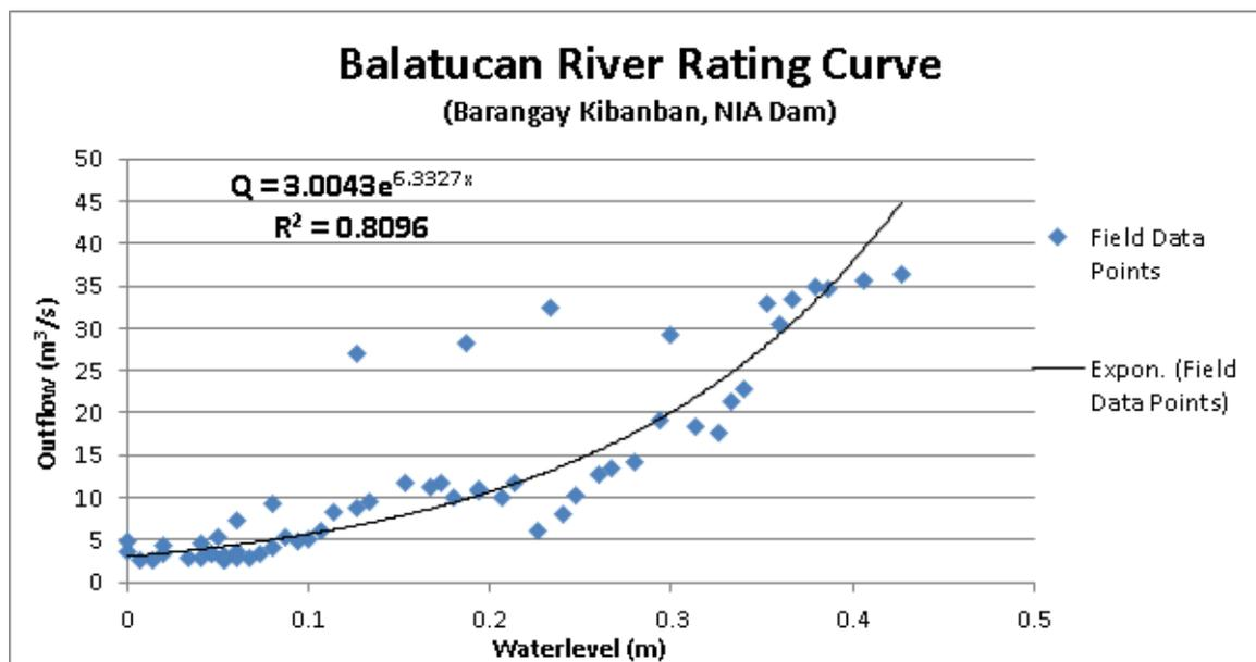
Figure 50. HQ curve of HEC-HMS model.
