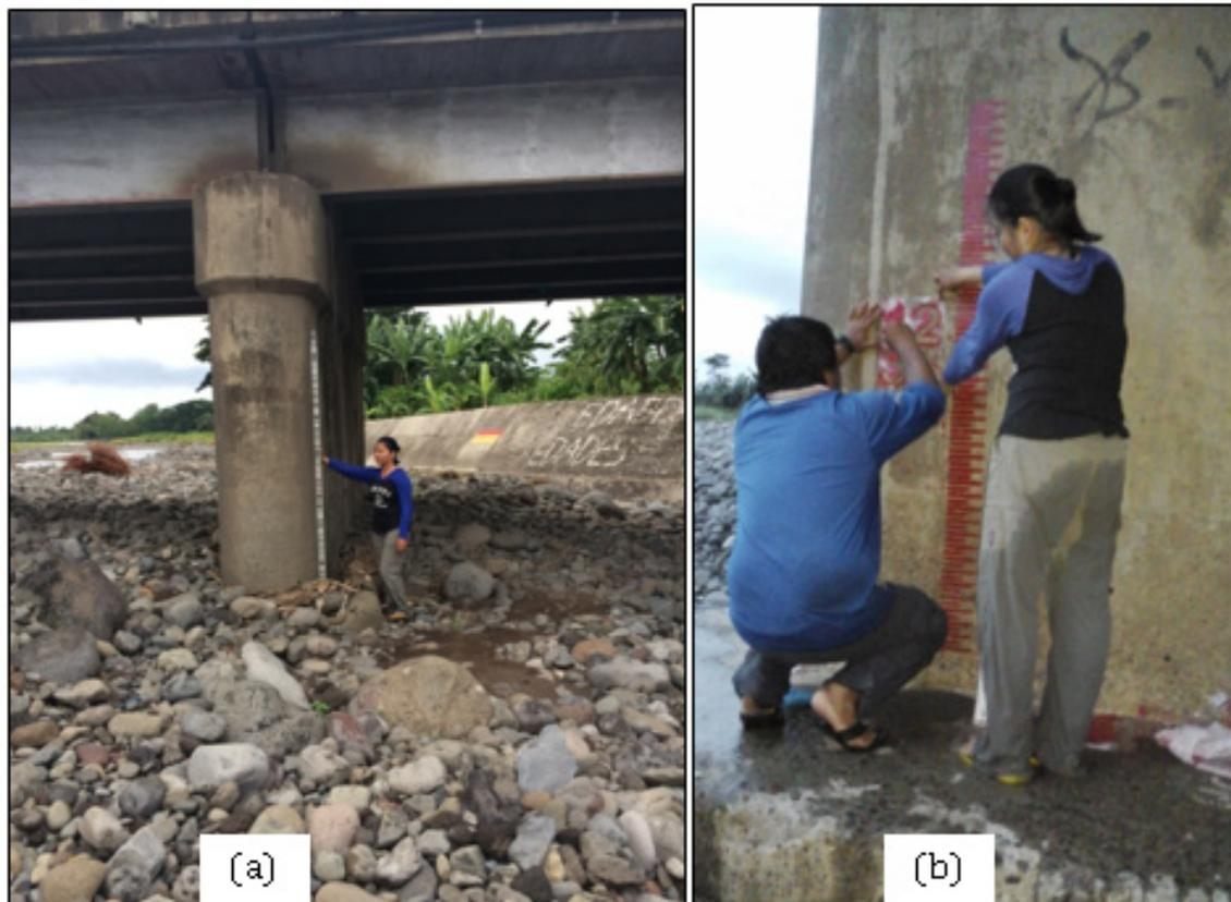
Figure 41. Water surface elevation marking on one of the bridge piers of Mambayan Bridge,
