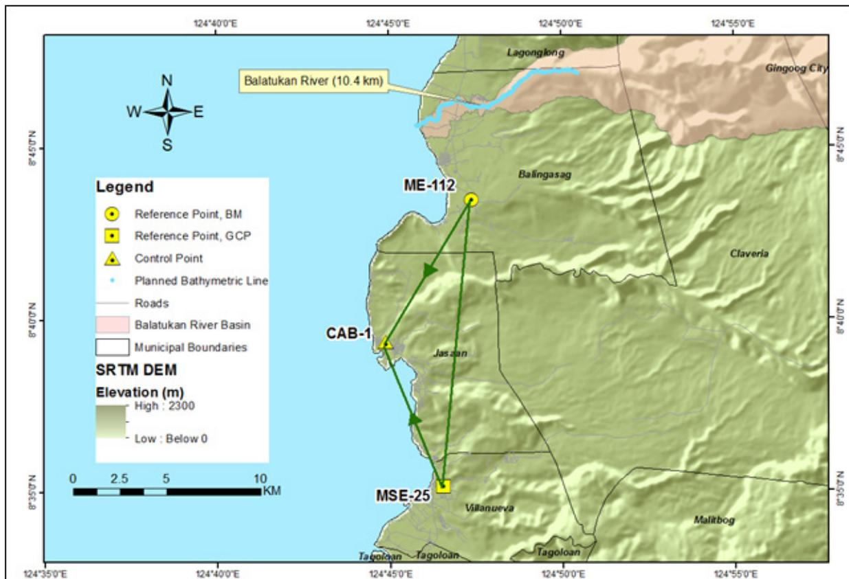
Figure 32. GNSS network covering the Balatukan River
