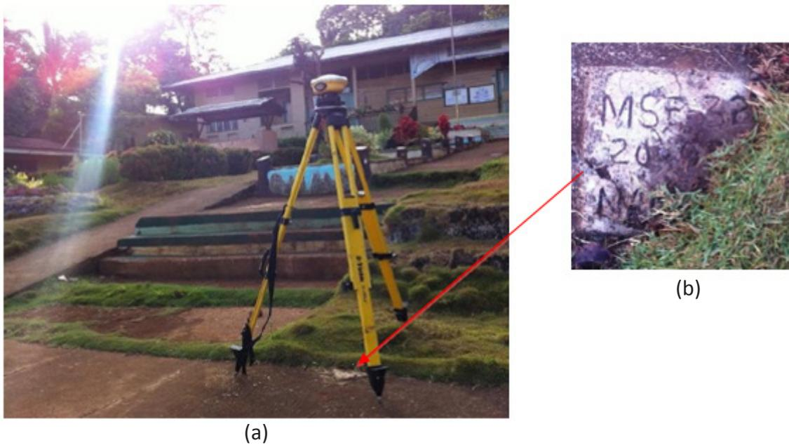
Figure 5. GPS set-up over MSE-32 inside Alicomohan Elementary school, just in front of the school’s flag pole, situated at Barangay Alicomohan, Sugbongcogon, Misamis Oriental (a) and NAMRIA reference point MSE-32 (b) as recovered by the field team.
