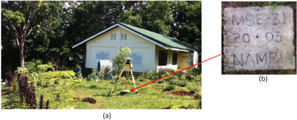
Figure 4. GPS set-up over MSE-31 inside the school grounds of Binuangan National High School of Sitio Naratulan, Binuangan, Misamis Oriental (a) and NAMRIA reference point MSE-31 (b) as recovered by the field team.
