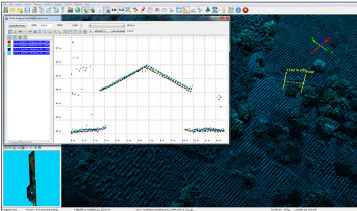
Figure 17. Quality checking for a Balatucan flight 1509P using the Profile Tool of QT Modeler.
