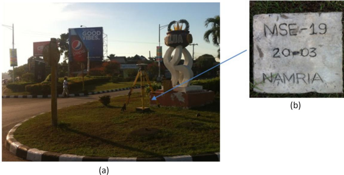
Figure 3. GPS set-up over MSE-19 at the center island located at the road intersections going to Cagayan de Oro, Butuan City and Iligan City (a) and NAMRIA reference point MSE-16 (b) as recovered by the field team.
