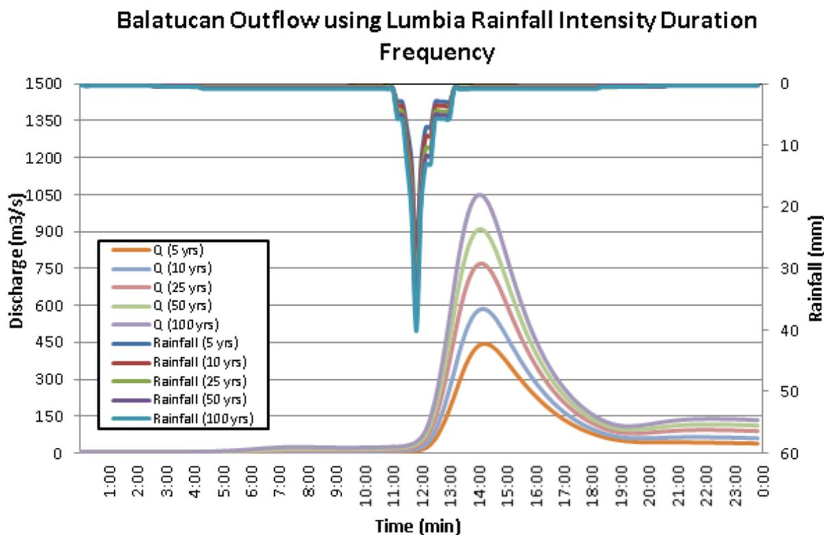
Figure 61. Outflow hydrograph at Balatucan Station generated using Lumbia RIDF simulated in HEC-HMS.
