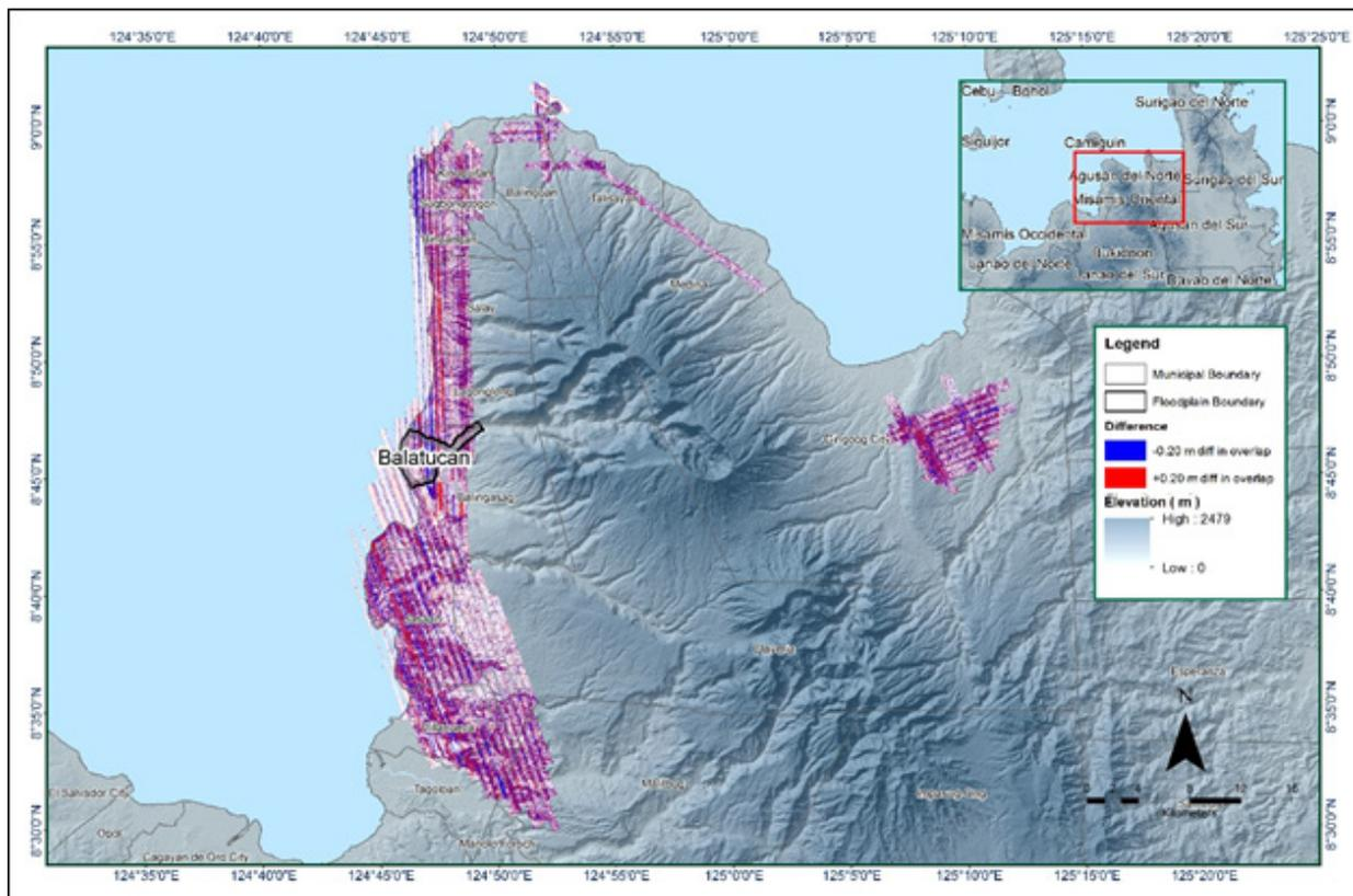
Figure 16. Elevation difference map between flight lines for Balatucan Floodplain
