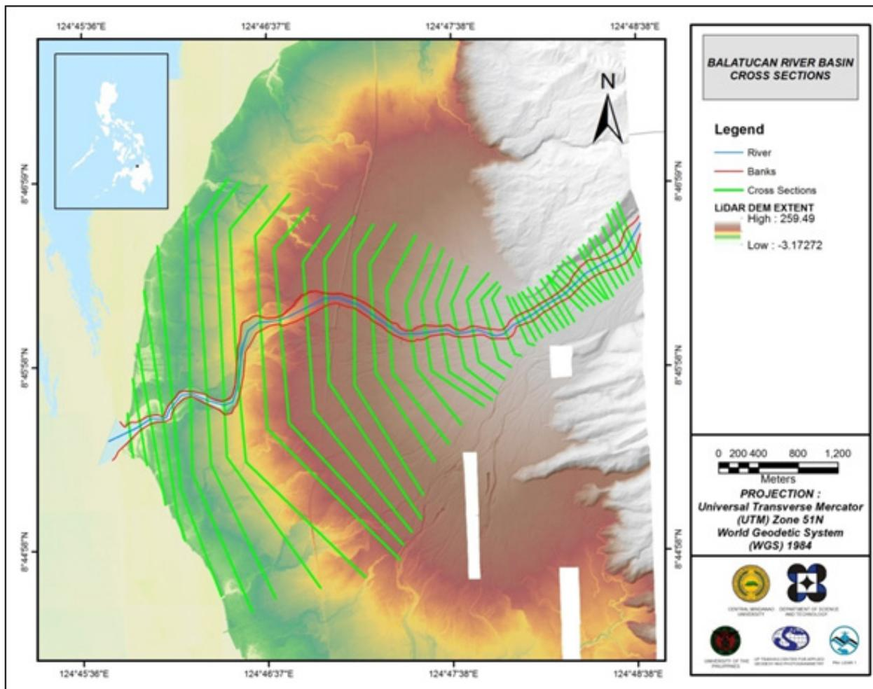
Figure 58. River cross-section of Balatucan River generated through Arcmap HEC GeoRAS tool.
