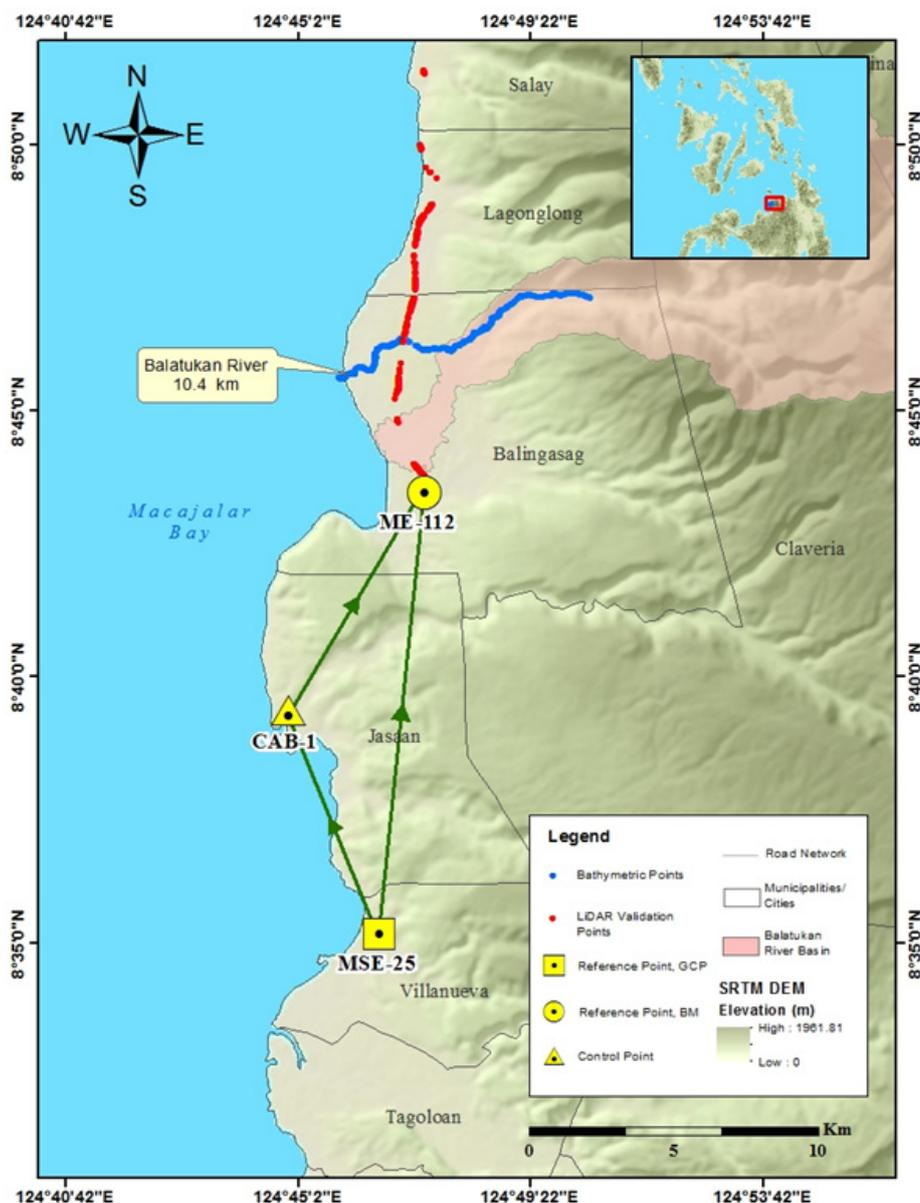
Figure 31. Extent of the bathymetric survey (in blue) in Balatucan River and the LiDAR validation survey (in red).
