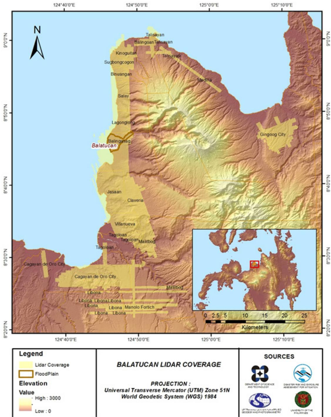
Figure 8. Actual LiDAR survey coverage for Balatucan Floodplain.
