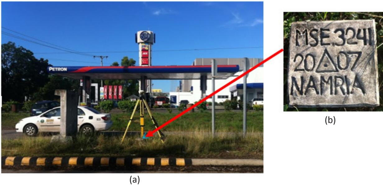
Figure 7. GPS set-up over MSE-3241 on a center island near a gasoline station beside SM Cagayan de Oro (a) and NAMRIA reference point MSE-3241 (b) as recovered by the field team.
