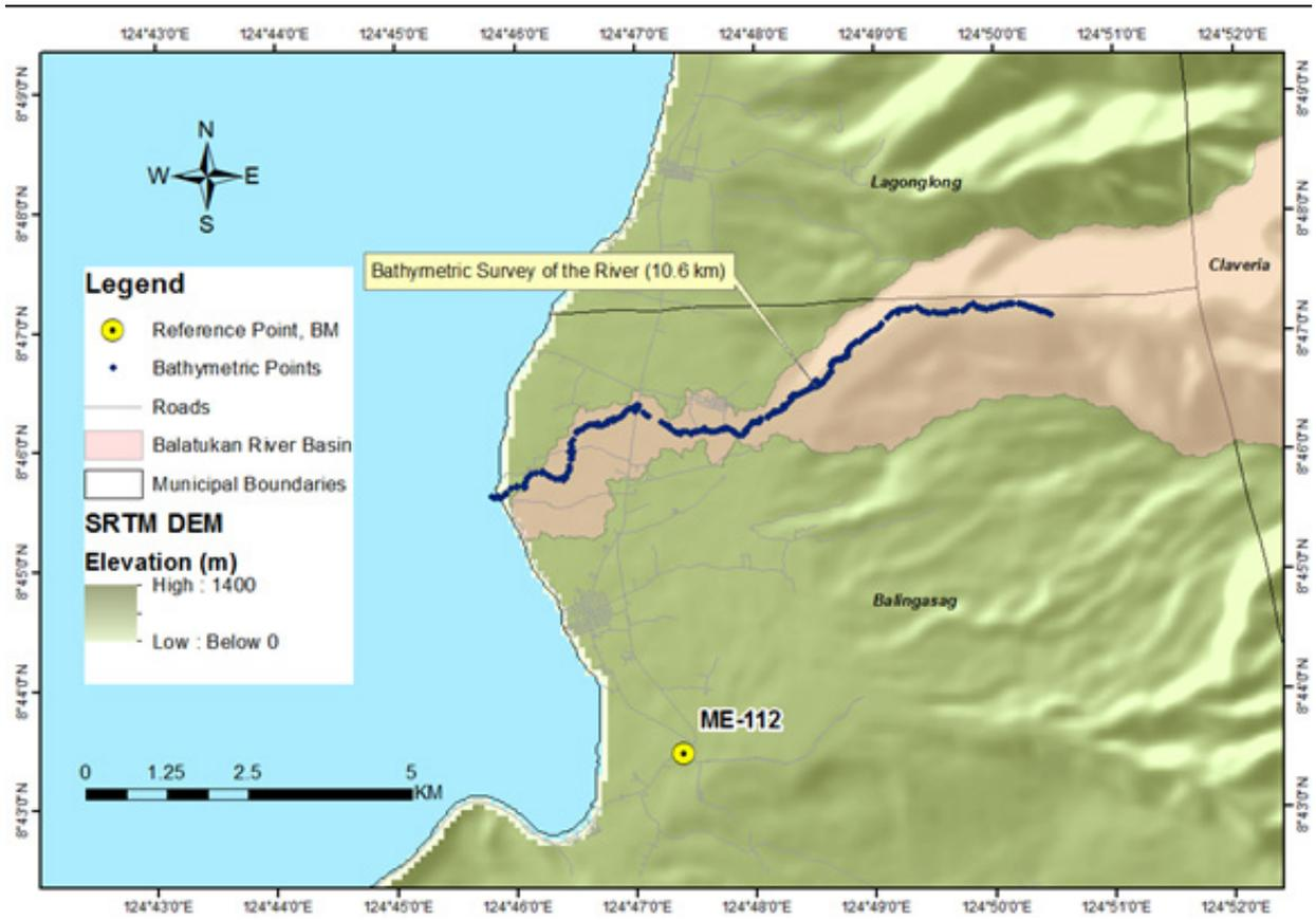
Figure 45. Bathymetric survey of Balatukan River
