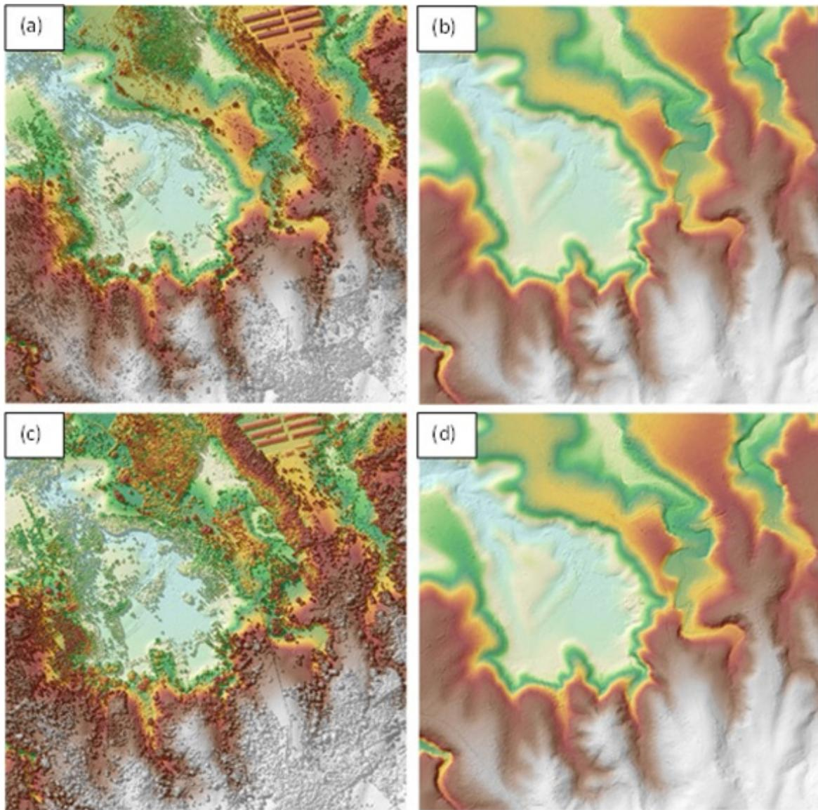
Figure 20. The production of last return DSM (a) and DTM (b); first return DSM (c) and secondary DTM (d) in some portion of Balatucan Floodplain.
