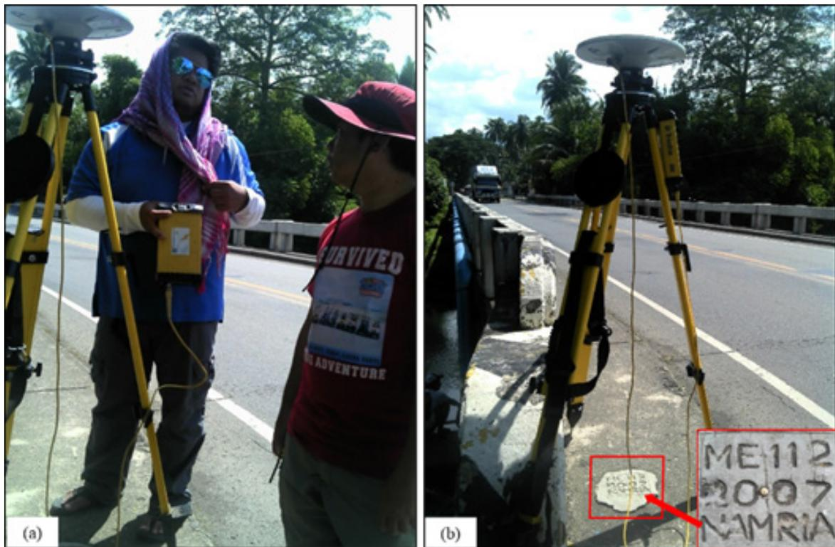
Figure 34. GNSS base receiver set-up, Trimble® SPS 852 at ME-112 at Musi-Musi Bridge in Brgy. Talusan, Municipality of Balingasag, Misamis Oriental.
