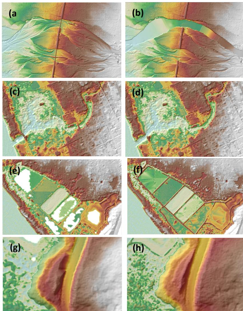
Figure 23. Portions in the DTM of Balatucan Floodplain—bridges before (a), (c) and after (b), (d) manual editing; a paddy field before (e) and after (f) data retrieval; and a misclassified hill before (g) and after (h) data retrieval.
