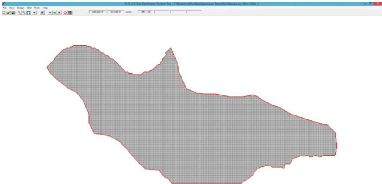
Figure 59. Screenshot of subcatchment with the computational area to be modeled in FLO-2D Grid Developer System Pro (FLO-2D GDS Pro).
