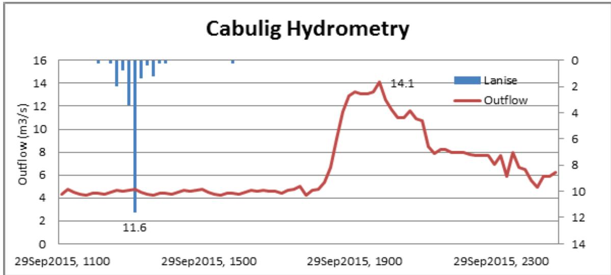
Figure 44. Rainfall and outflow data at Cabulig used for modeling
