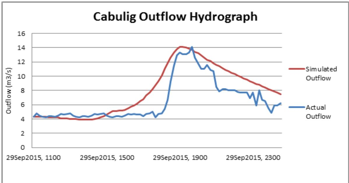
Figure 54. Outflow hydrograph of Cabulig produced by the HEC-HMS model compared with observed outflow
