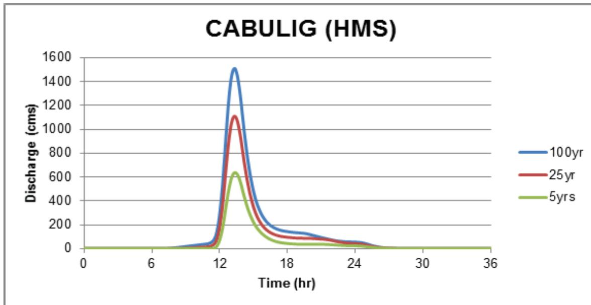
Figure 56. Cabulig River generated discharge using 5-, 25-, and 100-year Lumbia RIDF in HEC-HMS
