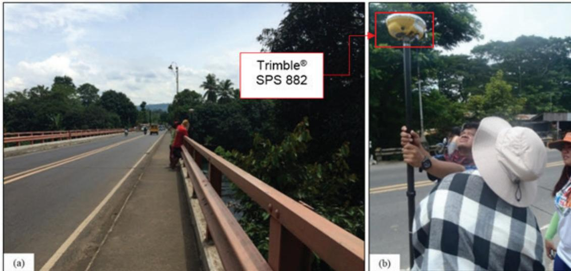
Figure 32. GNSS base occupation, Trimble® SPS 882 at CAB-1 along Iligan-Cagayan de Oro-Butuan Road at the approach of Cabulig Bridge in Brgy. Bobontugan, Municipality of Jasaan, Misamis Oriental
