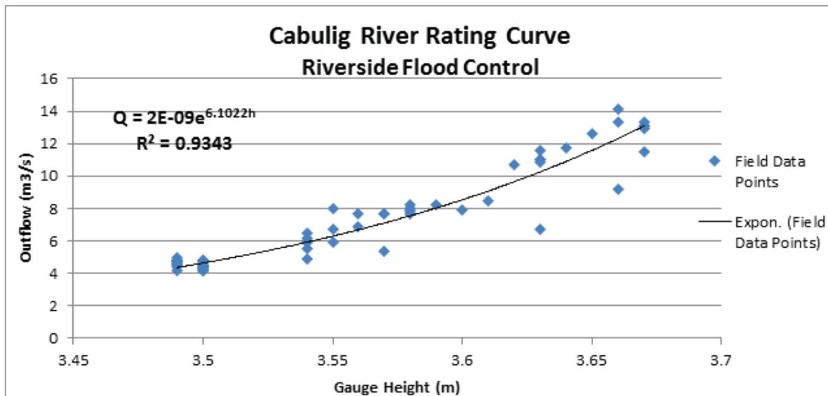
Figure 43. HQ curve of HEC-HMS model
