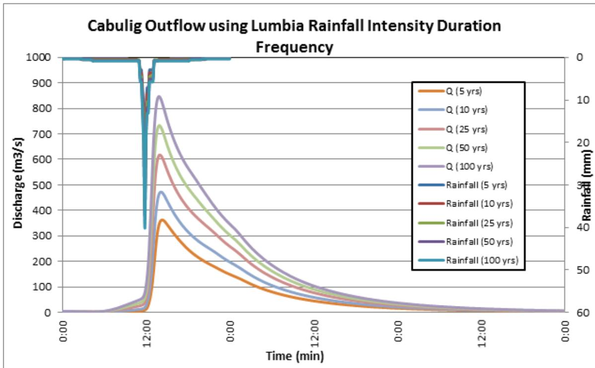
Figure 55. Outflow hydrograph at Cabulig Station generated using Lumbia RIDF simulated in HEC-HMS
