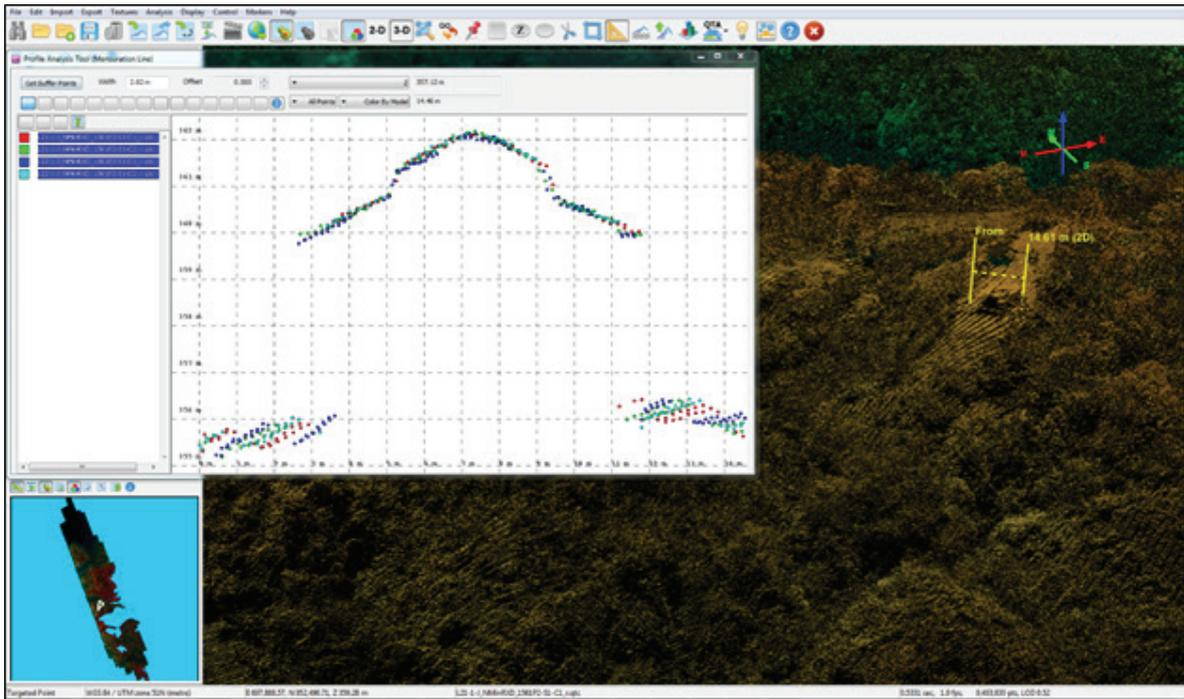
Figure 15. Quality checking for a Cabulig flight 1561P using the Profile Tool of QT Modeler
