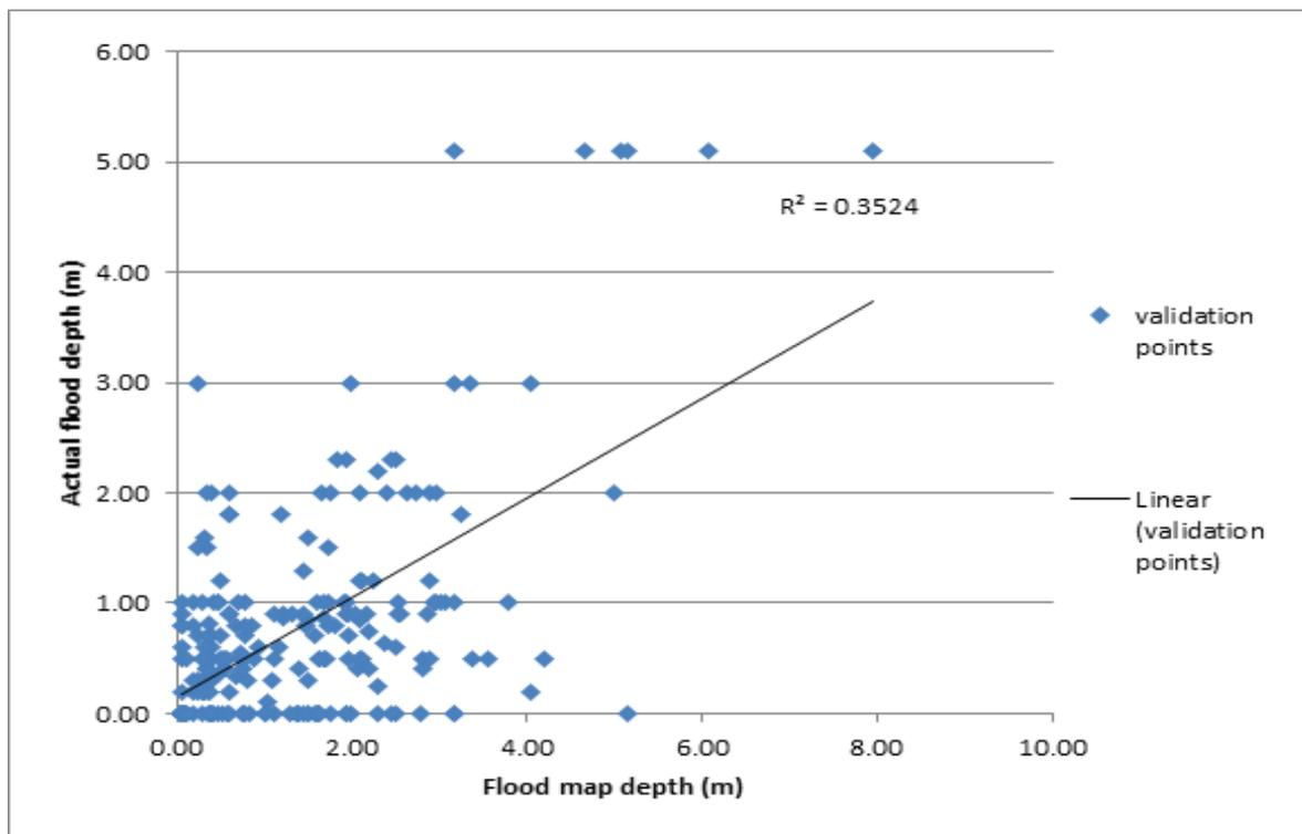
Figure 68. Flood map depth vs. actual flood depth
