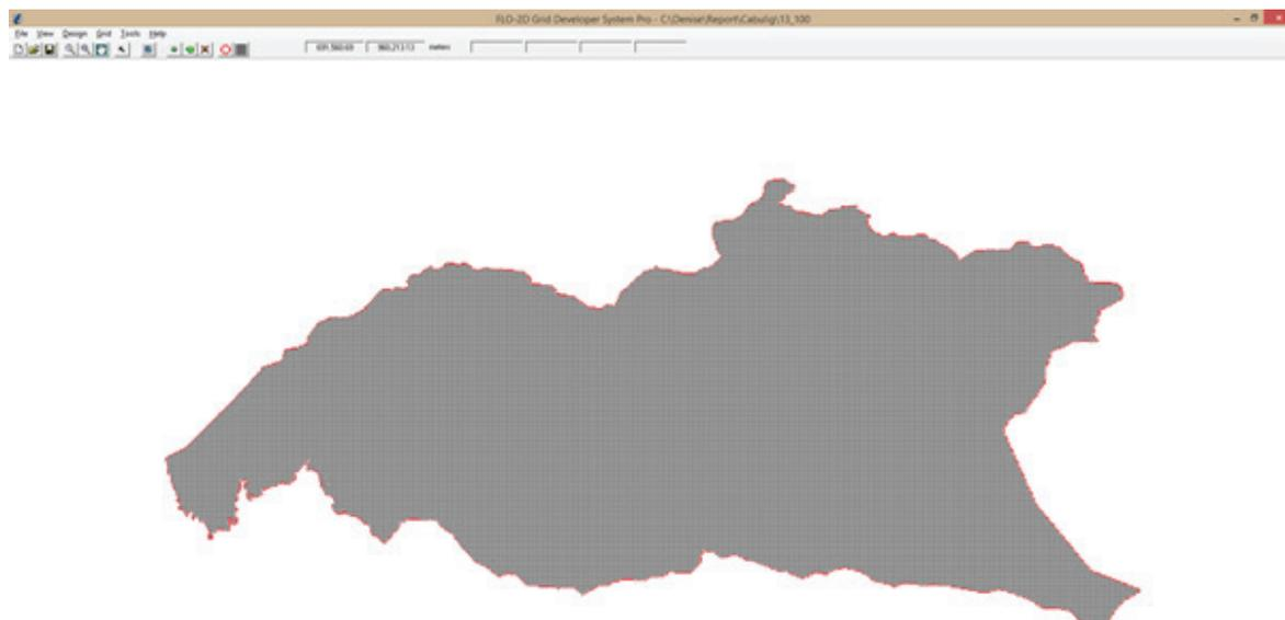
Figure 53. Screenshot of subcatchment with the computational area to be modeled in FLO-2D GDS Pro
