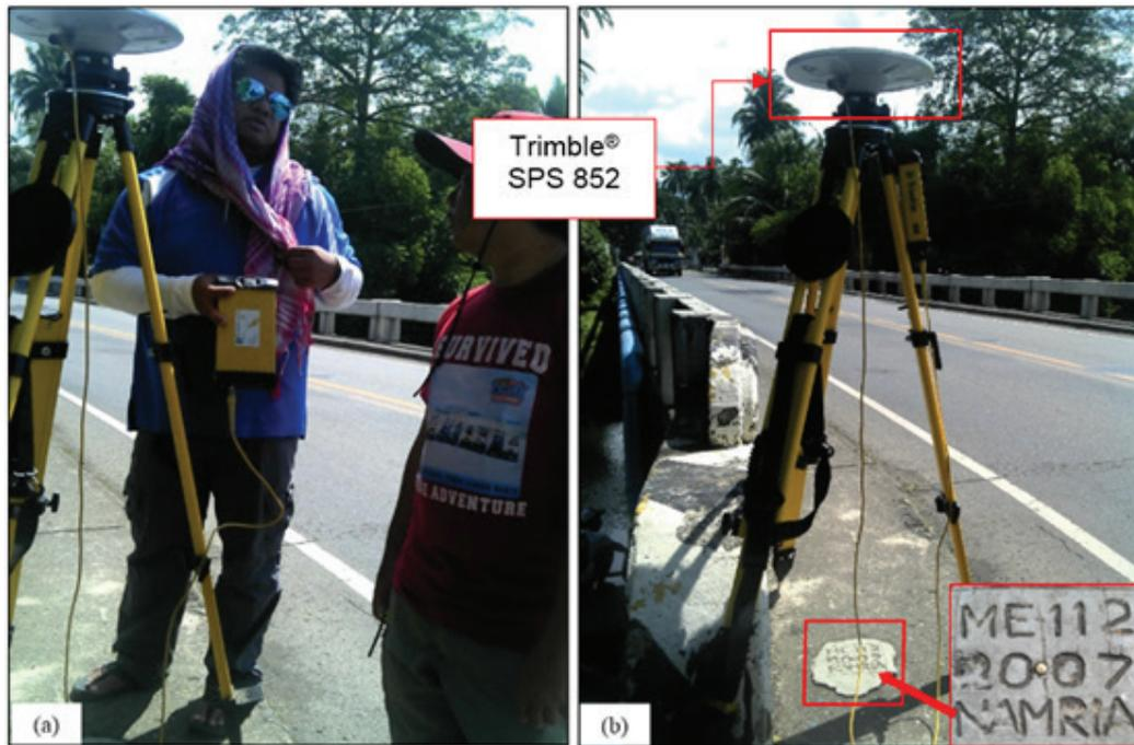
Figure 30. GNSS base receiver set-up, Trimble® SPS 852 at ME-112 at Musi-Musi Bridge in Brgy. Talusan, Municipality of Balingasag, Misamis Oriental
