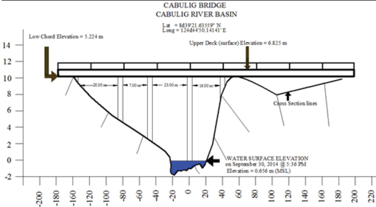
Figure 34. Cross-section diagram of Cabulig Bridge
