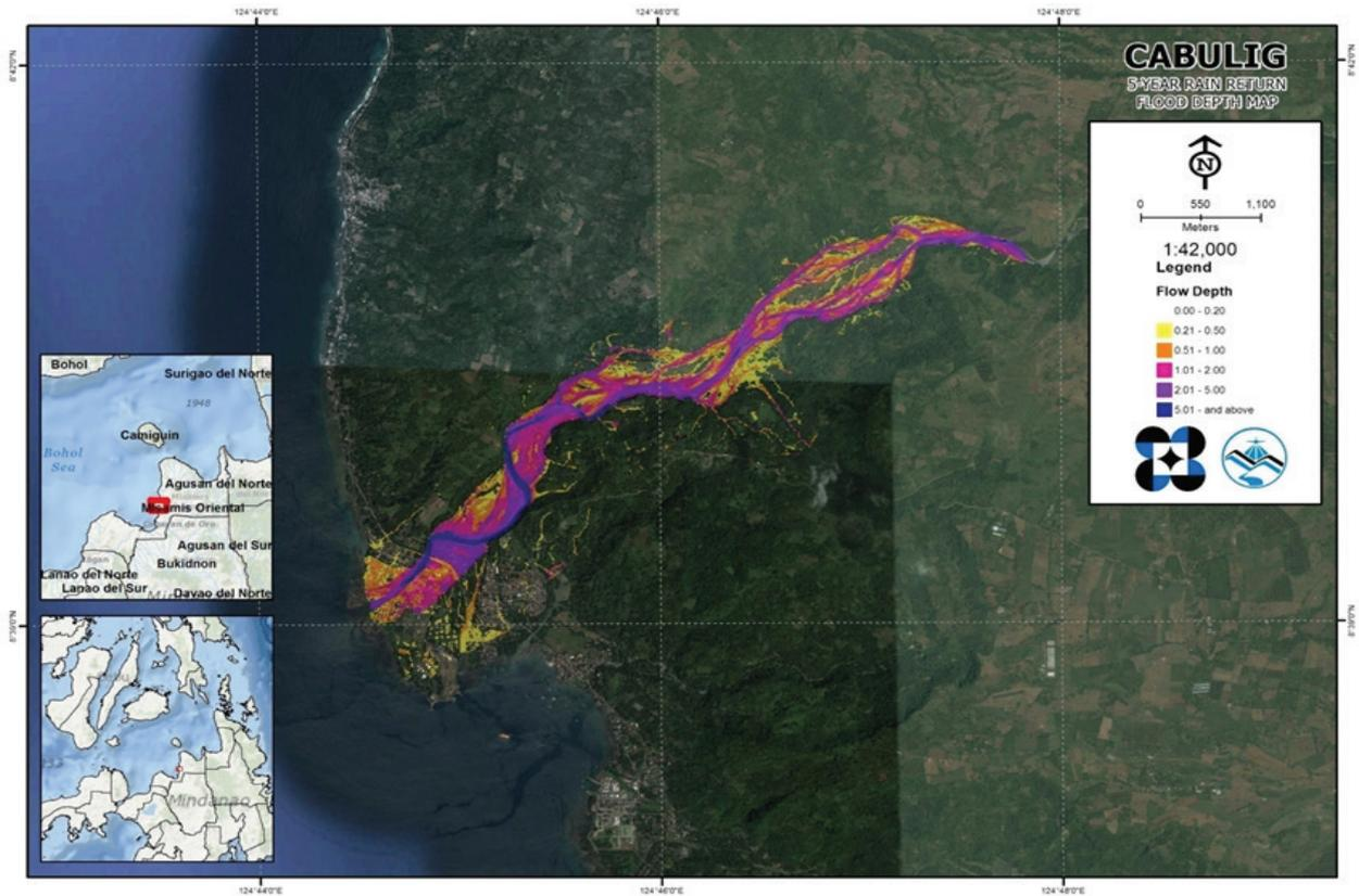
Figure 63. 5-year flood depth map for Cabulig Floodplain
