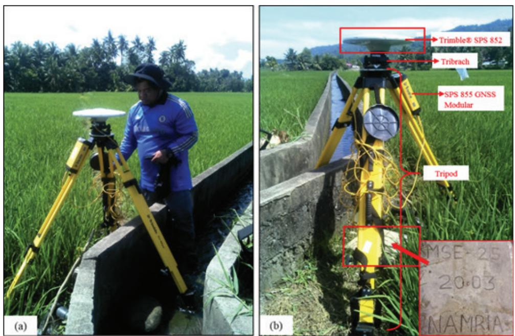
Figure 29. GNSS base receiver set-up, Trimble® SPS 852 at MSE-25 in Brgy. Poblacion 1, Municipality of Villanueva, Misamis Oriental
