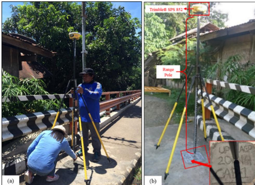
Figure 31. GNSS base occupation, Trimble® SPS 882 at CAB-1 along Iligan-Cagayan de Oro-Butuan Road at the approach of Cabulig Bridge in Brgy. Bobontugan, Municipality of Jasaan, Misamis Oriental
