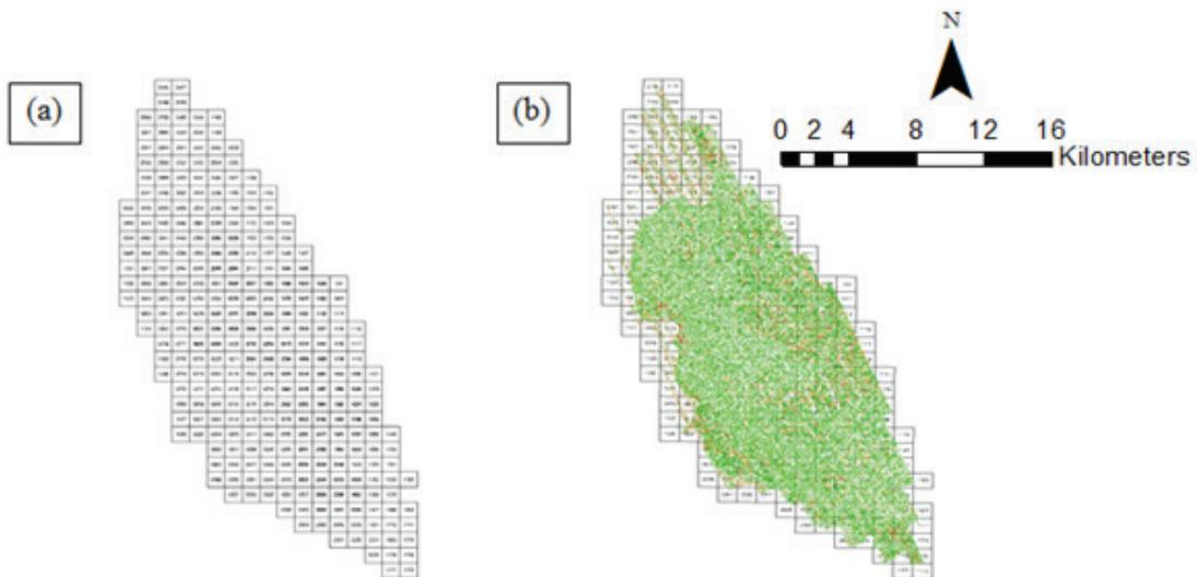
Figure 16. Tiles for Cabulig Floodplain (a) and classification results (b) in TerraScan
