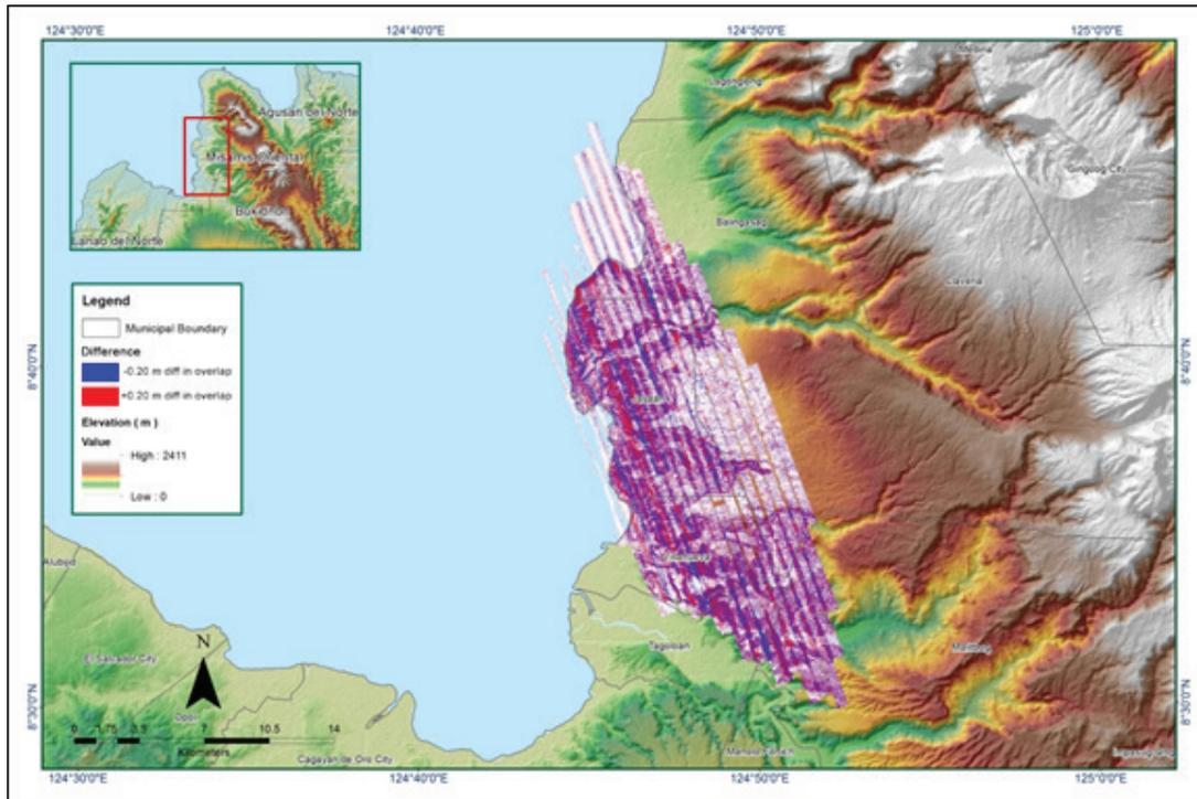
Figure A-8.7. Elevation difference between flight lines
