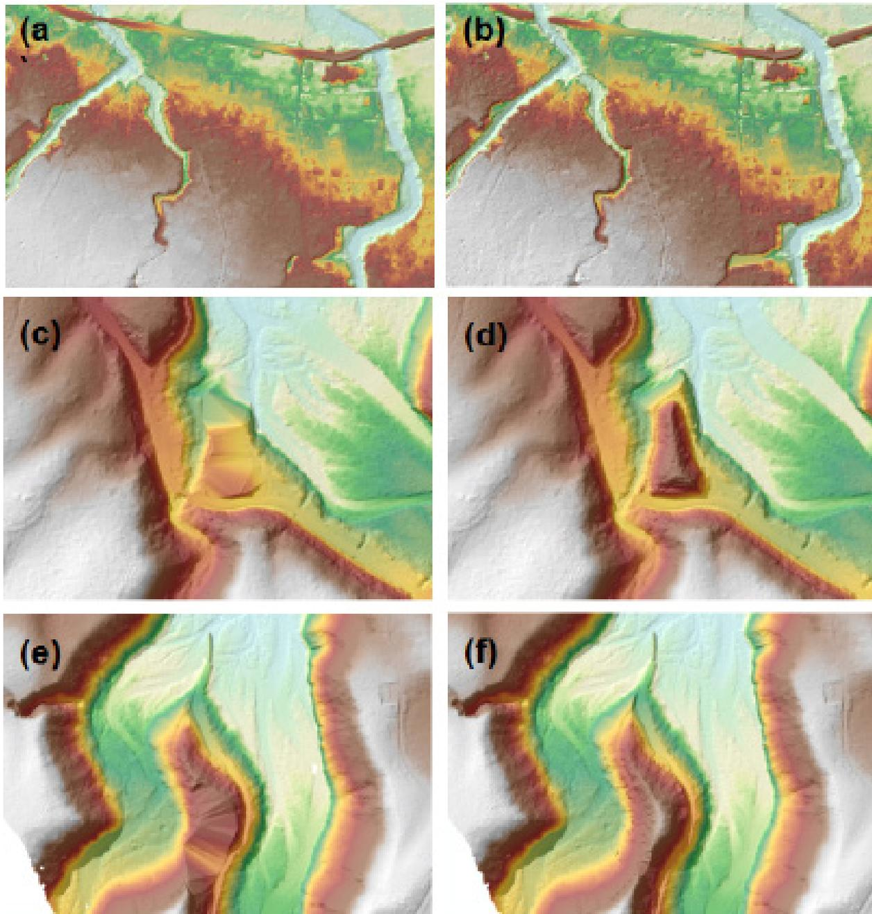
Figure 20. Portions in the DTM of Gahub Floodplain— – bridges before (a) and after (b) interpolation and misclassified ridges before (c, e) and after (d, f) data retrieval
