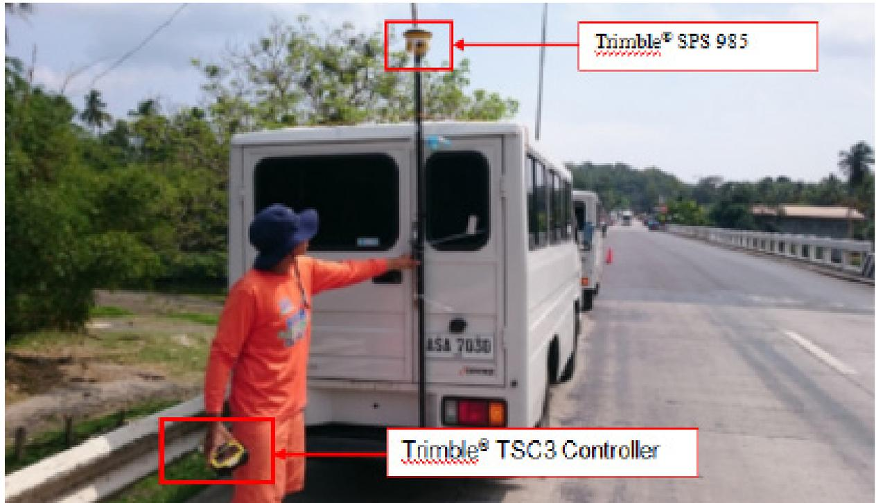
Figure 35. LiDAR Validation survey set up
