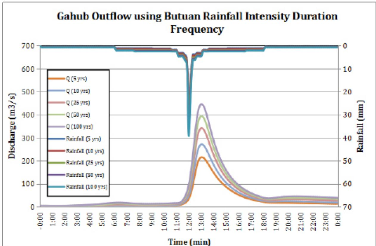
Figure 54. Outflow hydrograph at Gahub Station generated using Butuan RIDF simulated in HEC-HMS
