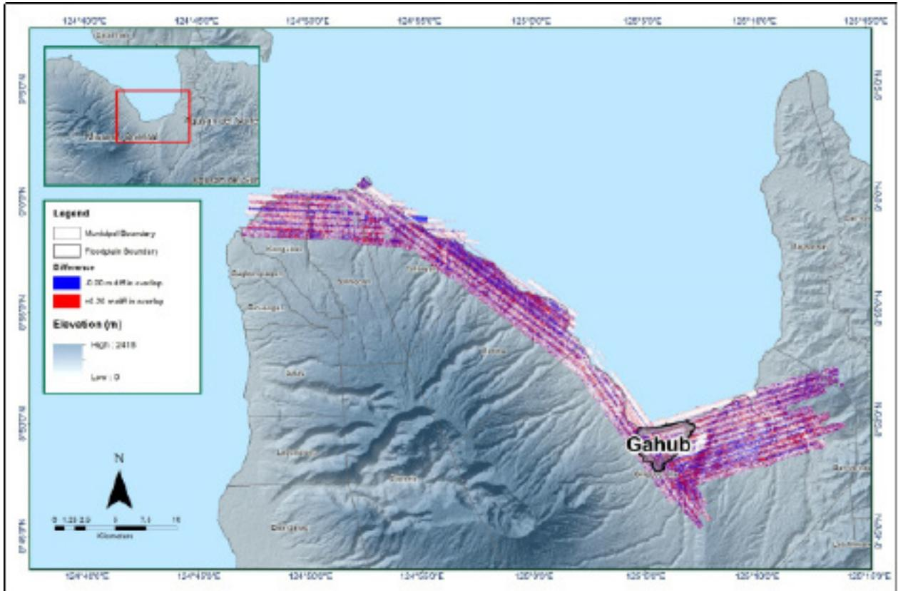
Figure 15. Elevation difference map between flight lines for Gahub Floodplain.
