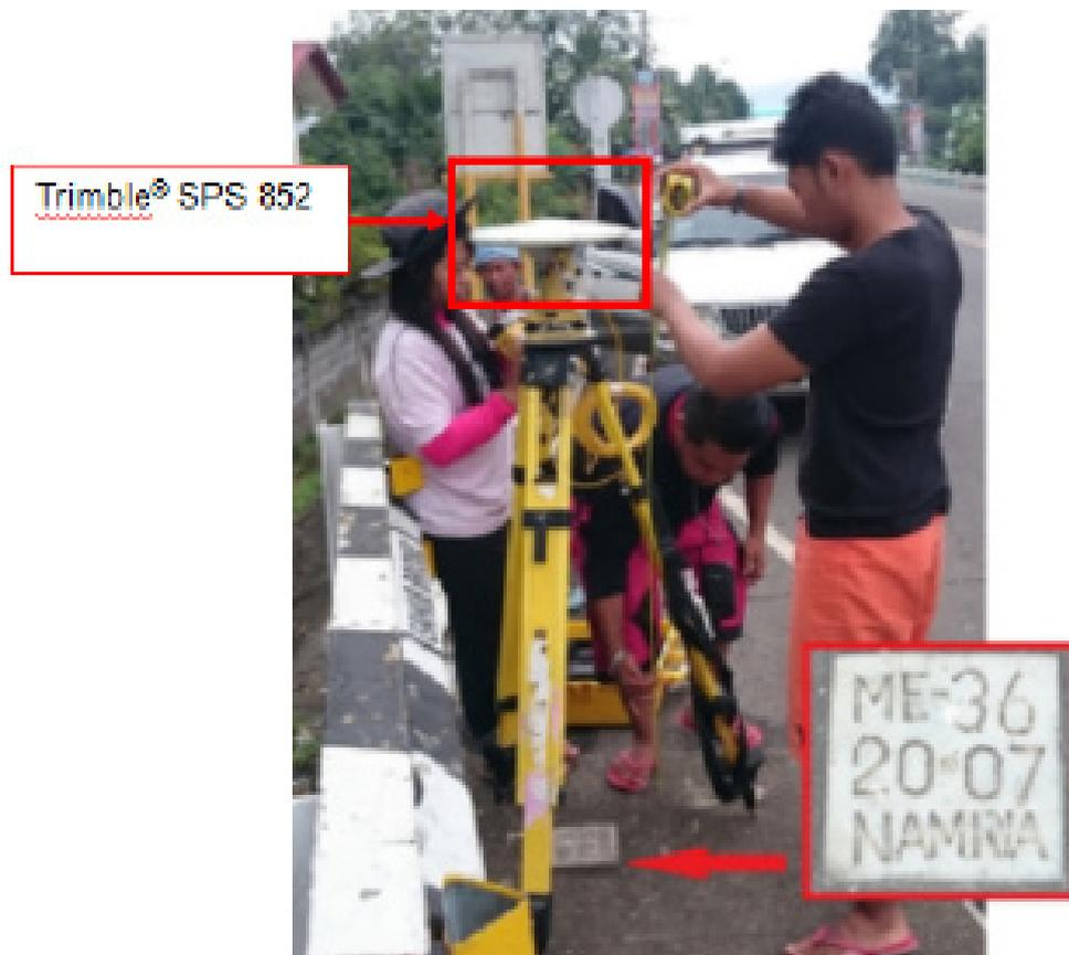
Figure 31. Trimble® SPS 852 Base set-up at ME-36, Gingoog Bridge located at Gingoog City
