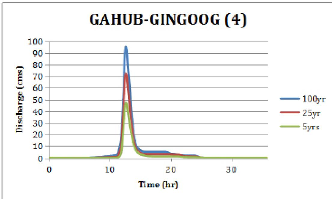
Figure 58. Gahub-Gingoog River (4) generated discharge using 5-, 25-, and 100-year Lumbia rainfall intensity-duration-frequency (RIDF) in HEC-HMS
