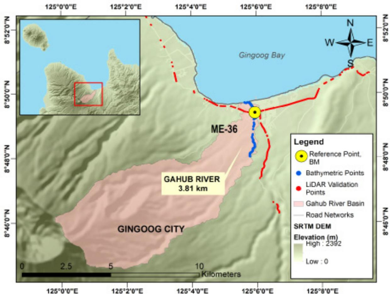
Figure 28. General survey area for Gahub River Basin Extent of the bathymetric survey (in blue) in Gahub River and the LiDAR data validation survey (in red)
