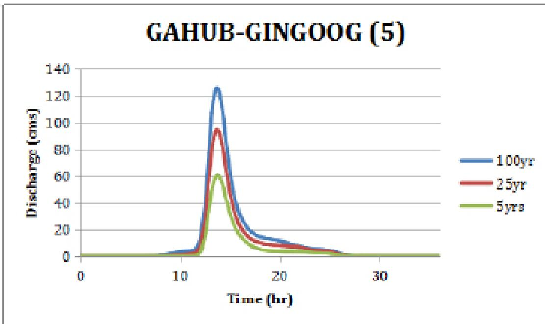
Figure 59. Gahub-Gingoog River (5) generated discharge using 5-, 25-, and 100-year Lumbia rainfall intensity-duration-frequency (RIDF) in HEC-HMS
