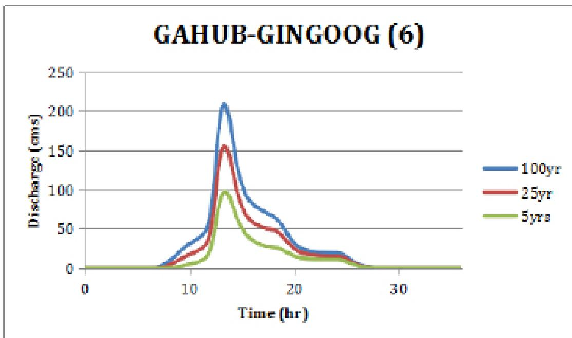
Figure 60. Gahub-Gingoog River (6) generated discharge using 5-, 25-, and 100-year Lumbia rainfall intensity-duration-frequency (RIDF) in HEC-HMS
