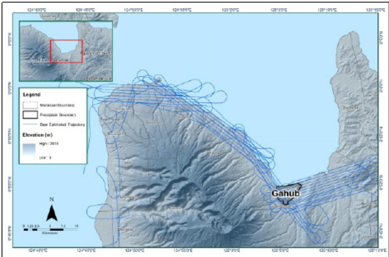
Figure 11. Best estimated trajectory for of LiDAR missions conducted over the Gahub Floodplain
