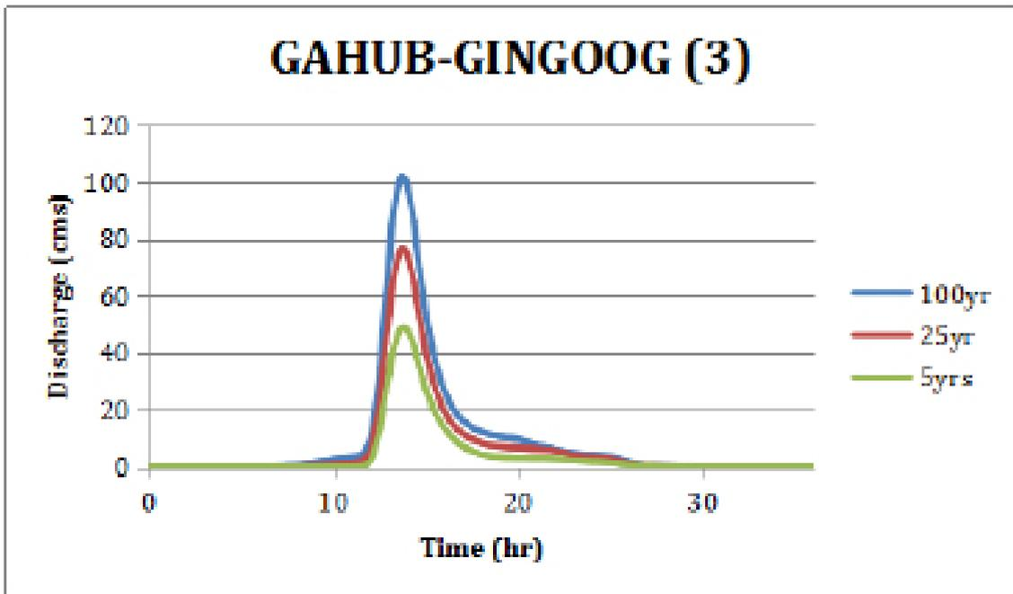
Figure 57. Gahub-Gingoog Rriver (3) generated discharge using 5-, 25-, and 100-year Lumbia rainfall intensity-duration-frequency (RIDF) in HEC-HMS
