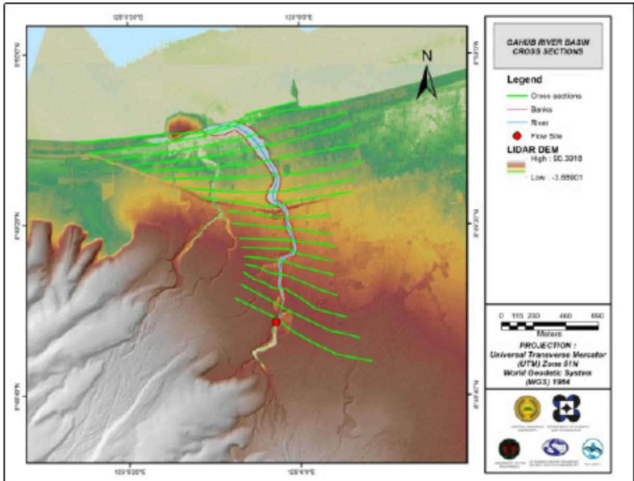
Figure 51. Gahub River Cross-section generated using HEC GeoRAS tool
