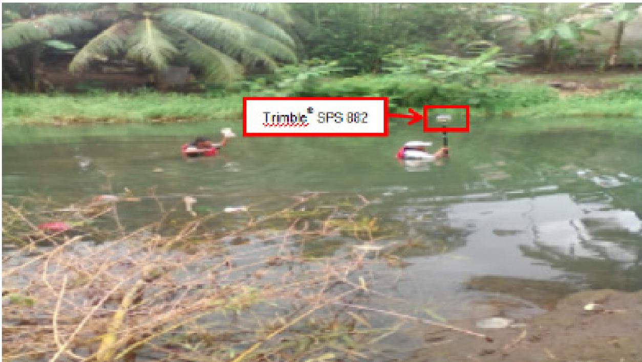
Figure 38. Set-up of manual bathymetry survey for Gahub River using a Trimble® SPS 882 Rover
