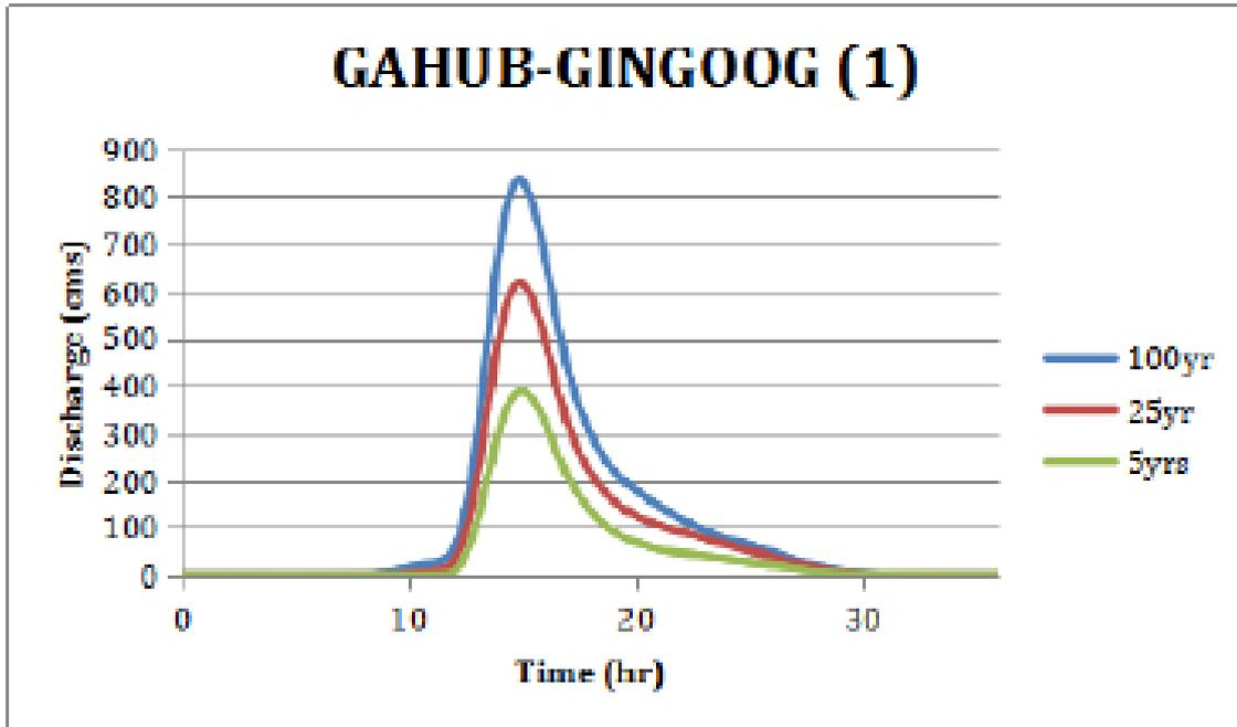
Figure 55. Gahub-Gingoog River (1) generated discharge using 5-, 25-, and 100-year Lumbia rainfall intensity-duration-frequency (RIDF) in HEC-HMS
