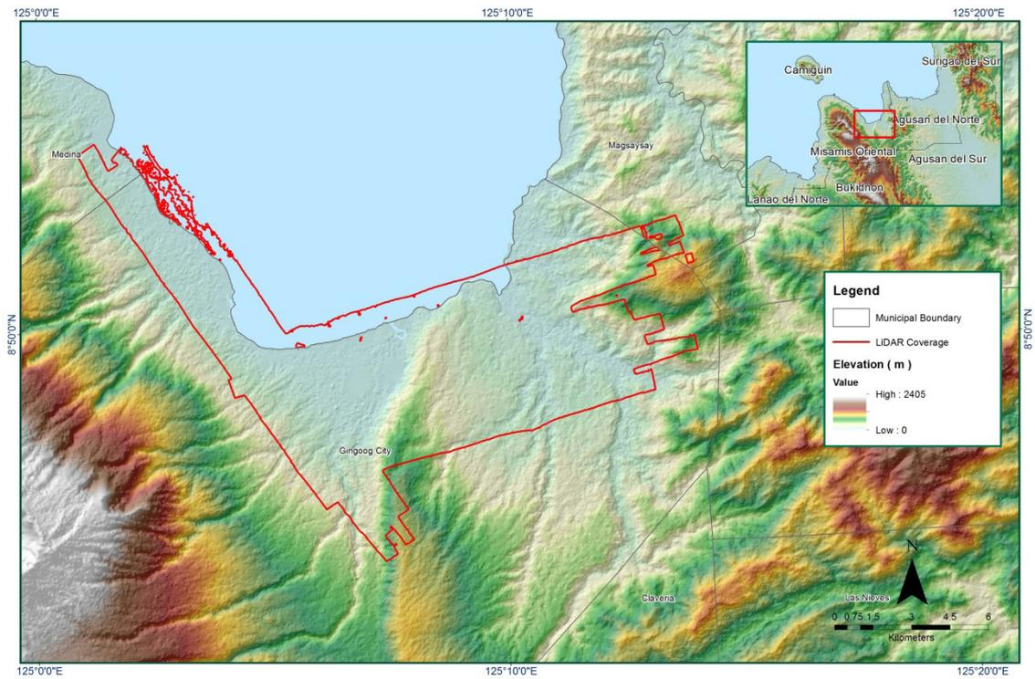
**Figure A-8.4 Coverage of LiDAR data**
