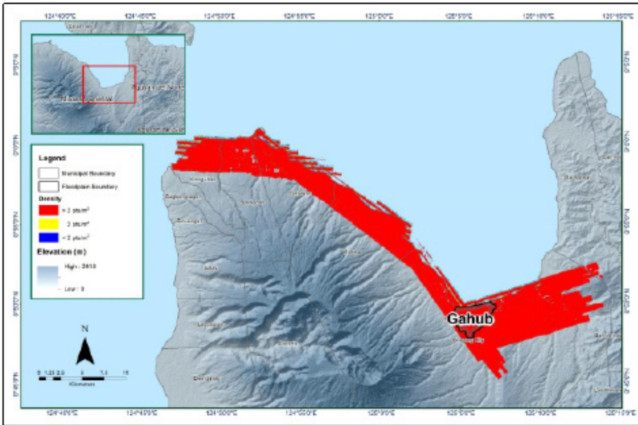
Figure 14. Pulse density map of merged LiDAR data for Gahub Floodplain.
