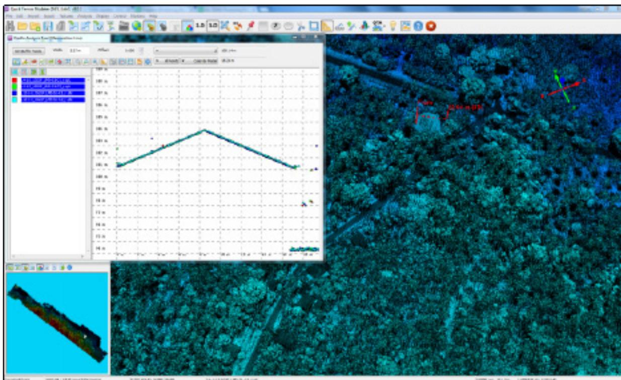
Figure 16. Quality checking for a Gahub flight 1521P using the Profile Tool of QT Modeler
