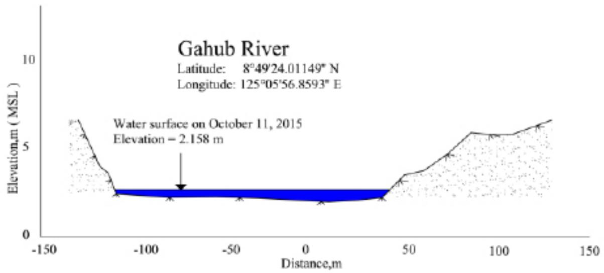
Figure 34. Cross-sectional diagram of Gahub River deployment site
