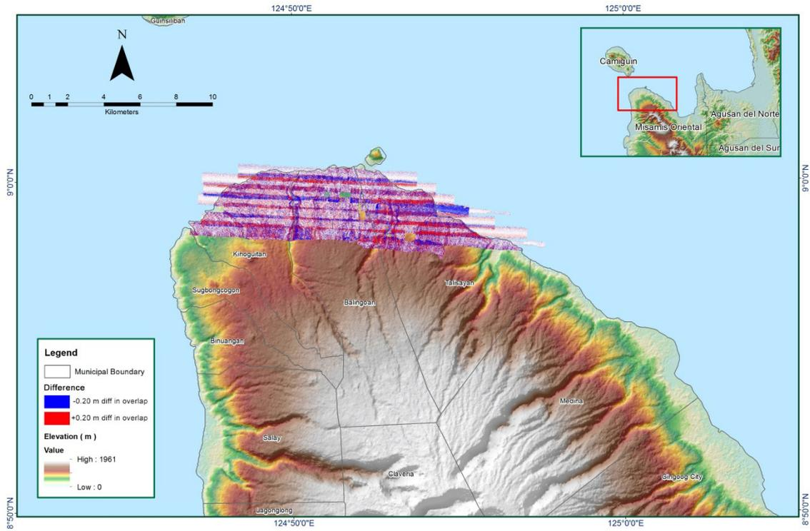
**Figure A-8.21** Elevation difference between flight lines
