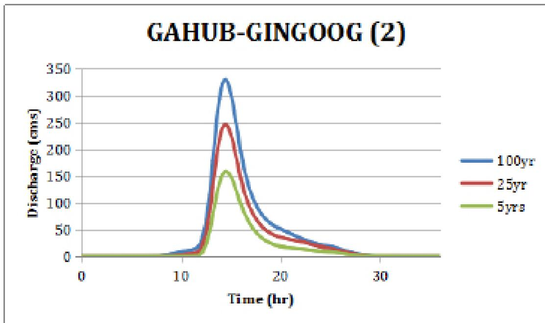
Figure 56. Gahub-Gingoog River (2) generated discharge using 5-, 25-, and 100-year Lumbia rainfall intensity-duration-frequency (RIDF) in HEC-HMS
