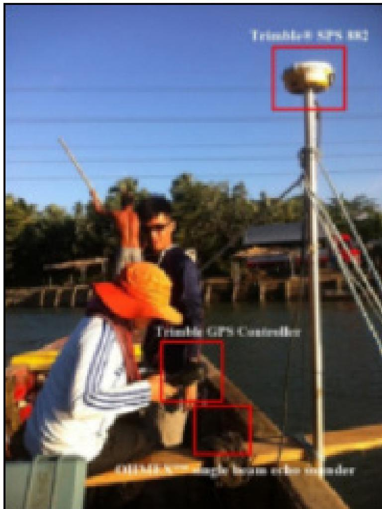
Figure 40. Bathymetric survey set-up using OHMEX™ single beam echo sounder and a mounted with a Trimble® SPS 882
