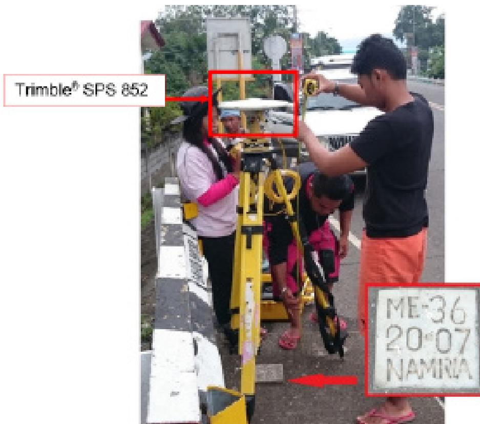
Figure 33. Trimble® SPS 852 Base set-up at ME-36 located at the approach of Gahub Bridge in Brgy. I Poblacion, Gingoog City, Misamis Oriental
