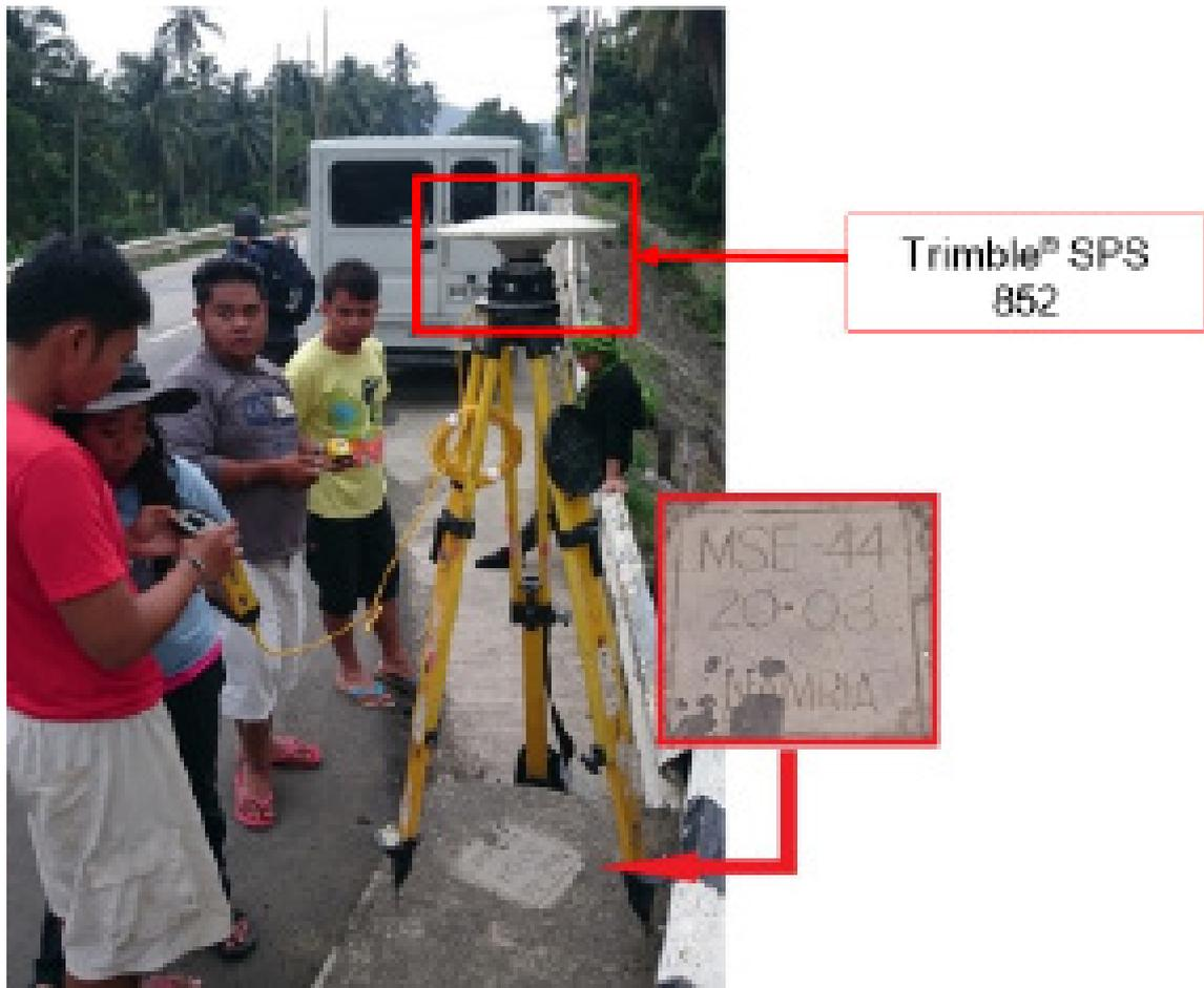
Figure 34. Trimble® SPS 852 Base set-up at MSE-44, located at the approach of Kibungsod Bridge in Brgy. Kibungsod, Municipality of Magsaysay, Misamis Oriental
