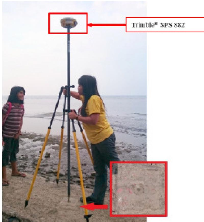
Figure 32. Trimble® SPS 882 GPS set-up at MSE-35 located on a seawall within Madahilag Elementary School in Brgy. Pahindong, Municipality of Medina, Misamis Oriental
