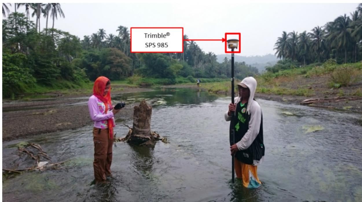
Figure 41. Manual Bathymetric survey in Linugos River using a Trimble® SPS 985 Rover
