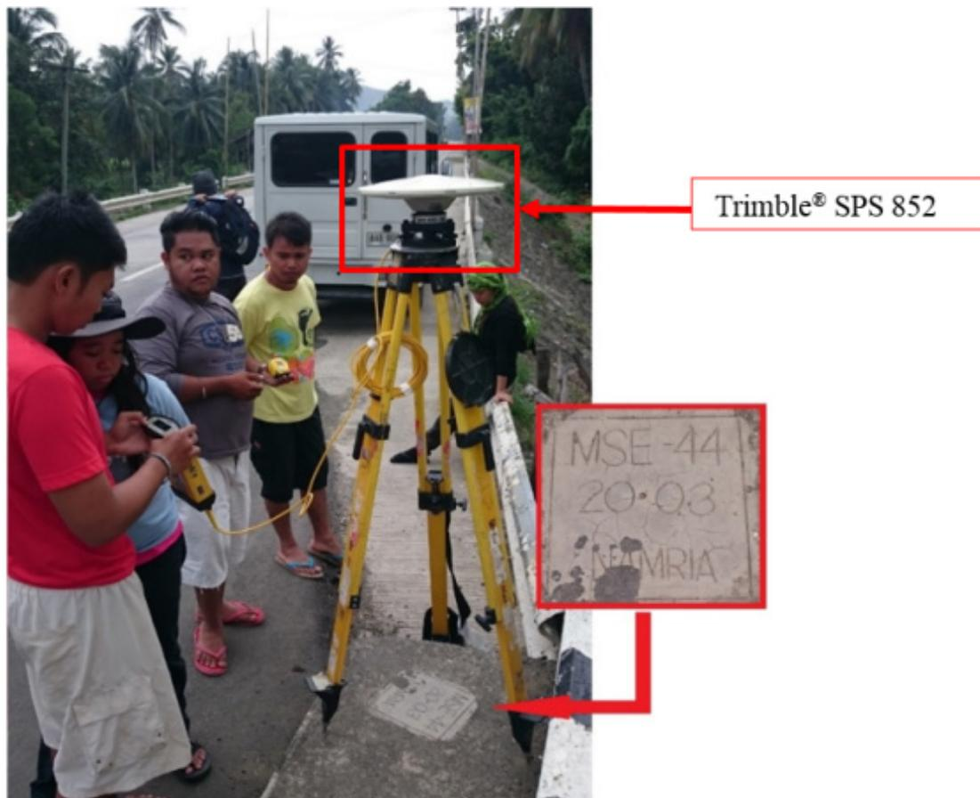
Figure 32. Trimble® SPS 852 Base setup at MSE-44, Kibungsod Bridge, located in Brgy. Kibungsod, Municipality of Magsaysay, Misamis Oriental
