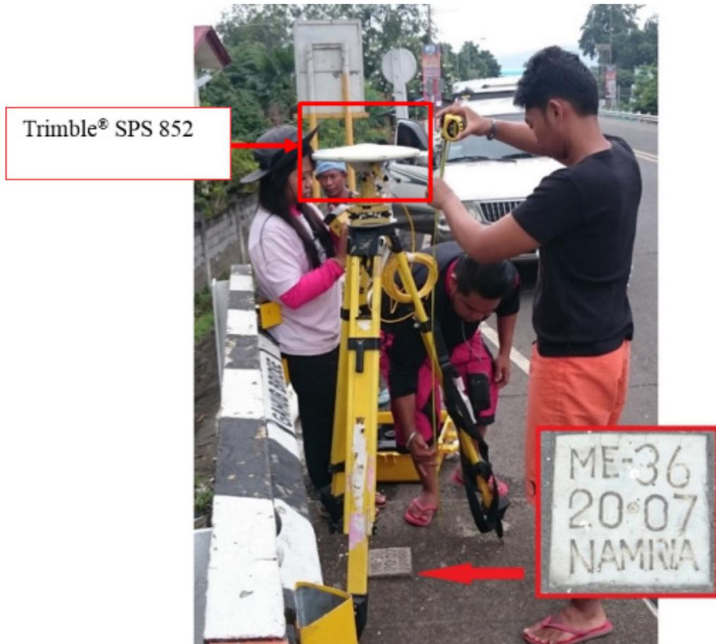
Figure 31. Trimble® SPS 852 Base setup at ME-36 located at the approach of Gahub Bridge in Brgy. Poblacion 1, Gingoog City, Misamis Oriental
