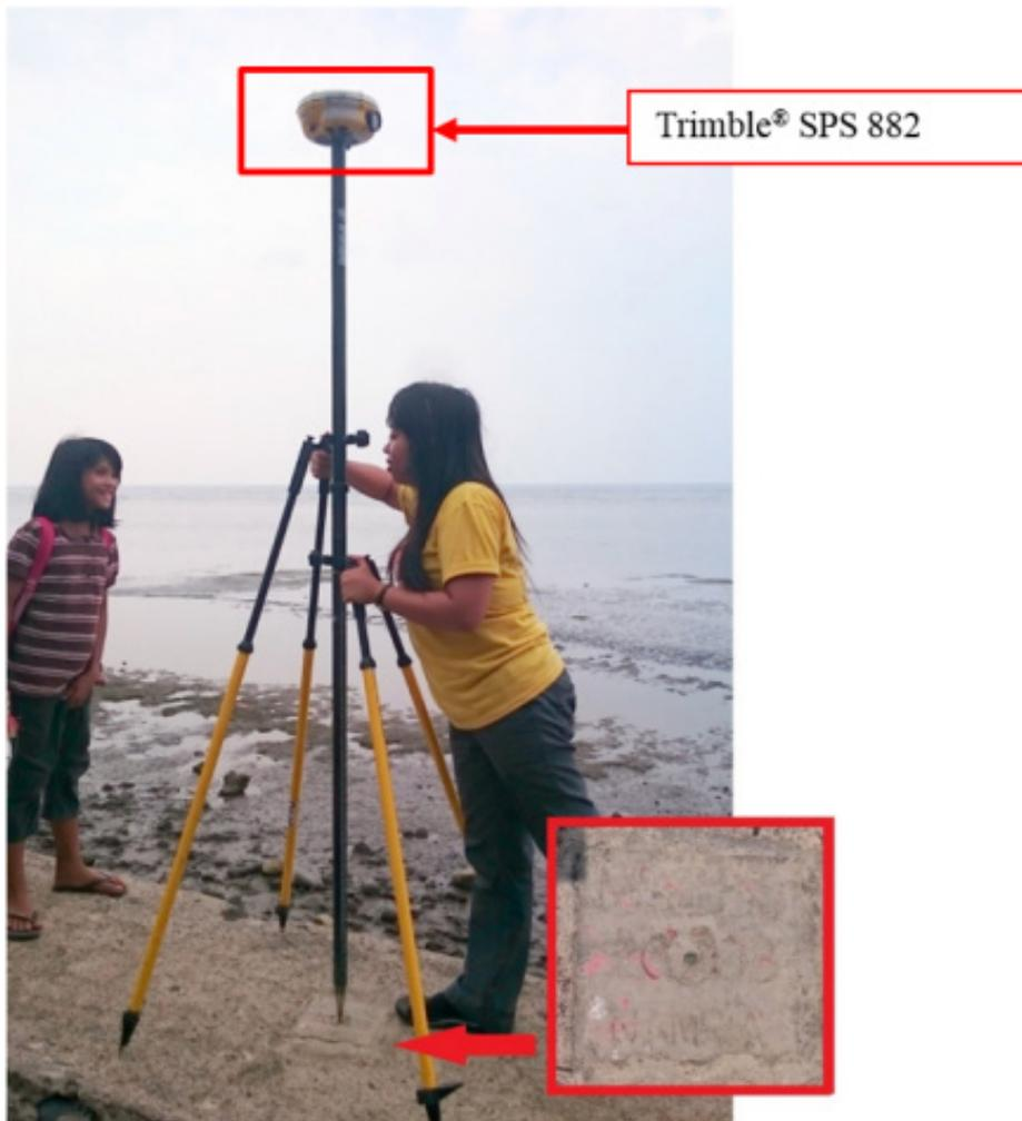
Figure 30. Trimble® SPS 882 GPS setup at MSE-35 located on a seawall within Mandahilag Elementary School in Brgy.Pahindong, Municipality of Medina, Misamis Oriental
