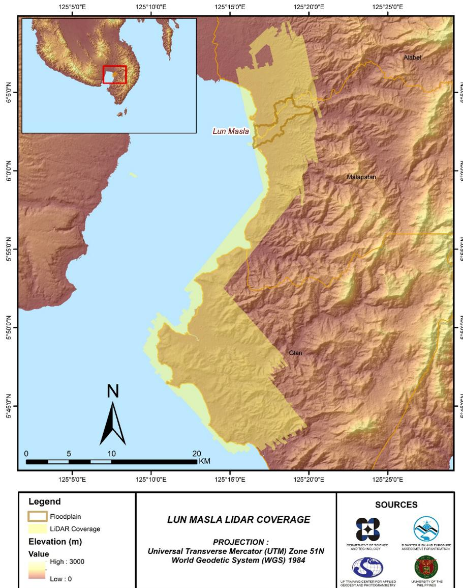
Figure 5. Actual LiDAR survey coverage for Lun Masla Floodplain.
