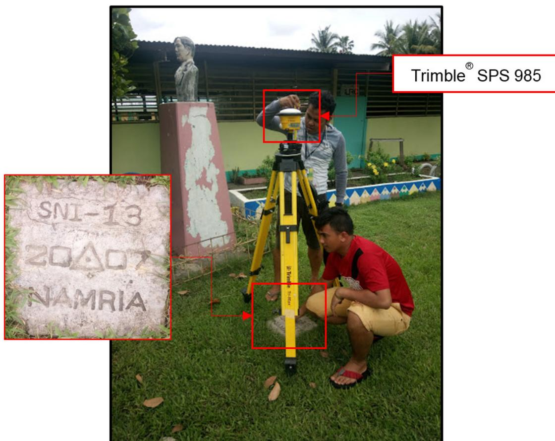
Figure 33. GNSS base set up, Trimble® SPS 985, at SNI-13, a second-order GCP, located beside a Jose Rizal bust inside Maguling Elementary School in Brgy. Maguling, Maitum, Sarangani
