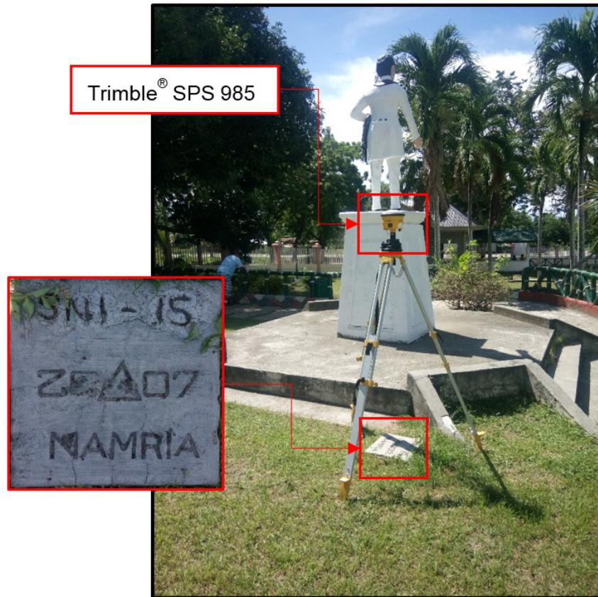
Figure 34. GNSS receiver set up, Trimble® SPS 985, at SNI-15, located behind a Jose Rizal monument inside the premises of Malapatan Municipal Hall in Brgy. Poblacion, Malapatan, Sarangani
