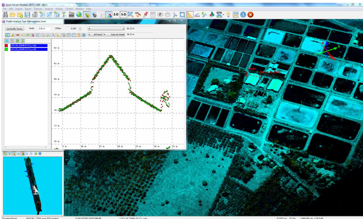
Figure 14. Quality checking for Lun Masla flight 2164 using the Profile Tool of QT Modeler.
