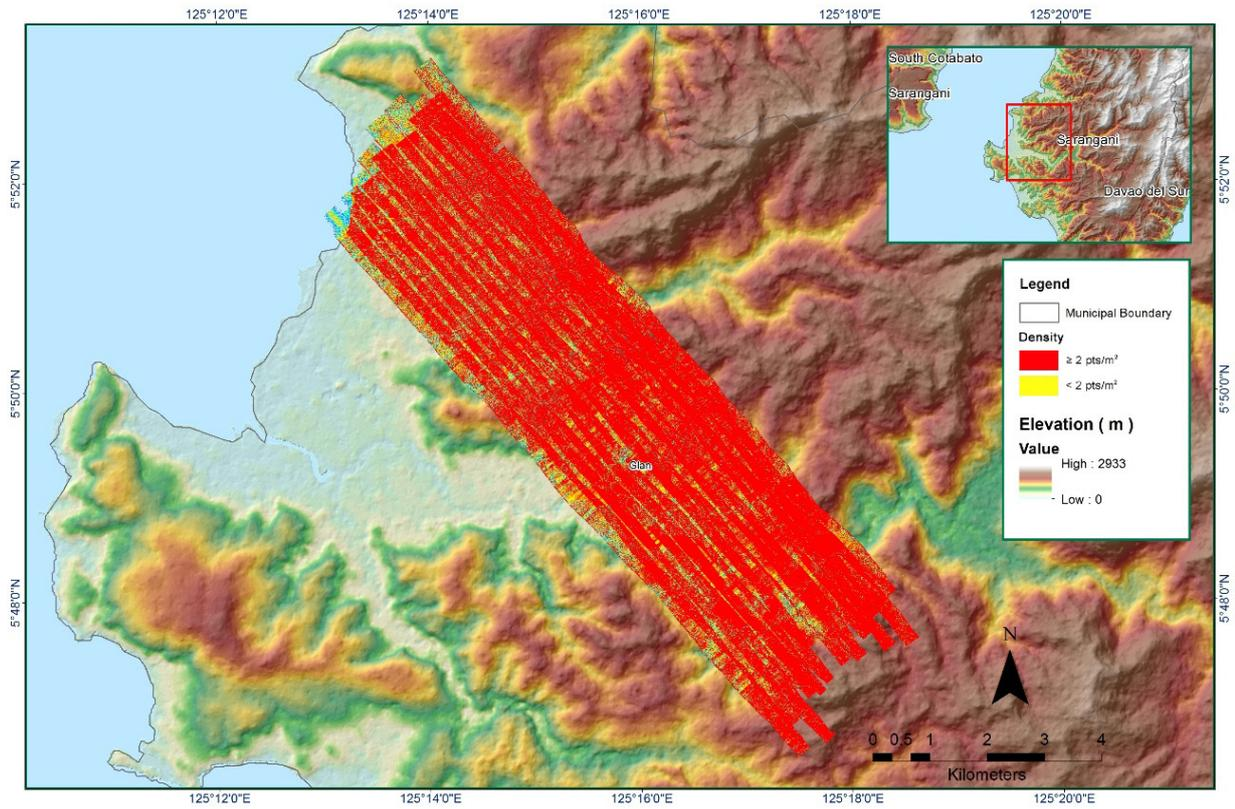
Figure A-8.27. Density of merged LiDAR data
