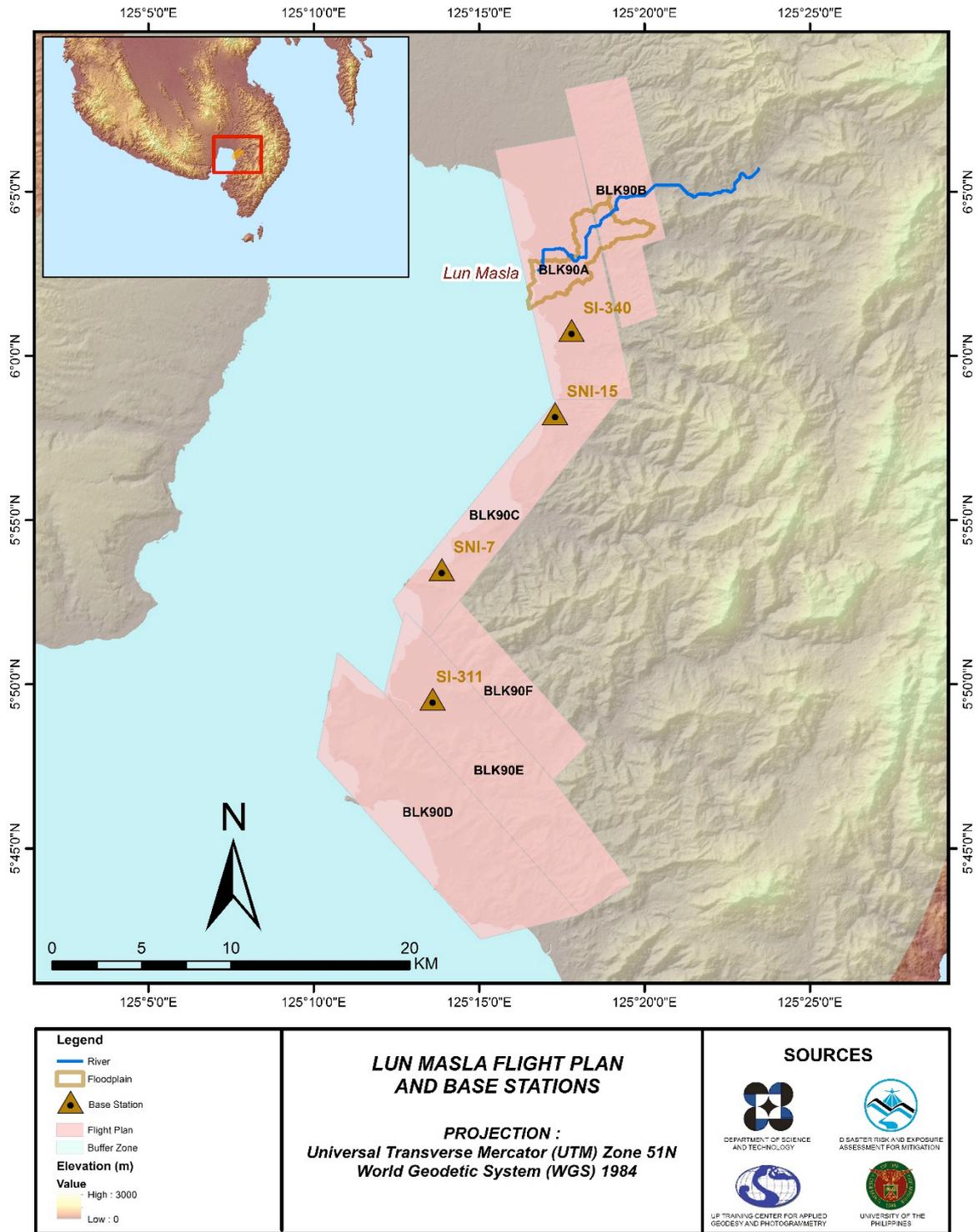
Figure 2. Flight plans and base stations used for Lun Masla Floodplain
