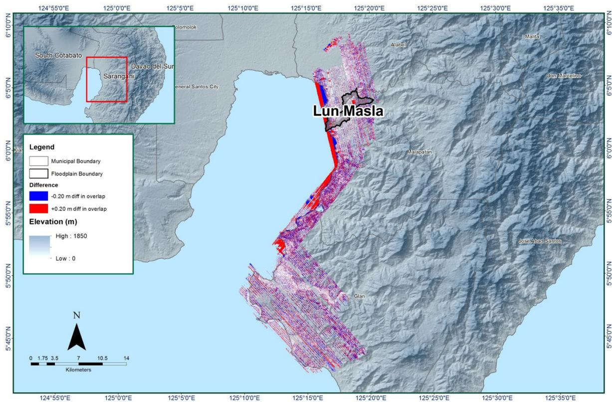
Figure 13. Elevation difference map between flight lines for Lun Masla Floodplain.
