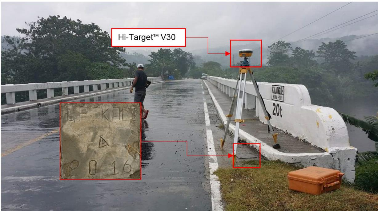
Figure 36. GNSS receiver set up, Hi-Target™ V30, at UP\_KAL-1, an established control point, located beside the approach of Kalaong Bridge in Brgy. Kalaong, Maitum, Sarangani
