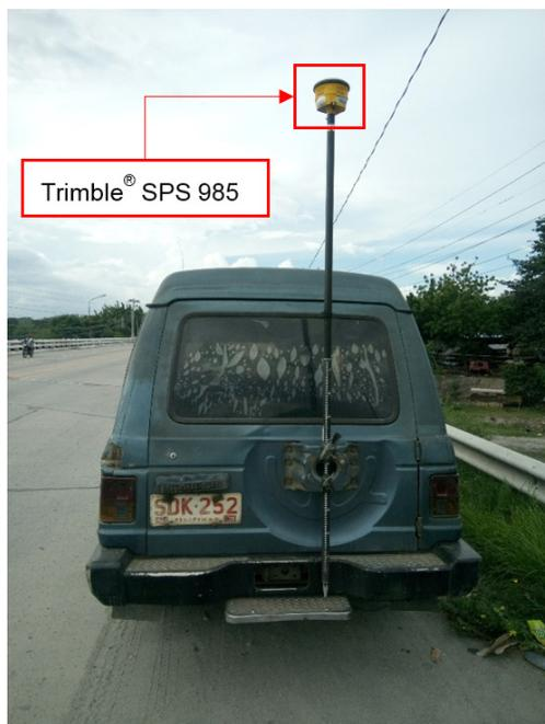
Figure 44. Validation points acquisition survey set-up for Lun Masla River
