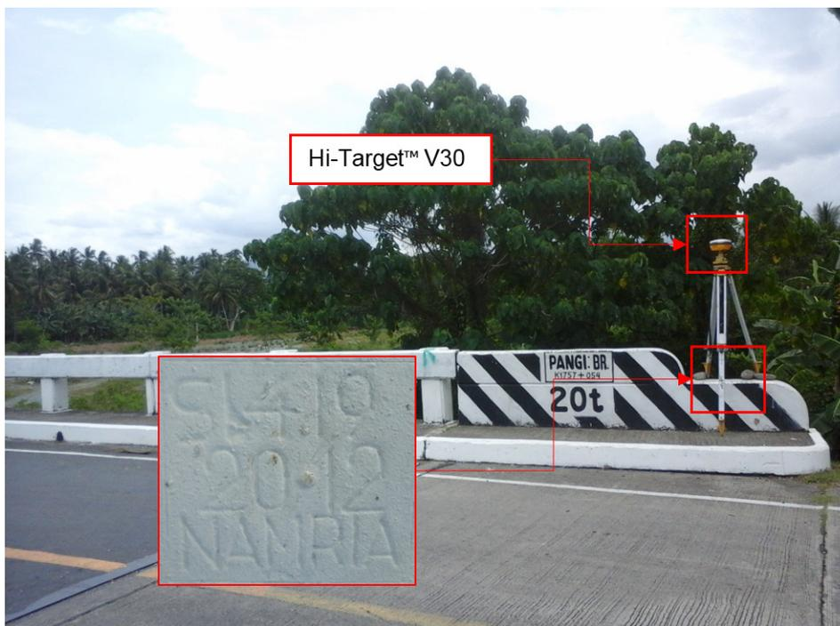
Figure 32. GNSS receiver set up, Hi-Target™ V30, at SI-419, a NAMRIA established BM, located on the barrier of Pangi Bridge in Brgy. Pangi, Maitum, Sarangani
