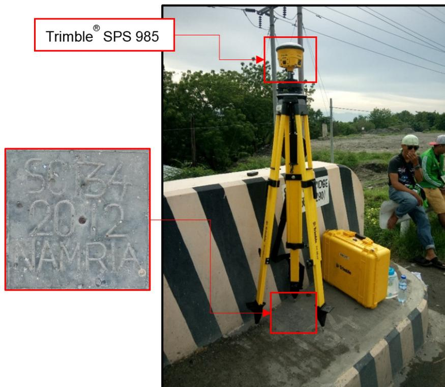
Figure 28. GNSS receiver set up, Trimble® SPS 985, at SC-134, located at the approach of Sinawal Bridge in Brgy. Labangal, General Santos City, South Cotabato
