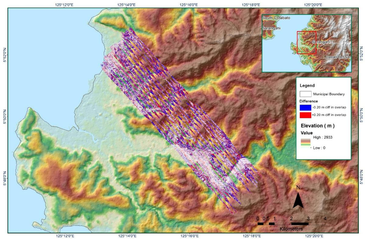
Figure A-8.28. Elevation difference between flight lines
