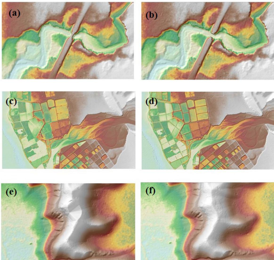
Figure 17. Figure 18. Portions in the DTM of Lun Masla Floodplain - -bridge, misclassified paddies and terrain before (a), (c), (e), and after (b), (d), (f) interpolation and data retrieval, respectively.
