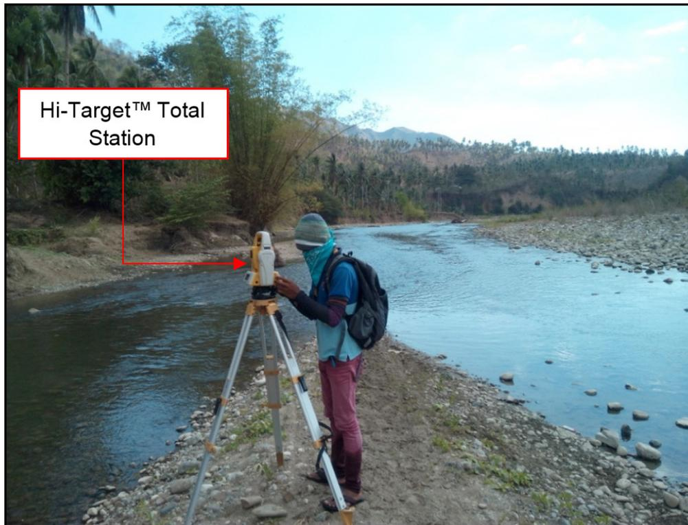
Figure 46. Manual bathymetric survey of ABSD at Lun Masla River using Hi-Target™ Total Station
