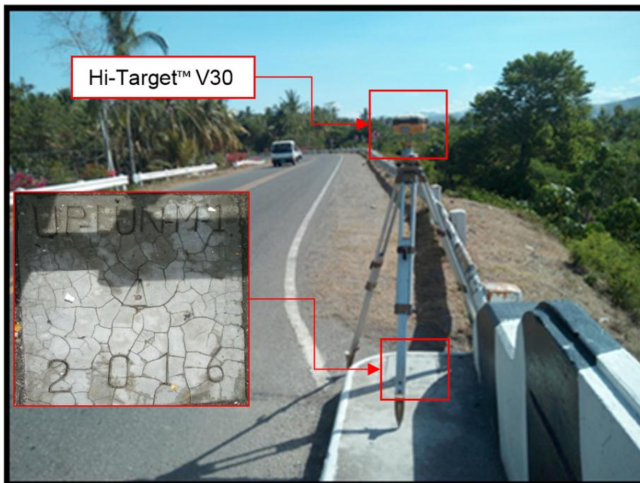
Figure 37. GNSS receiver set up, Hi-Target™ V30, at UP\_LUN-M-1, located at the approach of Lun Masla Bridge in Brgy. Lun Masla, Malapatan, Sarangani
