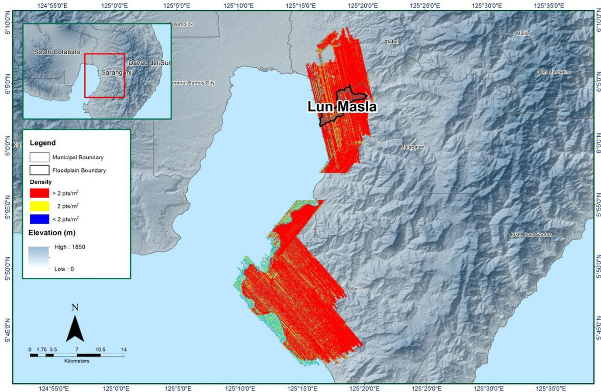
Figure 12. Pulse density map of merged LiDAR data for Lun Masla Floodplain.
