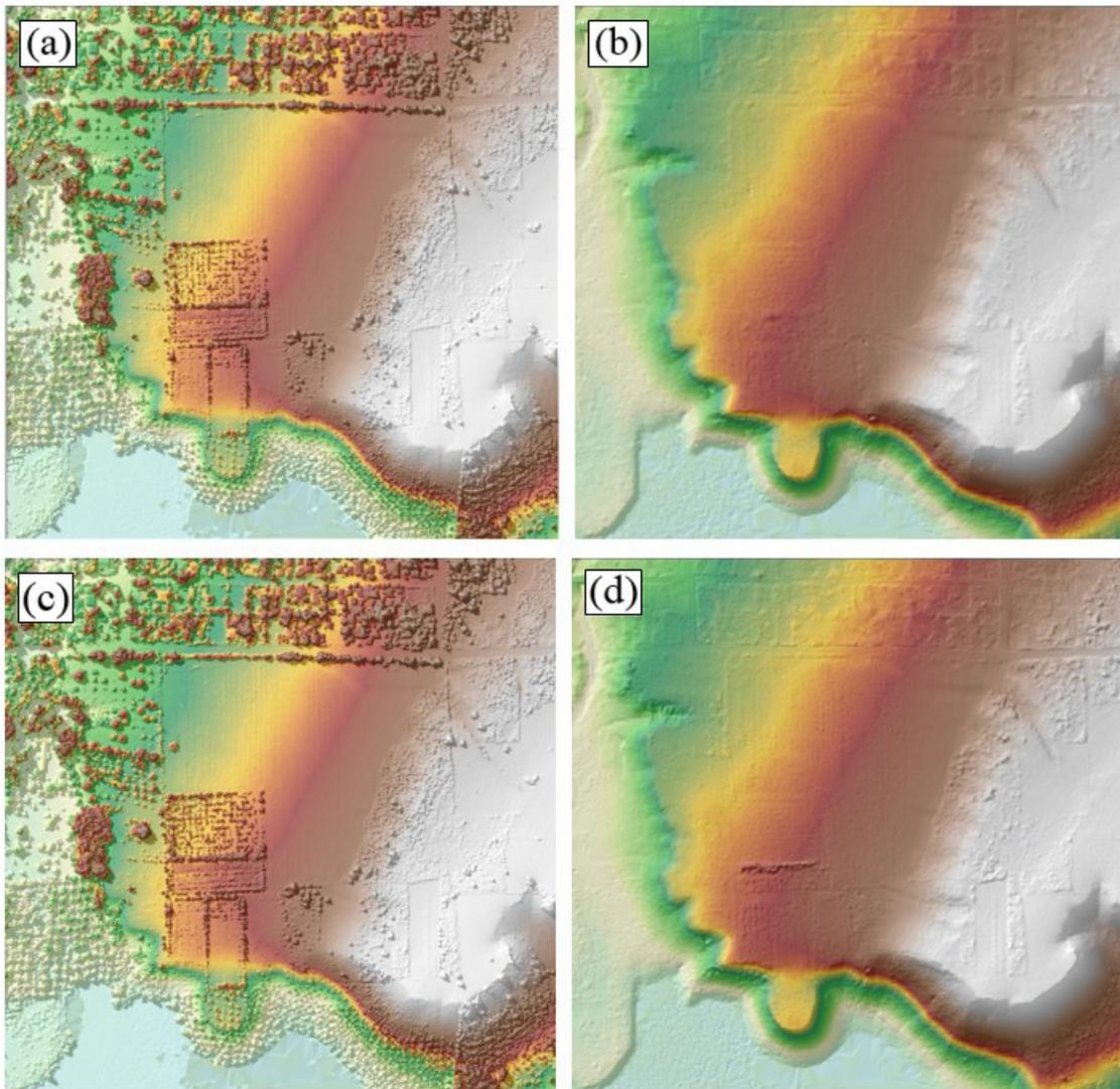
Figure 16. The production of last return DSM (a) and DTM (b), first return DSM (c) and secondary DTM (d) in some portion of Lun Masla Floodplain.
