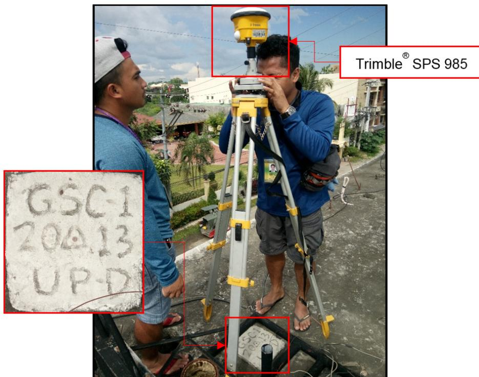
Figure 27. GNSS base set up, Trimble® SPS 985, at GSC-1, located on the rooftop of Ice Castle Experience Hotel in Ambassador Provido Village, Brgy. City Heights, General Santos City, South Cotabato
