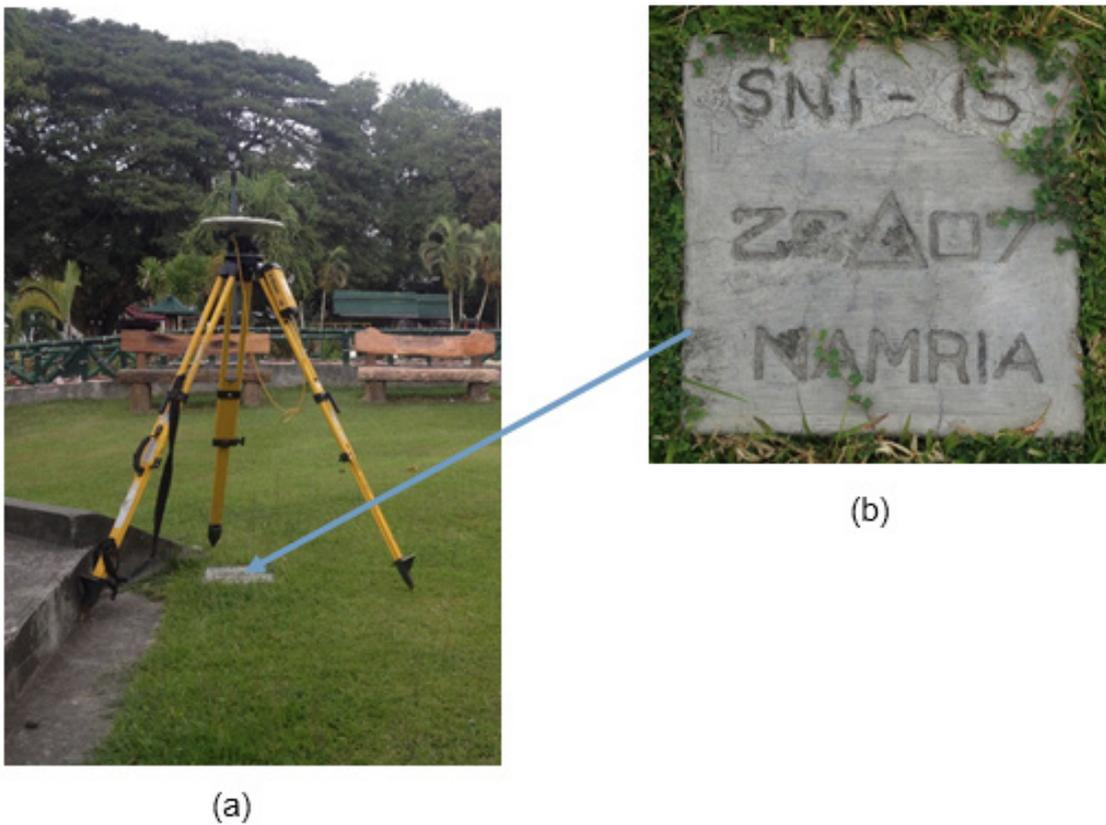
Figure 4. GPS set-up over SNI-15 outside the municipal hall of Malapatan, Sarangani (a) and NAMRIA reference point SNI-15 (b) as recovered by the field team.
