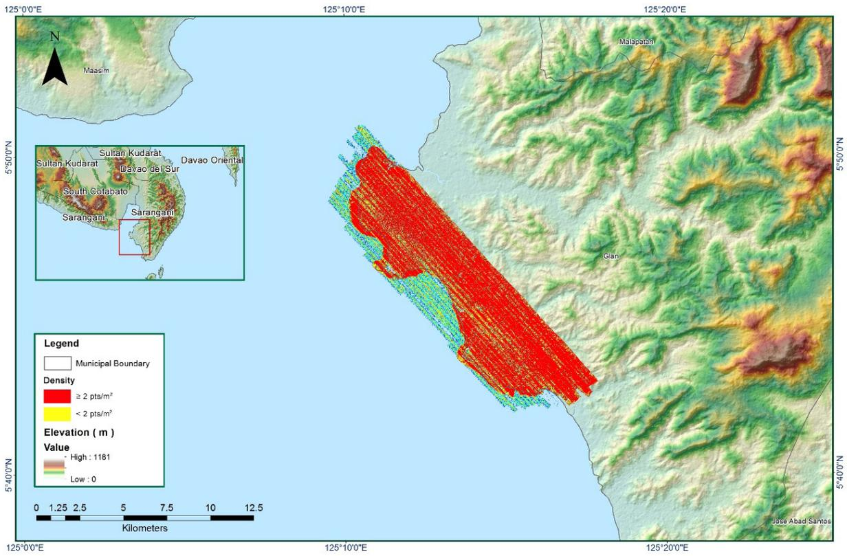
Figure A-8.34. Density of merged LiDAR data
