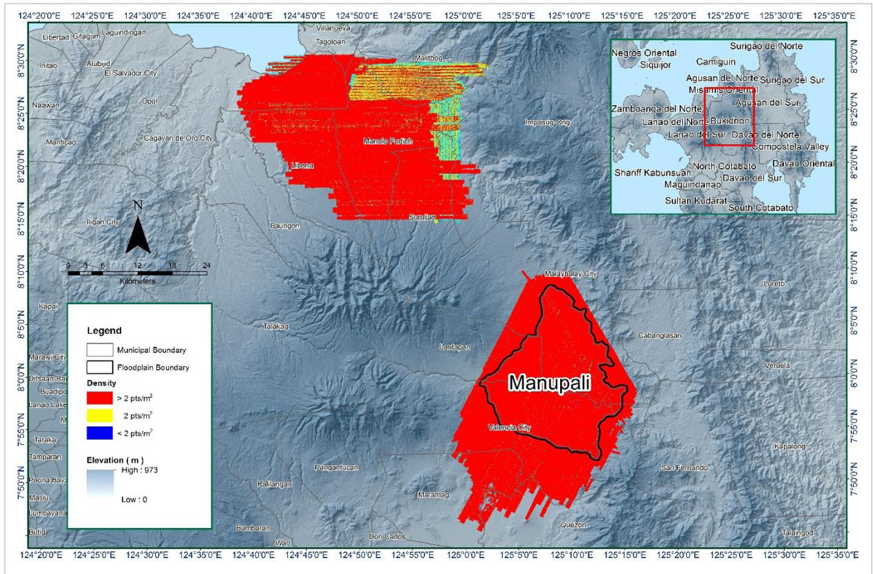
Figure 17. Density map of merged LiDAR data for Manupali floodplain.
