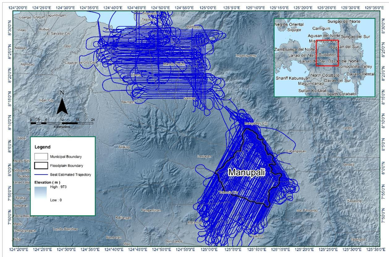
Figure 14. The best estimated trajectory of the LiDAR missions conducted over the Manupali floodplain
