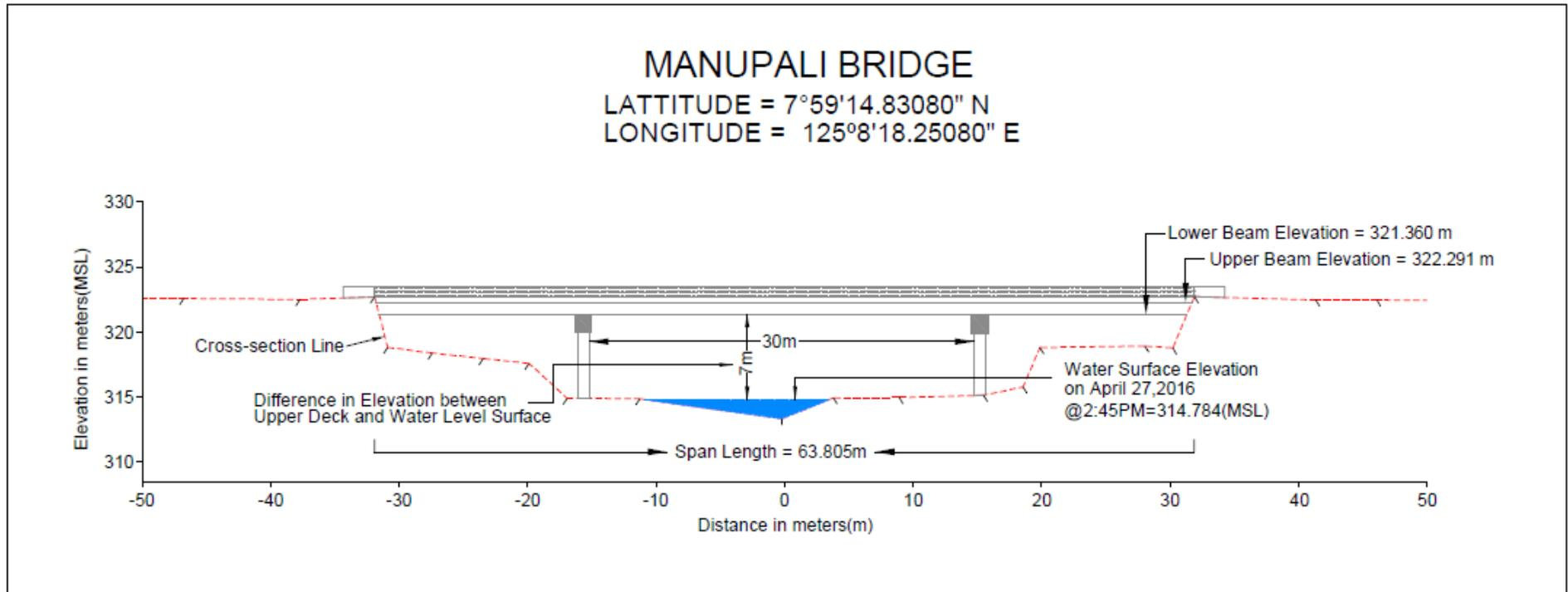
Figure 41. Manupali Bridge Cross-section Diagram
