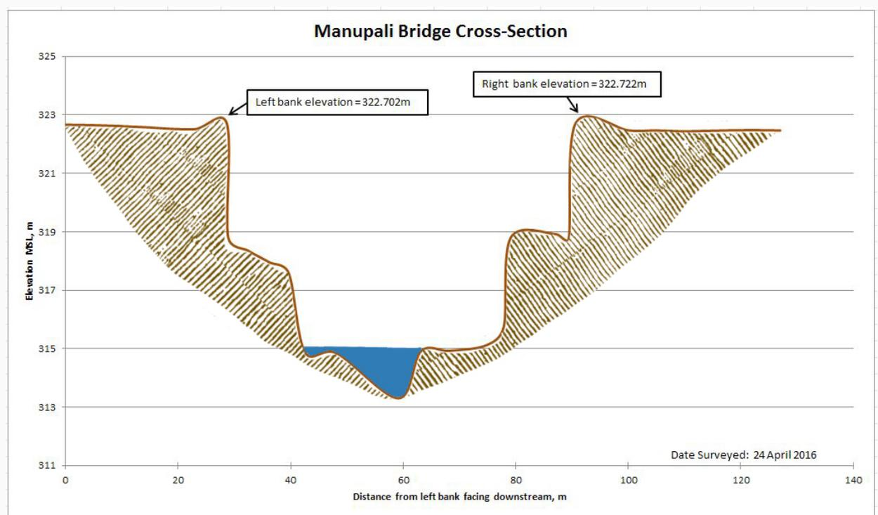
Figure 52. The cross-section plot of the Manupali Bridge
