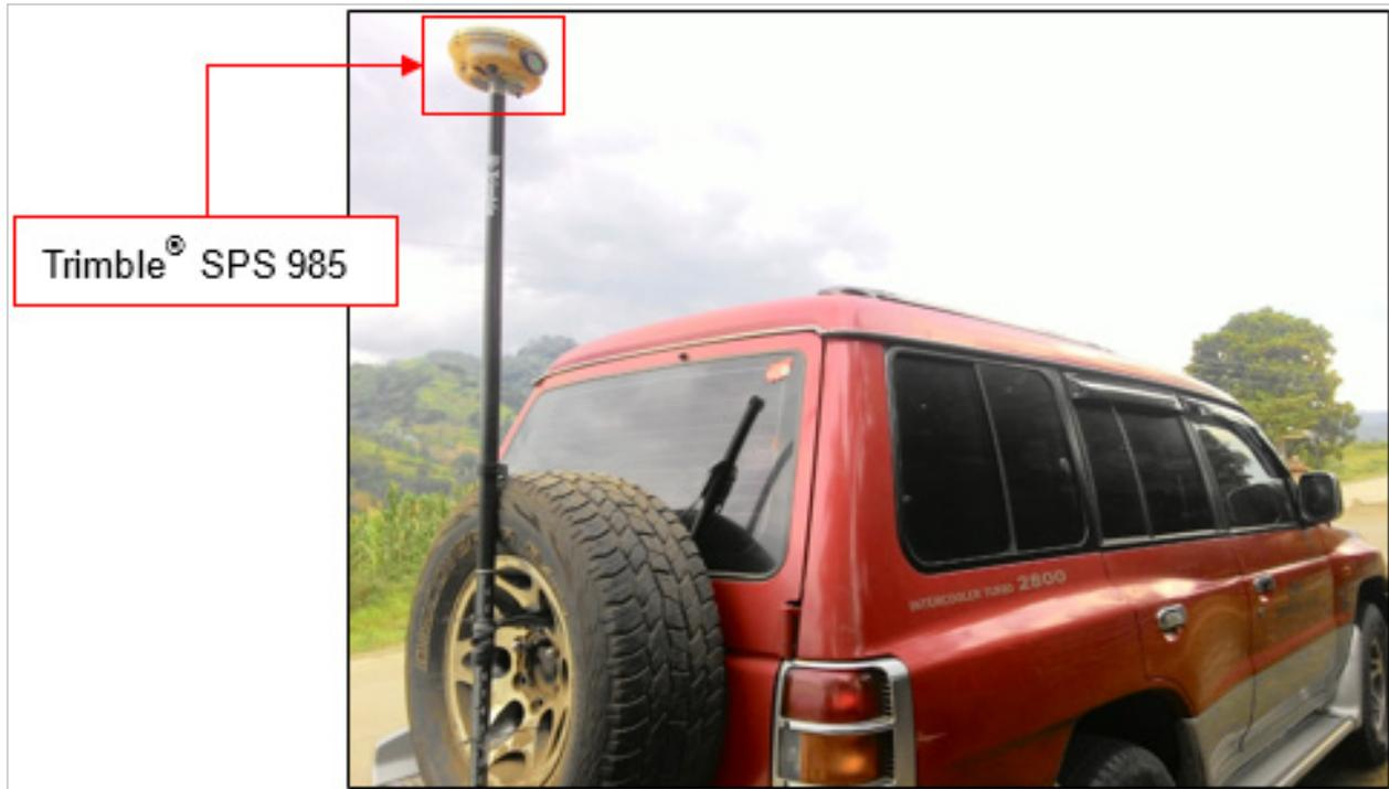
Figure 44. Validation points acquisition survey set-up for Manupali River
