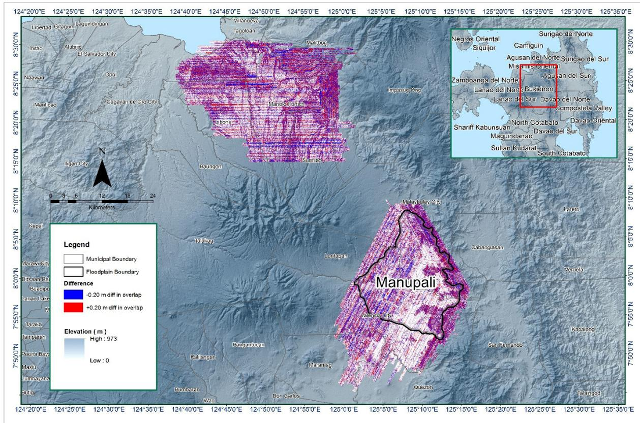
Figure 18. Elevation difference map between flight lines for Manupali floodplain.
