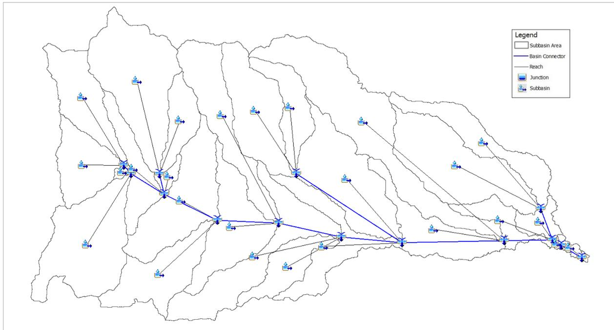
Figure 61. HEC-HMS generated Manupali River Basin Model.
