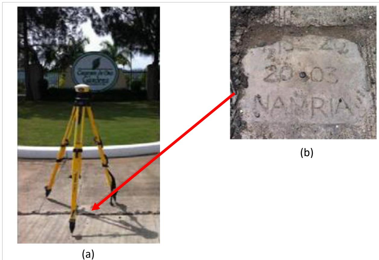
Figure 4. GPS set-up over MSE-20 in front of Cagayan de Oro Gardens Memorial Park, located at Barangay Lumbia, Cagayan de Oro City (a) and NAMRIA reference point MSE-20 (b) as recovered by the field team.
