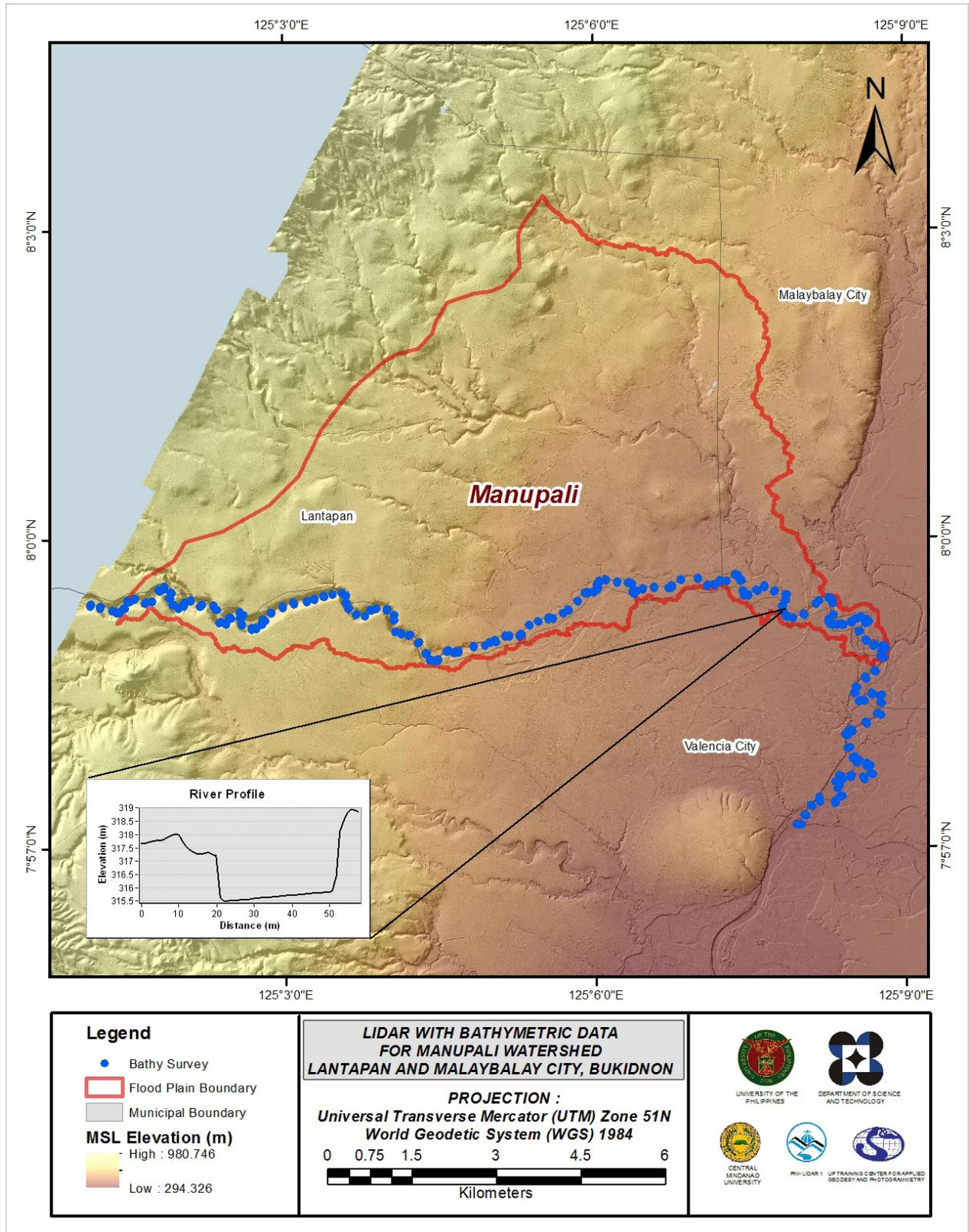
Figure 30. Map of Manupali Flood Plain with bathymetric survey points shown in blue.
