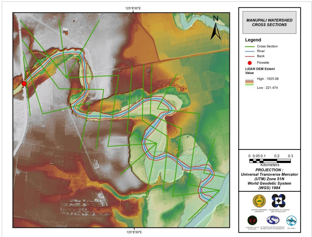
Figure 62. Manupali River Cross-section generated using HEC GeoRAS tool.
