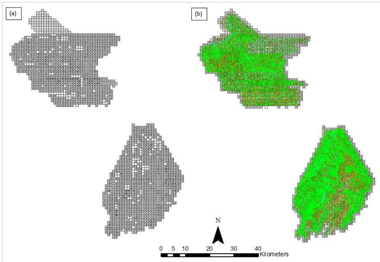
Figure 20. Tiles for Manupali floodplain (a) and classification results (b) in TerraScan.
