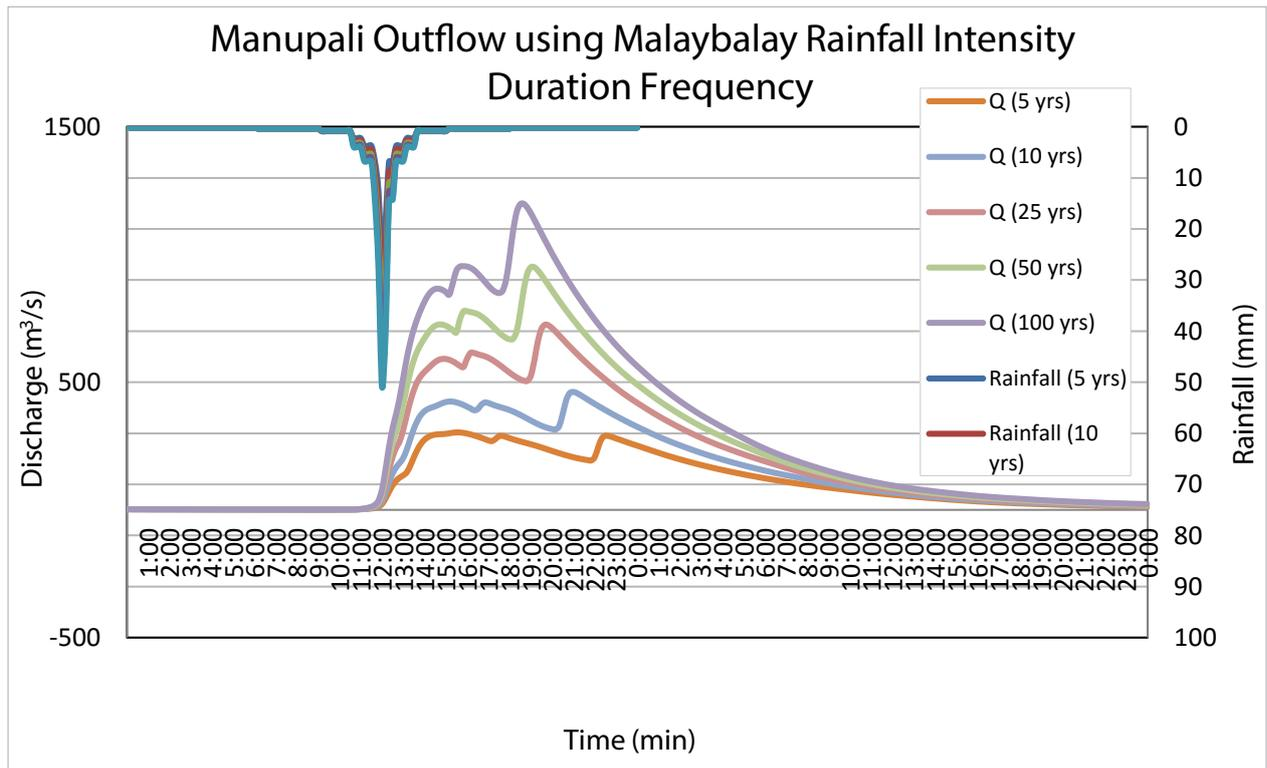
Figure 65. Outflow hydrograph at Manupali Station generated using Malaybalay RIDF simulated in HEC-HMS
