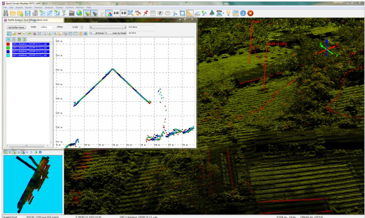
Figure 19. Quality checking for a Manupali flight 23534P using the Profile Tool of QT Modeler.
