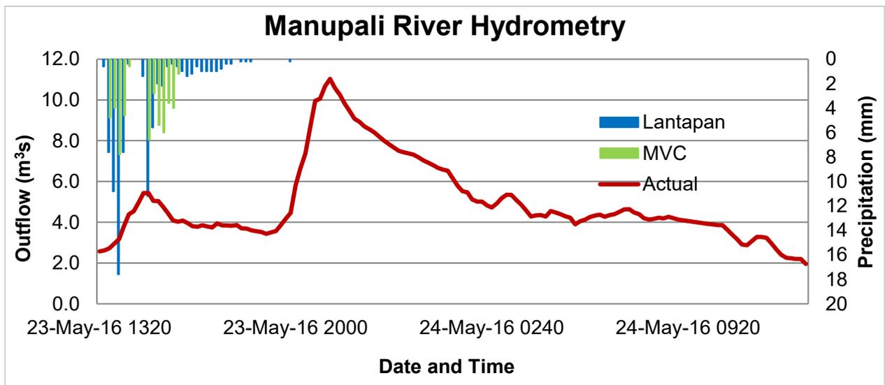
Figure 53. Rainfall and outflow data used for modeling.
