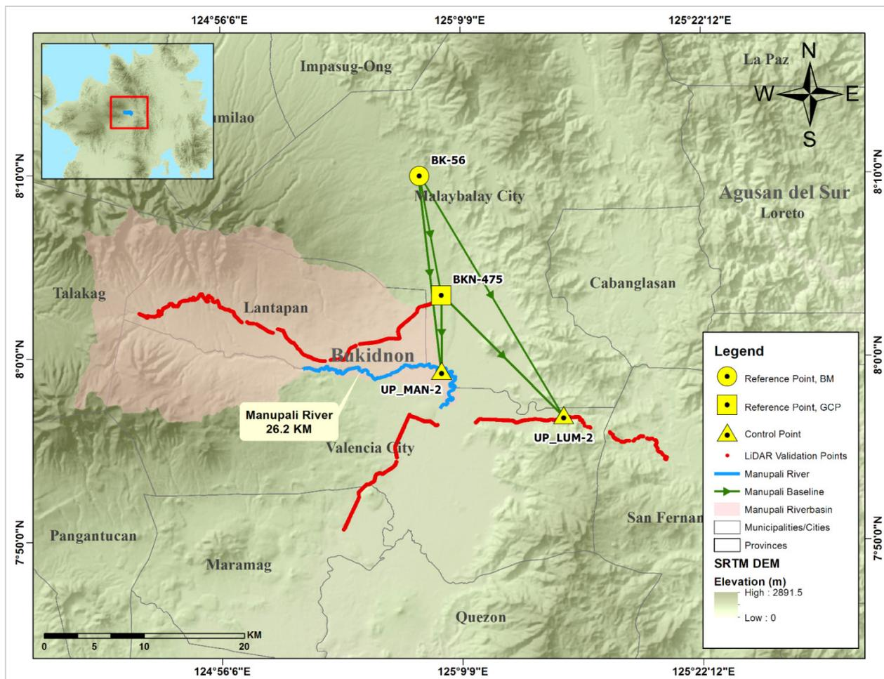
Figure 33. Extent of the bathymetric survey (blue line) in Manupali River and the LiDAR data validation survey (red)
