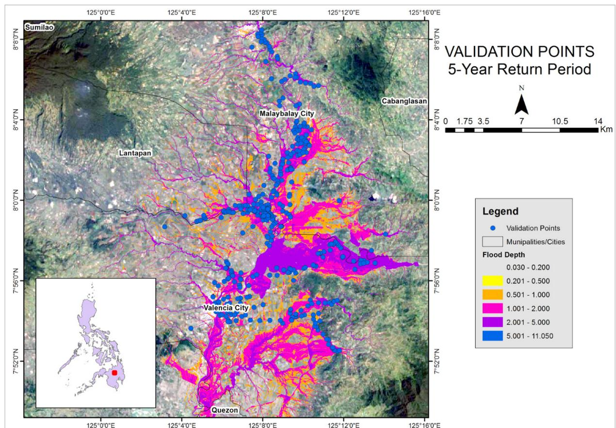
Figure 96. The Validation Points for a 5-year Flood Depth Map of the Manupali-Sawaga-Upper Pulangi Floodplain
