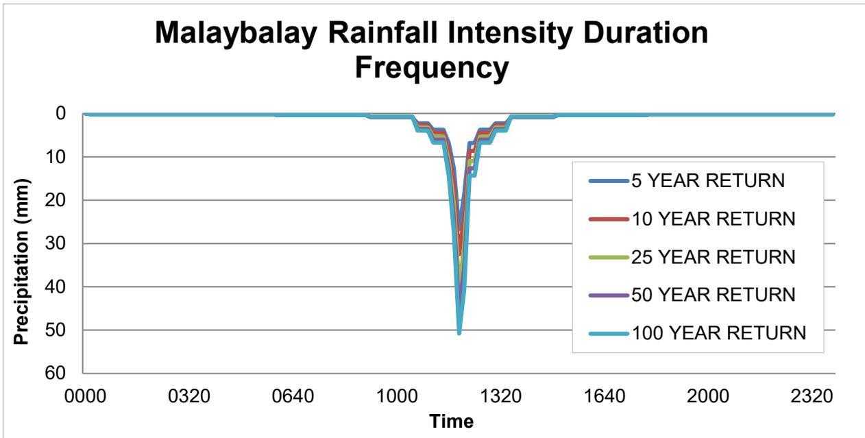
Figure 56. Synthetic storm generated for a 24-hr period rainfall for various return periods.
