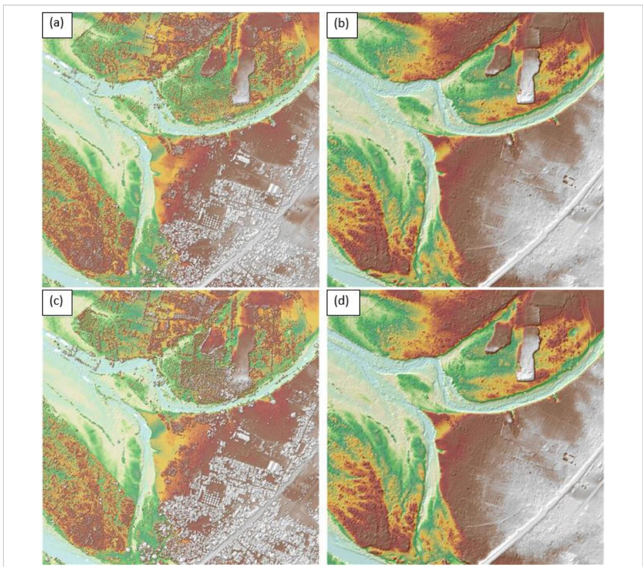
Figure 22. The production of the last return DSM (a) and DTM (b), first return DSM (c) and secondary DTM (d) in some portion of Manupali floodplain
