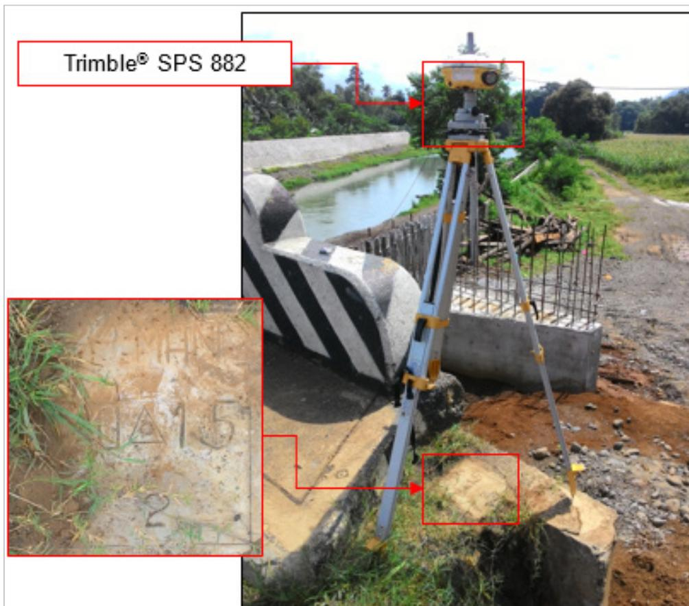
Figure 37. GNSS receiver set up, Trimble® SPS 882, at UP\_MAN -2, located near the approach of Manupali Bridge in Brgy. Bangcud, Malaybalay City, Province of Bukidnon
