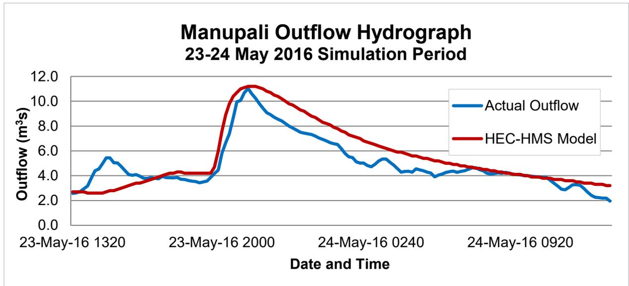
Figure 64. Outflow Hydrograph of Manupali produced by the HEC-HMS model compared with observed outflow.
