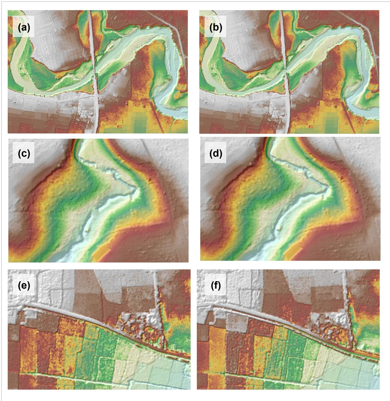
Figure 25. Portions in the DTM of Manupali floodplain – a bridge before (a) and after (b) manual editing; a point of high elevation before (c) and after (d) manual editing; and a paddy field before (e) and after (f) data retrieval.
