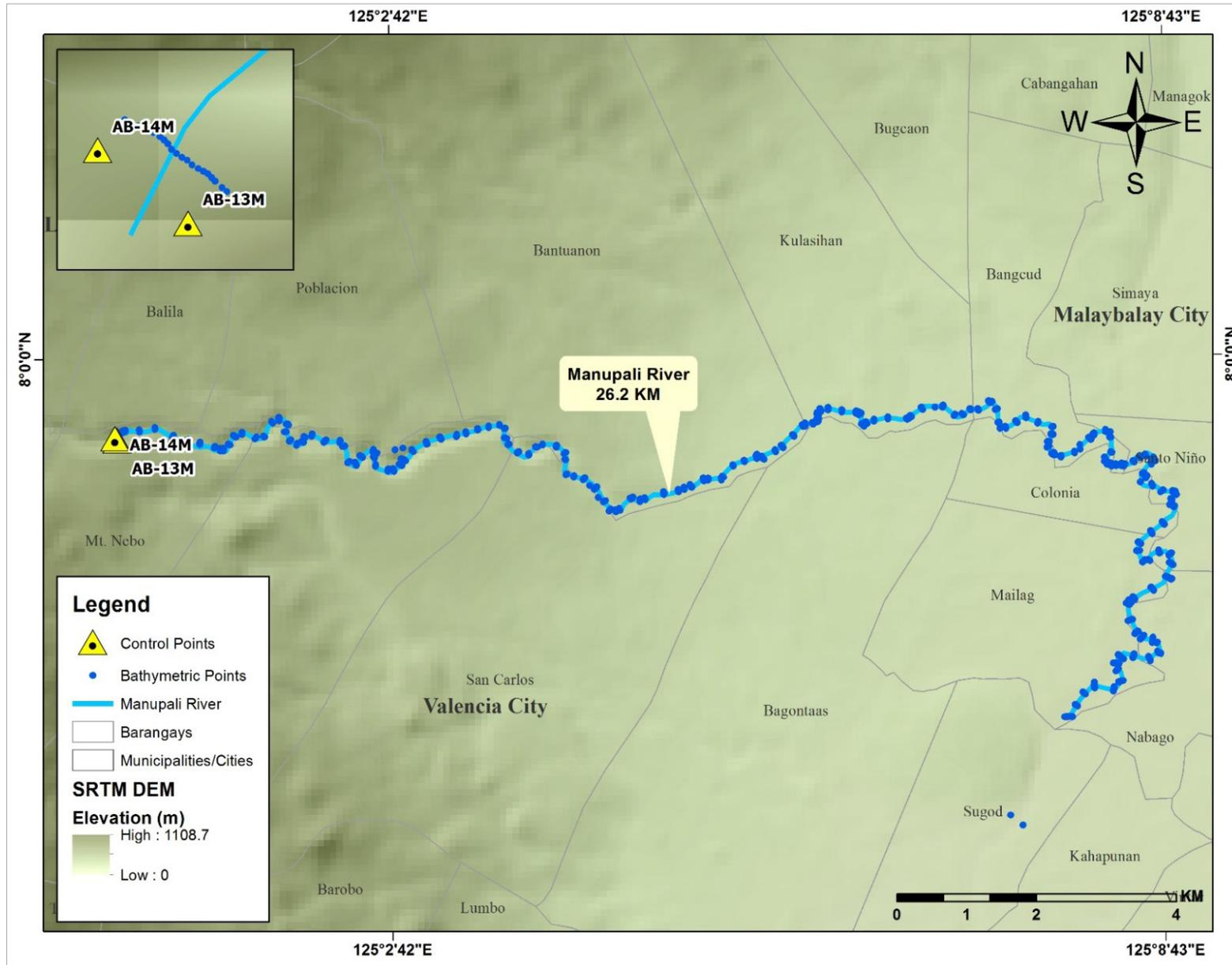
Figure 48. Bathymetric survey of Manupali River
