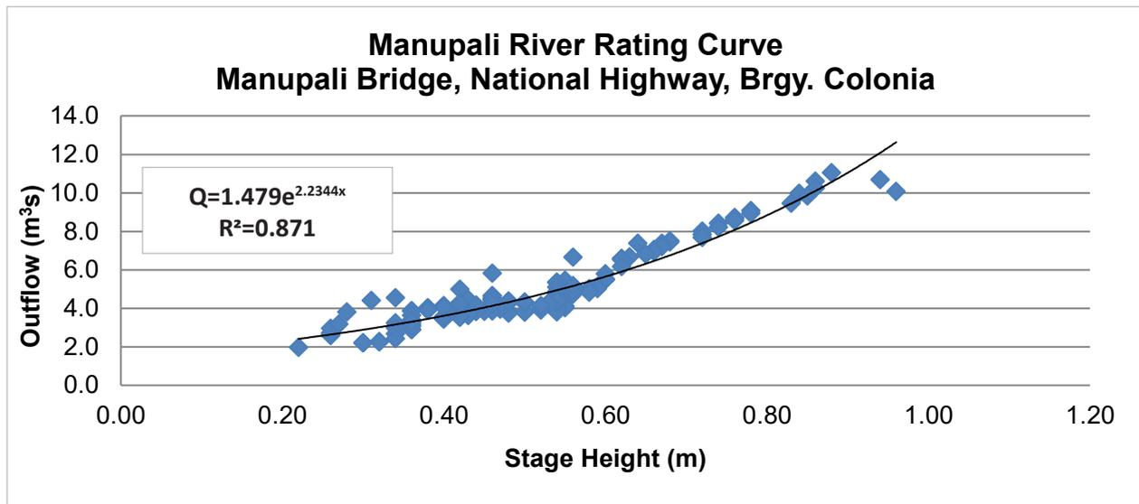
Figure 54. HQ Curve of HEC-HMS model.
