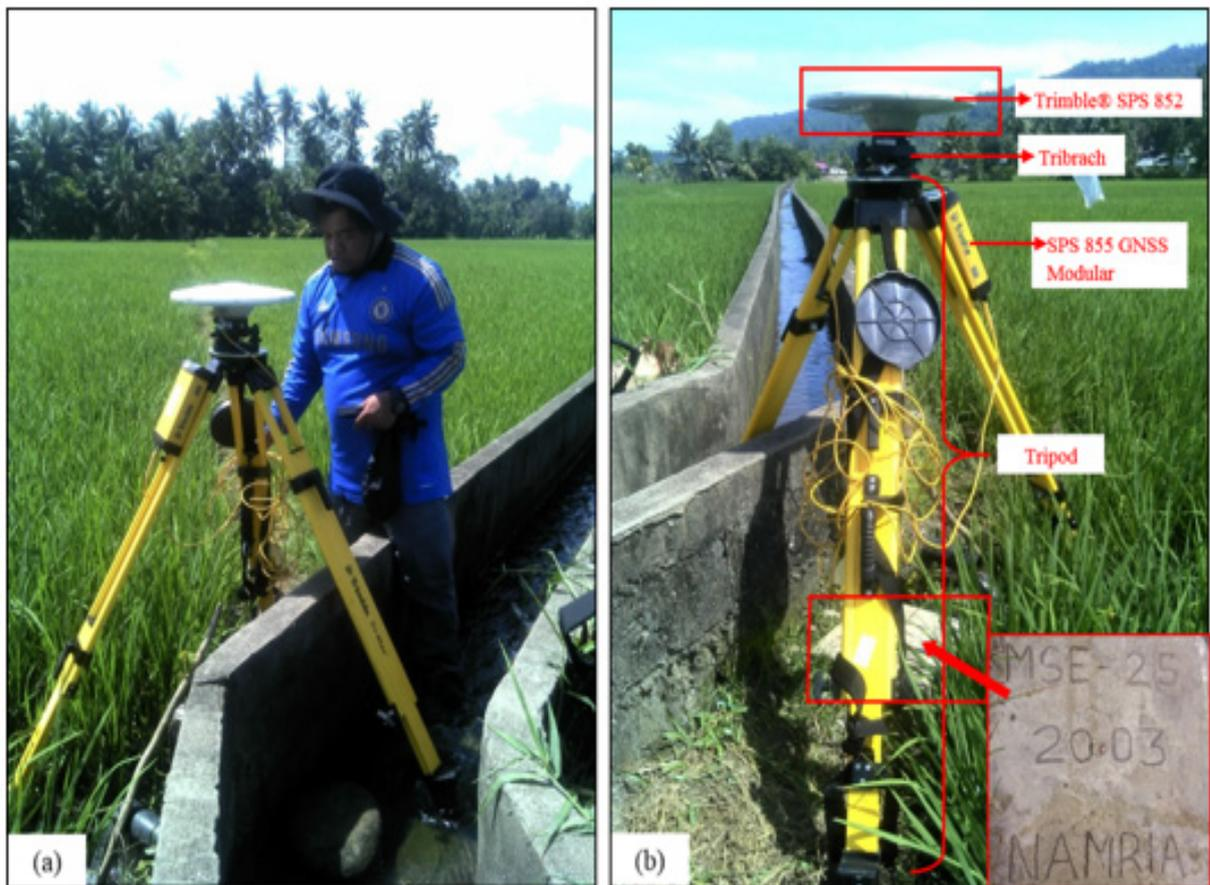
**Figure 33. GNSS base receiver setup, Trimble® SPS 852 at MSE-25 in Brgy. Poblacion 1, Municipality of Villanueva, Misamis Oriental**
