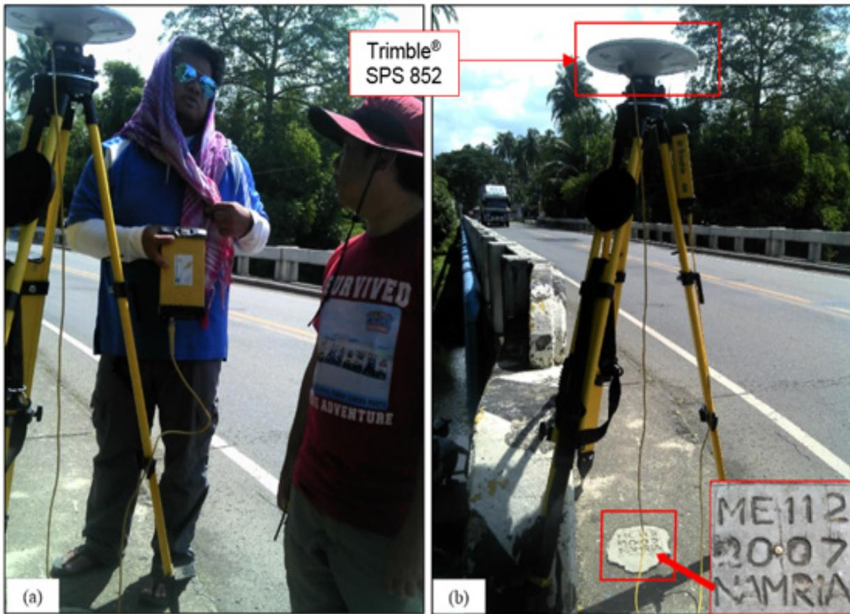
Figure 34. GNSS base receiver setup, Trimble® SPS 852 at ME-112 at Musi-Musi Bridge in Brgy. Talusan, Municipality of Balingasag, Misamis Oriental.
