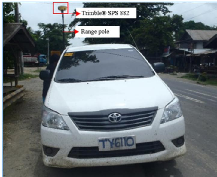
*Figure 42. Ground validation set-up*
