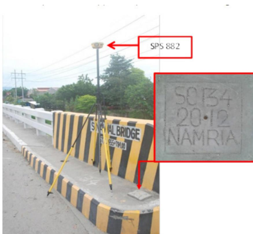
Figure 31. GNSS base set up, Trimble® SPS 882, at SC-134-43, at the approach of Sinawal Bridge in Brgy. Sinawal, General Santos City
