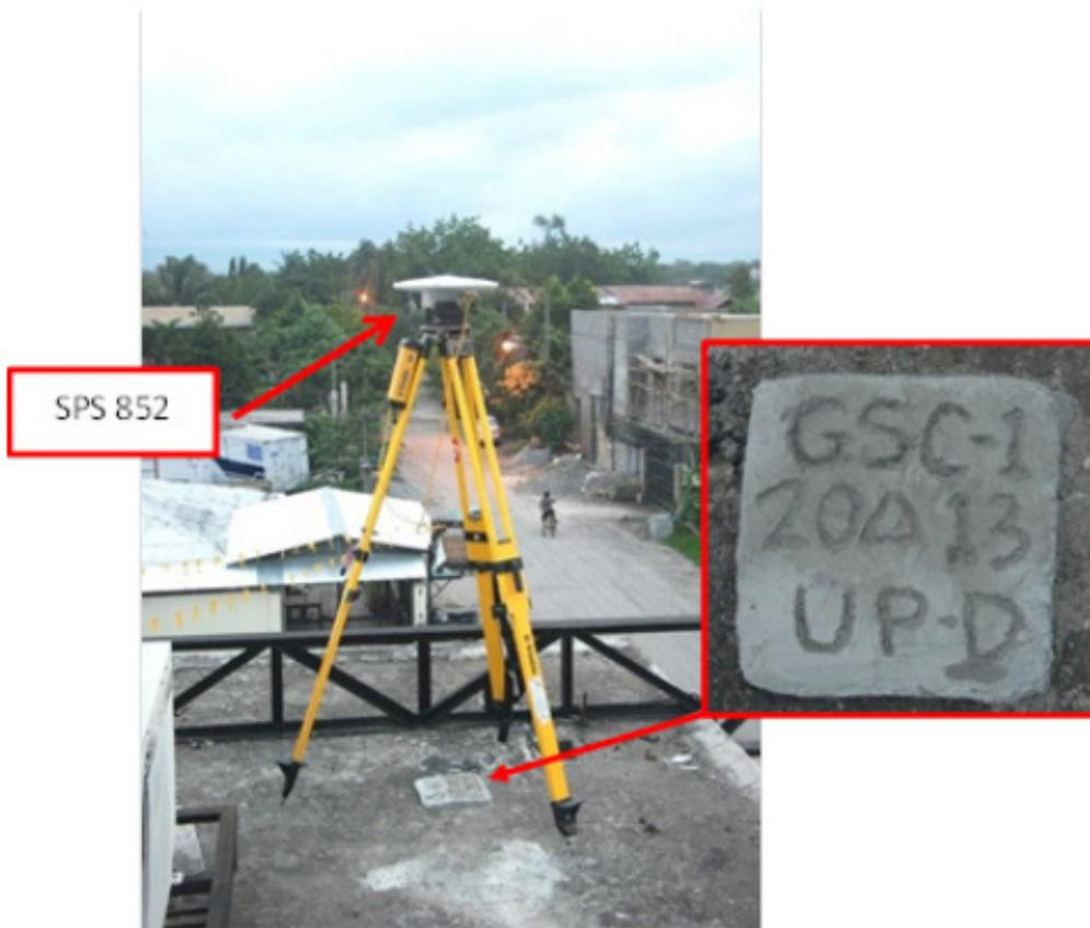
Figure 32. Trimble SPS® 882 set-up at AN-9 located at the approach of Silway Bridge, Brgy. Kauswagan, Silway City, Agusan Del Norte
