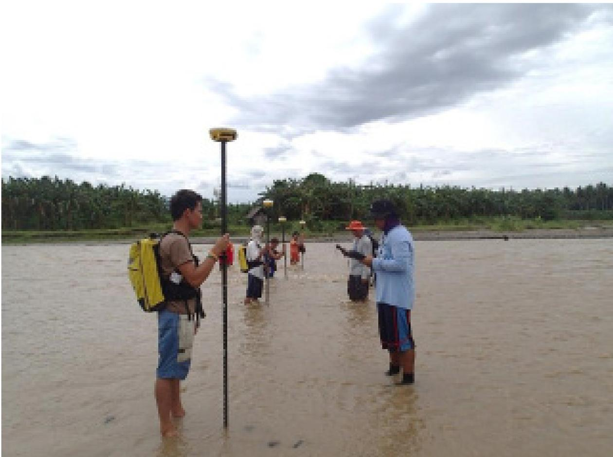
Figure 34. Manual bathymetric survey at Silway River using PPK GNSS technique
