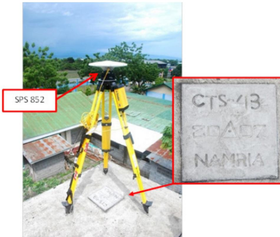
Figure 30. GNSS base set up, Trimble® SPS 852, at CTS-43, in Brgy. Tambler, General Santos City
