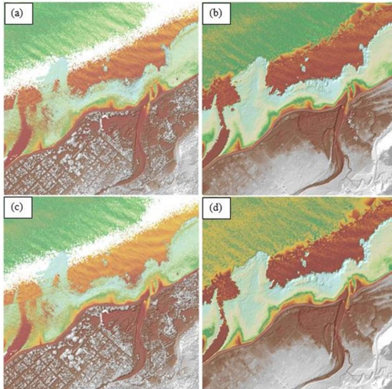
Figure 19 The production of last return DSM (a) and DTM (b), first return DSM (c) and secondary DTM (d) in some portion of Cantilan Floodplain
