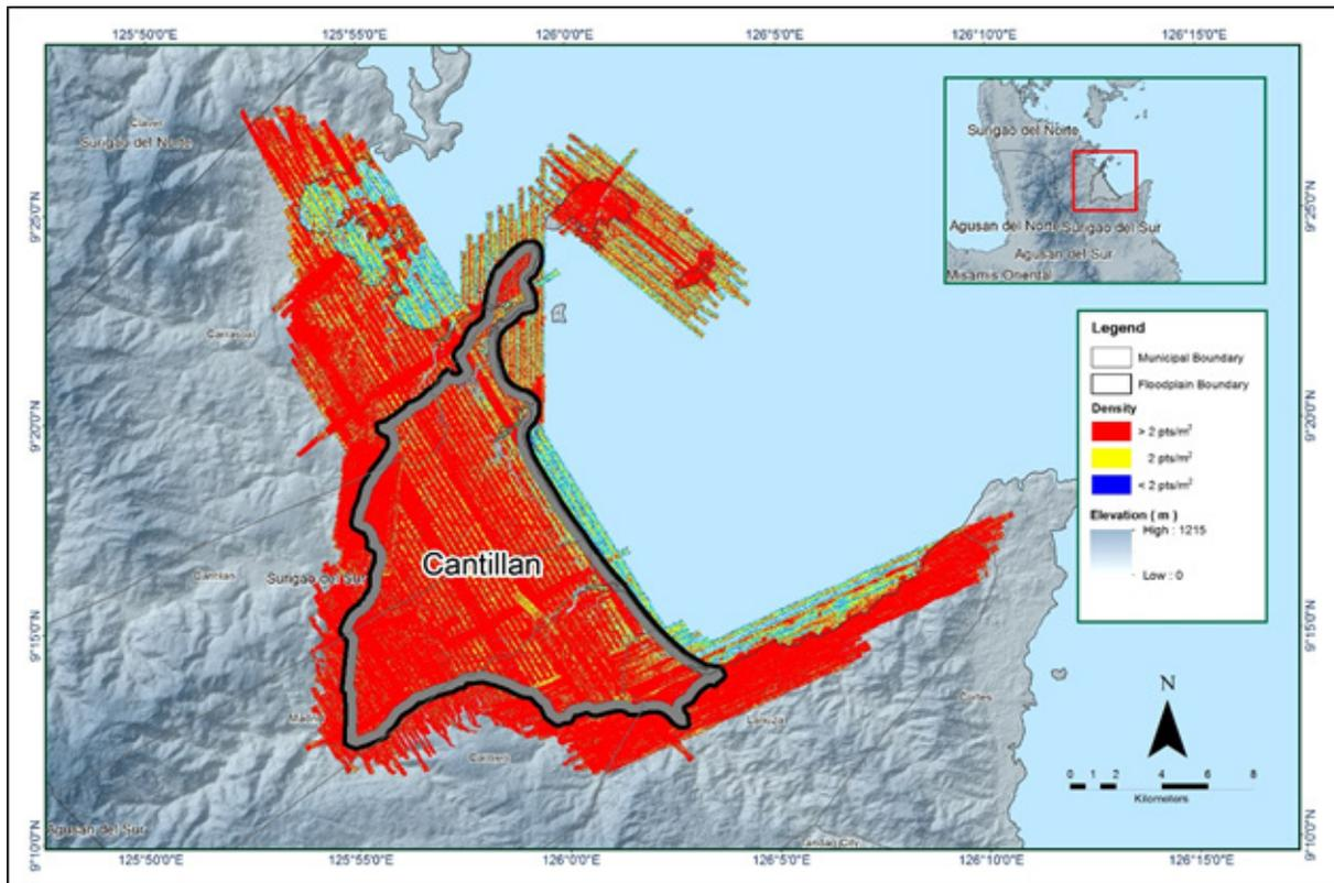
Figure 14 Density map of merged LiDAR data for Cantilan Floodplain
