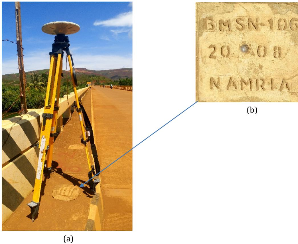
Figure 5 GPS set-up over SN-106 located on the first approach of Claver bridge going to Surigao del Sur (a) and NAMRIA reference point SN-106 (b) as recovered by the field team
