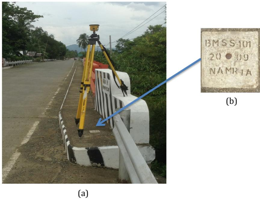
Figure 3 GPS set-up over SS-101 located at the first approach of Antao Bridge KM. post 1249+122.90 near a concrete electric post in Brgy. Antao, Carmen, Surigaodel Sur (a) and NAMRIA reference point SS-101 (b) as recovered by the field team.
