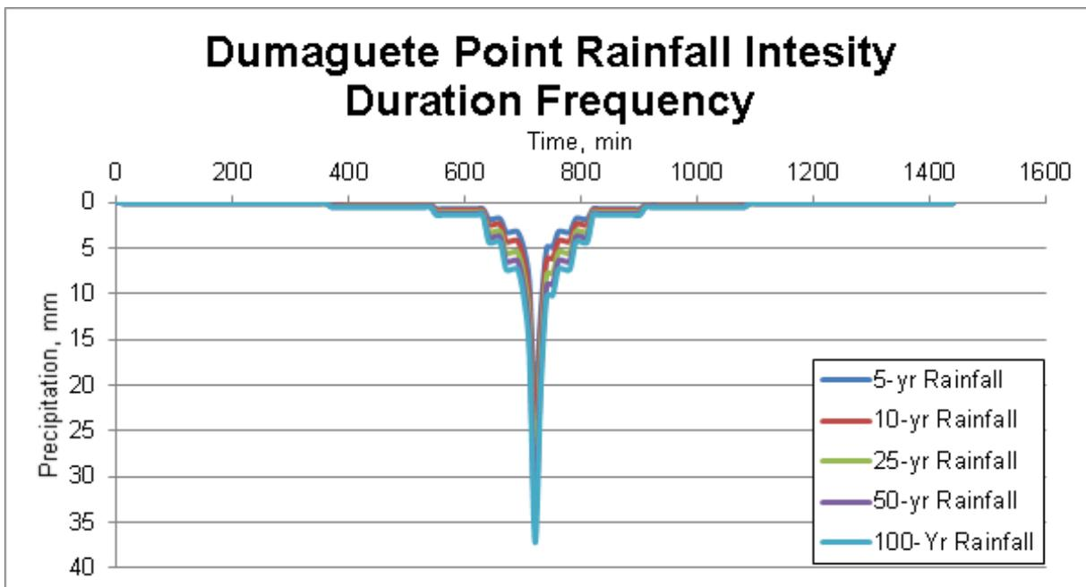
Figure 49. The synthetic storm generated for a 24-hour period rainfall for various return periods.
