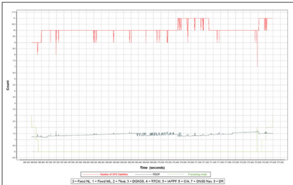
Figure 10 Solution Status Parameters of Cantilan Flight 8490A
