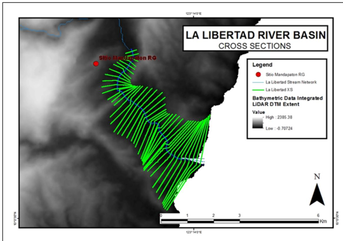
Figure 54. River cross-section of the Libertad River through the ArcMap HEC GeoRas tool.
