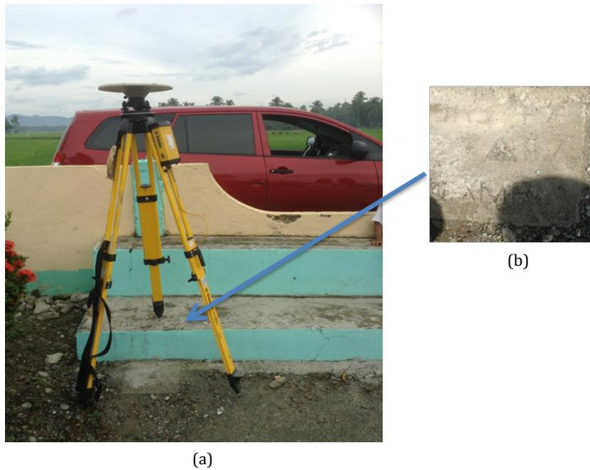
Figure 4 GPS set-up over SRS-47 located on the left side ground corner of the barangay hall about 60m from the crossing in Brgy. Manga, Madrid, Surigao del Sur (a) NAMRIA reference point SS-101 (b) as recovered by the field team
