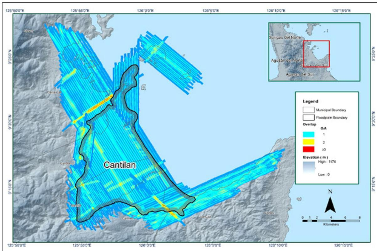
Figure 13 Image of data overlap for Cantilan Floodplain
