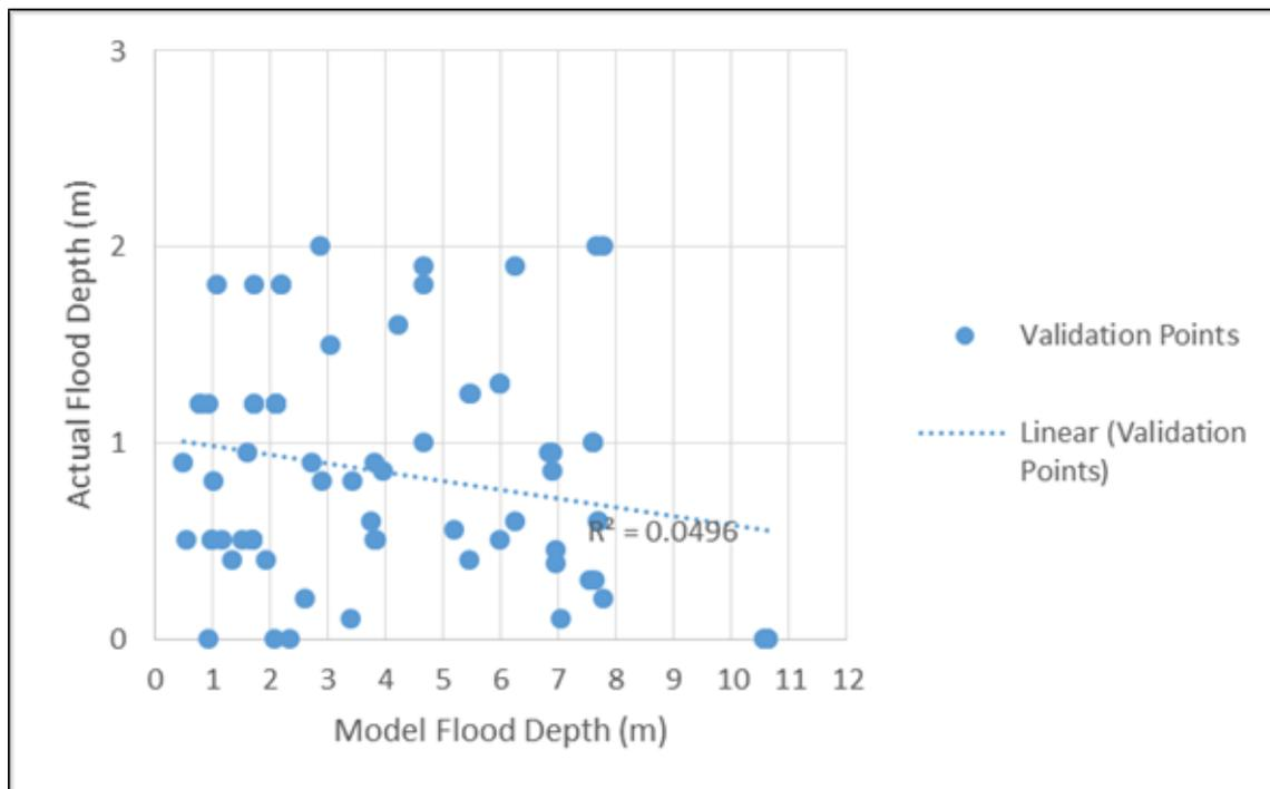
Figure 75. Flood Map depth versus Actual Flood Depth.
