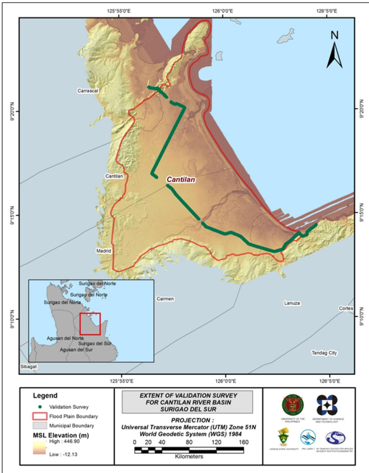
Figure 24 Map of Cantilan Floodplain with validation survey points in green
