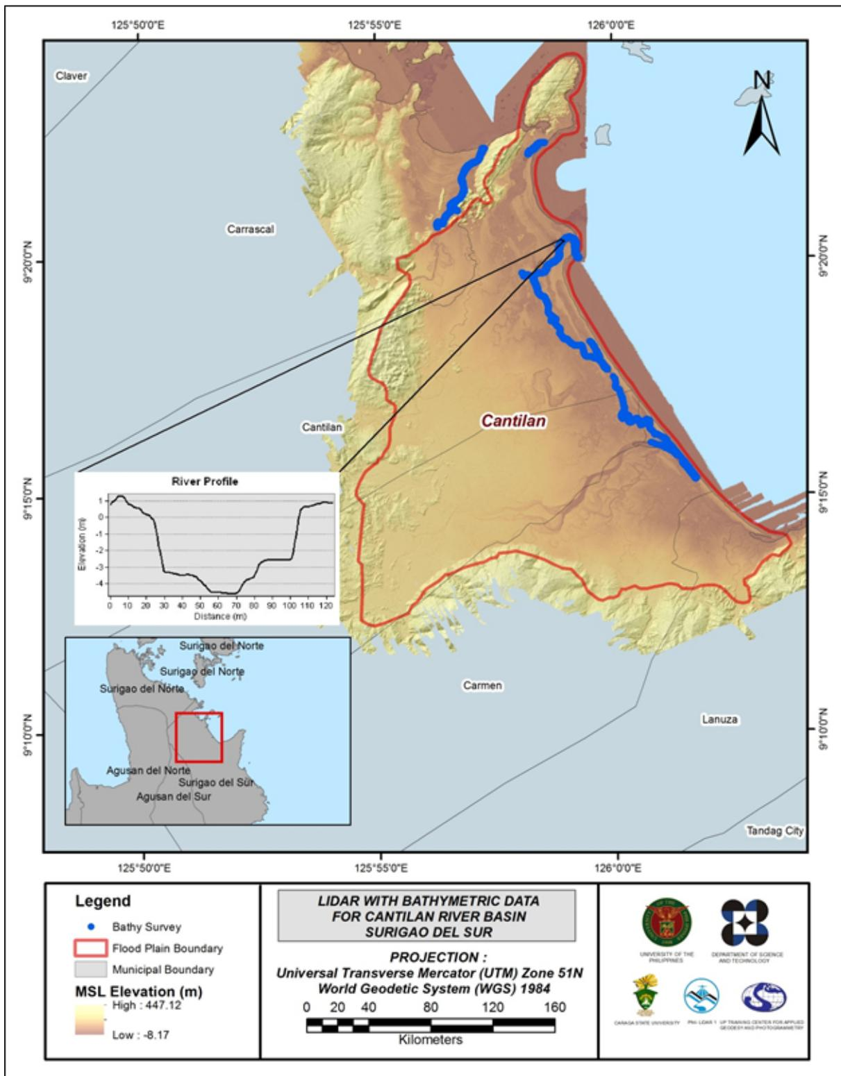
Figure 27 Map of Cantilan Floodplain with bathymetric survey points shown in blue
