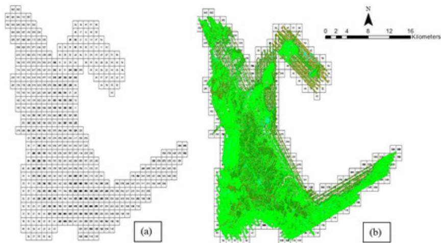
Figure 17 Tiles for Cantilan Floodplain (a) and classification results (b) in TerraScan
