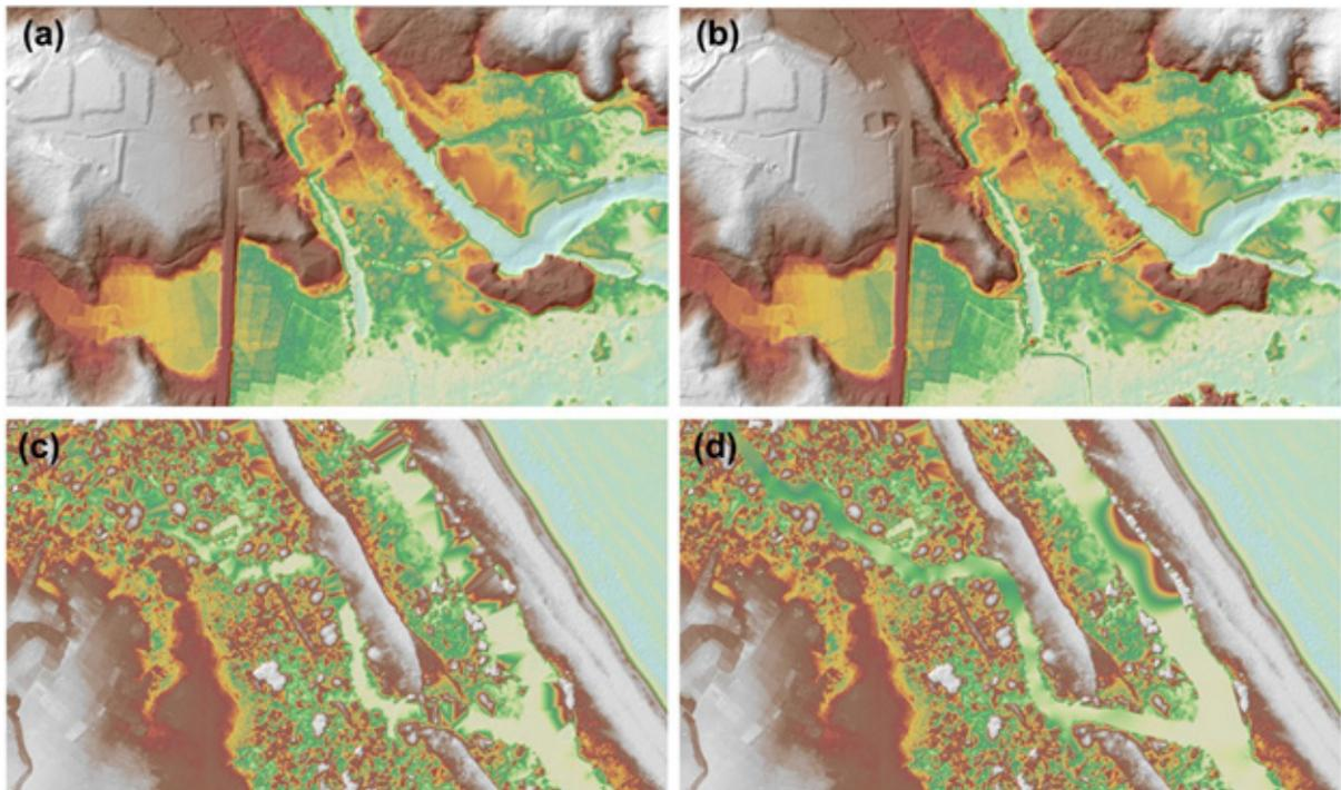
Figure 22 Portions in the DTM of Cantilan floodplain – a bridge before (a) and after (b) manual editing; and a paddy field before (c) and after (d) data retrieval
