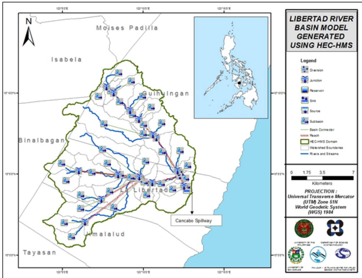
Figure 53. Libertad river basin model generated in HEC-HMS.
