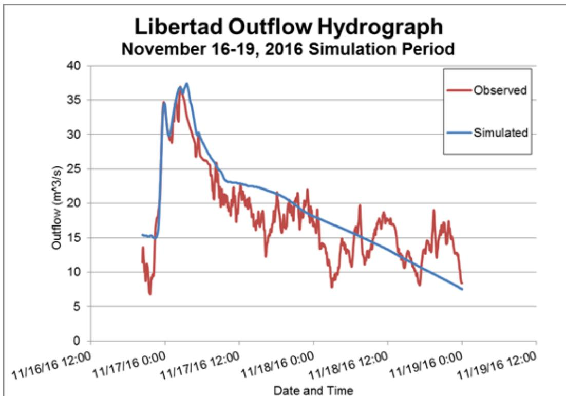
Figure 56. Outflow Hydrograph of Libertad produced by the HEC-HMS model compared with observed outflow.
