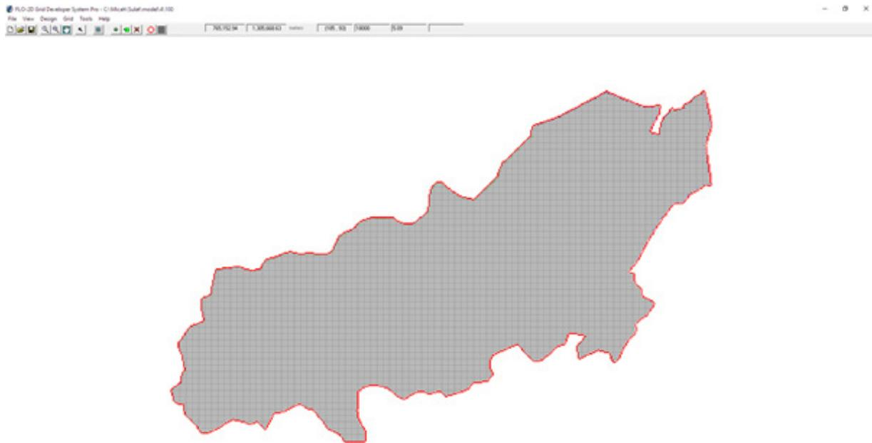
Figure 55. A screenshot of the river sub-catchment with the computational area to be modeled in FLO-2D Grid Developer System Pro (FLO-2D GDS Pro).
