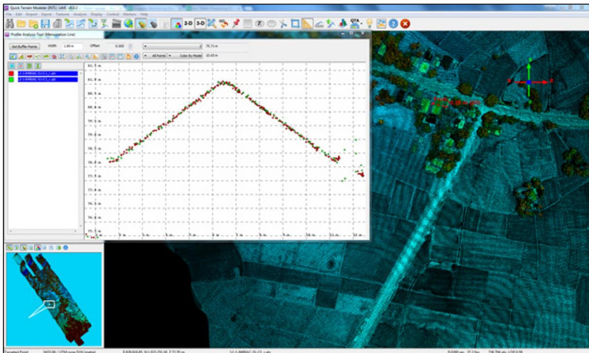
Figure 16 Quality checking for a Cantilan flight 8490A using the Profile Tool of QT Modeler
