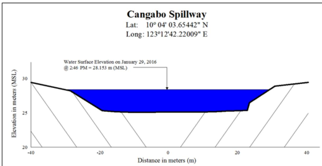
Figure 36. Deployment site, Cangabo Spillway, cross-section diagram
