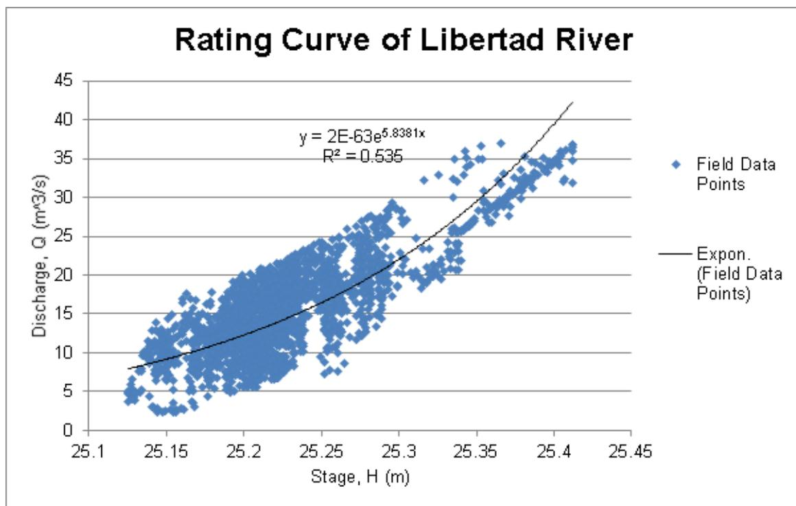
Figure 46. The rating curve at Libertad Bridge, Bohol.
