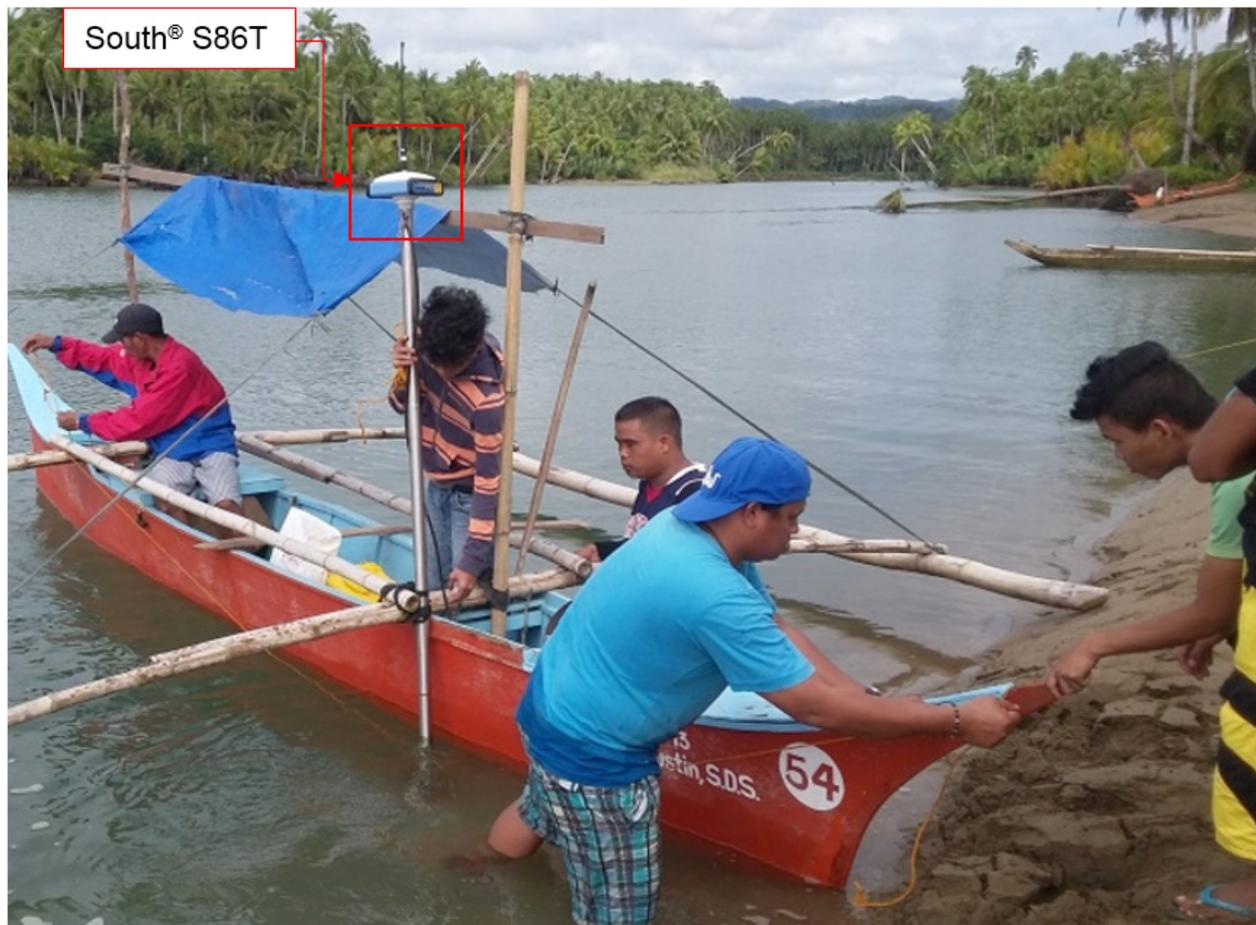
Figure 39. Set up of the bathymetric survey in Hubo-Otieza River
