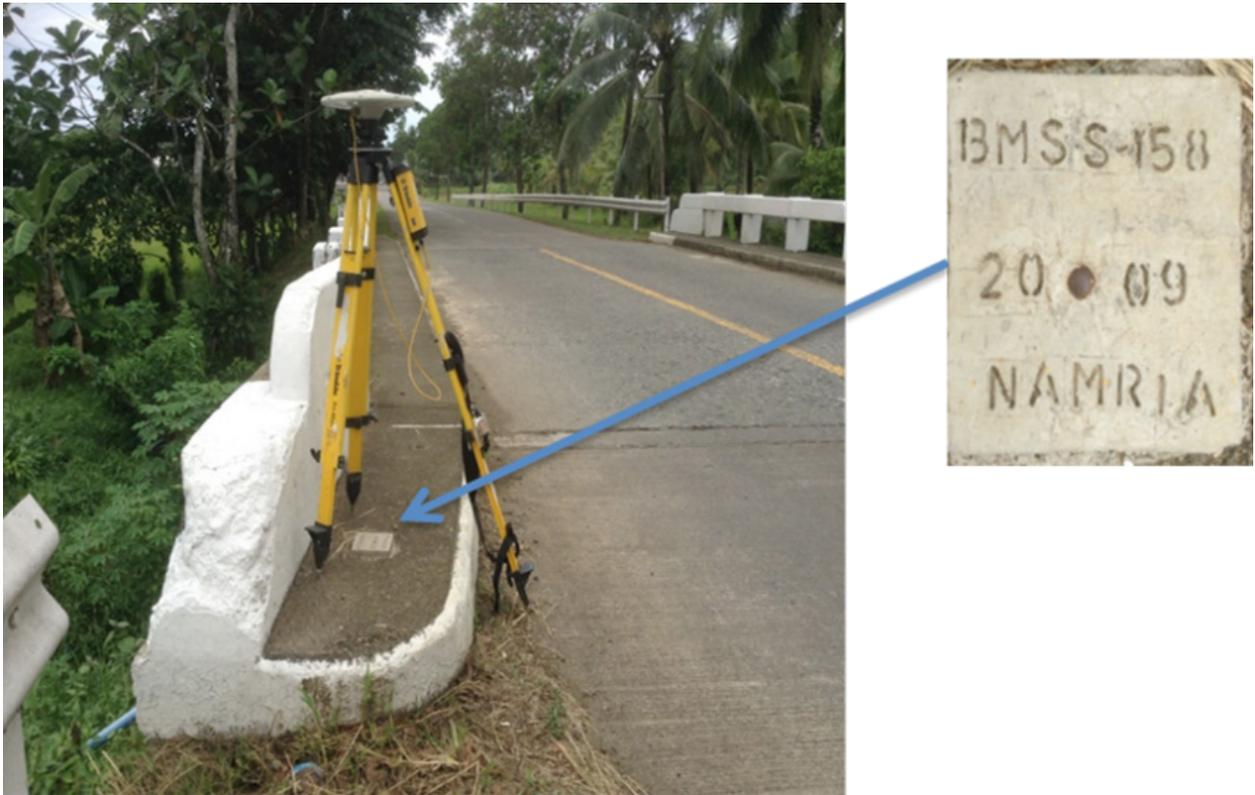
Figure 5. GPS set-up over SS-158 located at Batang Bridge in Brgy. Dayo-an, Surigao del Sur (a) and NAMRIA reference point SM-286 (b) as recovered by the field team.
