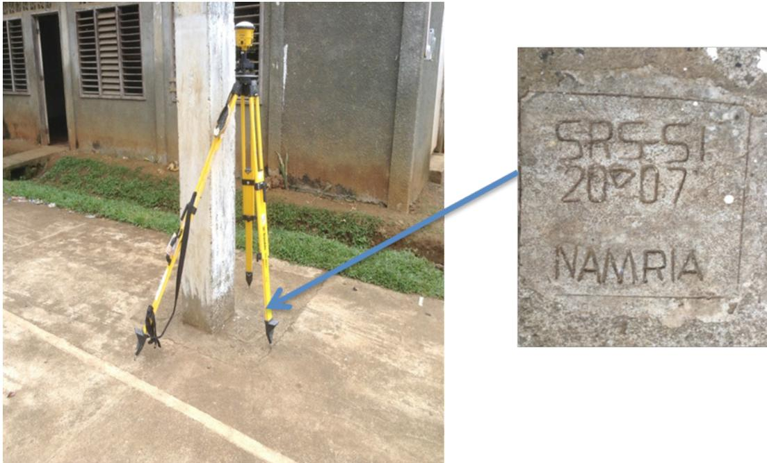
Figure 3. GPS set-up over SRS-51 recovered inside the compound of the barangay hall, beside the basketball court in Brgy. Bajao, Tandag, Surigao del Sur (a) and NAMRIA reference point SMR-33 (b) as recovered by the field team.
