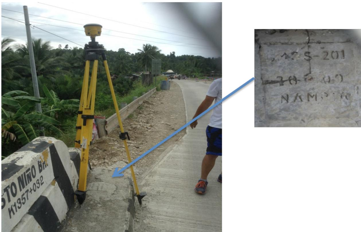
Figure 6. GPS set-up over SS-201 located in Sto. Nino Bridge in San Agustin, Surigao del Sur (a) and NAMRIA reference point SM-201 (b) as recovered by the field team.
