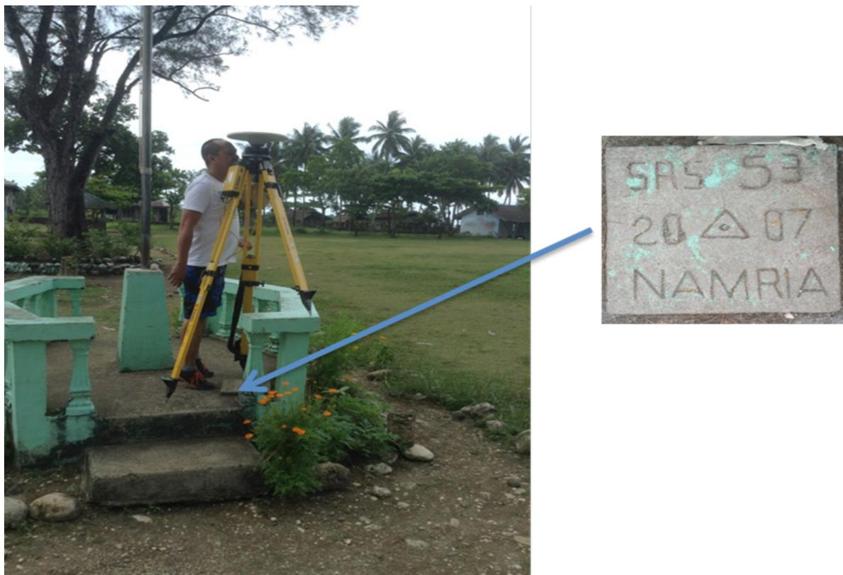
Figure 4. GPS set-up over SRS-53 located in the NE corner of the flagpole of San Agustin Central Elementary School in Brgy. San Agustin, Surigao del Sur (a) and NAMRIA reference point SMR-53 (b) as recovered by the field team..
