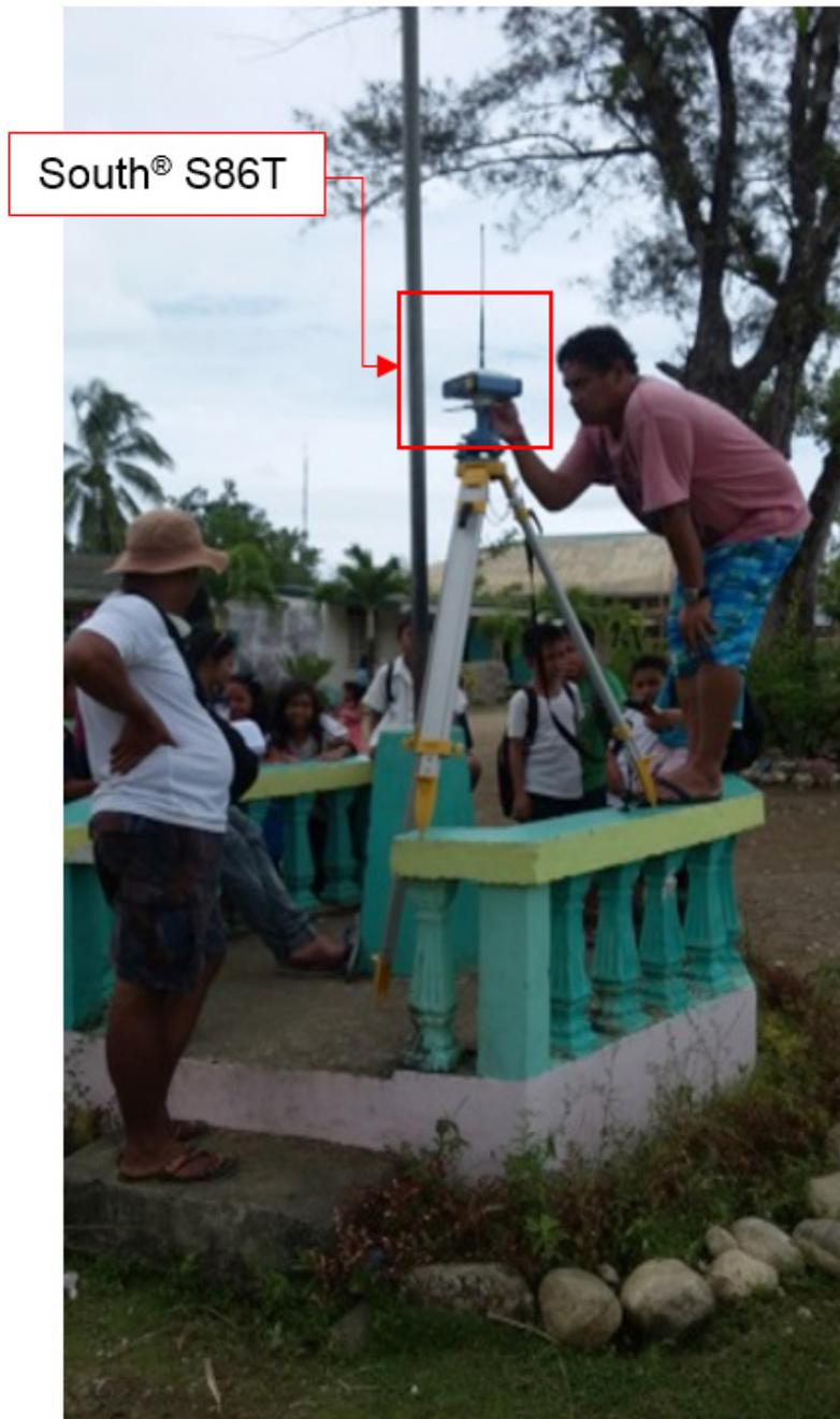
Figure 32. The GNSS base receiver setup, South<sup>®</sup> S86T, at SRS-53 in San Agustin Central Elementary School in Surigao Del Sur
