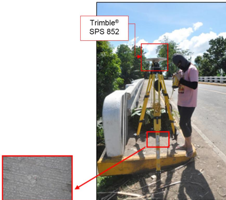
Figure 33. GNSS base receiver setup, Trimble® SPS 852, at SS-202 in Brgy. Otieza, Municipality of San Agustin, Surogao Del Sur
