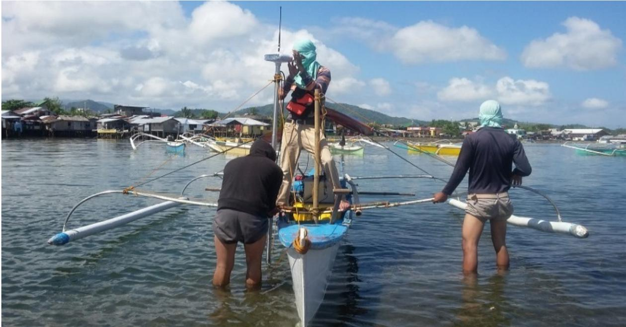
Figure 41. Bathymetric survey of CSU at Magallanes River using Hi-Target V30
