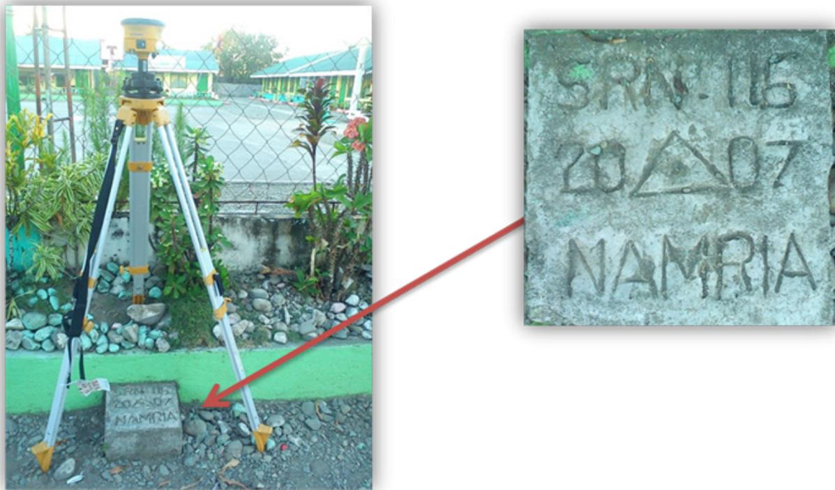
Figure 5. GPS set-up over SRN-116 in front of Ipil Primary School, near the concrete fence located at Gigaquit, Surigao Del Norte (a) and NAMRIA reference point SRN-116 (b) as recovered by the field team.
