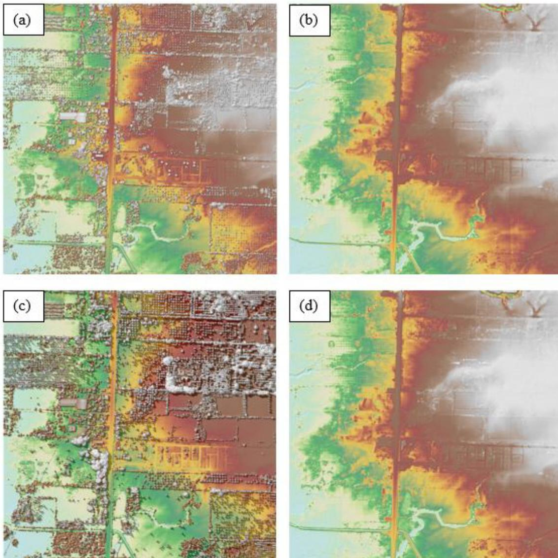
Figure 22. The production of last return DSM (a) and DTM (b), first return DSM (c) and secondary DTM (d) in some portion of Mainit-Tubay floodplain
