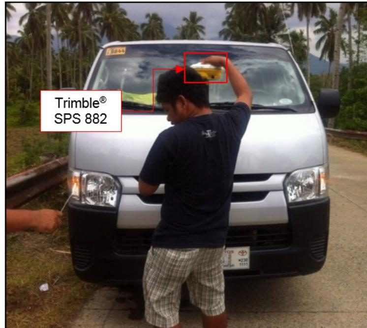
Figure 41. Setting up of GNSS rover receiver, Trimble® SPS882 in a vehicle
