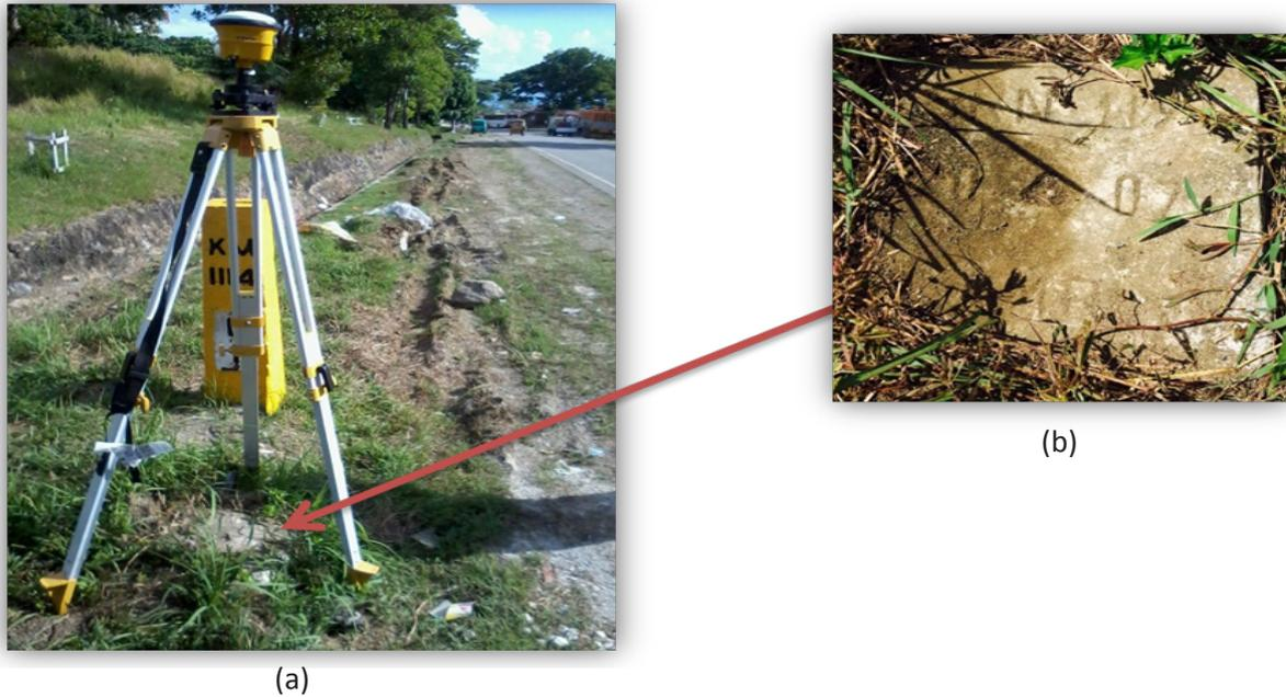
Figure 4. GPS set-up over SRN-119 Kilometer Post 1114 along the National Highway at Surigao City, Surigao Del Norte (a) and NAMRIA reference point SRN-119 (b) as recovered by the field team
