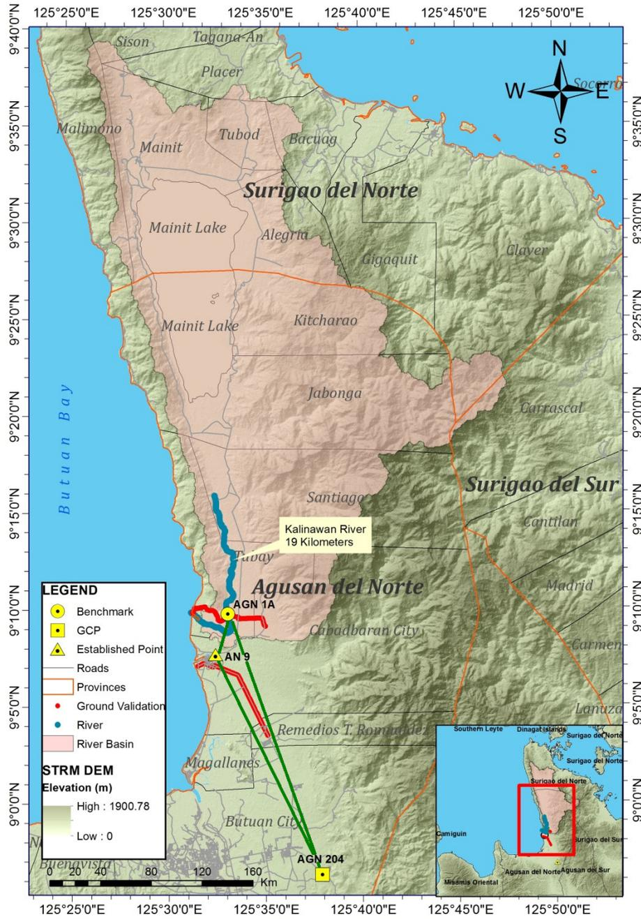
Figure 33. Extent of the bathymetric survey (in blue) in Mainit-Tubay River and the LiDAR data validation survey (in red)
