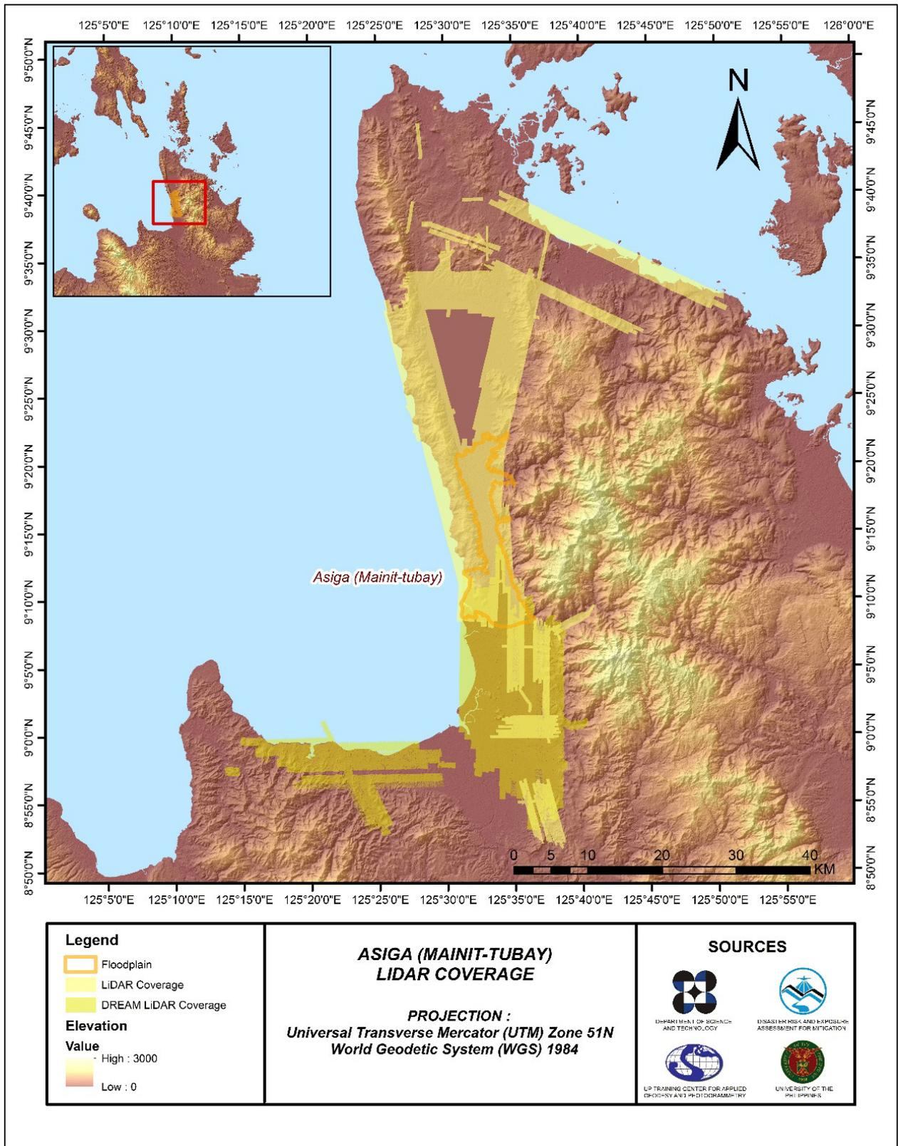
Figure 10. Actual LiDAR survey coverage for Mainit-Tubay (Asiga)floodplain
