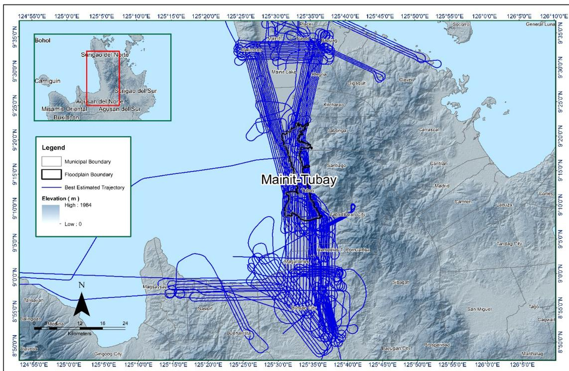
Figure 14. The best estimated trajectory of the LiDAR missions conducted over the Mainit-Tubay floodplain
