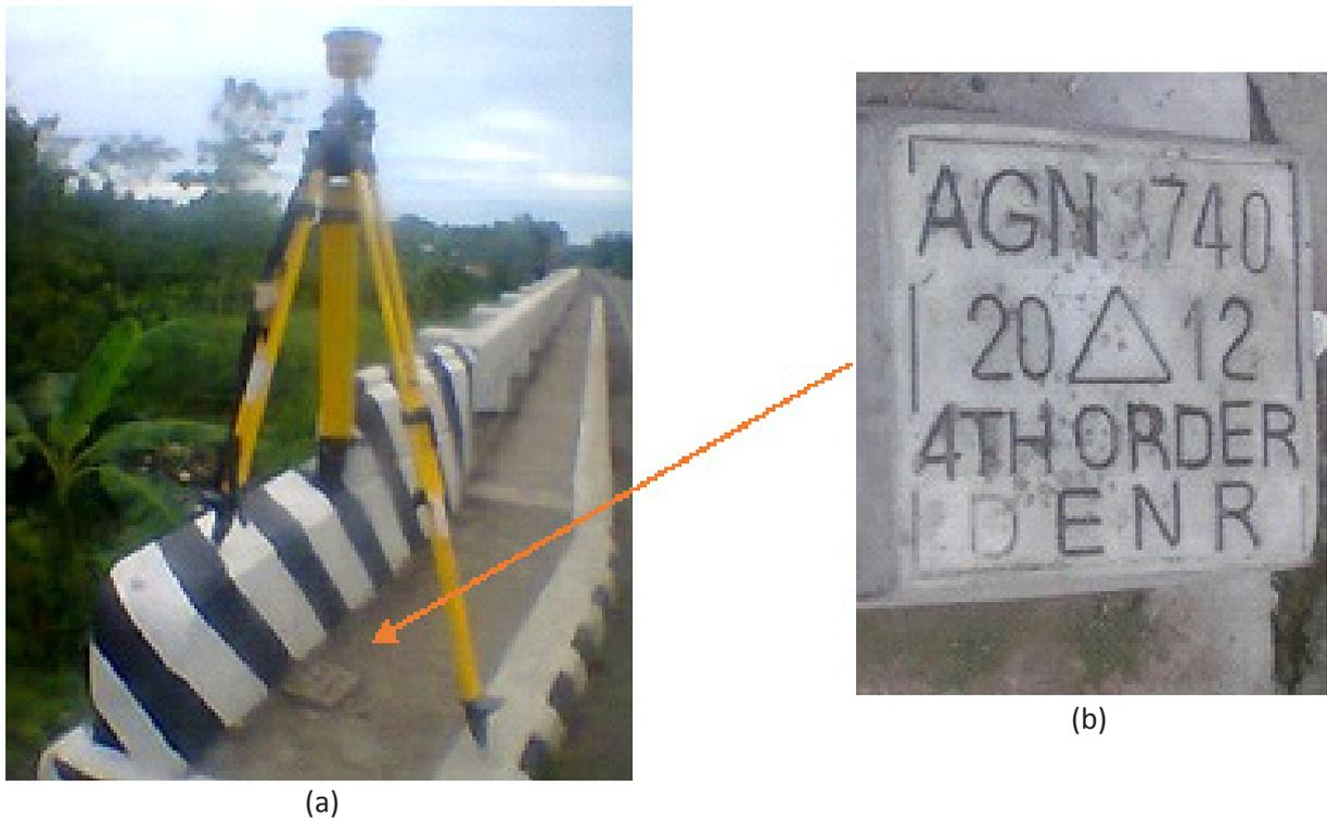
Figure 8. GPS set-up over AGN-3740 on the bridge at Barangay Sanghan, Asiga (mainit-tubay), Surigao del Norte (a) and NAMRIA reference point AGN-3740 (b) as recovered by the field team
