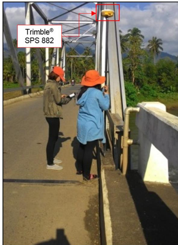
Figure 37. Gathering of cross-section points in Tubay Bridge using Trimble® SPS 882
