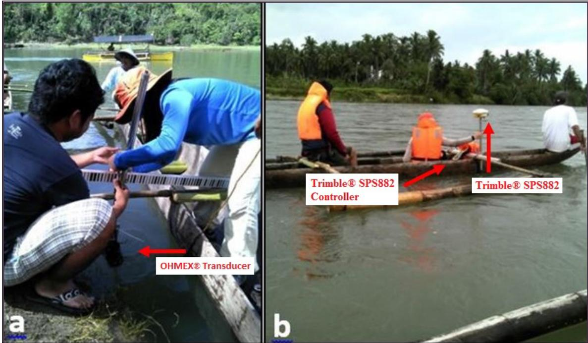
Figure 43. (a) Tying of the pole with transducer in one of the gunwales of the boat and (b) setup of bathymetric survey
