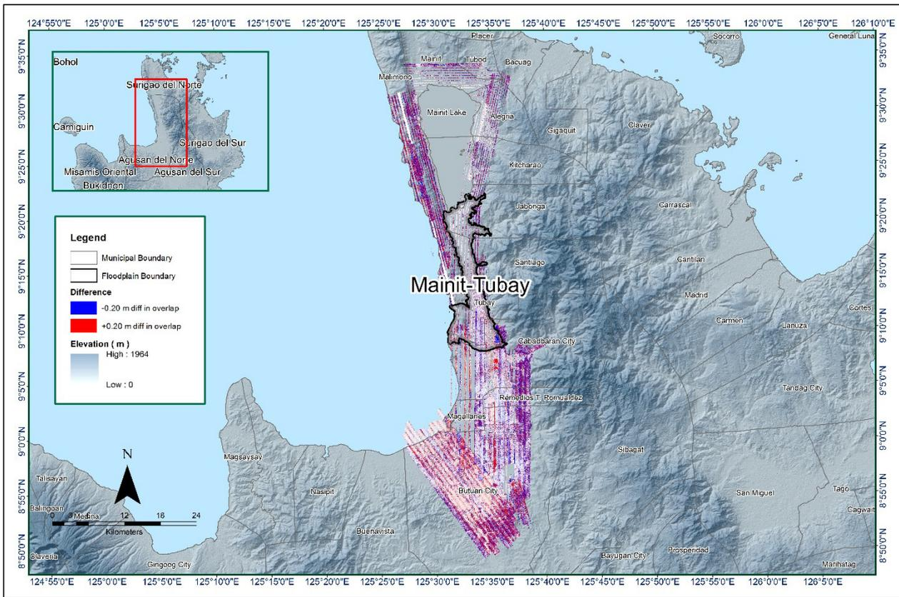
Figure 18. Elevation difference map between flight lines for Mainit-Tubay floodplain
