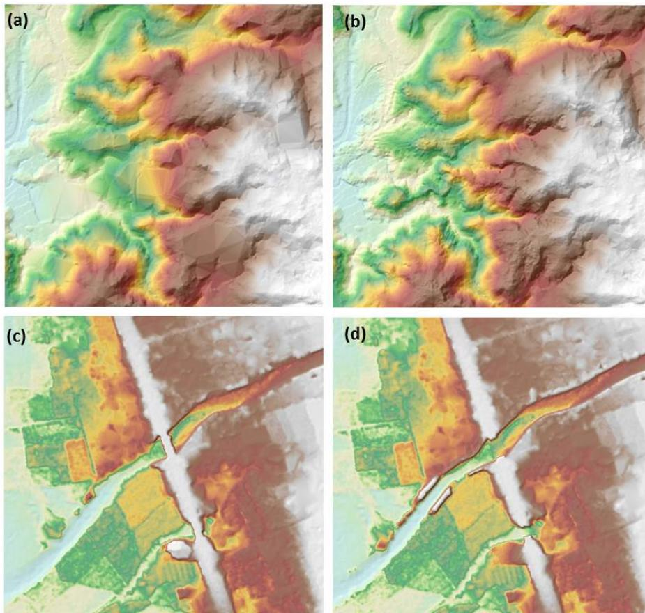
Figure 25. Portions in the DTM of Mainit-Tubay floodplain – a river embankment before (a) and after (b) data retrieval and a bridge before (c) and after (d) manual editing
