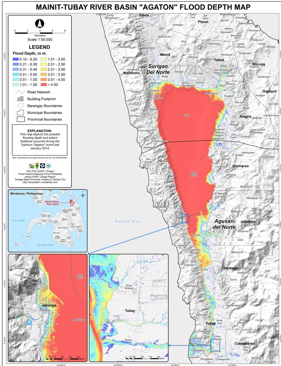
Figure 59. Flood depth and extent at Mainit-Tubay River basin during typhoon "Agaton"
