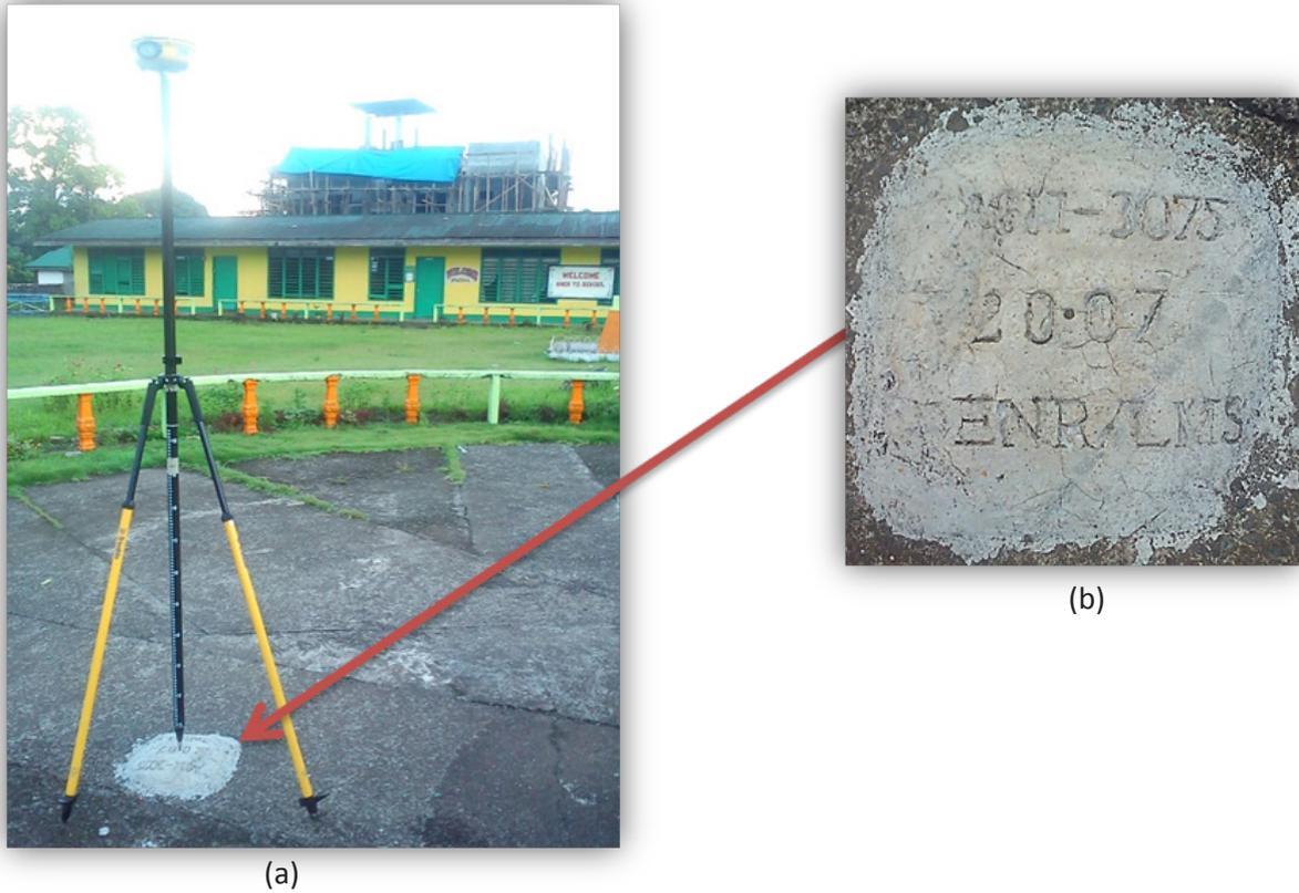
Figure 6. GPS set-up over AGN-3075 near the flagpole of Jaliobong Elementary School at Kitcharao, Surigao del Norte (a) and NAMRIA reference point AGN-3075 (b) as recovered by the field team
