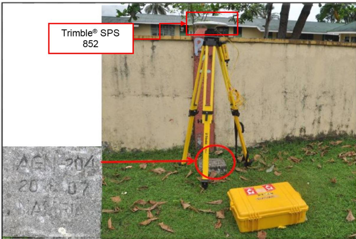
Figure 34. Base set-up using Trimble® SPS 852 at AGN-204 located near the concrete fence of Taligaman Elementary School, in Brgy. Basag, Butuan City, Agusan Del Norte.
