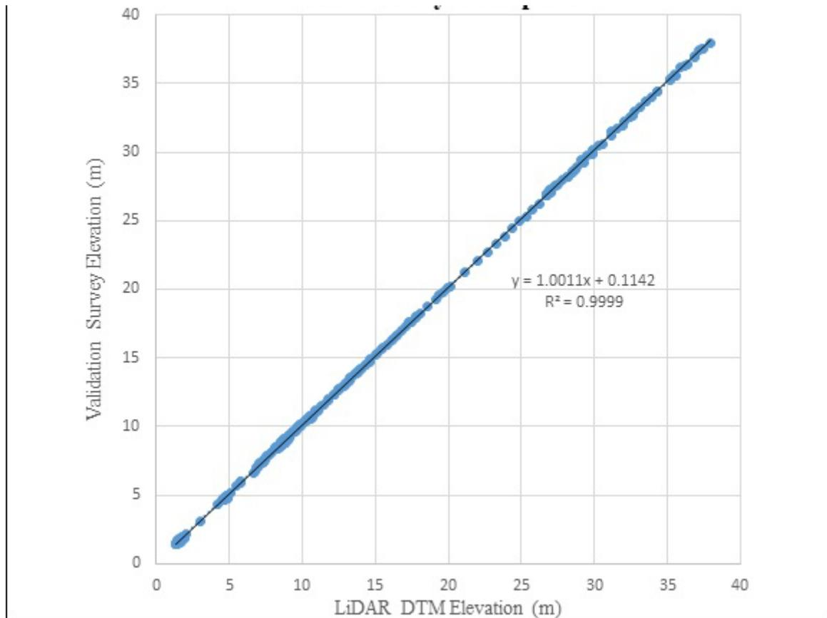
Figure 29. Correlation plot between validation survey points and LiDAR data
