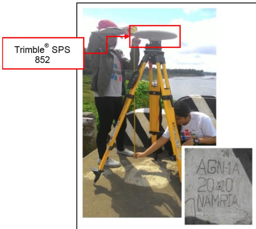
Figure 35. Base set-up using Trimble® SPS 882 at AGN-1A located along the approach of Tubay Bridge in Brgy. Doña Rosario, Municipality of Tubay, Agusan del Norte
