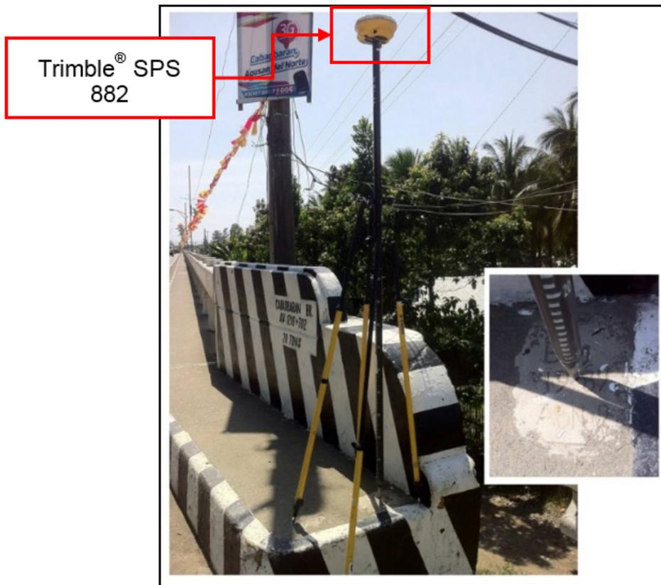
Figure 36. Base set-up using Trimble® SPS 882 at AN-9 located at the approach of Cabadbaran Bridge, Brgy. Kauswagan, Cabadbaran City, Agusan Del Norte
