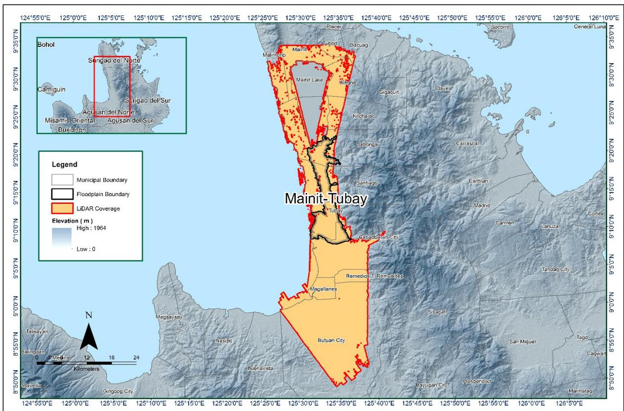
Figure 15. Boundary of the processed LiDAR data over Mainit-Tubay Floodplain
