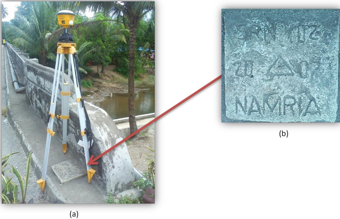
Figure 9. GPS set-up over SRN-102 at the first approach of Patag Bridge (right side) located at the Municipality of Sison, Surigao Del Norte (a) and NAMRIA reference point SRN-102 (b) as recovered by the field team
