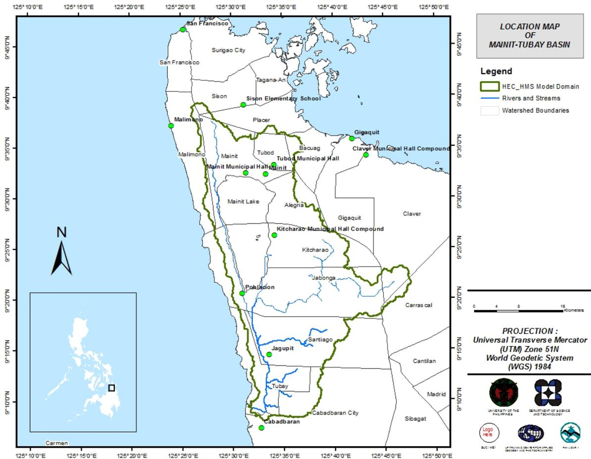
Figure 46. The location map of rain gauge used for the calibration of the Mainit-Tubay HEC- HMS model
