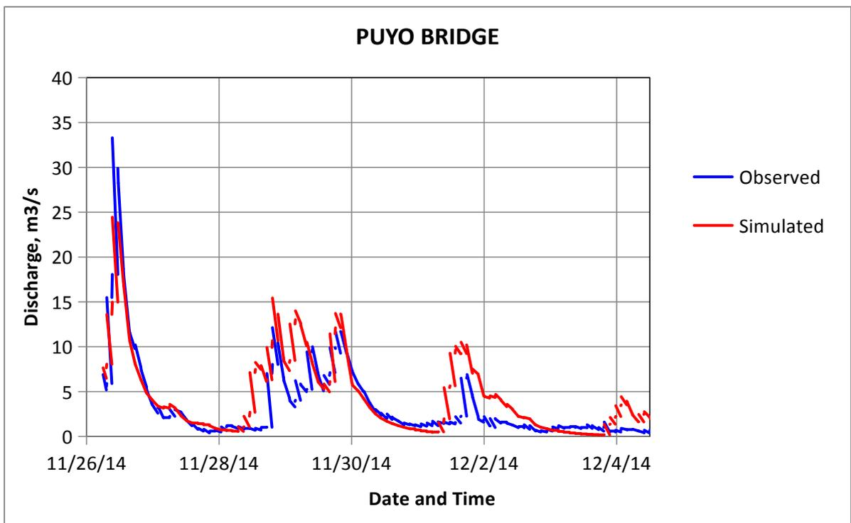
Figure 57. Outflow Hydrograph of Puyo Bridge produced by the HEC-HMS model compared with observed outflow.
