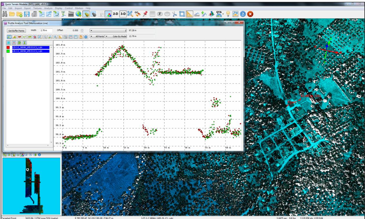
Figure 19. Quality checking for a Mainit-Tubay flight 1604A using the Profile Tool of QT Modeler
