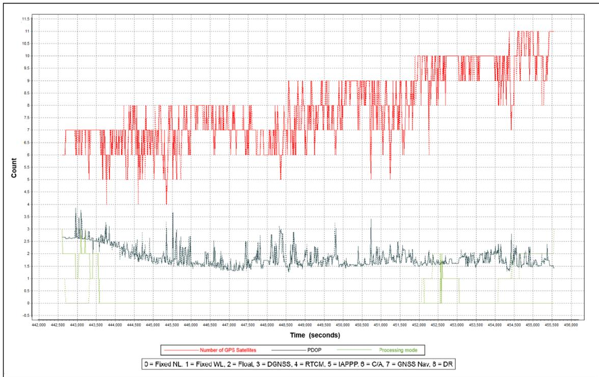
Figure 13. Solution Status Parameters of Mainit-Tubay Flight 1604A
