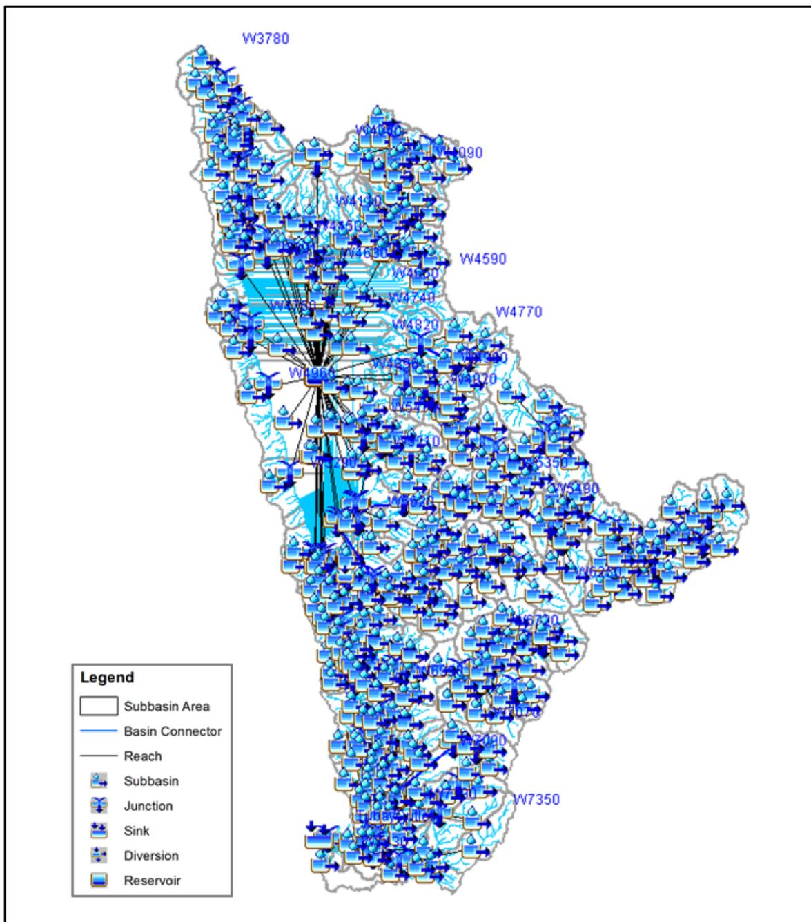
Figure 54. The Mainit-Tubay River Basin model generated using HEC-HMS.
