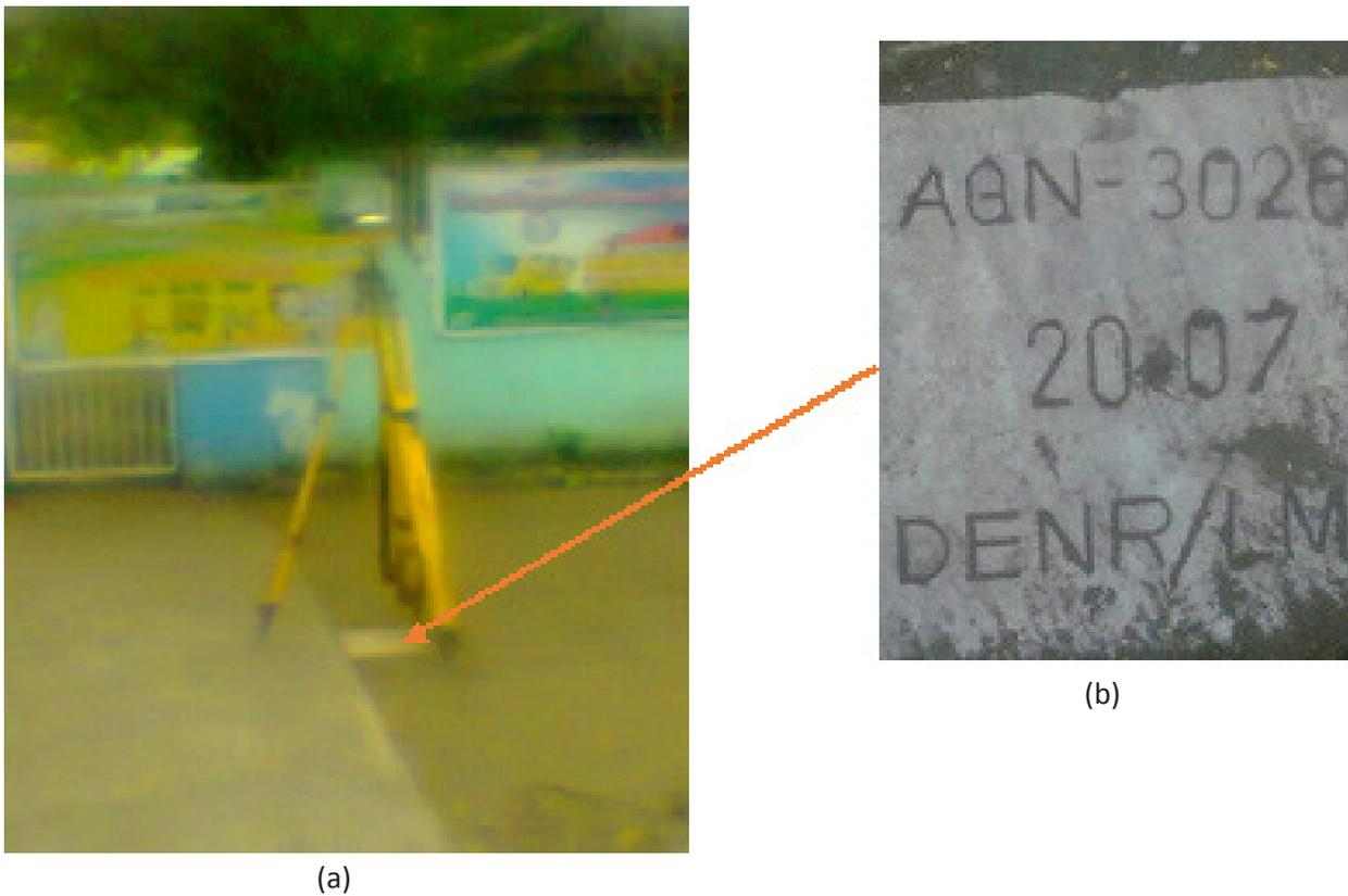
Figure 7. GPS set-up over AGN-3026 in front of Buhang National High School, Municipality of Magallanes, Surigao del Norte (a) and NAMRIA reference point AGN-3026 (b) as recovered by the field team
