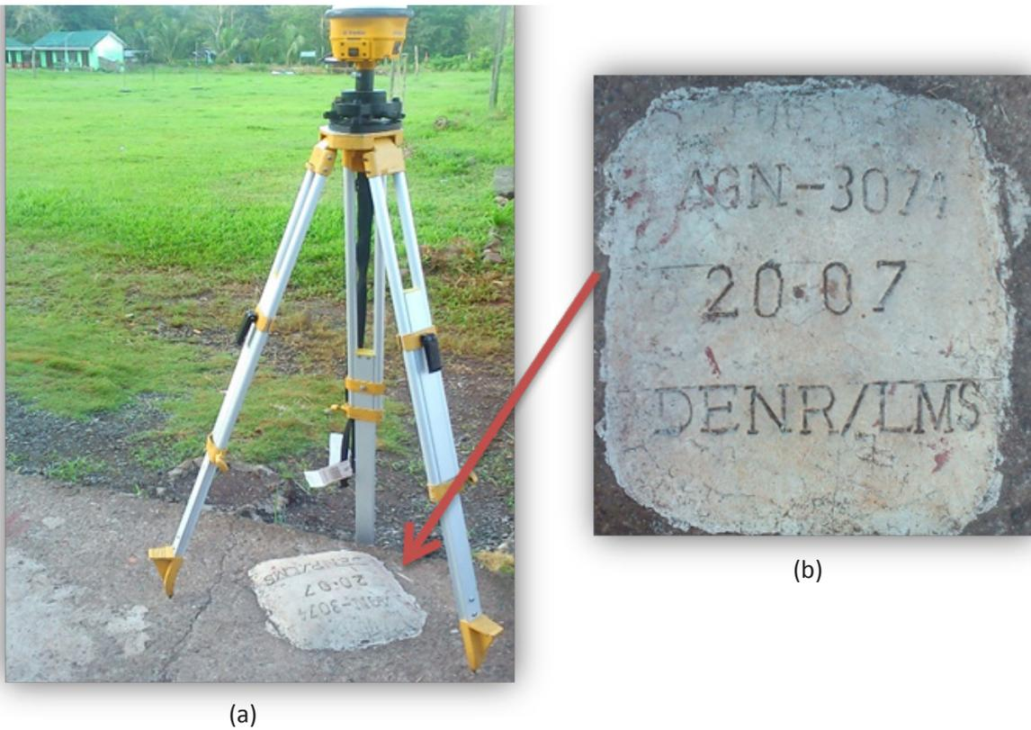
Figure 5. GPS set-up over AGN-3074 near the entrance gate of Jaliobong National High School at Kitcharao, Surigao del Norte (a) and NAMRIA reference point AGN-3074 (b) as recovered by the field team
