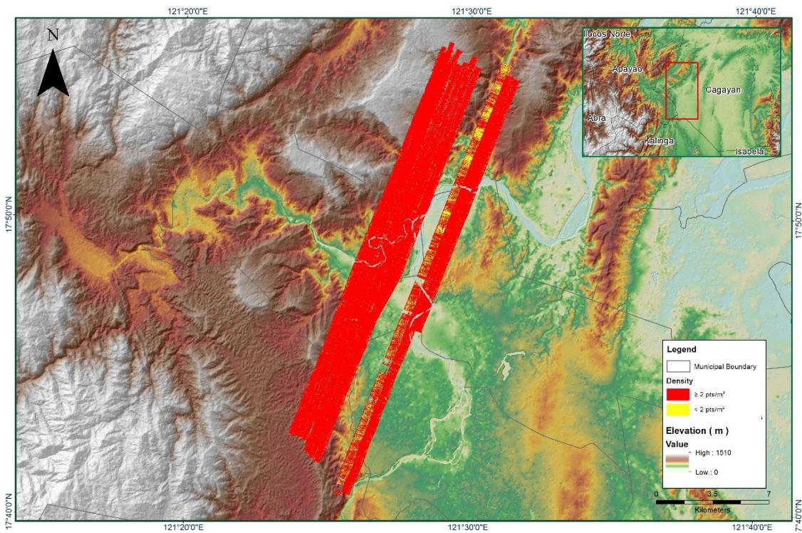
**Figure 1.19.6. Density map of merged LiDAR data**
