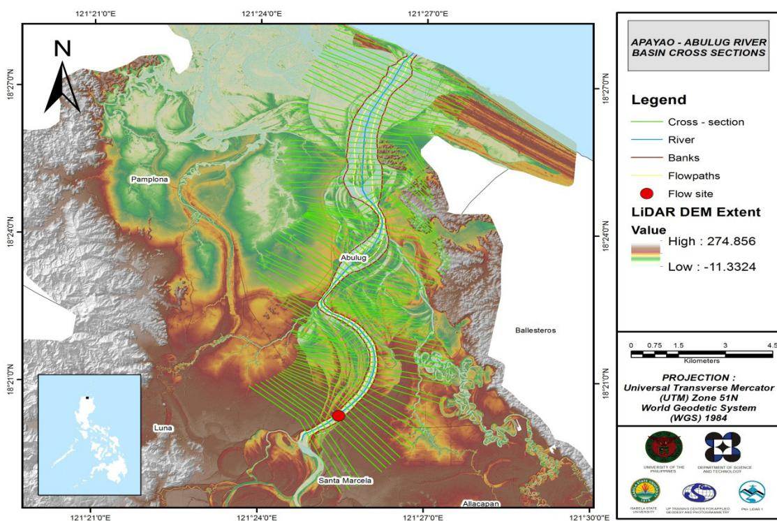
Figure 64. Abulog-Apayao River Cross-section generated using HEC GeoRAS tool
