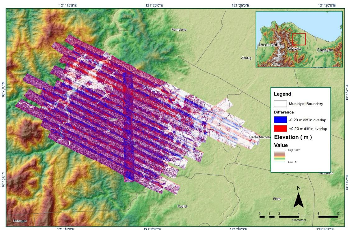
**Figure 1. 5. 7. Elevation difference between flight lines**
