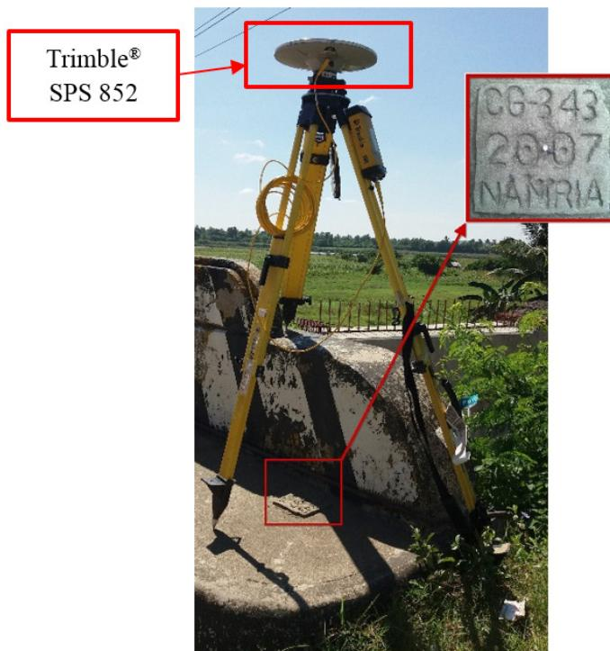
Figure 37. GNSS setup of Trimble® SPS 852 at CG-343, located at the corner of the bridge approach of Lukban Bridge, Brgy. Libertad, Municipality of Abulug, Cagayan
