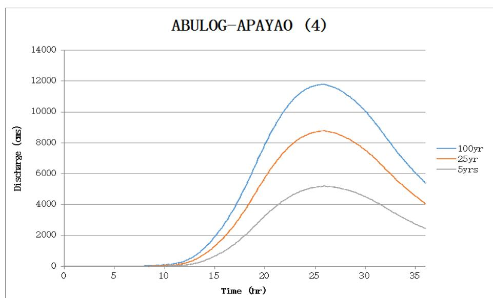
Figure 71. Abulog-Apayao river (4) generated discharge using 5-, 25-, and 100-year Aparri rainfall intensity-duration-frequency (RIDF) in HEC-HMS
