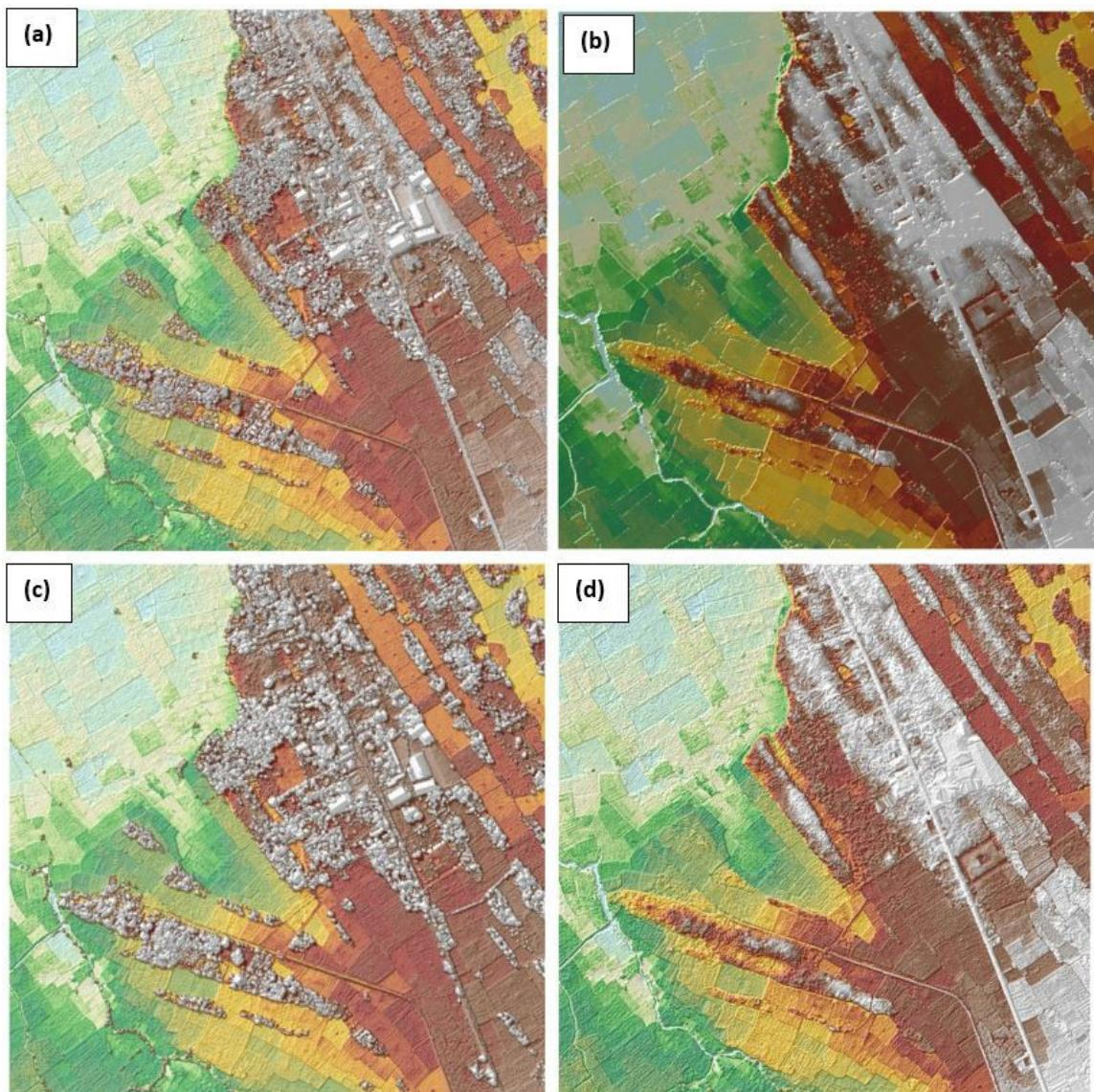
Figure 24. The production of last return DSM (a) and DTM (b), first return DSM (c) and secondary DTM (d) in some portion of Abulog-Apayao floodplain
