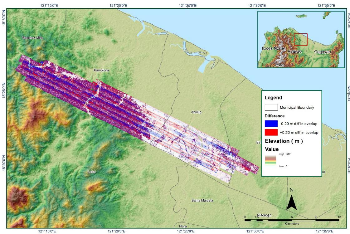
**Figure 1. 9. 7. Elevation difference between flight lines**
