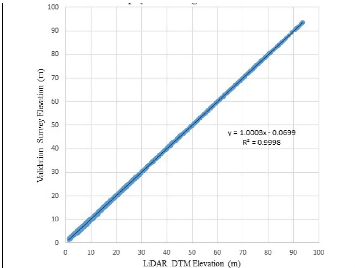
Figure 31. Correlation plot between validation survey points and LiDAR data
