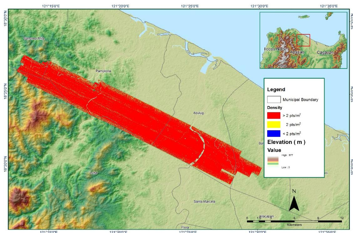
**Figure 1.9.6. Density map of merged LiDAR data**
