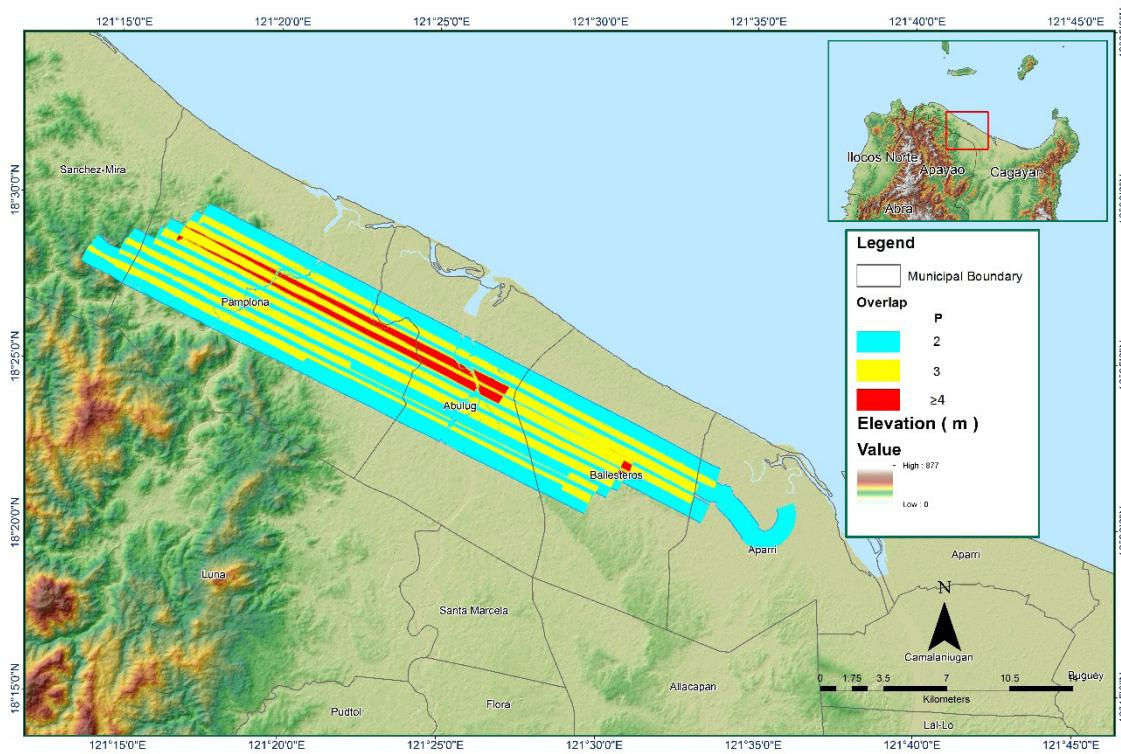
**Figure 1. 10. 5. Image of data overlap**
