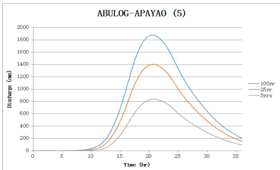
Figure 72. Abulog-Apayao river (5) generated discharge using 5-, 25-, and 100-year Aparri rainfall intensity-duration-frequency (RIDF) in HEC-HMS
