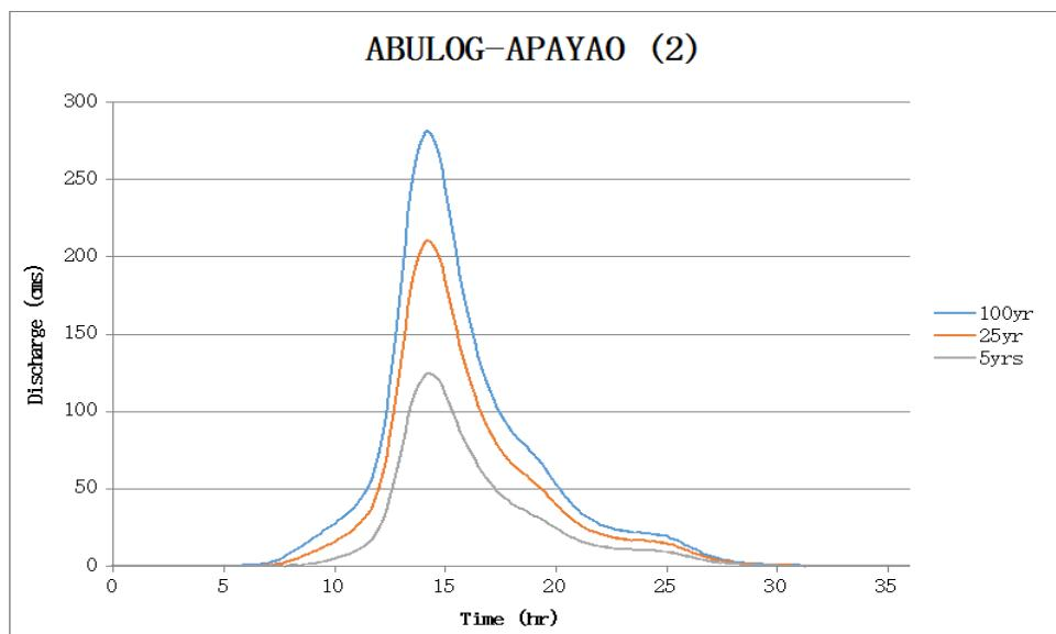
Figure 69. Abulog-Apayao river (2) generated discharge using 5-, 25-, and 100-year Aparri rainfall intensity-duration-frequency (RIDF) in HEC-HMS
