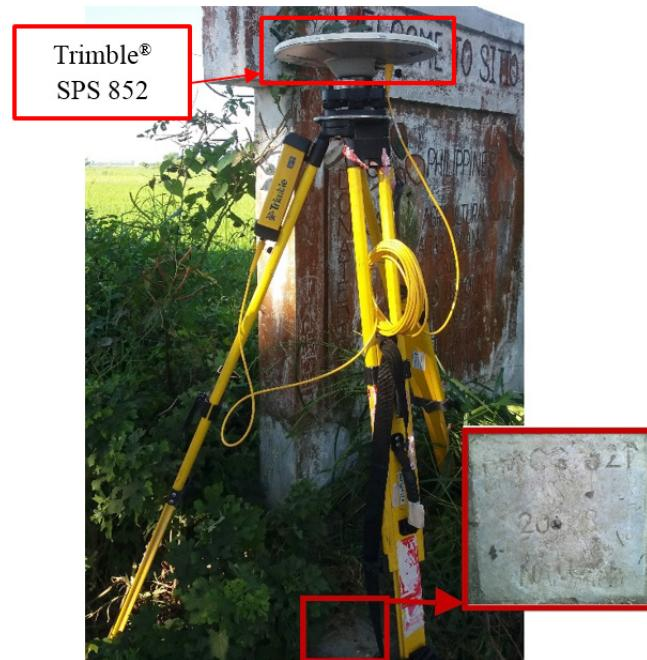
Figure 38. GNSS base setup of Trimble® SPS 852 at CG-521 situated on the pavement pf the concrete barangay sign board of Sittio Maquirre, Brgy. Guiddam, Municipality of Abulug, Cagayan
