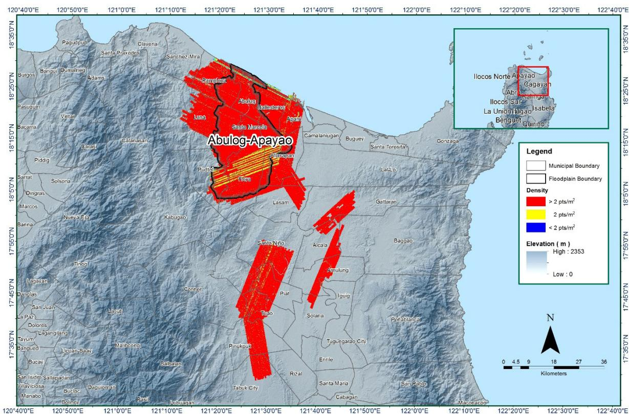
Figure 19. Pulse density map of merged LiDAR data for Abulog-Apayao floodplain
