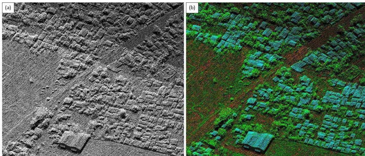
Figure 23. Point cloud before (a) and after (b) classification
