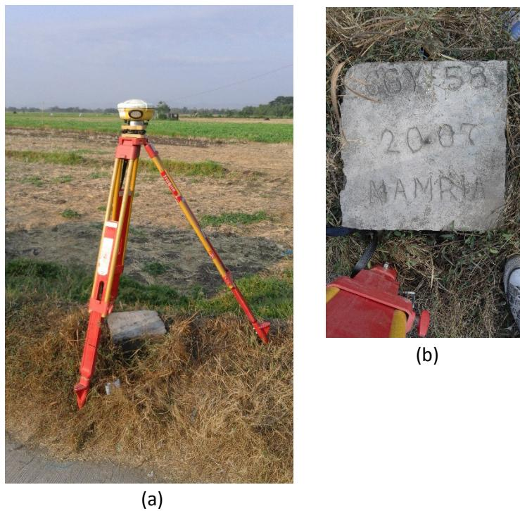
Figure 4. a) GPS set-up over CGY-58 located 15 m. E of the junction of the road leading to barangay. Kari-lukud, and is situated 10 meters southeast of Barangay. Ubong welcome monument. b) NAMRIA reference point CGY-58 as recovered by field team
