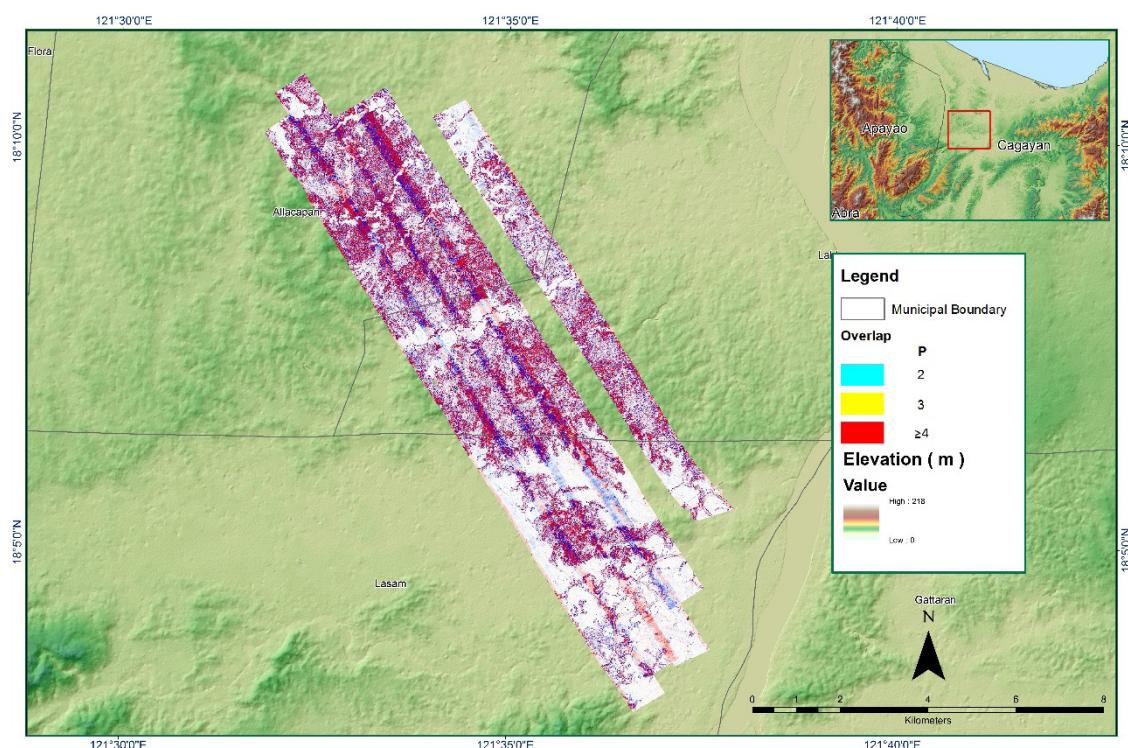
**Figure 1. 14. 7. Elevation difference between flight lines**
