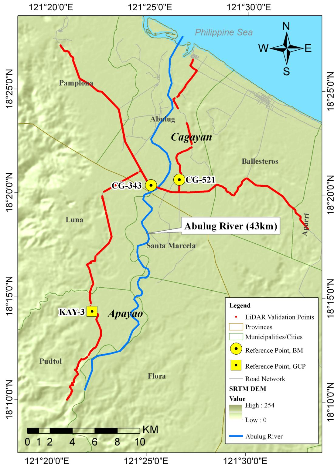
Figure 47. LiDAR ground validation survey coverage for Abulug River Basin
