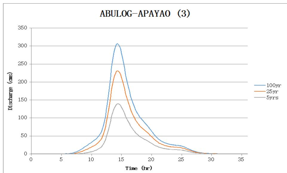
Figure 70. Abulog-Apayao river (3) generated discharge using 5-, 25-, and 100-year Aparri rainfall intensity-duration-frequency (RIDF) in HEC-HMS
