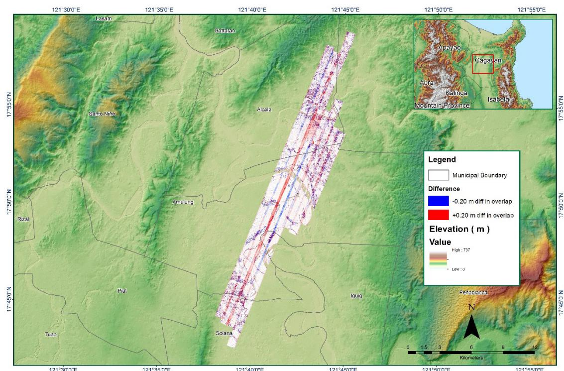
**Figure 1. 12. 7. Elevation difference between flight lines**
