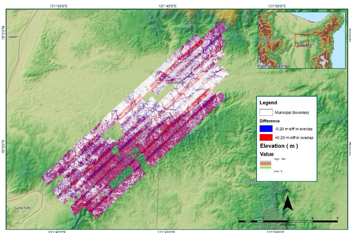
**Figure 1. 13. 7. Elevation difference between flight lines**
