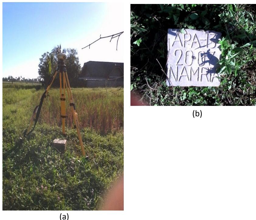
Figure 3. a) GPS set-up over APA-13 located on the barangay property lot of the barangay hall of Tumog in Luna, 8 m. from the north edge of the PCCP, and 70 meters northeast of a waiting shed, and b) NAMRIA reference point APA-13 as recovered by field team
