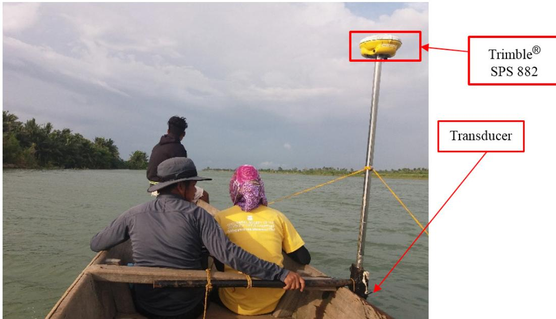
Figure 48. Bathymetric survey setup in Abulug River
