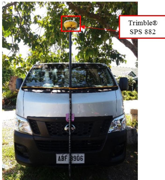
Figure 46. Validation Set-up for Abulug River
