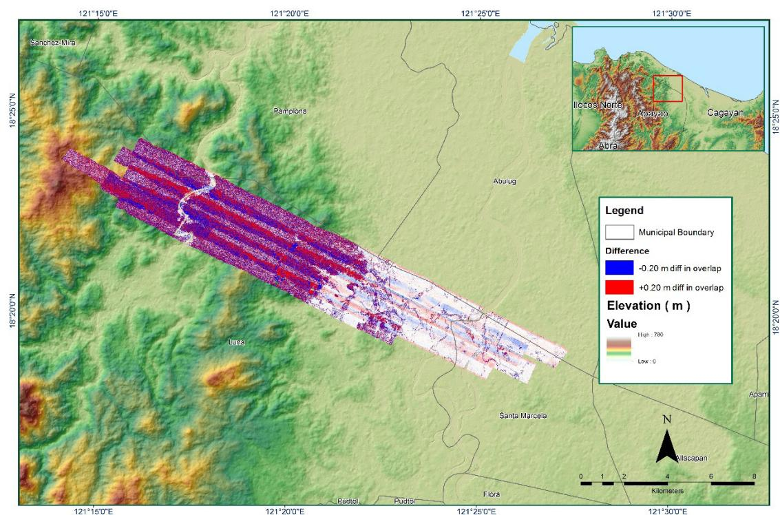
**Figure 1. 6. 7. Elevation difference between flight lines**
