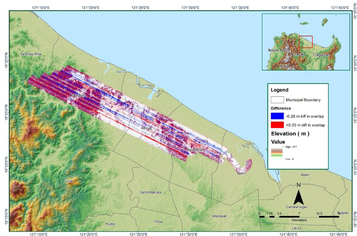
**Figure 1. 10. 7. Elevation difference between flight lines**
