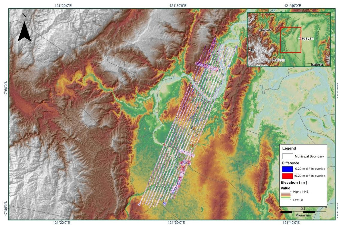
**Figure 1.17.7. Elevation difference between flight lines**
