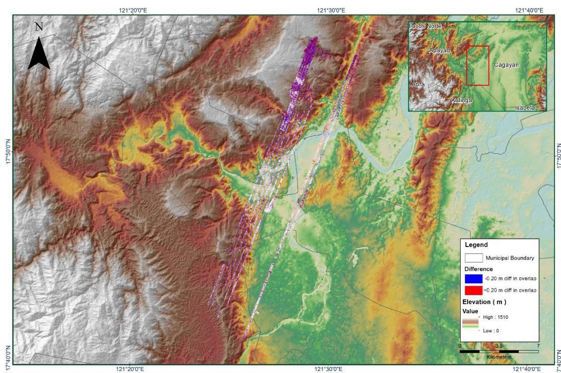
**Figure 1.19.7. Elevation difference between flight lines**
