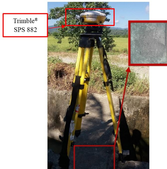
Figure 39. GNSS receiver setup of Trimble® SPS 882 at KAY-3 located on top of a concrete flood gate near the municipal building in Brgy. Imelda, Municipality of Pudtol, Apayao
