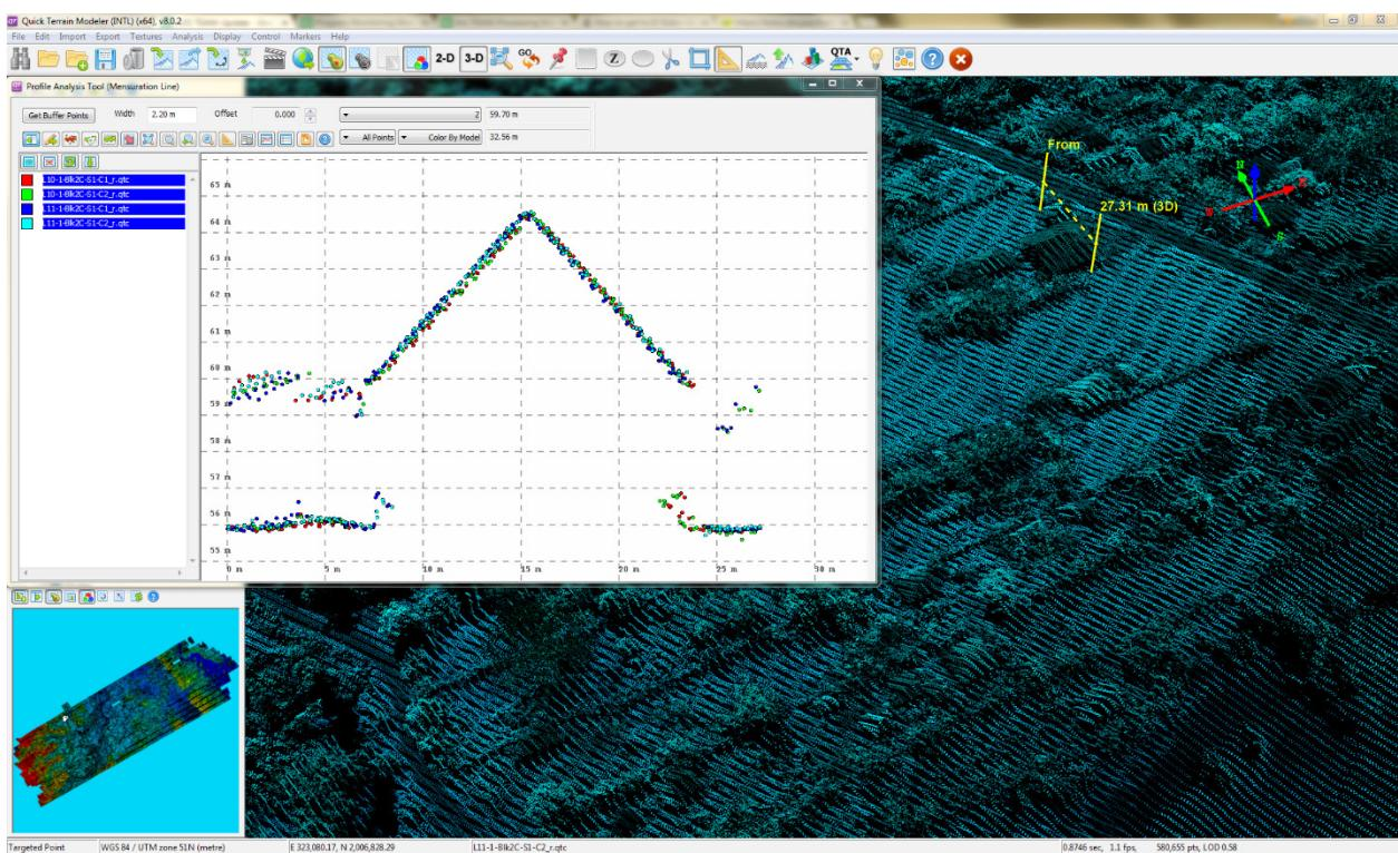
Figure 21. Quality checking for a Abulog-Apayao flight 2838P using the Profile Tool of QT Modeler
