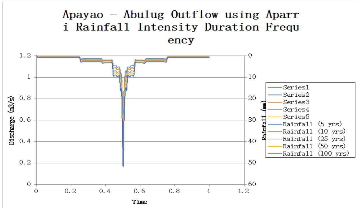
Figure 67. Outflow hydrograph at Abulug-Apayao Station generated using Aparri RIDF simulated in HEC-HMS
