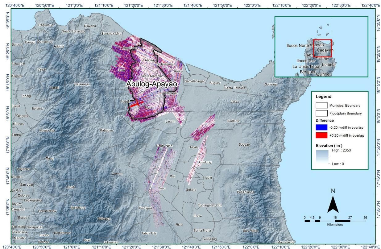
Figure 20. Elevation difference map between flight lines for Abulog-Apayao floodplain
