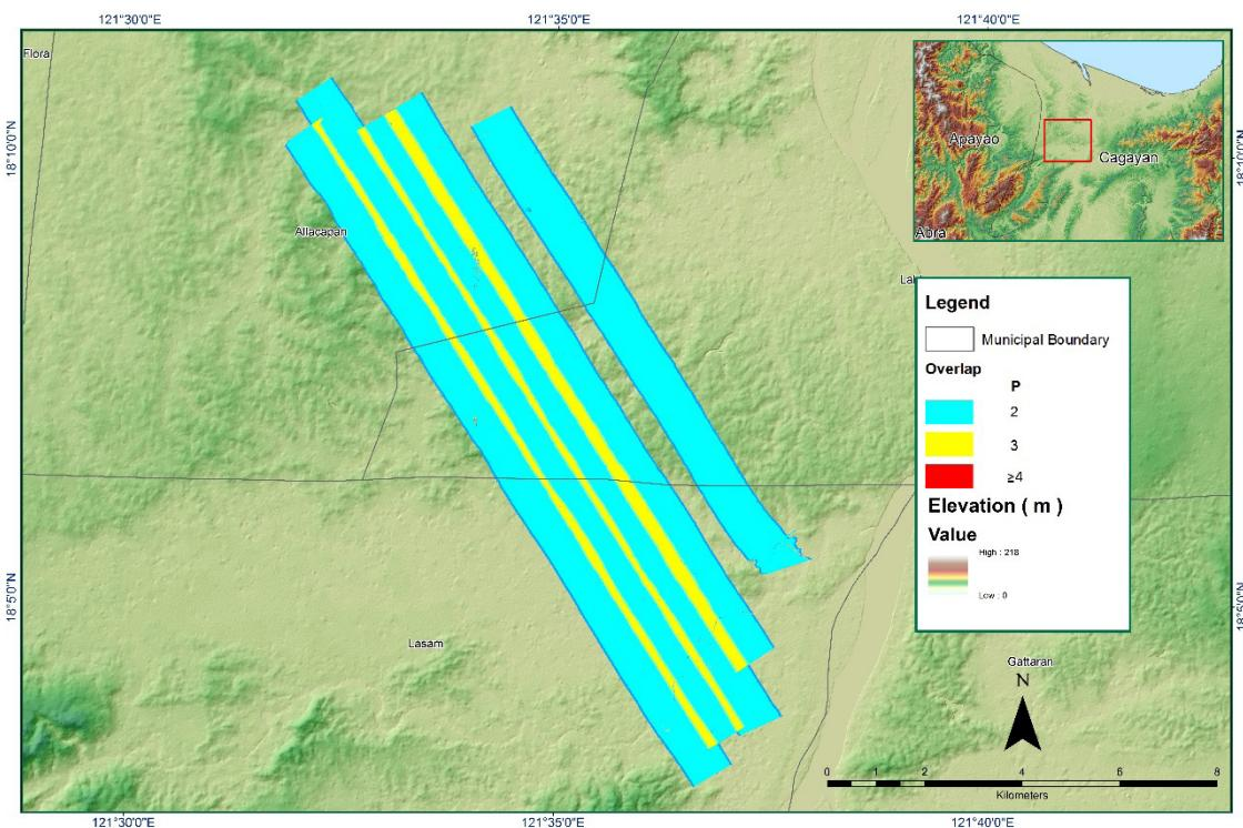
**Figure 1. 14. 5. Image of data overlap**
