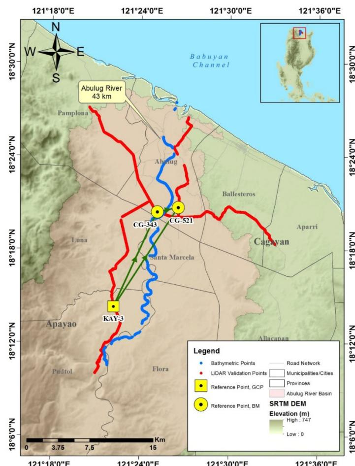
Figure 35. Extent of the bathymetric survey (in blue line) in Abulog-Apayao River and the LiDAR survey (in red)
