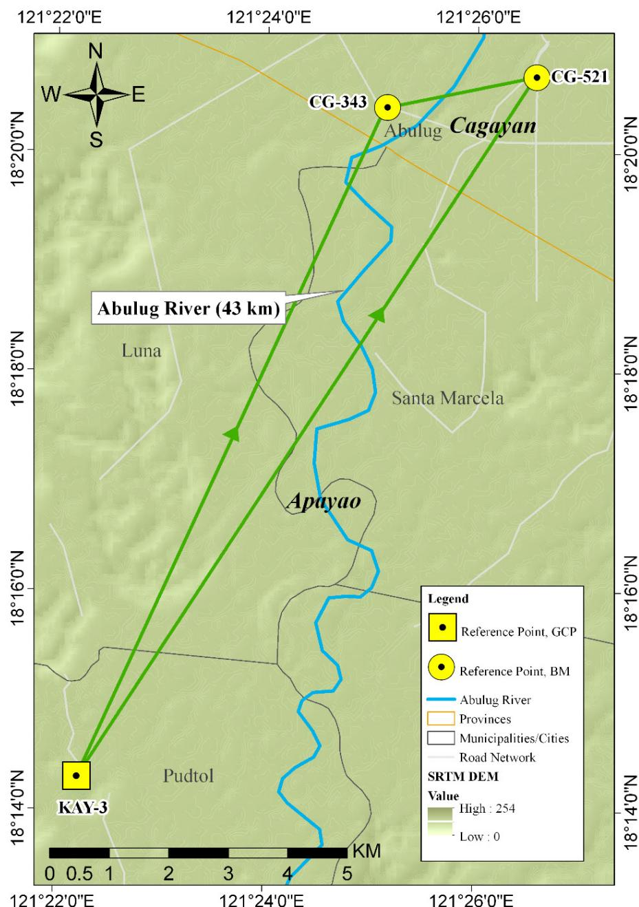
Figure 36. GNSS network covering the Abulug River
