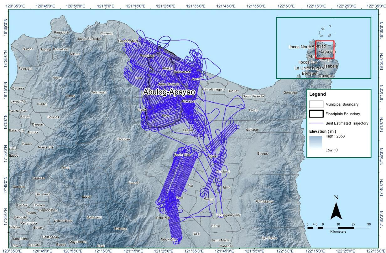
Figure 16. The best estimated trajectory of the LiDAR missions conducted over Abulog-Apayao floodplain
