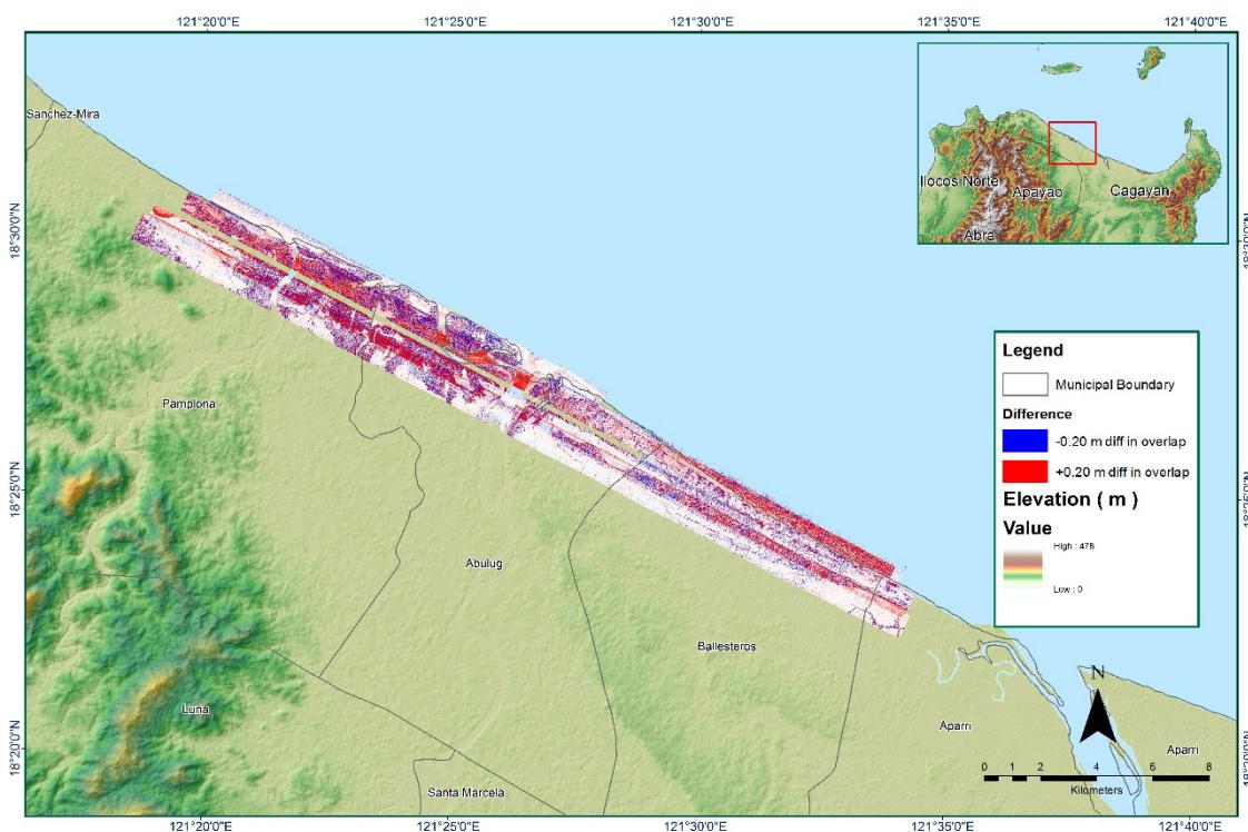
**Figure 1. 11. 7. Elevation difference between flight lines**
