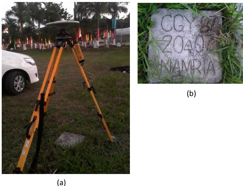
Figure 7. a) GPS set-up over CGY-87, located on a solar dryer at Barangay Cabayabasan, fronting the barangay hall. b) NAMRIA reference point CGY-87 as recovered by field team
