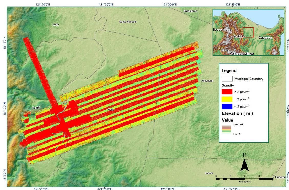
**Figure 1.7.6. Density map of merged LiDAR data**
