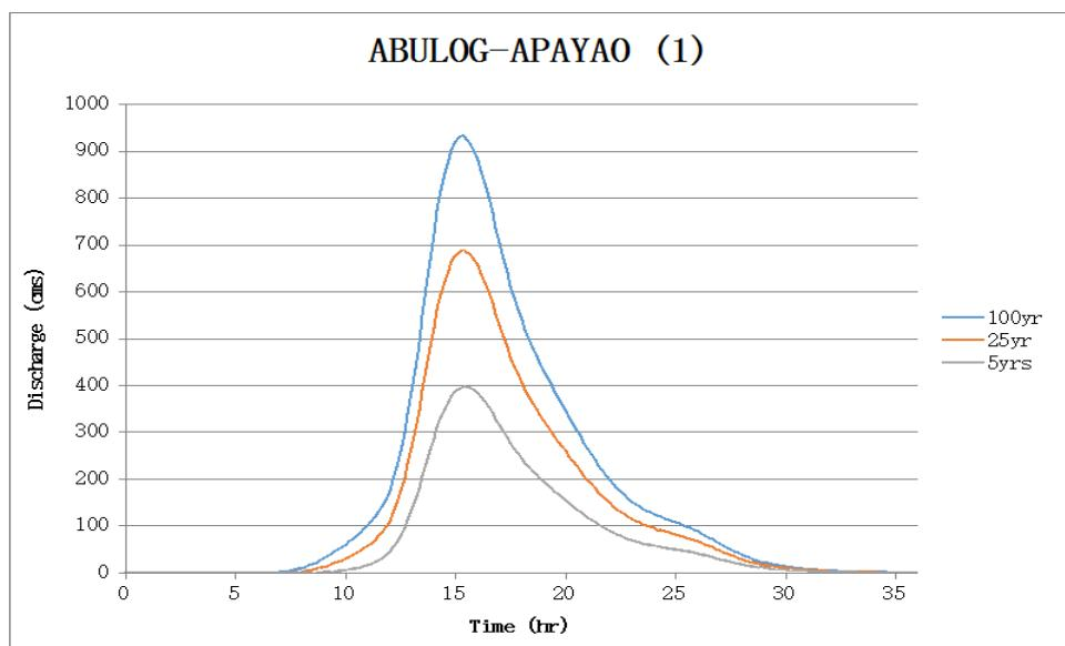
Figure 68. Abulog-Apayao river (1) generated discharge using 5-, 25-, and 100-year Aparri rainfall intensity-duration-frequency (RIDF) in HEC-HMS
