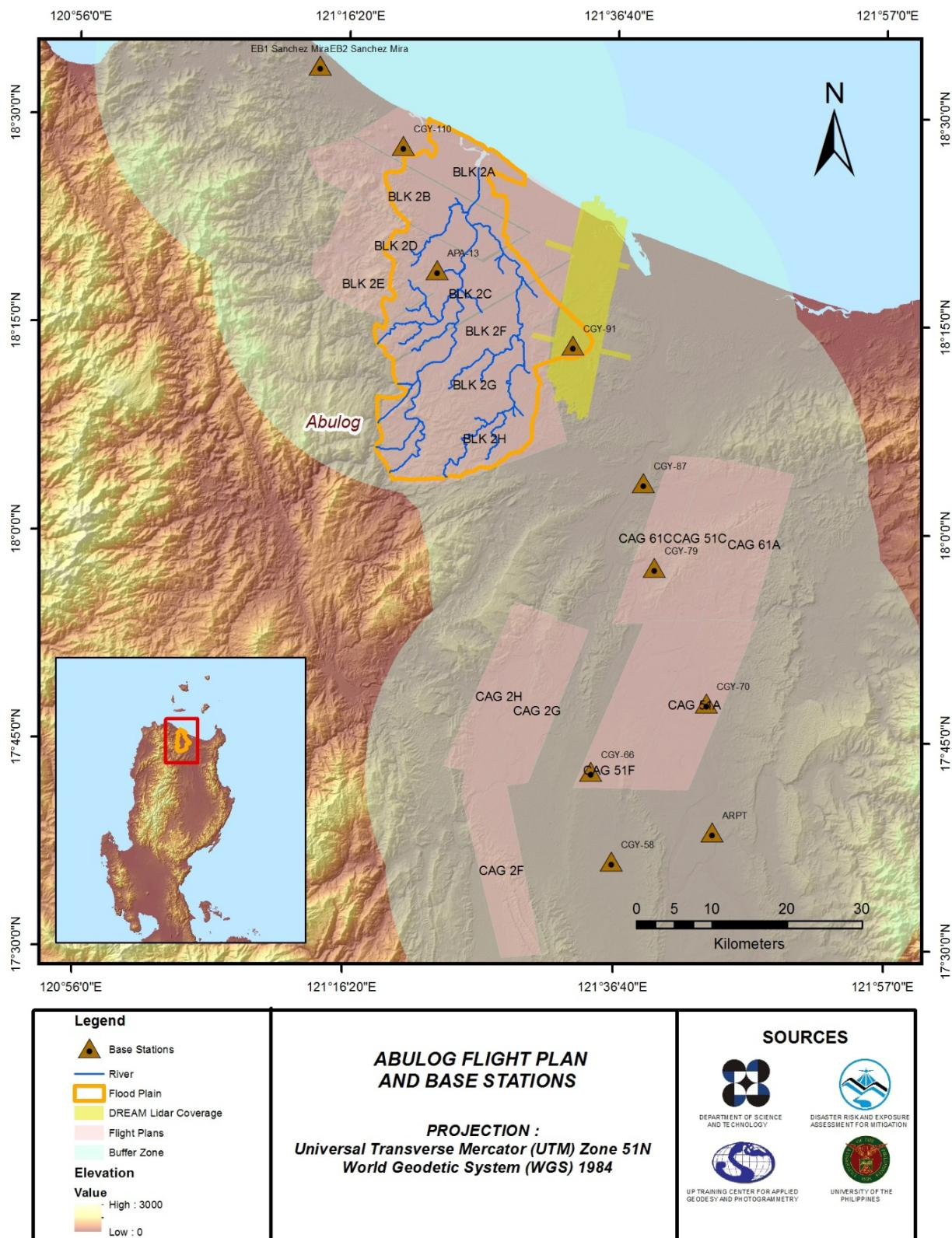
Figure 2. Flight plans and base stations used for Abulog-Apayao Floodplain survey
