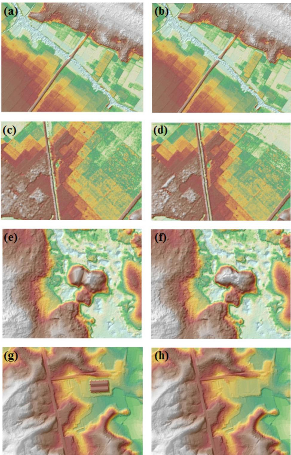
Figure 27. Portions in the DTM of Abulog-Apayao floodplain – a road before (a) and after (b) manual editing; an irrigation before (c) and after (d); interpolated ridge before (e) and after (f) object retrieval; and a building before (g) and after (h) manual editi
