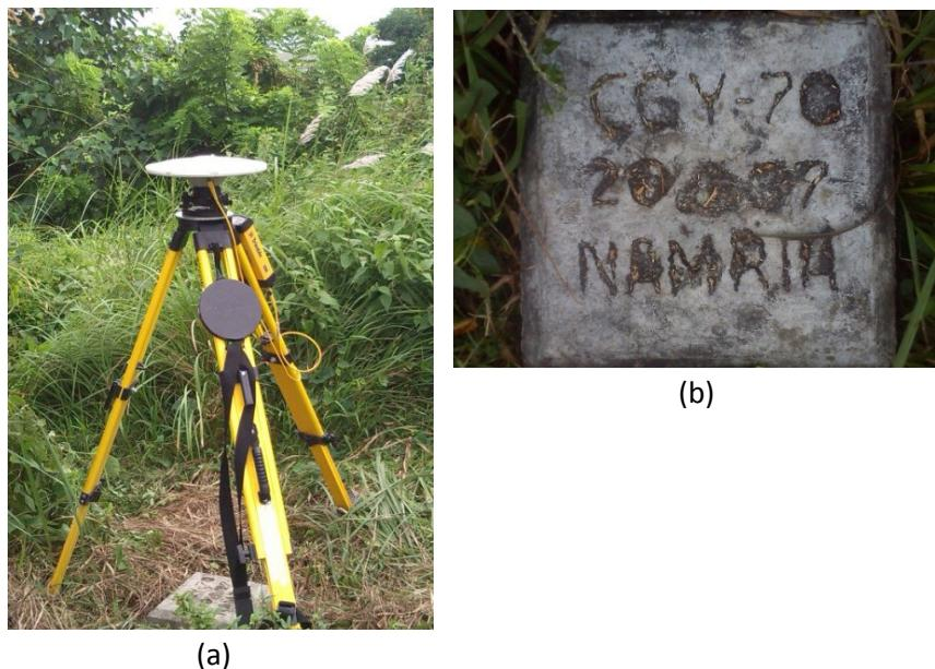
Figure 6. a) GPS set-up over CGY-70, located inside Estefania elementary school, and situated 1 meter east of the northeast corner of the basketball court. b) NAMRIA reference point CGY-70 as recovered by field team
