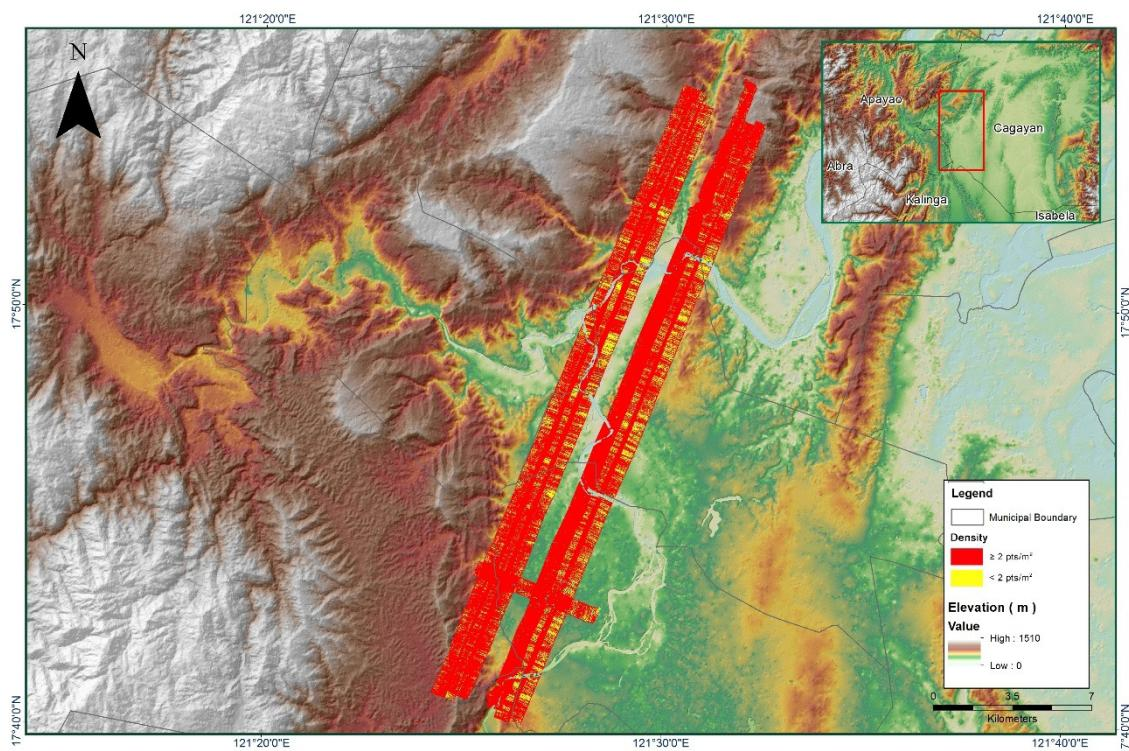
**Figure 1.18.6. Density map of merged LiDAR data**
