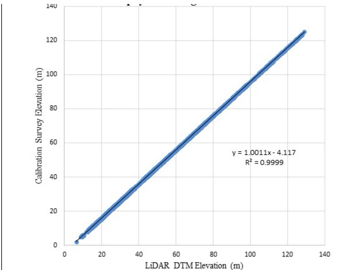
Figure 30. Correlation plot between calibration survey points and LiDAR data
