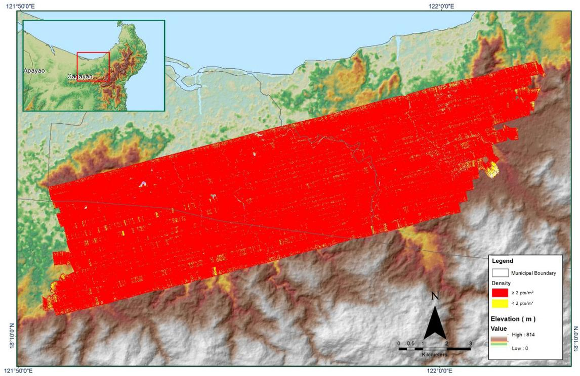
Figure 1.2.6. Density map of merged LiDAR data
