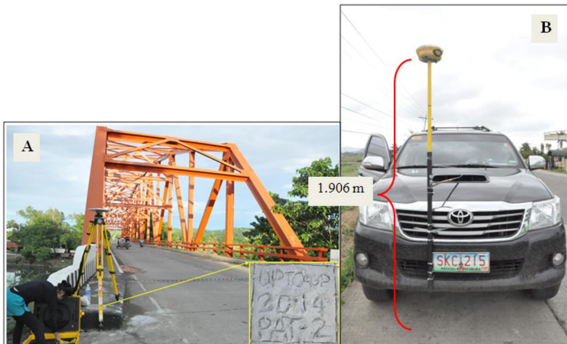
Figure 41. (A) Base setup at PAT-2 in Pateng Bridge, Municipality of Gonzaga and (B) Validation points acquisition survey setup attached in the vehicle
