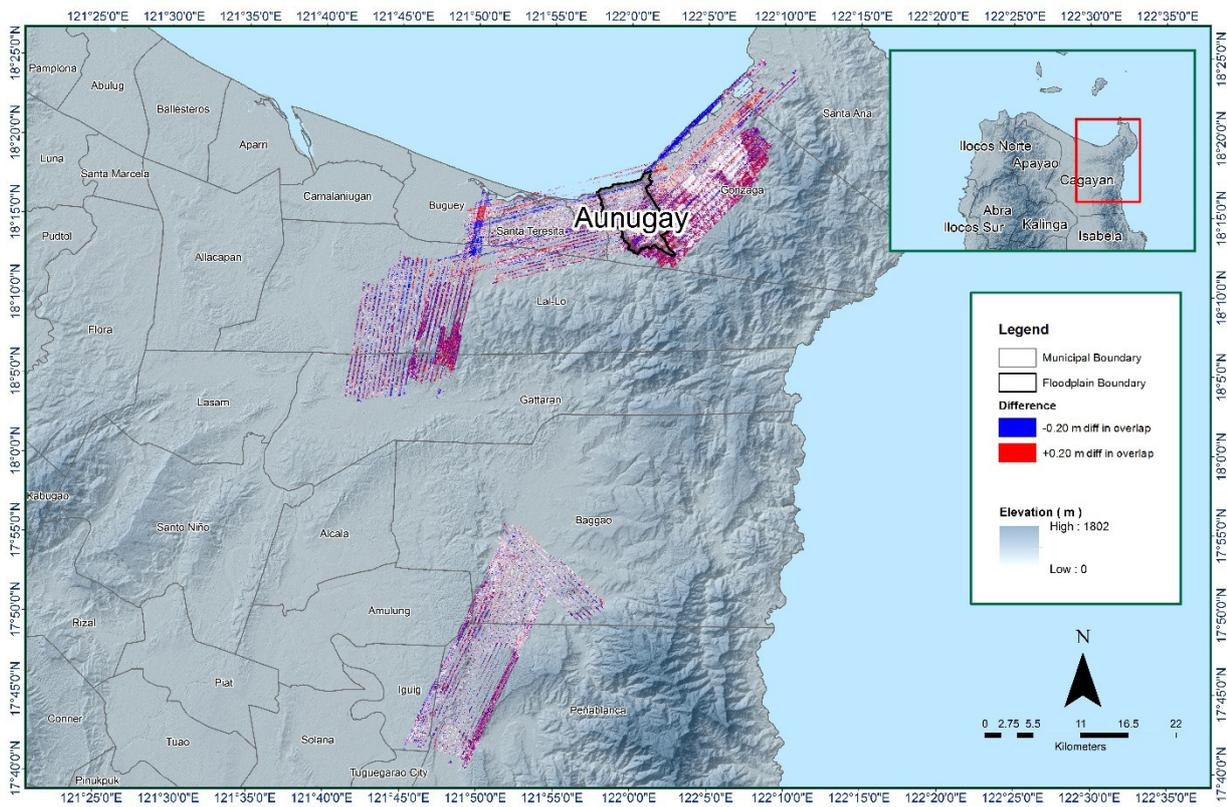
Figure 18. Elevation difference map between flight lines for Aunugay Floodplain
