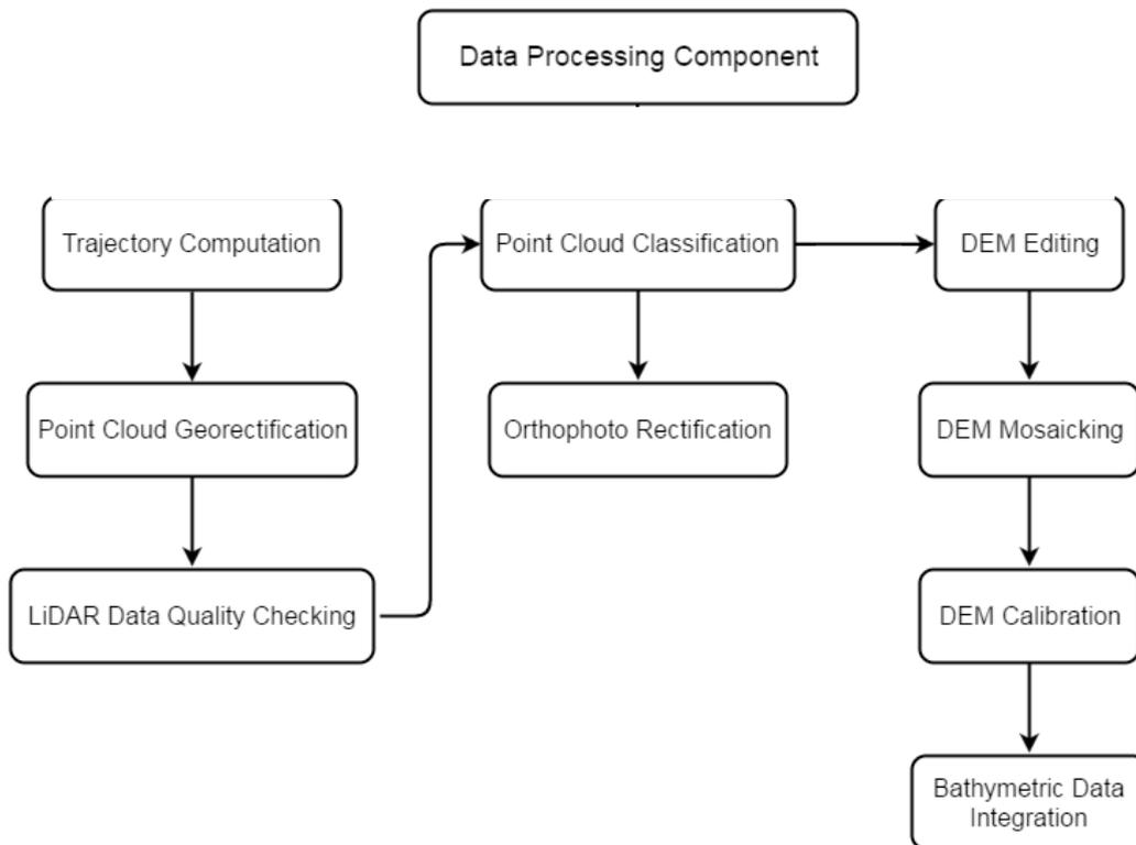
Figure II. Schematic Diagram for Data Pre-Processing Component
