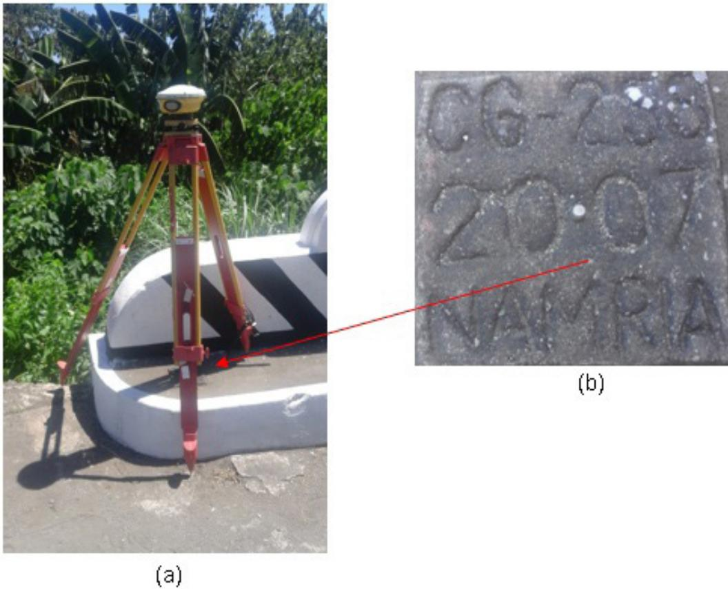
Figure 9. GPS set-up over CG-258 in the Municipality of Gonzaga (a) and NAMRIA reference point CG-258 (b) as recovered by the field team
