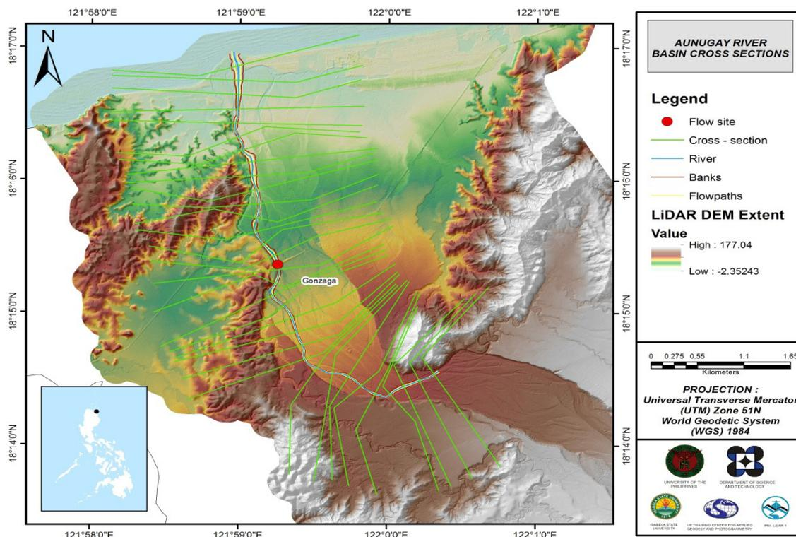
Figure 58. Aunugay River Cross-section generated using HEC GeoRAS tool
