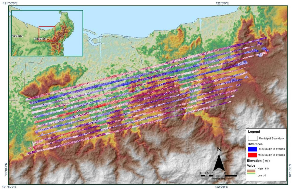
Figure 1.2.7. Elevation difference between flight lines
