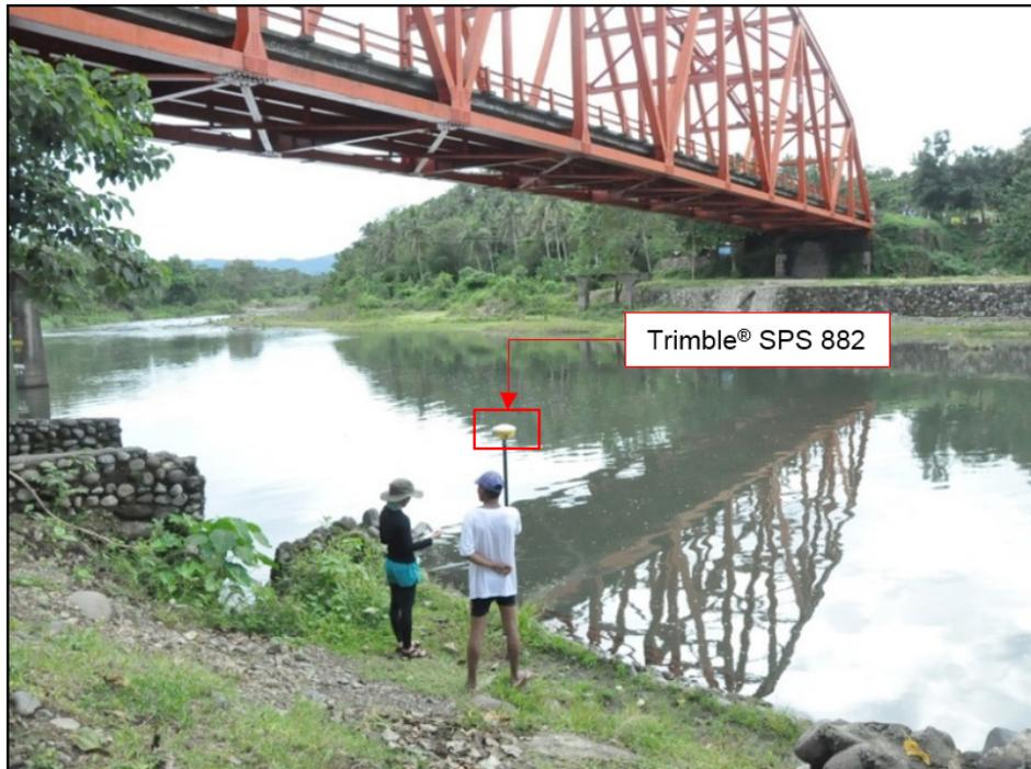
Figure 36. Left bank elevation acquisition (facing downstream) at Pateng Bridge, Brgy. Pateng, Municipality of Gonzaga
