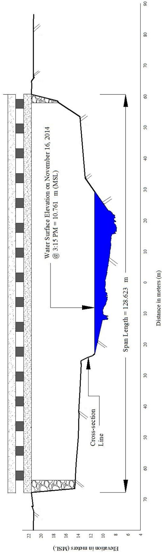
Figure 37. Pateng Bridge cross-section diagram
