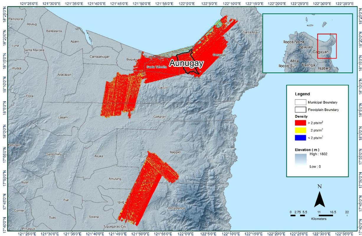
Figure 17. Density map of merged LiDAR data for Aunugay Floodplain
