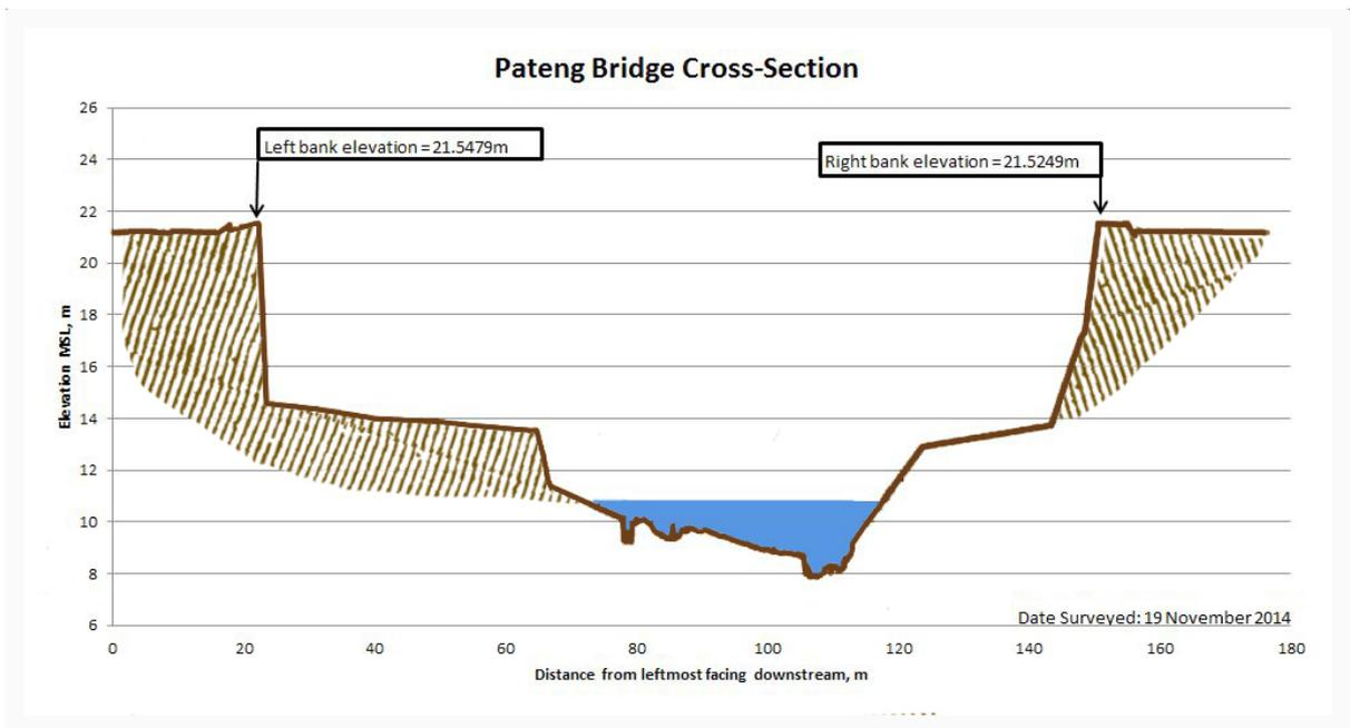
Figure 48. Cross-Section Plot of Pateng Bridge
