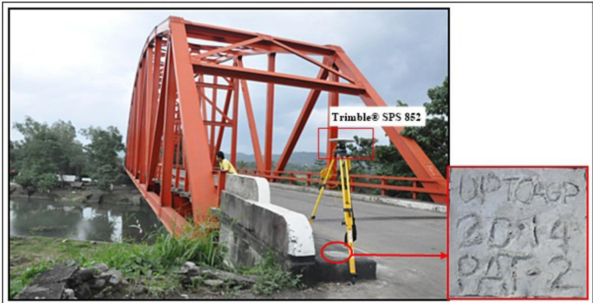
Figure 35. GNSS base receiver, Trimble® SPS 852, setup at PAT-2 in Pateng Bridge, Brgy. Pateng, Municipality of Gonzaga, Cagayan
