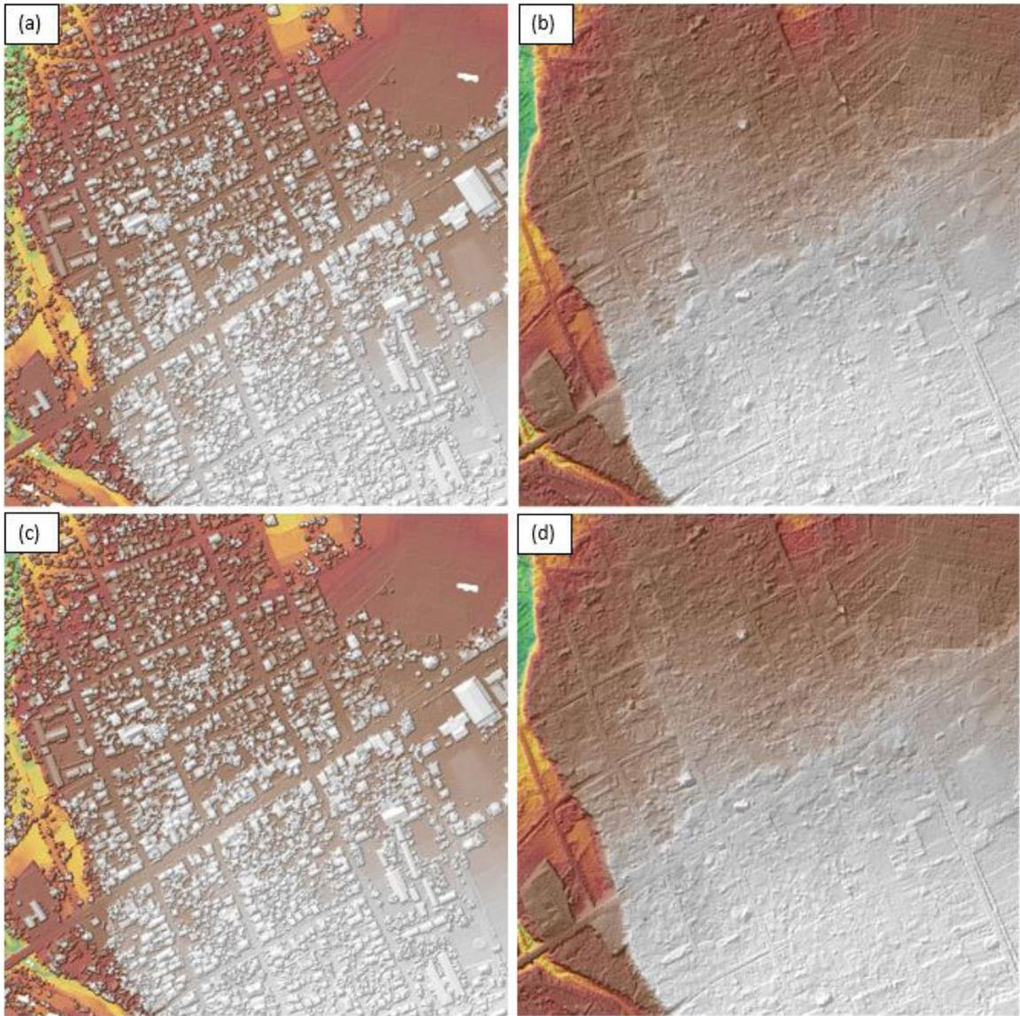
Figure 22. The production of last return DSM (a) and DTM (b), first return DSM (c) and secondary DTM (d) in some portion of Aunugay Floodplain
