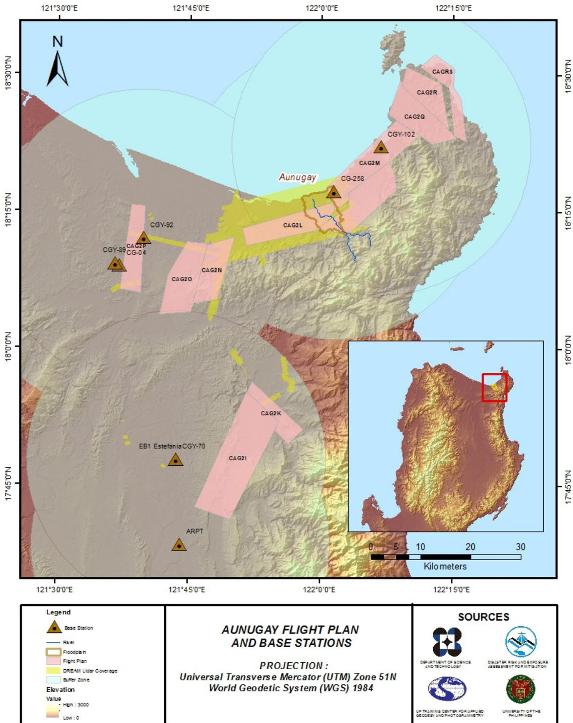
Figure 2. Flight plan and base stations used for Aunugay Floodplain
