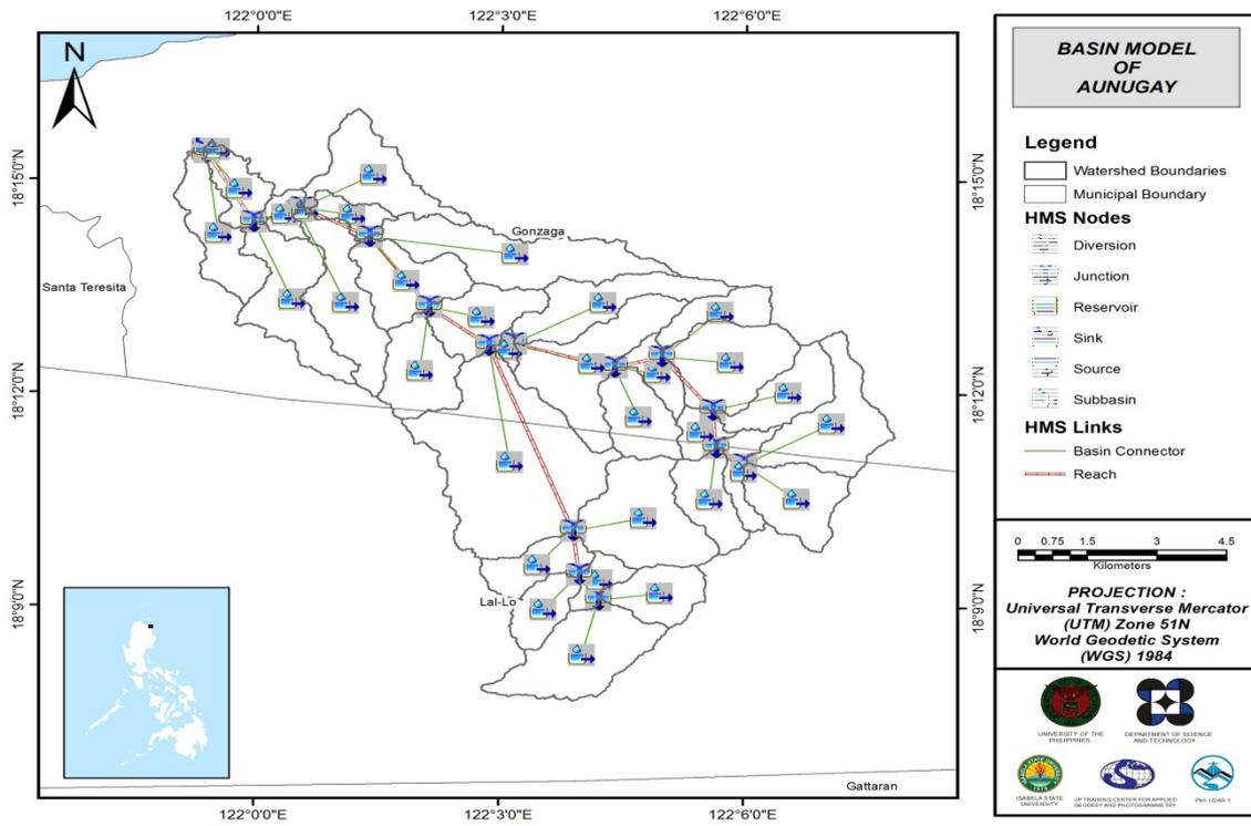
Figure 57. The Aunugay river basin model generated in HEC-HMS
