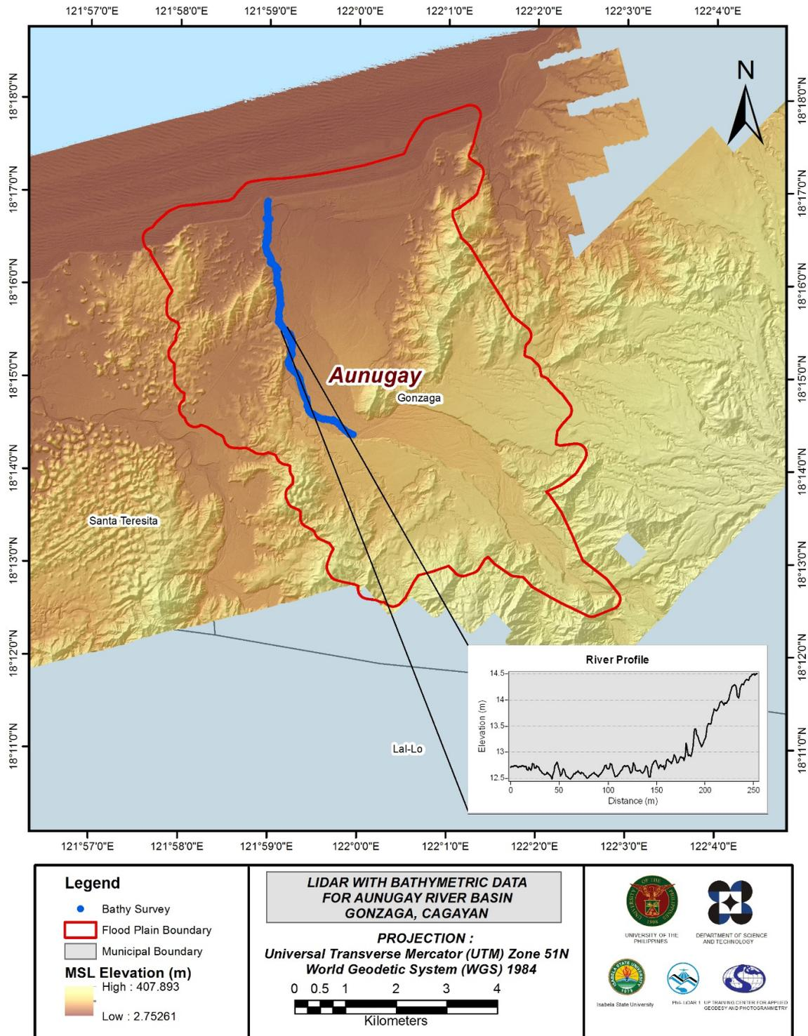
Figure 30. Map of Aunugay Floodplain with bathymetric survey points shown in blue.
