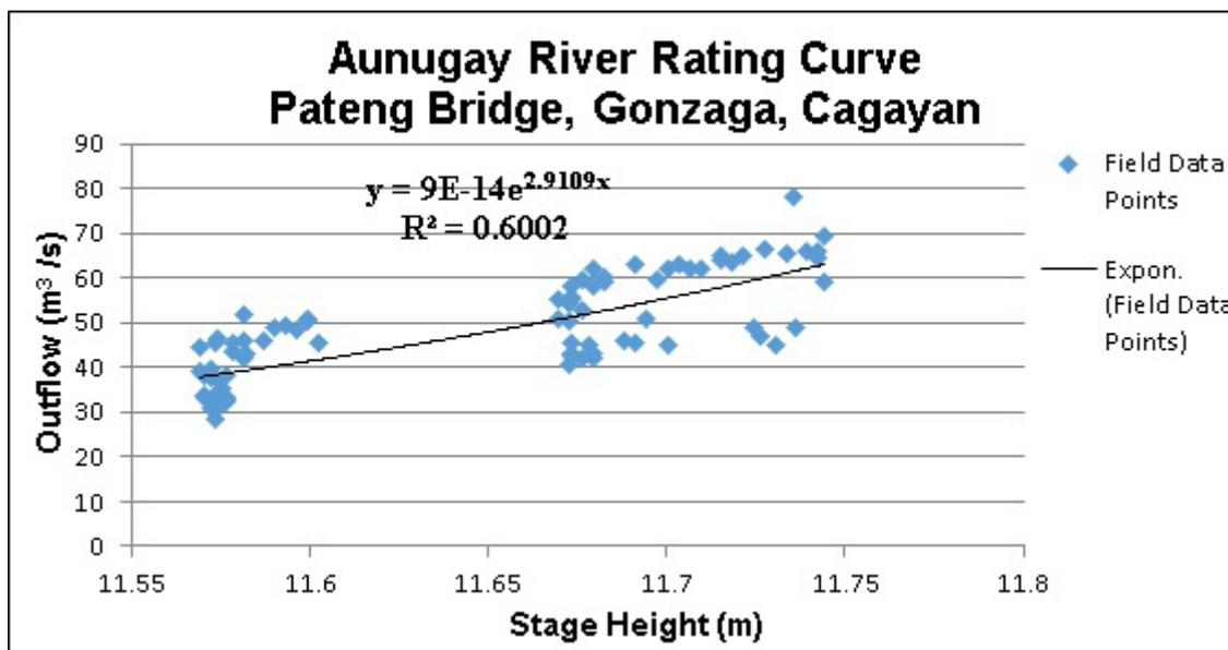
Figure 50. HQ Curve of HEC-HMS model
