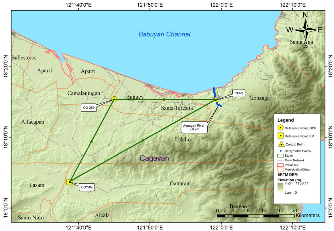
Figure 33. GNSS network of Aunugay River field survey
