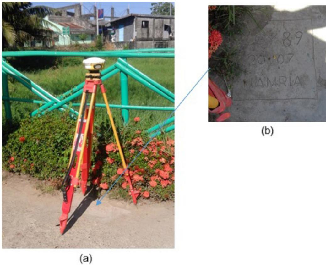
Figure 5. GPS set-up over CGY-89 located on the left side of the access to Logac National High School in Barangay Logac, Municipality of Lal-lo (a) and NAMRIA horizontal reference point CGY-89 (b) as recovered by the field team
