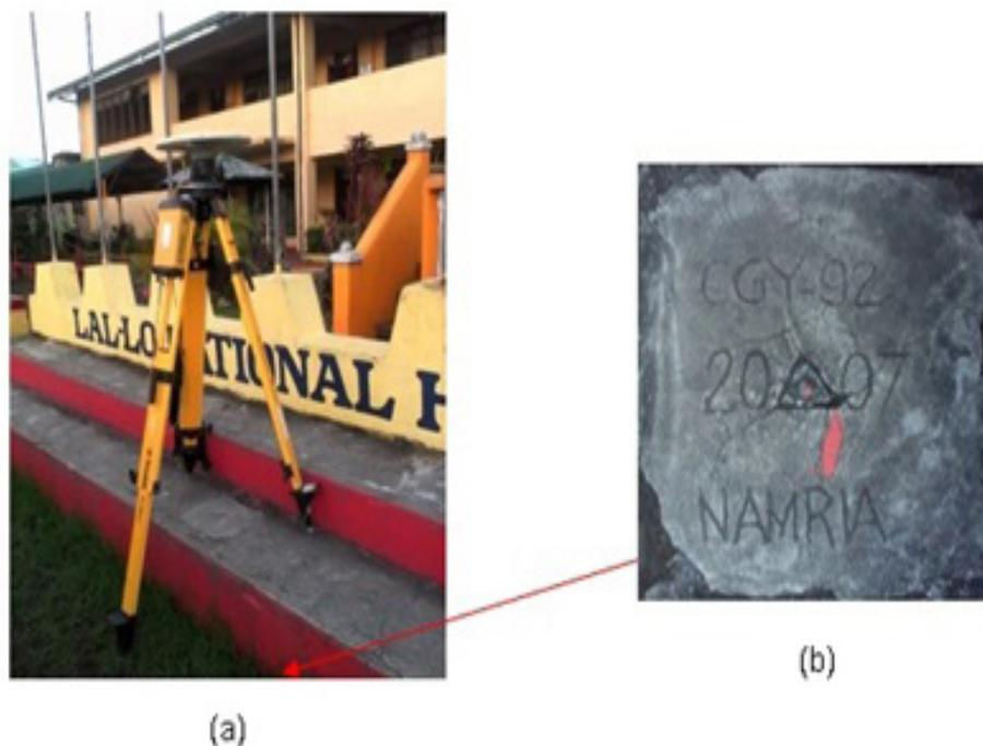
Figure 6. GPS set-up over CGY-92 at Lal-lo National High School (a) and NAMRIA reference point CGY-92 (b) as recovered by the field team
