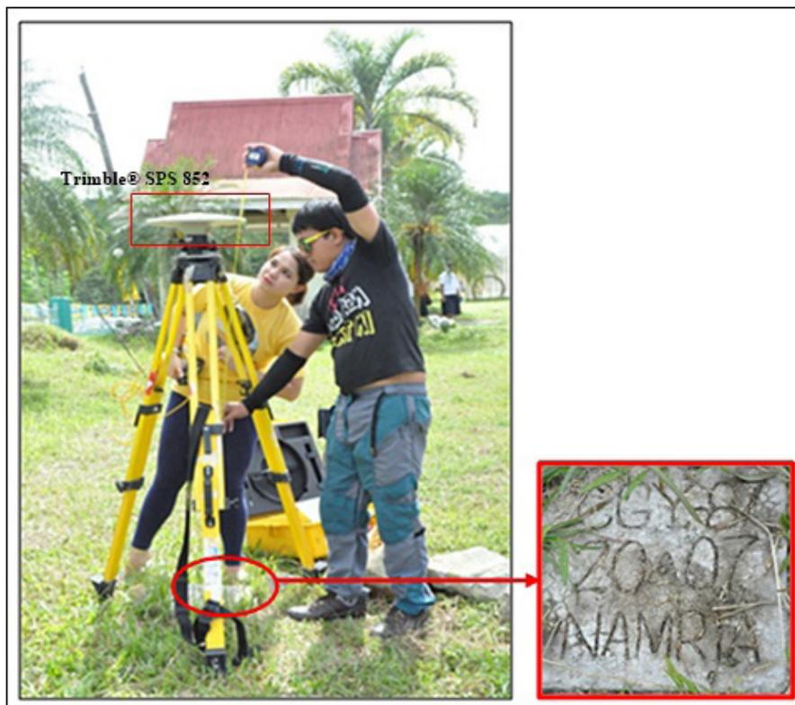
Figure 34. GNSS base receiver, Trimble® SPS 852 setup at CGY-87 in Brgy. Centro Sur, Municipality of Gattaran, Cagayan
