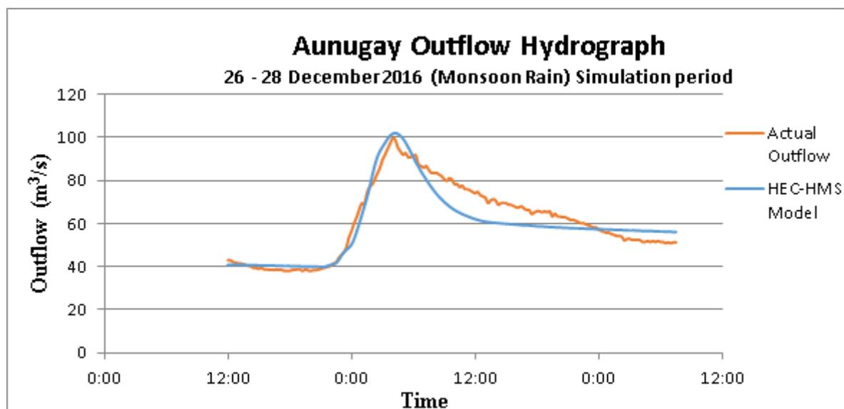
Figure 60. Outflow Hydrograph of Aunugay produced by the HEC-HMS model compared with observed outflow
