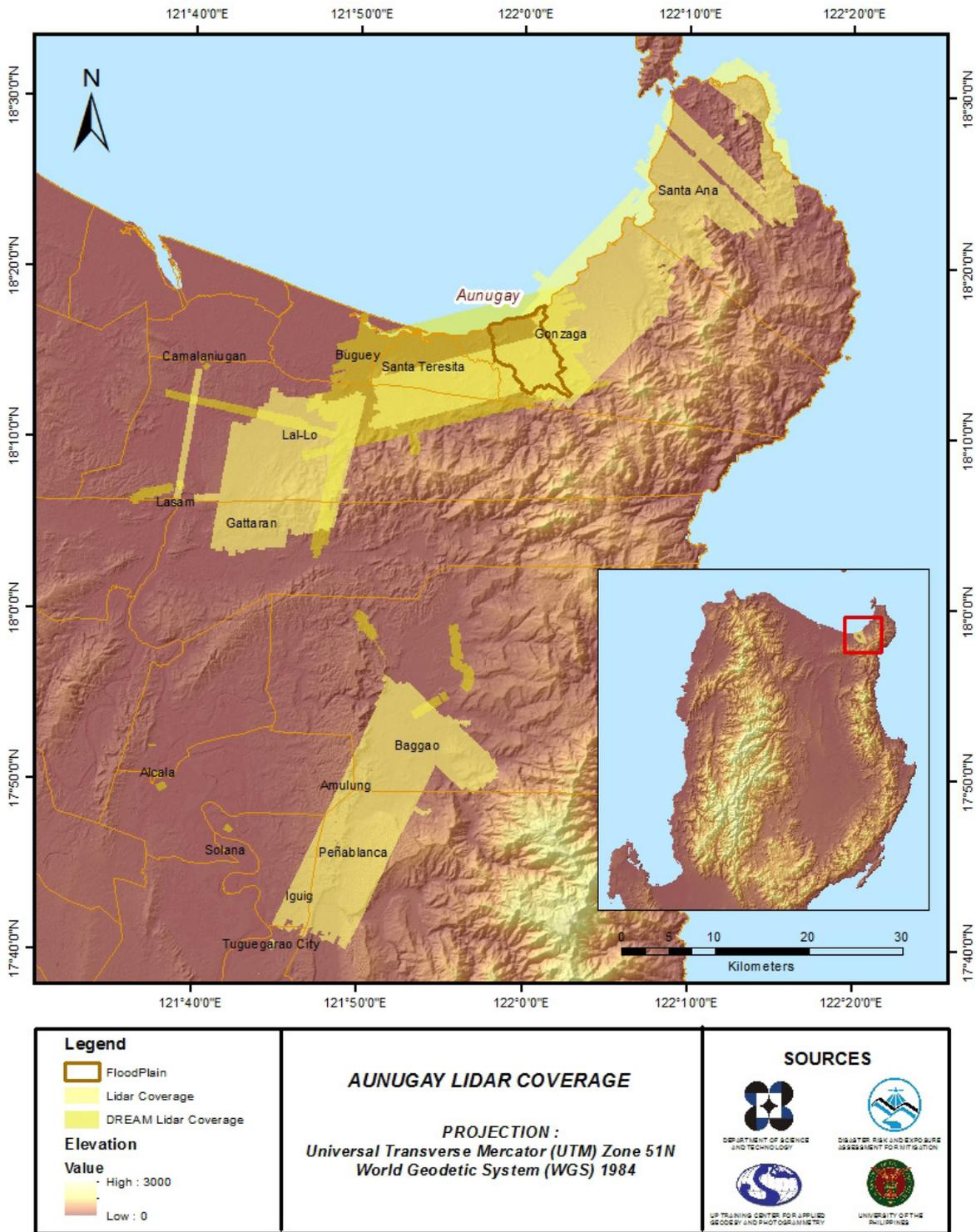
Figure 10. Actual LiDAR survey coverage for Aunugay Floodplain.
