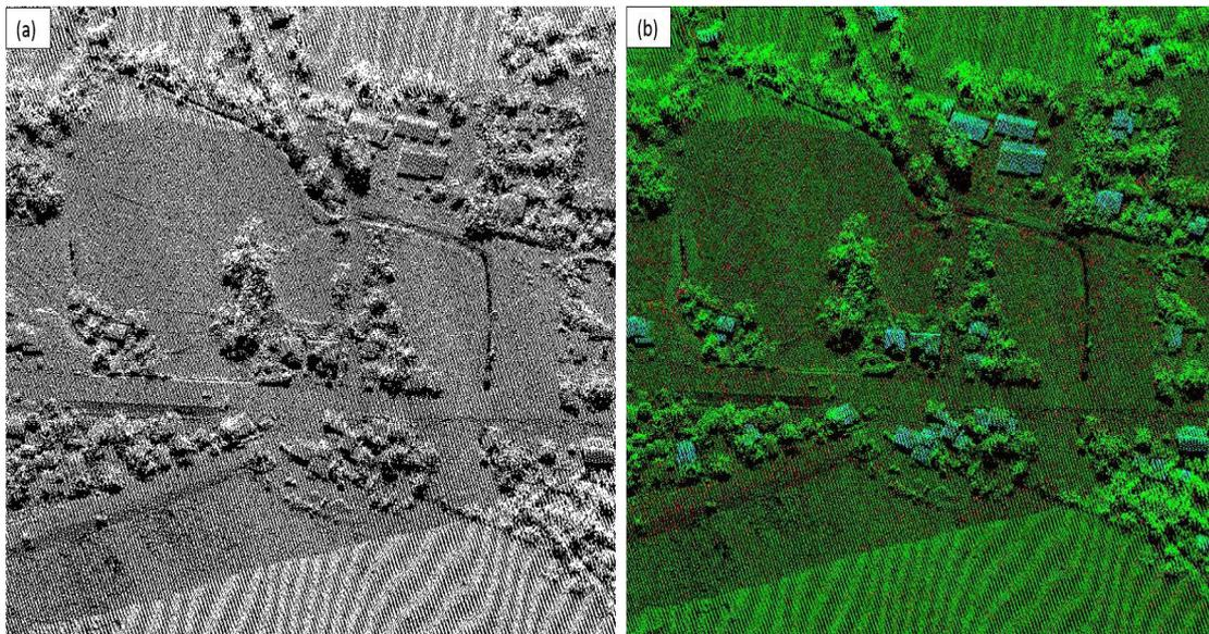
Figure 21. Point cloud before (a) and after (b) classification
