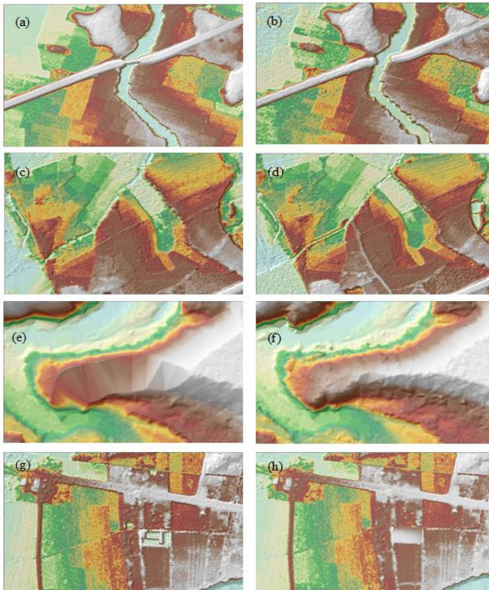
Figure 25. Portions in the DTM of Aunugay Floodplain – a road before (a) and after (b) manual editing; a paddy field before (c) and after (d) data retrieval; interpolated bank before (e) and after (f) object retrieval; and a building before (g) and after (h) manual editing
