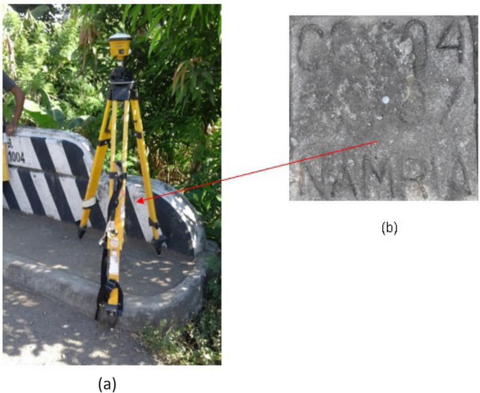
Figure 8. GPS set-up over CG-04 in the municipality of Lal-lor (a) and NAMRIA reference point CG-04 (b) as recovered by the field team
