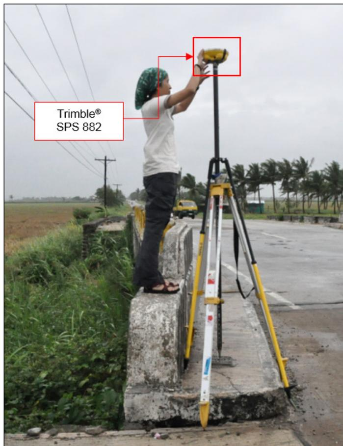
Figure 34. GNSS receiver, Trimble® SPS 882, setup at CG-289 in Cullit Bridge, Brgy. Dalaya, Municipality of Buguey, Cagayan
