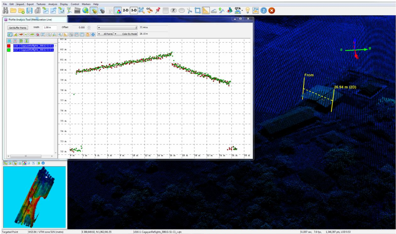
Figure 19. Quality checking for Aunugay flight 3981G using the Profile Tool of QT Modeler
