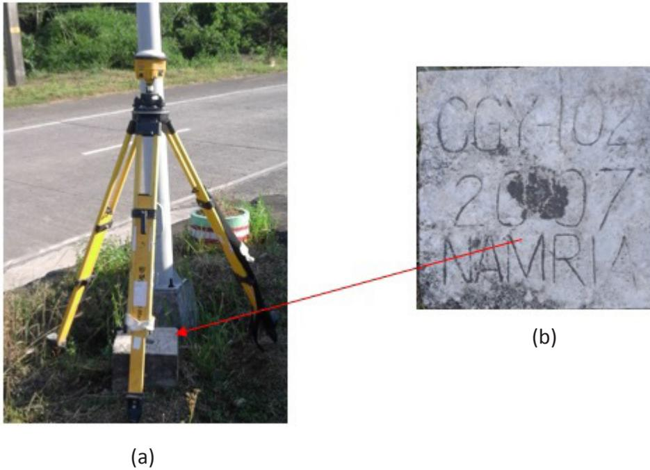
Figure 7. GPS set-up over CGY-102 at the intersection of the national highway and the road to Port Irene (a) and NAMRIA reference point CGY-102 (b) as recovered by the field team
