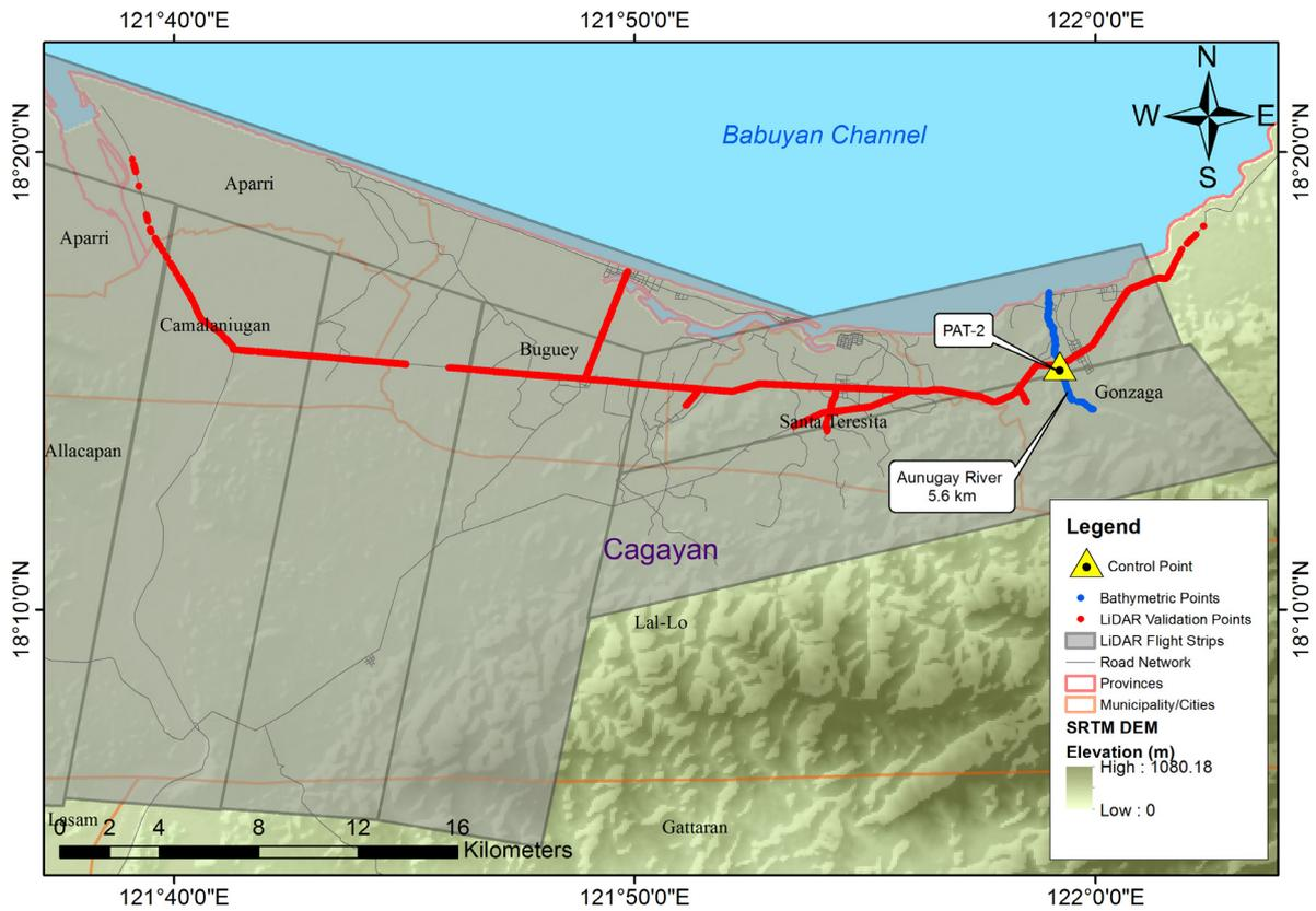
Figure 42. Validation Points Acquisition survey along Aunugay River Basin
