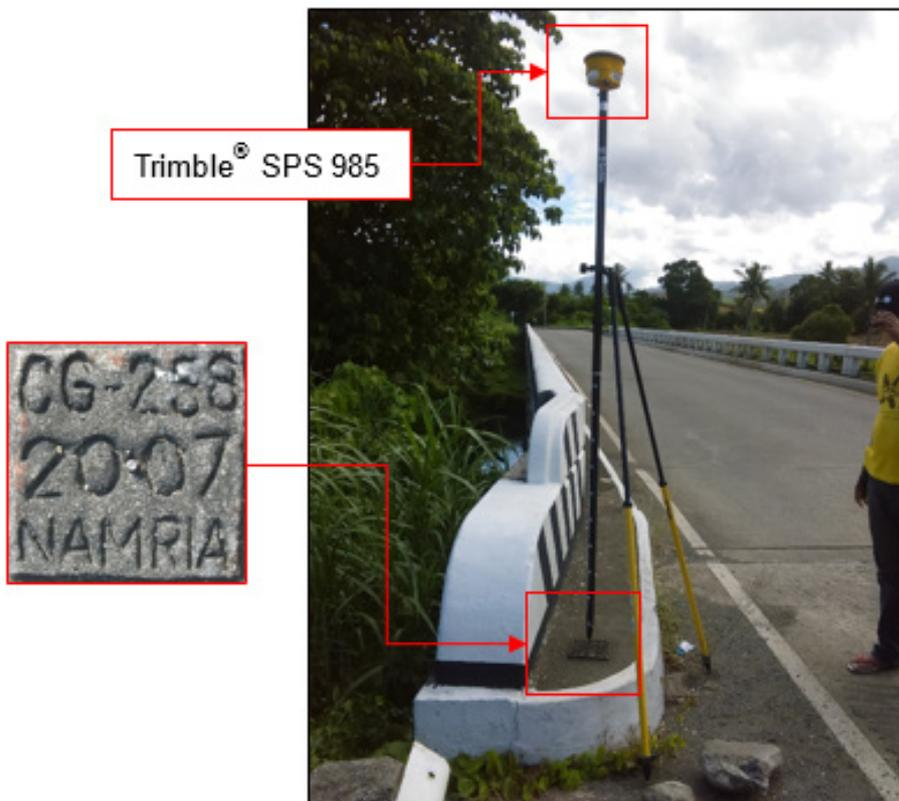
Figure 34. GNSS receiver set up, Trimble® SPS 985, at CG-258, located at the approach of the bridge near the welcome arch of Brgy. Tapel, Gonzaga, Cagayan
