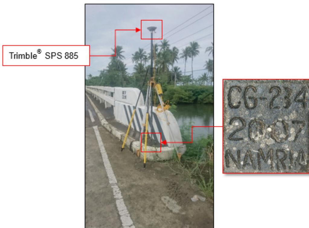
Figure 37. GNSS receiver set-up, Trimble® SPS 885, at CG-234, located at the approach of Diara Bridge in Brgy. Diara-Zinungan, Sta. Ana, Cagayan
