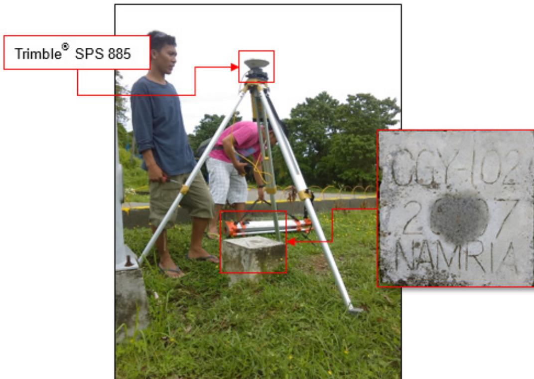
Figure 36. GNSS receiver set-up, Trimble® SPS 885, at CGY-102, located at the center island in front of the barangay marker of Brgy. Casambalangan in Brgy. San Jose, Gonzaga, Cagayan
