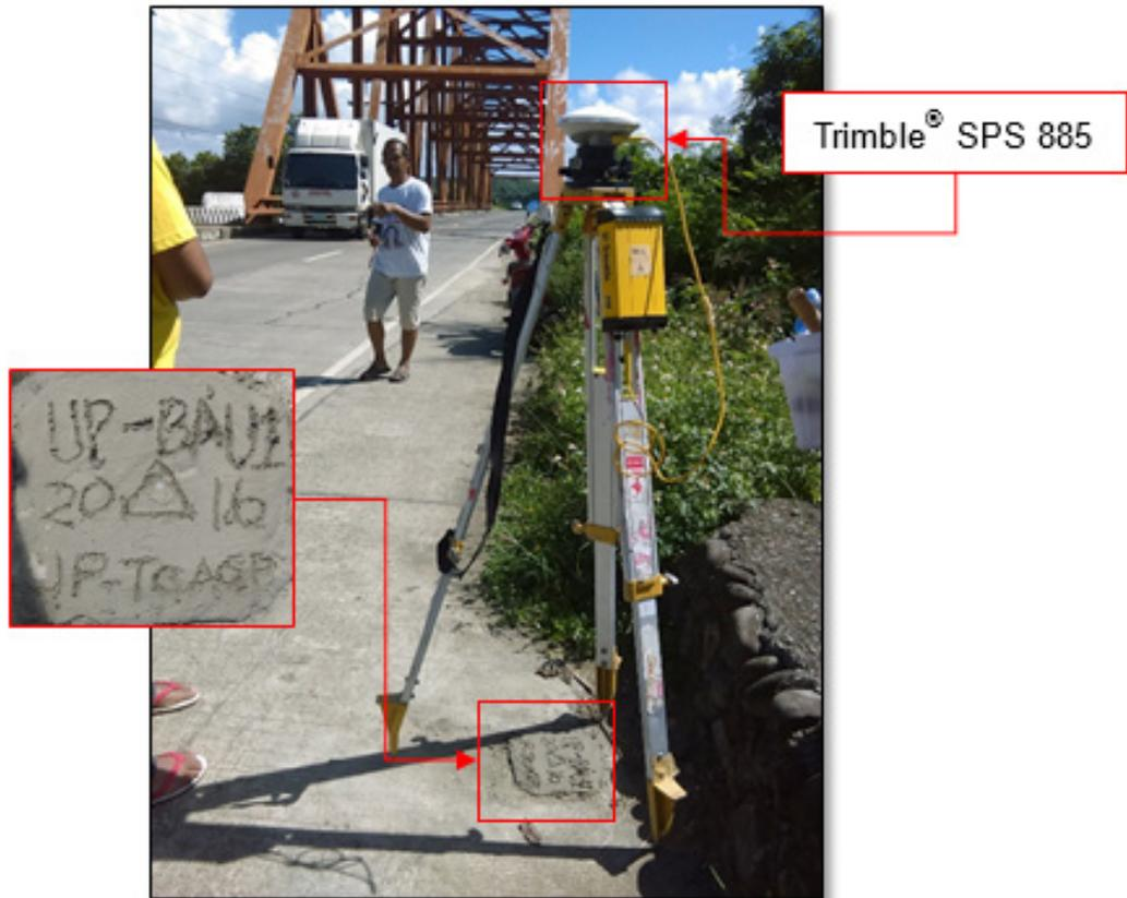
Figure 35. GNSS receiver set up, Trimble® SPS 885, at UP-BAU-1, located at the approach of Baula Bridge in Brgy. Baula, Gonzaga, Cagayan
