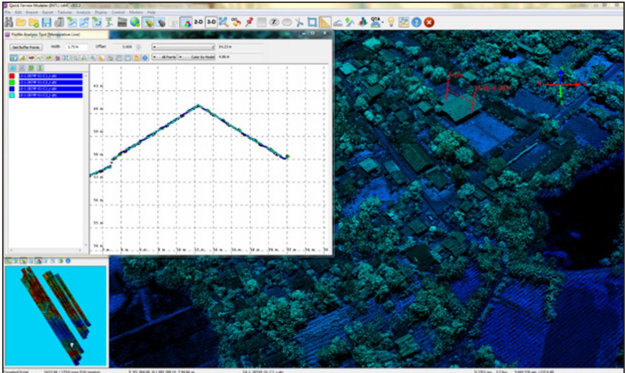
Figure 14. Quality checking for Cabicungan Flight 2874P, using the Profile Tool of QT Modeler
