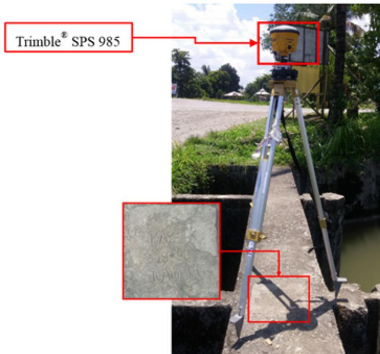
Figure 30. GNSS base set-up, Trimble® SPS 985 at KAY-3, situated on top of a flood gate near the Pudtol Municipal Building in Barangay Imelda, Municipality of Pudtol, Cagayan
