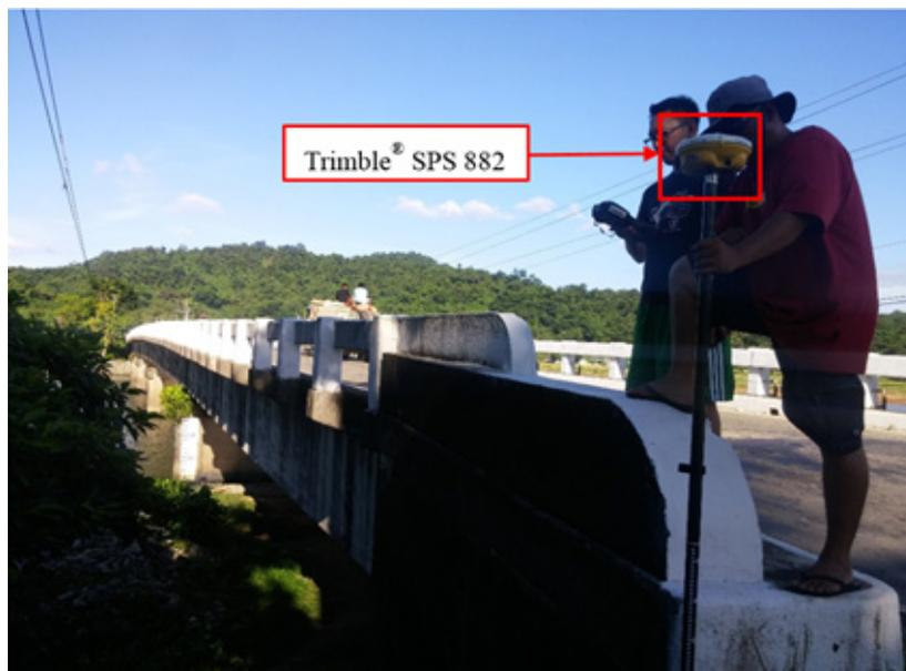
Figure 37. As-built survey of the Cabicungan Bridge
