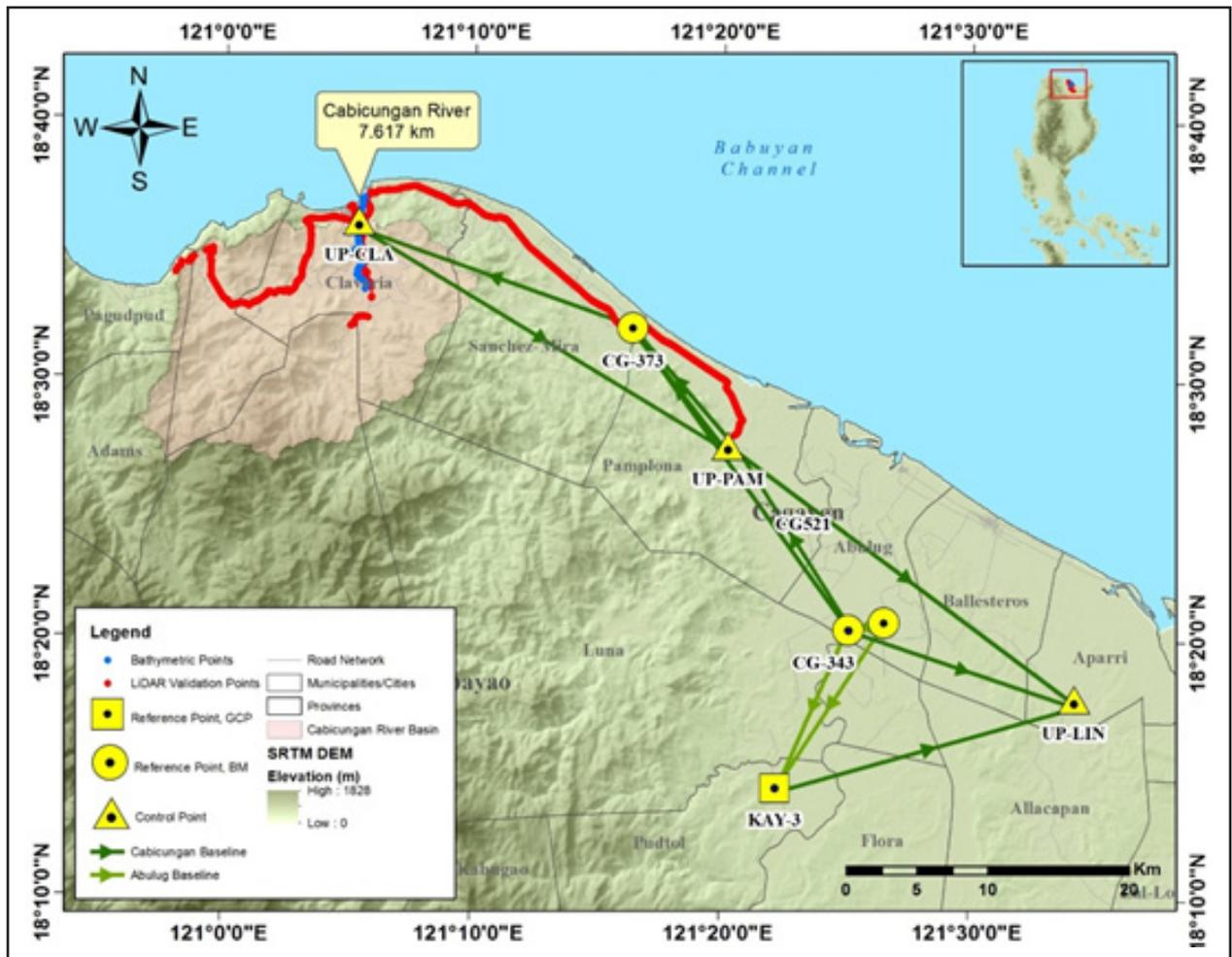
Figure 28. Extent of the bathymetric survey (in blue line) in Cabicungan River and the LiDAR data validation survey (in red)
