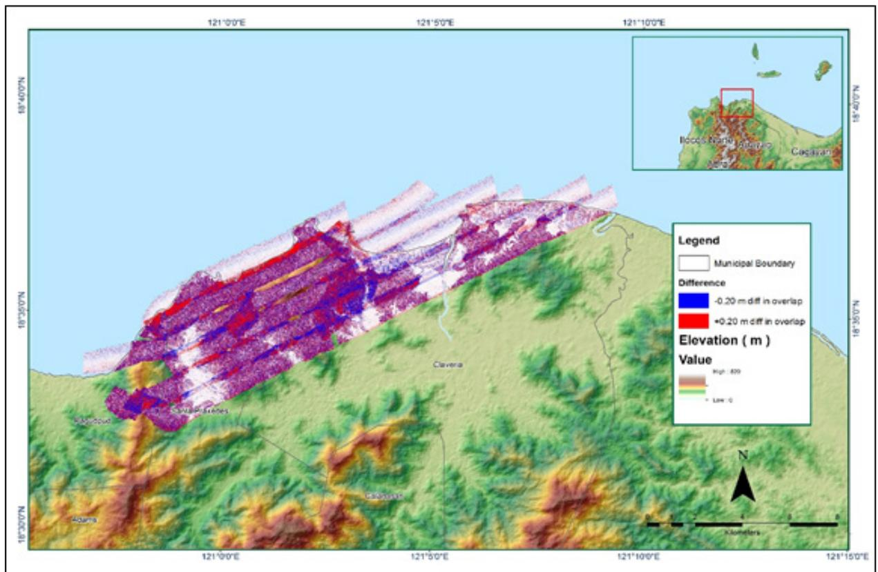
Figure A-7.7. Elevation difference between flight lines
