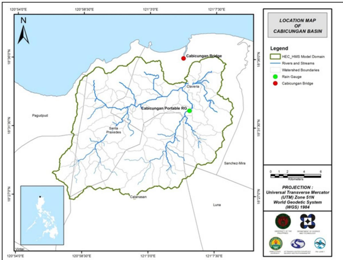
Figure 47. Location map of the Cabicungan HEC-HMS model, which was used for calibration
