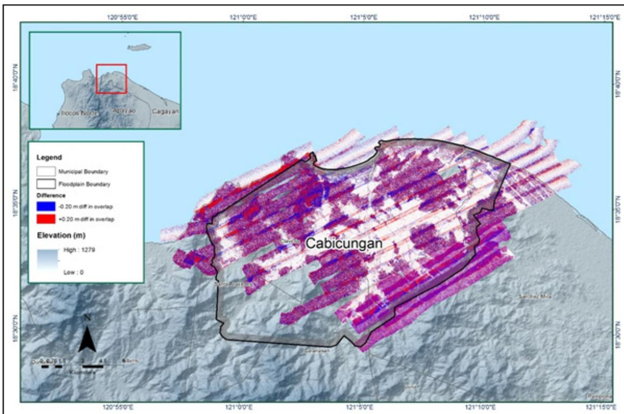
Figure 13. Elevation difference map between flight lines for the Cabcungan floodplain
