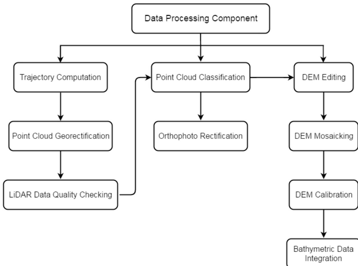
Figure 6. Schematic diagram for the Data Pre-Processing Component
