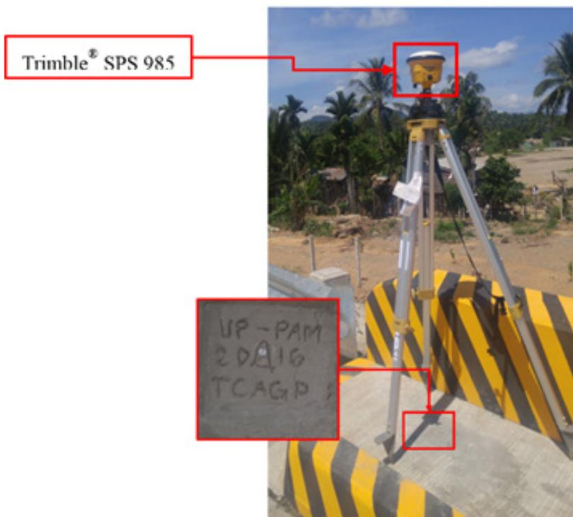
Figure 35. GNSS receiver set-up, Trimble® SPS 985 at UP-PAM, located at the approach of the New Pamplona Bridge in Barangay Masi, Municipality of Pamplona, Cagayan
