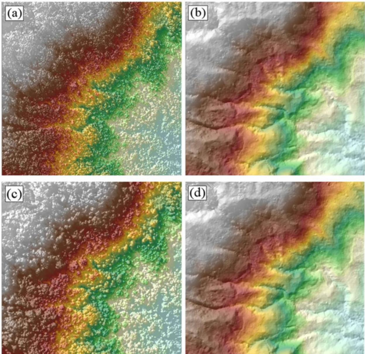
Figure 17. (a) The production of last return DSM and (b) DTM; and (c) first return DSM and (d) secondary DTM in some portion of the Cabicungan floodplain
