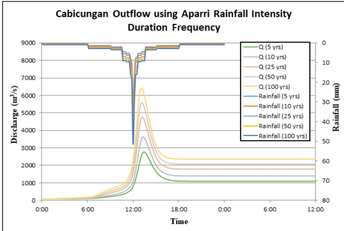
Figure 61. Outflow hydrograph at the Cabicungan Station generated using the Aparri RIDF, simulated in HEC-HMS
