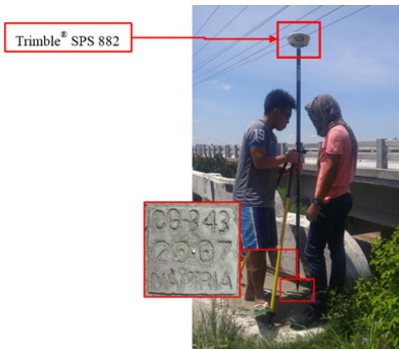
Figure 31. Trimble® SPS 882 GNSS receiver setup at BH-503 located inside the campus of Dao Elementary School, Brgy. Dao, Municipality of Dauis, Bohol
