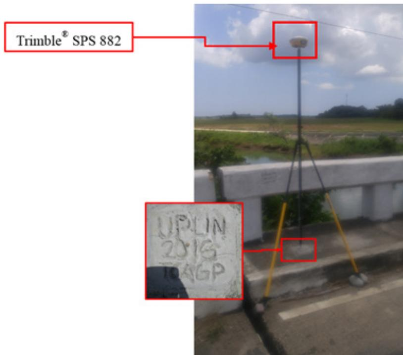
Figure 34. GNSS receiver set-up, Trimble® SPS 882 at UP-LIN, located at the approach of the Linao Bridge in Barangay Bangag-Zingag, Municipality of Aparri, Cagayan
