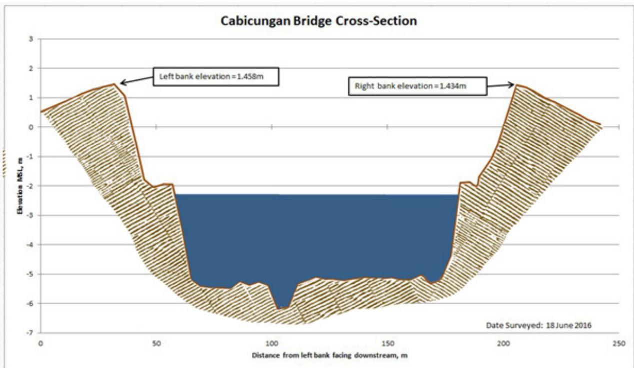
Figure 48. Cross-section plot of the Cubicungan Bridge
