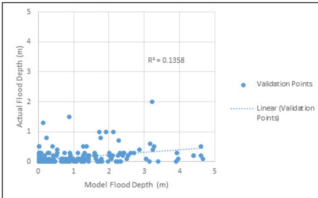
Figure 94. Model flood depth vs. actual flood depth
