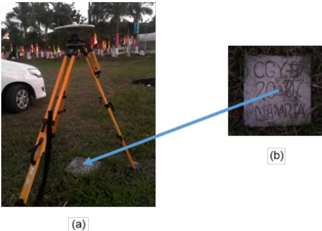
Figure 4. (a) GPS set-up over CGY-87, located on a solar dryer at Barangay Cabayabasan, fronting the barangay hall in the Municipality of Lal-lo; and (b) NAMRIA reference point CGY-87, as recovered by the field team
