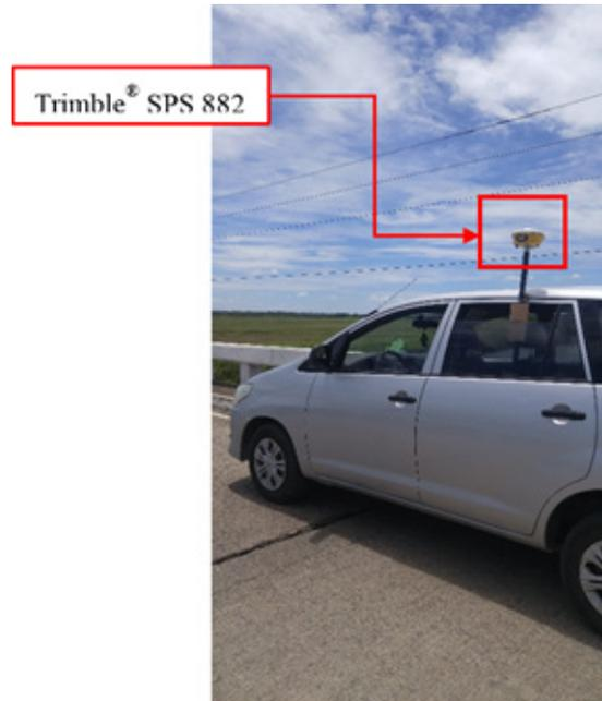
Figure 42. Validation points acquisition survey set-up along the Cabicungan River Basin
