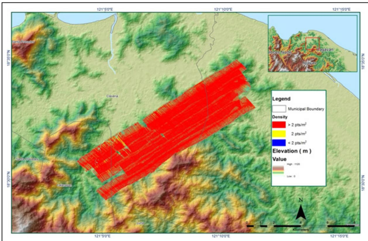
Figure A-7.20. Density map of merged LiDAR data
