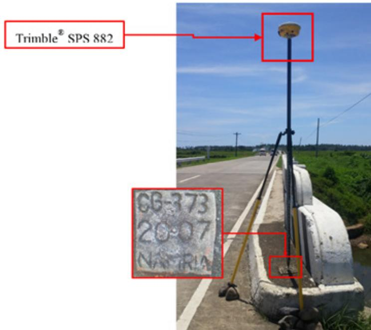
Figure 32. GNSS receiver set-up, Trimble® SPS 882 at CG-373, located at the approach of the Bangan Bridge in Barangay Bangan, Municipality of Sanchez Mira, Cagayan
