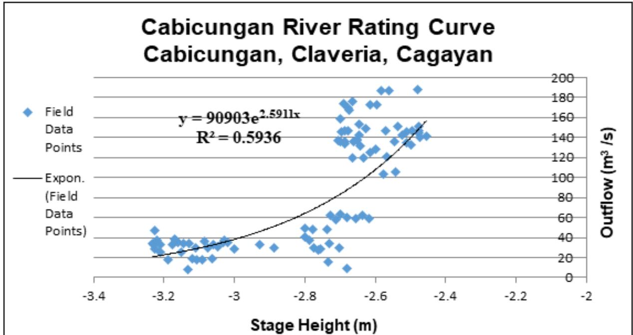
Figure 50. Rating curve at the Cabicungan Bridge, Claveria, Cagayan
