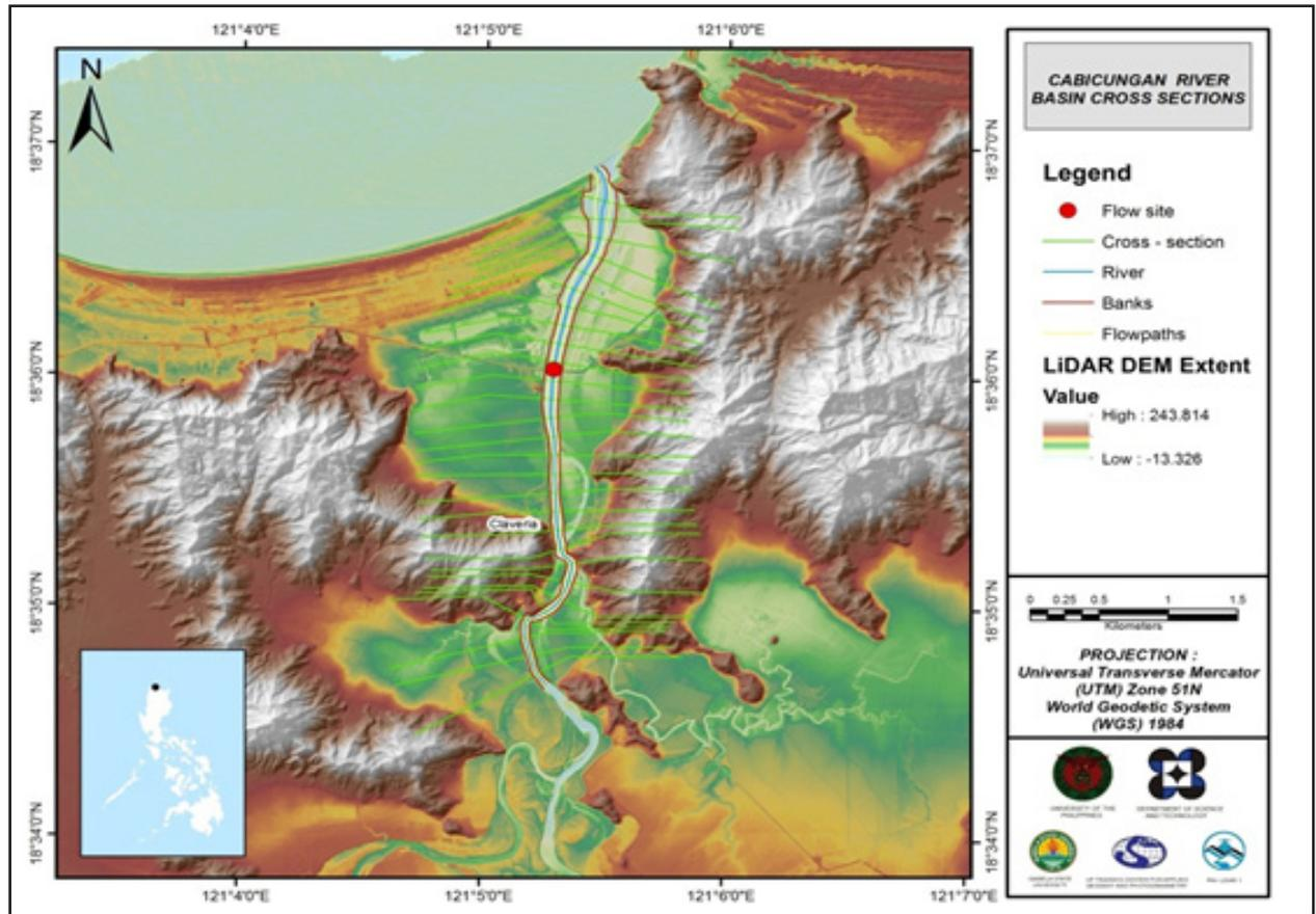
Figure 58. Cabicungan River cross-section, generated using the HEC GeoRAS tool
