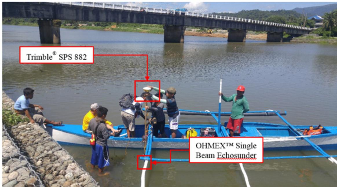
Figure 44. Bathymetric survey using Ohmex™ single beam echo sounder in the Cabicungan River
