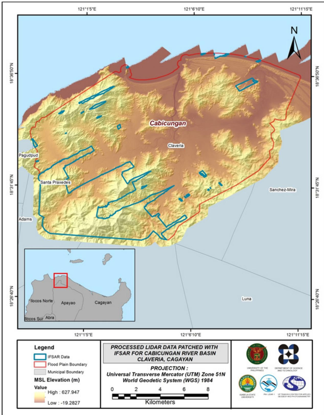
Figure 21. Map of processed LiDAR data for the Cabicungan floodplain
