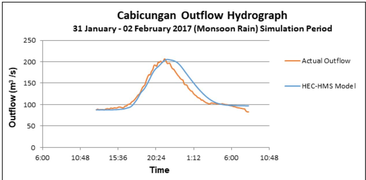
Figure 60. Outflow hydrograph of Cabicungan produced by the HEC-HMS model, compared with observed outflow
