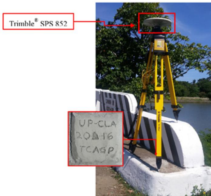
Figure 33. GNSS receiver set-up, Trimble® SPS 852 at UP-CLA, located at the approach of the Cabicungan Bridge in Barangay Dibalio, Municipality of Claveria, Cagayan
