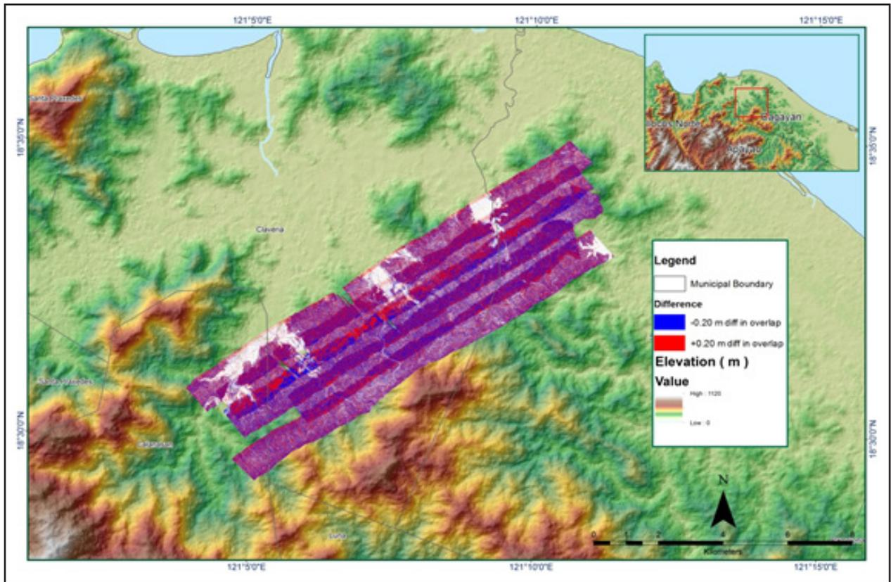
Figure A-7.21. Elevation difference between flight lines
