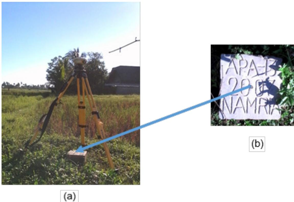
Figure 3. (a) GPS set-up over APA-13, located at the edge of the PCCP, 70 meters northeast of a waiting shed near the barangay hall in Tumog, Municipality of Luna; and (b) NAMRIA reference point APA-13, as recovered by the field team
