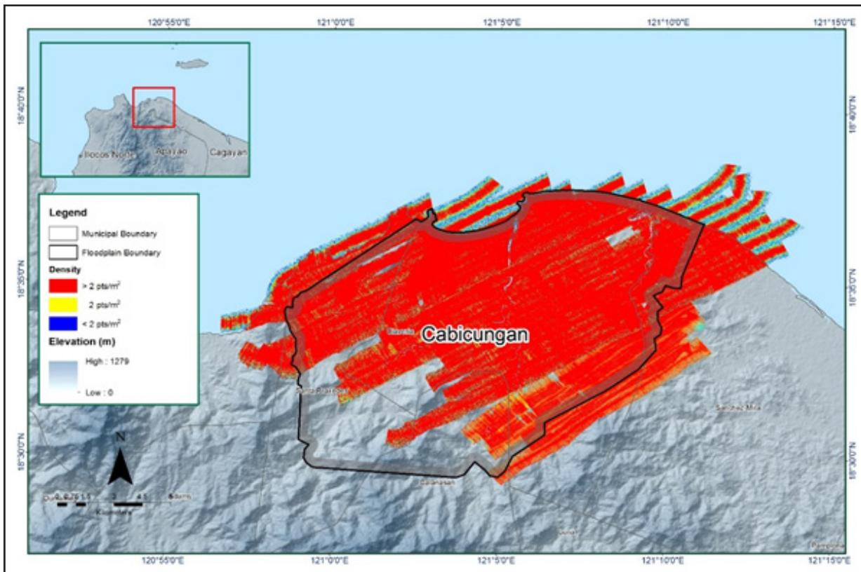
Figure 12. Pulse density map of merged LiDAR data for Cabcungan floodplain
