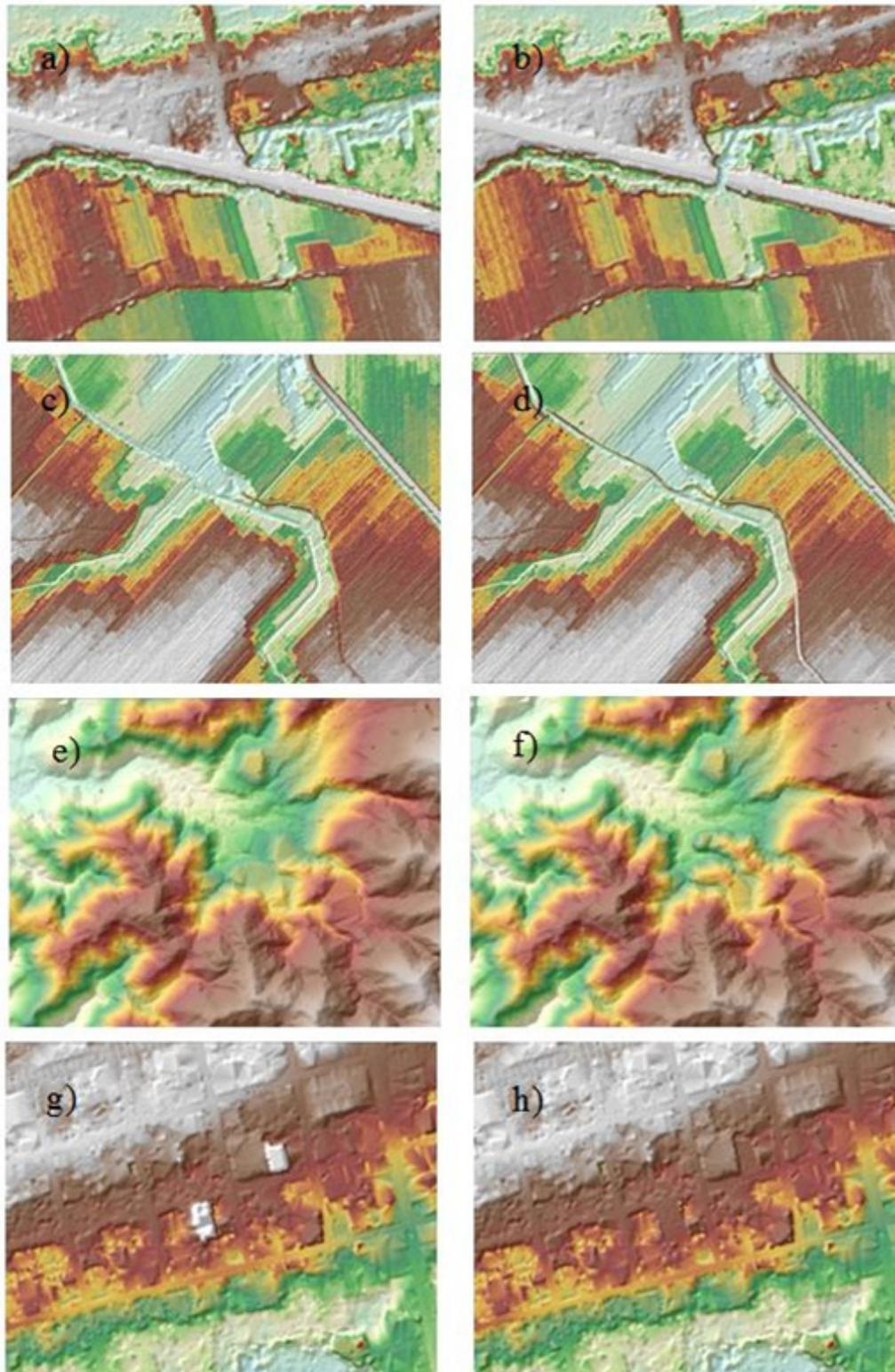
Figure 20. Portions in the DTM of the Cabicungan floodplain – a bridge (a) before and (b) after interpolation; an irrigation (c) before and (d) after object retrieval; interpolated ridge (e) before and (f) after object retrieval; and a building (g) before and (h)
