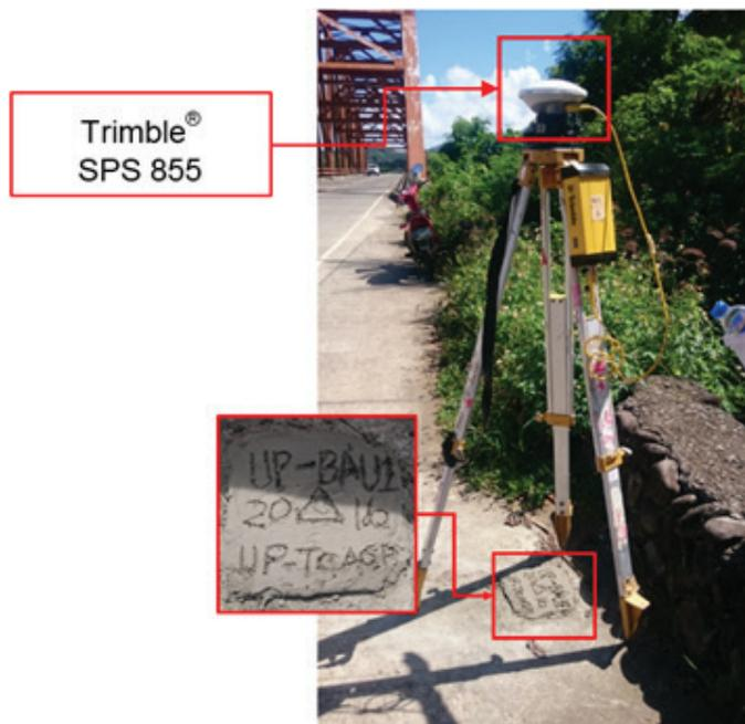
Figure 32. GNSS receiver setup, Trimble® SPS 855, at UP-BAU1, located at the approach of Baua Steel bridge in Brgy. Baua, Municipality of Gonzaga, Cagayan
