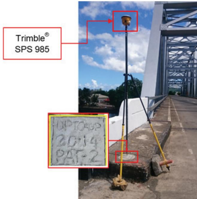
Figure 27. GNSS receiver setup, Trimble® SPS 985, at PAT-2, located at the approach of Pateng Bridge in Brgy. Pateng, Municipality of Gonzaga, Cagayan
