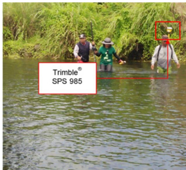
Figure 42. Manual bathymetric survey using a Trimble® SPS 985 in GNSS PPK survey technique in Casambalangan River
