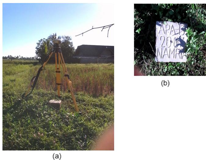
Figure 3. GPS set-up over APA-13 located at the edge of the PCCP, 70 meters northeast of a waiting shed near the barangay hall in Tumog, Municipality of Luna.
