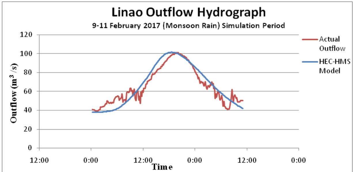
Figure 63. Outflow Hydrograph of Linao produced by the HEC-HMS model compared with observed outflow.
