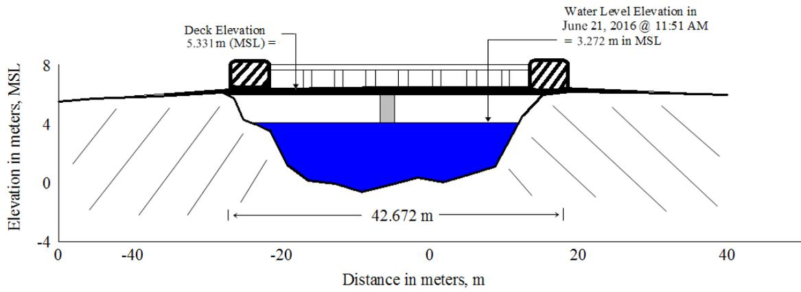
Figure 42. Linao Bridge cross-section diagram
