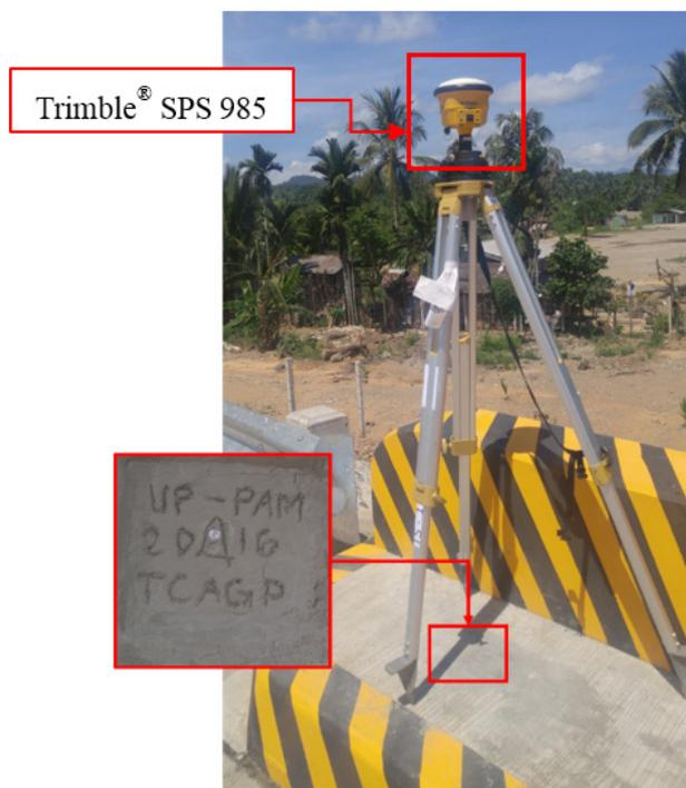
Figure 39. GNSS receiver set-up, Trimble® SPS 985, at UP-PAM, located at the approach of the New Pamplona Bridge in Barangay Masi, Municipality of Pamplona, Cagayan
