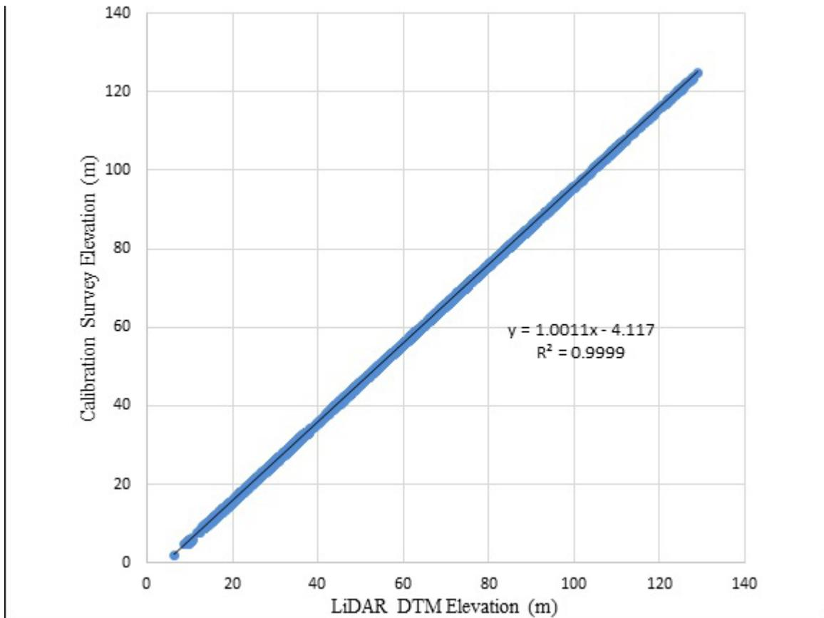
Figure 27. Correlation plot between the calibration survey points and the LiDAR data.
