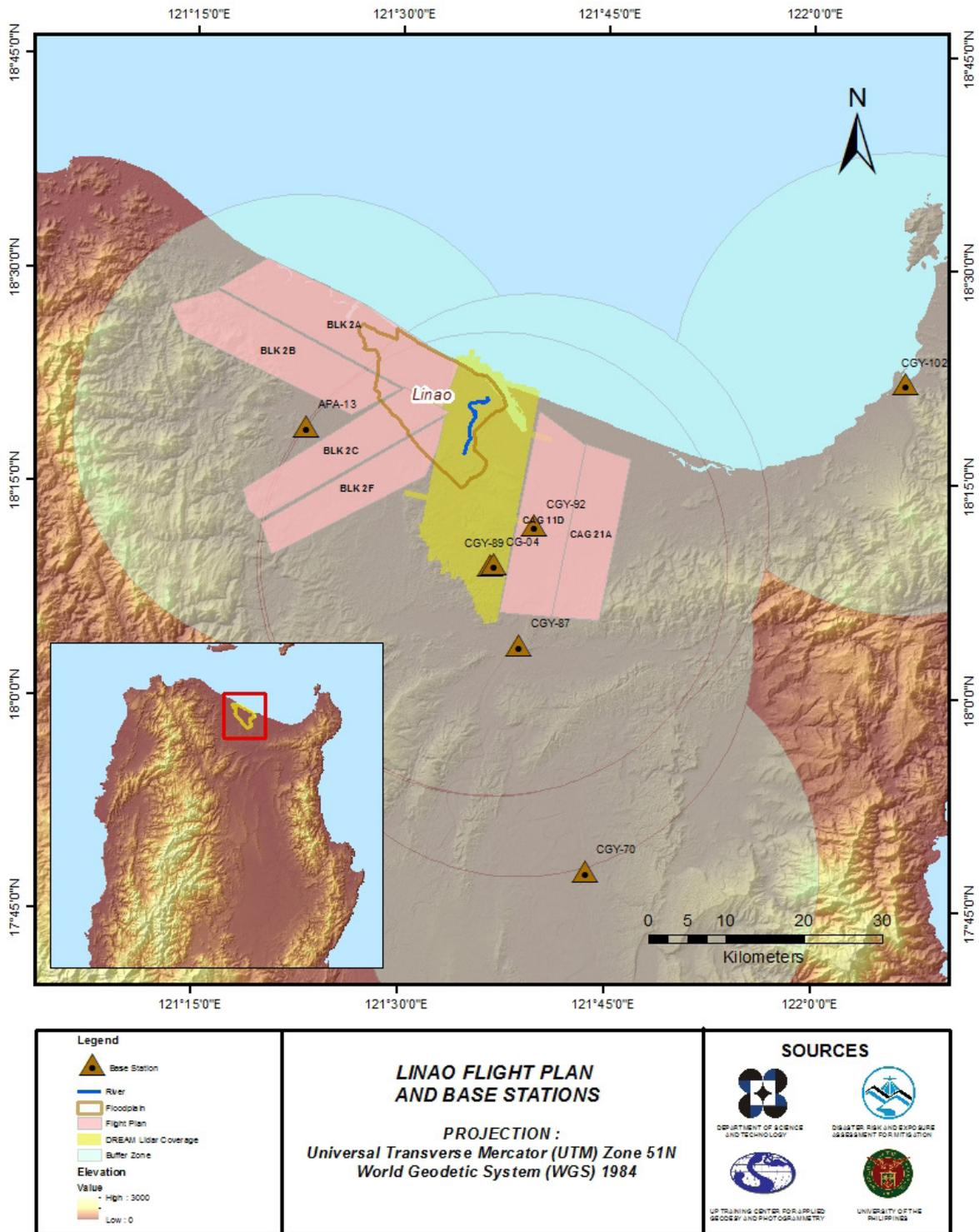
Figure 2. Flight plans and base stations used to cover the Linao floodplain survey
