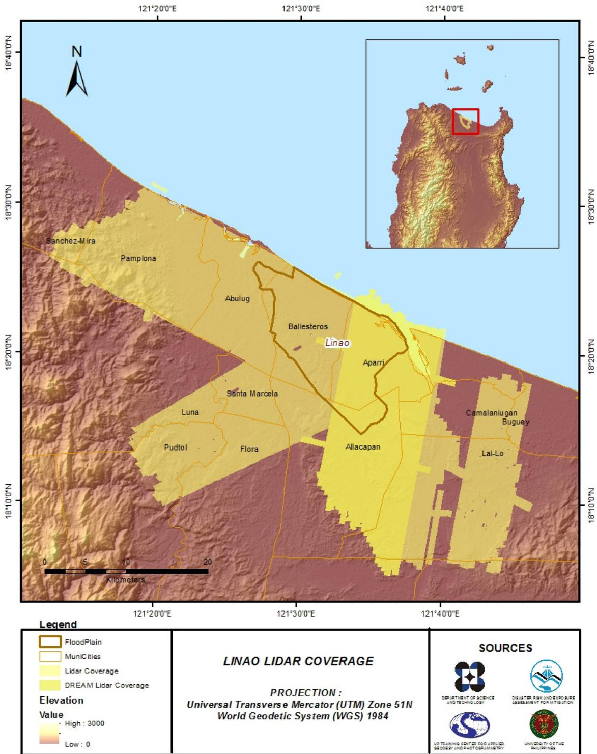
Figure 9. Actual LiDAR survey coverage of the Linao floodplain.
