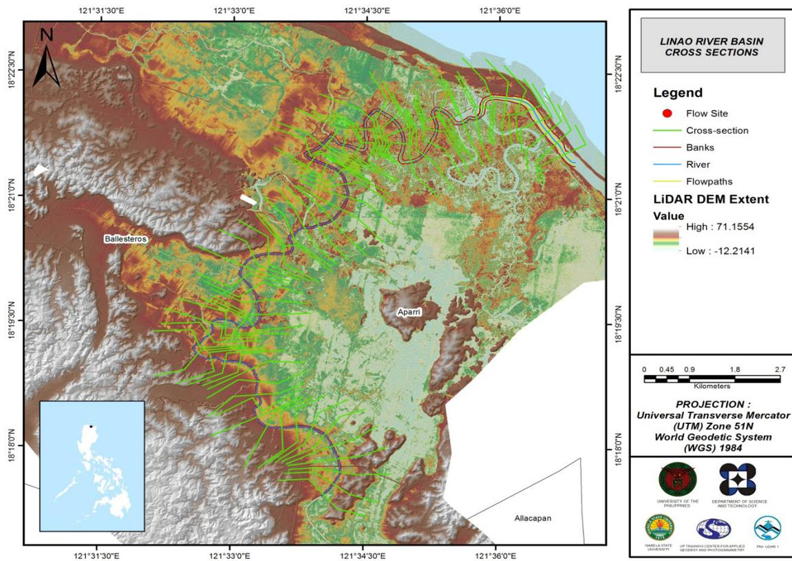
Figure 61. Linao River cross-section generated using HEC GeORAS tool
