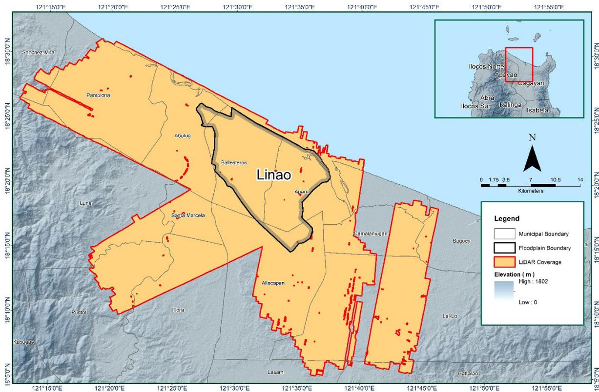
Figure 14. Boundaries of the processed LiDAR data over the Linao Floodplain
