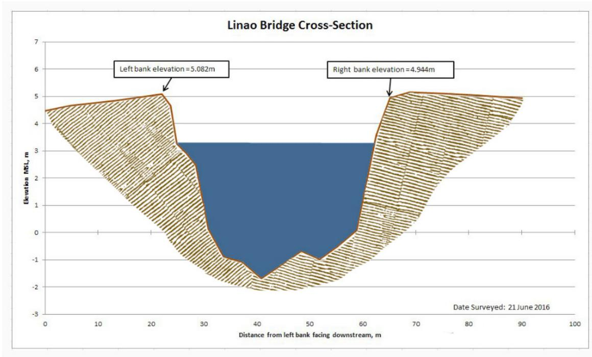
Figure 51. Cross-Section Plot of the Linao Bridge
