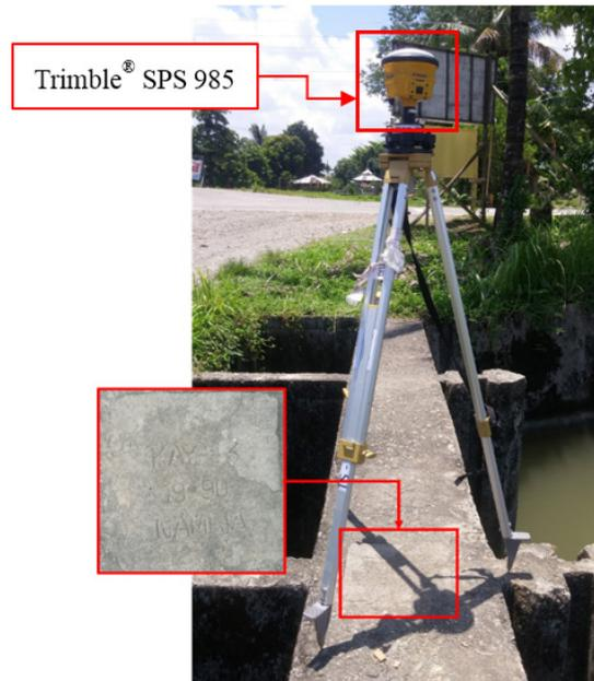
Figure 34. GNSS base set-up, Trimble® SPS 985, at KAY-3, situated on top of the flood gate near Pudtol Municipal Building in Barangay Imelda, Municipality of Pudtol, Cagayan
