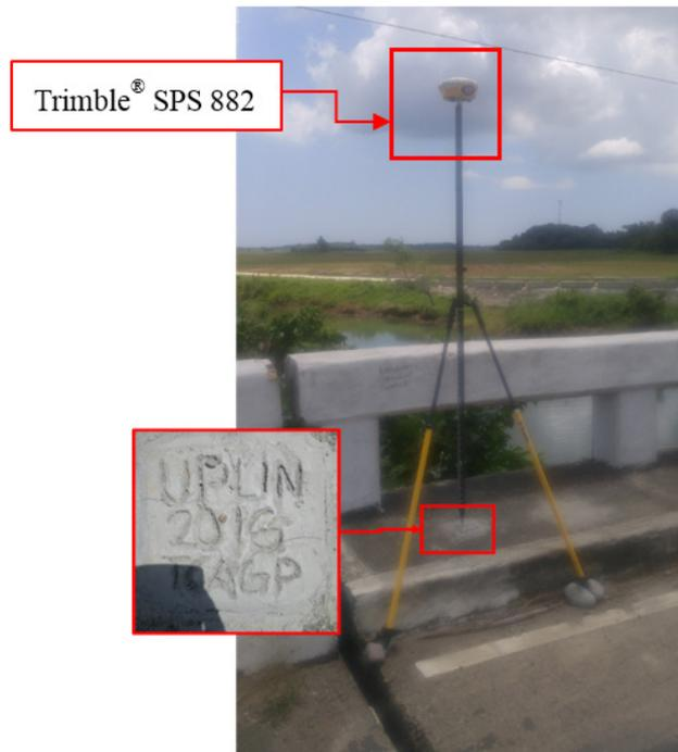
Figure 38. GNSS receiver set-up, Trimble® SPS 882, at UP-LIN, located at the approach of the Linao Bridge in Barangay Bangag-Zingag, Municipality of Aparri, Cagayan
