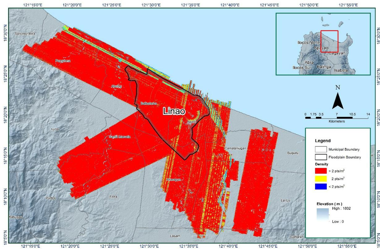
Figure 16. Pulse density map of merged LiDAR data for the Linao floodplain.
