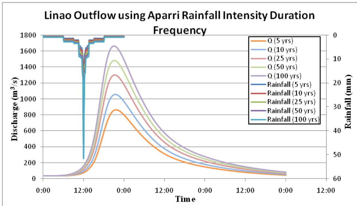
Figure 64. Outflow hydrograph at the Linao Station, generated using the Aparri RIDF simulated in HEC-HMS
