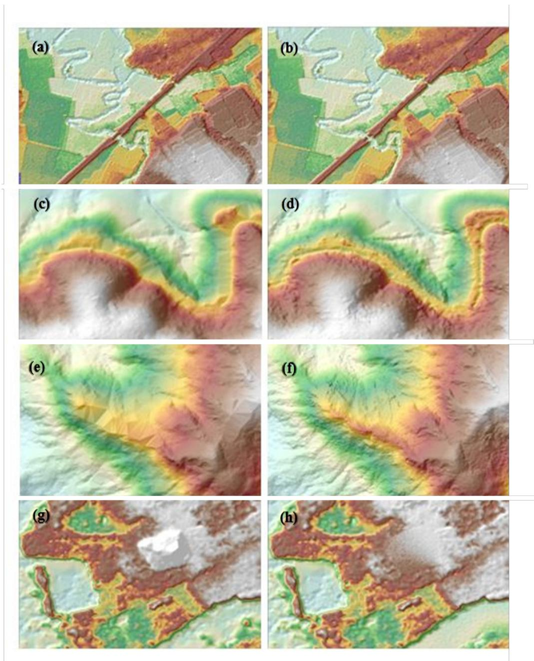
Figure 24. Portions in the DTM of the Linao floodplain – a road before (a) and after (b) manual editing; an irrigation before (c) and after (d) retrieval; interpolated ridge before (e) and after (f) object retrieval; and a building before (g) and after (h) manual editing.
