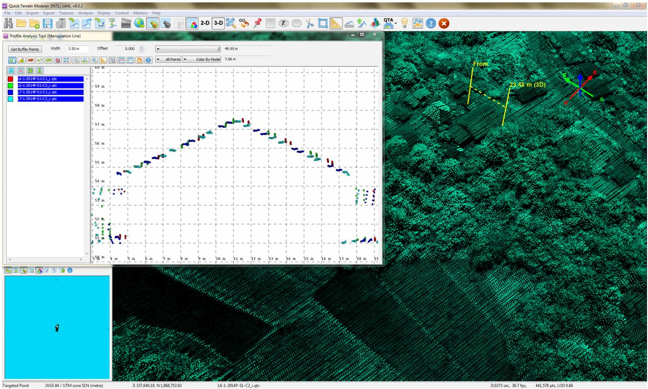
Figure 18. Quality checking for a Linao flight 2914P using the Profile Tool of QT Modeler.
