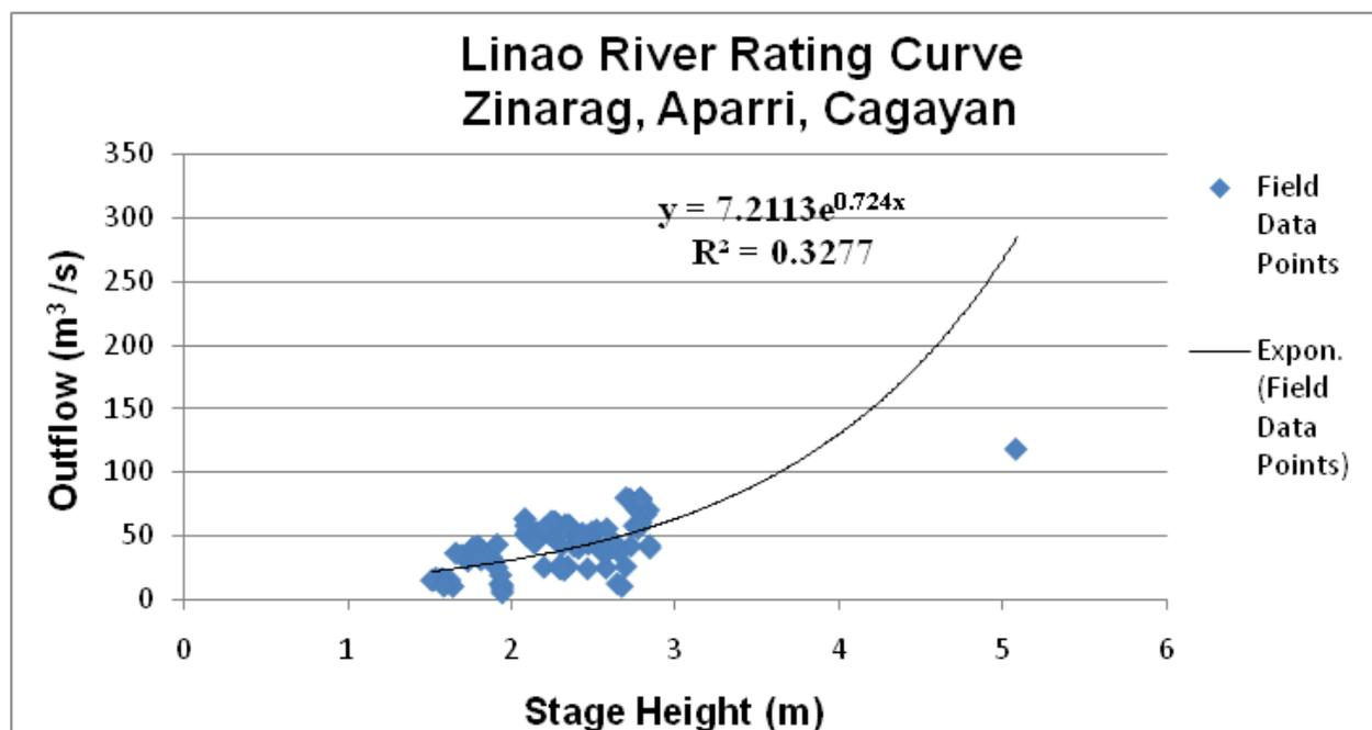
Figure 53. HQ Curve of the HEC-HMS model
