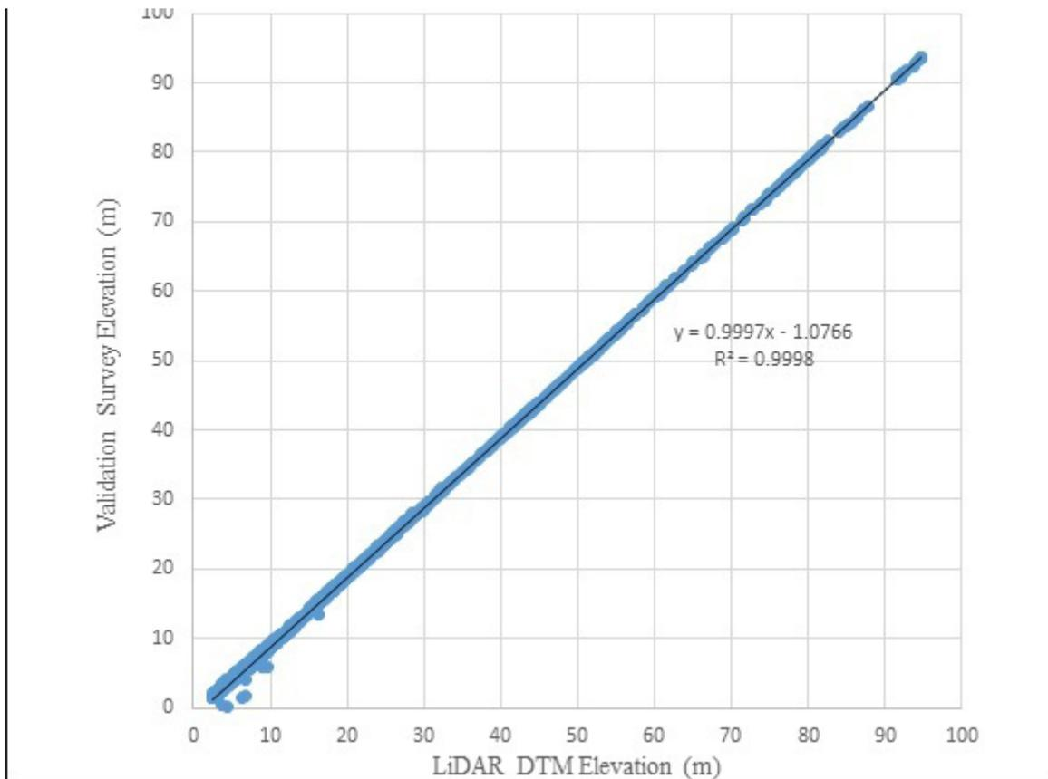
Figure 28. Correlation plot between the validation survey points and the LiDAR data.
