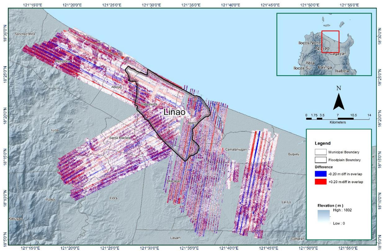
Figure 17. Elevation difference map between flight lines for Linao floodplain.
