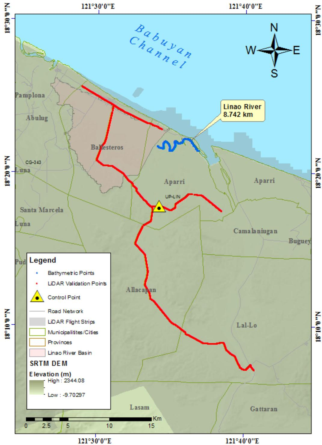
Figure 46. Extent of the LiDAR ground validation survey of the Linao River Basin
