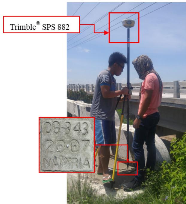
Figure 35. GNSS receiver set-up, Trimble® SPS 882, at CG-343, located at the approach of the Lukban Bridge in Barangay Libertad, Municipality of Abulug, Cagayan
