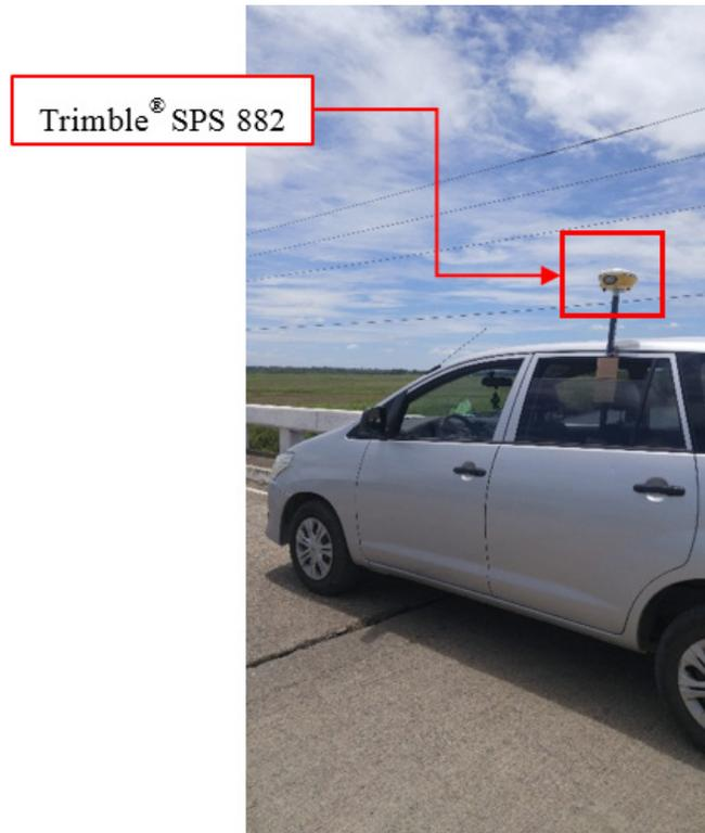
Figure 45. Validation points acquisition survey set-up along the Linao River Basin
