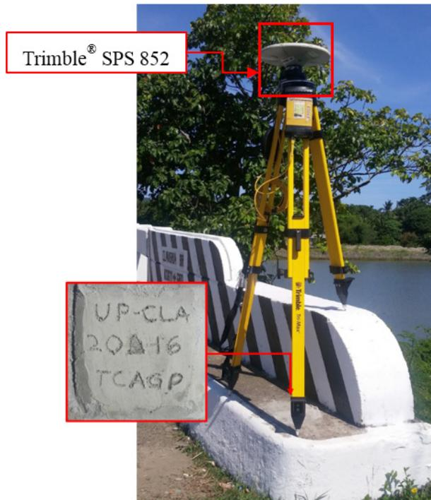
Figure 37. GNSS receiver set-up, Trimble® SPS 852, at UP-CLA, located at the approach of Cabicungan Bridge in Barangay Dibalio, Municipality of Claveria, Cagayan
