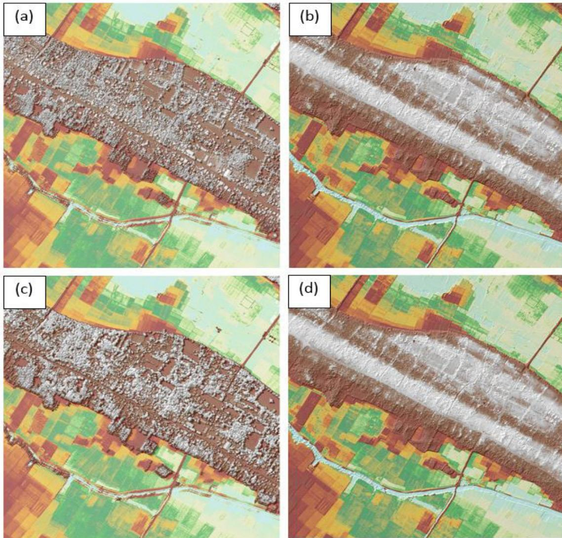
Figure 21. The production of last return DSM (a) and DTM (b), first return DSM (c) and secondary DTM (d) in some portion of the Linao floodplain
