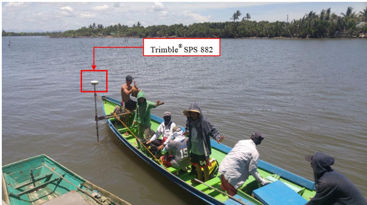
Figure 47. Bathymetric survey using Ohmex™ single beam echo sounder in Linao River
