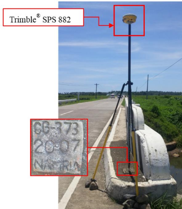
Figure 36. GNSS receiver set-up, Trimble® SPS 882, at CG-373, located at the approach of the Bangan Bridge in Barangay Bangan, Municipality of Sanchez Mira, Cagayan
