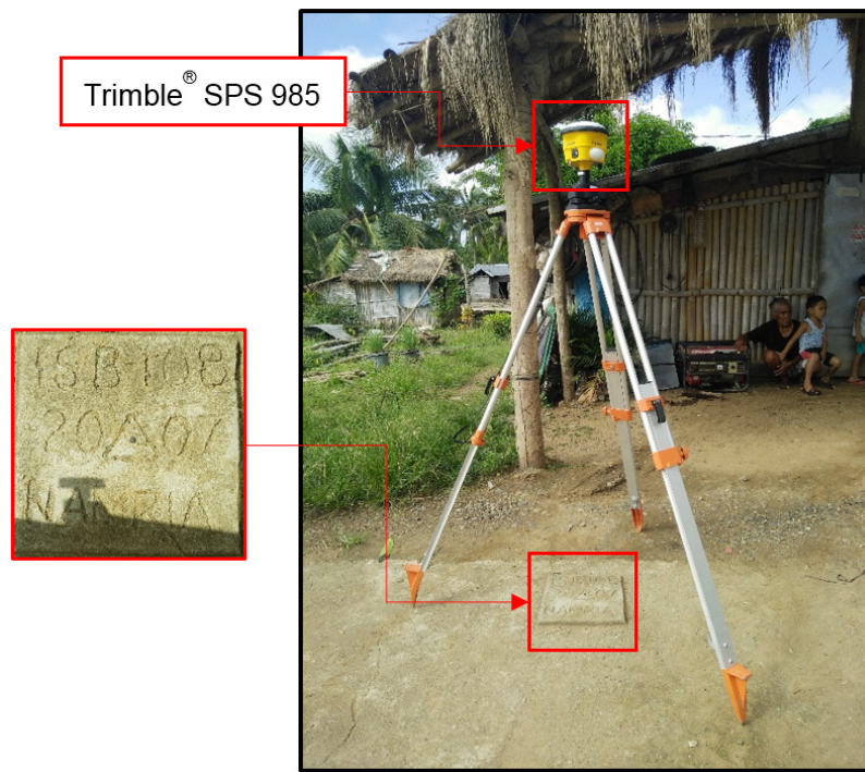
Figure 45. GNSS receiver set up, Trimble® SPS 985, at ISB-108, located at the corner of a basketball court in Brgy. San Juan, Ilagan, Isabela.
