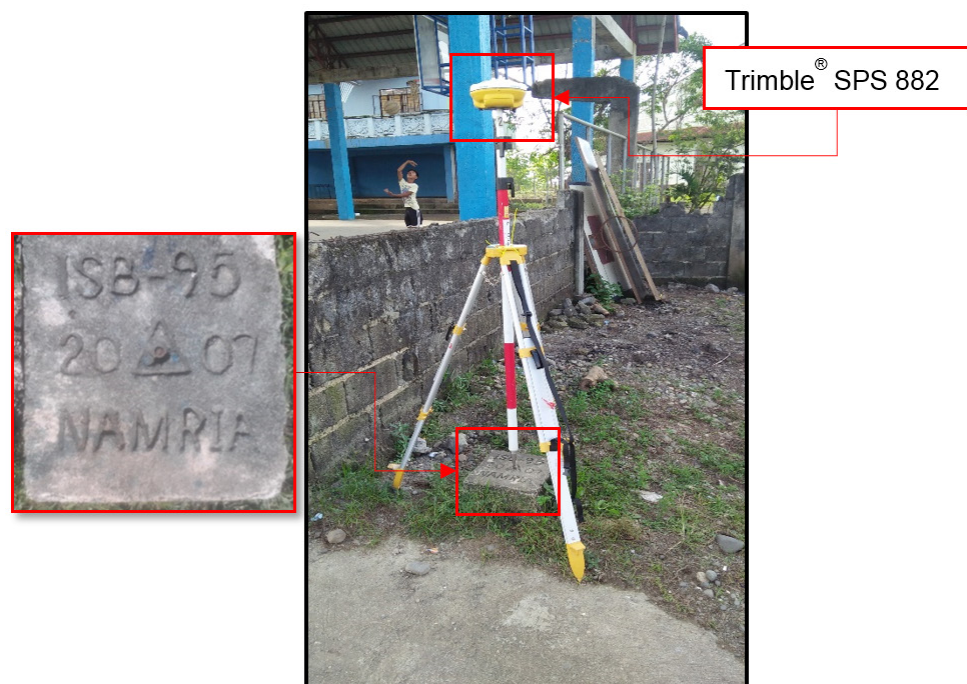
Figure 44. GNSS receiver set up, Trimble® SPS 882, at ISB-95, located behind a basketball court in Brgy. Morado, Ilagan, Isabela.
