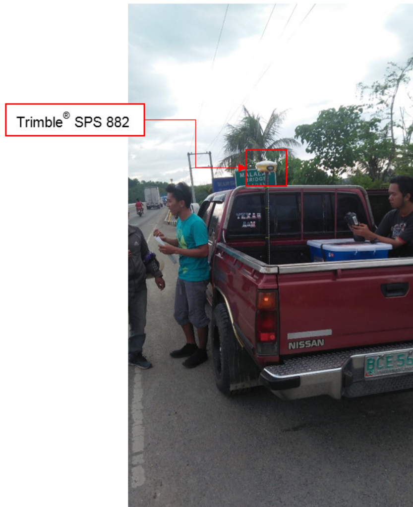
Figure 55. GNSS Receiver Trimble® SPS 882 installed on a vehicle for Ground Validation Survey.
