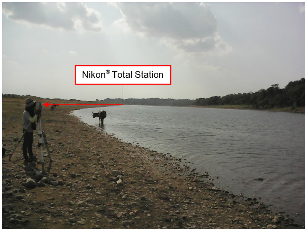
Figure 57. Set-up for the manual bathymetric survey of ABSD along Pinacanauan de Ilagan River.
