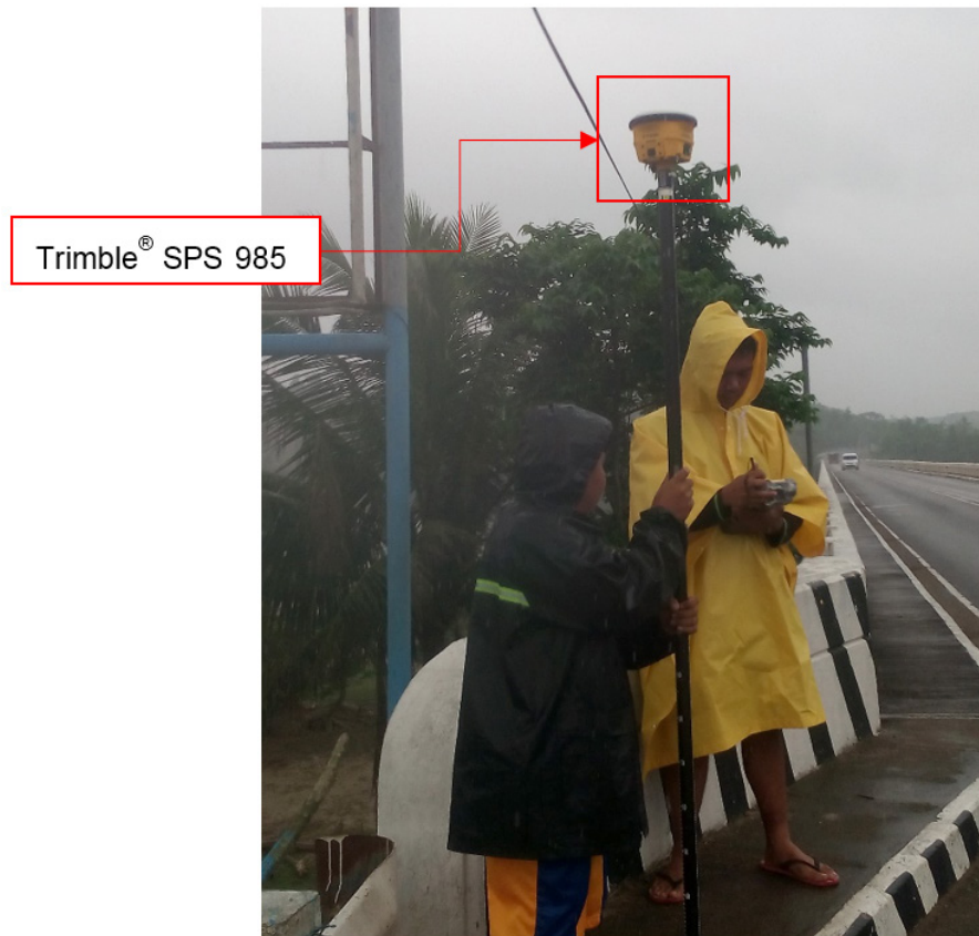
Figure 50. Gathering of random cross-section points along Malalam Bridge.
