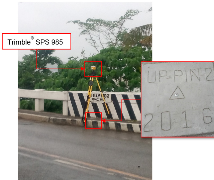
Figure 47. GNSS receiver set-up, Trimble® SPS 985, at UP_PIN-2, an established control point, located at the approach of Malalam Bridge in Brgy. Alliguigan 2 nd , Ilagan, Isabela.
