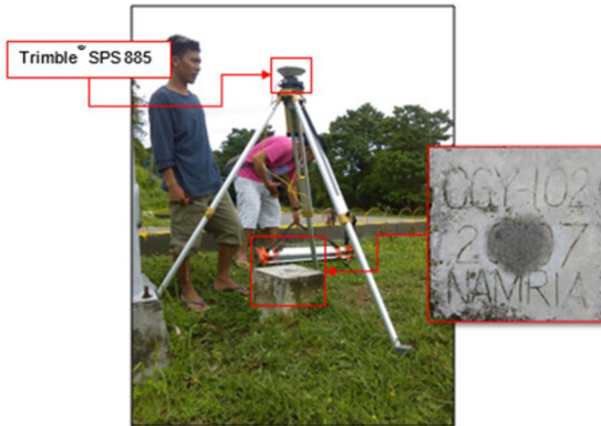
Figure 27. GNSS receiver set-up, Trimble® SPS 885, at CGY-102, located at the center island in front of the barangay marker of Brgy. Casambalangan in Brgy. San Jose, Gonzaga, Cagayan
