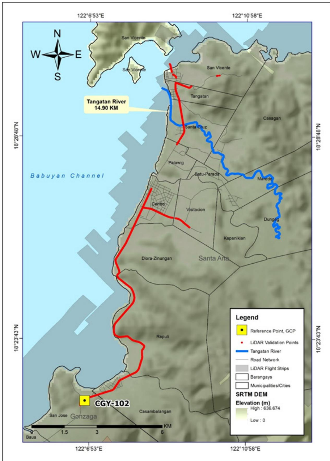
Figure 44. Validation points acquisition survey coverage for Tangatan River Basin
