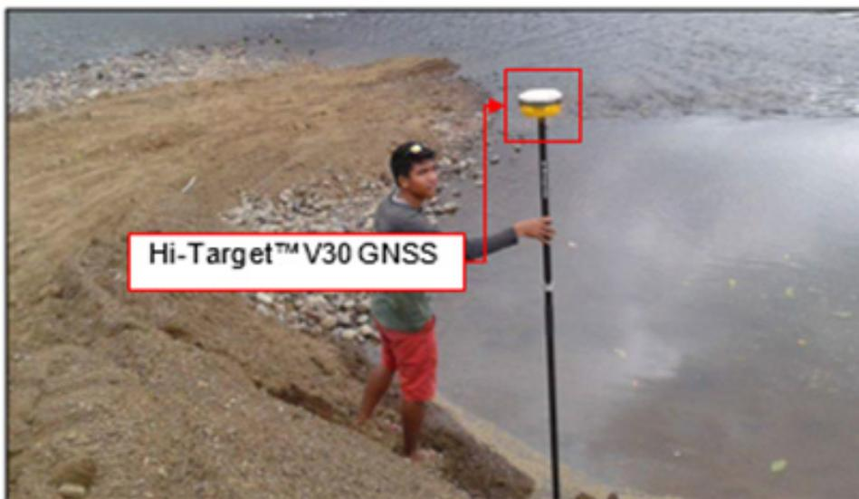
Figure 46. Manual bathymetric survey of HONS along Tangatan River
