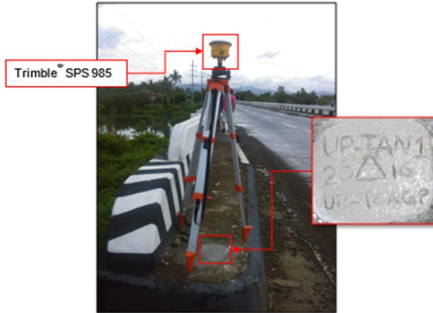
Figure 29. GNSS receiver set-up, Trimble® SPS 985, at UP-TAN-1, located at the approach of Sta. Cruz Bridge in Brgy. Sta. Cruz, Sta. Ana, Cagayan
