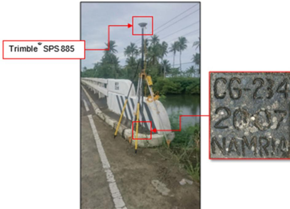
Figure 28. GNSS receiver set-up, Trimble® SPS 885, at CG-234, located at the approach of Diora Bridge in Brgy. Diora-Zinungan, Sta. Ana, Cagayan
