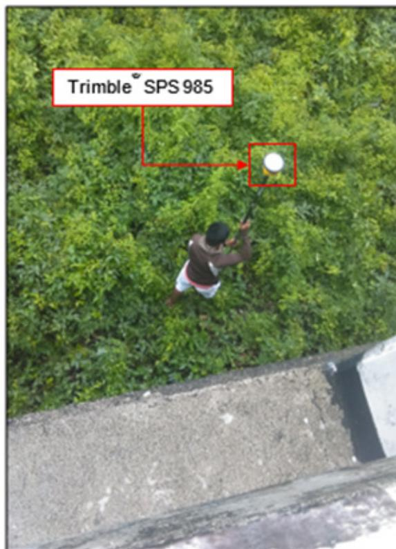
Figure 40. Gathering of random cross-section points along Sta. Cruz Bridge
